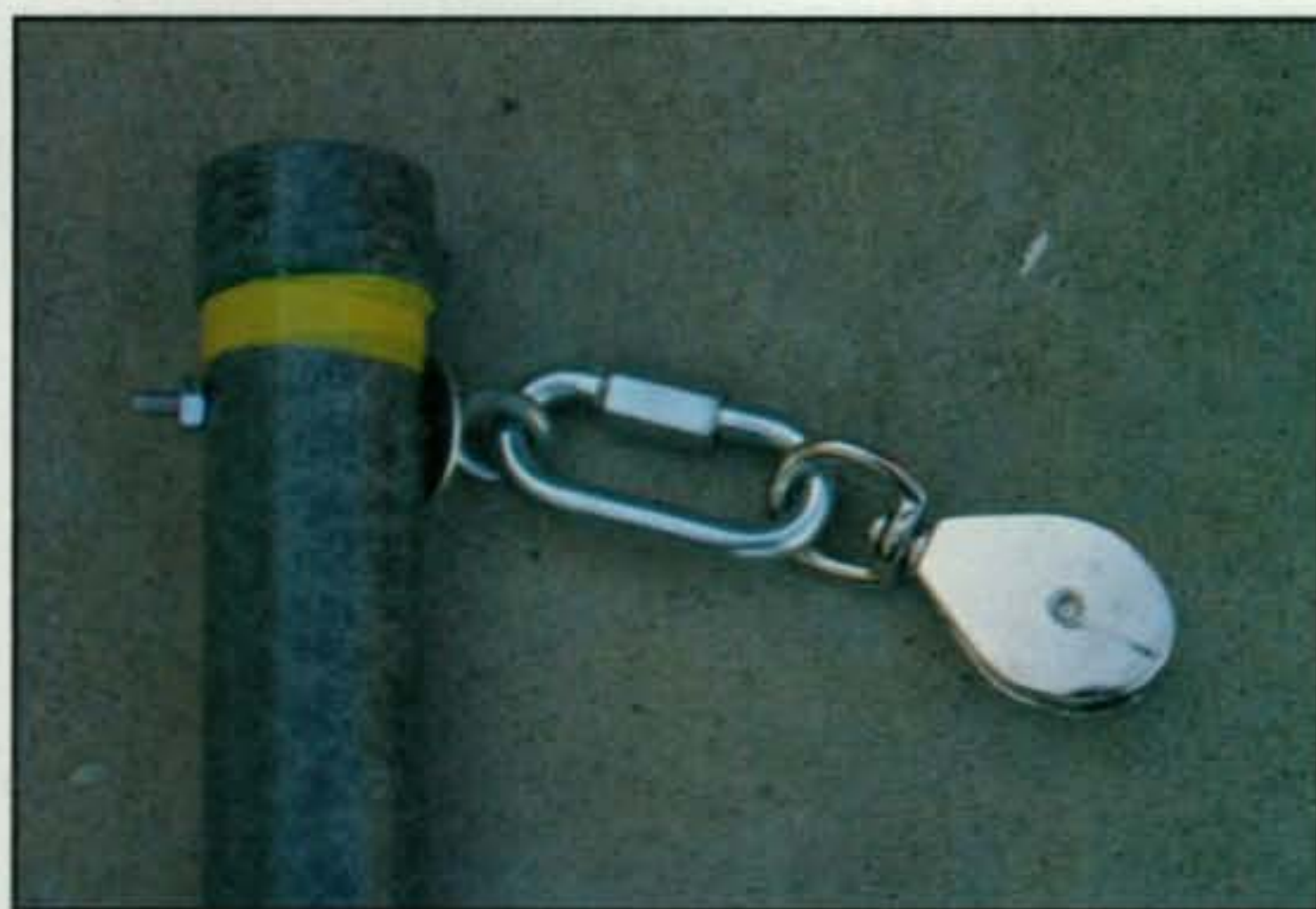
Photo 6— Here is one way to attach a pulley to a mast. Drill a hole through the mast, insert a long eye-bolt, and use a link to secure the pulley to the eye-bolt.
