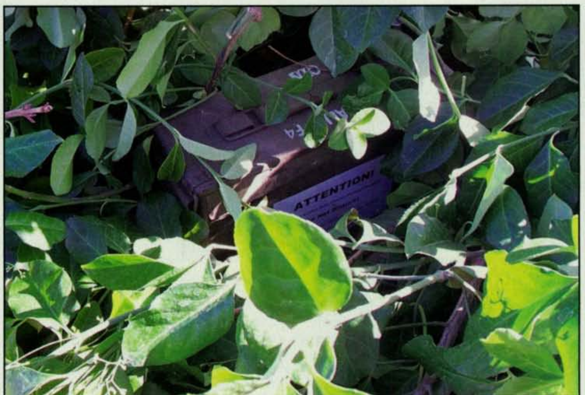
Surplus steel ammunition boxes are popular weatherproof containers for remote-controlled 2-meter transmitters. Be sure to label the box with your name and contact information to keep citizens from reporting a suspicious object to the authorities. (Photo by Randy Holland, KO6KC of Las Vegas, Nevada from Foxhunt Weekend 2004)
