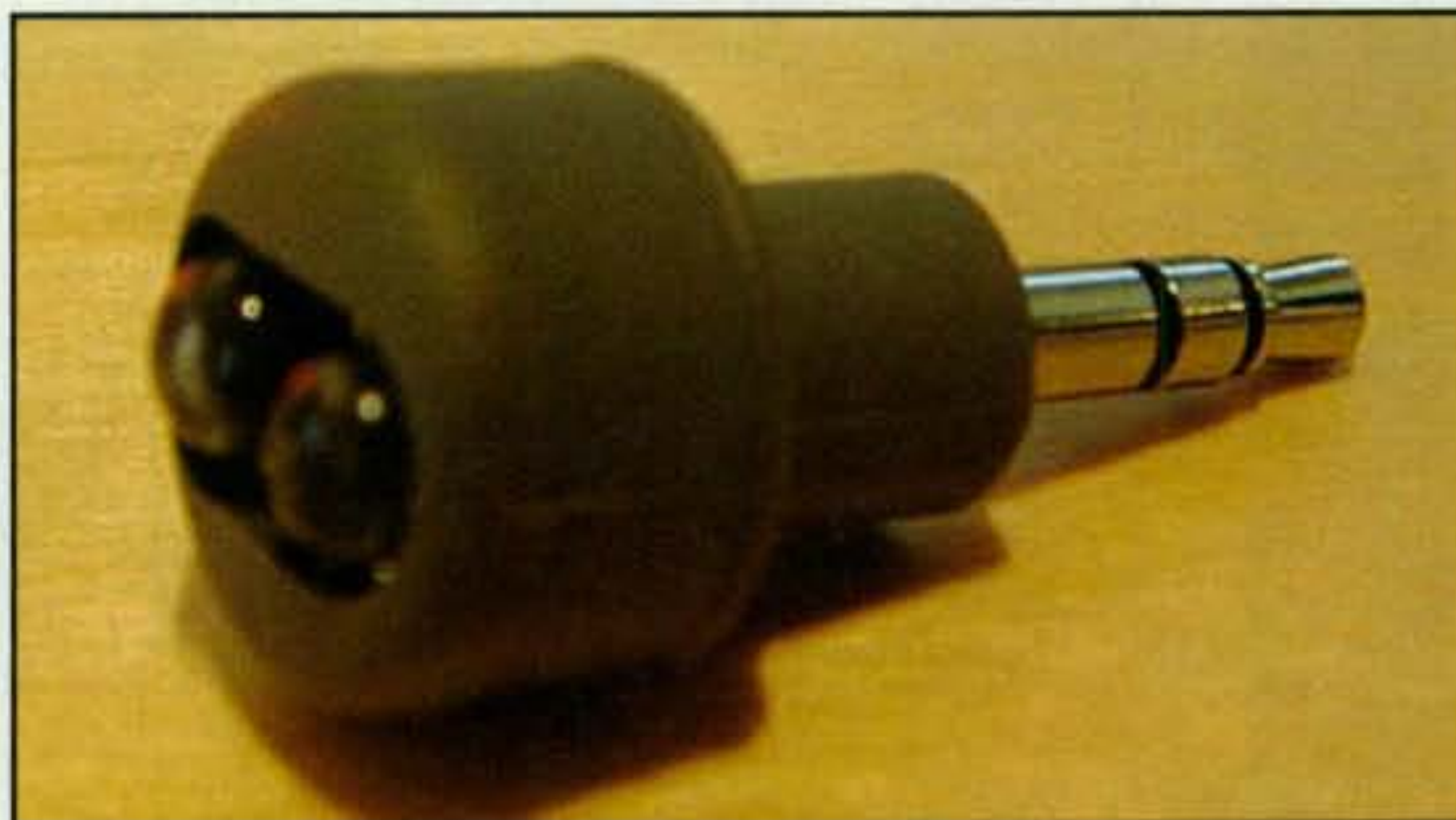
Fig. 1— A key component of the system is the sound-to-IR converter. This is an early model produced by Griffin. Some readers even may want to build their own converter. (See the discussions in note 2.)
