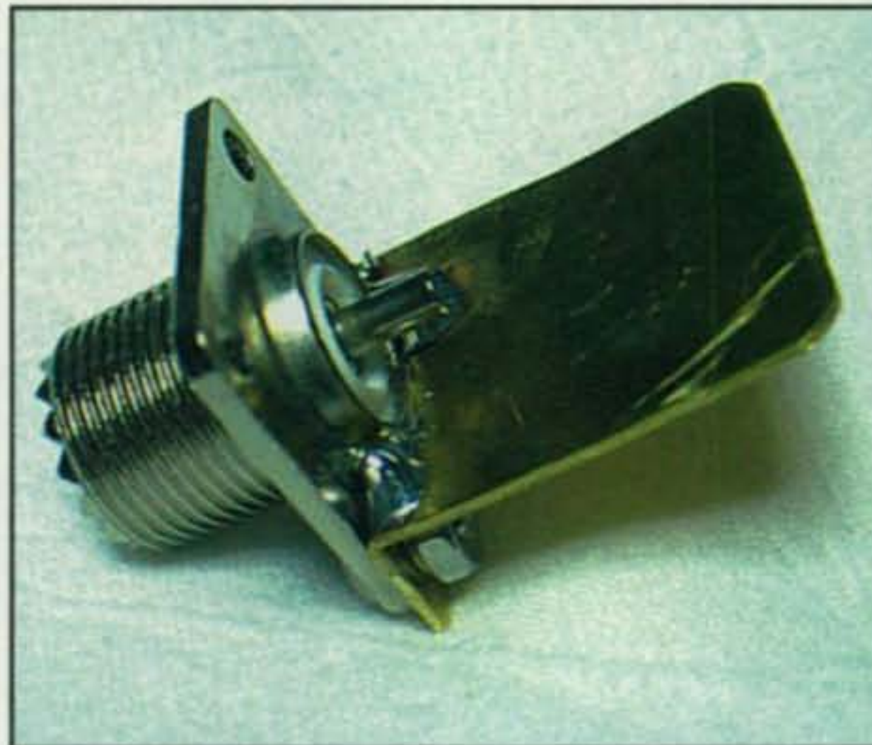
Photo A—The brass plate mounted and soldered in place.
