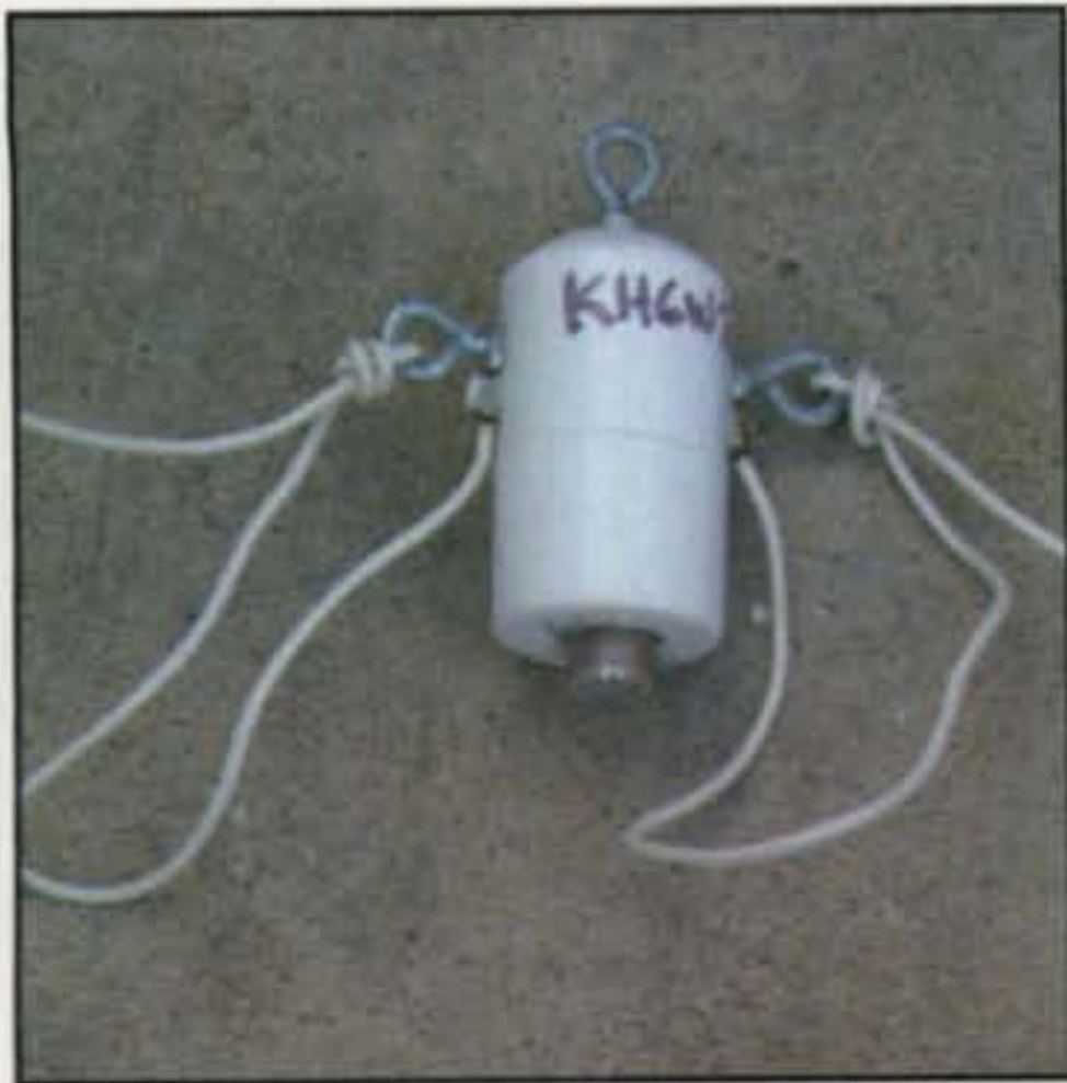
Photo 2— The store-bought center insulator includes an SO-239 coax connector and terminals for the antenna wire elements. The screw-eyes are used to mechanically secure the wire elements to the center insulator unit and remove the pulling force from the electrical connection.
