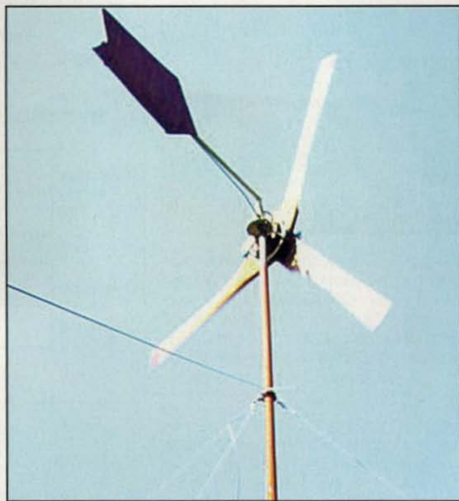
Photo C— This 10-foot wind turbine produced by Dan Bartmann, KC0VSV, of < www.otherpower.com > produces up to 700 watts in a 20–25 mph wind and doesn't require fueling for operation. It's a good source of alternate energy and it is also an excellent way to back up a solar-power system. E-mail < Danb@otherpower.com > for more information.
