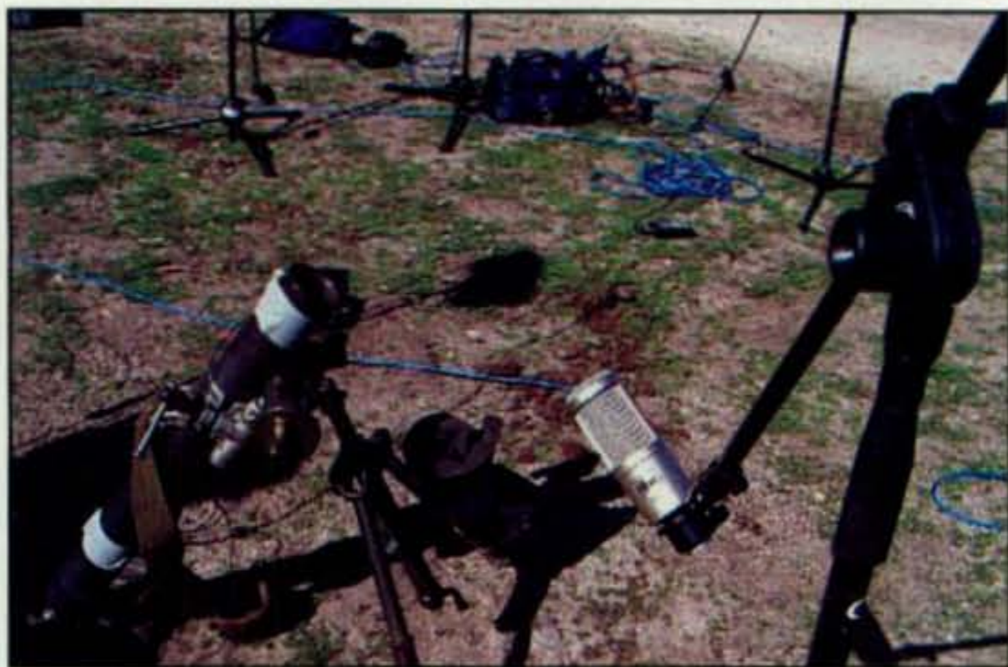
Photo G— The sounds of the cannons and guns in the powerful World War II epic movie Flags of our Fathers were captured by the new technology of several Heil PR 40 dynamic mics on the movie set. (Photo courtesy of Heil Sound)
