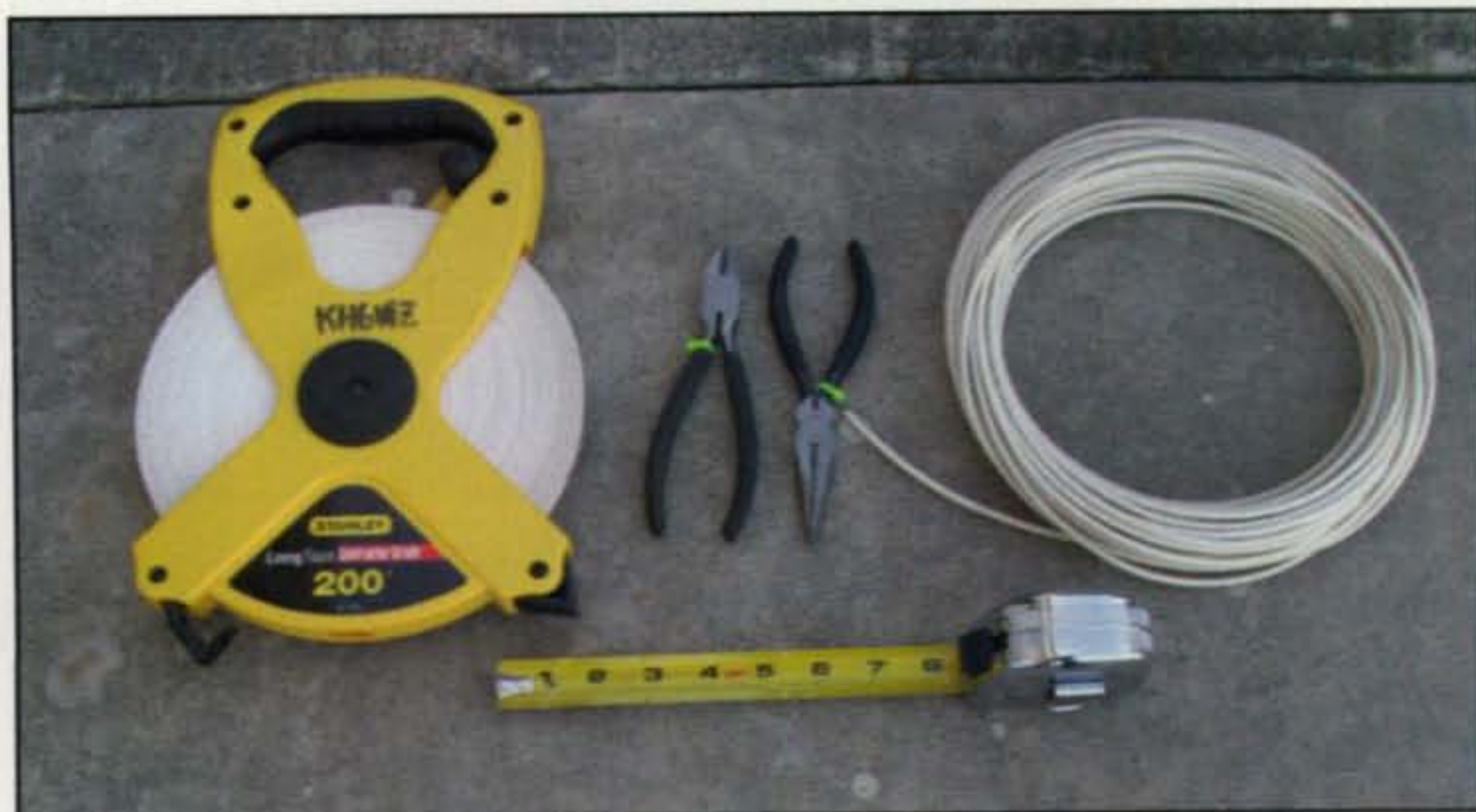
Photo 3— Here are some of the materials and tools needed to build wire antennas. The "extra long" tape measure is very handy when using long runs of wire.
