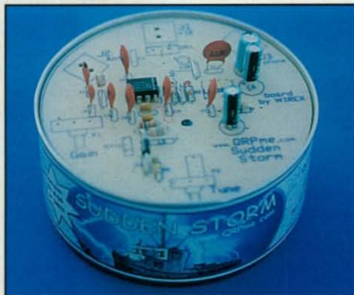
Photo B— The Sudden Storm goes together so quickly that pausing to shoot this photo midway during assembly was the most time-consuming step. There are no off-board components to wire, no toroids to wind, and performance is quite good for a two-IC receiver.
