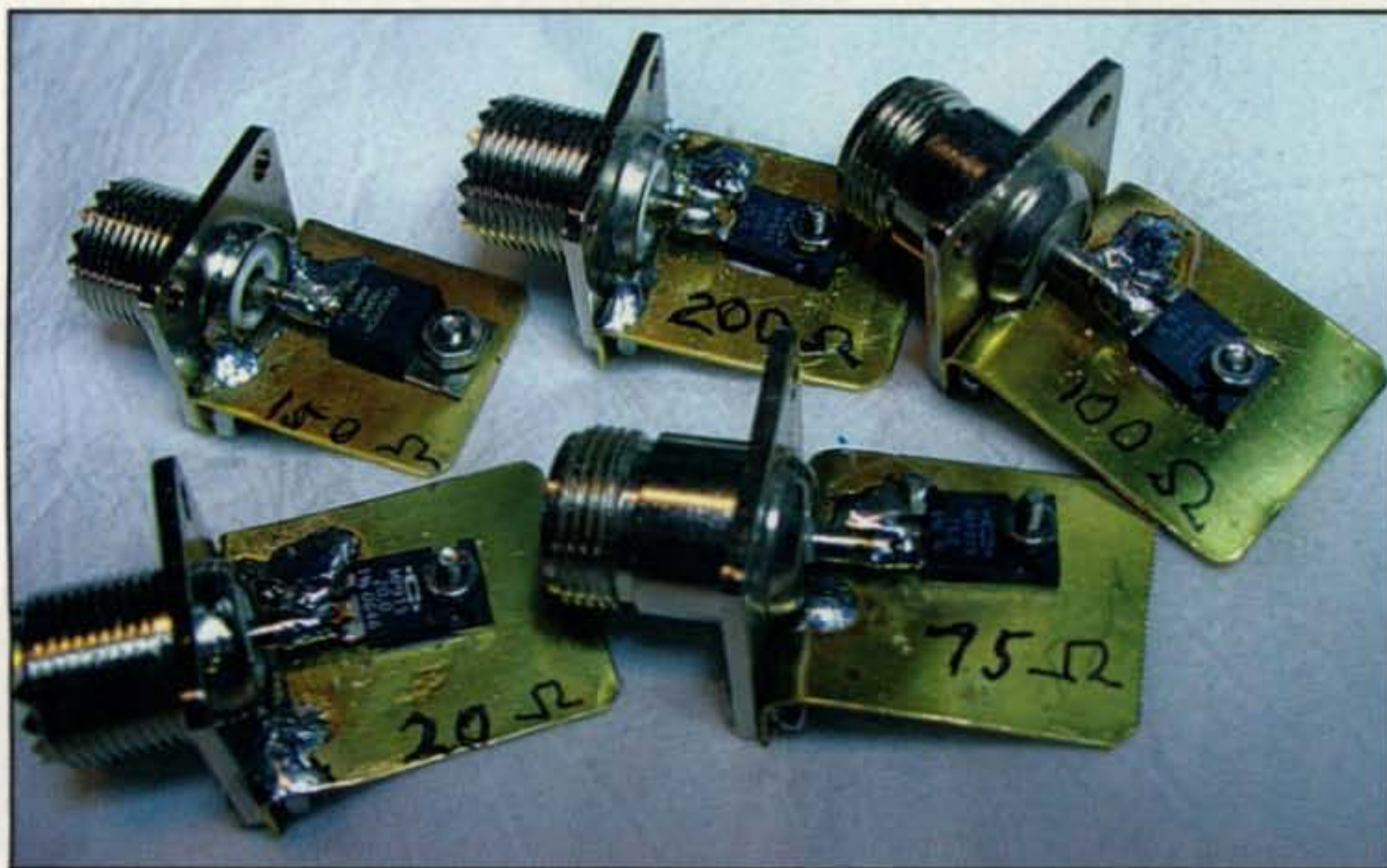
Photo B— The assembled precision loads using both SO-239 and N connectors.
