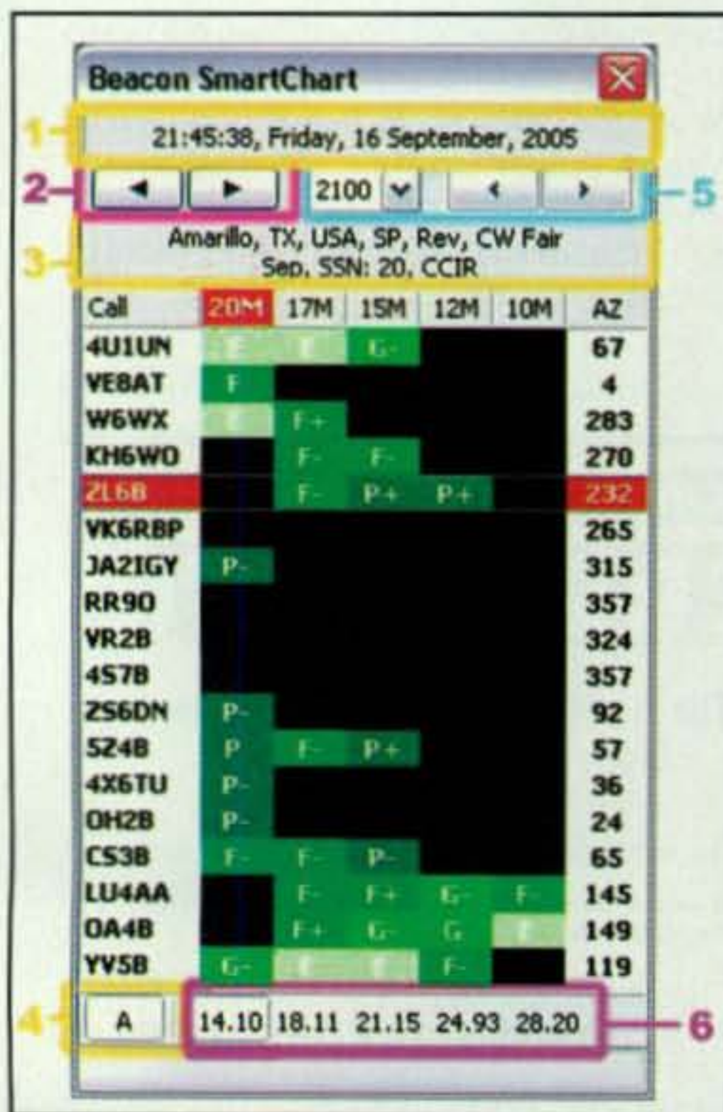
Fig. 1—WinCAP Wizard 5 represents the latest generation of the popular Taborsoft HF propagation prediction engine interface. The “Beacon SmartChart” depicted here is a new and innovative view of the associated VOACAP prediction data. You’ll find details and contact information in this month’s column. (Image from the Taborsoft website)
