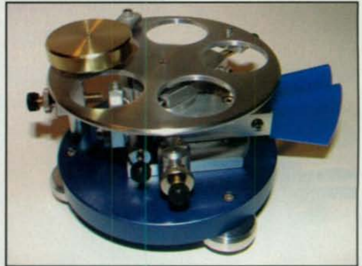
Photo 1—Left-side view of the incredible RotoBug designed and made by Richard Meiss, WB9LPU. Three-tier design consists of a 3-inch diameter steel base, aluminum center mechanism, and top-mounted rotor that oscillates back and forth within a magnetic field to produce dots. Speed is adjusted by the arm with the weight near the rim of the rotor. (Photo by WB9LPU)
