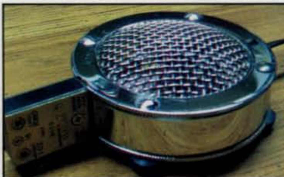
Photo 4— This eye-catching gem is an iambic touch paddle Doug Fabian, N8EPE, built around a pre-assembled PC board from <www.cwtouchkeyer.com> and installed in a D-104 microphone head. The attached FT-243 crystal case with metal plates on both sides serves as the fingerpieces. Suggestions for quick-brewing a similar paddle are in the text.
