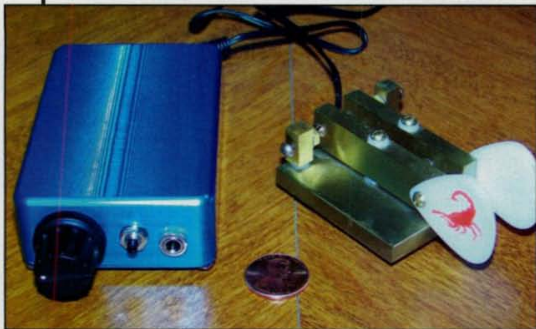
Photo A—Paul Huff, N8XMS, uses this pocket-size setup for casual QRP fun, and has contacted 17 states with it on a strictly spare-time basis. The Rock Mite mini transceiver kit can be obtained from < www.smallwonderlabs.com >. The "Mite box" is available from < www.americanmorse.com >, and the paddle (also a kit) was offered by the Arizona SQRPIon QRP Club. Total class for sure! (Photo via N8XMS)
