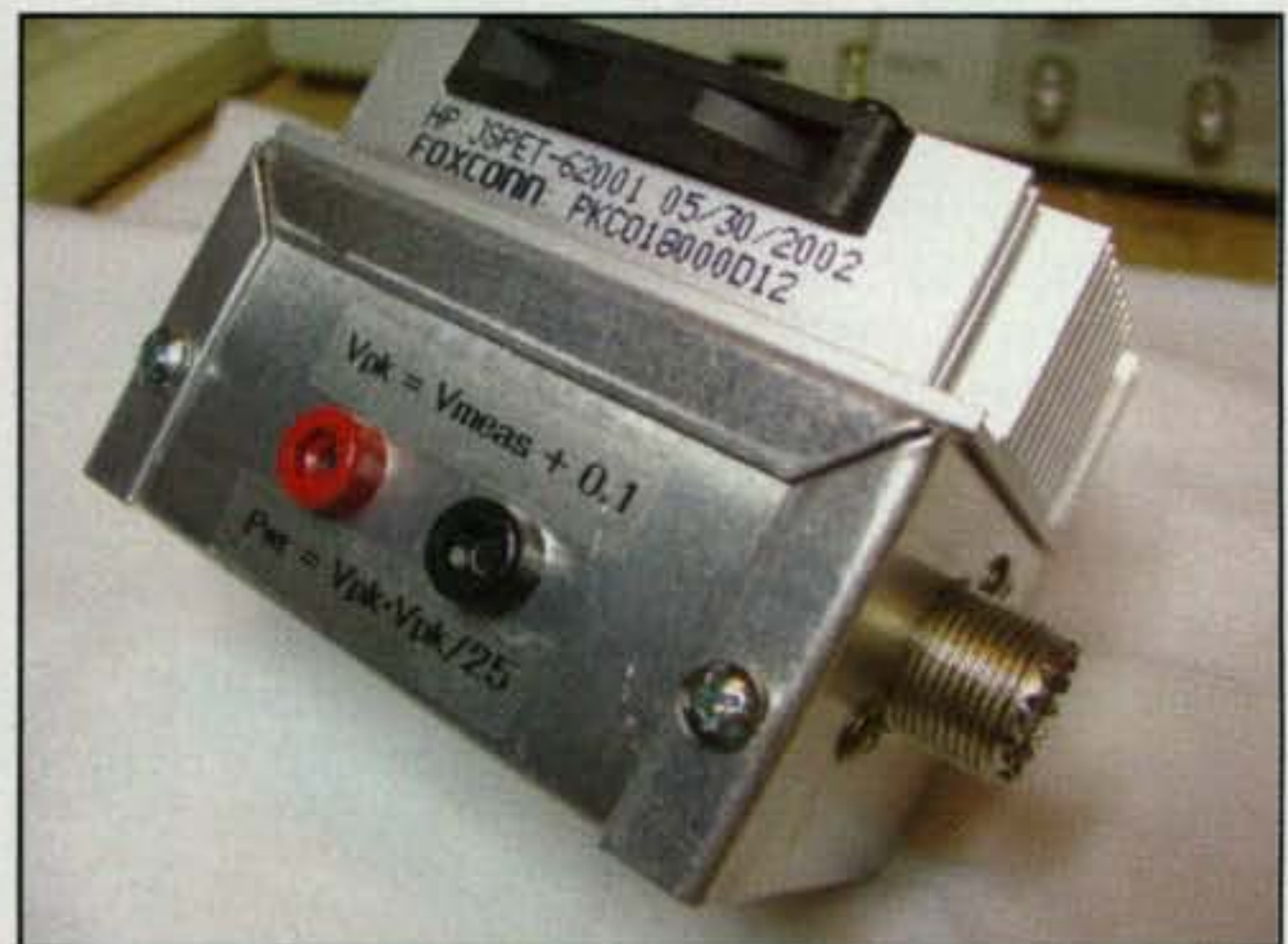
Photo C— Final 200-watt dummy load/peak detector view showing the detector connectors and UHF connector.
