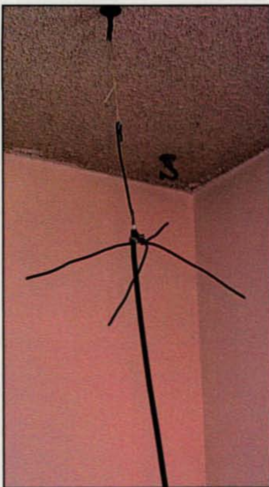
Photo 2— The "ugly ground-plane antenna" might not look pretty, but it is also an effective and small antenna for VHF-FM work, curing scratchy and noisy signals.
