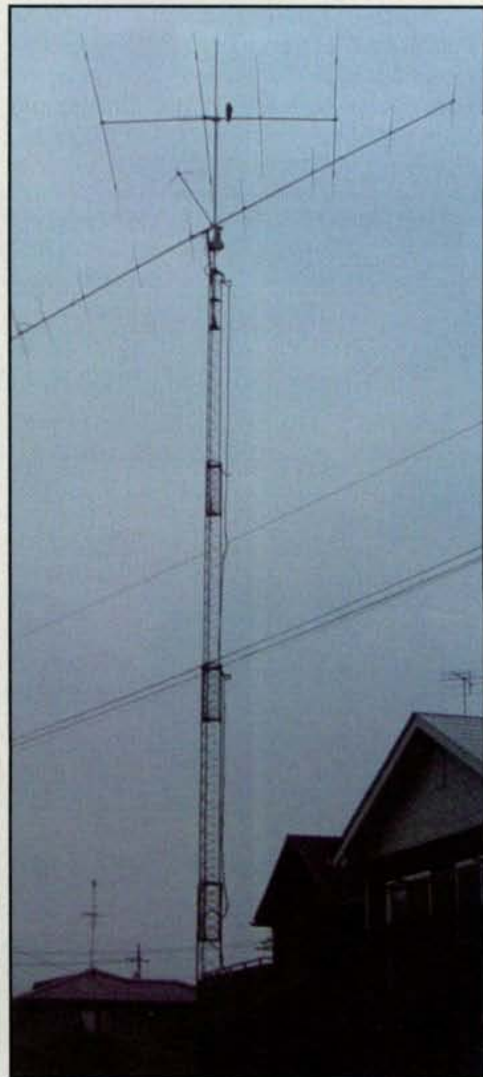
Photos A & B—JM1DTF's 10-element, long-boom 6-meter Yagi at a “standard” 0-degree elevation in photo A (left) and rotated up to a 30-degree elevation in photo B (right).
