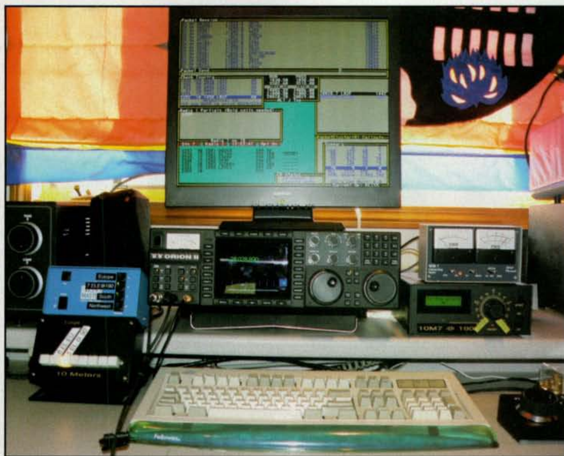
Photo C— The Orion II at the KC1XX 10-meter operating position. The switch-boxes to the left of the keyboard select various transmit antennas. The window behind the radio is oriented to highlight sunrise, normally indicating that 10 is about to come alive. (Photo courtesy of K1GQ)
