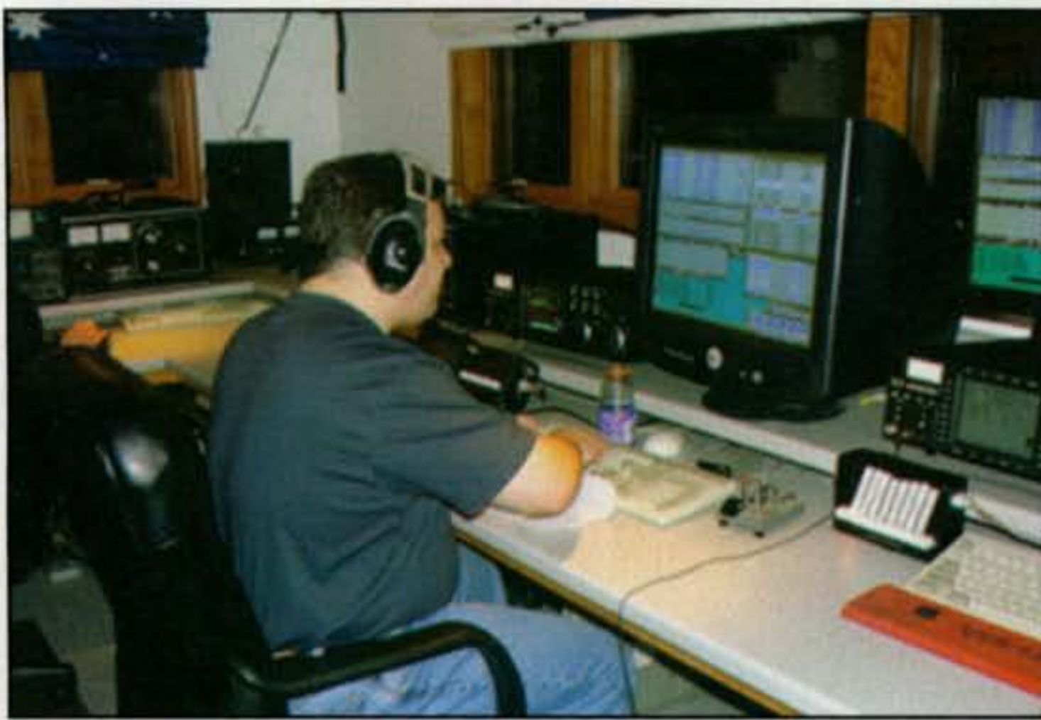
Photo B— Bob Raymond, WA1Z, operating the Orion II at KC1XX in the 2007 CQ 160 Meter CW contest. The spotting position is to his right, and the second transmit position to his left, operated by John Kaufmann, W1FV. The two beady red eyes atop the amplifier to Bob's left are indicators on the transmit interlock switch. (Photo courtesy of K1GQ)
