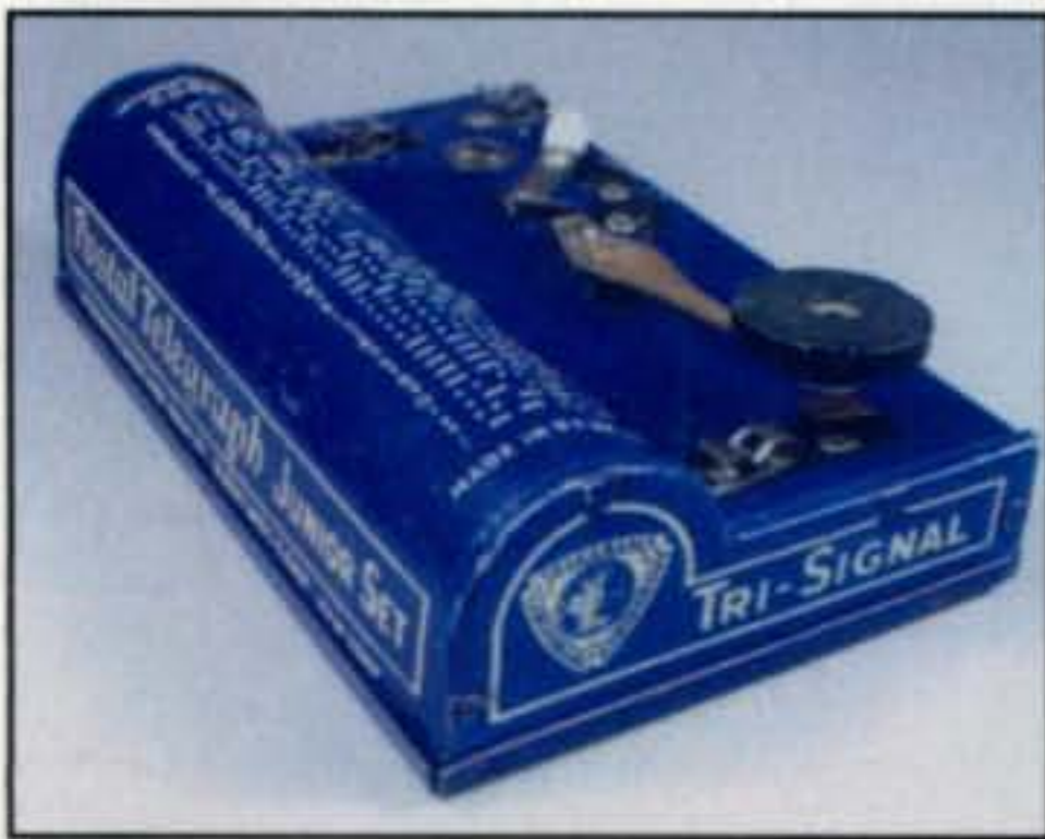
Photo 14—Roaring back from the 1950s is this exceptionally well-preserved Tri-Signal Telegraph Practice Set owned and operated—err . . . photographed—by James H. Richards (an attorney with an appreciation for the finer things in life, such as telegraphy). The set was manufactured by L. K. Elkay Mfg. Corp. NY and uses a buzzer or pilot light for operation. (Details in text.)
