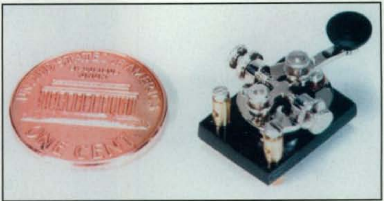
Photo 10— This is an honest-to-goodness working hand key the size of a penny. It is called the Nanokey and is made by noted clock maker W. R. Smith, W4PAL. It is complete with knurled thumbscrews and nuts for gap and tension adjustments, silver contacts with insulating washers, and a tiny plastic knob. It is amazing! (Photo courtesy of W4PAL)
