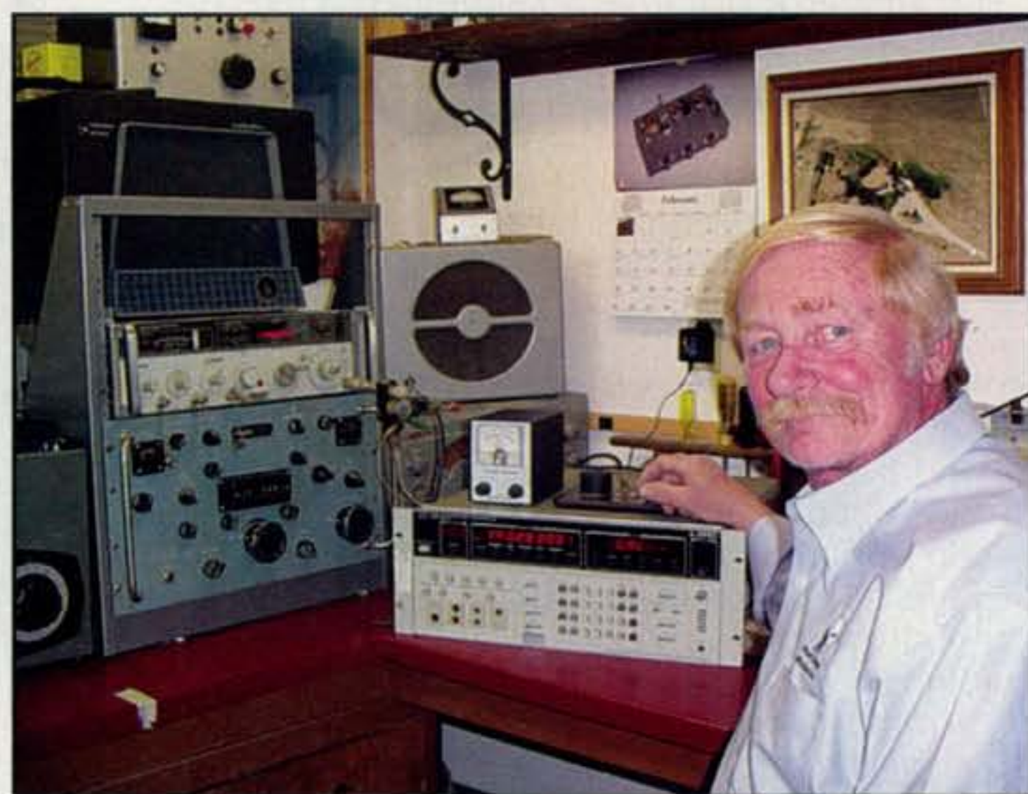
Photo D— Keith Ericson, KØKE, with his workbench test equipment used for milliwatt fun on 20 and 15 meters. The receiver is an HP-3746A Frequency Selective Level Meter and the transmitter is an HP-8640B keyed through a Dow Key T/R relay on its output. It's wild, but Keith worked VK9NDX—with a scant 200 mw output! (Photo courtesy of KØKE)
