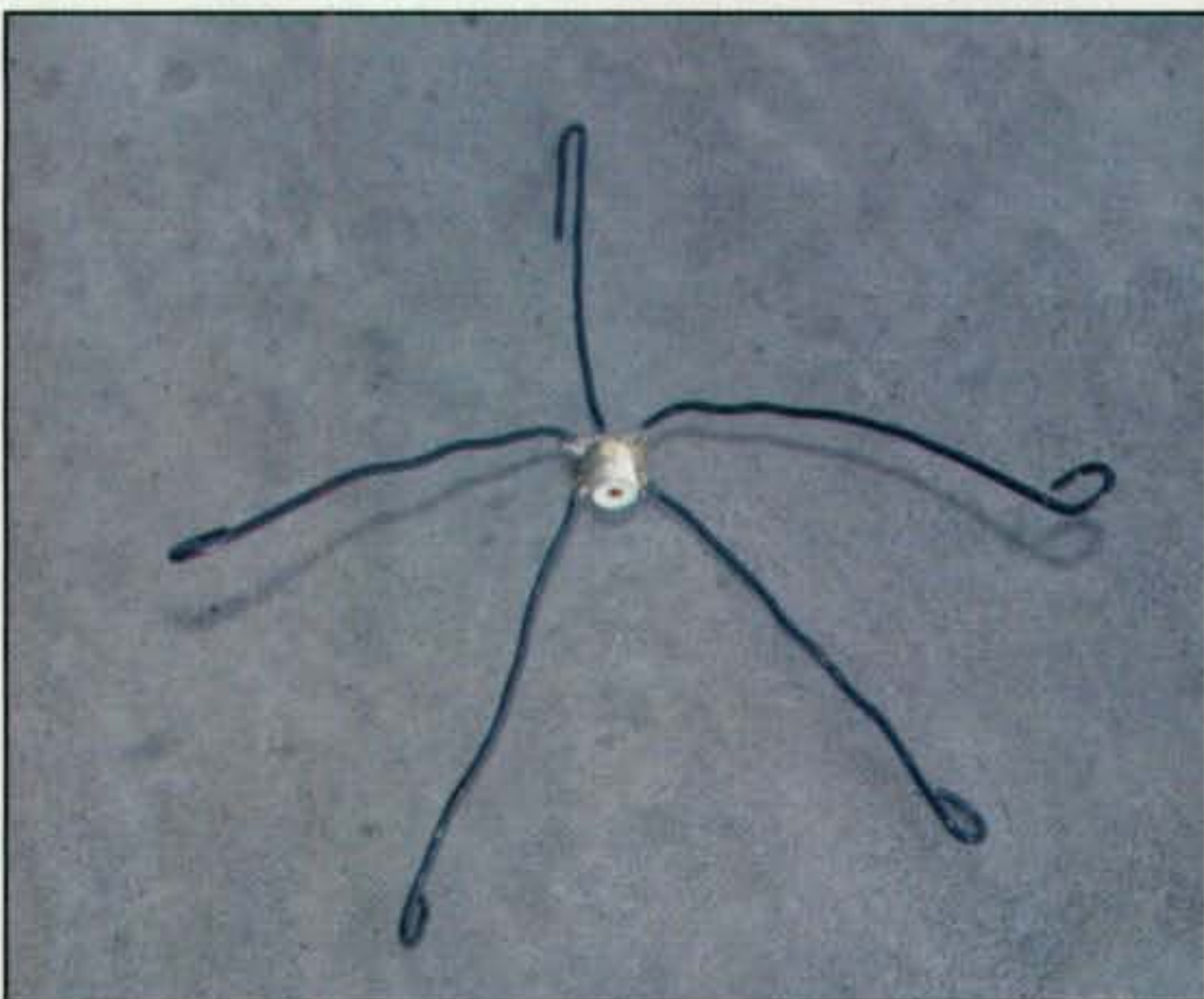
Photo 4— This is another view of the antenna. Remember, it is better to cut the wires a little long, since it is easier to trim the lengths to the proper length after the assembly is completed.
