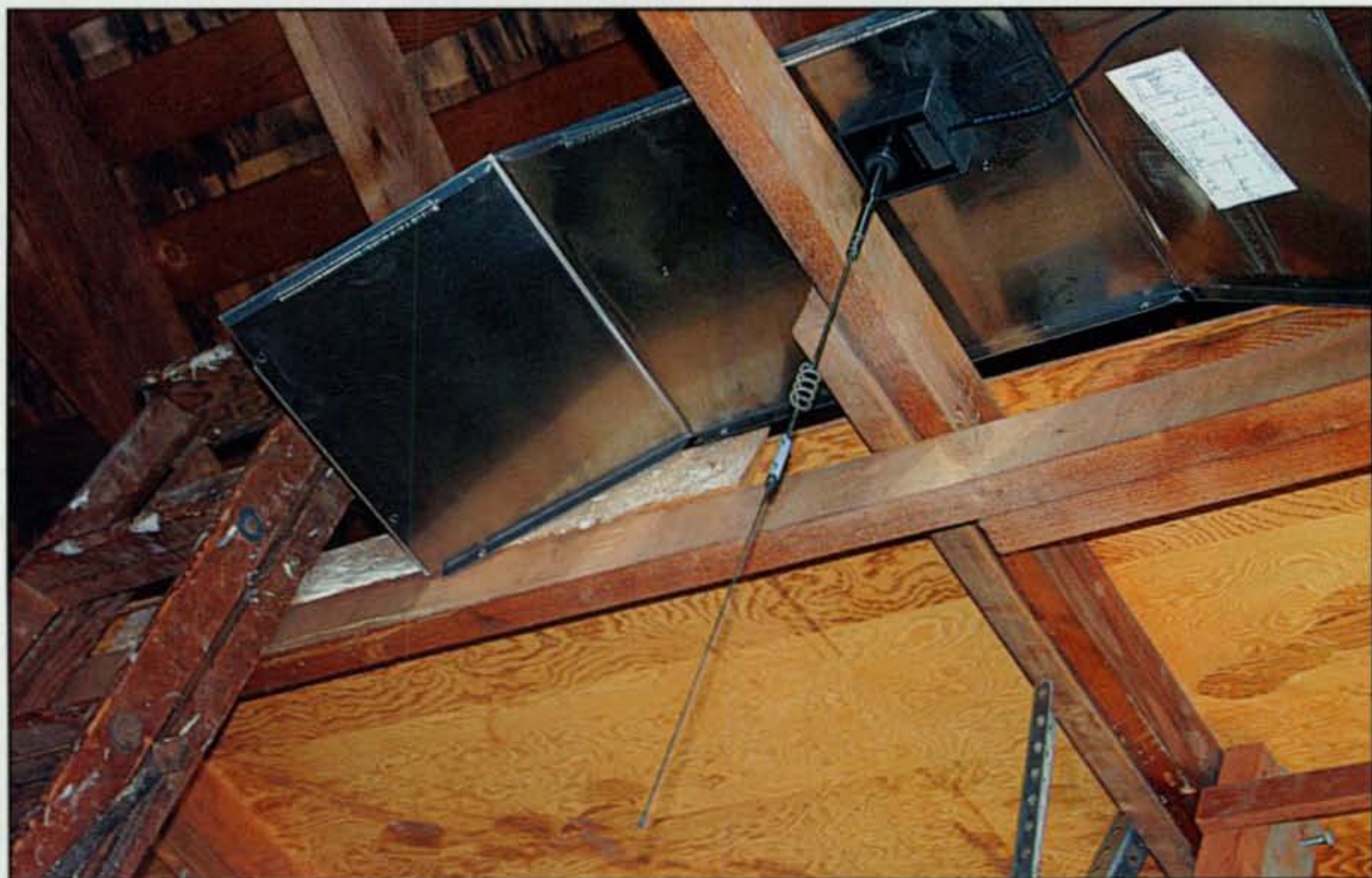
Photo 1— The simple, cheap, and portable dual-band antenna system is effective and easy to install. But wait . . . the antenna is upside-down. See the text for more details.
