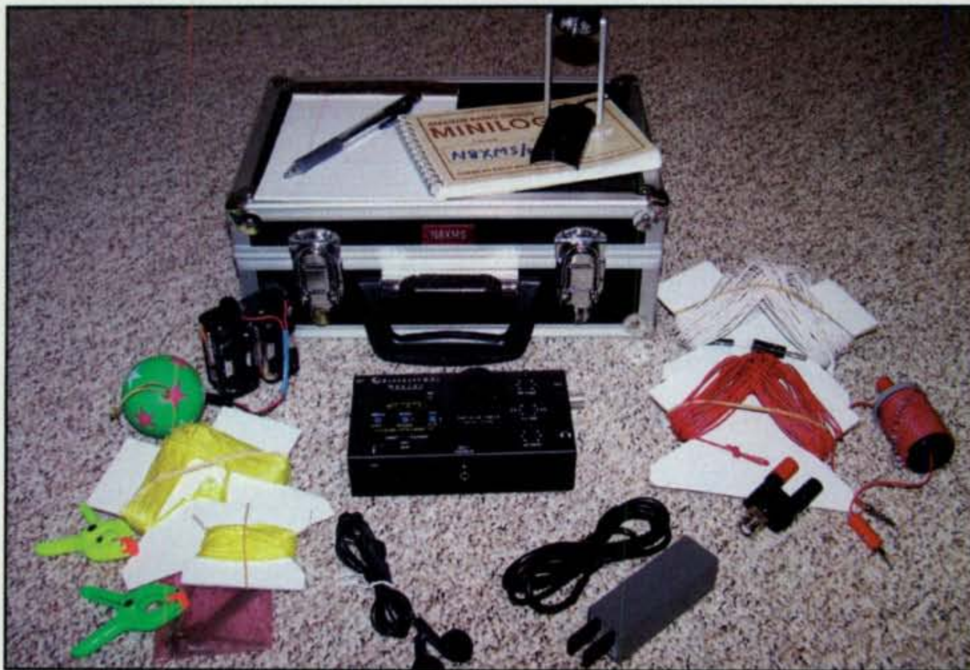
Photo B— This tiny “grab-and-go” QRP setup, also built by N8XMS, has it all! The Elecraft KX-1 transceiver is equipped with an automatic antenna tuner and SWR monitor and may be powered by internal batteries or an external battery pack. The roll-up 42-ft. long wire antenna and ground radial system are designed for easy deployment using a rubber ball. The banana adapter is handy for quickly connecting antenna wires to the BNC socket on the KX-1. (Photo via N8XMS)
