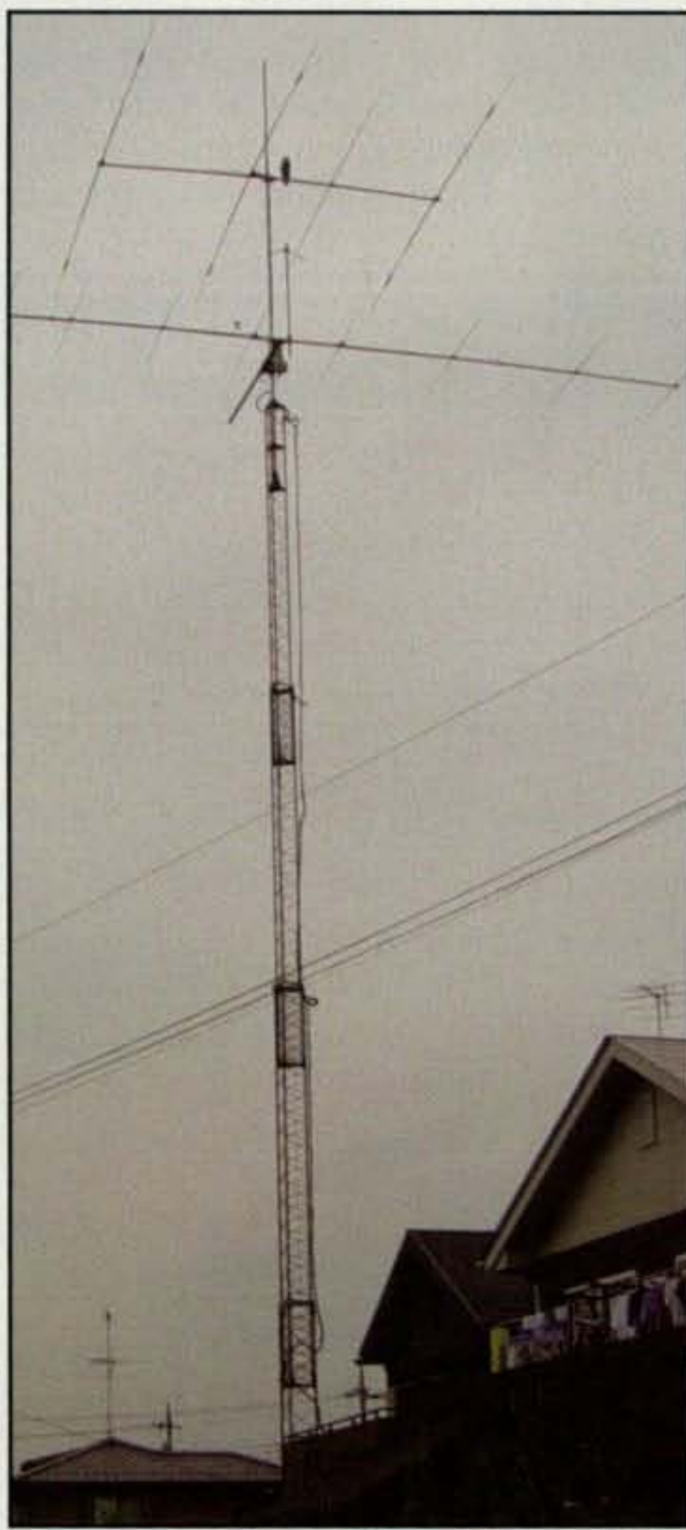
Photos A & B—JM1DTF's 10-element, long-boom 6-meter Yagi at a “standard” 0-degree elevation in photo A (left) and rotated up to a 30-degree elevation in photo B (right).
