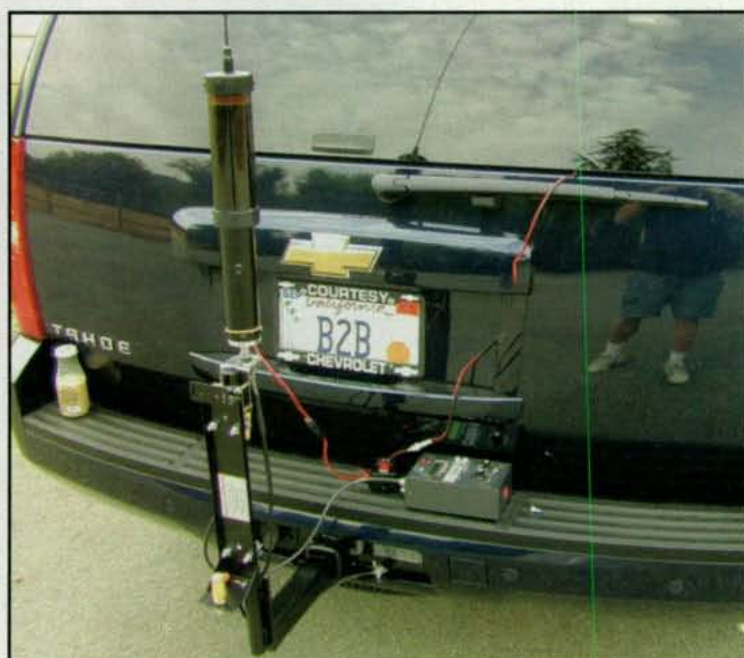
Photo G— A High Sierra 1800 screwdriver mobile antenna is rather large and heavy, so Rick had this special mount custom-made for securing it "trailer hitch style" to his GMC Tahoe. It also includes a standard 3/8-24 base fitting for accepting standard mobile whips.
