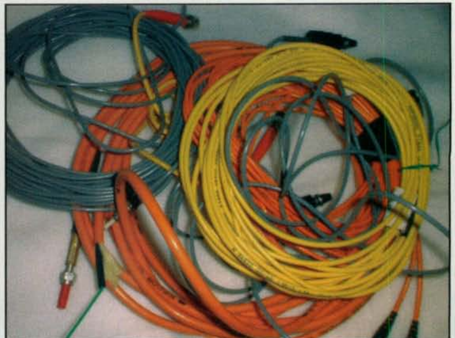
Photo G— Using surplus fiber-optic cable as guy wires.
