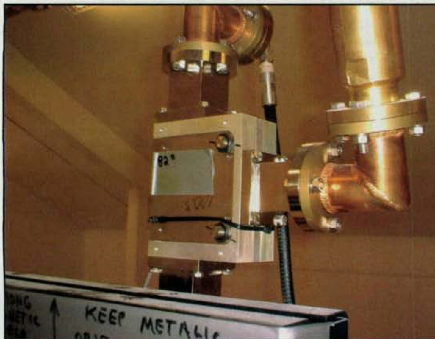
Photo F— High-power 100.3-MHz ferrite circulator.
