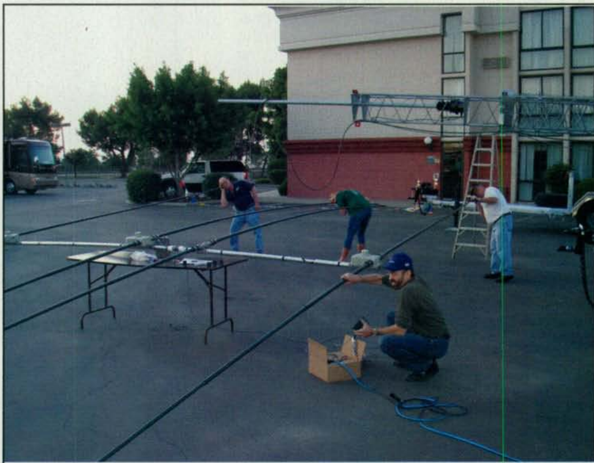
Can you hear me now? At the International DX Convention in Visalia this past May the crew from SteppIR listens for movement of antenna elements while owner Mike Mertel, K7IR, tests the motors of the three-element SteppIR Yagi with a 30-40 meter dipole outside the convention hotel. (Photo by W2VU)
