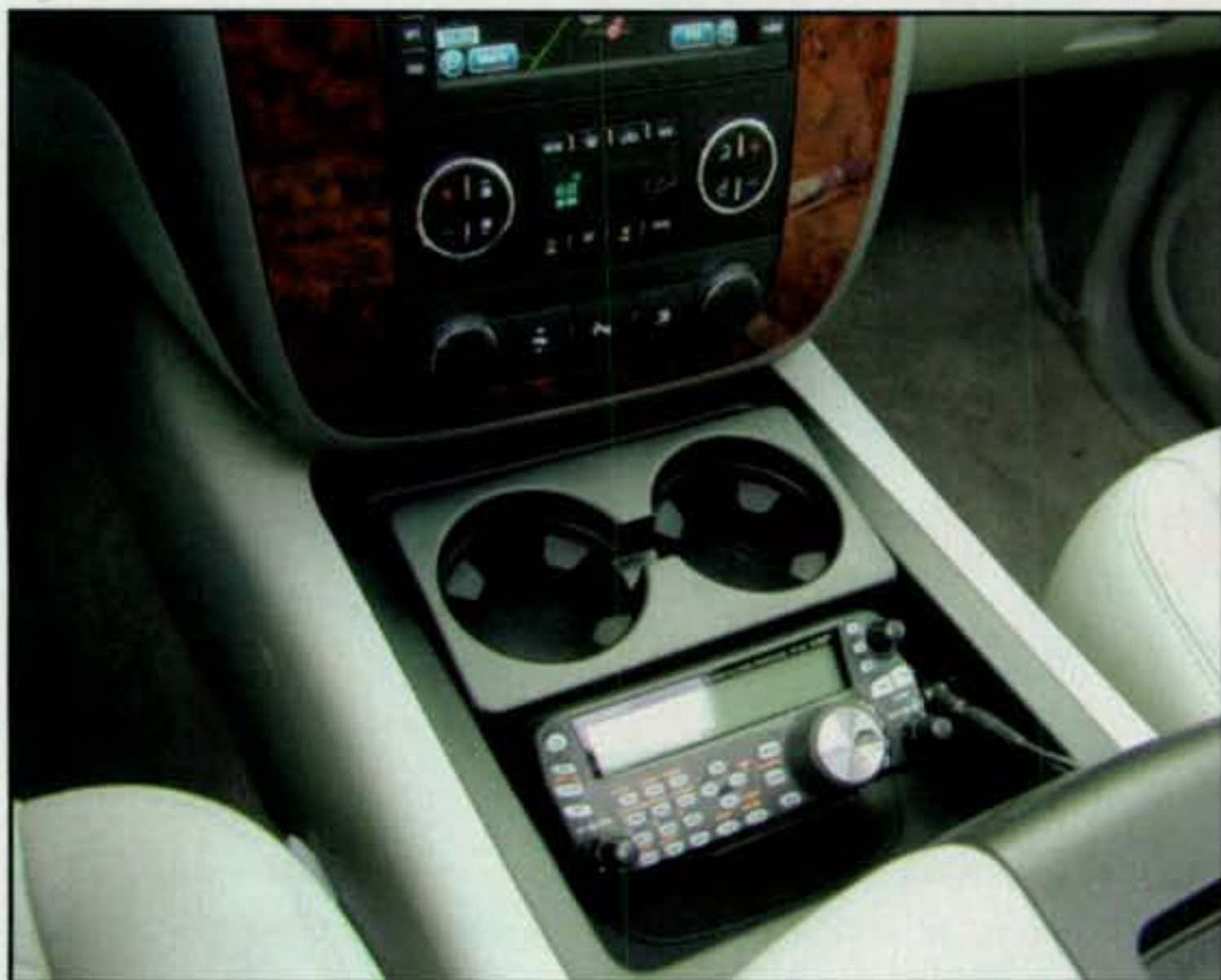
Photo F— The driver's seat view of the TS-480SAT in a GMC Tahoe setup put together by Rick Hilding, K6VVA. The front/control panel tilts left or right for operation from either seat or removes and hides in a flash for security. The main body of the transceiver is mounted in the rear of the vehicle. Rick has two more transceivers; they are mainly used at home, and they are both TS-480s!
