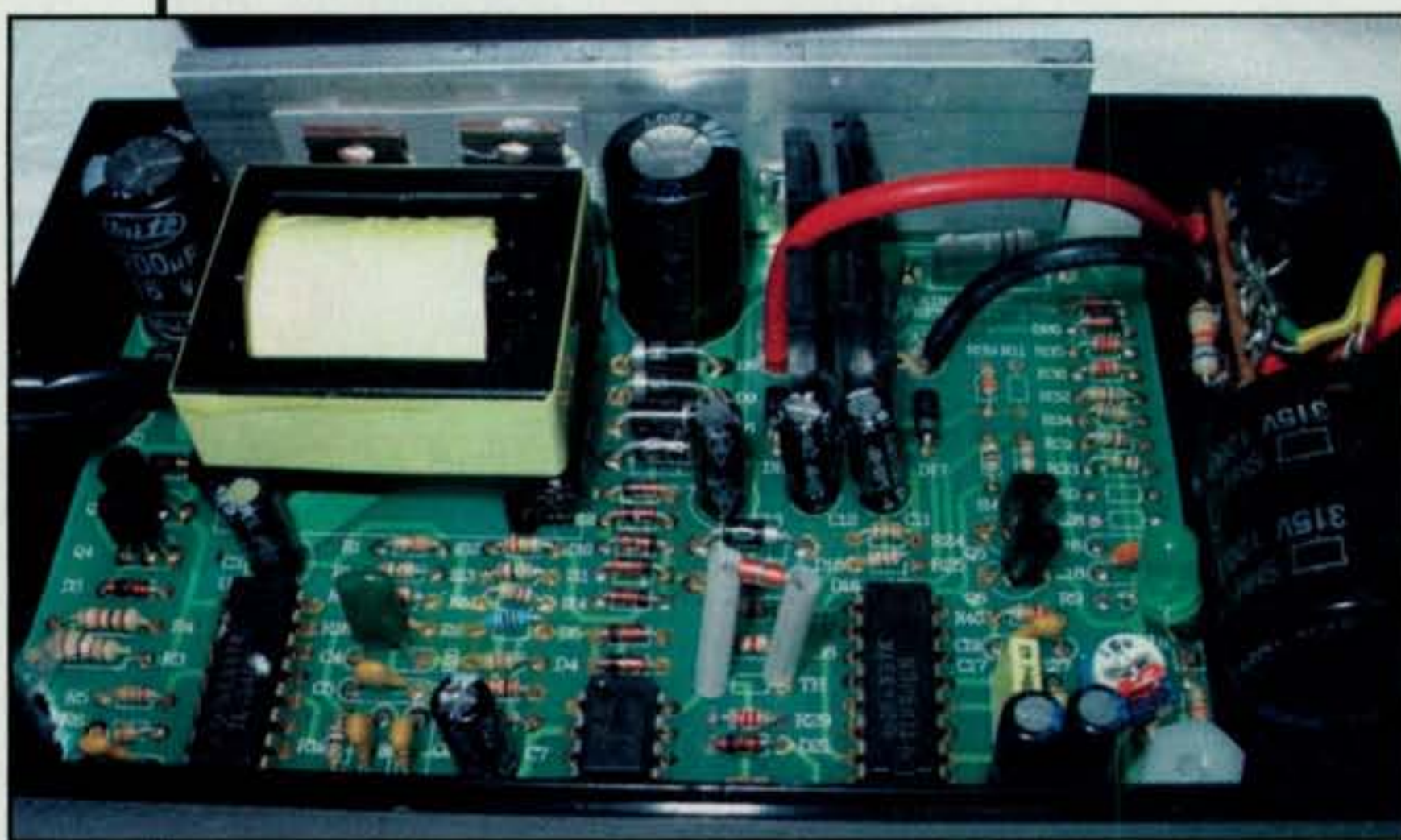
Photo B— Internal view of the inverter mounted in the new box with the rectifier circuitry.
