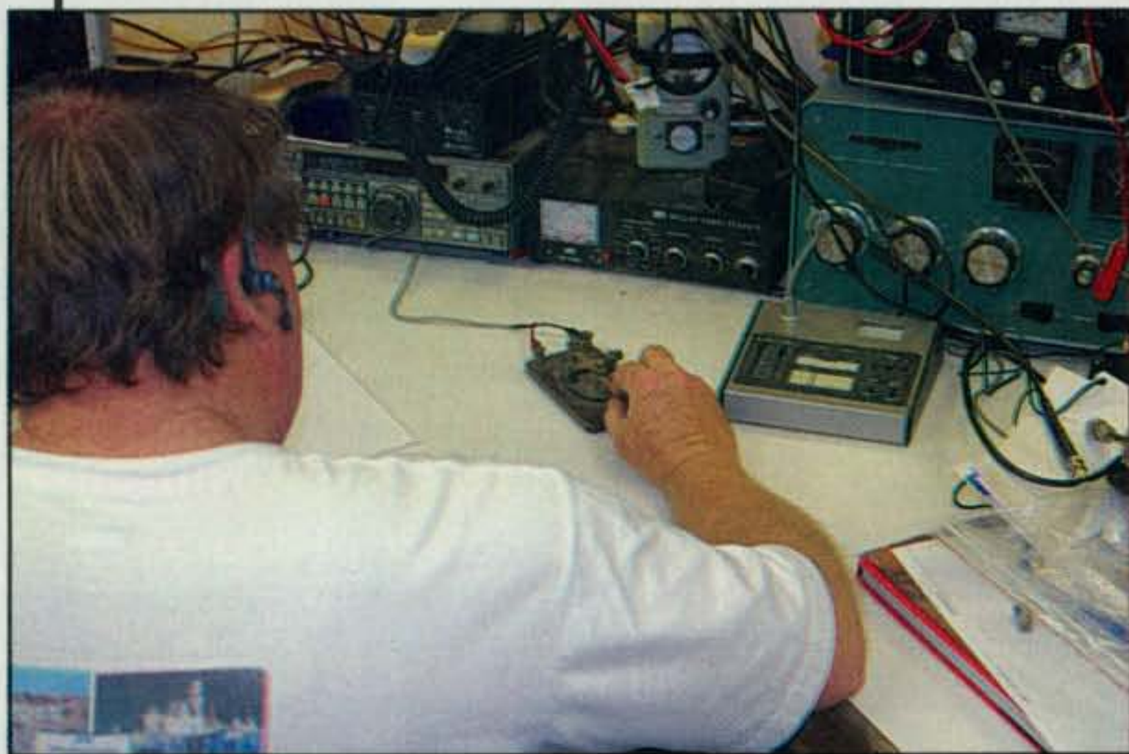
Here is a look over the shoulder of Dave Glawson as he sends a message using a straight key. Notice the firm grip on the knob, and his forearm rests on the tabletop. Dave is WA6CGR, located in Diamond Bar, California.
