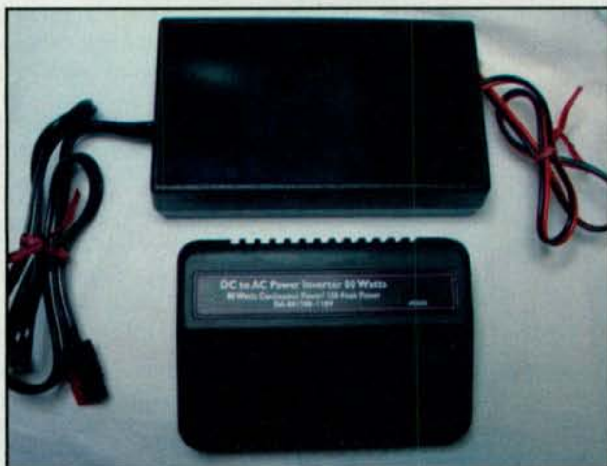
Photo A— Remounted power supply in larger box compared to original inverter case.
