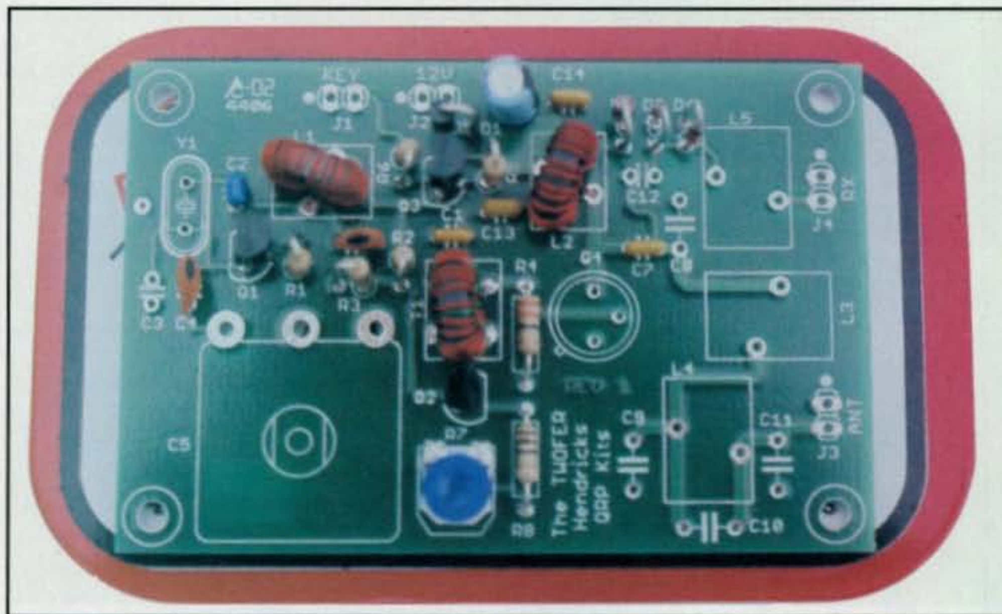
Photo B— Approximately midway during assembly, I paused to shoot this photo. Actually, all the small components (resistors, capacitors, and transistors) have been installed and only band-related components plus power amplifier transistor and VXO capacitor are yet to be installed. Assembly time to this point was approximately 30 minutes.
