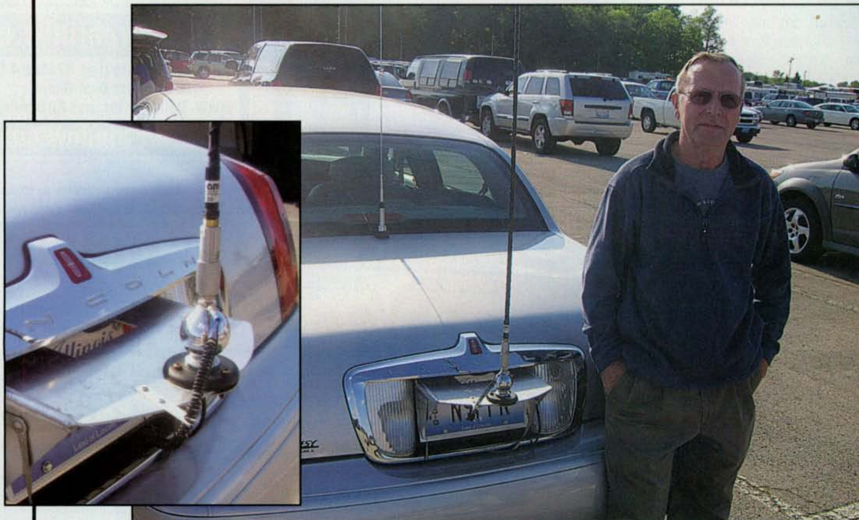
N9FPR took advantage of the area behind and above his license plate to mount a good-performing HF antenna that did not require drilling conspicuous holes in his vehicle.
