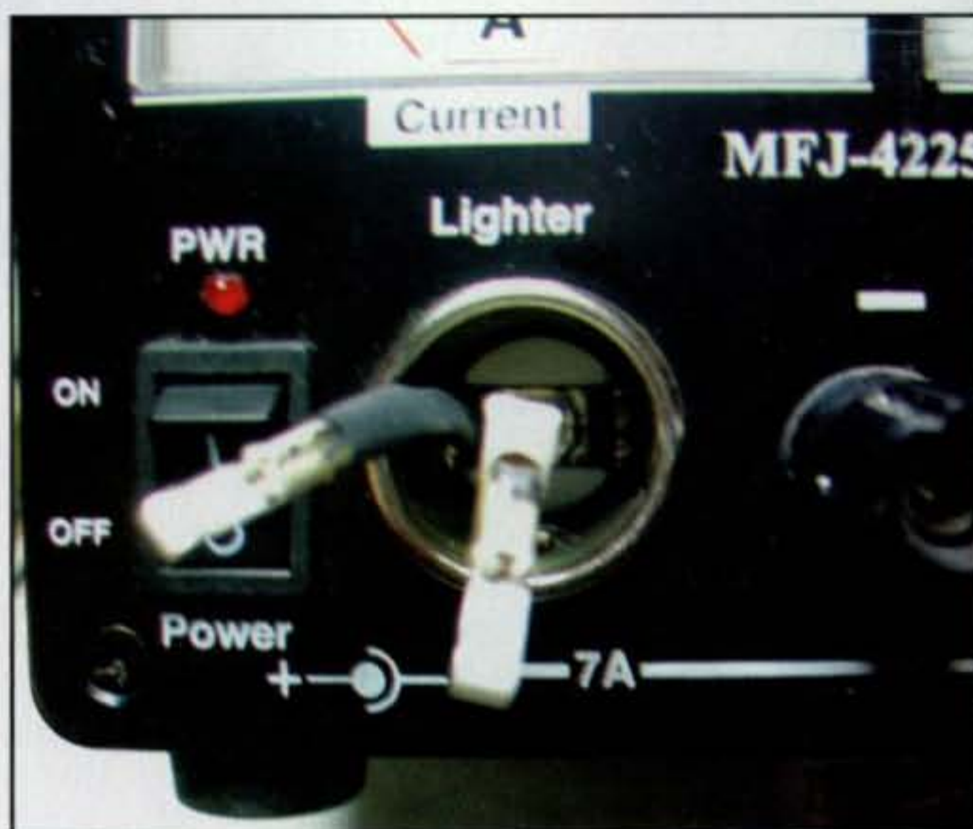
Photo C— Braid assemblies soldered in place.
