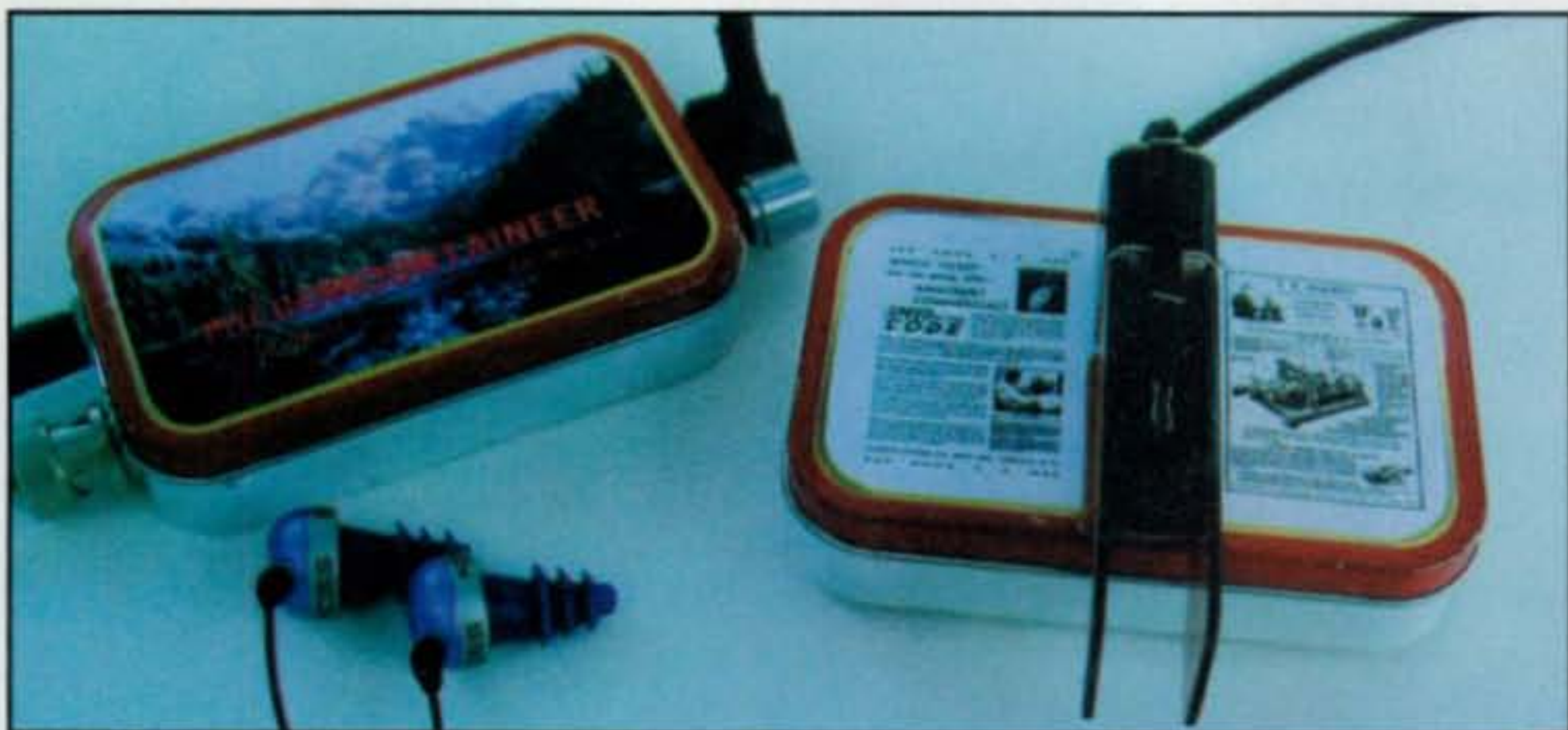
Photo D— Supporting the philosophy “if it fits in an Altoids® tin, it is genuine QRP” is this two-tin station built by Dennis Payton, N9JXY. The upper-left item is a classic “Micromountaineer” mini transceiver designed by W7ZOI. The item on the right is a Jackson Harbor in a tin with a homebrew paddle attached to the top. Note the unique labels on the lid of each tin. (Photo courtesy of N9JXY)
