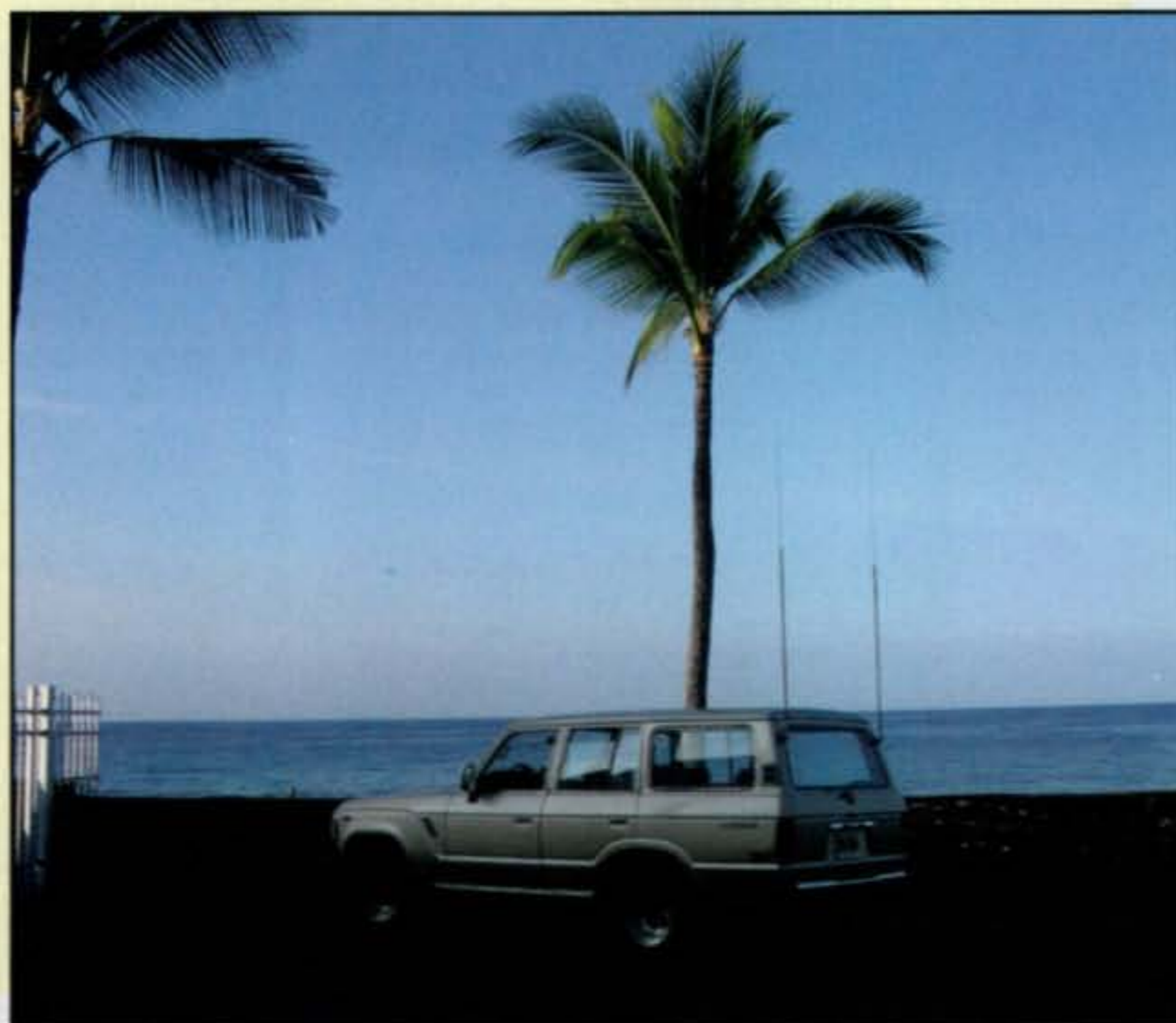
Photo C—KH6/W7UEA mobile at the oceanside in Hawaii. Dual/phased 20-meter Hamsticks are supported by Diamond K400 trunk lip mounts on each side of Land Rover's tailgate. The antennas consistently exhibit 2 to 2.5 S units gain over a single antenna. (Photo courtesy of KH6/W7UEA)
