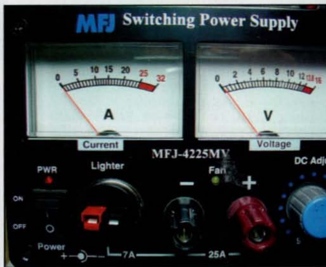
Photo D— The final Powerpole-equipped power supply.
