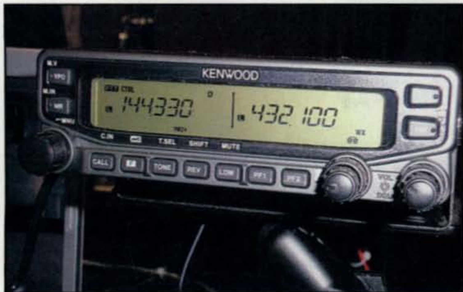
Photo J— The control head of the new Kenwood TM-V71A is detachable and reversible, so you can mount the rig with the speaker facing either up or down, and still have the head right-side-up. It includes a weather-alert feature and is compatible with the ARRL's Travel-Plus repeater mapping program
