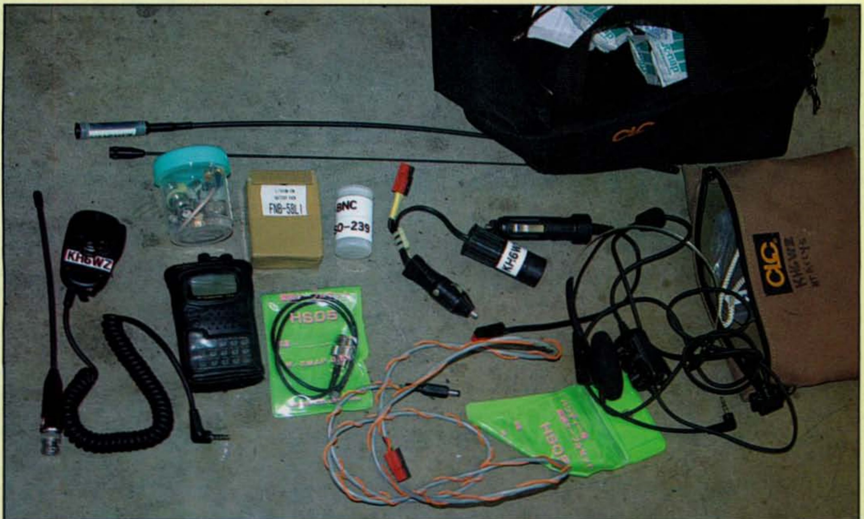
The "all mission" gear Grab and Go Kit, with all of the absolutely essential items needed for an emergency communications assignment: a dual-band HT, an extra battery pack, a gain antenna, and other accessories. All items are carried in a fanny pack or my pockets for total portability. Longer duration assignments call for more items, such as an external gel-cell, a compact battery charger, and a small solar panel.
