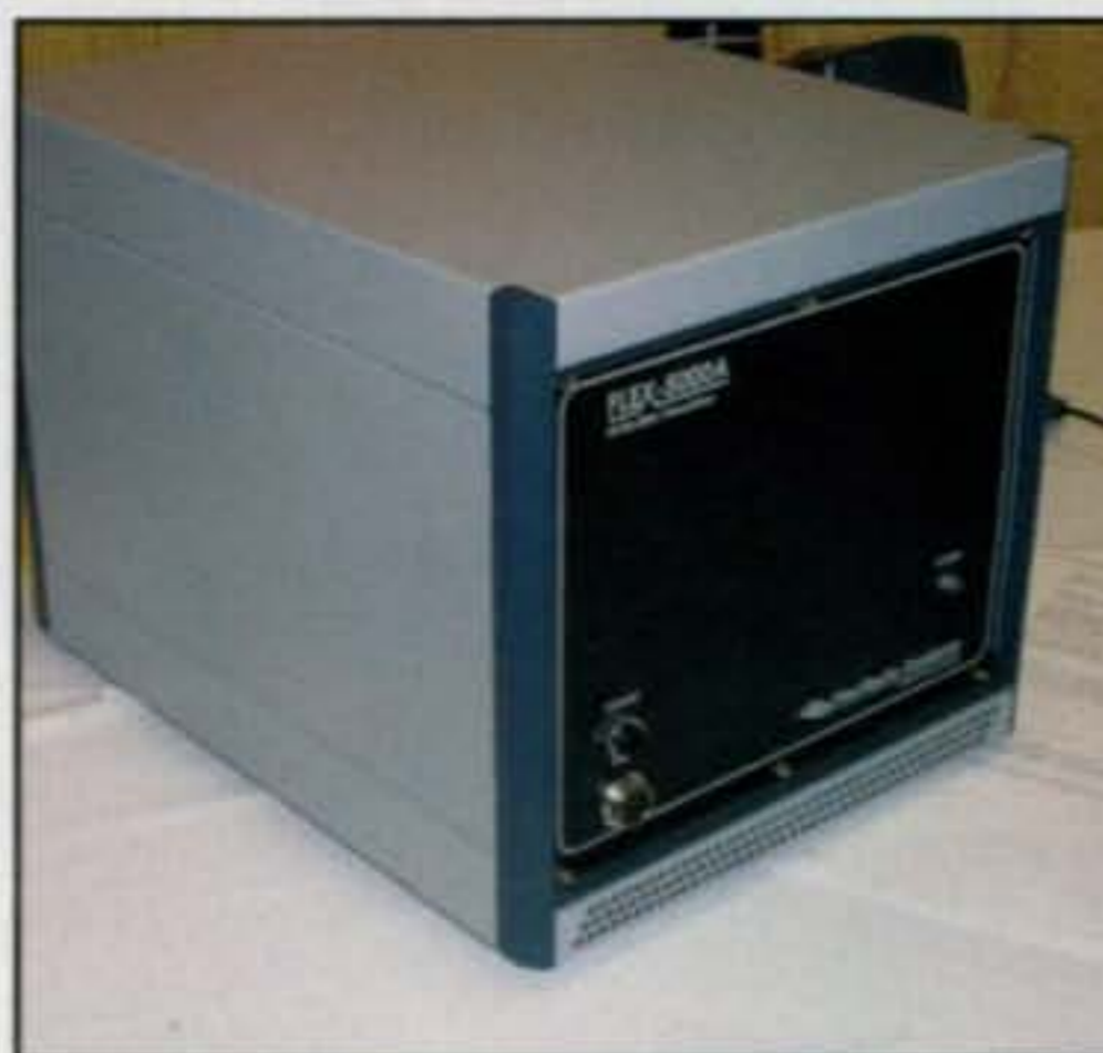
Photo B— FlexRadio's Flex-5000, representing a new generation in software defined radios, is a "black box" with connectors on it, as all settings are controlled from your computer.
