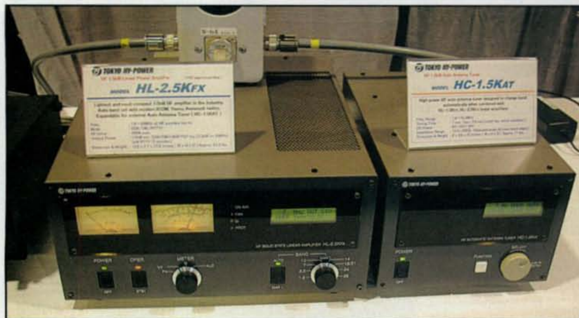
Photo H— Tokyo Hy-Power's HL-2.5KFX is a 1500-watt PEP solid-state amplifier covering 160–10 meters. It's shown here next to another new unit, the HC-1.5KAT automatic antenna tuner.
