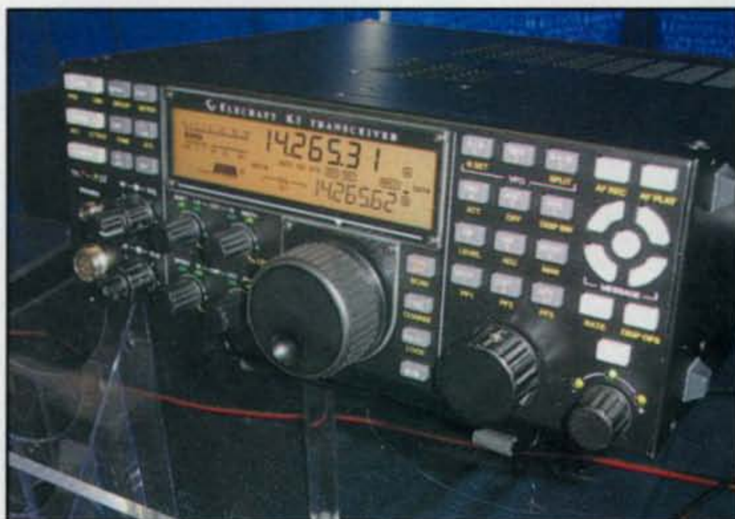
Photo A— The Elecraft K3 transceiver is a "modular kit" in which all the circuit boards are pre-assembled. It covers 160–6 meters at either 10 or 100 watts. (Photos by the author unless otherwise noted)
