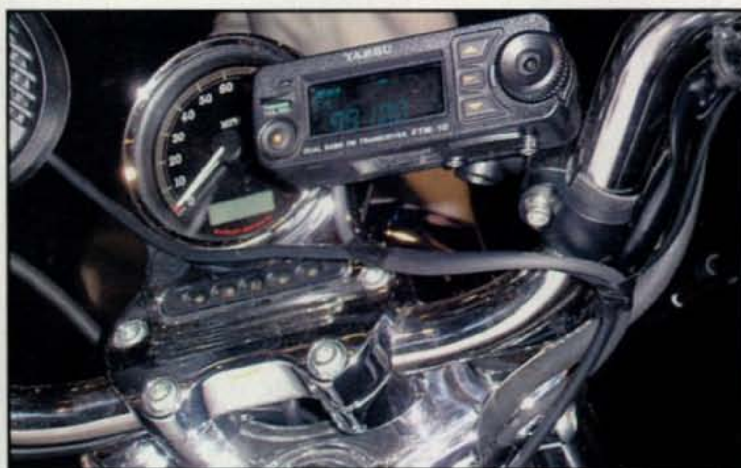
Photo K— The weather-resistant Yaesu FTM-10R is designed with the motorcycling ham in mind. One unique feature is that the mic and push-to-talk switch are located in the detachable front panel, so you can hold the whole front panel in your hand and talk into it. The radio will also be Bluetooth-compatible.
