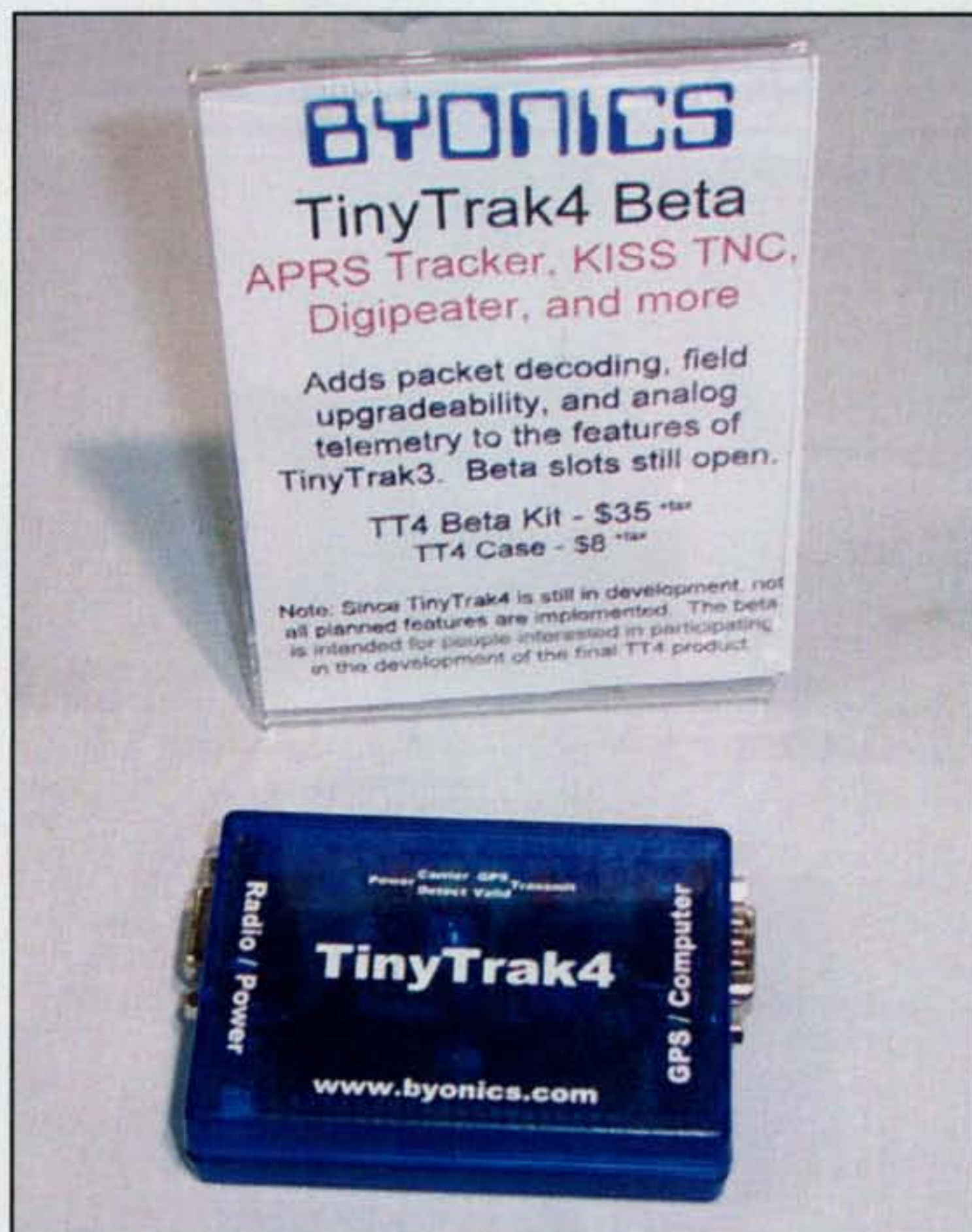
The TinyTrak4 Beta, from Byonics, is the latest incarnation of a family of APRS-ready modules. This one serves as an APRS tracker, KISS TNC, and digipeater and is the size of a small box of matches. If you’re not the beta-version type, the TinyTrak3 is still available.
