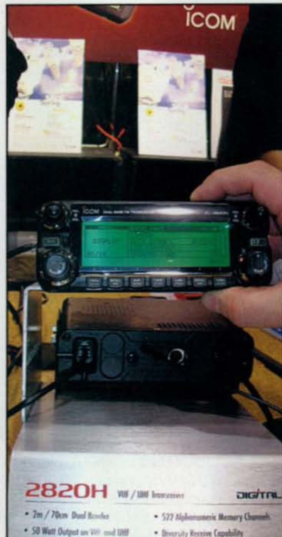
Photo I— ICOM's IC-2820 is a dual-band 144/440 MHz transceiver which (with an optional digital unit) features D-Star digital voice capability and internal Global Positioning System capability, the first ham rig to do so.
