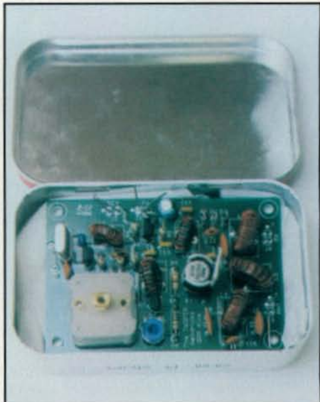
Photo C— The assembled, tested, and fully operational Twofer nestled in an Altoids® mint tin. After adding my “Ingram Mod” described in the text, I moved the Twofer into a plastic case so it could freely radiate a wireless BFO/conversion signal into a nearby AM-type shortwave receiver.
