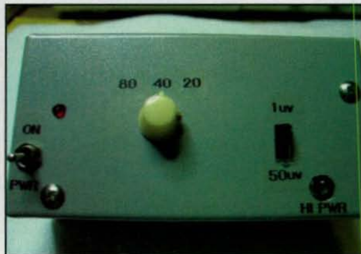
Photo C— Control-side view of the packaged XG2. Isn't this more convenient to operate than the original PC assembly?
