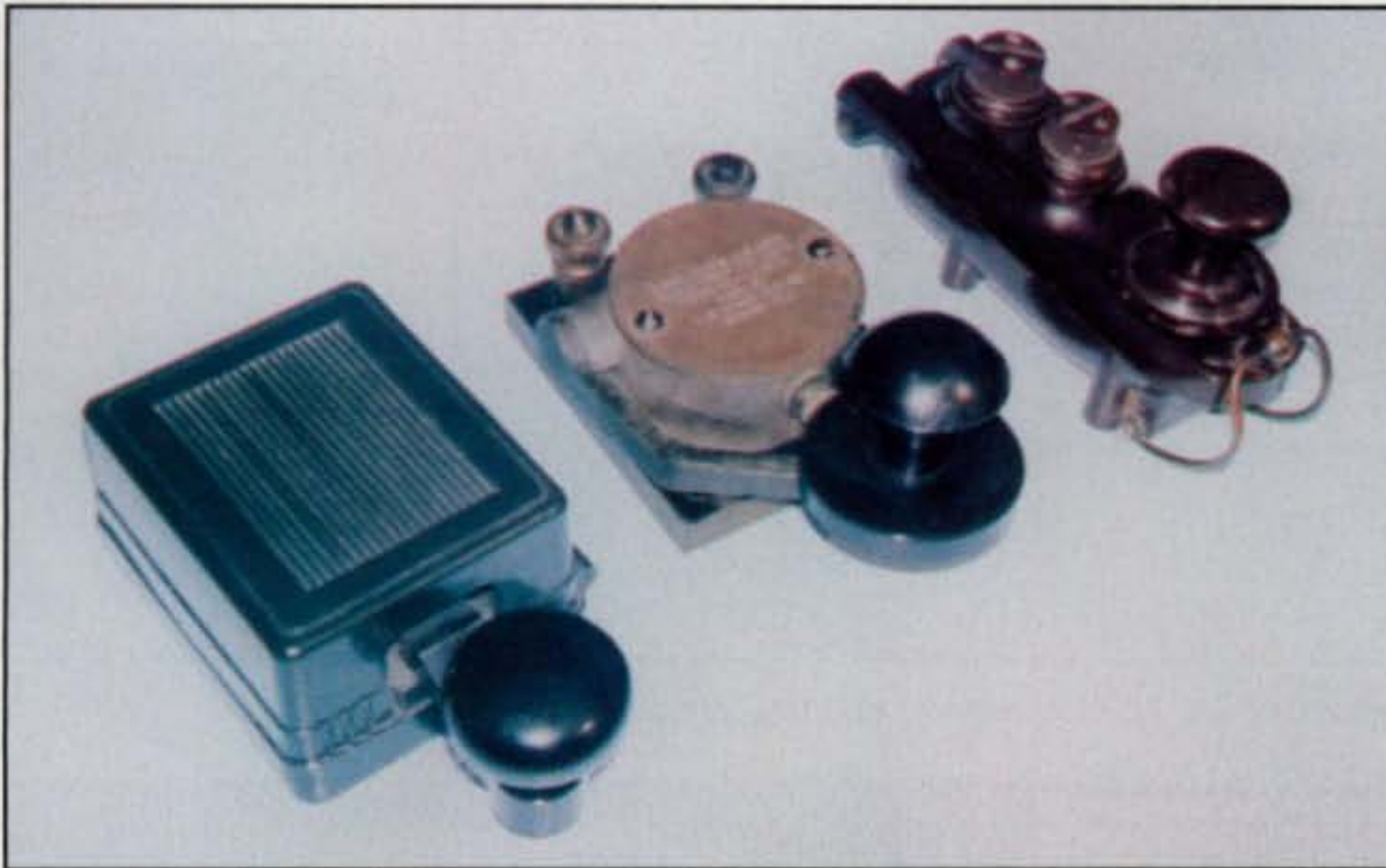
Photo C— Keying relays and/or other safety precautions/devices definitely have their benefits when using vacuum-tube transmitters, but somehow they lack the genuine thrill (and danger!) of using an authentic era key. As a happy medium, you might consider using an enclosed-mechanism key like the ones shown here, but only if you are well-trained in working with high voltage. The vintage keys are (left to right) a Russian pumper, U.S. Army J5A, and British Bathtub key. Modern-style enclosed-mechanism keys are available from < www.MorseX.com >.
