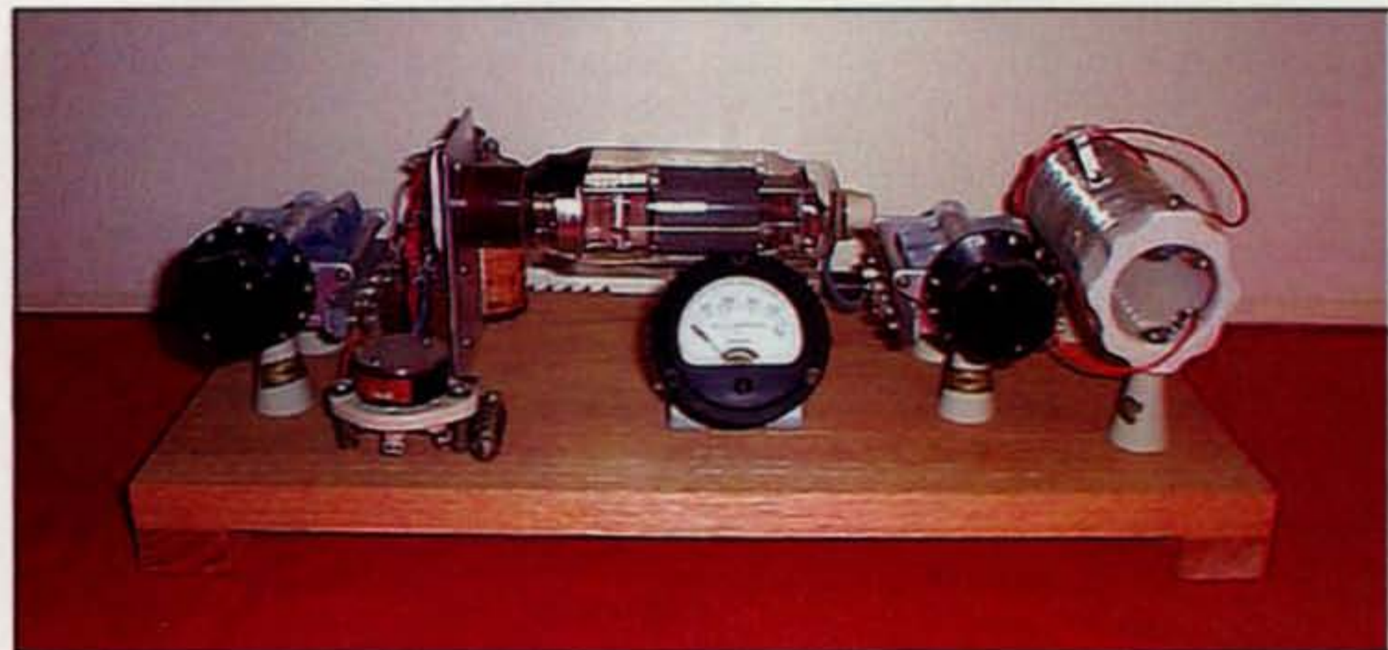
Photo B—The remarkable reproduction of the glamorous 804 horizontal-tube transmitter made by W6JRY. Look at that tube, that plate, that round Bliley crystal, those vintage knobs!
