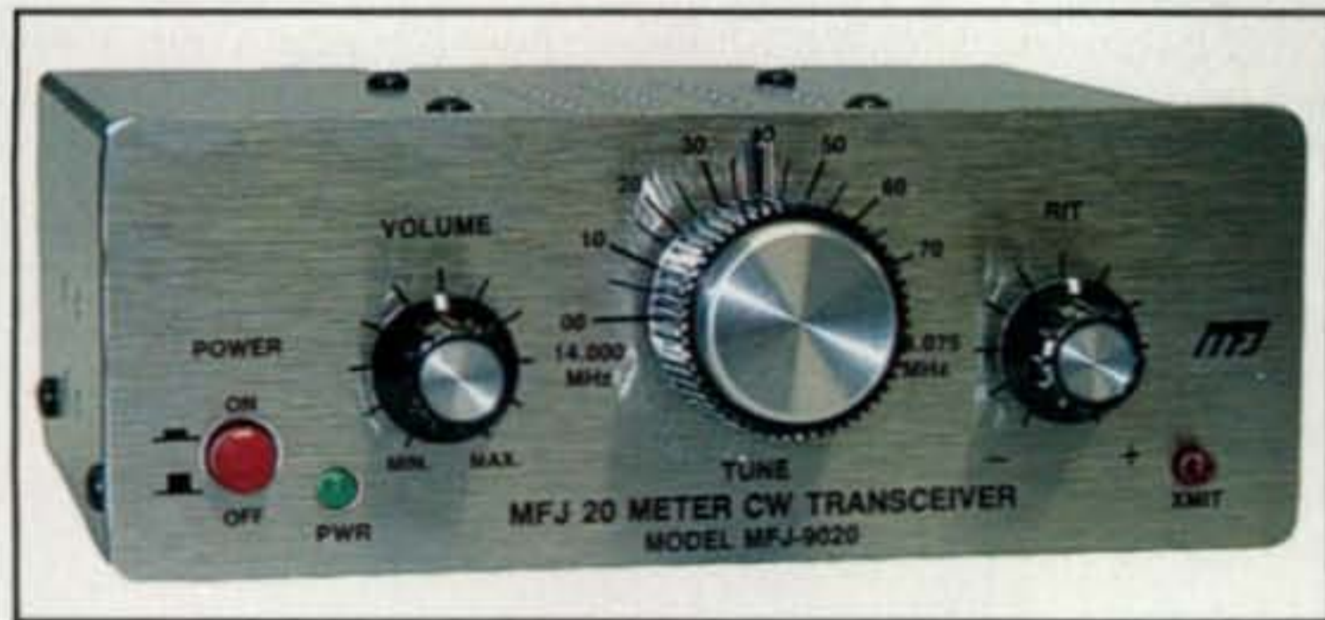
Photo A—MFJ's "90s" series of 5-watt CW monoband transceivers are well-known for their easy operation and stout-hearted reliability. The transceivers feature a sensitive receiver with sharp 500-Hz IF filter, rugged power-output transistor, semi break-in operation, and measure 2.5" x 6" x 6.5". More (Details in text.)
