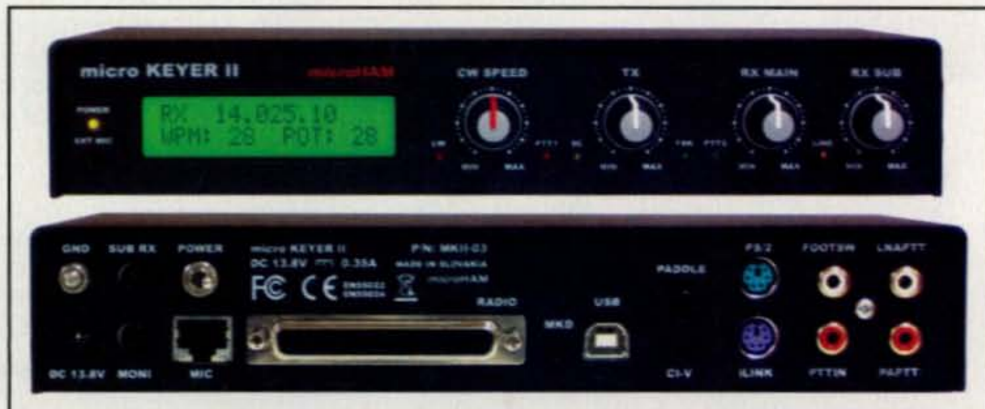
Photo C— microHAM's microKEYER-II front/back views showing many of the features of this powerful all-in-one radio controller. (Photo courtesy of microHAM)
