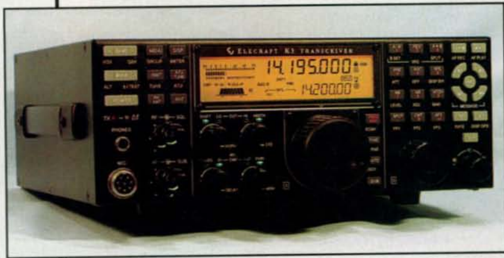
Photo A— Elecraft's new high-performance K3 transceiver. This photo, from the Elecraft website, is of a beta unit. Final layout of controls may vary slightly from production model. (Photo courtesy of Elecraft)
