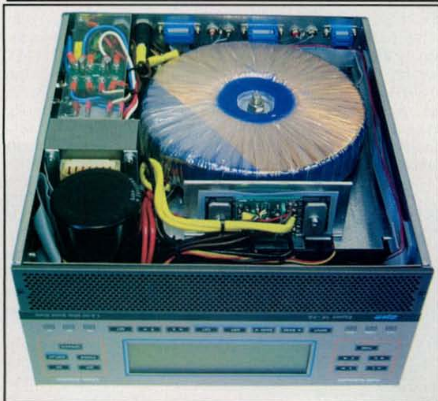
Photo B— The bottom (power supply) portion of the amplifier. Look at that power transformer!
