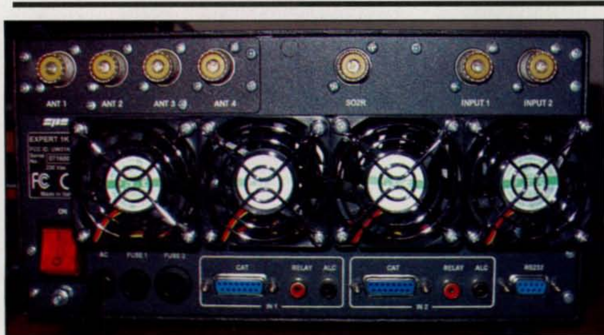
Photo F— Interfaces for transceivers and antennas are well-marked and self-explanatory. Note the SO2R connector.
