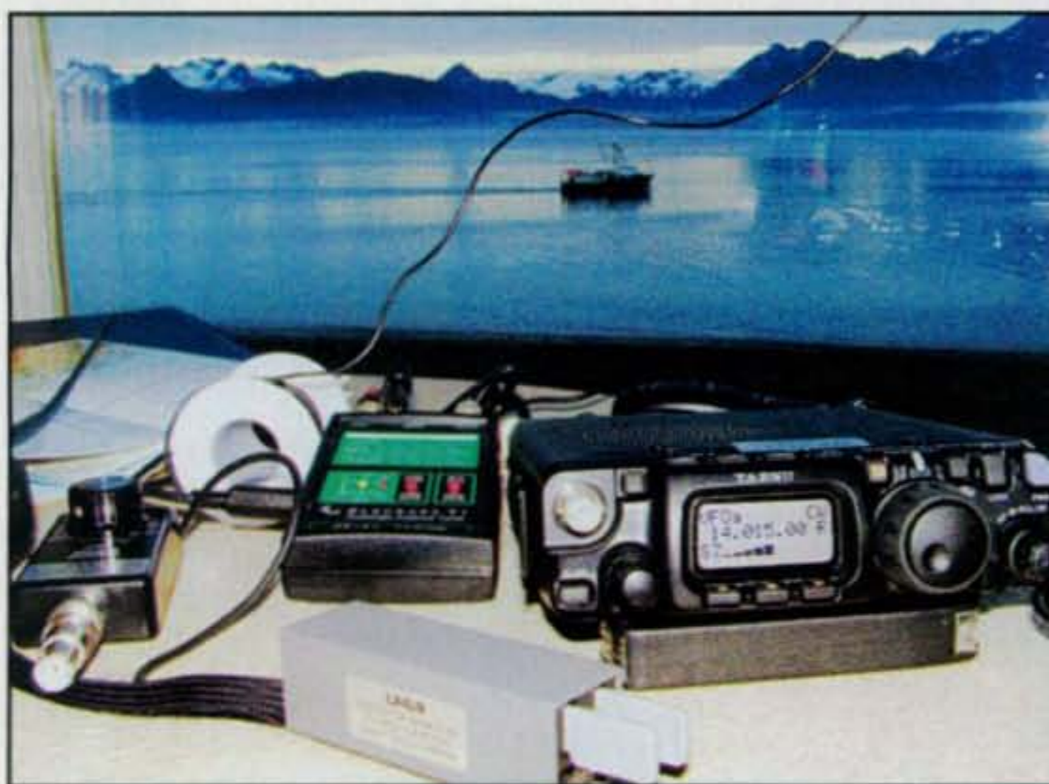
Tom, LA4LN, spent a few weeks in Alaska. This picture shows the "scene of action" out of the hotel window. The Yaesu FT-817 was using the fully automatic Elecraft T1 antenna tuner (middle left) hooked up to his Bobtail-Curtain's antenna wire. The manually operated Miracle Antenna tuner (far left) was used in some rare high-impedance antenna cases, when the Elecraft tuner wouldn't obtain a match. The Palm Radio Mini Paddle shines in the front. A fishing vessel is seen on the fiord in front of the glacier-laden mountains in the background under the light Arctic night sky. (Photo courtesy of Tom, LA4LN)
