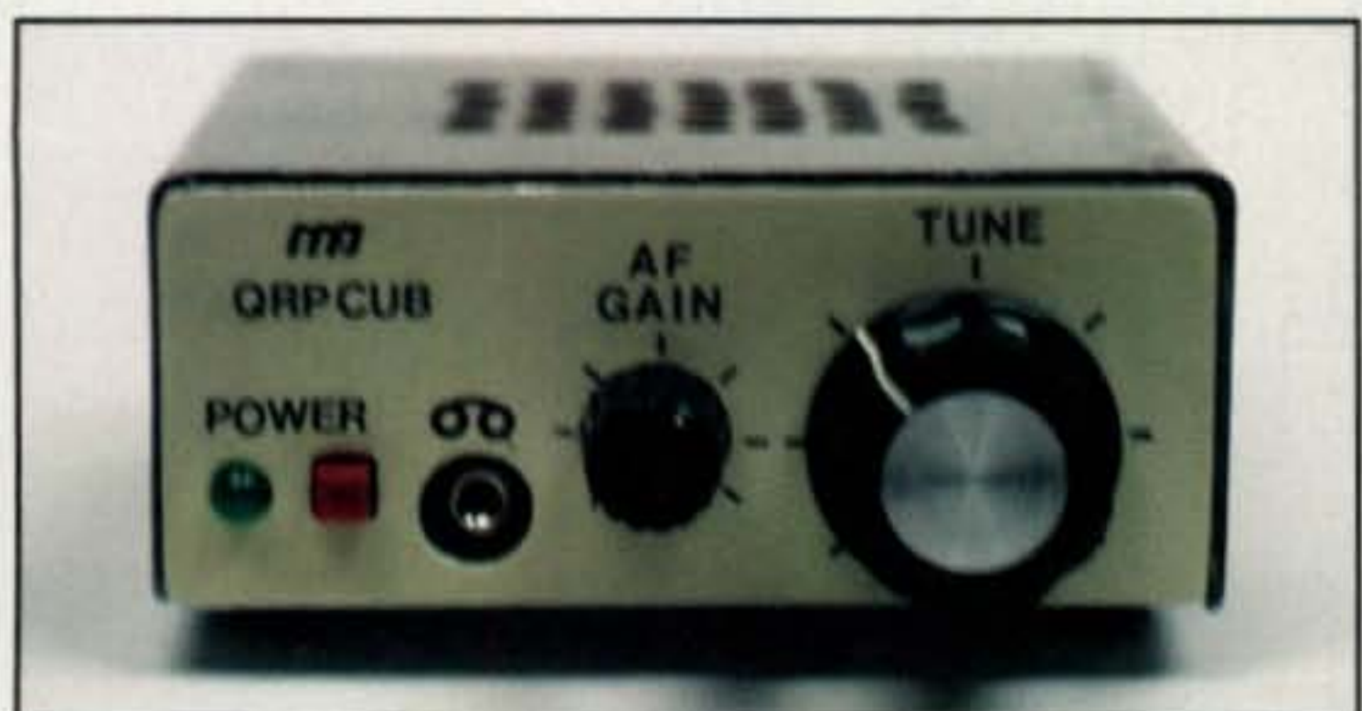
Photo C—Thinking about handheld QRP? MFJ's monoband "Cub" CW transceiver kit is available in 80-, 40-, 30-, 20-, 17-, and 15-meter versions. The little rig pumps out a clean 2-watt signal (4 watts with optional transistor) and measure only 1.5" x 4" x 4.5". It is a toss-'n-go mini rig you can use and enjoy without serious "high-cost rig" concerns.
