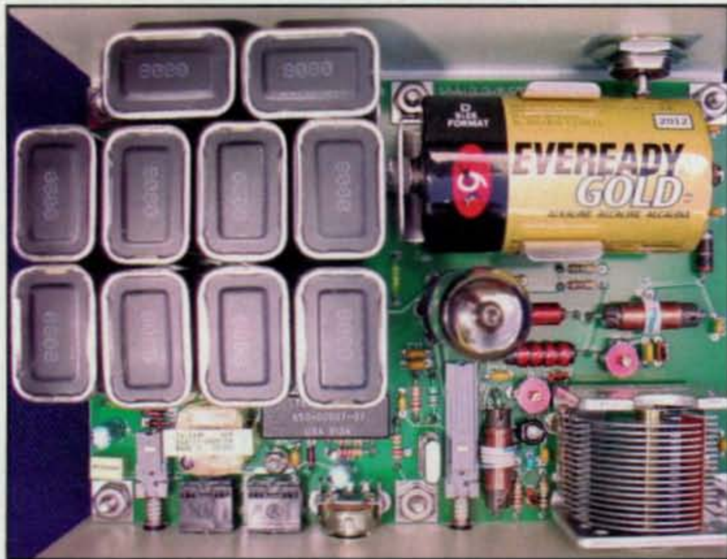
Photo E— Interior view of the 1-DER shows how everything installs on the rig's single circuit board for "can't miss" assembly. A large D cell powers the tube filament and keying relay; ten 9-volt batteries for plate power attach directly to clips on the board. Look closely and you will notice all the front-panel controls and sockets also mount directly on the PC board and slip through the panel holes. (Photo courtesy of KG4HSY)
