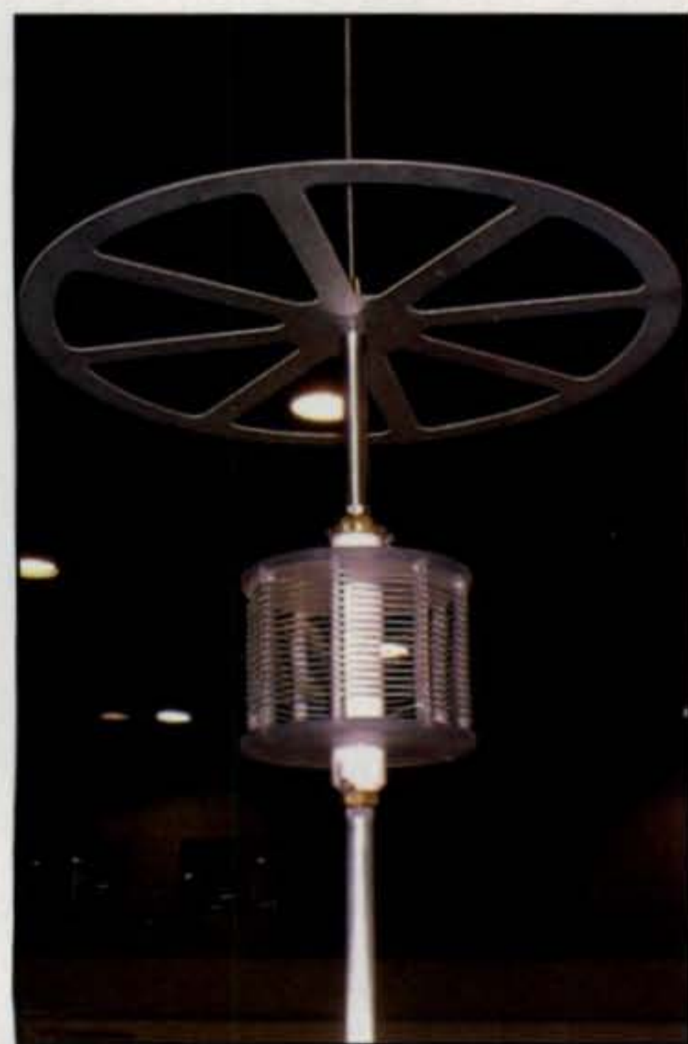
Photo B—Loading coils.
