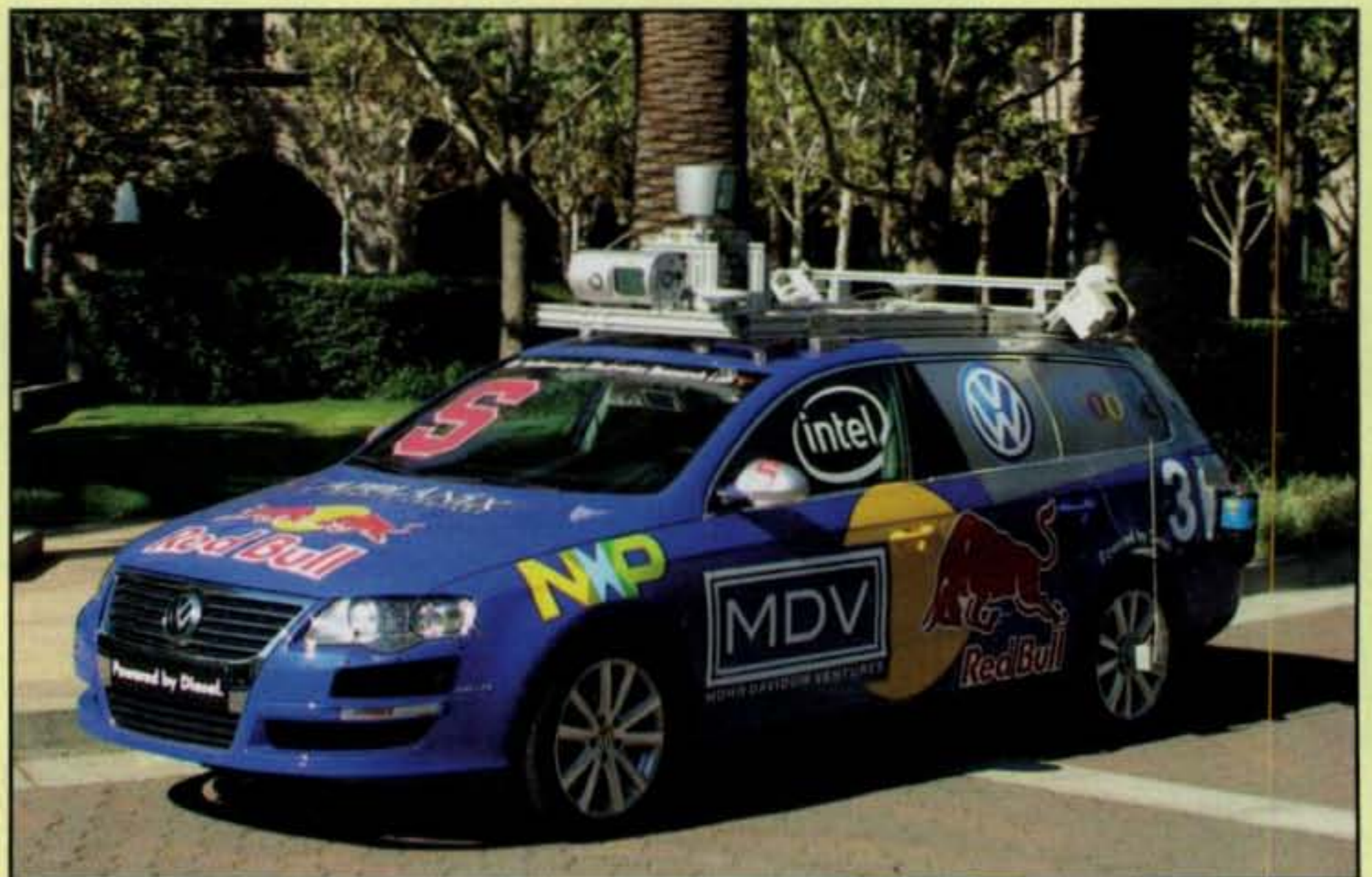
DARPA Urban Challenge semifinalist. Stanford University's "Junior" is a 2006 VW Passat wagon whose steering, throttle, and brakes all have been modified by engineers at the Volkswagen of America Electronics Research Lab in Palo Alto, California, to be completely computer-controllable. Junior's predecessor, "Stanley," won the DARPA Challenge competition in 2005. (Photo courtesy The Stanford Racing Team)
