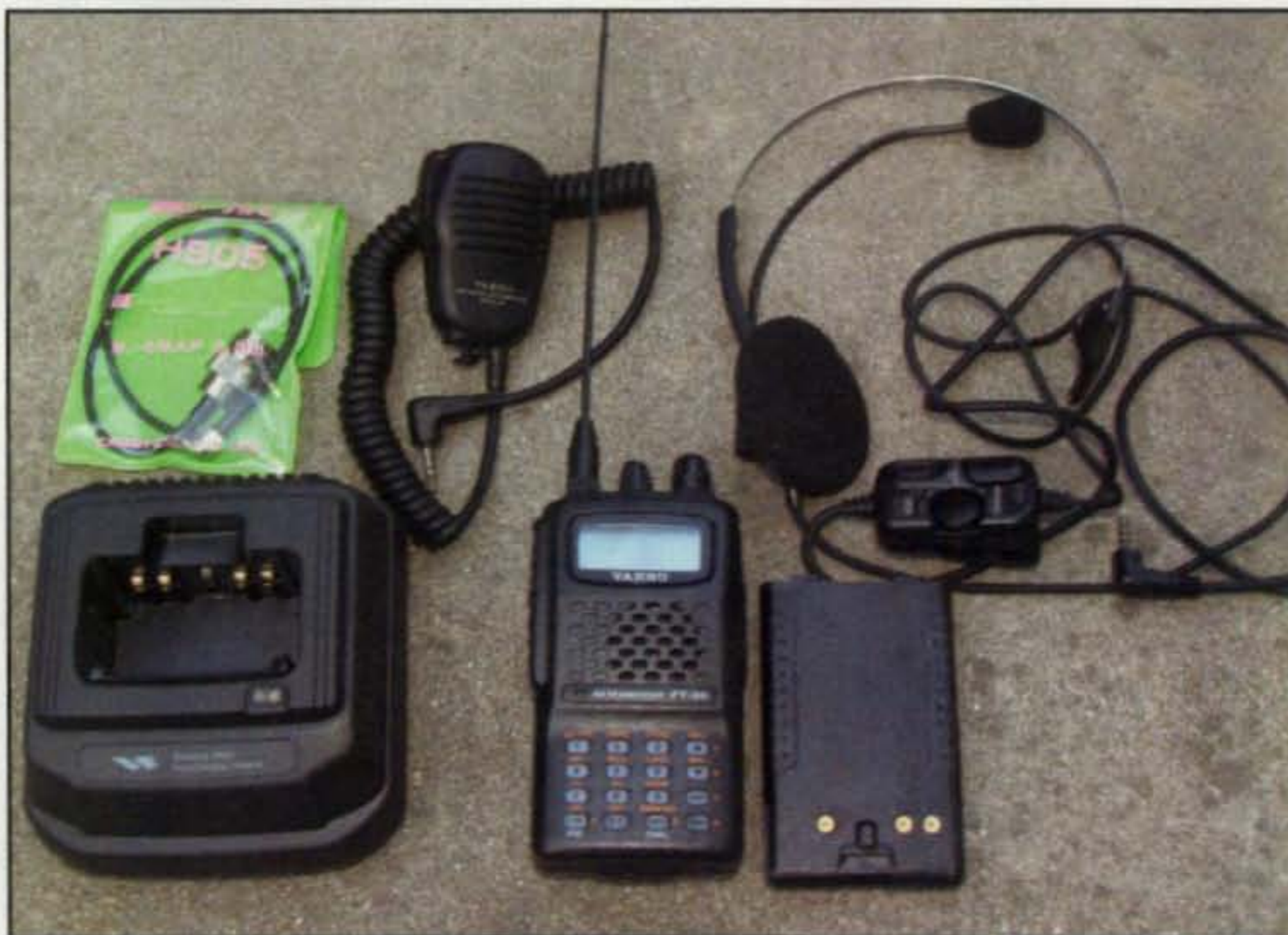
Photo B—These useful accessories will increase your operating enjoyment. You can convert the battery-operated rig into a mobile setup with the proper accessories, such as the speaker/microphone.
