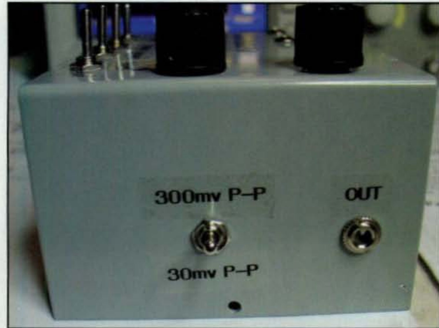
← Photo D— Output side of the packaged 2T-gen. Note the output-level range selector switch.
