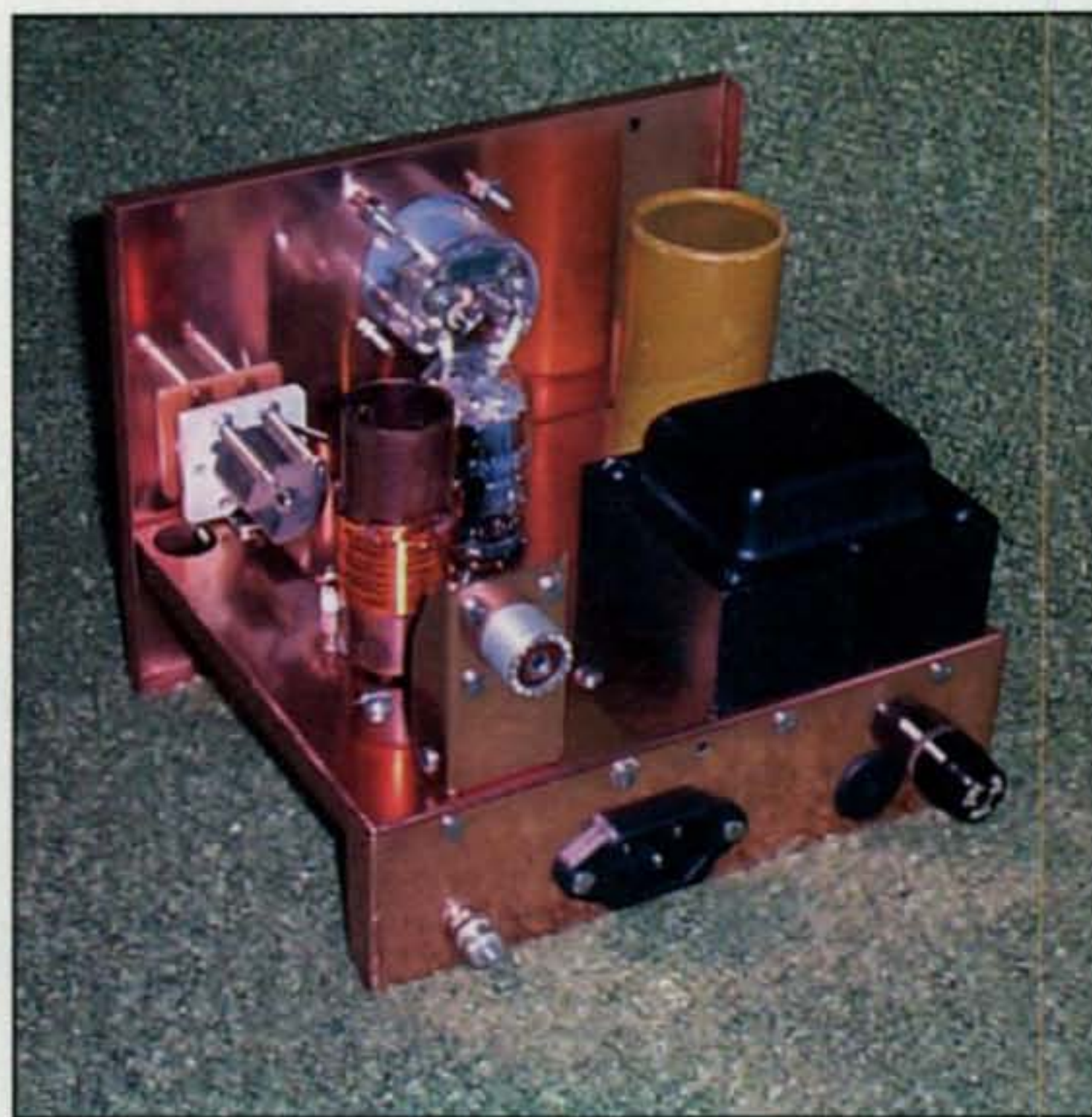
Photo D—Rear view of the W9SAY 6T9 transmitter reveals a clean layout with a "canned" filter capacitor under the cardboard wrapper and a Hammarlund 100-pF miniature tuning capacitor. All that copper reminds us of the classic R. L. Drake gear, doesn't it? (Photo curtesy of W9SAY)
