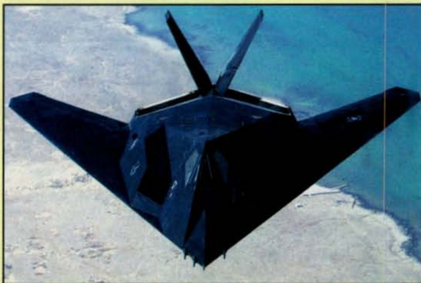
The F-117 fighter was the first operational aircraft to use stealth technology. The stealth aircraft program began at DARPA. (U.S. Air Force photo)
