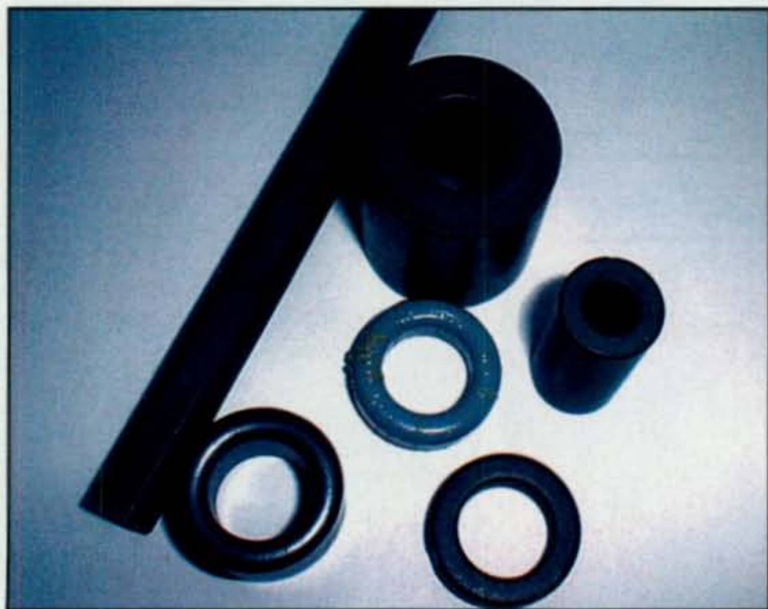
Photo D— Ferrite cores are not something you want in antenna loading coils.
