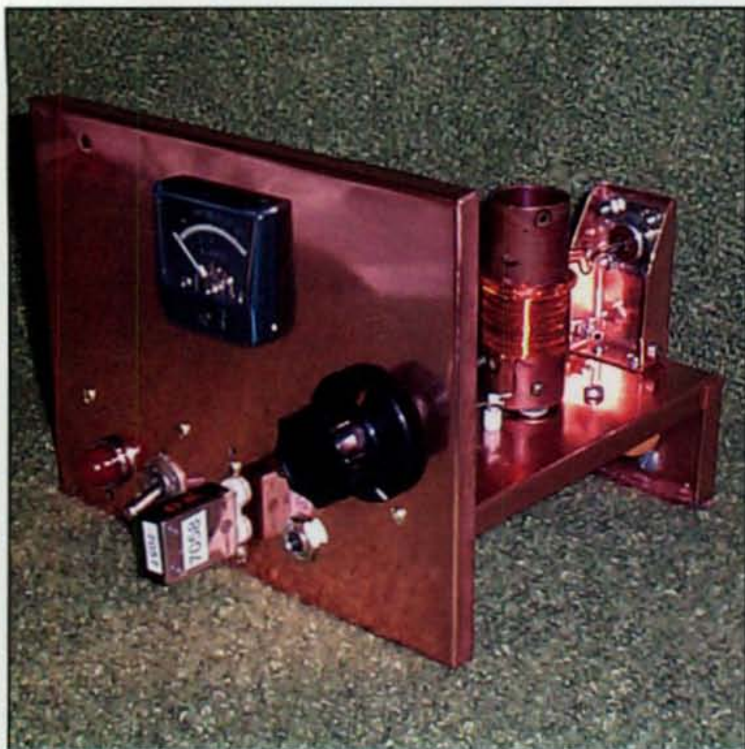
Photo C—Delightfully dangerous amply describes this open-air and copper-framed 6T9 transmitter built by Charlie Zarek, W9SAY. It runs 10 to 15 watts on 40 meters, has an on-board power supply, and sports a classic Heathkit meter on the front panel. Nice! (Photo courtesy of W9SAY)
