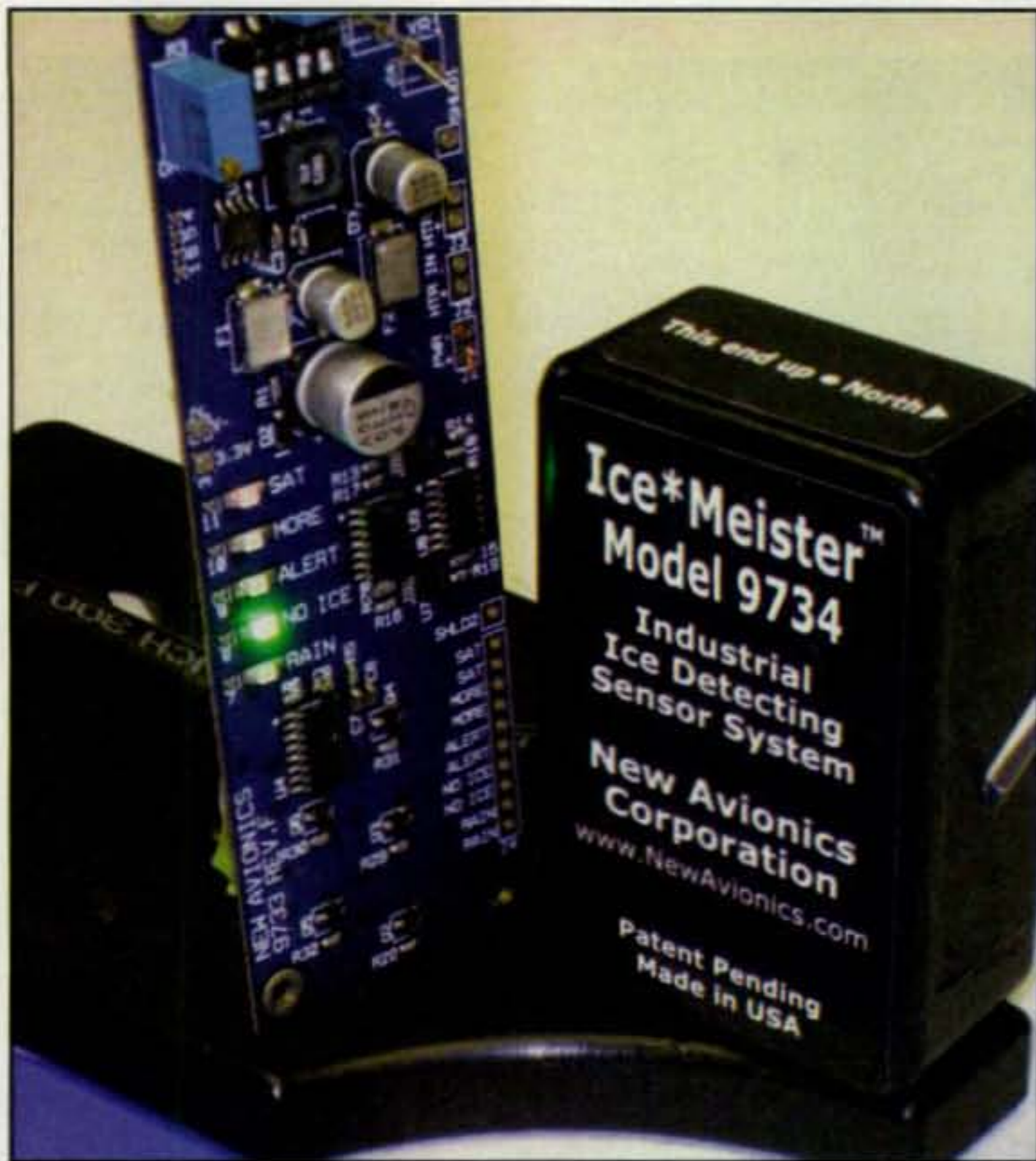
Photo D— The new Avionics Corporation's Ice*Meister Model 9734 Industrial Ice and Precipitation Detecting Sensor System. (Photo courtesy of Ice*Meister)
