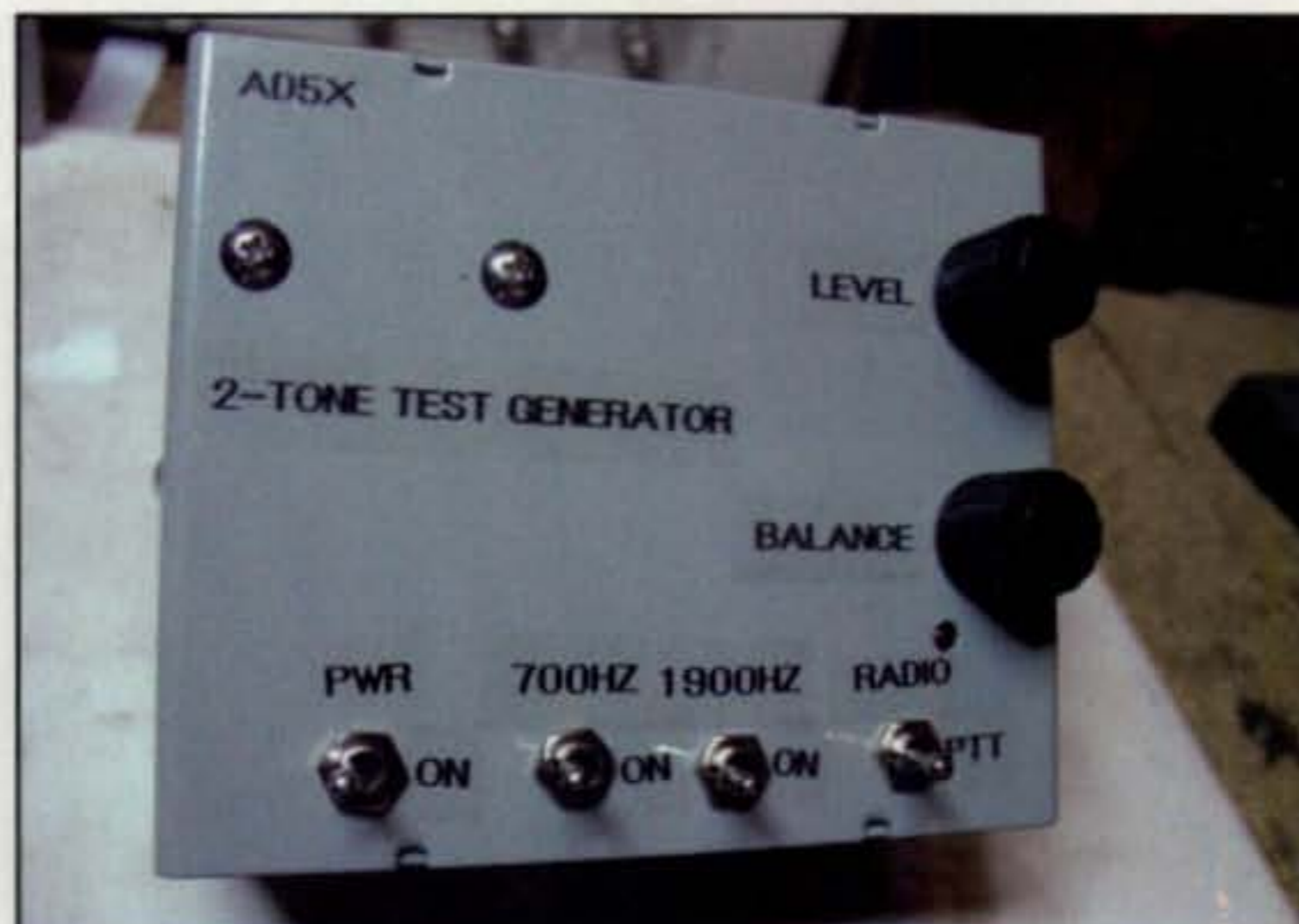
Photo C— Control-side view of the packaged 2T-gen. Aren't these controls much more convenient to operate than the original PC assembly?
