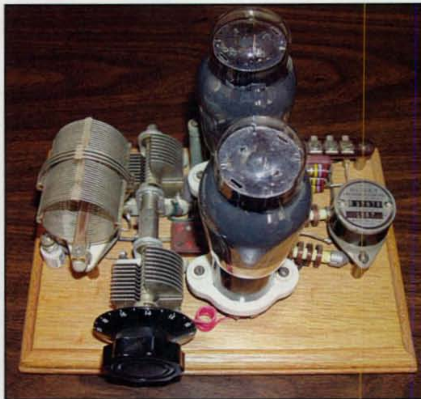
Photo A— Twins! The marvelous push-pull 6L6 transmitter Jerry Fuller, W6JRY, built on a 6" x 9" oak wood base with routed edges and authentic-era parts. Details on homebrewing a copy of the B&W "JCL" plug-in plate coil and dual-section tuning capacitor are in the text. (Photo courtesy of Jerry, W6JRY)
