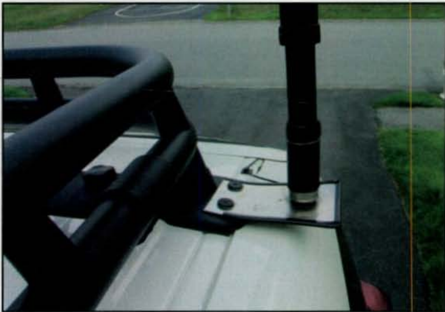
KC1HD took advantage of existing holes for his antenna mount. The location also allows him to remove the antenna while standing on the ground.
