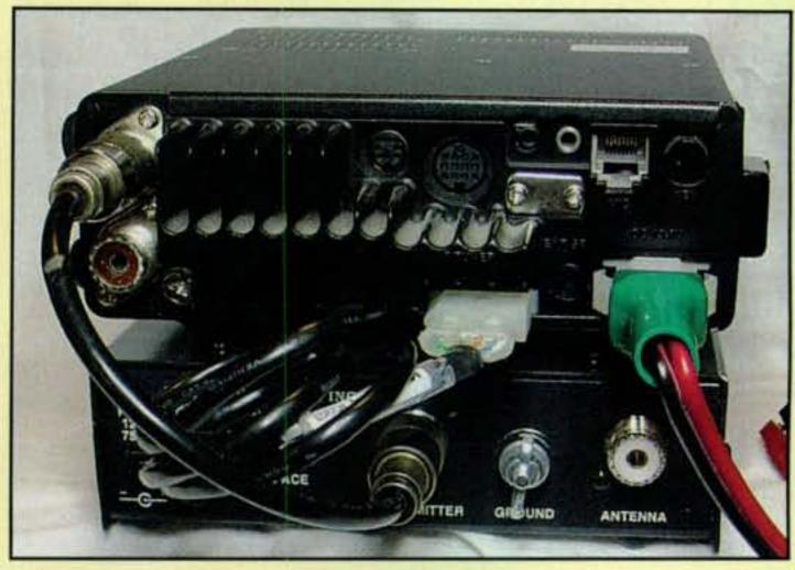
Photo F- Transceiver interface and coax interconnections between the MFJ-925 and the IC-706MkIIG.
