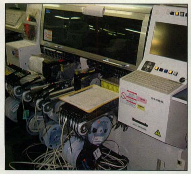
This machine places components on circuit boards. The tapes contain components that are placed on the boards with great precision and speed.
