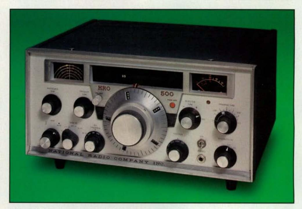
Photo C- The solid-state, synthesized National HRO-500 retained the classic PW dial of its predecessors but did away with the plug-in coils that had defined the HRO series.
