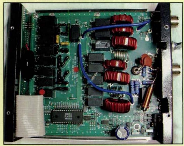
Photo G- Inside view of the MFJ-925. The inductor on the right-hand side is part of the internal bias-Tee, and the audio transducer is in the lower center. The author nibbled notches in the back-side lip so he could more easily play with the calibration procedure.
