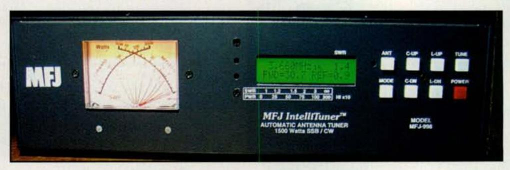
Photo A- The new MFJ-998 provides automatic antenna matching for QRP to full-legal-limit stations. (All photos by the author)
