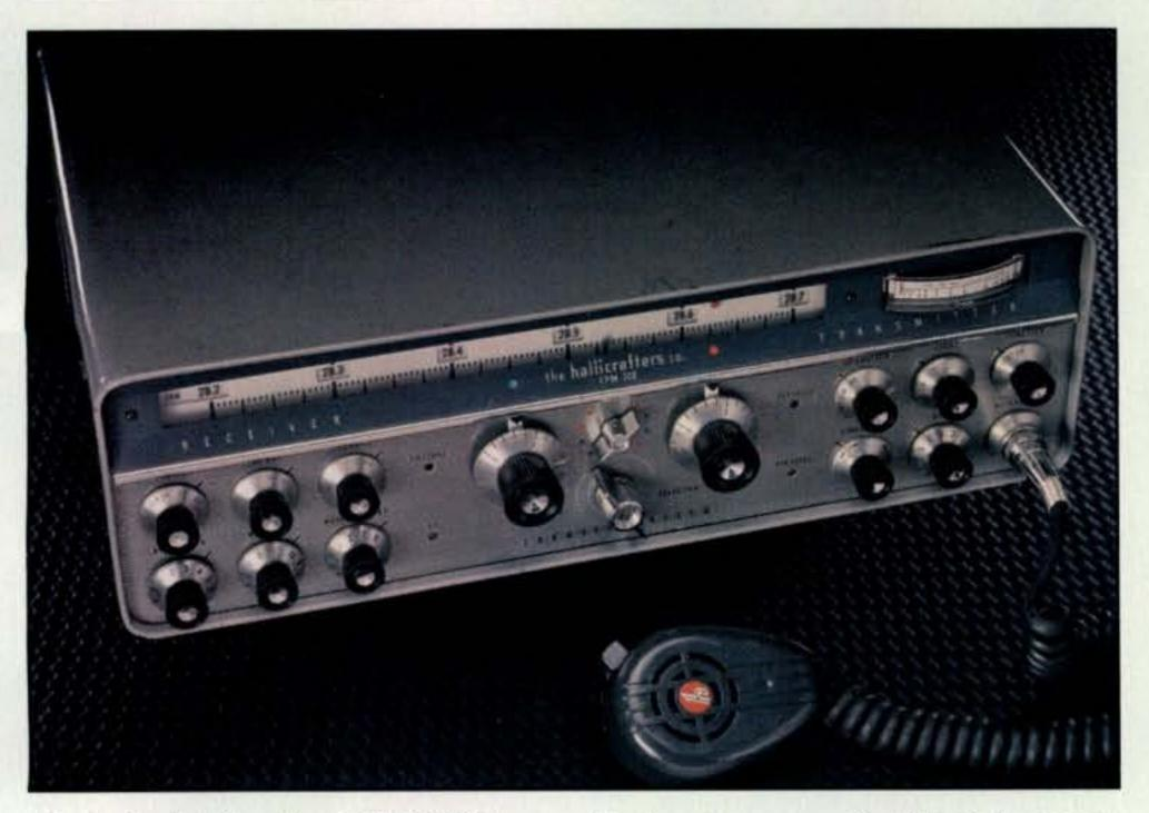
Photo B— Hallicrafters' FPM-200 transmitter/receiver was all solid state except for its 6146 finals, their 12BY7 driver, and a pair of OB-2 VR tubes.
