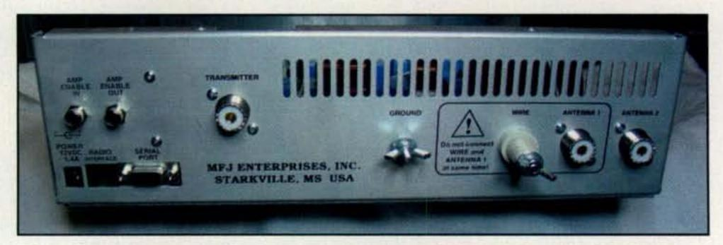
Photo D- Note the amplifier bypass connectors (labeled "Amp Enable"), as well as connectors for firmware upgrades and transceiver control.
