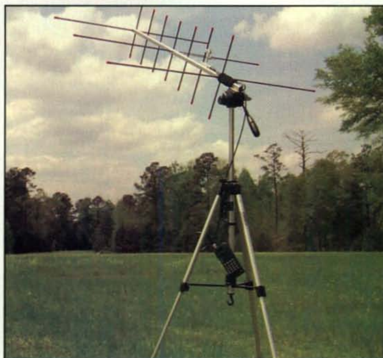
Photo 9— Operating the OSCAR satellites in a "now you see it" (antennas, that is), "now you don't" manner is a snap with Arrow Antennas' popular hand-positioned 2-meter/70-cm Yagis mounted on a camera tripod. Antennas are available from < www.visradio.com >.
