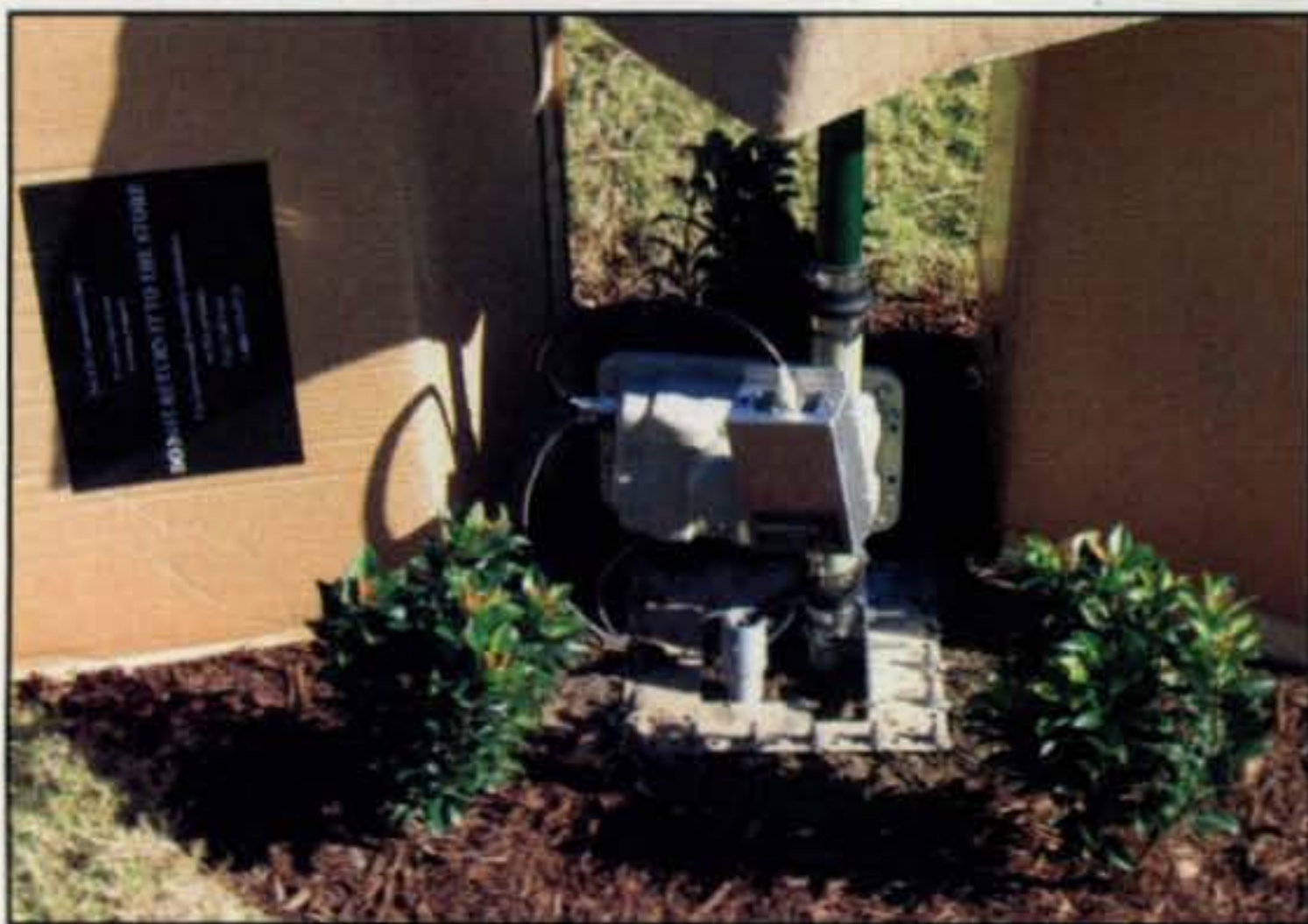
Photo 3— Bob raised the fiberglass rock, propped it up with boxes, and took the photograph to show us his work. The rock hides the SteppIR motor control, feed point, radial connection plate, a base-loading coil Bob added for 40-meter operation, and double coax relays for switching the coil in/out of the line.
