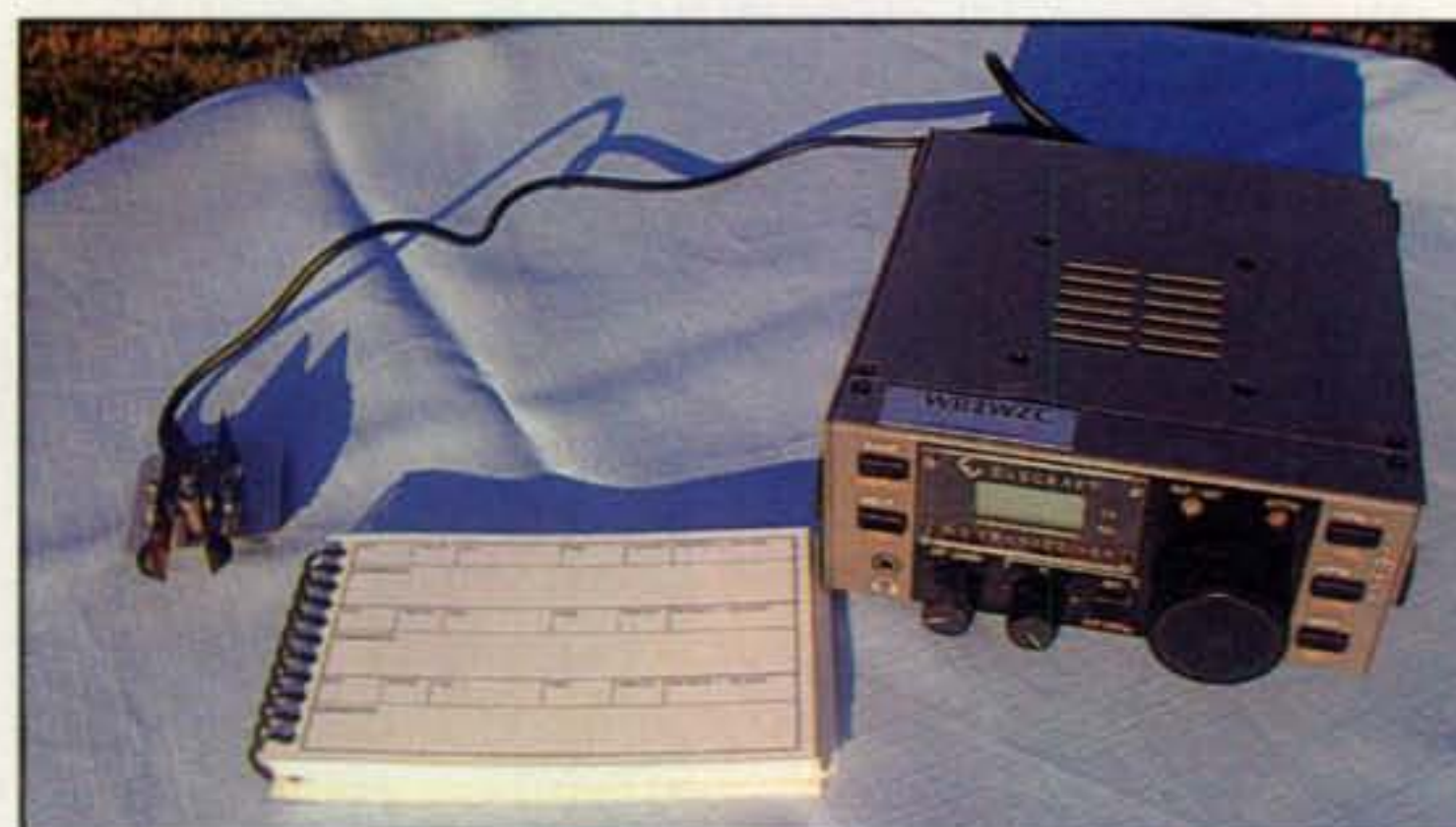
Photo 6— This "go-anywhere" setup of Andy Kabaskalian, WB2WZC, is perfect for Spartan Sprints, but its main attraction is the shirt-pocket-size (3 inch by 5 inch) waterproof logbook. It is made with synthetic paper, you can write on it with a regular pencil or ballpoint pen, and it stays clean and wrinkle free—even in the rain or snow. Details can be found at www.waterprooflogbooks.com .
