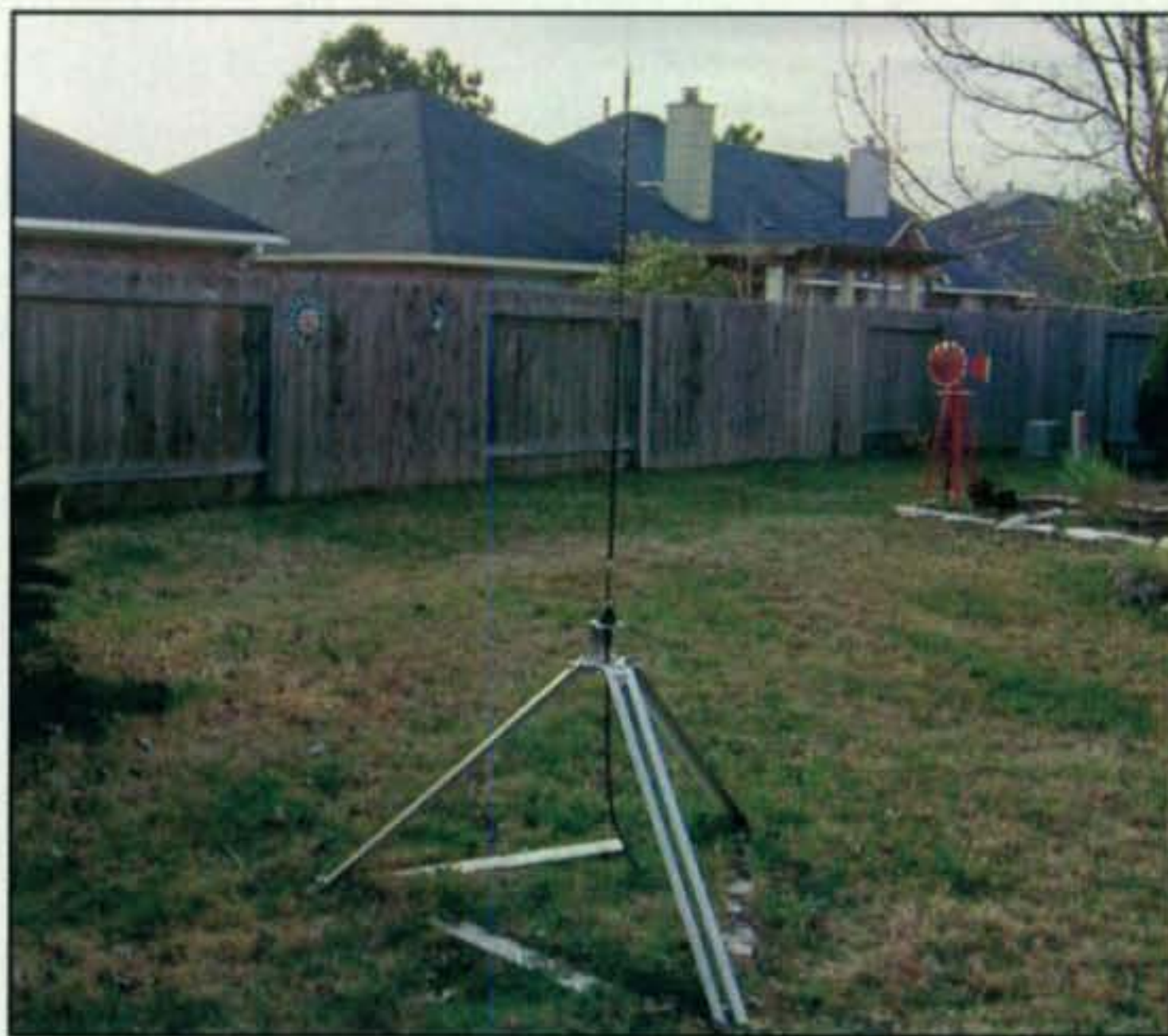
Photo 7— Don put his yard's privacy fence to good use in obstructing the neighbors' view of his vertical whip on the Outbacker Outpost mount/ground coupler. A quick step into the yard lets him swap whips to change bands. The red mini-windmill makes a nice decoy for inquisitive eyes. Again notice the clean skyline and exclusion of trees or utility lines in this highly restrictive community.
