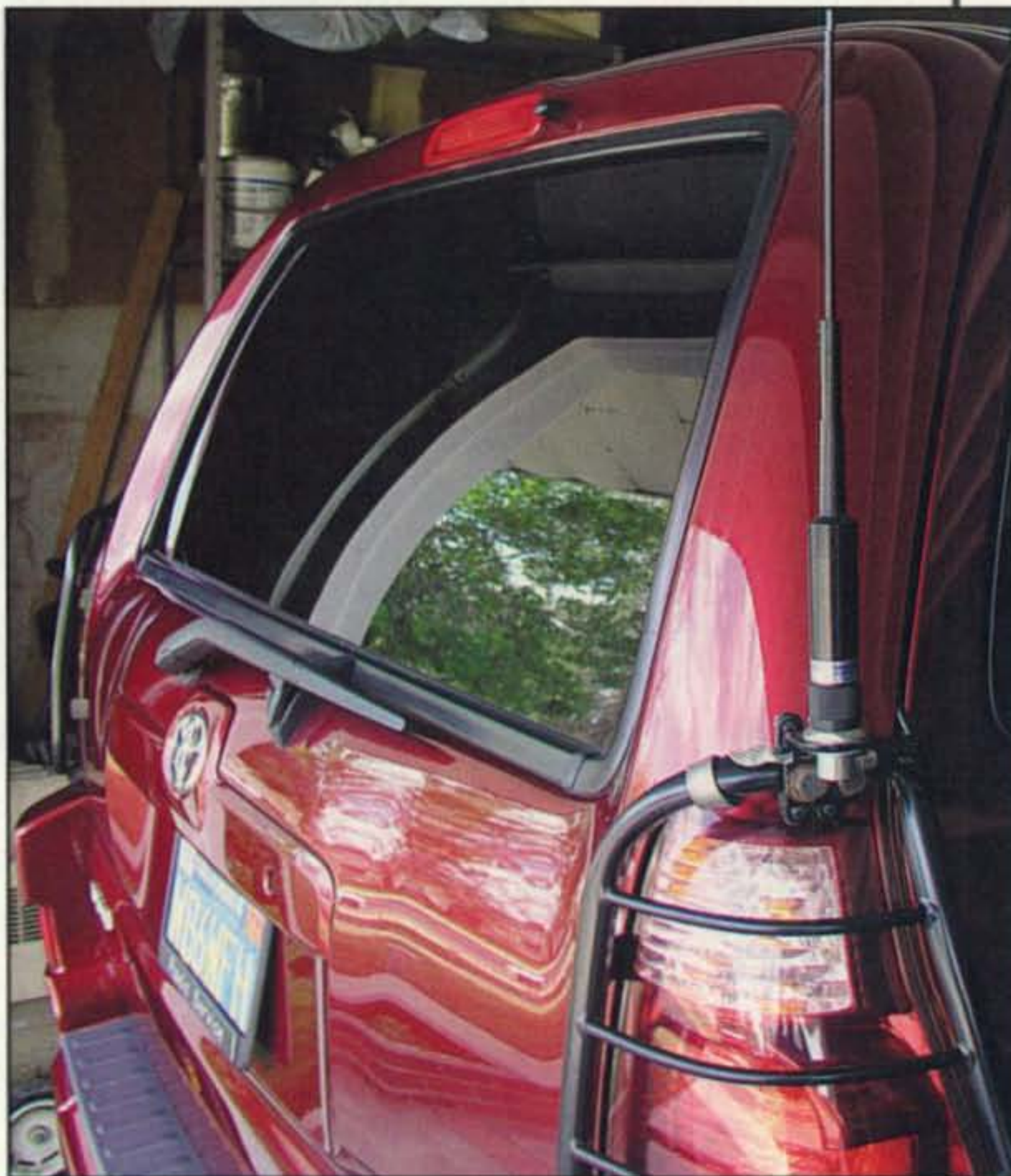
Rick, WB6WFH, saw accessory "brush guards" as a means to achieve an effective "no holes" antenna installation. While somewhat expensive at $150, they are attractive and useful as a light-duty antenna mount. (All photos courtesy of Rick Leyton, WB6WFH)
