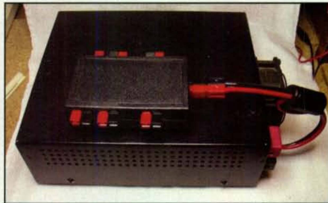
Photo B— The modified Astron SS-25 power supply with snap-on ferrite and MFJ-1106 distribution unit.
