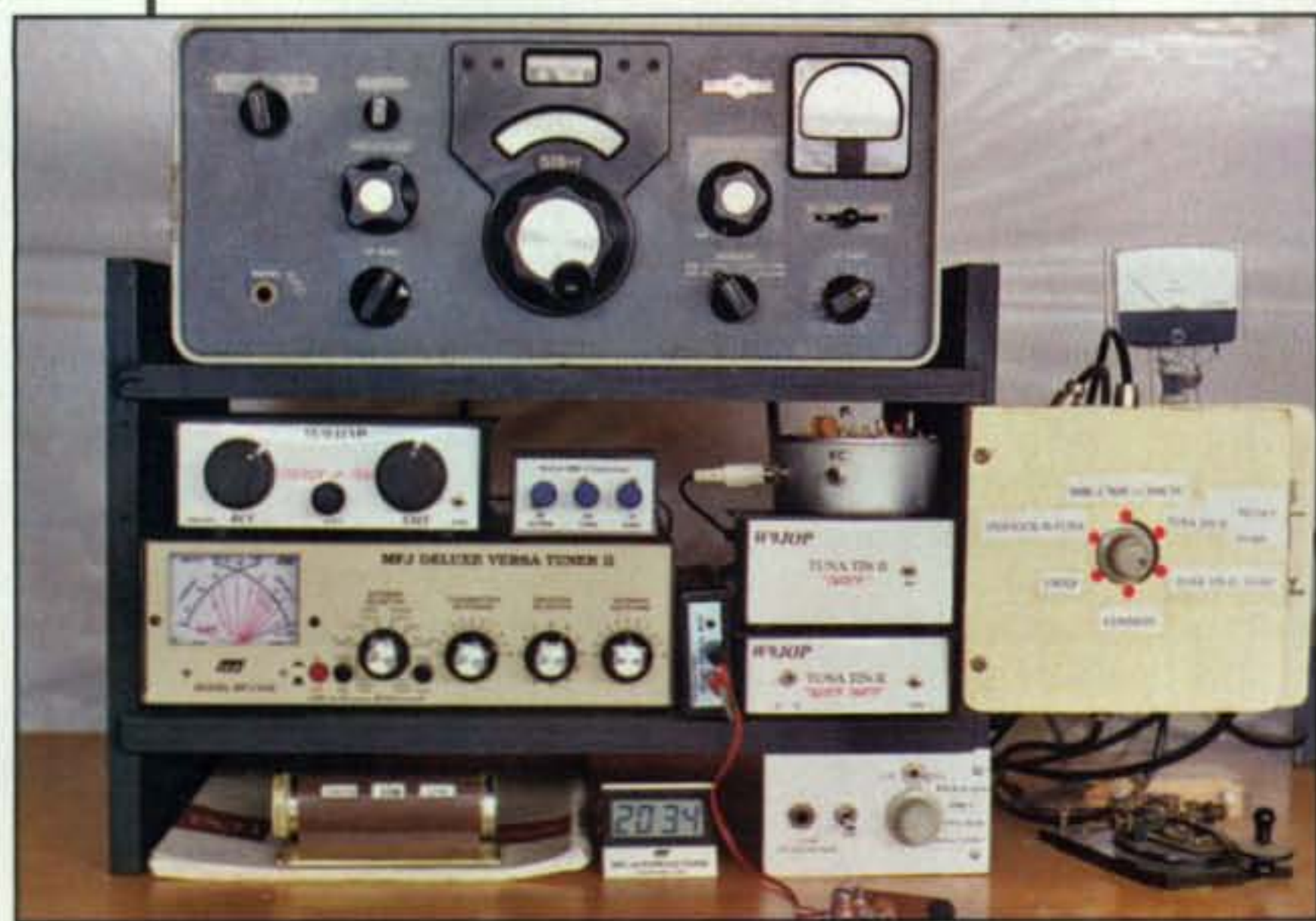
Photo 1— The "total QRP" setup Bob Chapman, W9JOP, used for Working All States with milliwatts of power. The receiver is a Collins 51S-1. The unit below it and atop the MFJ tuner on the left is a combination receiver and Tuna Tin 2 for 40 meters. The unit to its right is an SMK1 surface-mount kit transceiver. The three items to the right of the tuner are a round-can and two square-box Tuna Tin 2 transmitters. Stated mathematically, that's "Tins Times Four." (Photo courtesy of W9JOP)
