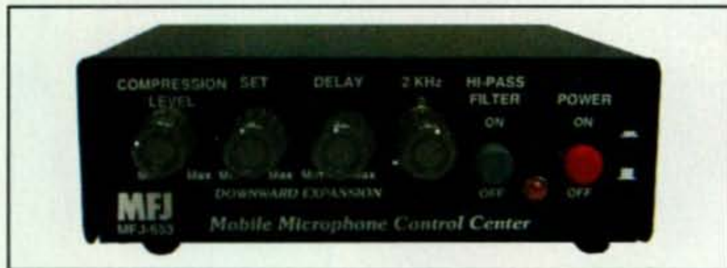
Photo C— The MFJ-653 allows you to tailor your transmit audio to improve readability on the end of your QSOs. (Photo courtesy of MFJ)
