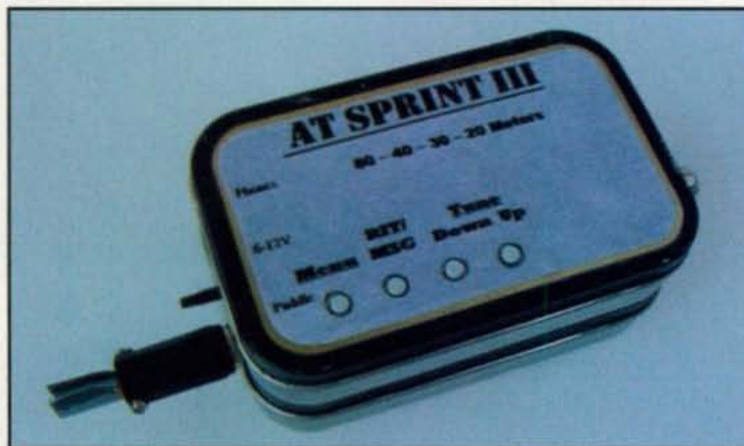
Photo 5— Dennis Payton, N9JXY, mounted his AT Sprint III rig in an Altoids tin and made a new label for the lid. He also modified the pushbuttons' positions for easy access with the lid closed, built a dual-lever paddle into the 3.5-mm plug, and added a second snap-off bottom tin to hold batteries and band modules. Three watts in a pocket. Nice! (Photo courtesy of N9JXY)
