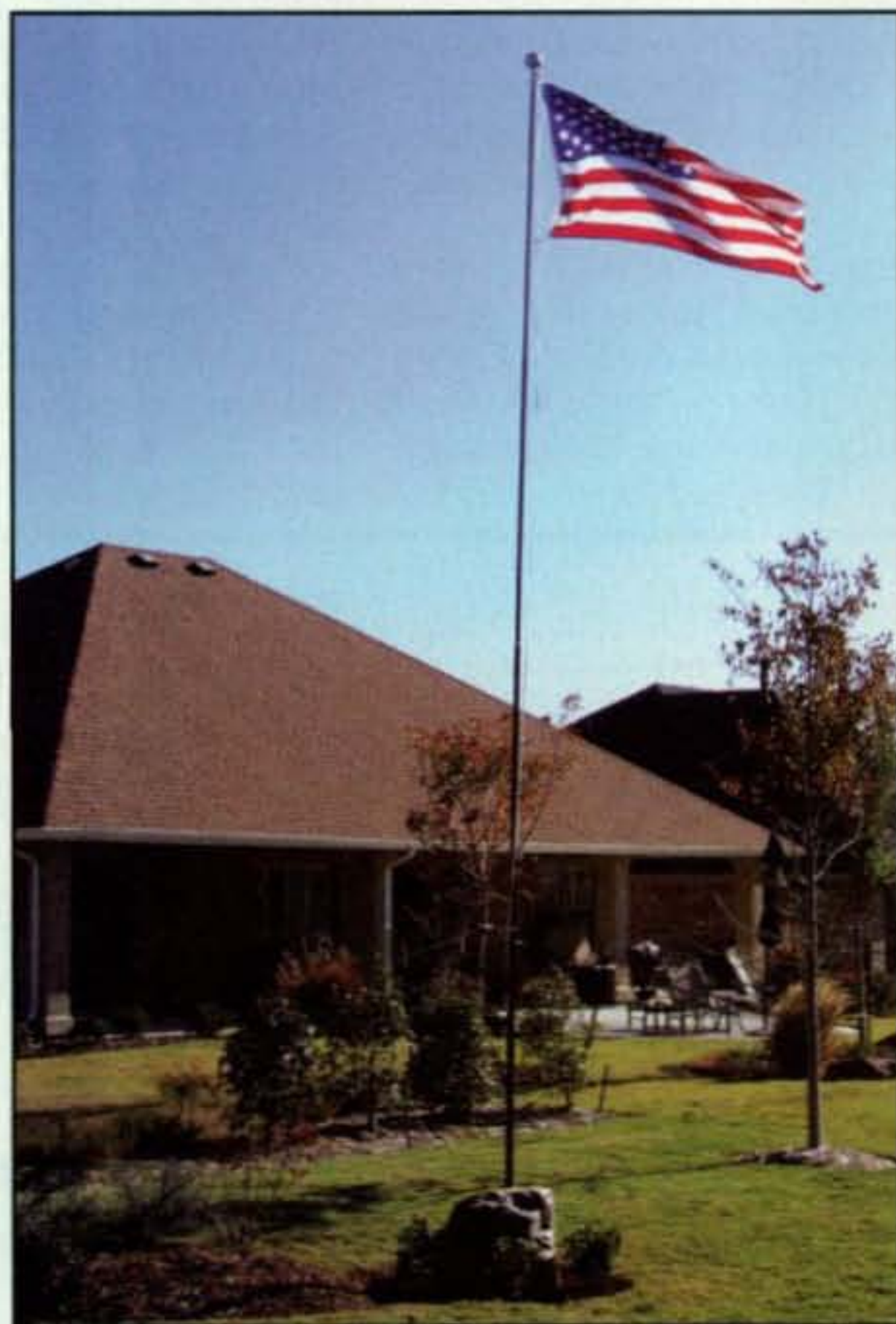
Photo 1— This first-class undercover antenna system devised by Bob Rumsey, KZ5R, almost qualifies for a neighborhood beautification award. The 17-foot SteppIR vertical is installed in the clear area between rows of adjacent homes and complemented with a full set of buried radials and disguised as a flagpole. Note the ultra-clear skyline without trees for supporting wire antennas and closely spaced homes that promote RFI problems. (Photos 1 through 5 courtesy of KZ5R)
