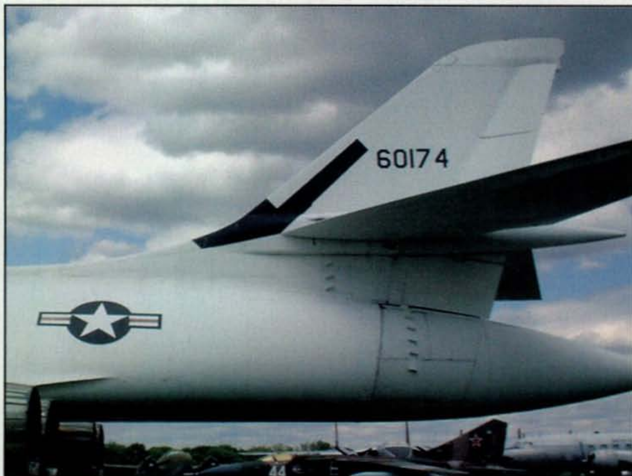
Photo 1— Tail section of the B1 bomber and its HF antenna (black area), as seen at the U.S. Air Force Museum in Dayton, Ohio.
