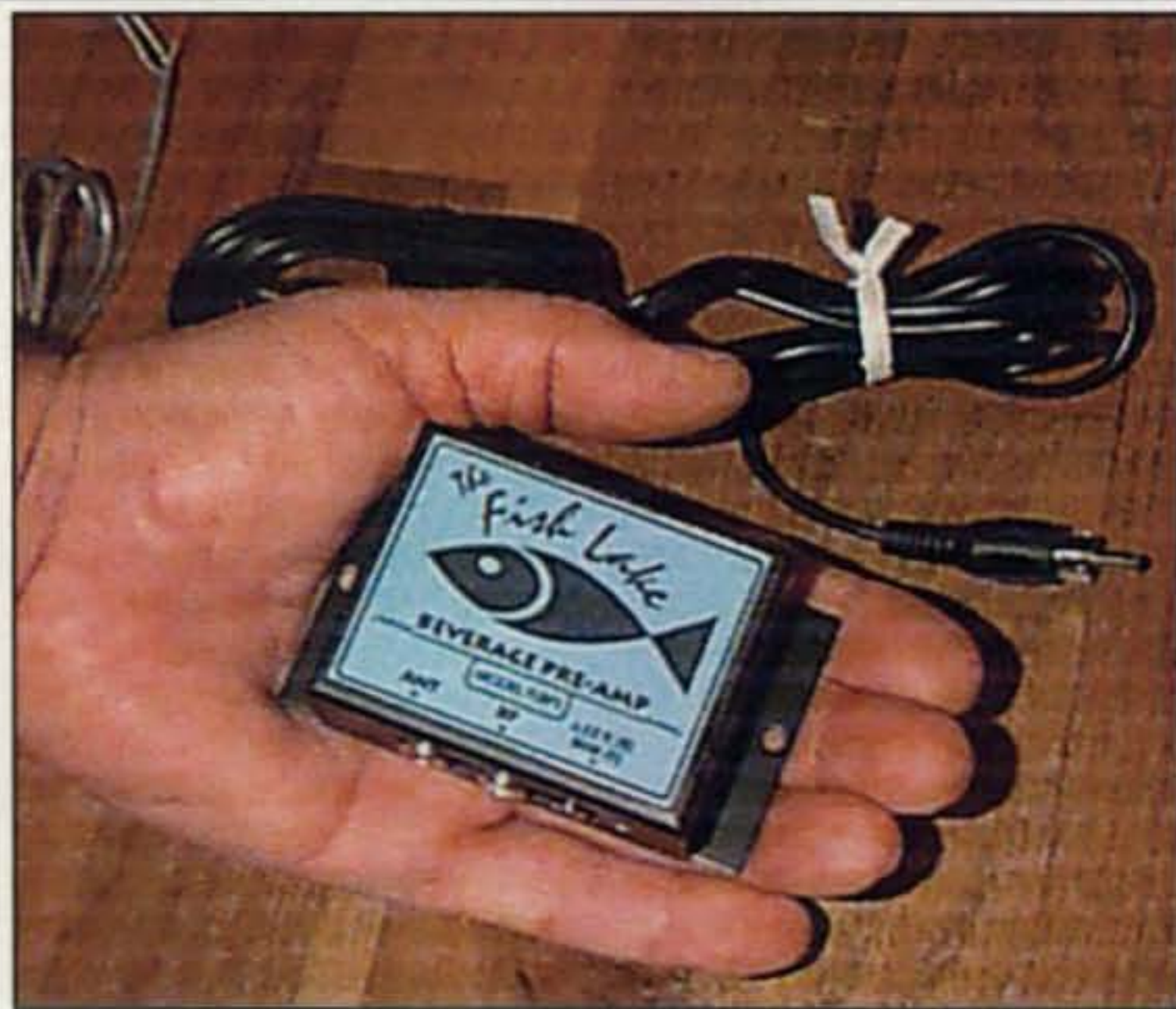
Photo C — The small size of the K8LV Fish Lake Beverage Pre-Amp (FLP1) is evident in this photo. (Photo courtesy of K8LV)
