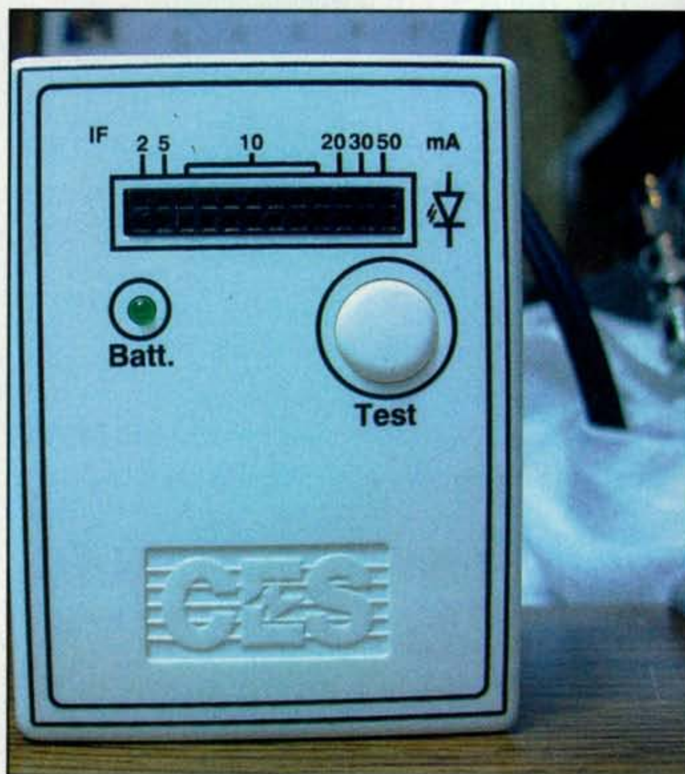
Photo A— An inexpensive LED tester permits you to easily determine LED polarity and brightness at different current levels.
