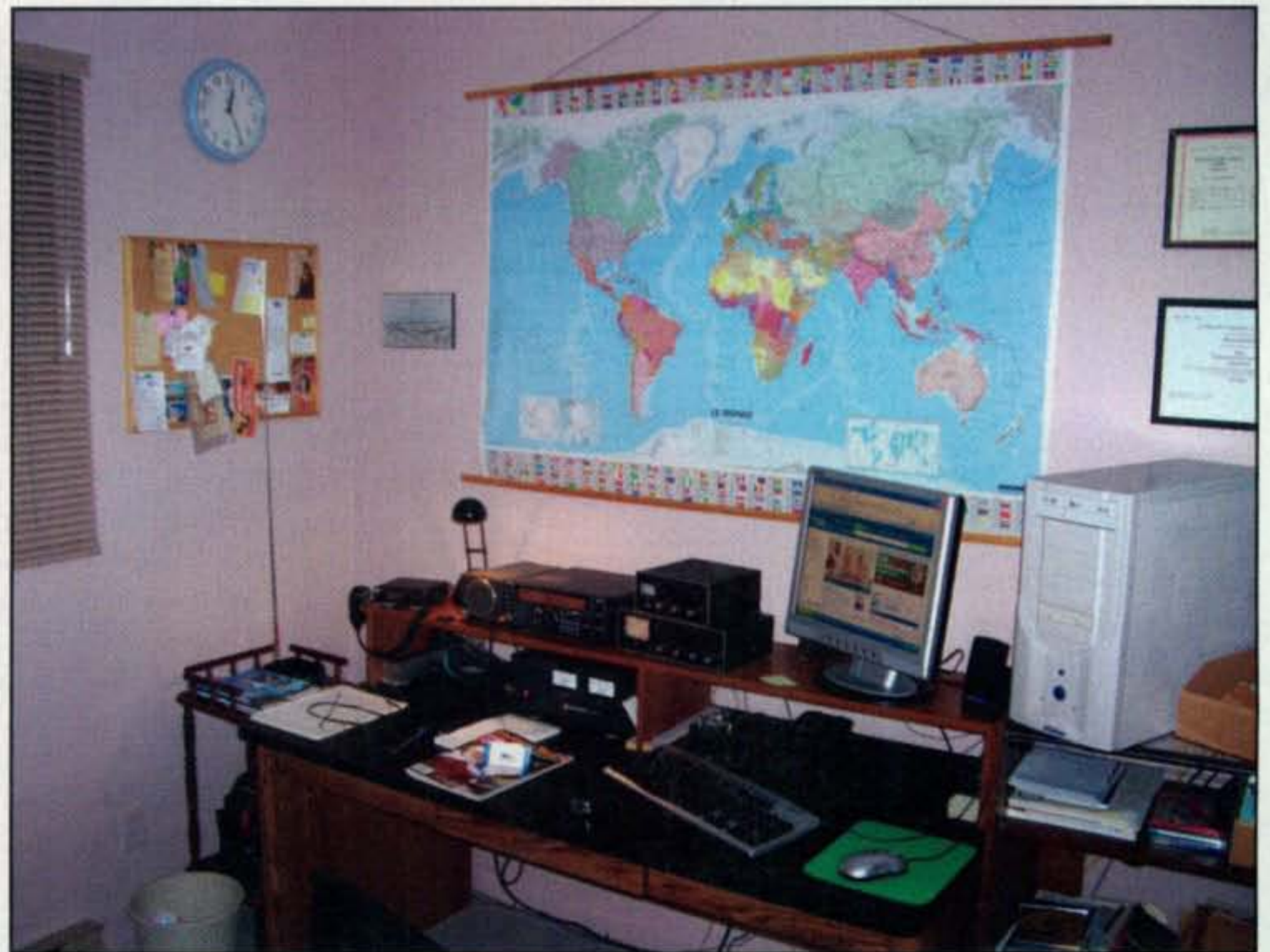
Photo G— Pierre's indoor setup consists of a Kenwood TS-570, an auxiliary tuner, an MFJ artificial ground, a 2-meter rig, and various other goodies. Home is where the ham gear is located! (Photo courtesy of VE2OPB)
