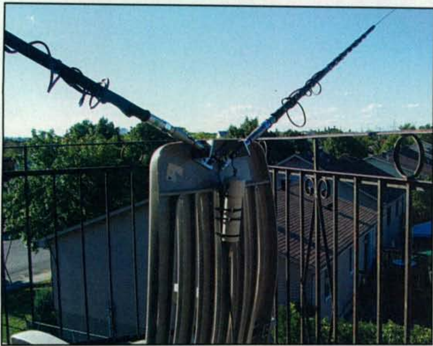
Photo E— Pierre Bordeleau, VE2OPB, lives in a condo with nothing but a balcony to install an antenna. What to do? He devised a mount for two multiband Outbacker mobile whips, installed it on a patio chair, and added a balun at the feedpoint. The balcony is up four floors and overlooks the neighborhood, so the antenna radiates a good signal in unobstructed directions. (Photo courtesy of VE2OPB)
