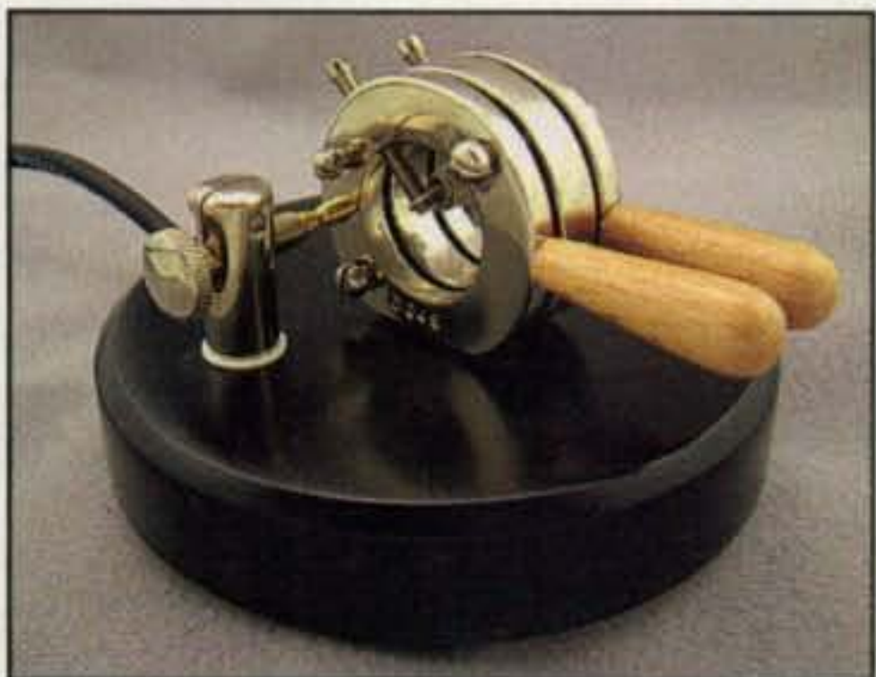
Photo 8— Shifting size while continuing the round-base key theme, we find this intriguing dual-lever paddle Morse Express owner Marshall Emm, N1FN, uncovered at the Friedrichshafen Convention (Germany) in 2004. It's all circles—right down to its round "broomstick" fingerpieces! (Photo courtesy of N1FN)
