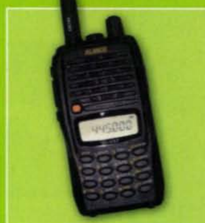
DJ-V47 4.5 WATT 440 MHz Frequency range: TX 430 - 449.995MHz RX 410 - 470MHz approx
