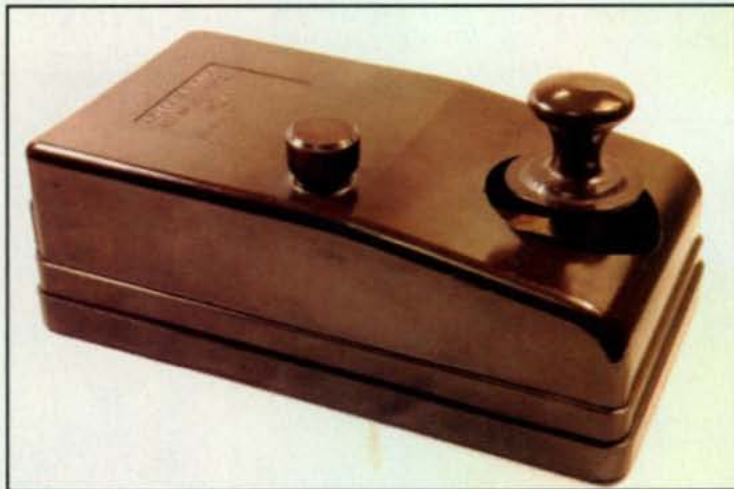
Photo 11—Ray Jacob, W2RJJ, was using this WW II British Air Ministry key when I contacted him recently, and he cheerfully shared a picture for inclusion in this column. The overall case design leads me to think it was a forerunner of the famed NATO keys. (Photo courtesy of W2RJJ)
