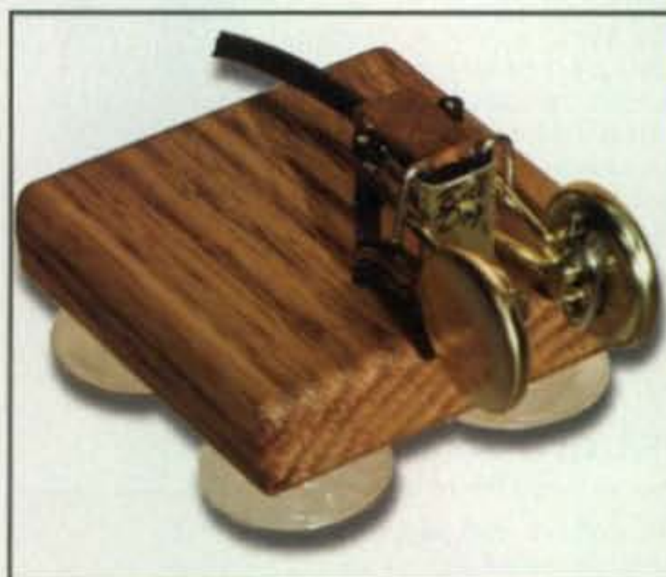
Photo 6— Louis Petkus, K9LU, makes this miniature iambic paddle from a modified bulldog paper clip. It is rugged, reliable, economically priced, and handles remarkably well for such a small key. It is also silent in operation, so it is ideal for times when you operate quietly and use earphones. You can order one at www.bulldogkey.com .
