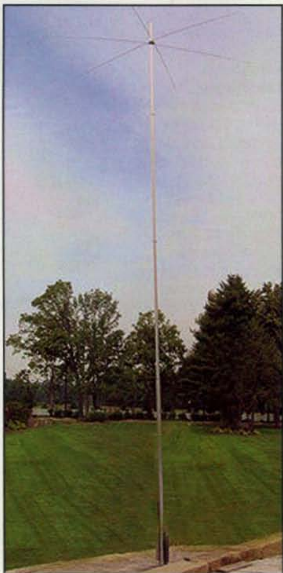
Photo B—DX Engineering's 40VA-1 is a monoband 40-meter vertical antenna. Note the top capacity hat, which allows the antenna to provide good performance on 40 meters with only 24-foot height. (Photo courtesy of DX Engineering)
