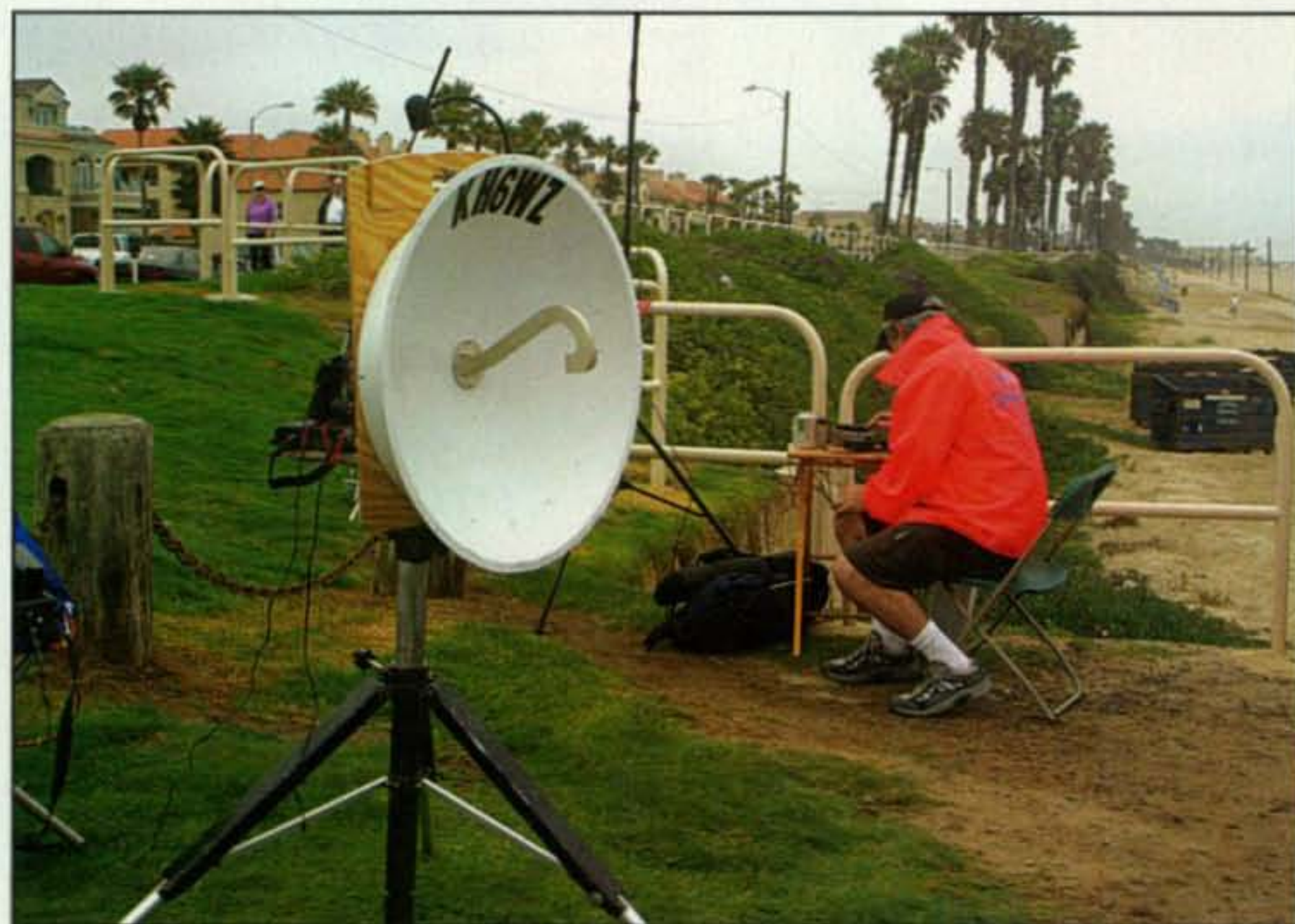
Photo 4— Microwave rigs can look very suspicious. Here is my 10-GHz rig set up in Huntington Beach, CA, the ARRL Orange section.
