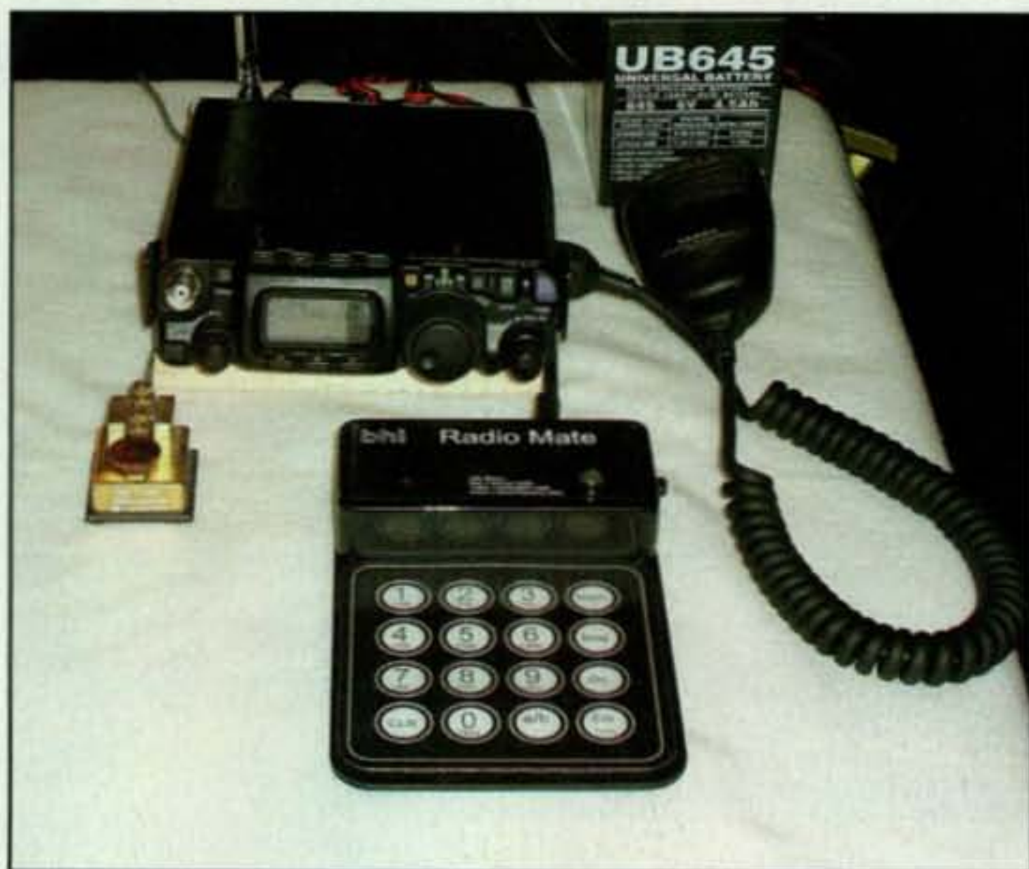
Photo 1— The Radio Mate makes the small buttons on the Yaesu FT-817 easier to deal with.
