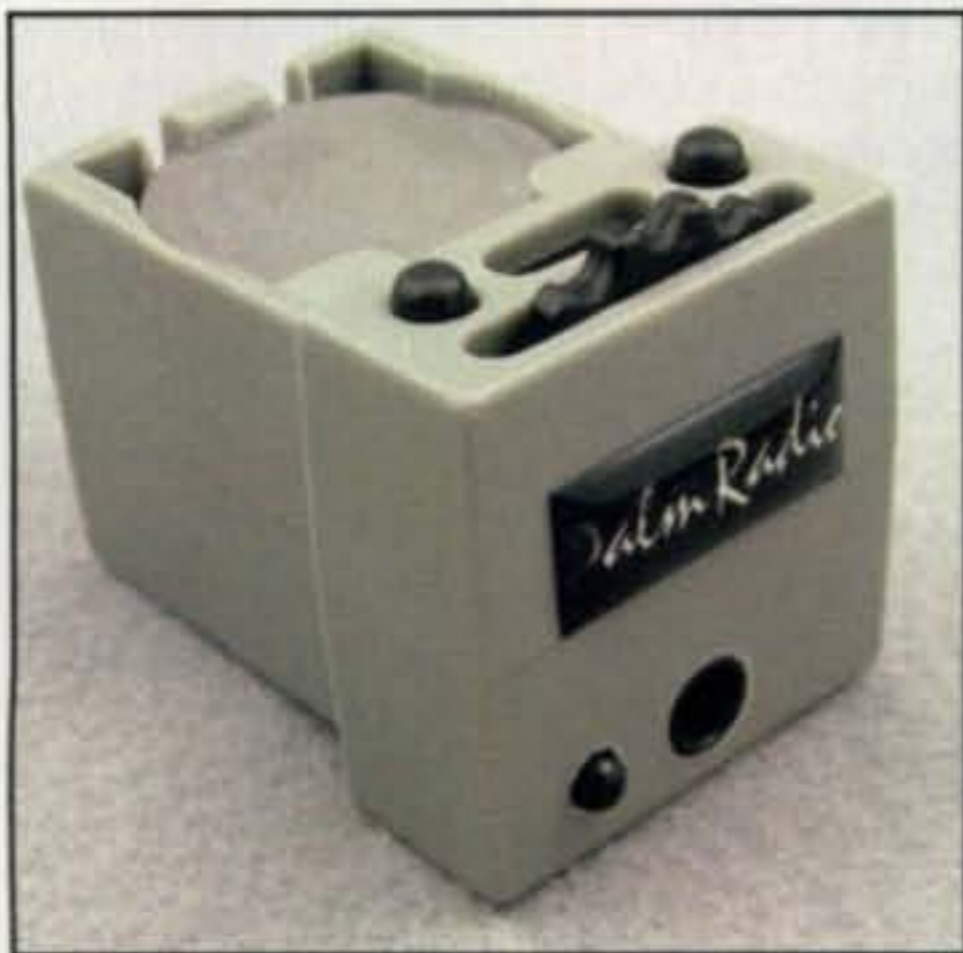
Photo 8— This one-inch cube is a plug-in electronic keyer for the Palm Mini Paddle, and it includes a wireless infrared link to its connected/unconnected transceiver. The keyer has a built-in battery (at rear), and "toothy" speed control (near front). A similar infrared LED-type transmitter is available for the Palm Radio Pump Key. (Photo courtesy Morse Express)
