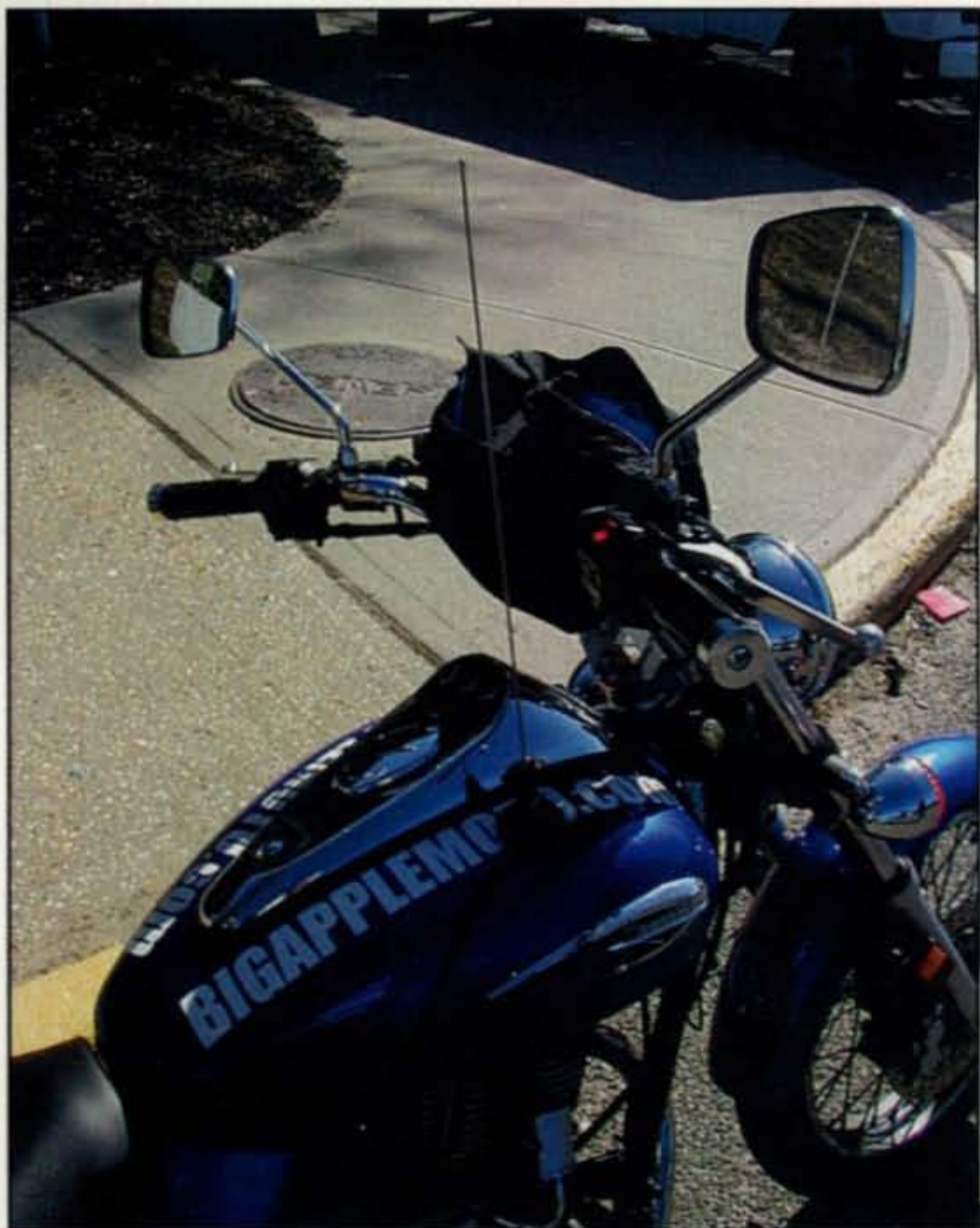
Photo D— A quarter-wave mag-mount antenna was attached to the top of the motorcycle's fuel tank.
