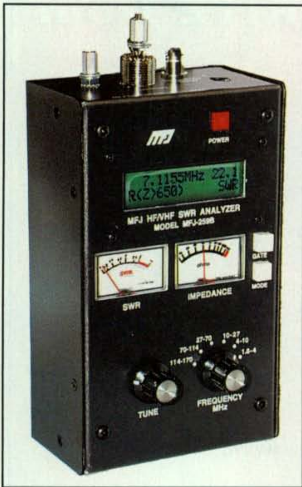
Photo C— The ever-popular MFJ-259B Antenna Analyzer measures resonant frequencies, impedance and resistance of antennas, plus coax-cable link losses, faults, etc. The unit covers 1.8 to 170 MHz and indicates SWR and impedance on separate meters plus resonance frequency and inductive/capacitive reactance on its LCD panel. It is self-contained and battery powered, so you can pre-tune an antenna before even switching on your transceiver. (Photo courtesy of MFJ Enterprises, Inc.)
