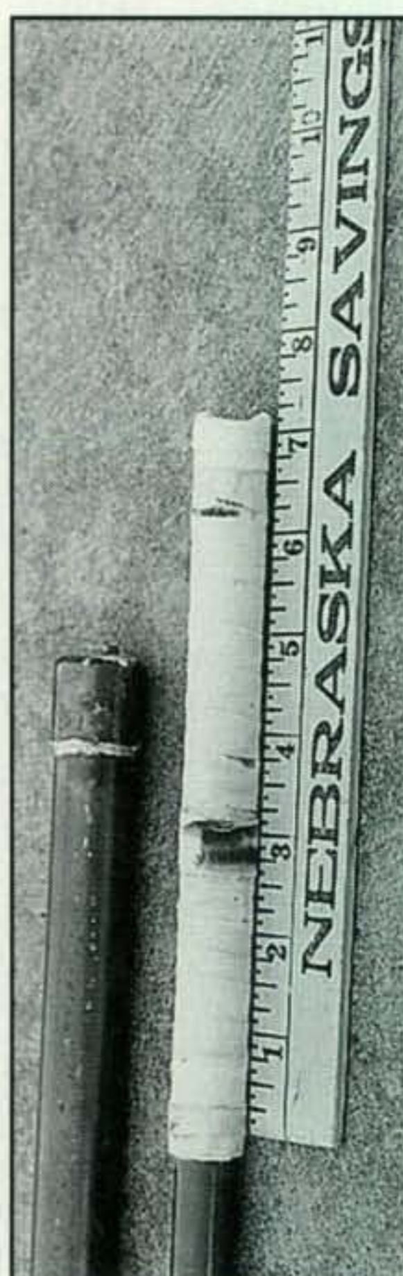
Photo C—Close-up of the prepared inner tube.
