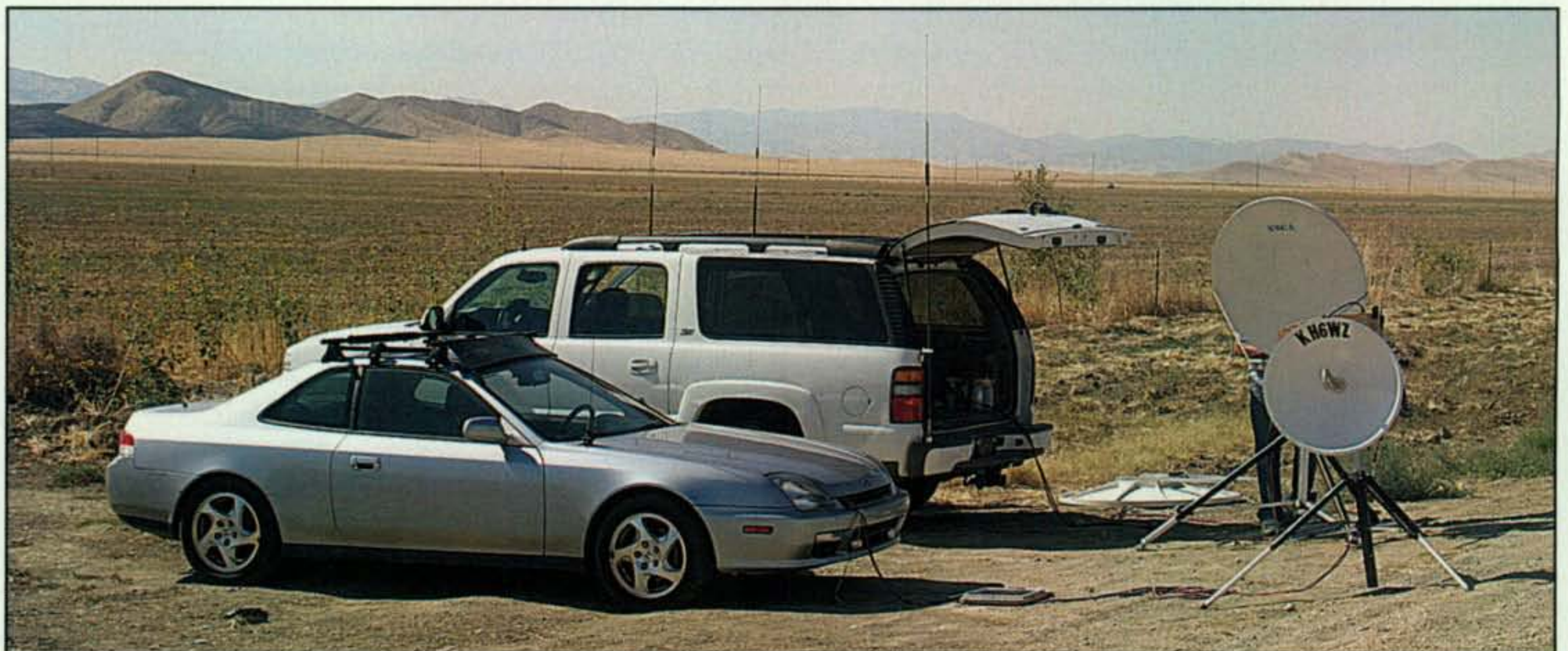
Photo 4— A portable power cable sticks out from the front of the car to feed two portable radio systems. Just park the car and plug in the gear!
