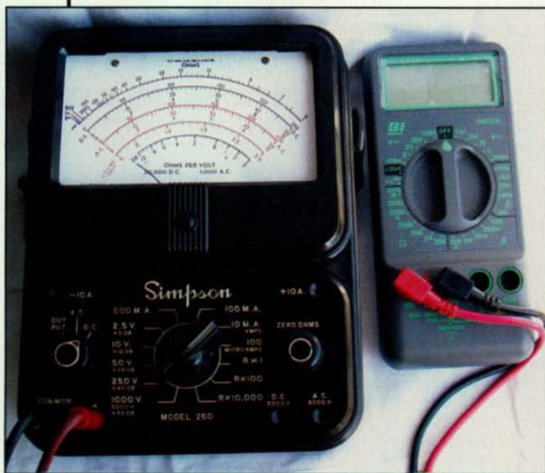
Photo A— Two easily recognized examples of Volt Ohm Meters are the ever-famous (and analog-type) Simpson 260 meter (left) and the Beckman DM-15XL digital-type meter (right). I am partial to the Simpson, as my father designed the original burnout-proof model 260.
