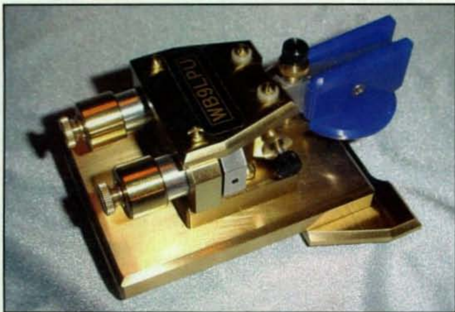
Photo 4— Richard, WB9LPU, also designed and made this beautifully crafted "PaddleKey," and it is totally unique. The paddle's arm pivots on a double stack of three ball bearings and moves left and right to function as a single-lever paddle or moves up and down to function as a hand key. It uses two cables to connect to a rig's key and paddle sockets. (Photo via WB9LPU)
