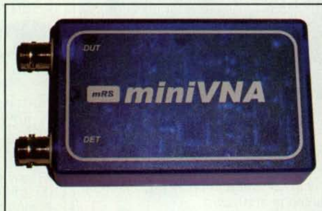
Photo D— The new miniVNA software-defined antenna analyzer is available from < www.w4rt.com >. The unit connects to a computer and antenna and displays your selected parameters (sweep range, SWR, 2:1 bandwidth points, etc.) on the monitor's screen. (Photo courtesy of Barry Johnson, W4WB)
