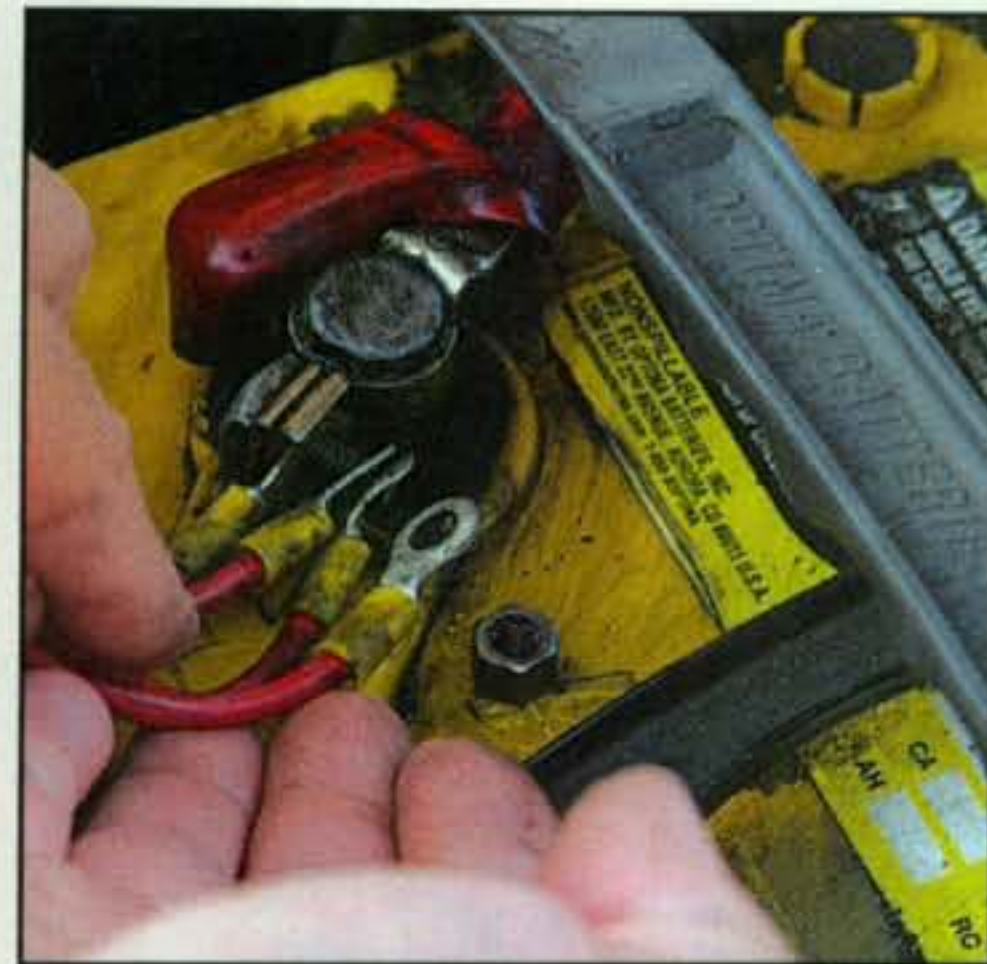
Photo 11— The battery end of the cable terminates with four ring terminals which mount onto the 10-mm battery-post terminal bolts. This is a secure way to attach a wire to a car battery.
