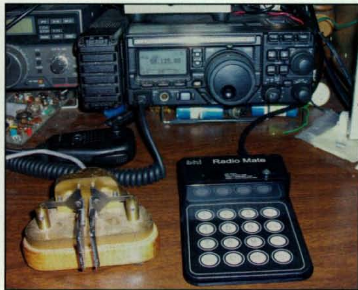
Photo 2— Button size isn't as big a problem on the FT-897 as on the 817, but the Radio Mate is able to make some of the more commonly-used functions much more accessible.
