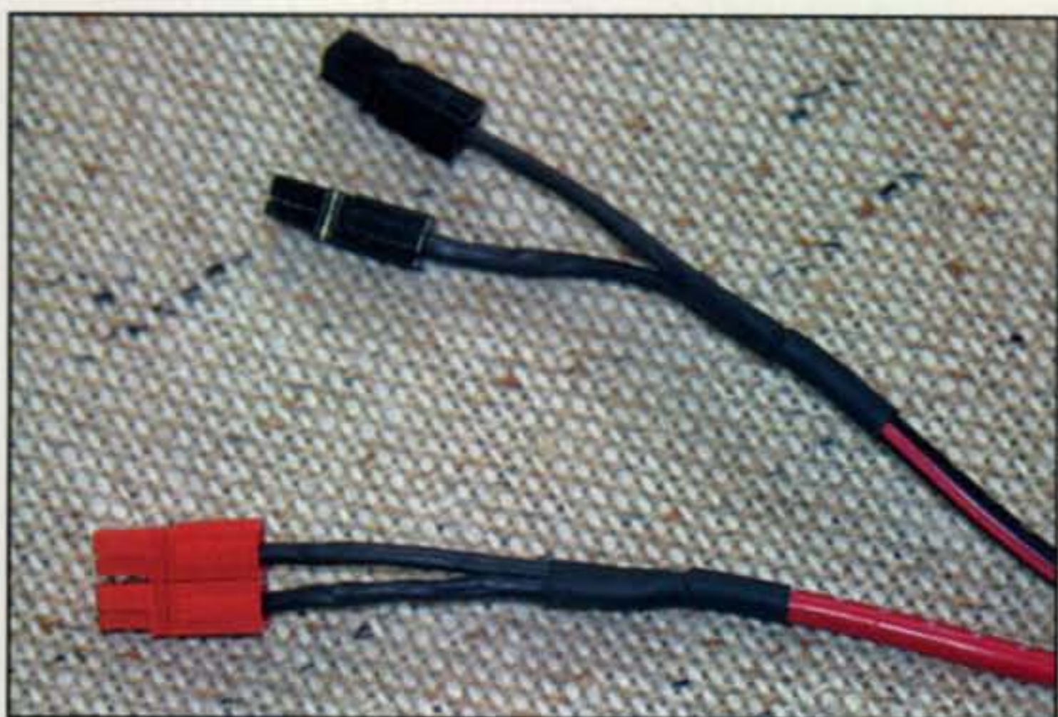
Photo 7— Snap on the plastic housing.
