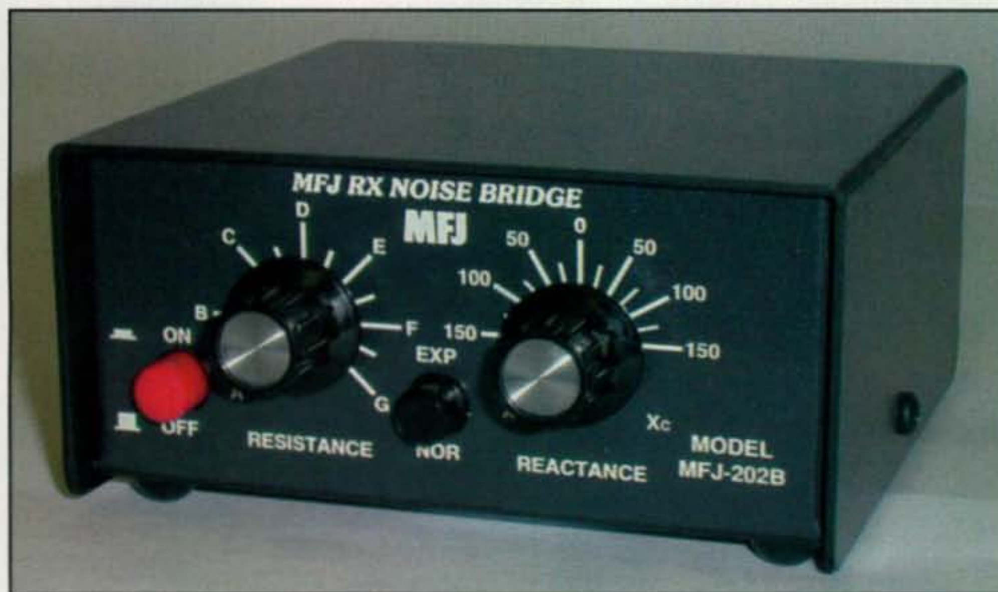
Photo B— This affordably priced MFJ-202B Noise Bridge works in conjunction with an HF transceiver to measure an antenna's resonant frequency, resistance, and capacitive or inductive reactance. Since it is small and affordably priced, some folks call it "a poor man's antenna analyzer."
