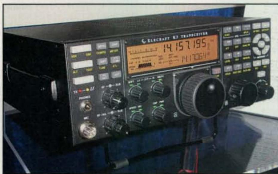
The Elecraft K3 introduces a new concept in kitbuilding ... and lets you use a keyer paddle to send RTTY and PSK-31 without a computer! (Photos by W2VU unless otherwise noted)
