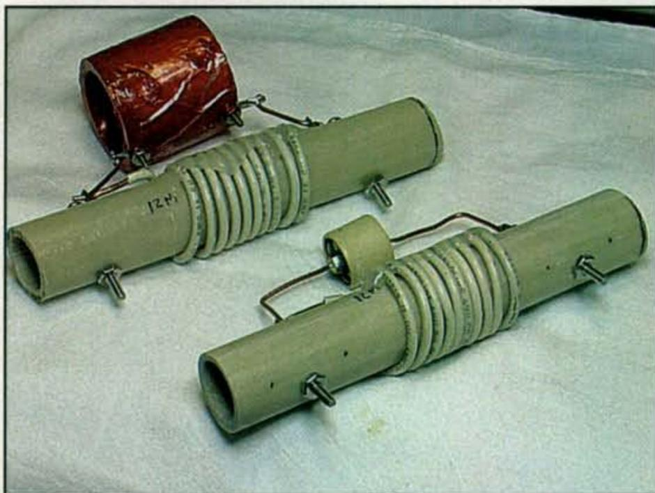
Photo B— Two 12-meter traps, one (top) with the homebrew capacitor and the other (bottom) with a doorknob capacitor.
