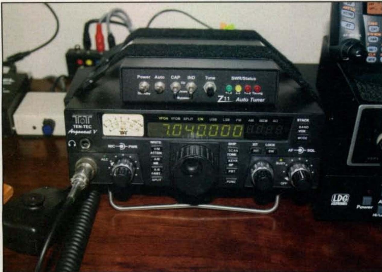
Photo B— The indoor setup of W4MQC reveals an ever-popular Argonaut V transceiver with an LDG Z11 auto tuner plus a few smooth-handling CW keys for flavor. Very nice! (Photo courtesy of W4MQC)
