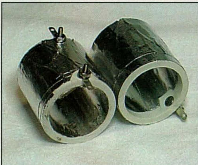
Photo A— Homebrew capacitors showing the inside/outside screw contacts.
