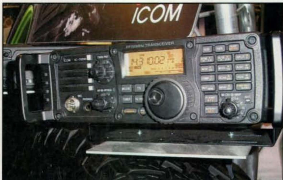
*The truck tire is not where ICOM recommends that its new IC-7200 transceiver be mounted. It's part of the display to convey an image of toughness for this entry-level HF/6-meter rig.*
