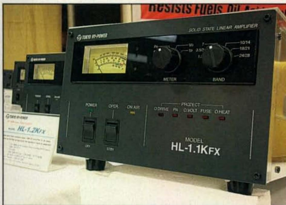
This year's newest entries from Tokyo Hy-Power are the 600-watt solid-state HL-1.1Kfx HF amp shown here, plus the 45-watt HL-45B designed for use with Yaesu's low-power FT-817.
