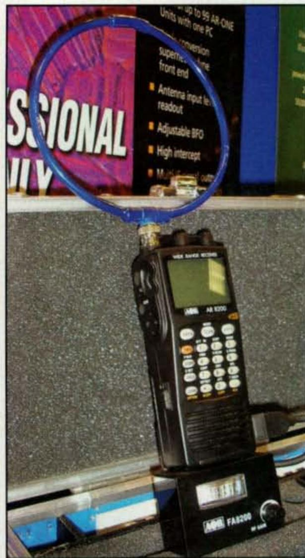
The FA-8200 from AOR is a specialized foxhunting setup for tracking aircraft emergency locator transmitters.
