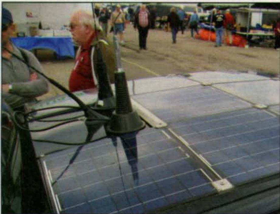
Photo 6— The roof and hood of Bob Bruninga's Prius are put to work gathering sunlight to charge the batteries, perhaps posing at least one good response to \$6.00 a gallon gasoline.
