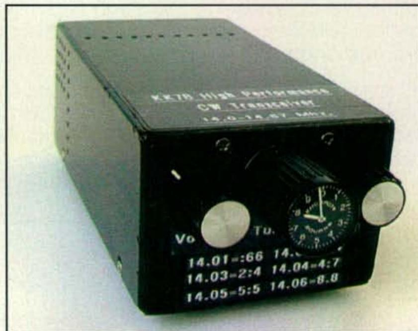
Photo E— Check out this "High Performance CW Transceiver" built by Dennis Payton, N9JXY. It covers 20 meters beautifully, and the main tuning knob and control are multi-turn Bourne Electronic items with clock or altimeter-type hands for precise readout. Cost of the knob and control? Don't ask! (Photo courtesy of N9JXY)
