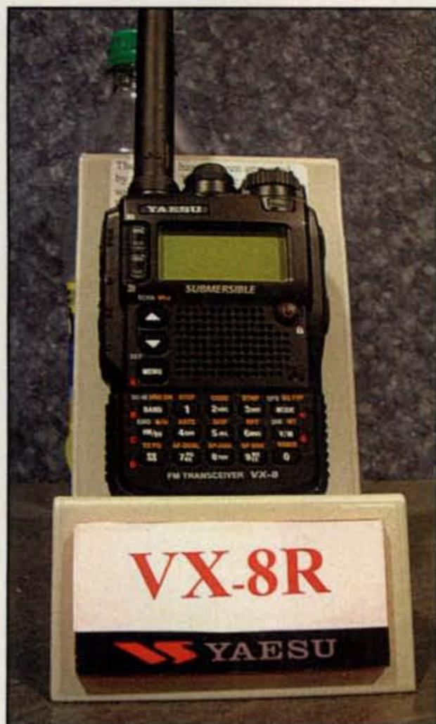
The only new handheld transceiver introduced this year at Dayton was the triband Yaesu VX-8R, which appeared only as a prototype. It will cover 2 meters, 222 MHz and 440 MHz, with additional features that are yet to be finalized.
