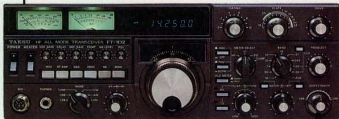
Photo A— Older model HF transceivers such as this impressive-looking Yaesu FT-102 are often available at an attractive price, but do a thorough checkout before purchasing. If repairs are necessary and beyond your expertise, your overall investment may exceed that of a new "economy" model transceiver. Performance of newer transceivers with their high-tech circuitry is also better than that of older transceivers.
