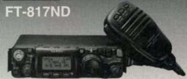
The Yaesu FT-817ND is an improved, deluxe version of the hugely popular FT-817. It includes 60 meter coverage plus the new high capacity FNB-85 battery. The radio is a fully self-contained, battery-powered, low power amateur MF/HF/VHF/UHF transceiver. Great for portable QRP operation!
