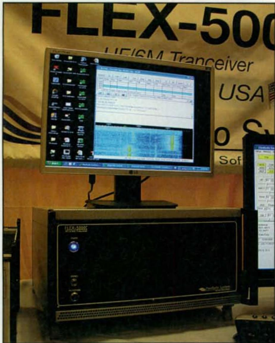
*FlexRadio's Flex-5000C software defined radio includes a built-in computer and now has an option for a second receiver that can share the screen with the primary one.*
