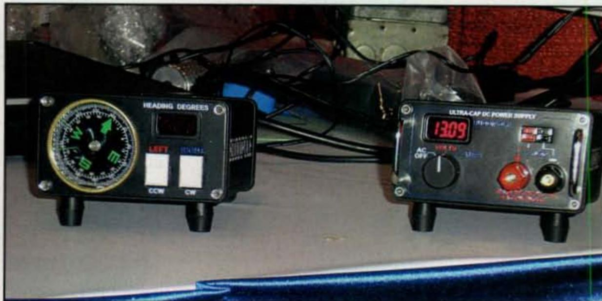
Two new accessories from Buddipole Antennas are a mini rotor control (left) and a mini 40-amp power supply (right) that uses an ultra capacitor to store power.
