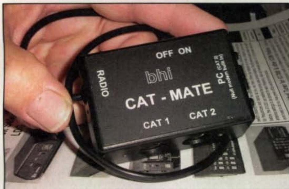
The CAT MATE from bhi, Ltd., is an electronic "Y" splitter that lets you use two devices through the computer port of certain Yaesu transceivers.
