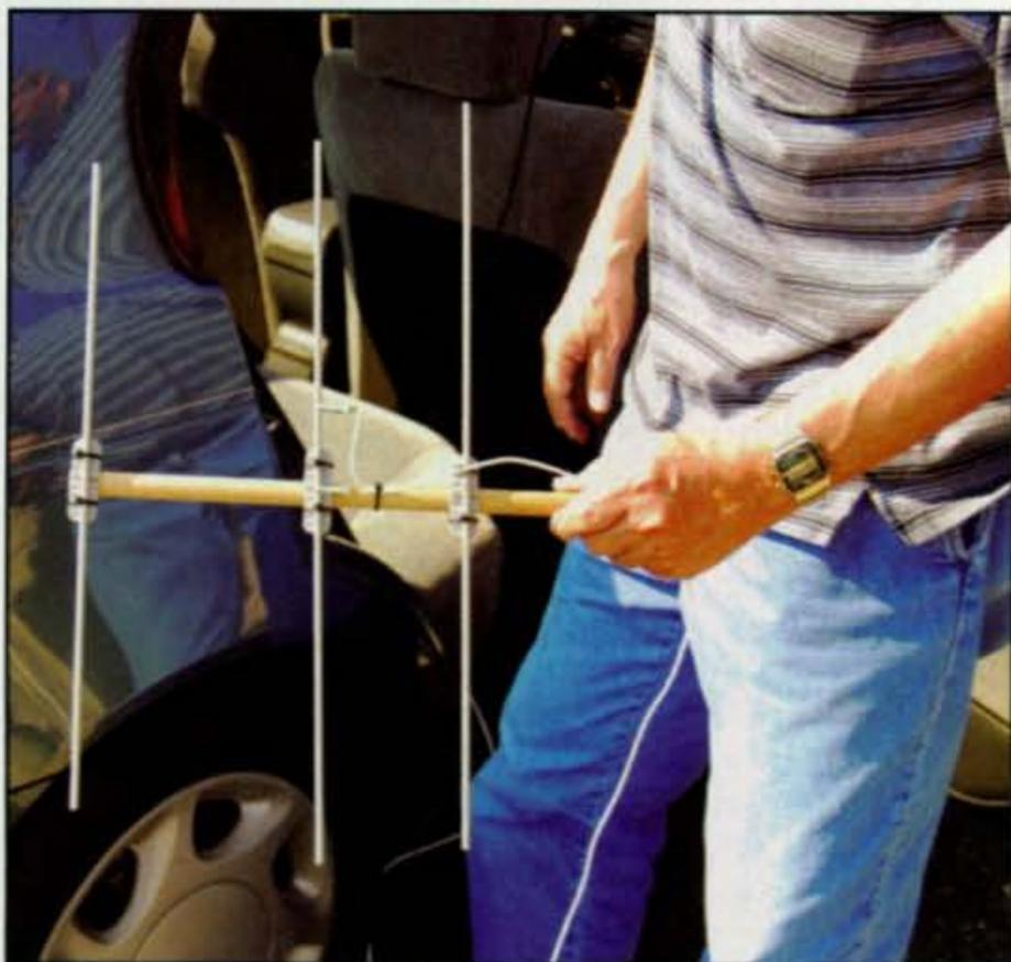
Bob Rex, K3DBD, built an antenna for finding signals at the remote key operating frequency of 315 MHz. In the course of normal "fox hunting" activities, you just track down a signal on an amateur radio band, such as 2 meters. In this case, hams had to identify the exact frequency and then build the antenna to match it. (Photo courtesy of Jim Toth, K3CHJ)
