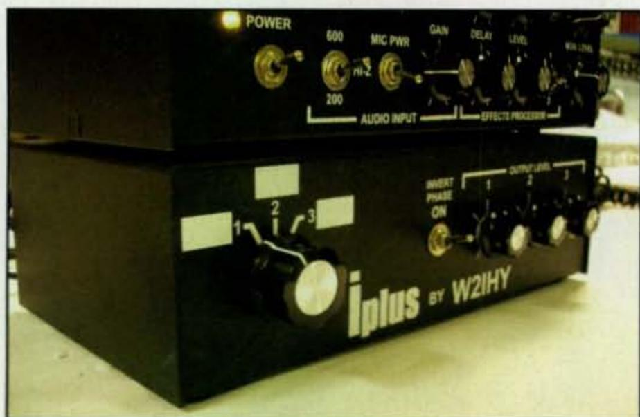
W2IHY's iPlus audio switch lets you consolidate audio gear through this one box to feed as many as three different radios with the flip of a switch.
