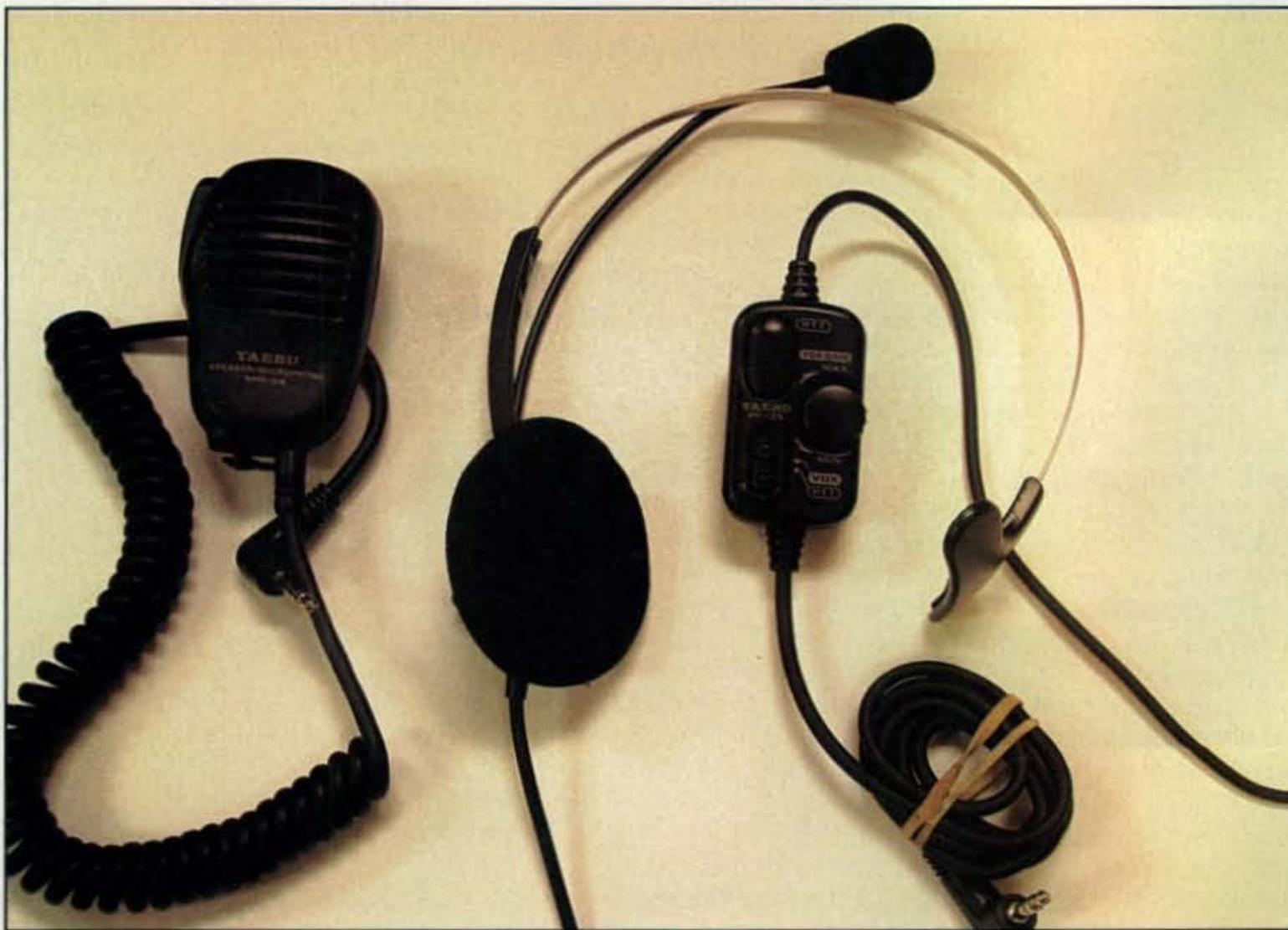
Handy accessories for HTs include the speaker-microphone (on the left) and the boom-microphone headset. When using a speaker-mic, try not to crank up the volume too high. The headset enables hands-free operation, but should be used in the PTT mode (see text).
