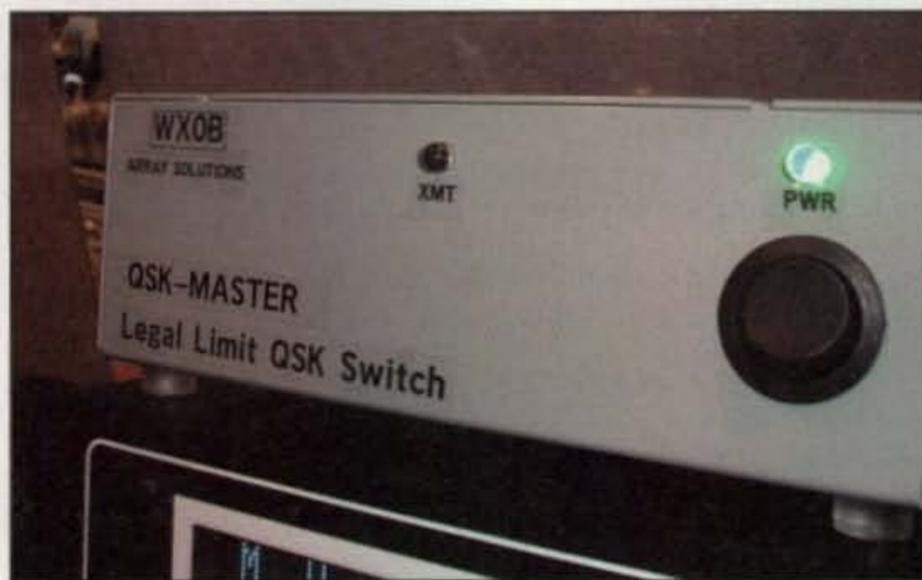
*The QSK-Master, one of several new products from Array Solutions, allows any radio/amplifier combination to use full break-in keying (QSK), even if the units weren't designed to work together.*
