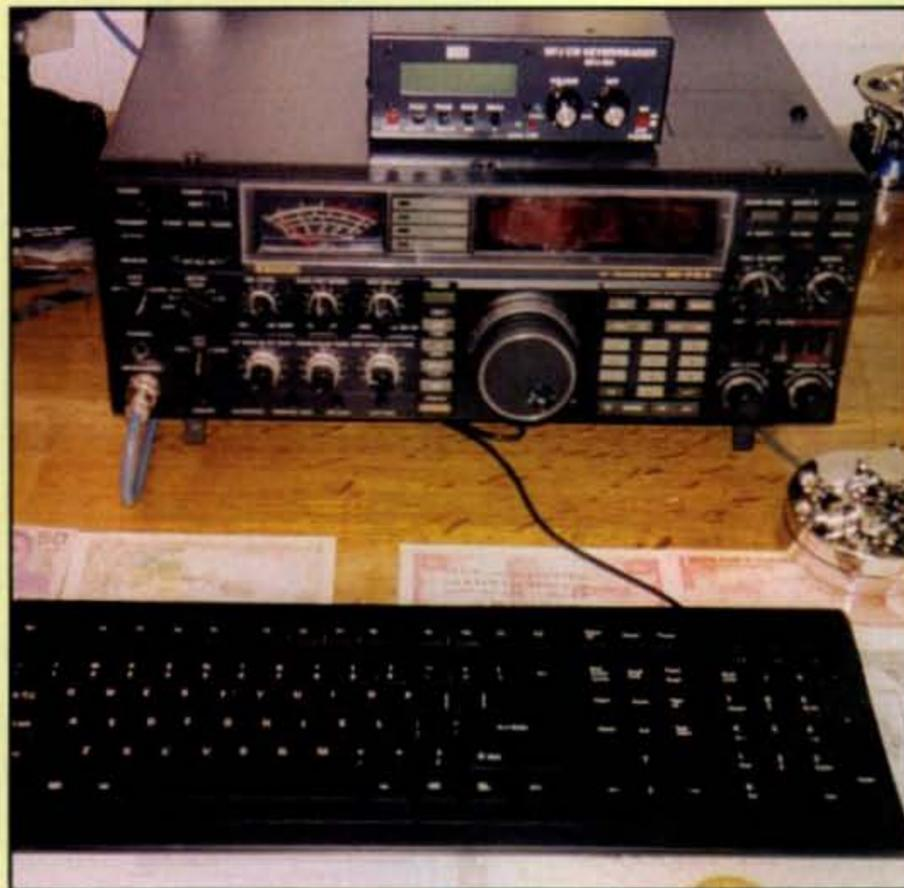
*An MFJ-464 Morse code reader/keyer is usually set atop a station transceiver so you can watch its "code lock" LED and Morse read-out while tuning in signals. A keyboard for transmitting your own CW messages plugs into the socket on the rear of the MFJ-464. If preferred, you can also use a paddle for transmitting CW messages in real time or for loading memories for instant pushbutton replay.*
