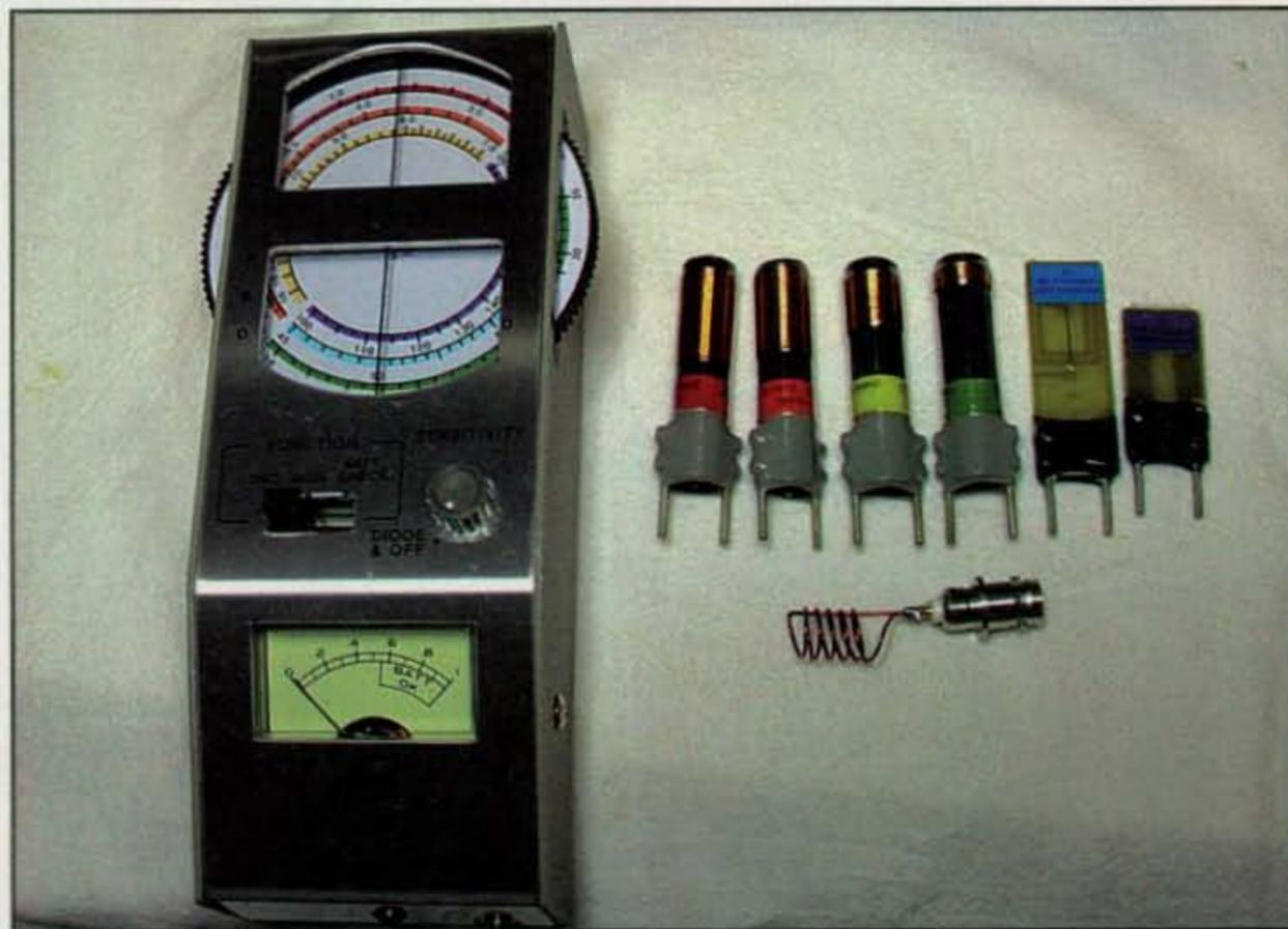
Photo B— The MFJ-201 grid dip oscillator.
