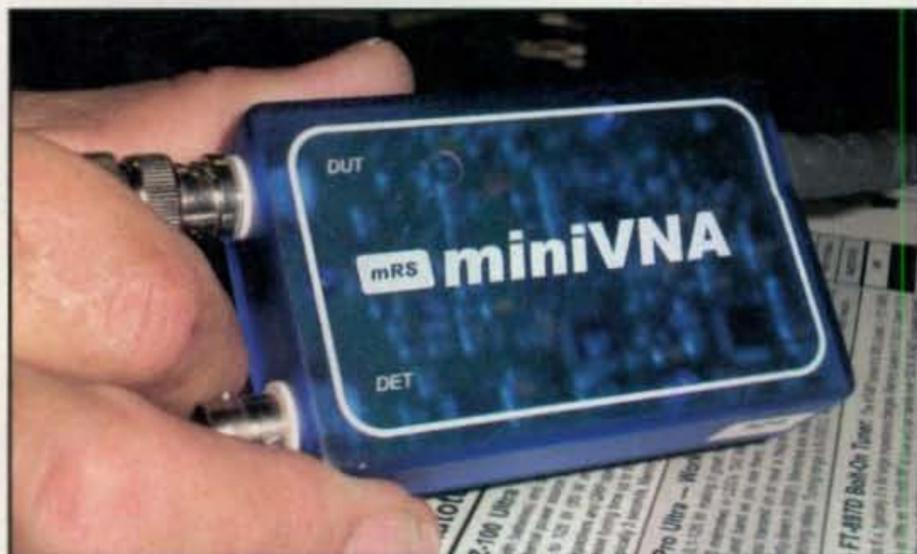
The miniVNA from W4RT Electronics, plus your own computer, gives you the power of a professional-grade network analyzer at a fraction of the price.
