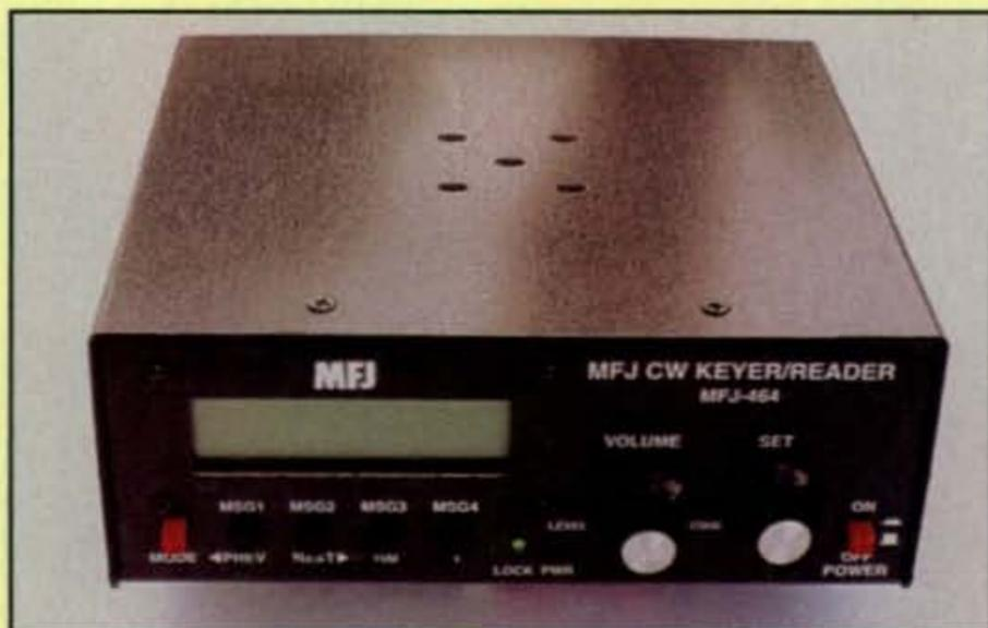
*Need a little help learning Morse code for copying off-the-air CW? Would you like the ability to send CW from your own keyboard-type messages? This MFJ-464 Morse Reader/Keyer does both. Just connect it to the speaker and key sockets of your transceiver, plug a computer keyboard into it, tune to the CW portion of a band, and read code as it is displayed on the MFJ-464. It is not a substitute for knowing code, but it is a good "crutch" when coming up to speed.*
