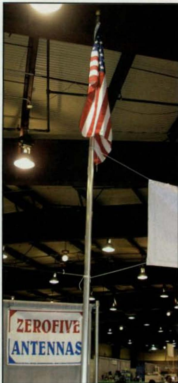
Stand up and salute! This flagpole is also a vertical antenna that can handle full legal power on 40–10 meters. It's made by ZeroFive Antennas and distributed by Array Solutions.
