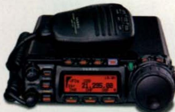
HF/VHF/UHF Multimode Mobile Transceiver,
