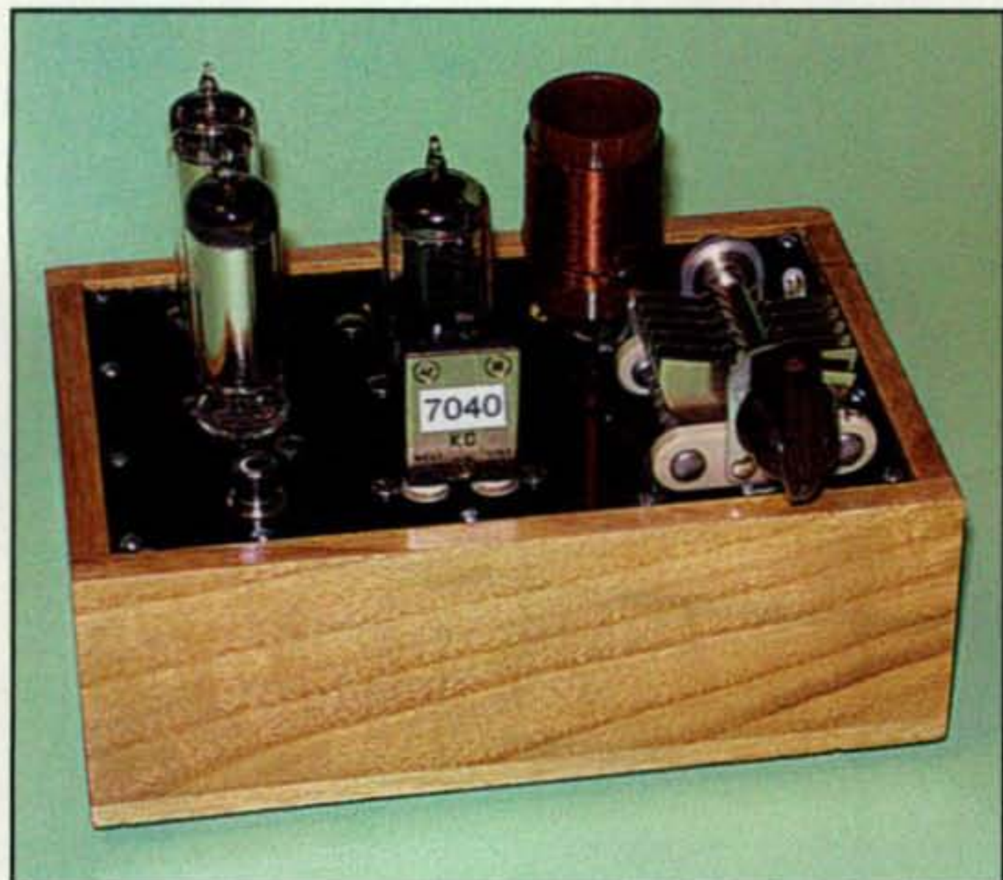
Photo D— This work of art is a 40-meter 6CL6 transmitter built by Charlie Zarek, W9SAY, and it delivers a clean 5-watt signal. It is loaded with good looks and class, and the pair of grid-voltage-stabilizing 0B2s blink blue in time with CW keying for extra flash. (Photo courtesy of W9SAY)
