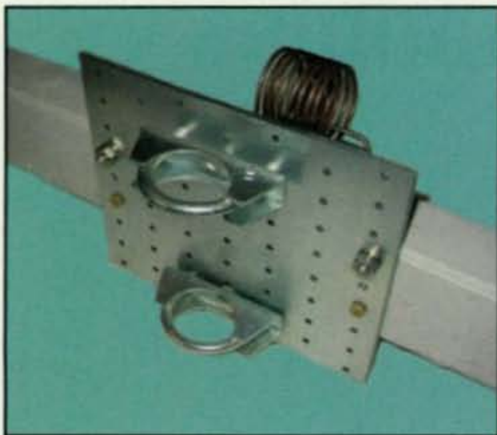
Photos D1 & D2— Here's a mast-side view (D1, above) of another mounting option using standard deck hardware for an antenna support-to-mast plate and stainless-steel U-bolts with saddles. Photo D2 (right) shows the antenna-side view of the same configuration with the balun attached.
