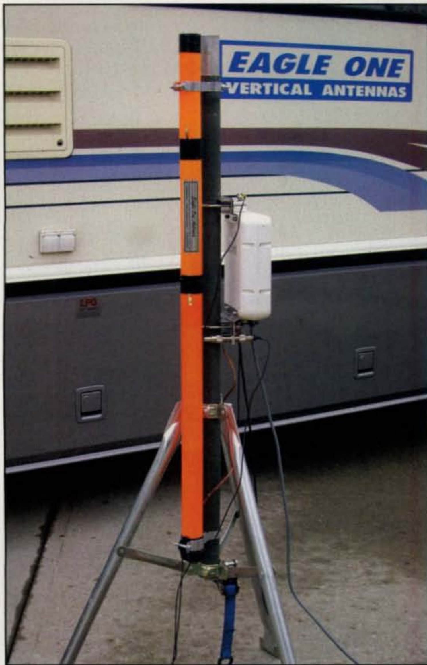
Photo D— The Eagle One vertical antenna in collapsed position with included mounting brackets, optional tripod, and a user-supplied tuner. When fully extended, the antenna is 31 feet in height and it collapses to 44 inches for easy transporting. (Photo courtesy of S & G Engineering)
