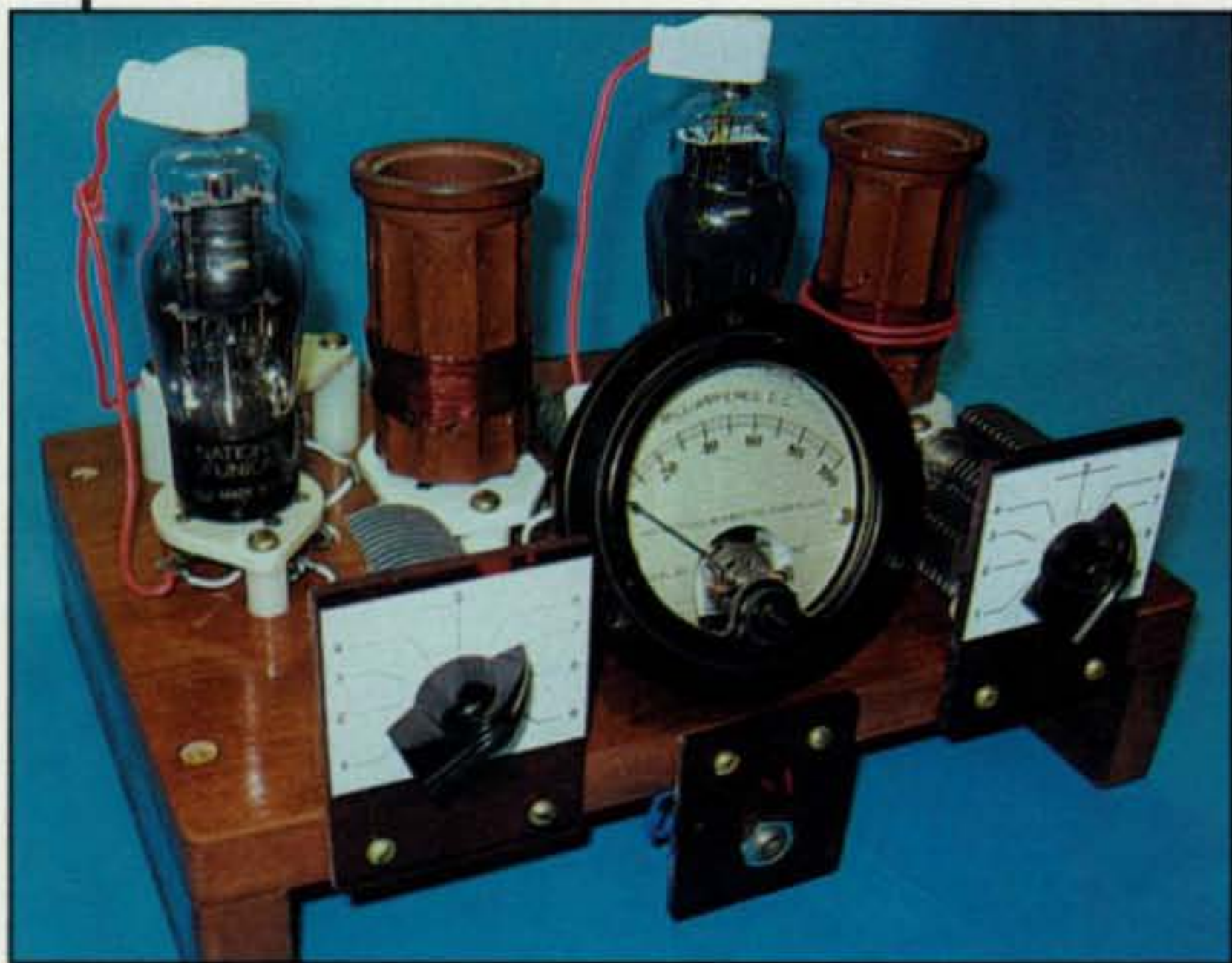
Photo A— Dazzling and beautiful appropriately describe this dual type 38 tube 80/40-meter transmitter John Karasz, WB2MGY, built and designated the "38 Special." Look at those ceramic grid caps, those lily-white isolantite sockets, the round-faced Weston analog meter, and the soft glowing base! (Photo courtesy of John, WB2MGY)
