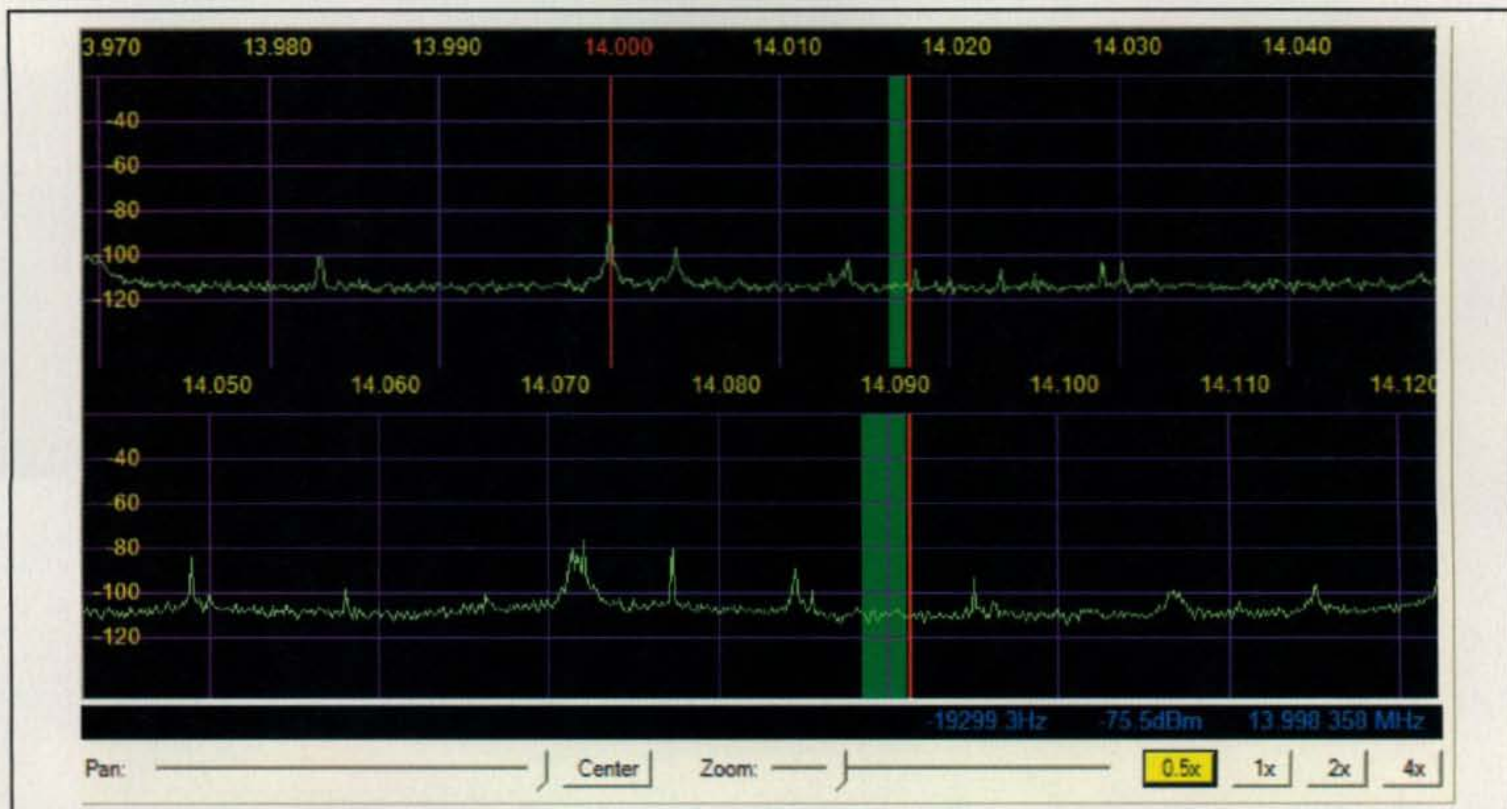
Fig. 2— Dual-receive panadapter display. The green bars represent the receiver's actual passband, set up for CW at the top and RTTY on the bottom. (Image courtesy of K3NC)
