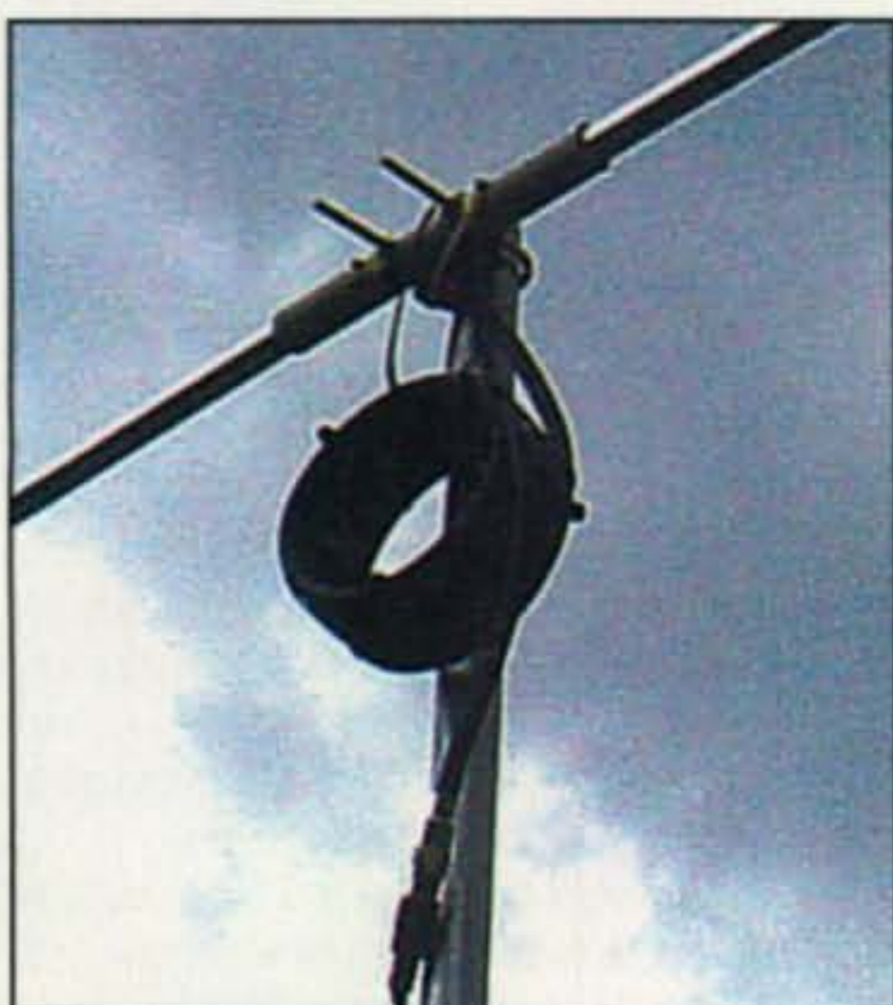
Photo C— The feedline balun consists of a 5-inch diameter coil of six turns of coax.
