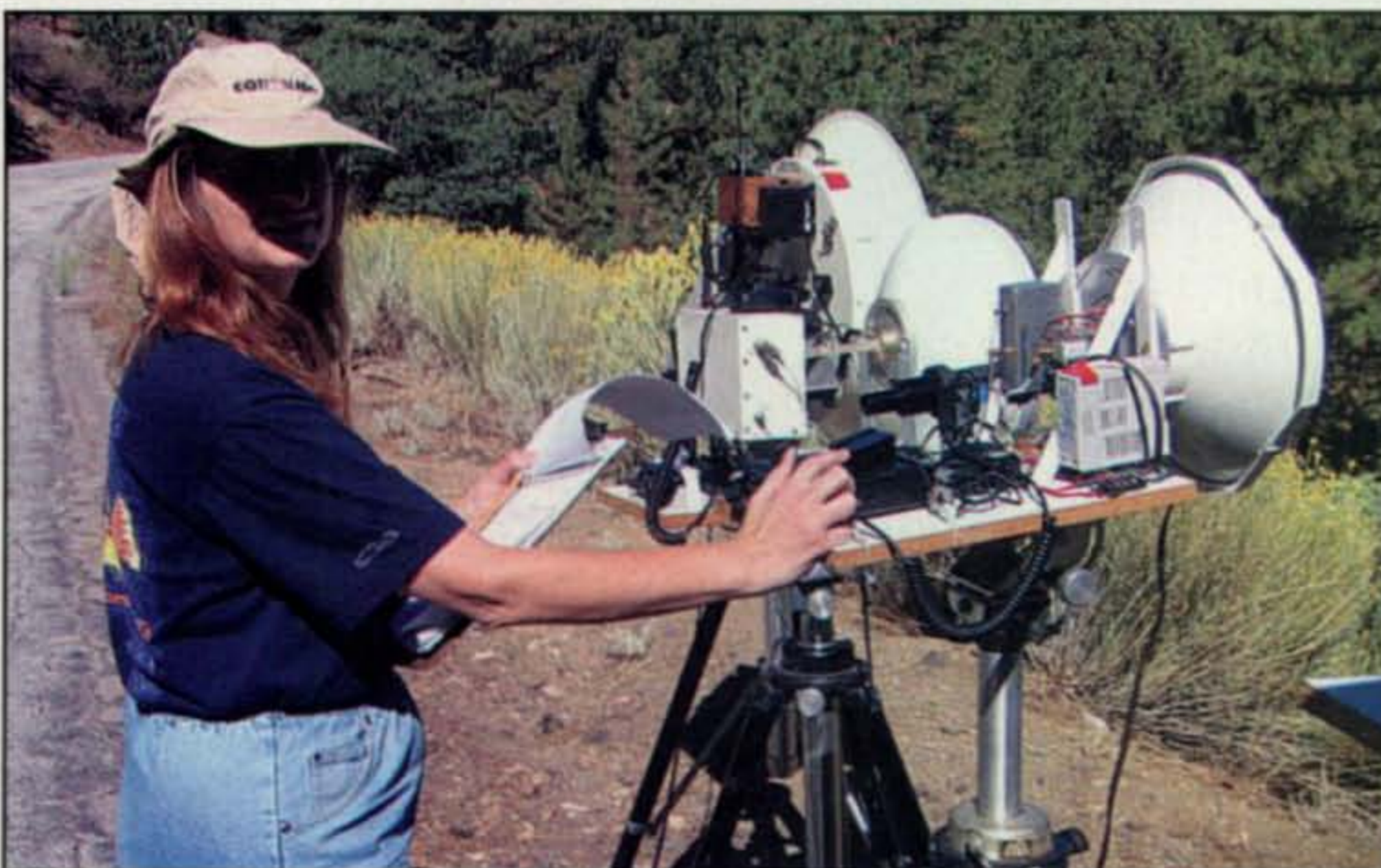
Photo B— Here is Helen in contact with Gary, AD6FP, on 79 GHz CW. Learning Morse Code many summers ago paid off! (Photo by Doug Millar, K6JEY)
