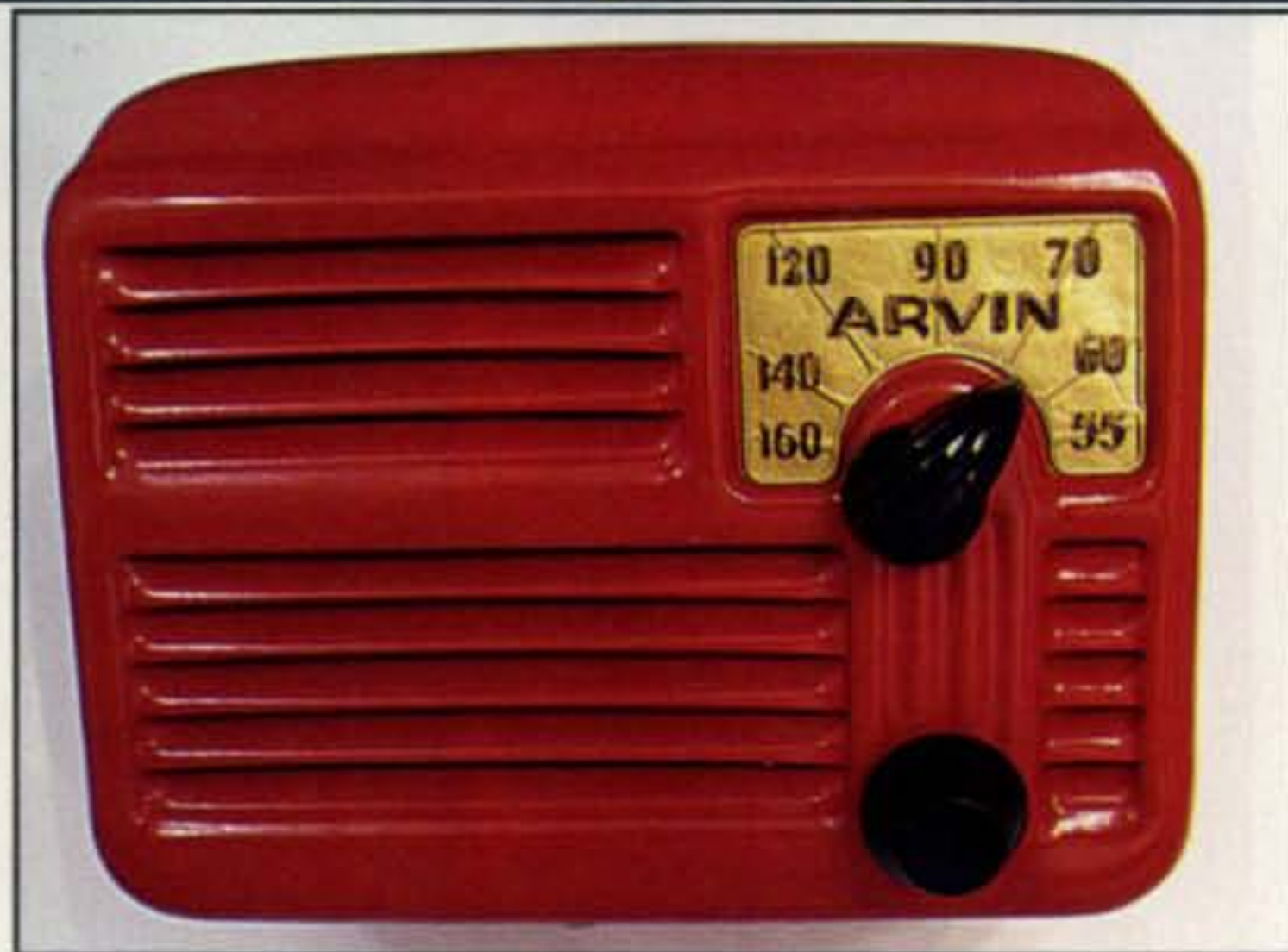
Photo F— How many of our readers remember this sweet little four-tube AC/DC Arvin AM radio? It was especially noted for its "backward dial" (550 kHz on the right rather than the left side), it ran hot as a firecracker (four big bottles in a tiny metal cabinet), and it had quite a "kick" when plugged backwards into a home 120-volt outlet. Oh those wonderful days of yesteryear! (Photo by K4TWJ)
