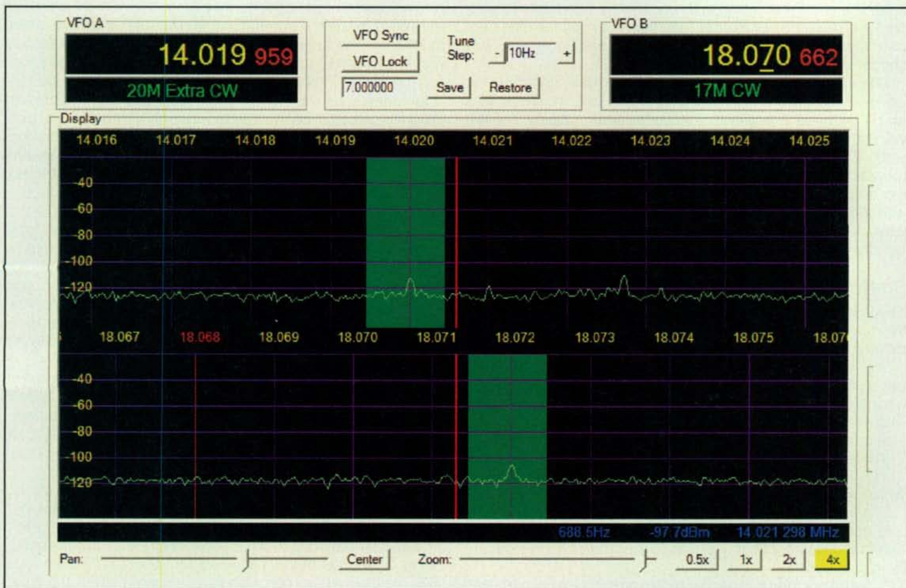
Fig. 4— PowerSDR on split band in CW-L and CW-U modes. The passbands appear much wider here than in previous shots, but only because the panadapter is displaying a much narrower segment of spectrum (approximately 9 kHz here vs. about 70 kHz in the others). (Image courtesy of K3NC)
