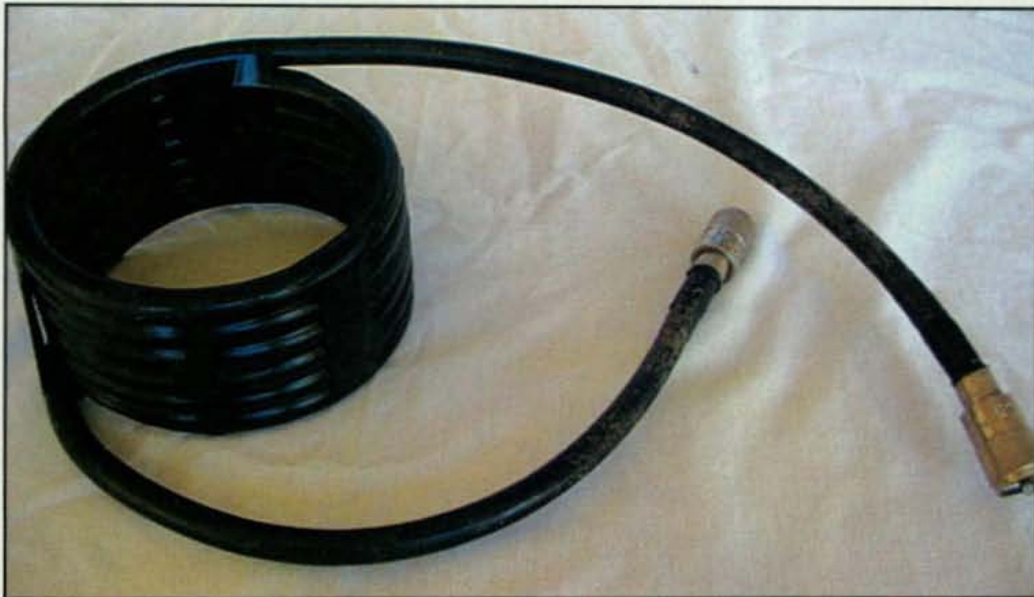
Photo C— The balun is made with RG-8/U-type coax. The author suggests putting a PL-259 on each end and connecting the feedline through a barrel connector.
