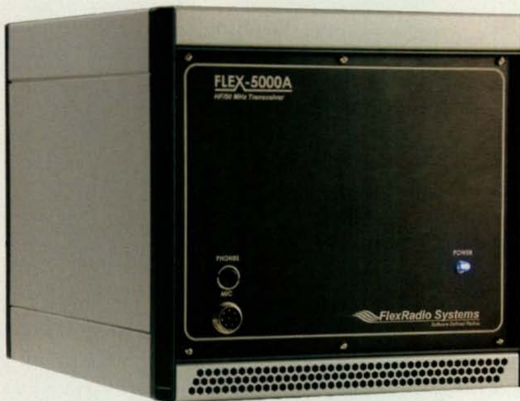
Photo A— Front-panel view of the FLEX-5000A. There's only one control, an on-off switch! Everything else is done in software. (Photo courtesy of FlexRadio Systems)
