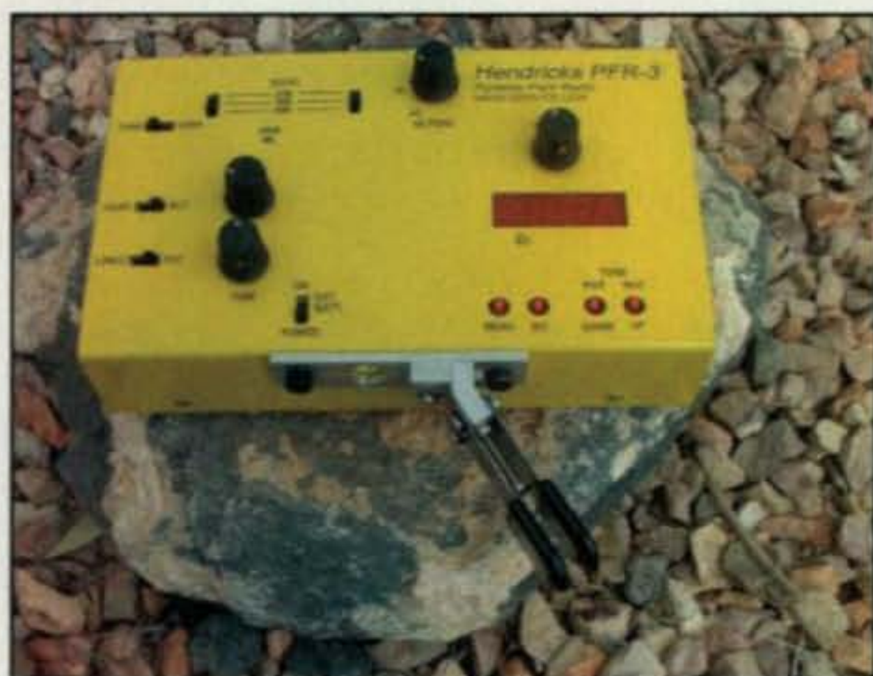
Photo A— Front top view of Hendricks QRP Kits recently introduced three-band portable field radio, the PFR3 XCVR, with optional paddles. (Photos A, B & C courtesy of Hendricks QRP Kits)
