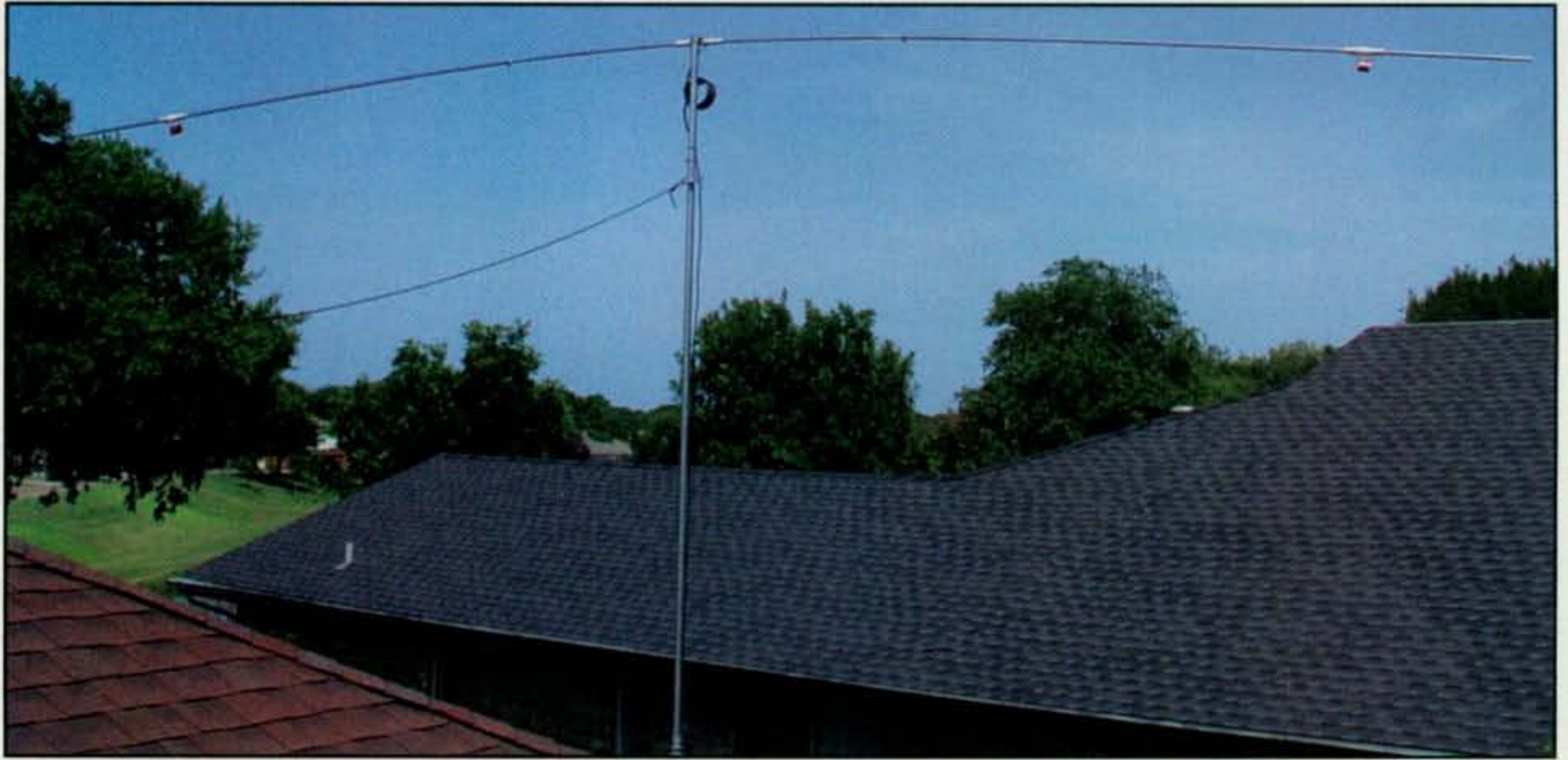
Photo A— The completed 17/12-meter trap dipole ready for working some DX. Now if only the sunspots co-operate!
