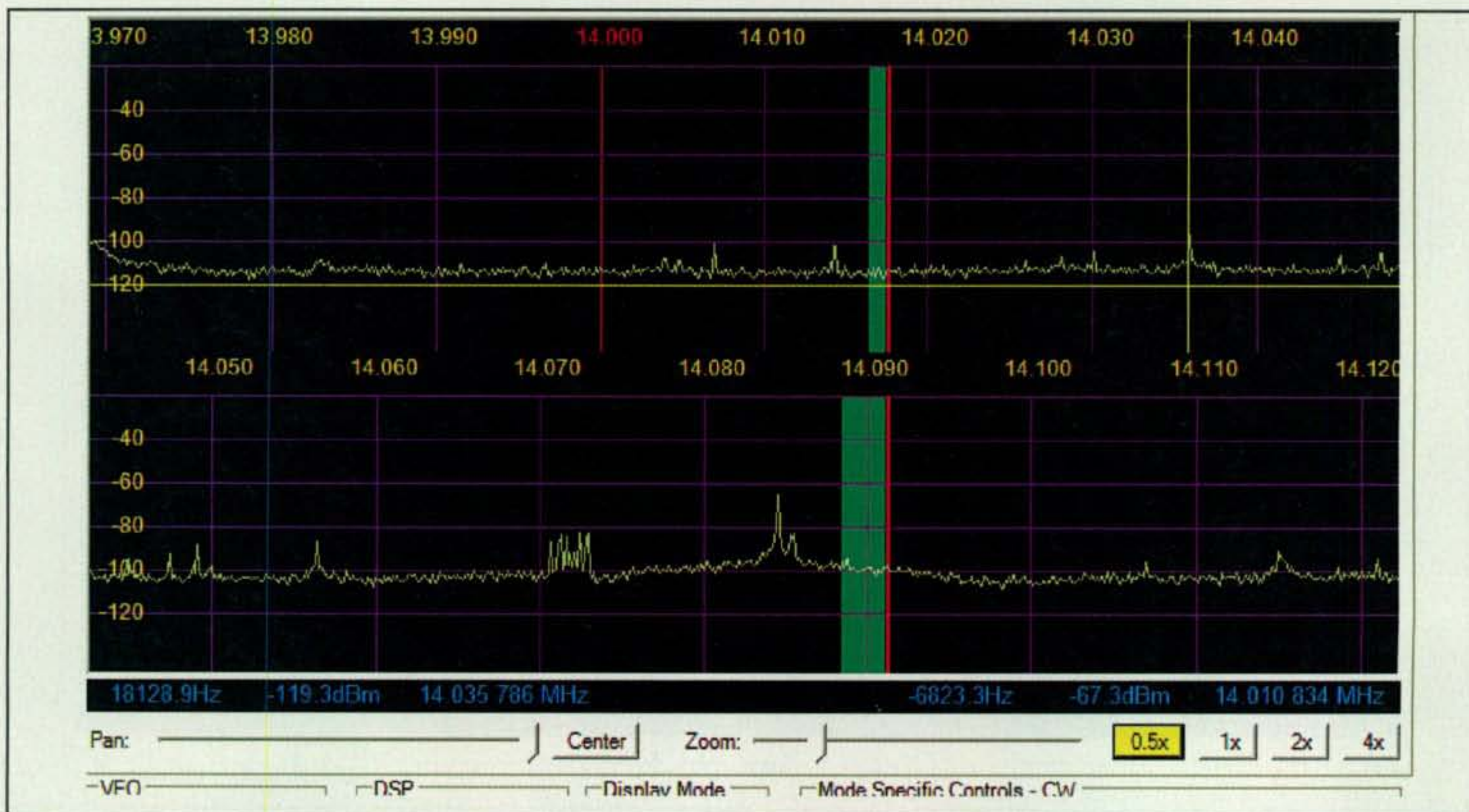
Fig. 3— PowerSDR with ClickTune™ control. Note the yellow lines that intersect at about 14.035 MHz. This is where a user has right-clicked the mouse. A left-click will retune the rig to that spot. (Image courtesy of K3NC)
