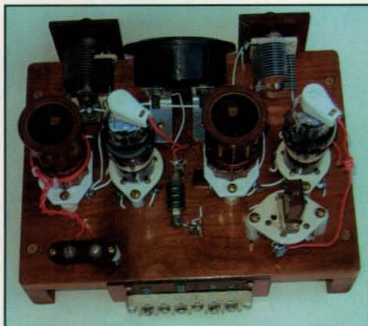
Photo B— Rear view of the WB2MGY 38 Special reveals an incredible collection of classic parts, including Hammarlund midget variable tuning capacitors and 1 1/2 inch diameter plug-in coil forms. Photo courtesy of WB2MGY)
