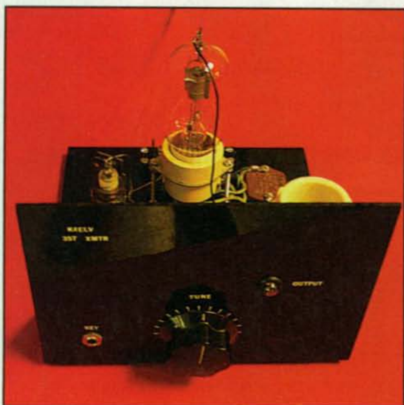
Photo 1— The magnificent Super T transmitter built by Mike Lord, K4ELV, uses a genuine Eimac 35T tube and works 40 meters in high style. Power output is determined by the amount of plate voltage. The pilot lamp on the right side of the front panel serves as tuning aid.
