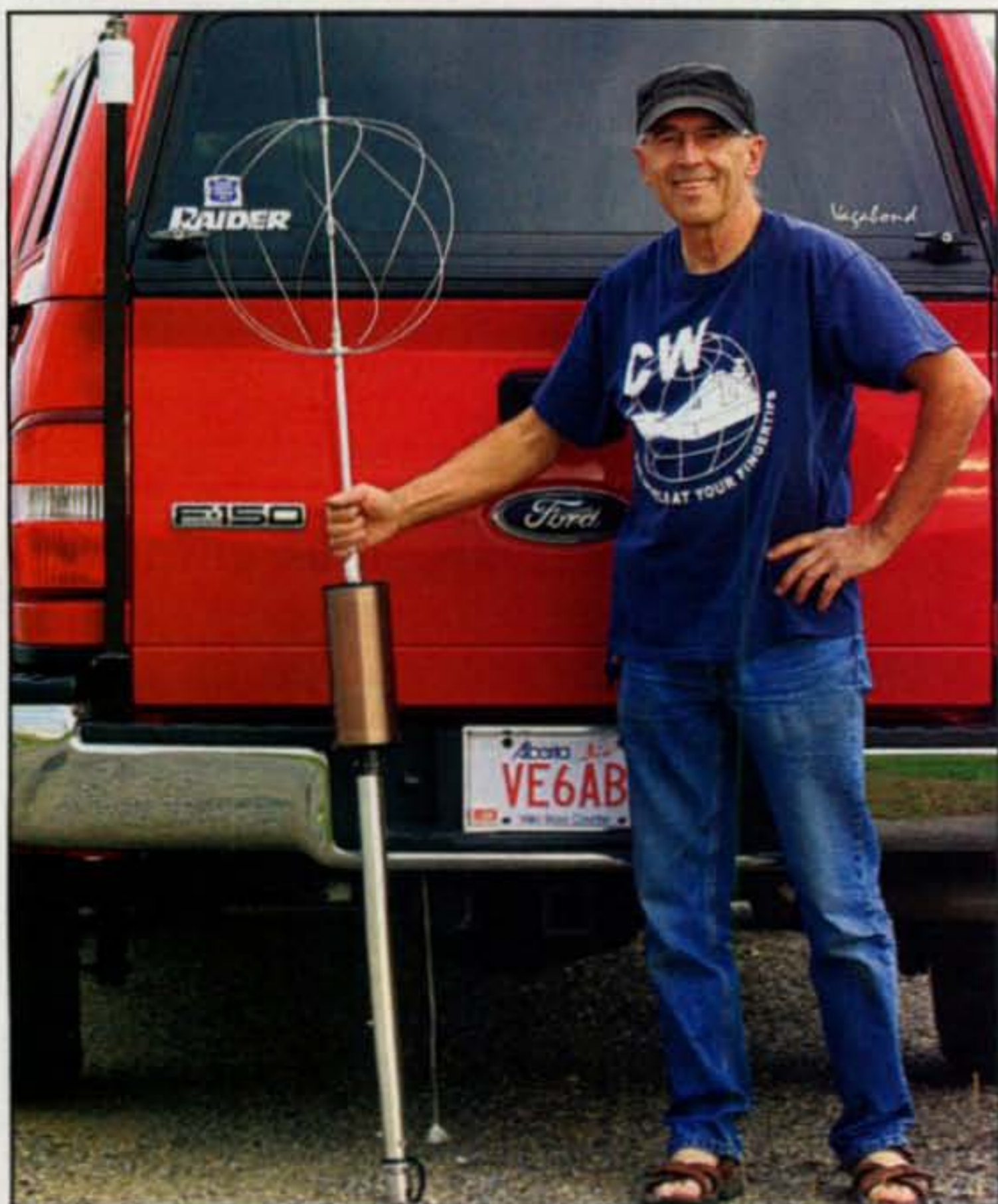
Close-up of the egg-beater capacitance hat for 80-meter mobile operation.
