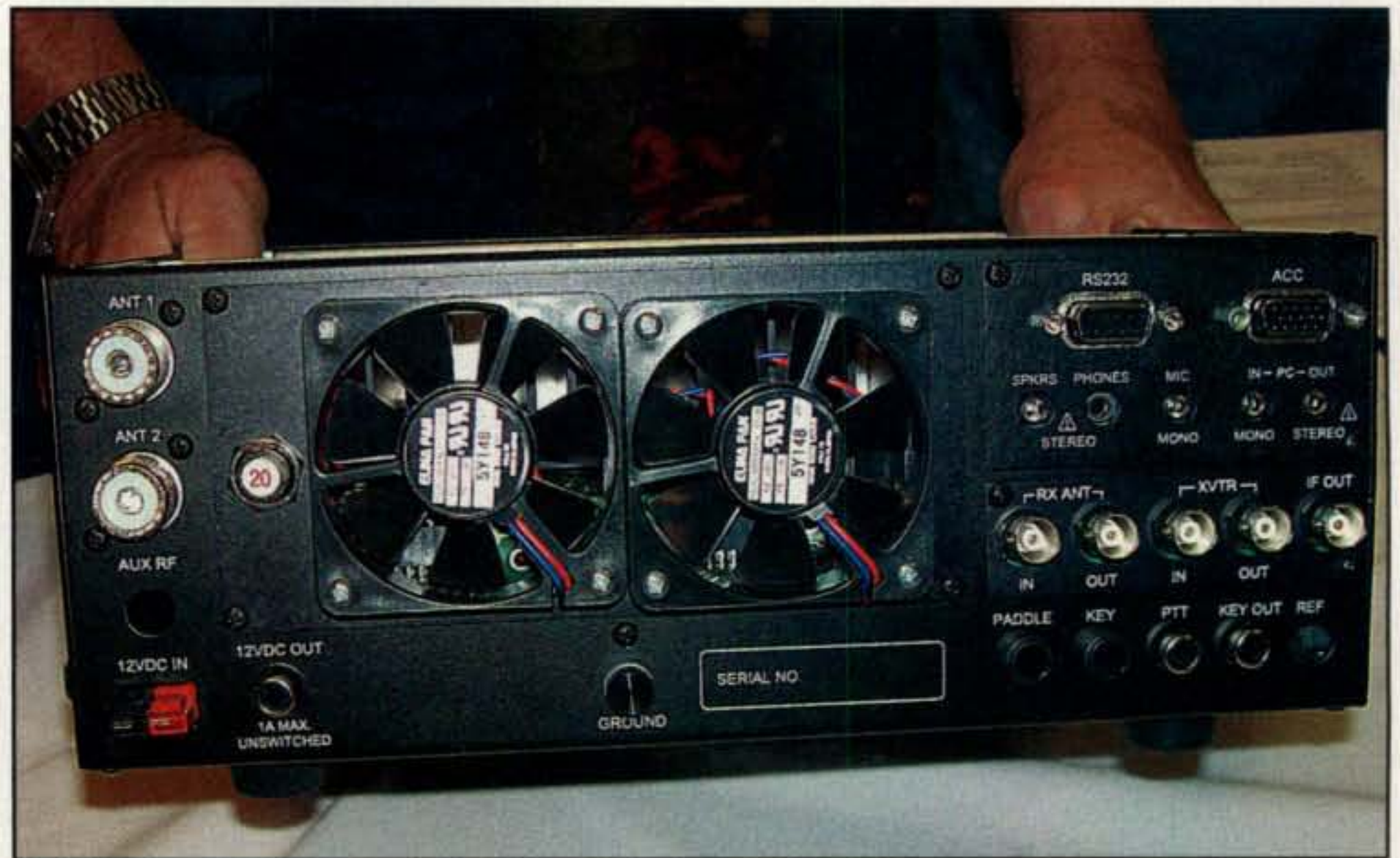
Rear view of the K3. Note the dual cooling fans, the variety of input/output options, and the Anderson PowerPole™ power connector. (Photo courtesy of Cecil Bayona, K5NWA)
