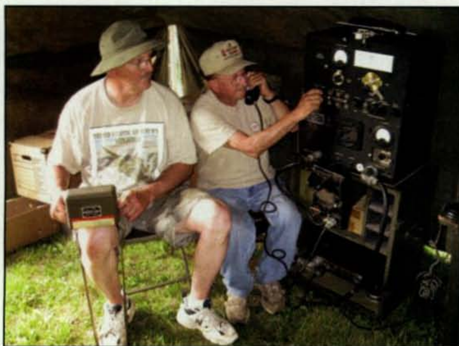
Photo A— Ted Young, W3PWW, operates his perfectly restored BC-669 75-meter AM transmitter-receiver at the Reading PA WW II reenactment while David Kormanicki, KB3ELD, demonstrates the operation of his American WW II M-209 cipher machine. (All photographs by and courtesy of the author)
