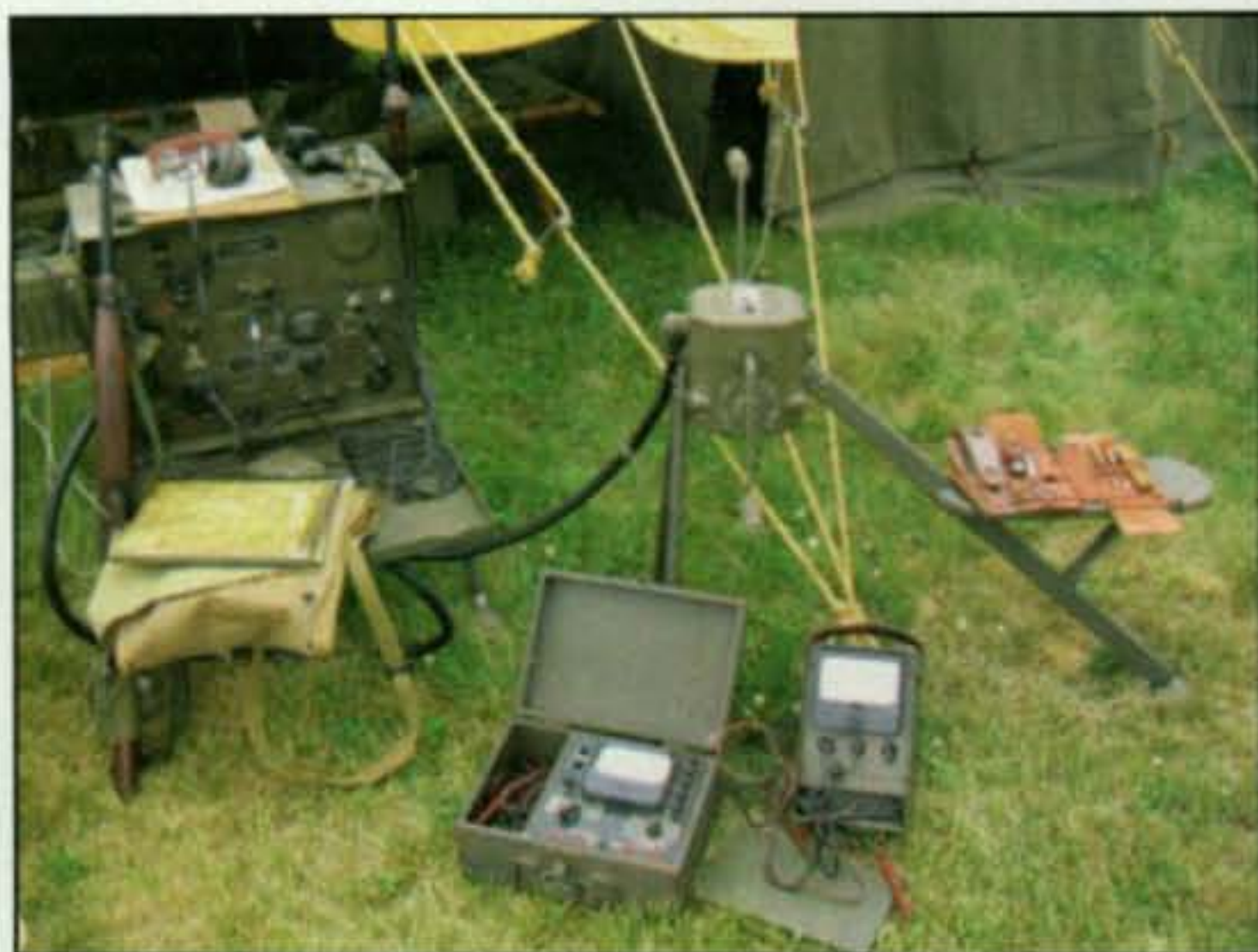
Photo B— This is a complete BC-654 transmitter-receiver set up in a field with all of the appropriate accessories, including the hand-cranked generator and some test equipment.
