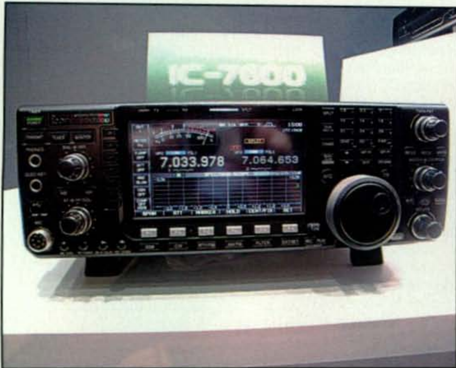
The ICOM 7600! This unit was displayed at the Tokyo Hamfair 2008 the end of August and is the newest addition to the ICOM line. It has three roofing filters, USB ports in front and back, scope features like the IC-7700, and more. (Photo and info courtesy of Bill, N2WB, and Markus, DL9RCF)
