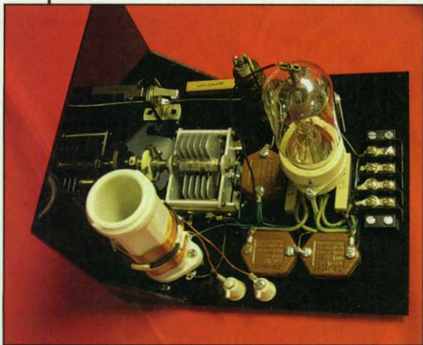
Photo 2— A behind-the-panel view of the K4ELV Super T transmitter showing the layout of parts and rustic glamour of the open-air design. The tube stands almost 5 inches tall, and like the plug-in coil form and magnificent "domino" capacitors, they are slowly disappearing from existence. (Photo courtesy of Mike, K4ELV)
