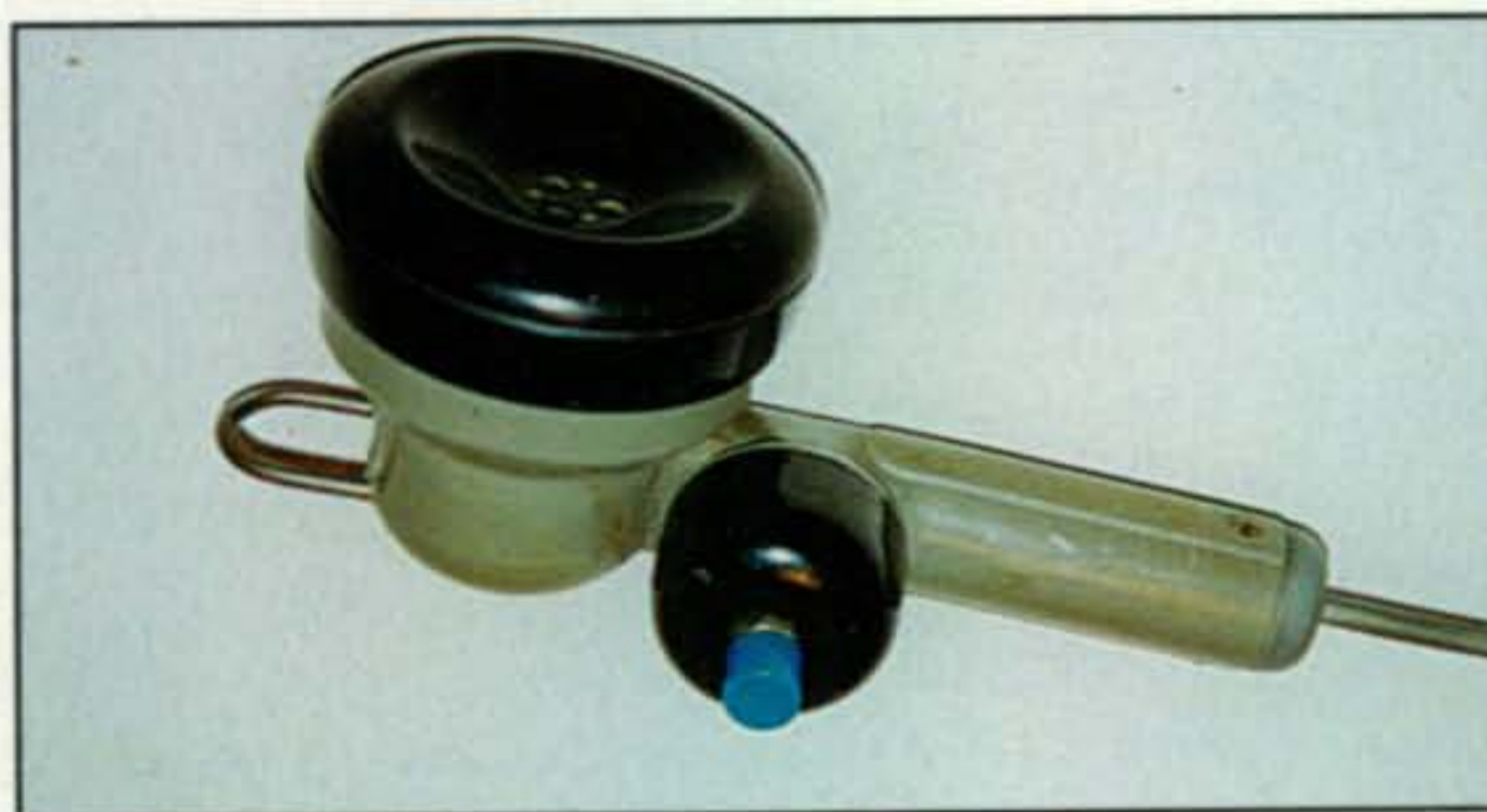
Photo A— Modified WW II Military Microphone T-17PPT. (All photos by the author)
