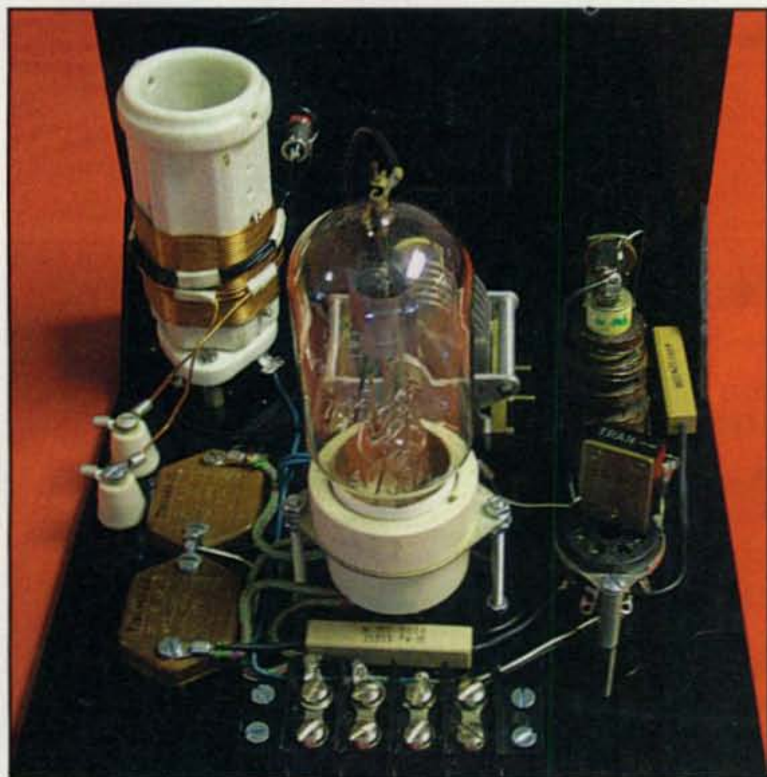
Photo 3— Straight-on rear view of the K4ELV transmitter shows how Mike used long screws with extra nuts and spacers to mount the tube and crystal socket above the base—a clever idea worth remembering. Those with sharp eyes will also notice the second “sensing” pickup coil for pilot-lamp tuning aid on the coil form. Thanks to K4ELV for sharing views of this rig with us.
