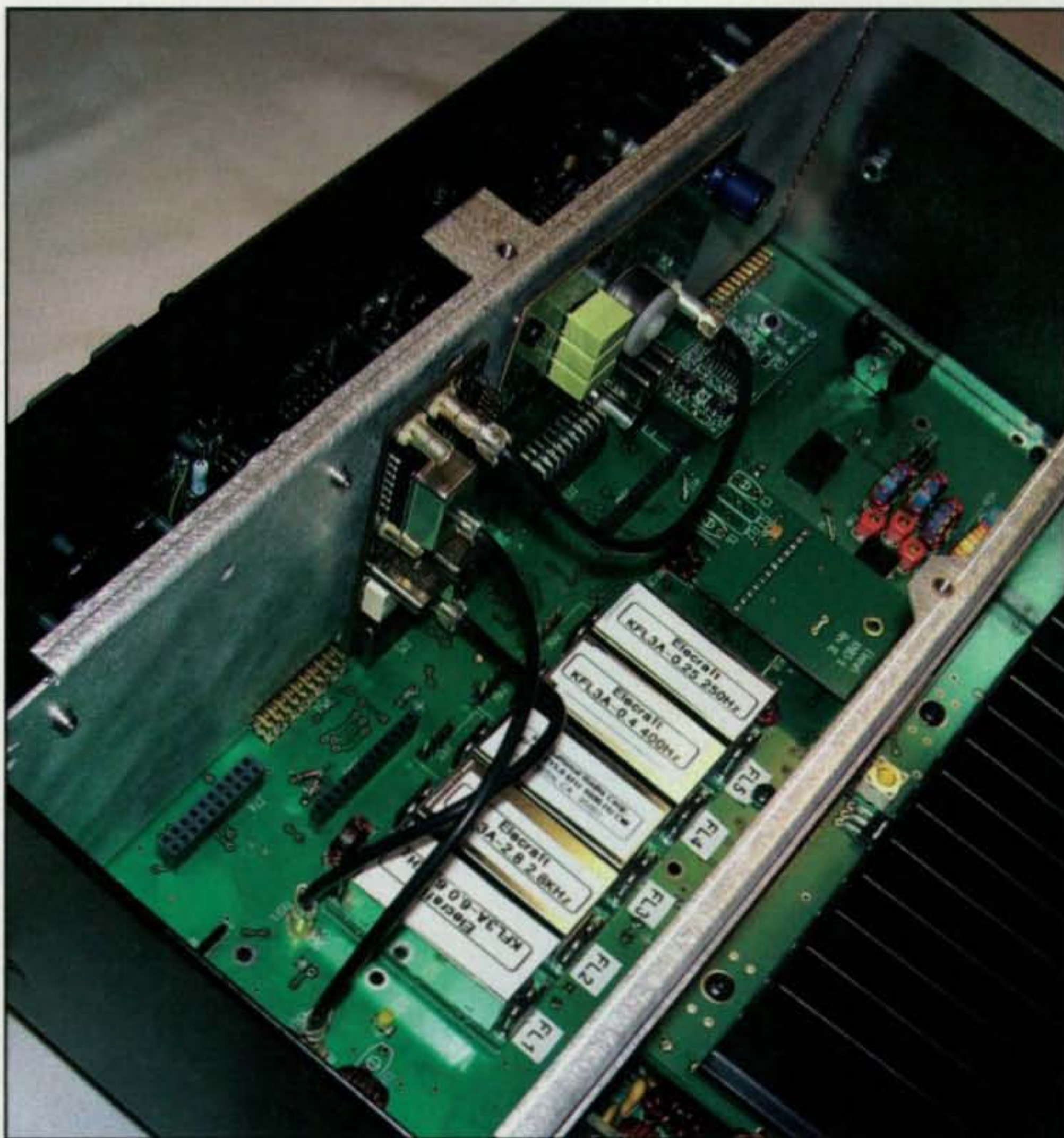
Interior view. The K3 is available fully assembled or as a "semi-kit" in which the circuit boards are preassembled and the builder installs and interconnects them, in much the same way as "building" a computer from a variety of preassembled circuit boards. (Photo courtesy of Cecil Bayona, K5NWA)
