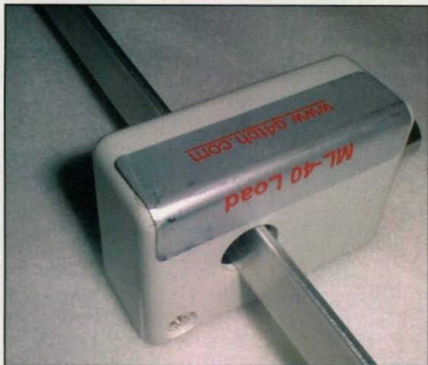
Photo D— Installed magnetic coupler.
