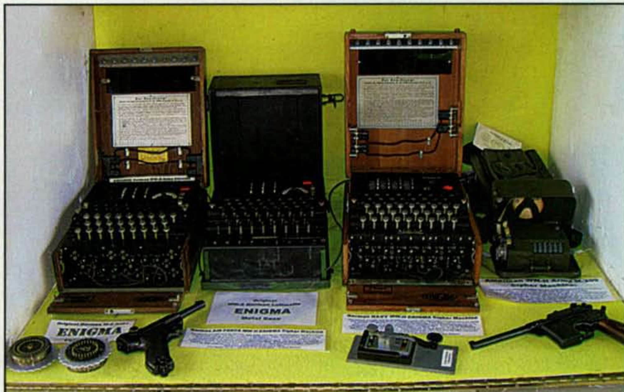
Photo G— In addition to some WW II radios, the author's display at military meets and hamfests includes German Army, Navy, and Air Force Enigma cipher machines, an American M-209 cipher machine, and various accessories. You can visit his Enigma museum at < http://www.w1tp.com/enigma >.
