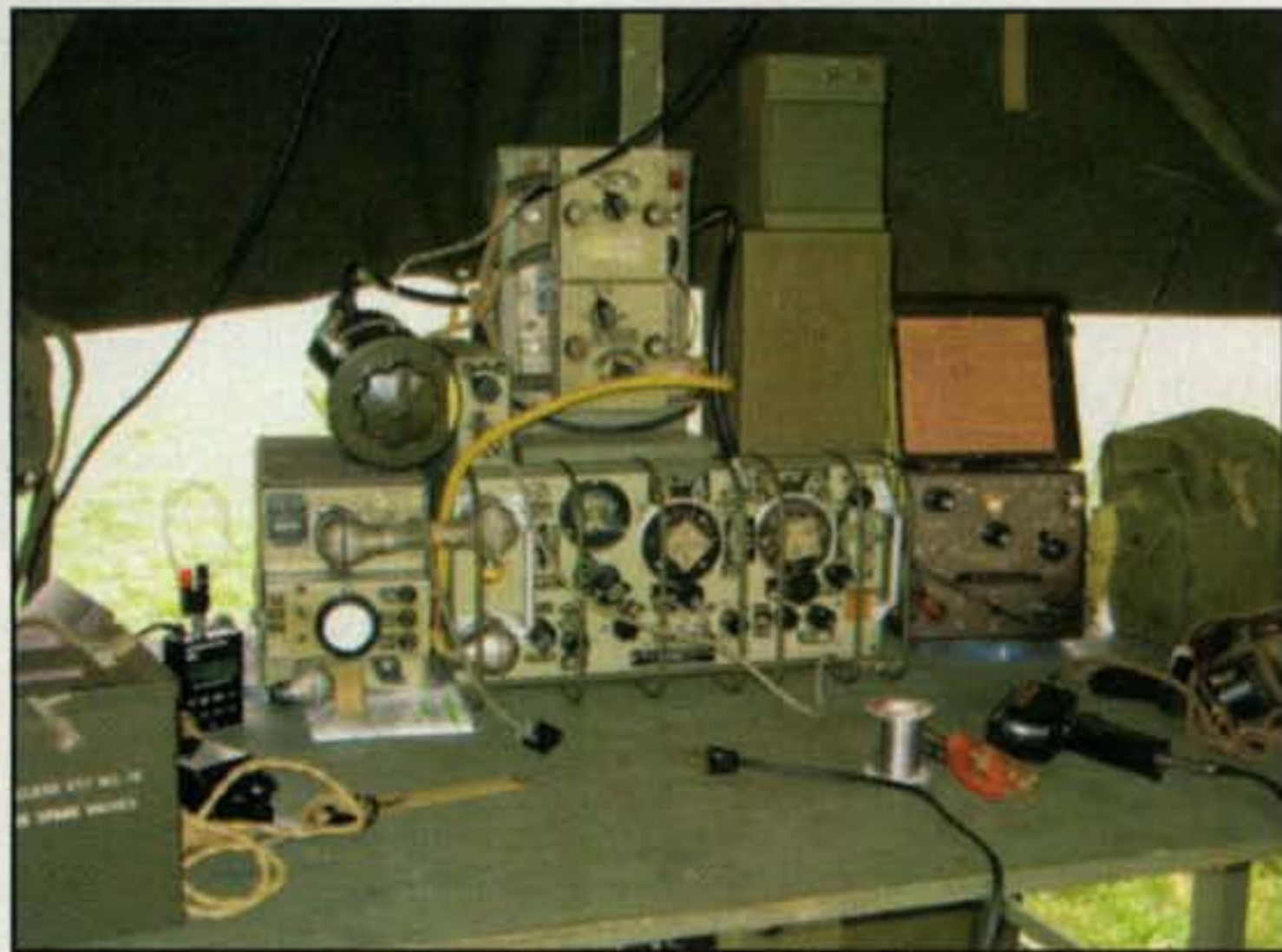
Photo F- This is a complete and authentic British WW II Wireless Set 19 transmitter-receiver with all of the appropriate and very hard-to-find accessories. (The much more modern Weller soldering gun and frequency counter are hidden during show hours.)
