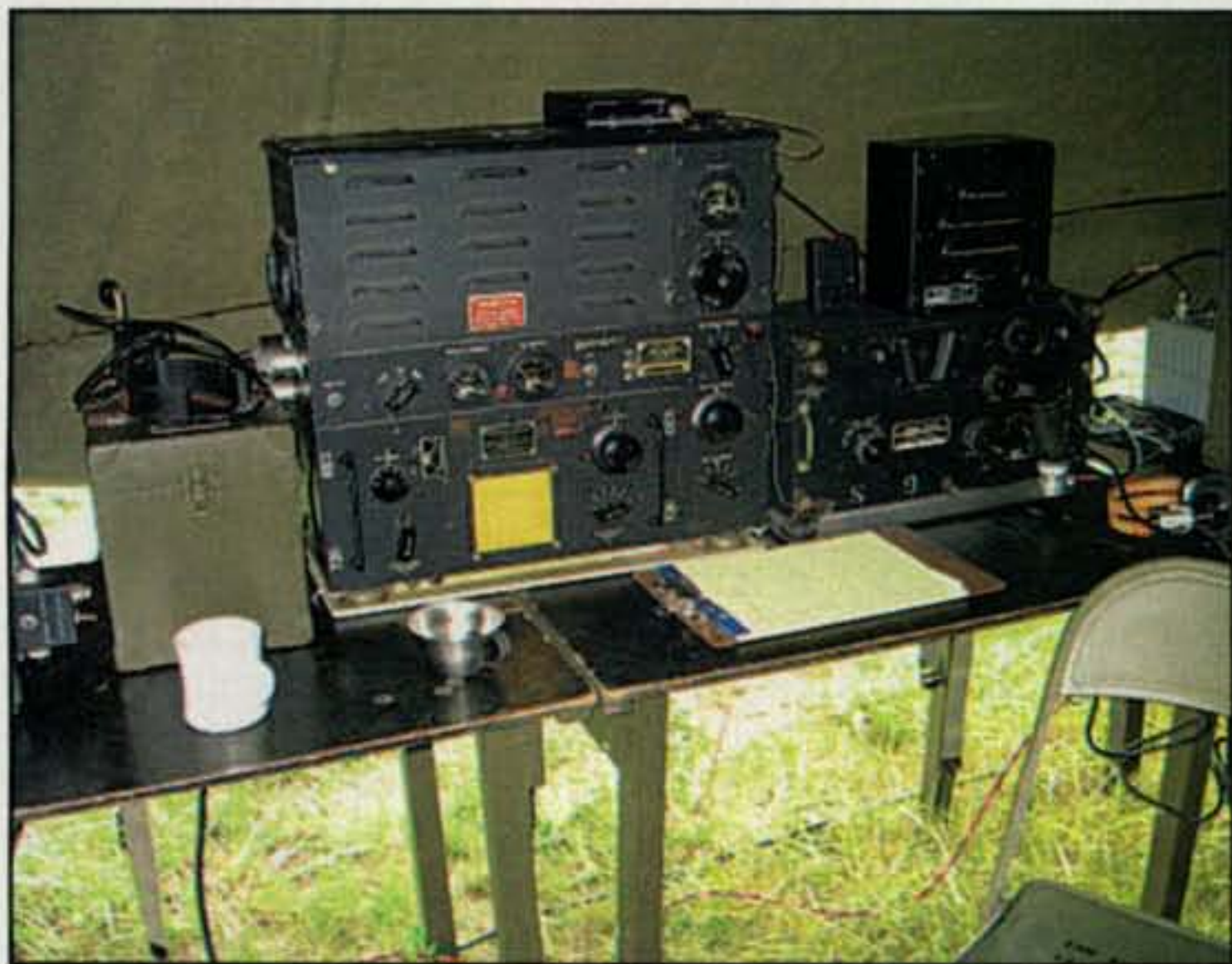
Photo E- This is a beautifully restored and fully functional BC-191 transmitter and BC-312 receiver operating on 3885 kHz AM, which is the standard frequency used by hams to operate their military radios at military meets and hamfests.
