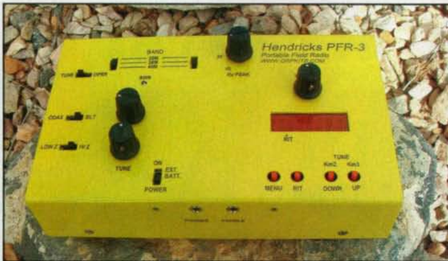
Photo 5— The new PFR-3 40/30/20-meter CW transceiver kit from <www.qrpkits.com> sports a hot receiver with 300-Hz filter, 5-watt transmitter, built-in antenna tuner, keyer with memory, and more. Install eight AA cells internally and it makes a good stand-alone transceiver for portable operations. (Photo courtesy of KI6DS)
