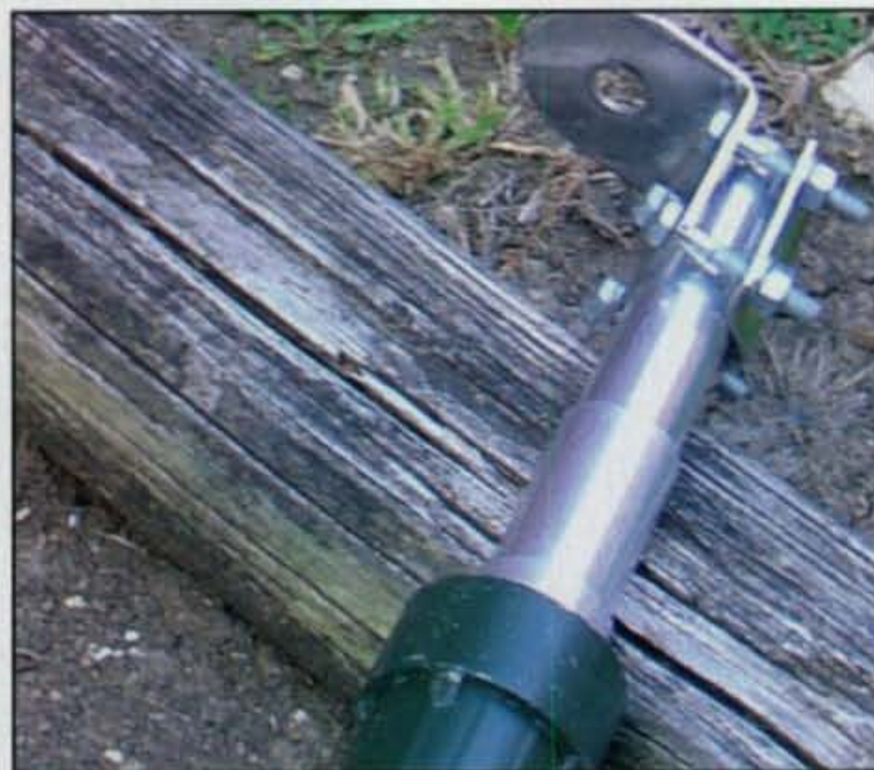
Photo C— One means of mounting a CB-type whip to the top of the mast sections.
