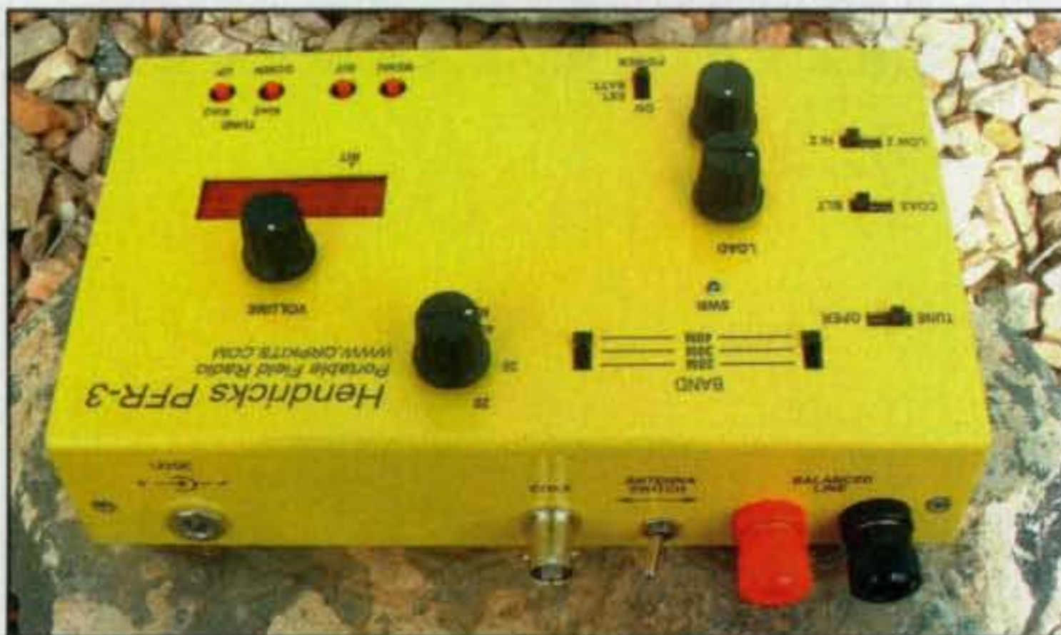
Photo 6— Reverse view of the PFR-3 showing connections for both balanced and unbalanced antenna lines. (Photo courtesy of KI6DS)
