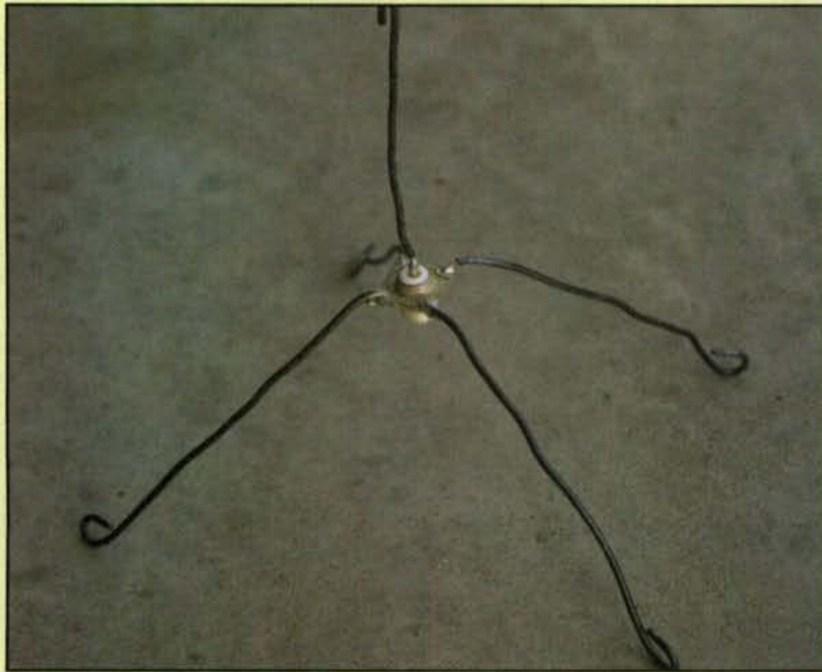
The ugly ground plane is simple to make, but a lot of soldering heat is required (see the text for more details).
