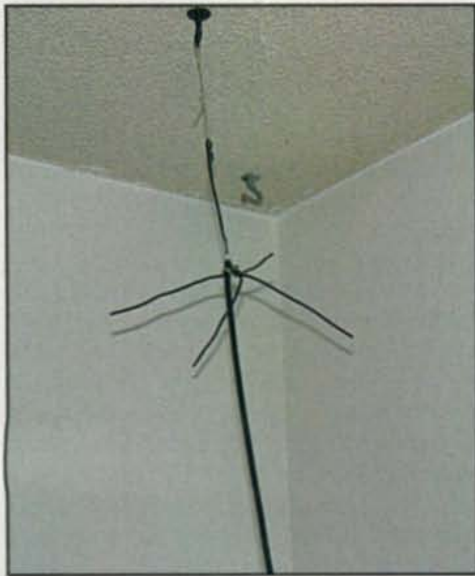
Photo 2— The indoor ground plane is easy to make and will extend the range of VHF and UHF communications. This antenna may look a little ugly to non-hams, so it may be best to hide an antenna like this in the attic.
