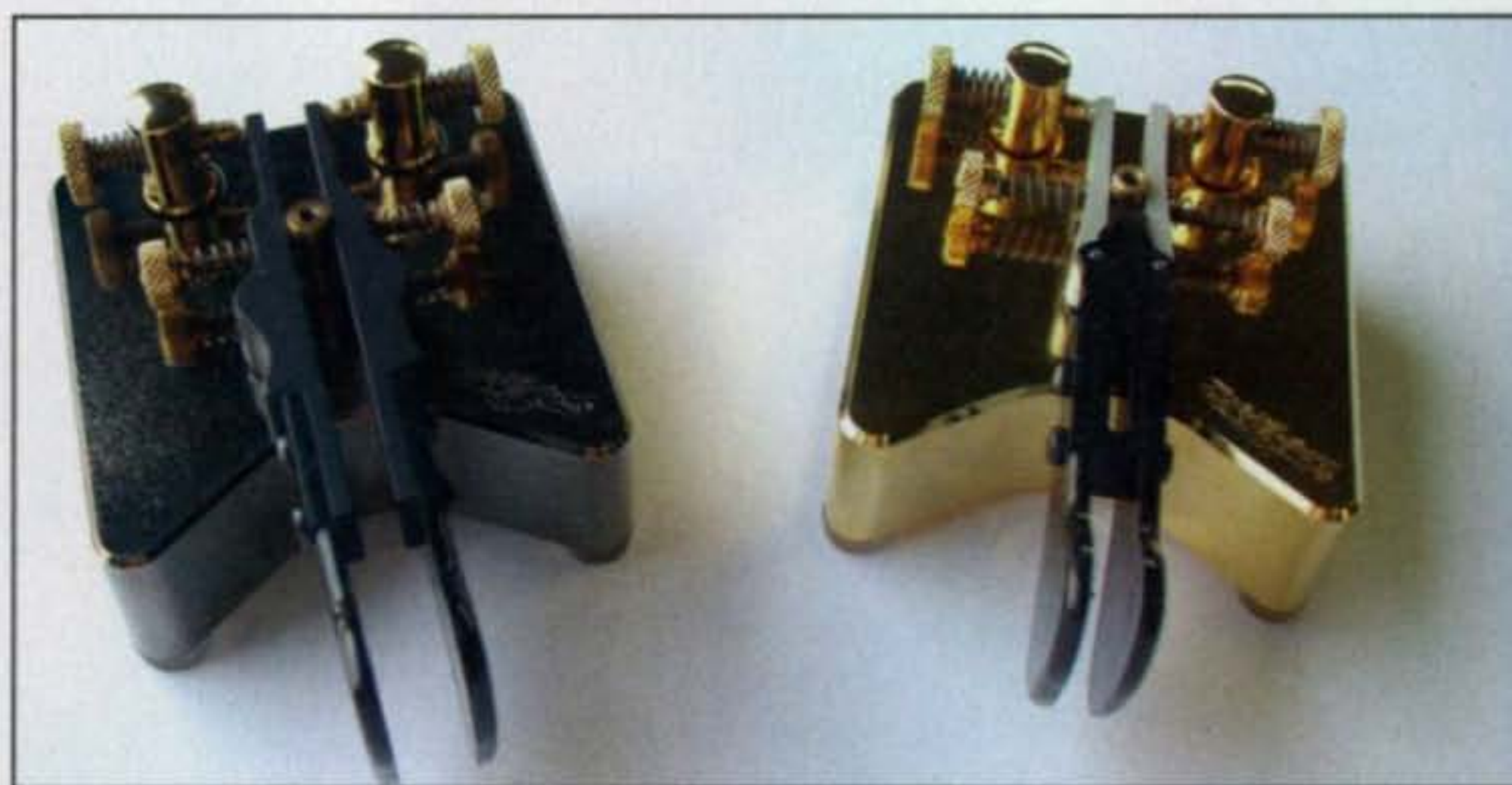
Photo 1— The Begali Simplex (dual lever, left) and Simplex Mono (single lever, right) paddles feature gold-plated upper parts mounted on either a gold-plated or a palladium-plated base. They have ball-bearing movements, fine gap/tension adjustments, corrosion-resistant contacts, and anodized aluminum-alloy fingerpieces for a quite stylish and modern look. (Photos by Bruna Begali, courtesy of Pietro Begali, I2RTF)
