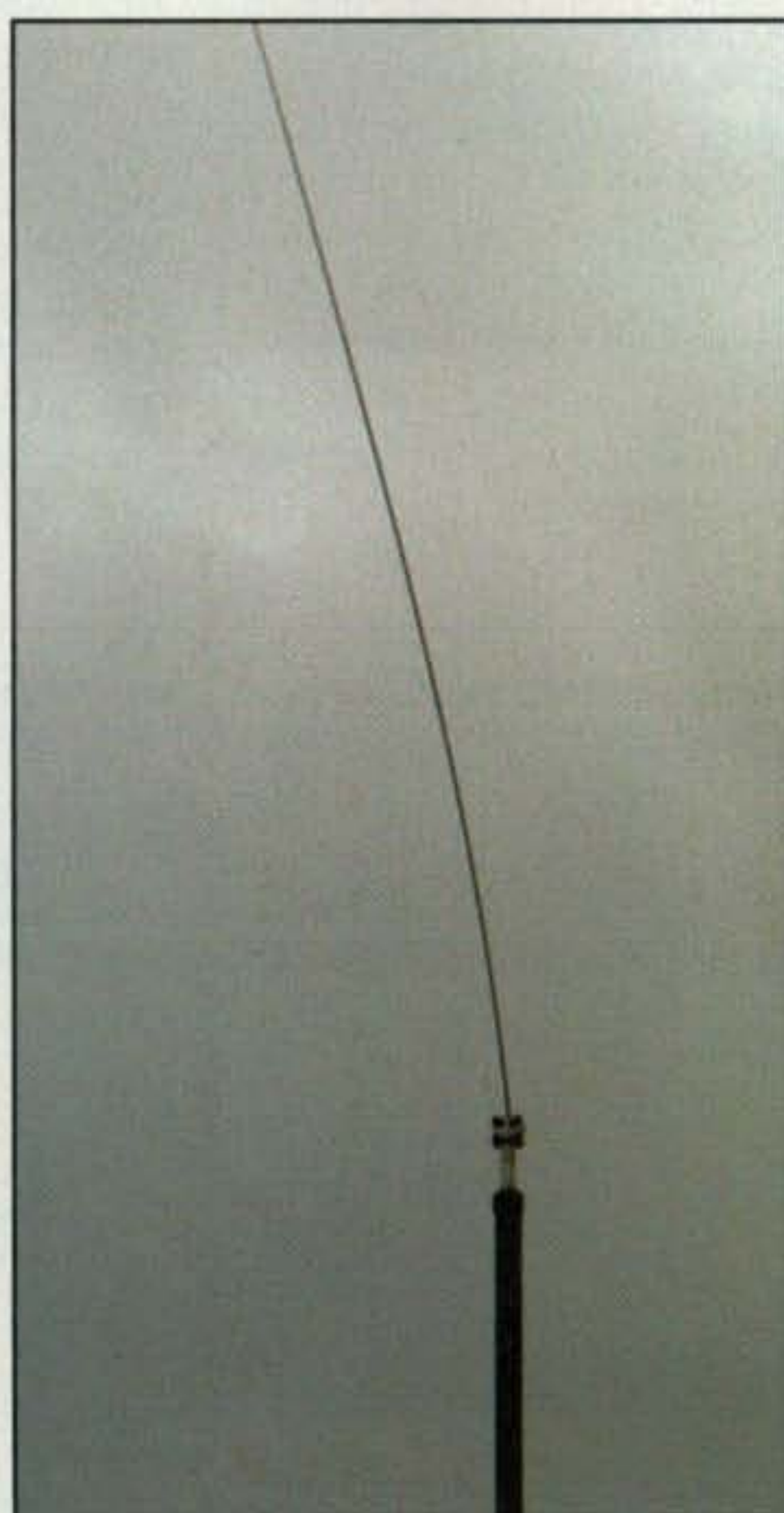
Photo G— Top whip bending during high winds.
