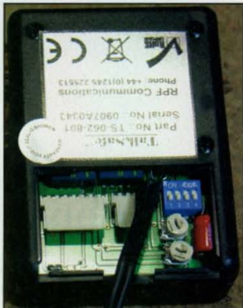
Photo C— Cable connectors (left); time out timer and mic and receive audio gain controls (right).
