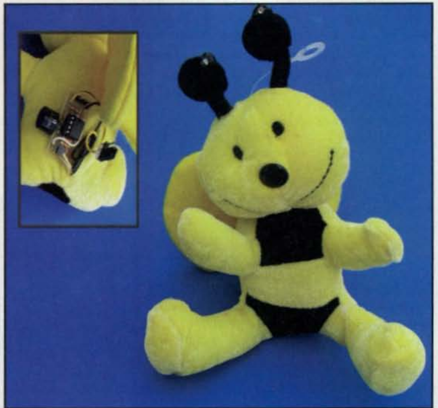
Photo 7— Check out this “Busy Bee” Rex, W1REX, found at a variety store and equipped with a Maine Bug Kit. LEDs mounted atop antennas blink your call, the PC board on the back supports temperature chirping piezo, and a 3-volt coin cell is stuffed inside the bee under its wing. (Photo courtesy of W1REX)
