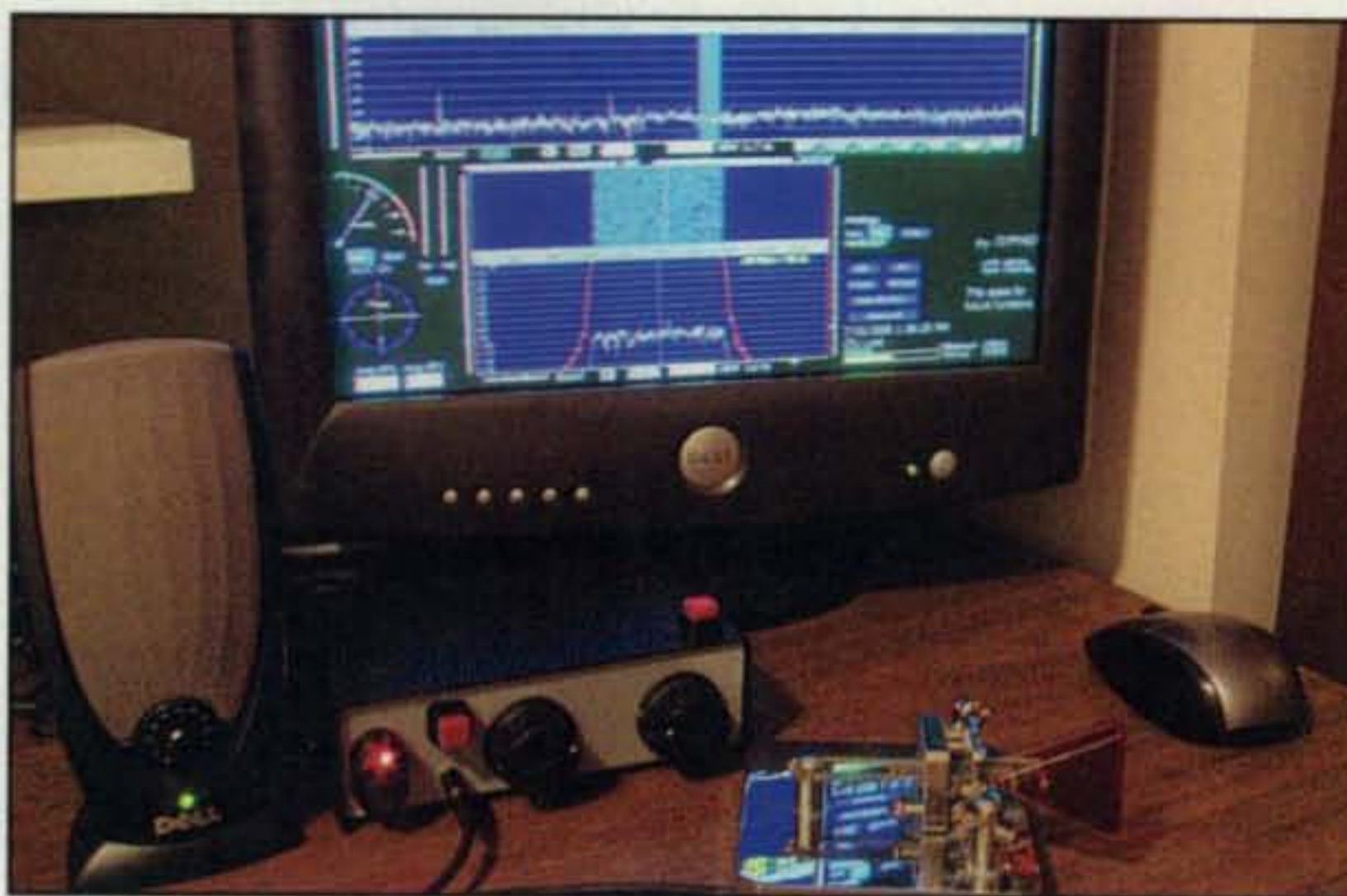
Photo 2— Thoroughly modern QRP! Fred, WA8PGE, works 30 meters in high style with his tiny Firefly software defined transceiver (box with two knobs and pushbutton) and desktop computer. Mouse runs the computer, MFJ paddle runs the rig, and speaker pumps out cheerful CW notes. Classy! (Photo courtesy of WA8PGE)
