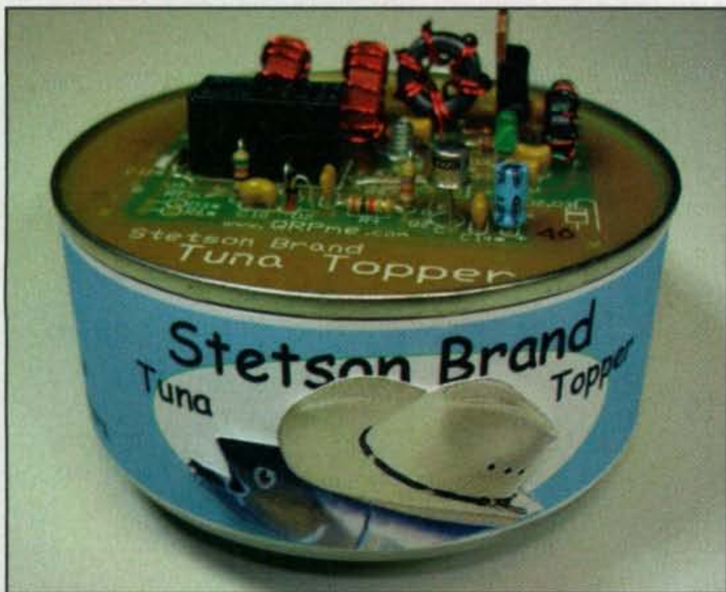
Photo 7— Heads up, milliwatts maestros. This tin's for you! It is an easy-to-assemble 40-meter RF amplifier kit that will boost the output power of your Tuna Tin 2, DC-40, Rockmite, or similar milliwatt rig to a full 5 watts output, and it is available from W1REX at <www.qrpme.com>. (Photo courtesy of W1REX)
