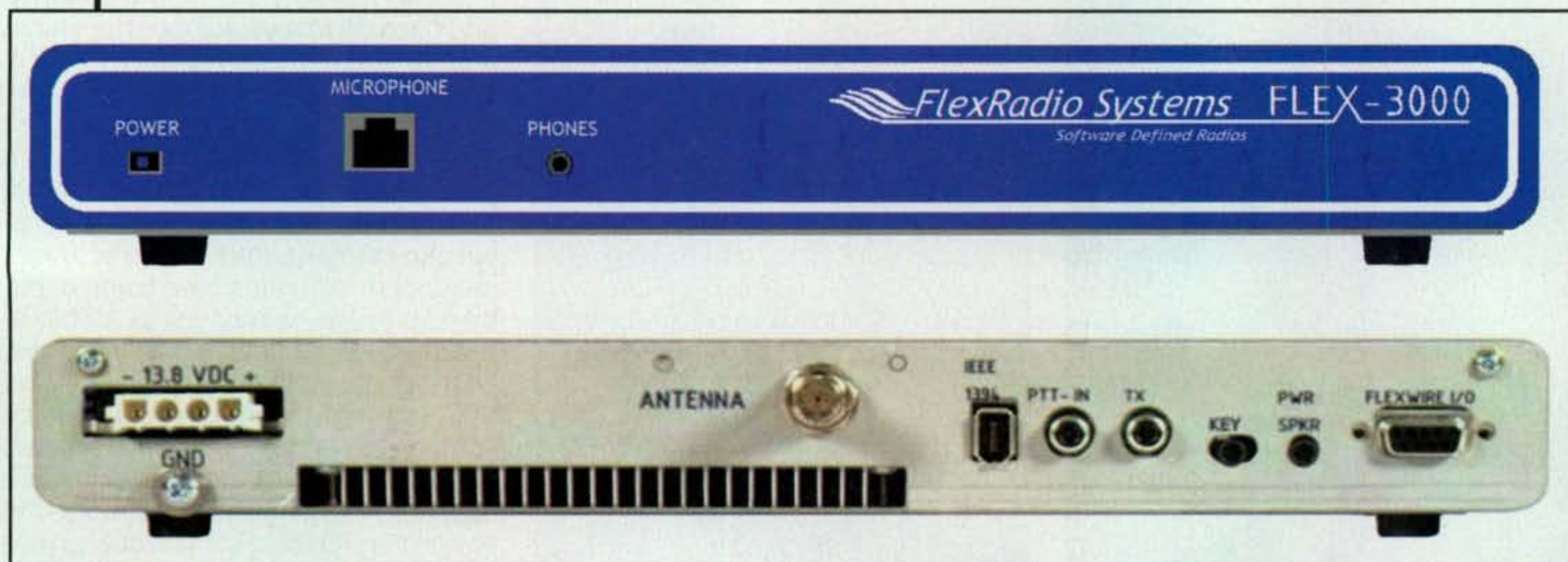
Photo A— The FLEX-3000 is a scaled-down software defined radio in the lineage of the FLEX-5000™ and designed for portable and fixed operation. (Photo courtesy of FlexRadio)
