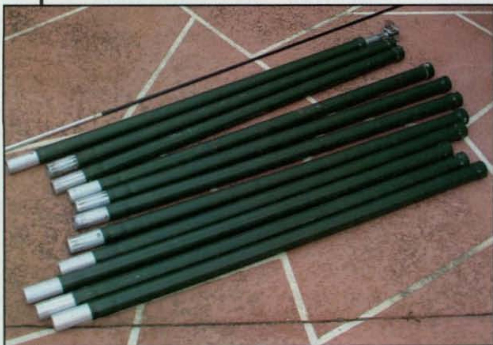
Photo A— The 1.8-inch diameter by 4-foot long surplus aluminum mast sections.
