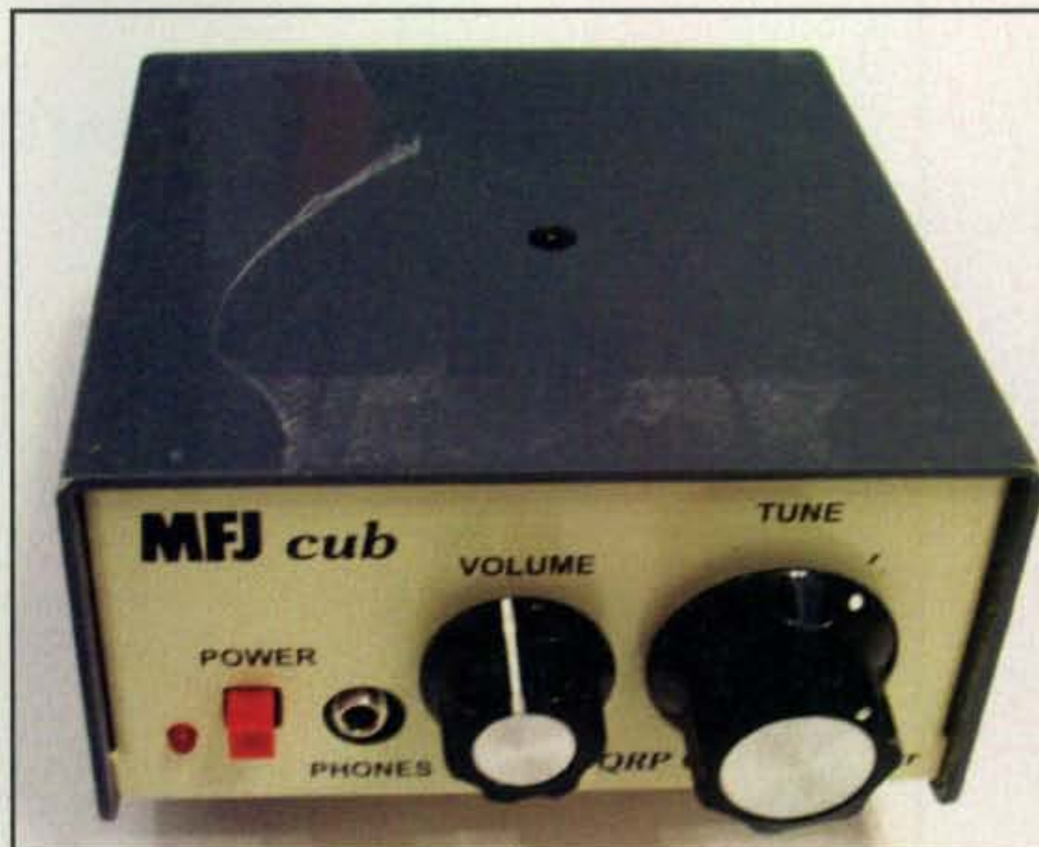
Photo 10— The MFJ Cub is a popular and quite versatile QRP transceiver that usually produces a 2-watt output signal. A simple power transistor change as described in the text increases output to 3 or 4 watts for reaching out like a pro. (Photo courtesy of MFJ Enterprises)
