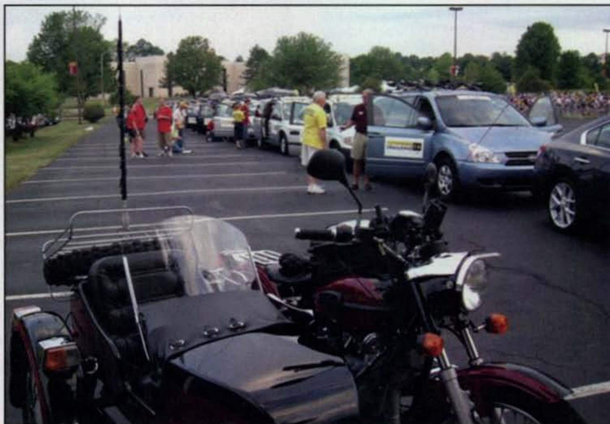
Clay Owen, AA3JY, went mobile using a Kenwood D7A (APRS) mounted on the handle bar, a Garmin ZUMO 550 (no NMEA output) mounted on the handle bar for mapping, a Garmin GPS V (NMEA for the D7A) mounted on Tank Bag, an ICOM 706MkIIIG control head, and external speaker mounted on the sidecar's windshield grab-hold bar. All were powered from a marine deepcycle 27D battery in the sidecar trunk. (Photo courtesy of N3LJZ)
