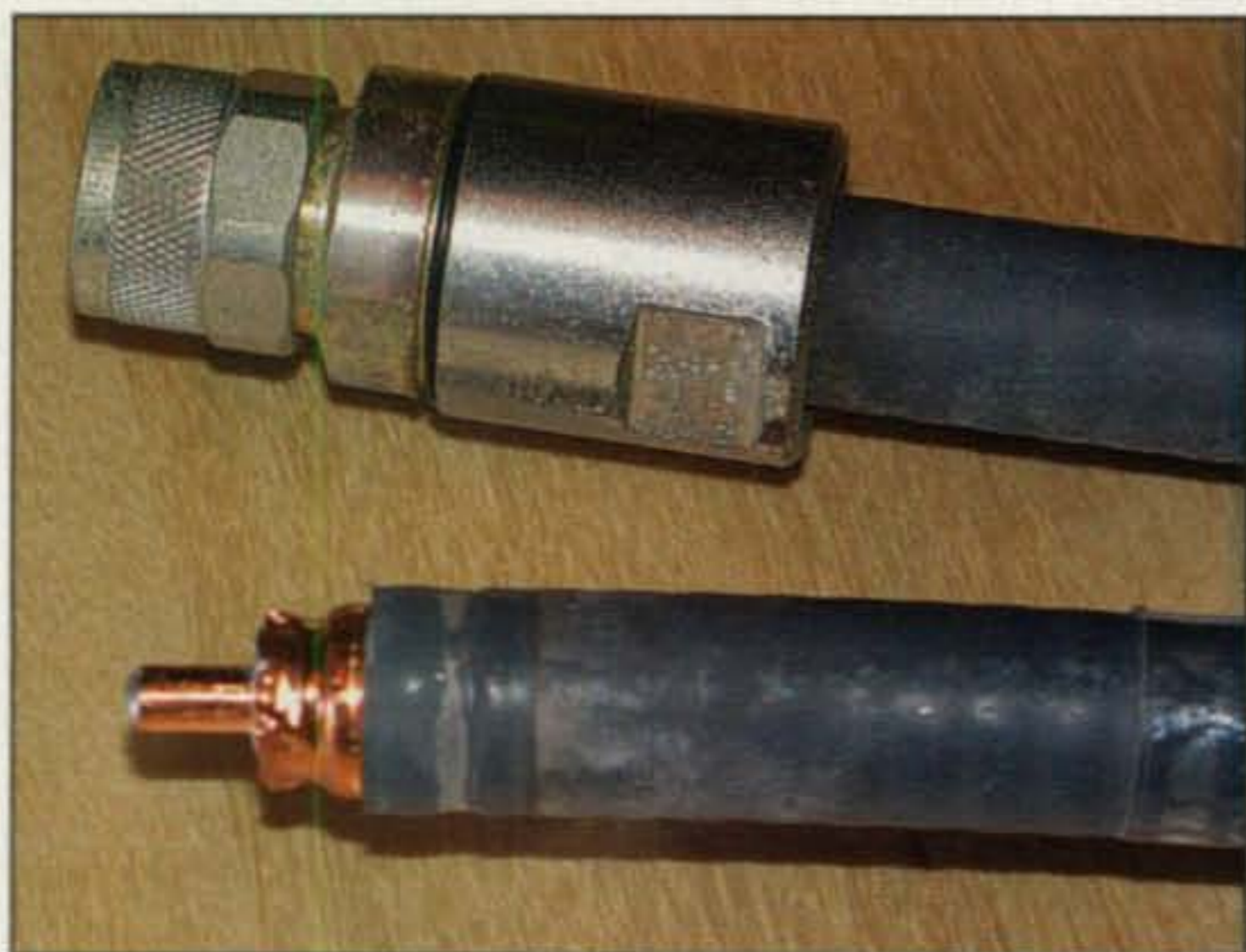
Photo 1—A very low-loss coax-cable type is called hardline . In this cable, the outer shield is made of solid copper, rather than woven wire braid. This type of cable is used on VHF-and-above frequencies and is particularly useful when long runs are needed.
