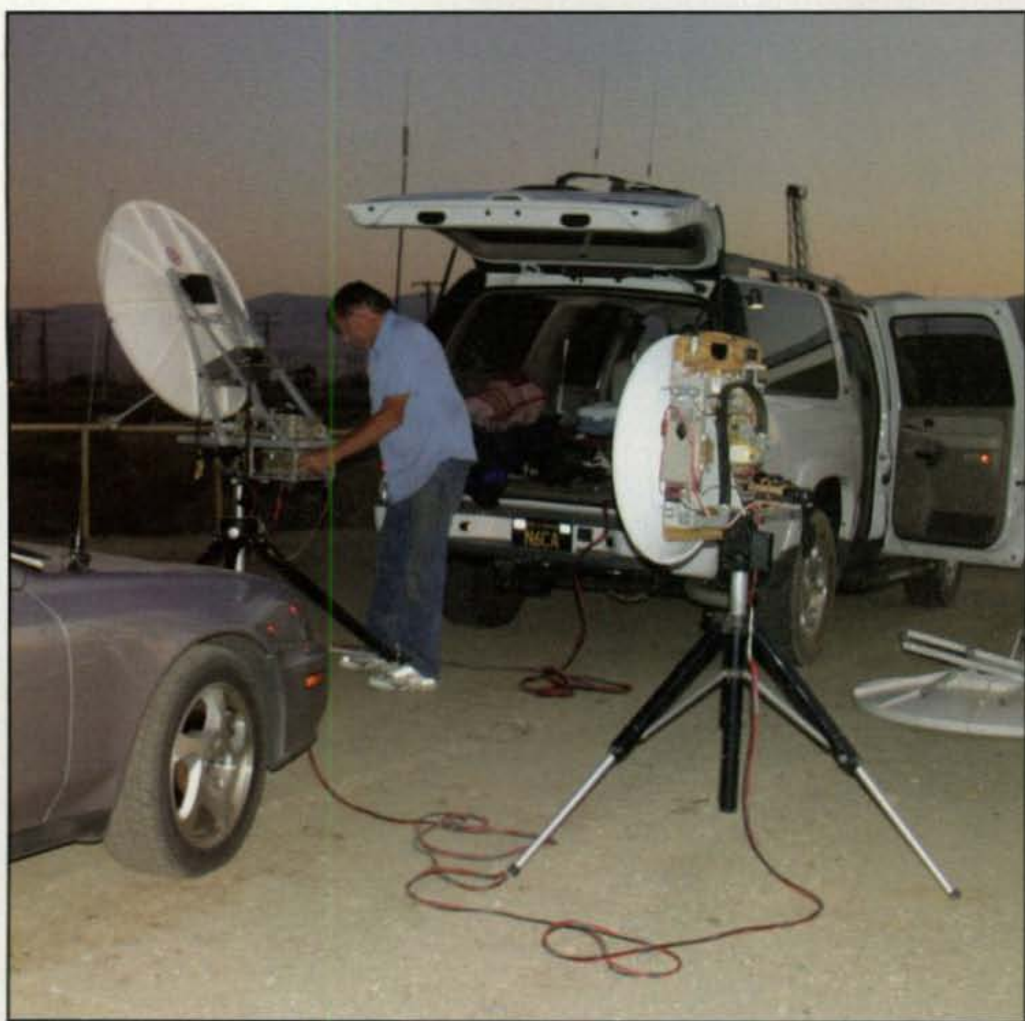
Photo 3— In this not-so-typical radio setup the rig is located far away from the power source (car battery). The voltage drop at the radio end of the long cable can be enough to cause the radio system to malfunction. Minimize this loss and maximize performance by using a cable made with thick wires.
