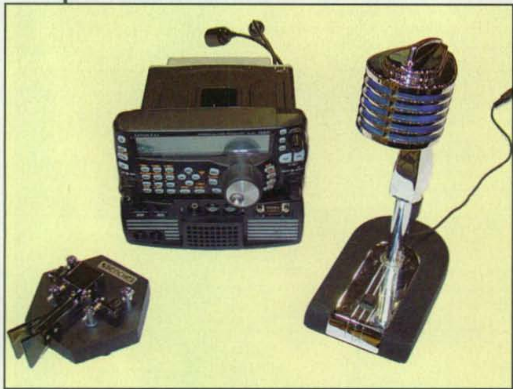
Photo 1— There is no better way to rekindle your interest in amateur radio than with a new rig, a new antenna, and/or new mic and key. As shown by the Kenwood TS-480, Bencher Hex key, and Heil FIN microphone shown here, the endeavor can also be quite affordable—and reward you with many years of enjoyable operation.
