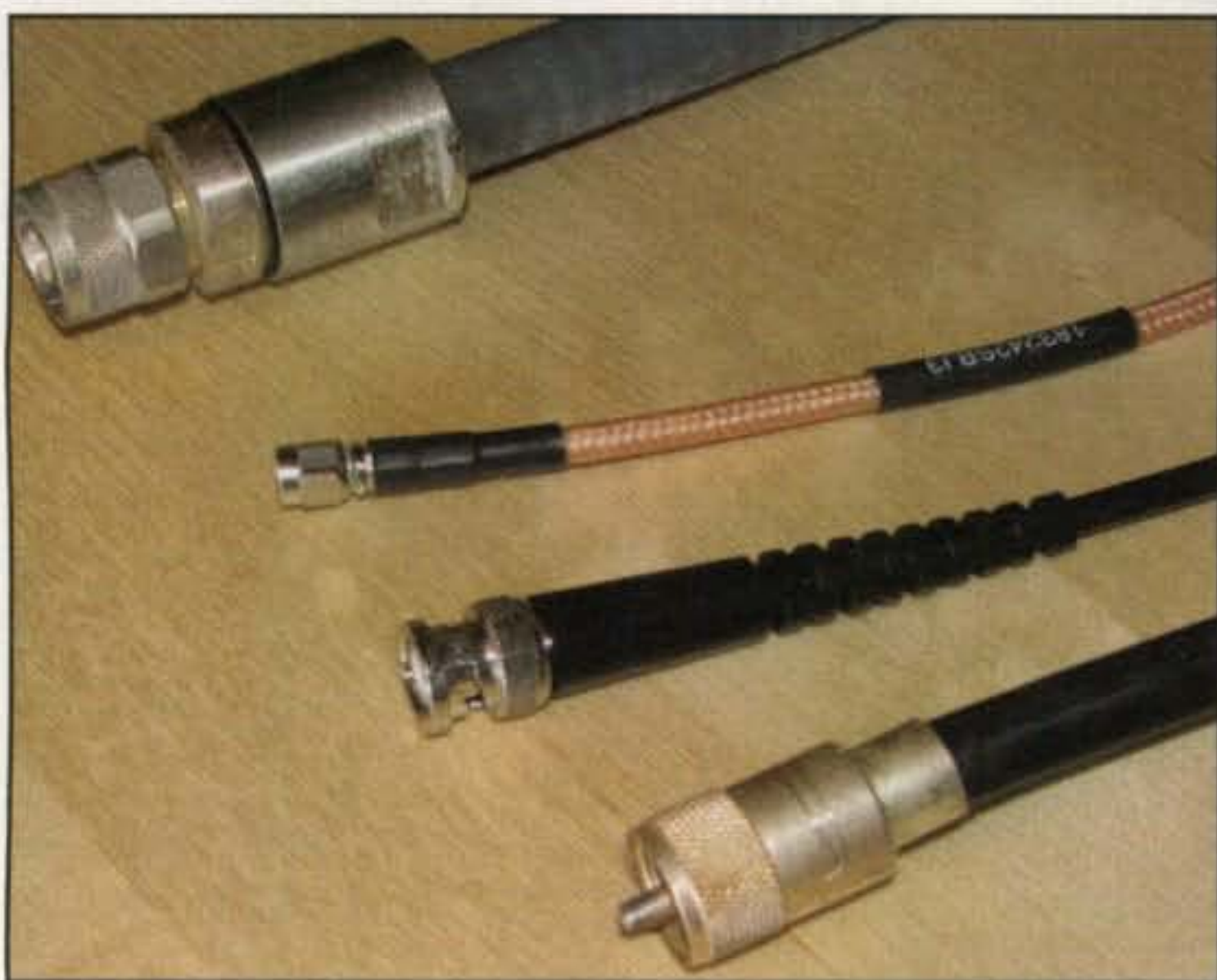
Photo 2— From bottom right to upper left, typical cables and connectors found on ham radio gear: PL-259 on RG-213, BNC on RG-58, SMA on some sort of very flexible cable, and Type N on 1/2-inch hardline.
