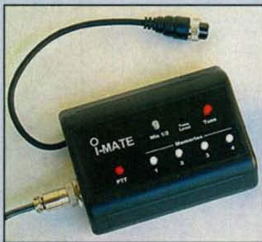
Photo A— BetterRF's I-Mate implements the external selection of pre-recorded voice and keyed messages for many of the recent ICOM rigs.
