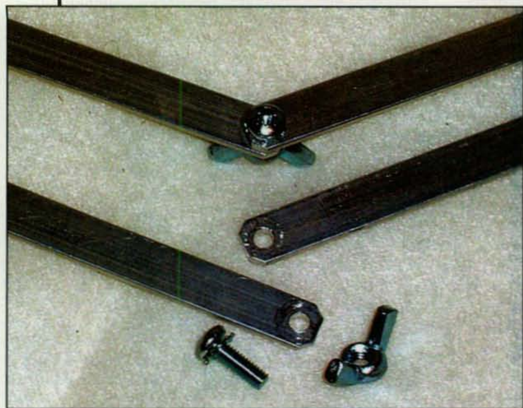
Photo A— Low-resistance contact points.
