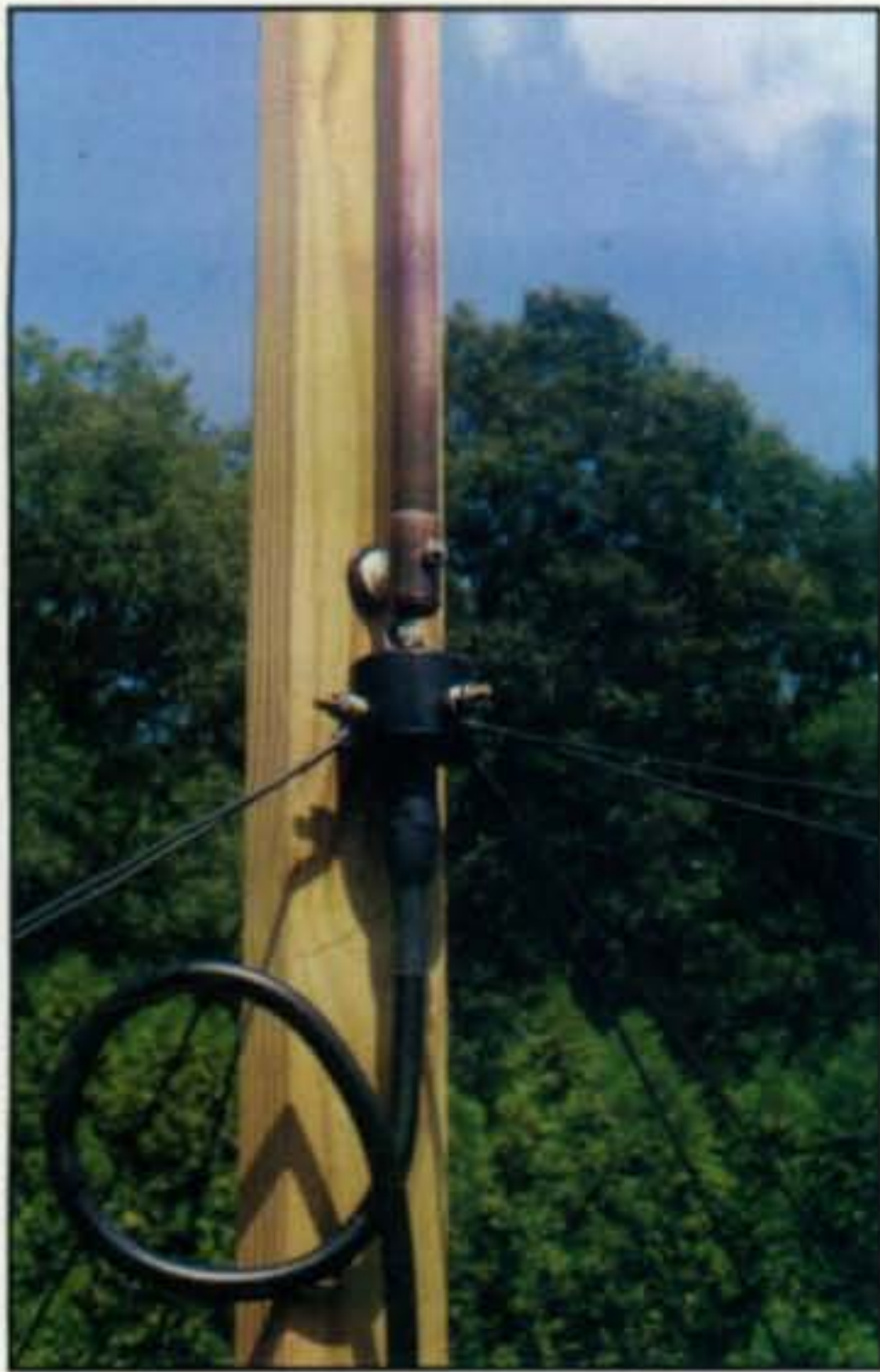
Photo F— Mounting detail of the feed unit. It is attached to the vertical radiator with coax shield. There are four pairs of radials creating the ground plane.
