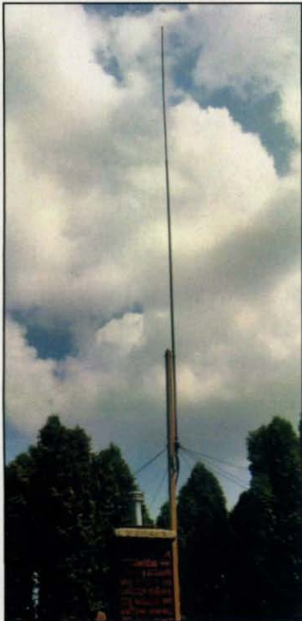
Photo A— K3KR's elevated 20-meter ground plane. Note that this photo was taken before the top hat was added. (All photos by the author)
