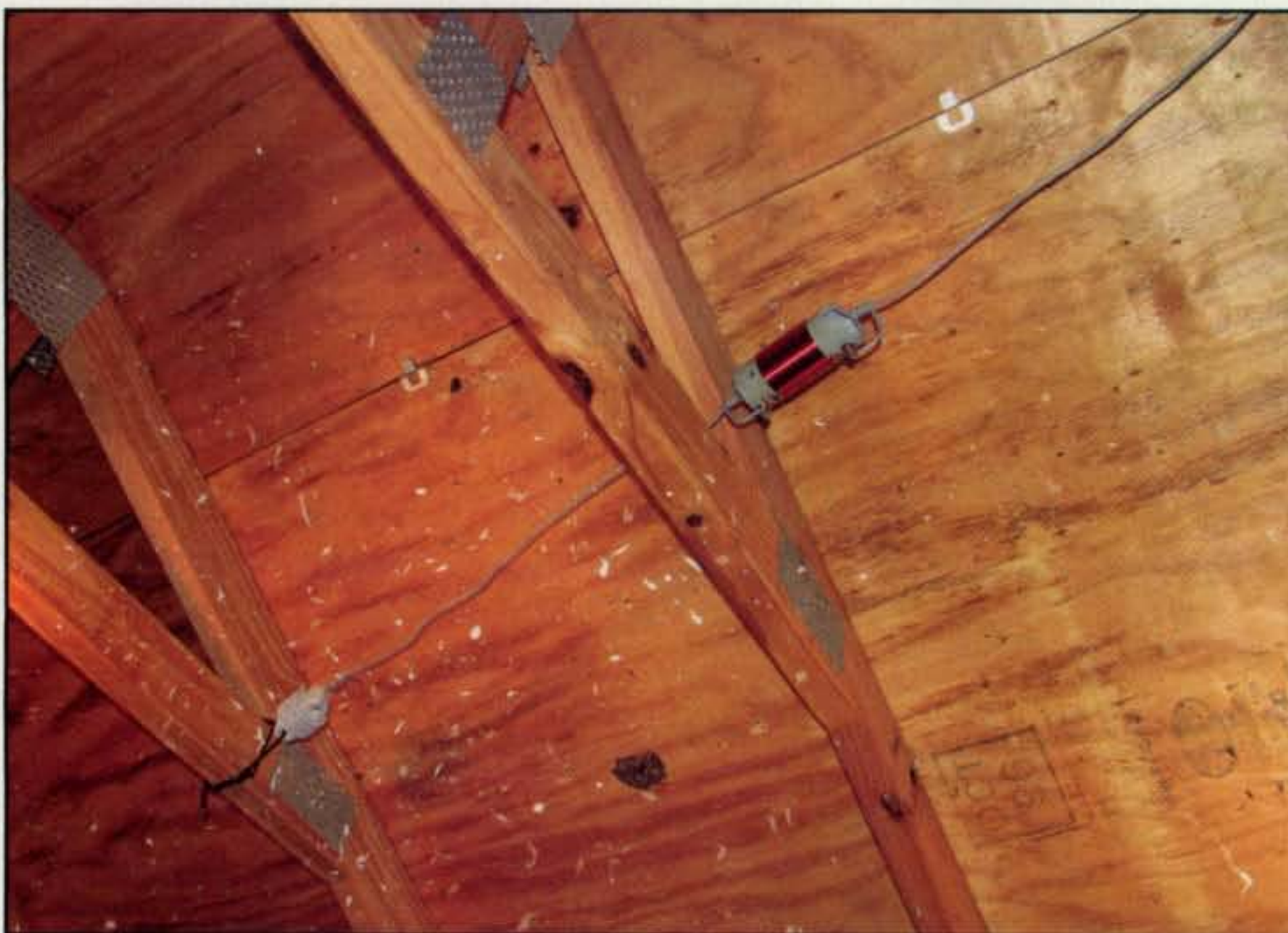
Photo D— Photographing a doublet strung in an attic is a formidable challenge, but Joan Jones, W4JMJ, accomplished the feat to show us part of her secret pride. Like N6SL and other amateurs who are sidestepping antenna restrictions, she too confirms low-height antennas can reach out surprisingly well. (Photo courtesy of W4JMJ)
