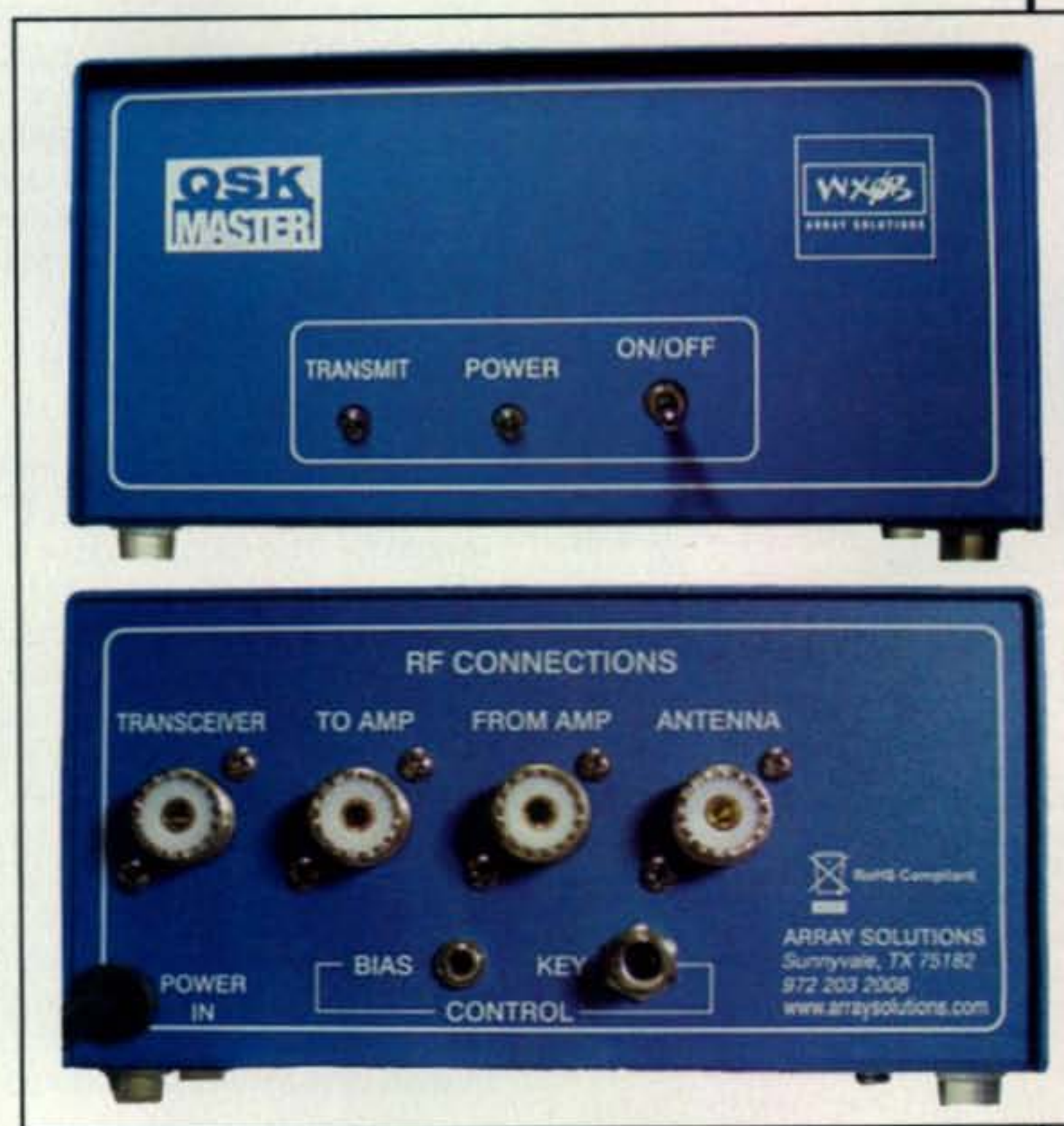
Photo A— Array Solutions' QSK MASTER is a 160-6 meter, 2500-watt, continuous-power external QSK switch.
