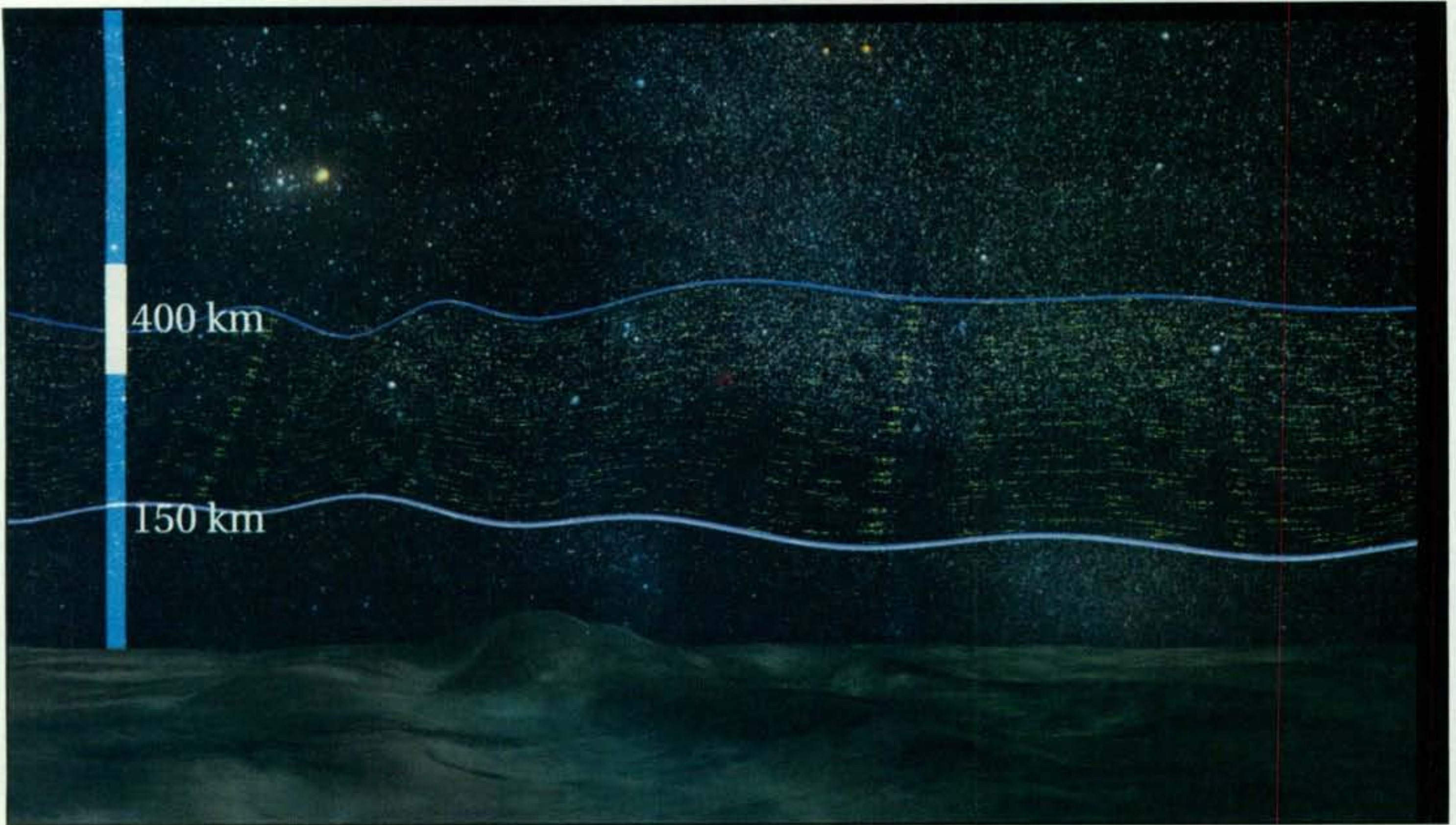
Fig. 2— This graphic shows that the ion density of the ionosphere practically disappears during the night. With the current unexpected low level of the boundary between space and the Earth's atmosphere, the distance of the propagation of radio waves off the ionosphere is much shorter than if the ionosphere were higher. (Credit: NASA/Goddard Space Flight Center)
