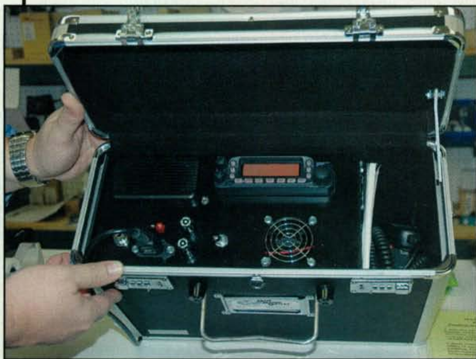
Photo A— A 1950s' era marketer might have referred to this as "Box 'o Radio to Go." It's a nicely designed, "all in one," portable package of power supply, radio, external speaker, and easy power and antenna connections assembled by Harry, KG6OTW. (KD6ARA photo)
