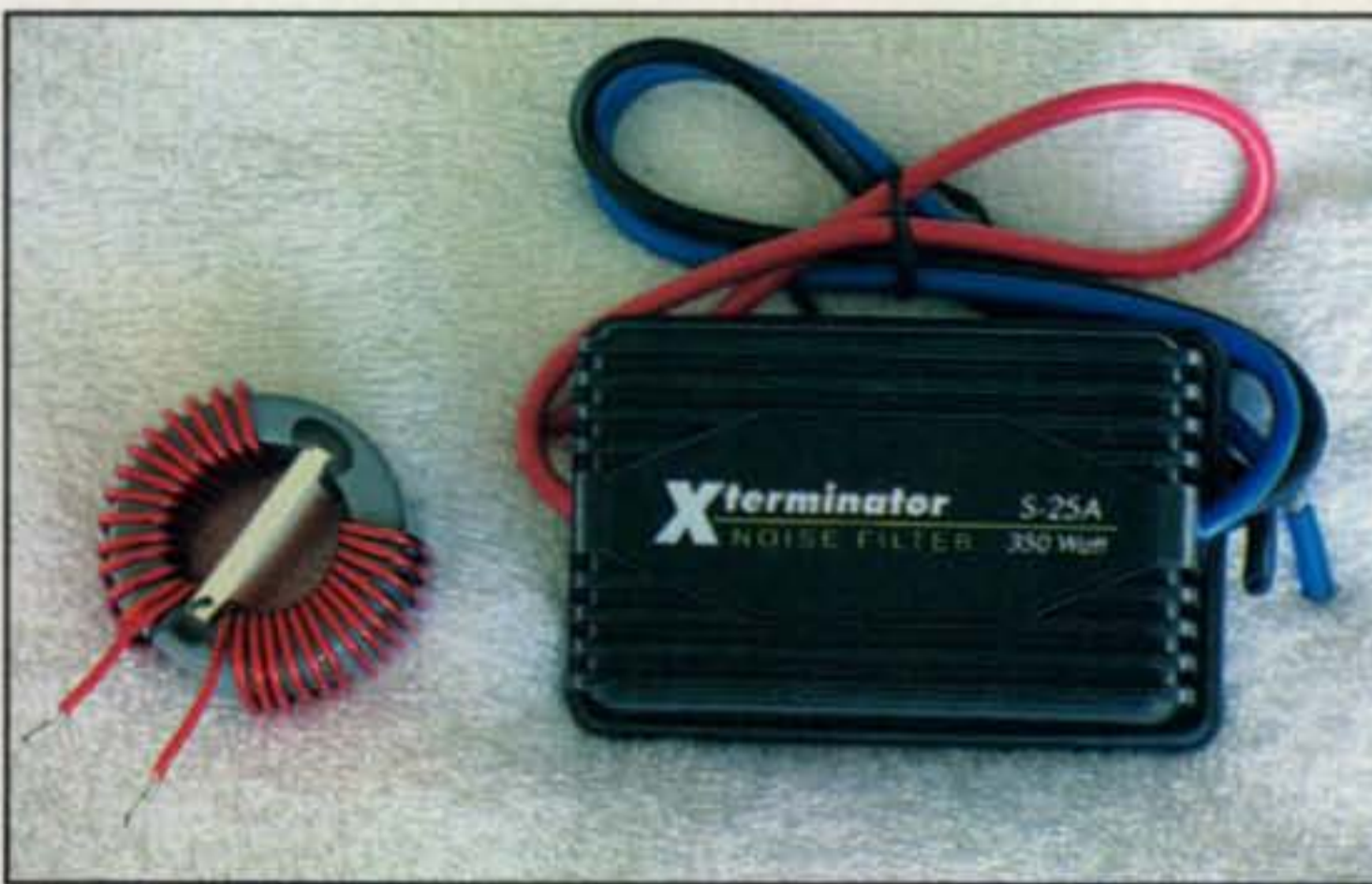
Photo C— A choke can sometimes be used to filter the DC line and minimize noise. A store-bought filter is a more elegant way to filter the DC line. Check with your favorite radio dealer for a recommendation.
