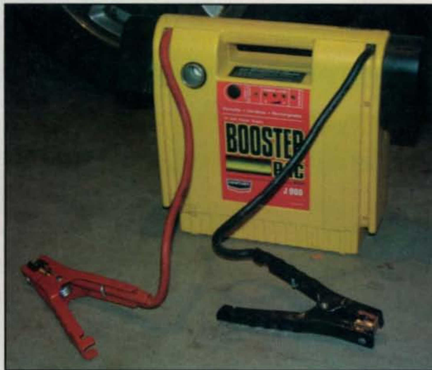
Photo B— A booster battery like this can be used to power a mobile rig temporarily as you make tests and adjustments. Be very careful not to short the positive terminal to any electrical ground!
