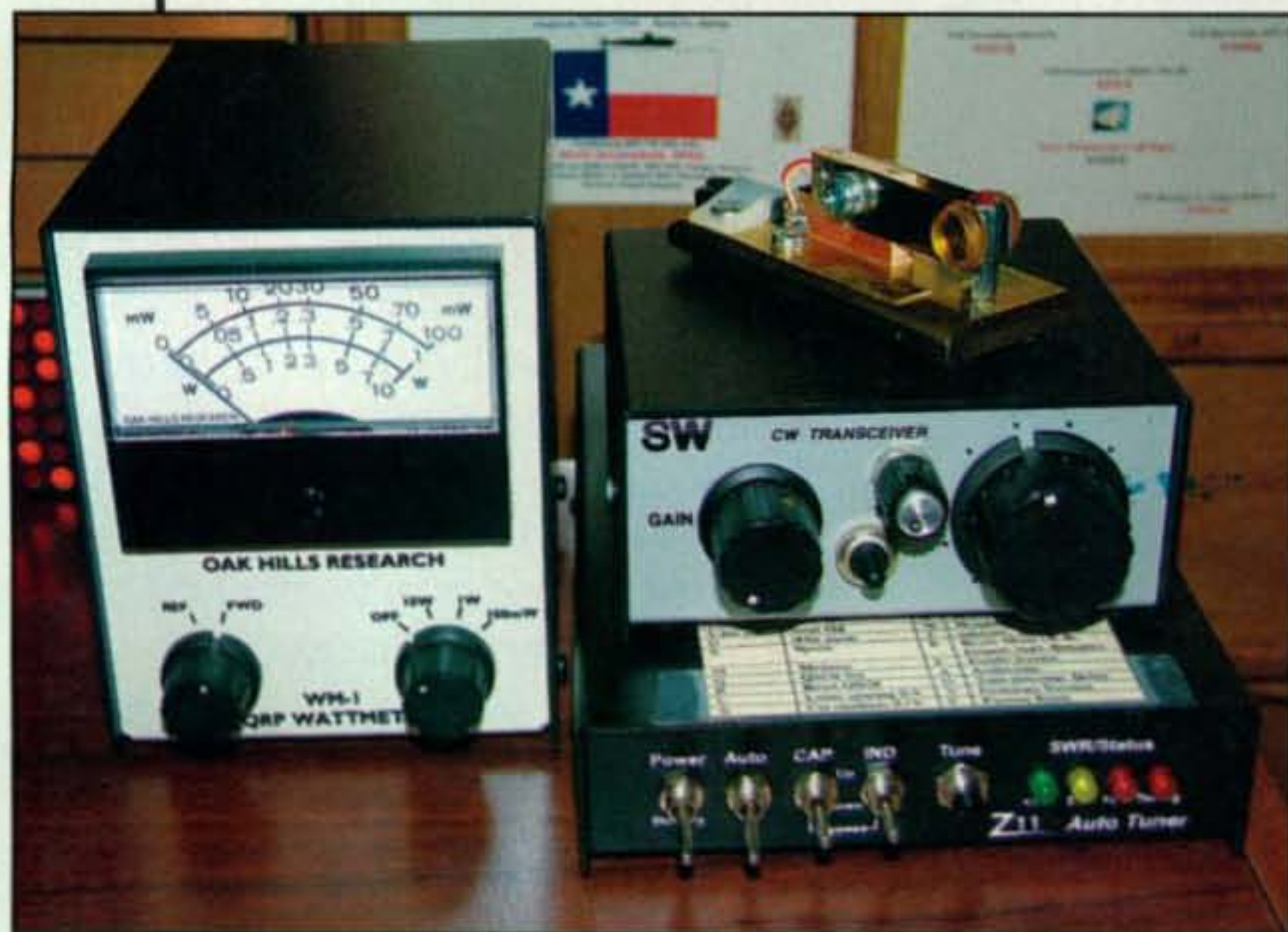
Photo A— Once again proving QRP is big-time fun in a small-size package, Pete Haddad, W5PEH, has worked numerous states plus several countries with this palm-size 40-meter Small Wonders transceiver and LDG Z11 tuner. He also uses it with a homebrew audio amplifier and speaker for easy in-shack band monitoring. Nice! (Photo via Pete, W5PEH)
