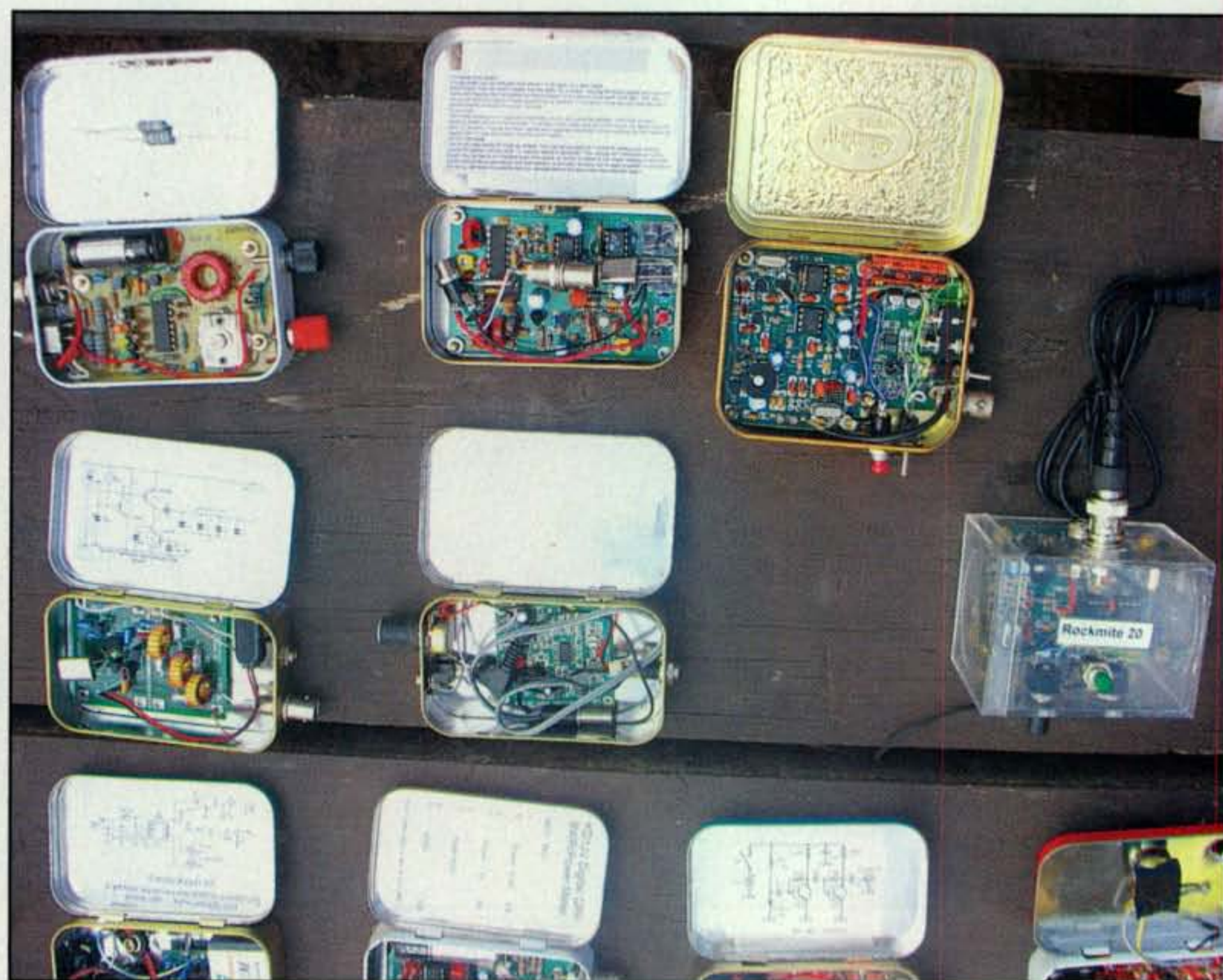
Photo J— Like any good QRP meet, Lobstercon also had its share of rigs built in Altoids® tins on display. This is only a small sampling of the little delights. You know it is QRP if it is in an Altoids tin!
