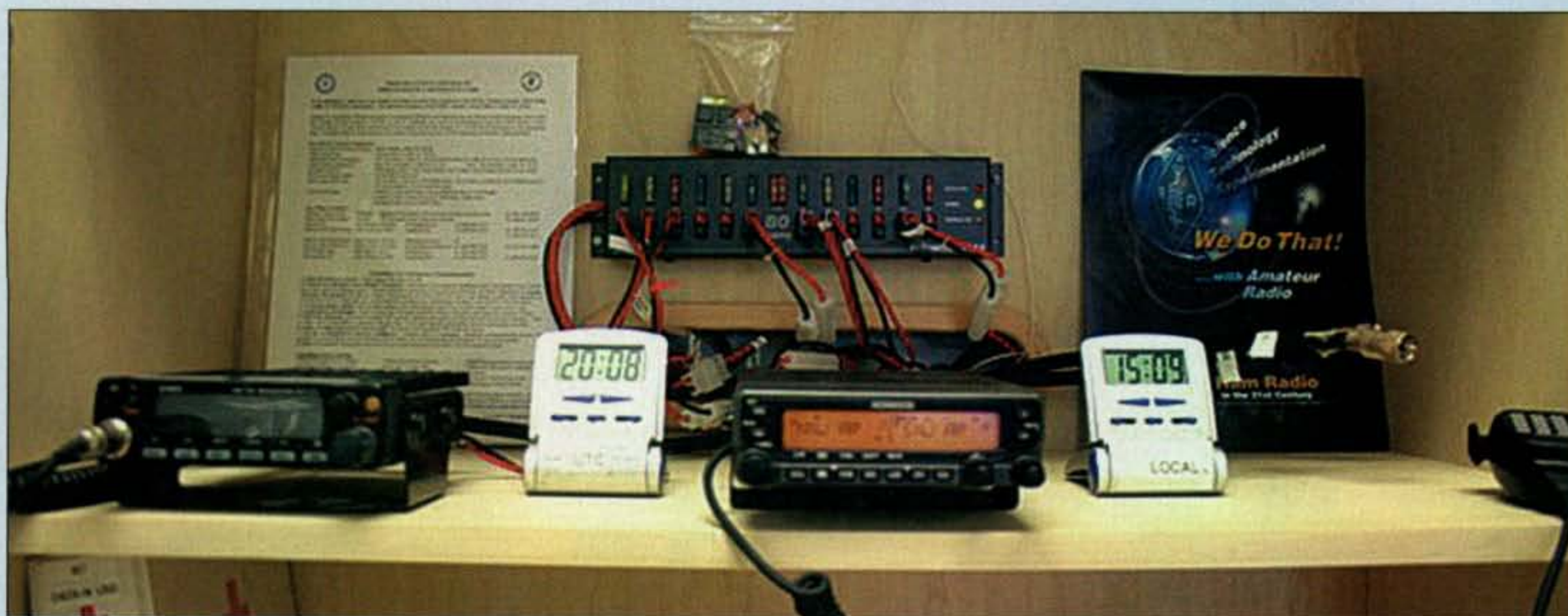
The Mercer County ARES/RACES communications unit also includes shelter kits designed and built by Gary Wilson, K2GW. This unit holds a 2-meter FM rig, an Astron switching power supply, and a magnetic-mount antenna. (Photo courtesy N2GJ)
