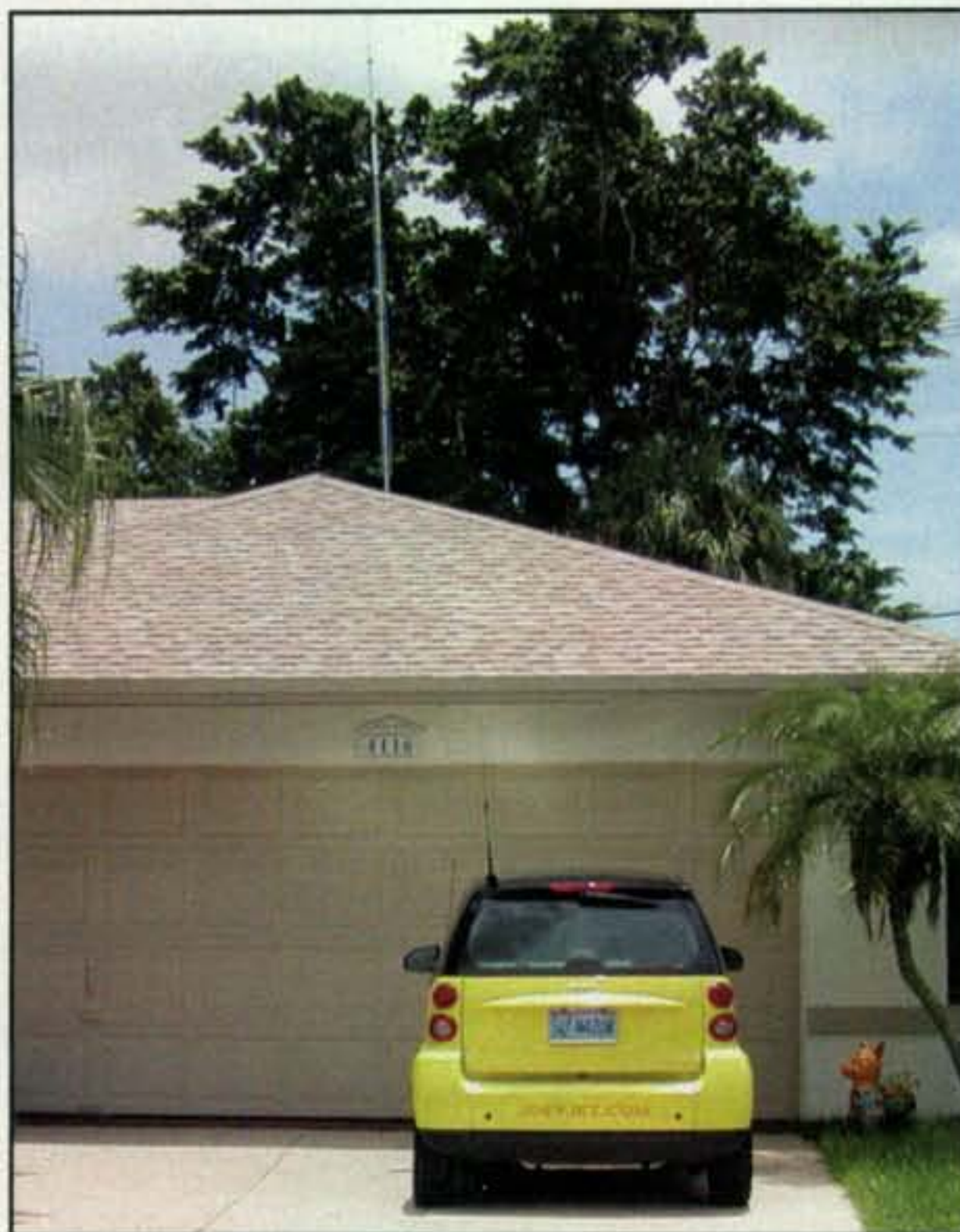
Photo 1— This mild-mannered Cushcraft R-8 vertical at the home of Joey Jet, N4ZUW, is probably the most high-profile antenna one can hope to use in a CC&R-limited community. Make no mistake here, however; a 3/8 - and/or 1/2 -wave vertical is cost-effective, does not require an extensive radial system, and its performance is often comparable to a 2-element beam. Check <www.joeyjet.com> (shown on bumper of Smart Car) to see Joey flying stars and VIPs nationwide.
