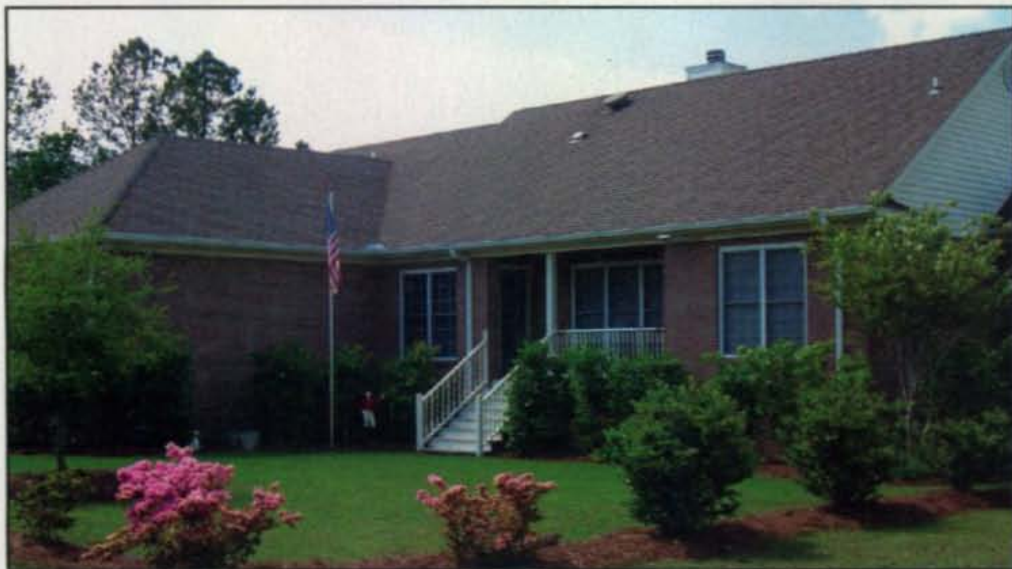
Photo 3— You are looking at the CC&R-regulated home and multiband antenna system of Jeff, K8CQ. What and where is the antenna? It is a short vertical with a giant capacity hat, and it is disguised as a prim and proper white rain gutter routing around the house at the roof's edge. Yes it works well. Jeff has contacted over 200 DX entities with it.
