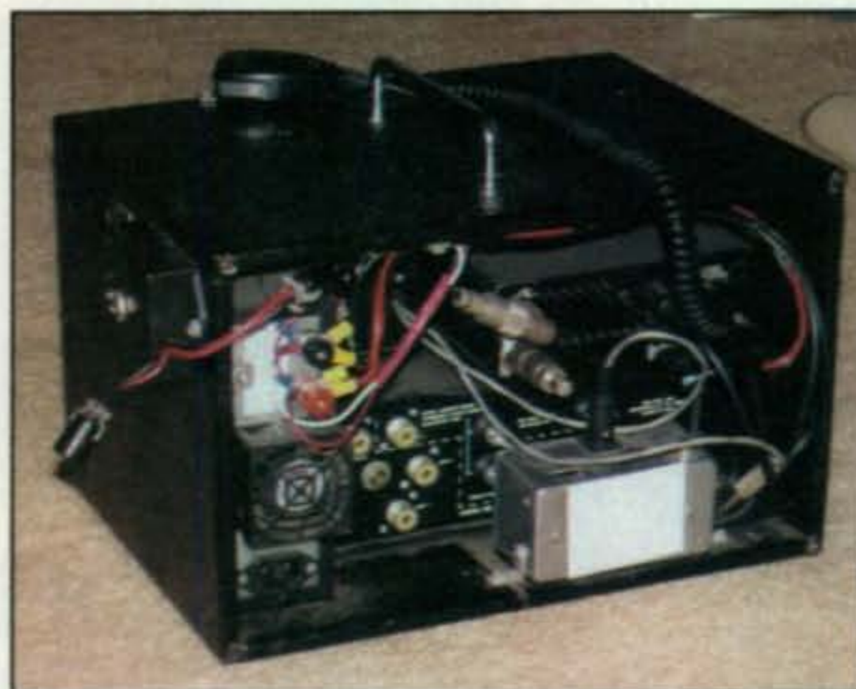
Photo B— Rear view of the box. You can see the connections as well as the interface box and the outboard antenna control switch.
