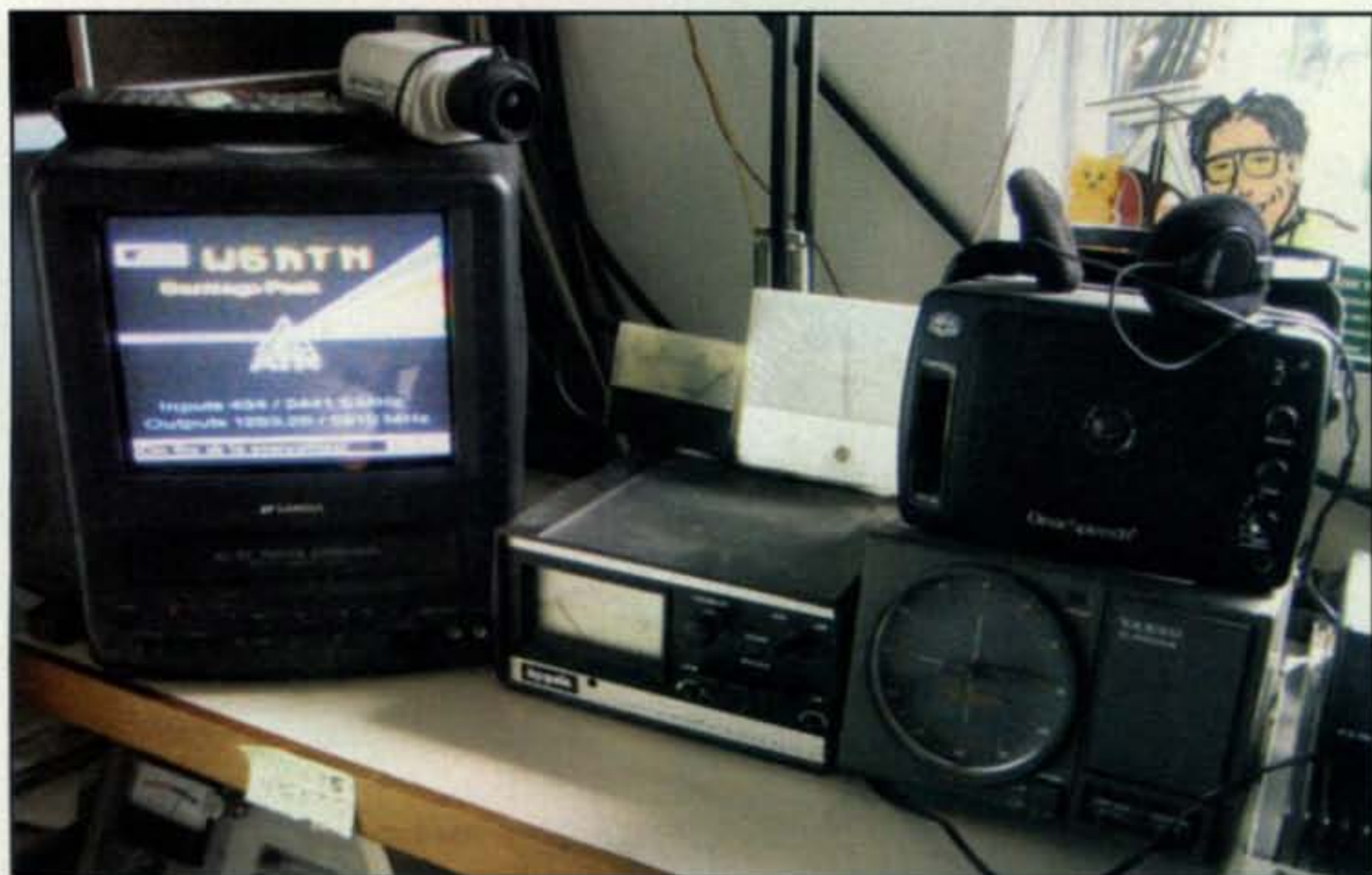
The author's ATV station monitoring an ATV repeater. You may be able to find a good camera cheap or in the trash if someone is getting rid of a camcorder with a mechanical tape drive problem. Chances are the camera part will still work fine. Then all you will need for full two-way video capabilities is an ATV transmitter.
