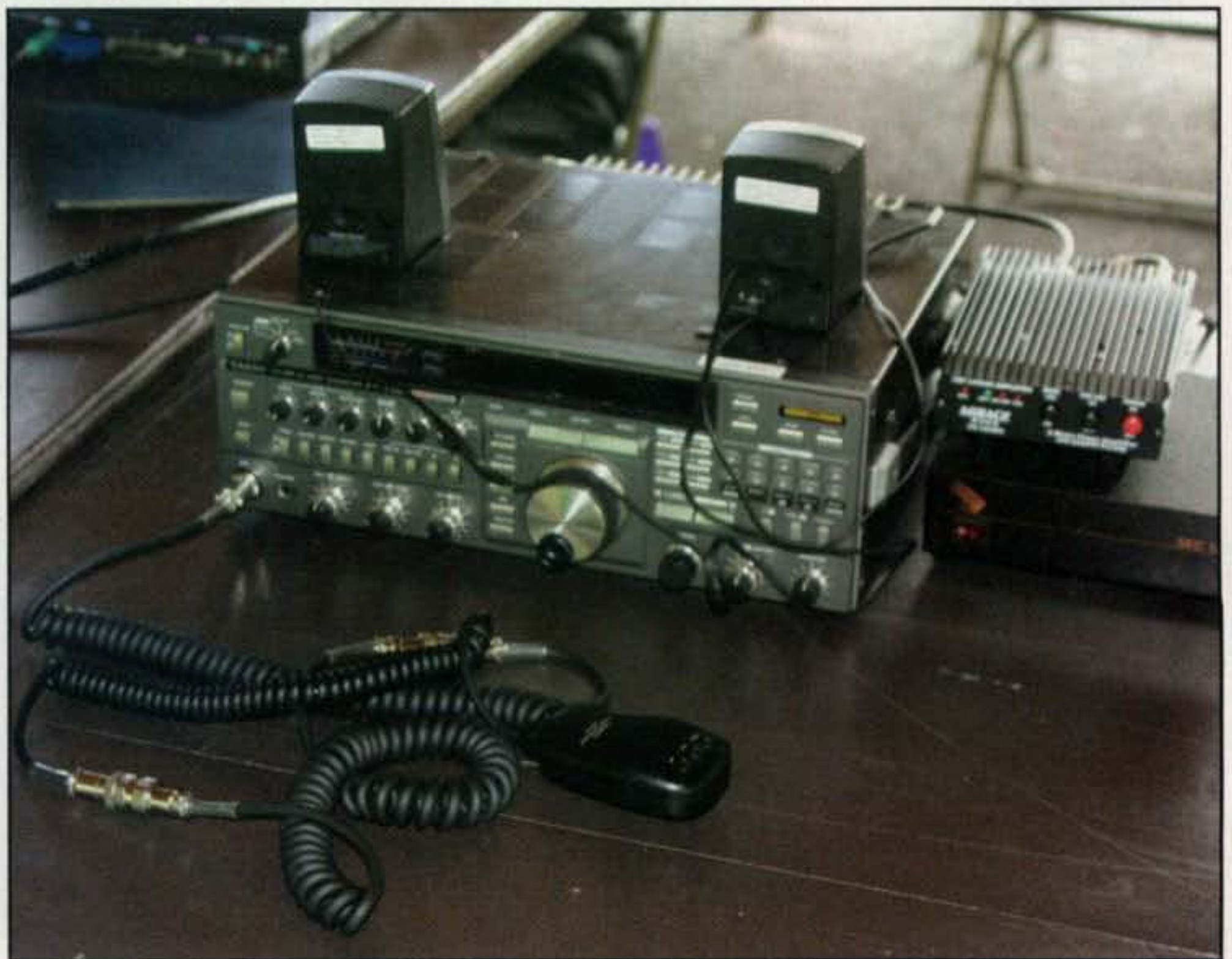
Photo B— The radio setup for the contact with the International Space Station. Note the very long mic cable which allowed the mic to be taken to each child with a question.
