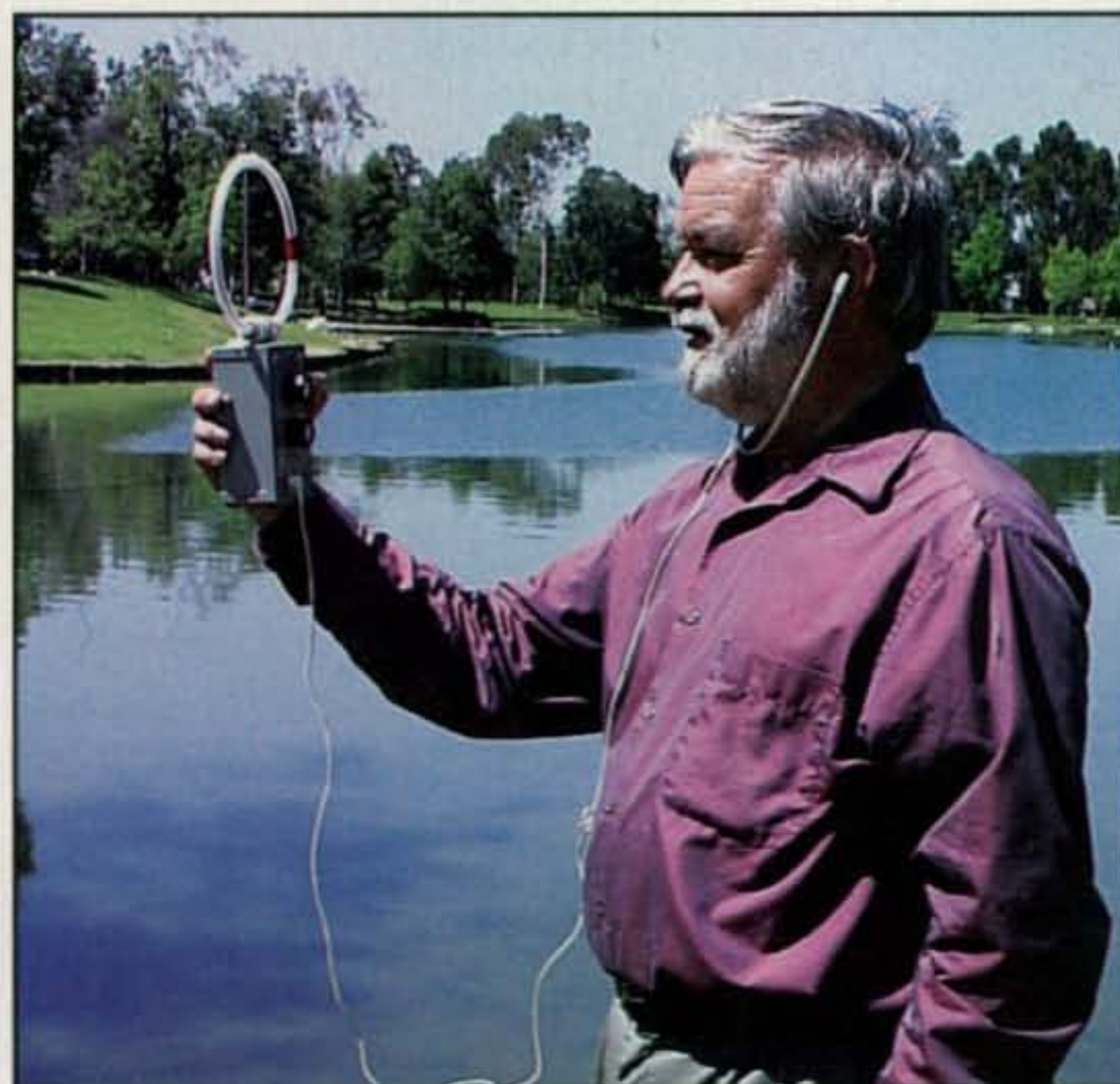
ARDF receiver/antenna sets for the 80-meter band are small and easy to carry. Plans and parts are available for home construction. Marvin Johnston, KE6HTS, tested this unit at a hunt in Placentia, California.
