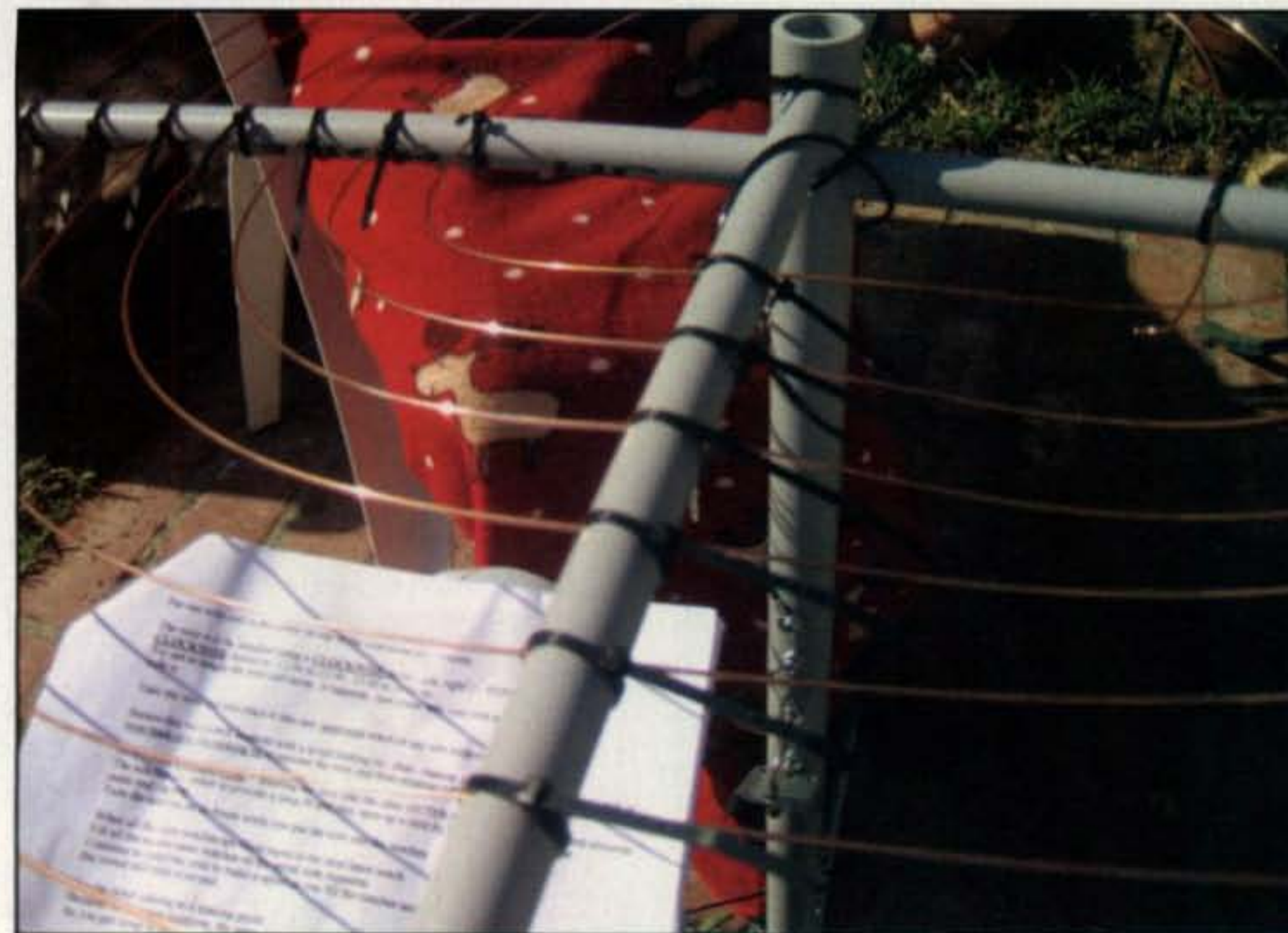
Photo C— Black plastic cable ties (provided) hold the wires in place.
