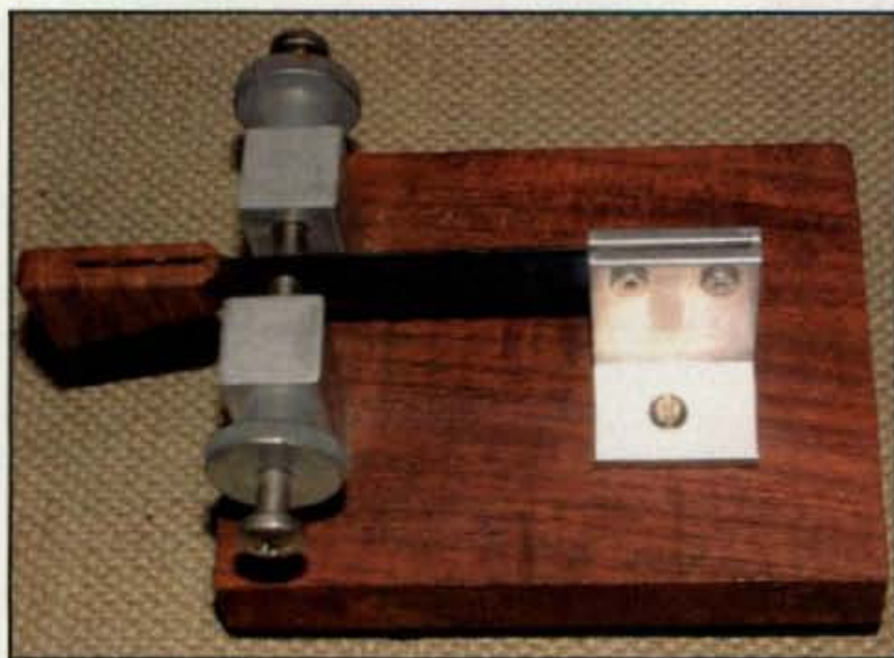
Photo 1— One of the most accurate and authentic examples of a genuine Sideswiper or Cootie key is this "Kungsimport" made in Sweden during the 1980s. Note the wood base, twin angle brackets supporting an honest-to-goodness hacksaw-blade lever (with cutting teeth intact!), and single-piece wood knob. What a heartthrob! (Photos of Kungsimport via N1EA)
