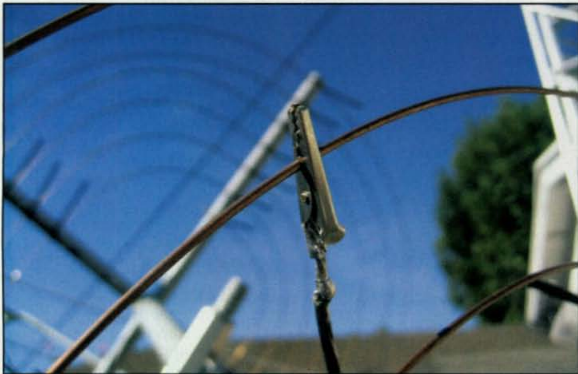
Photo D— The key to resonance is the exact placement of clip leads between the feedline and the antenna elements.
