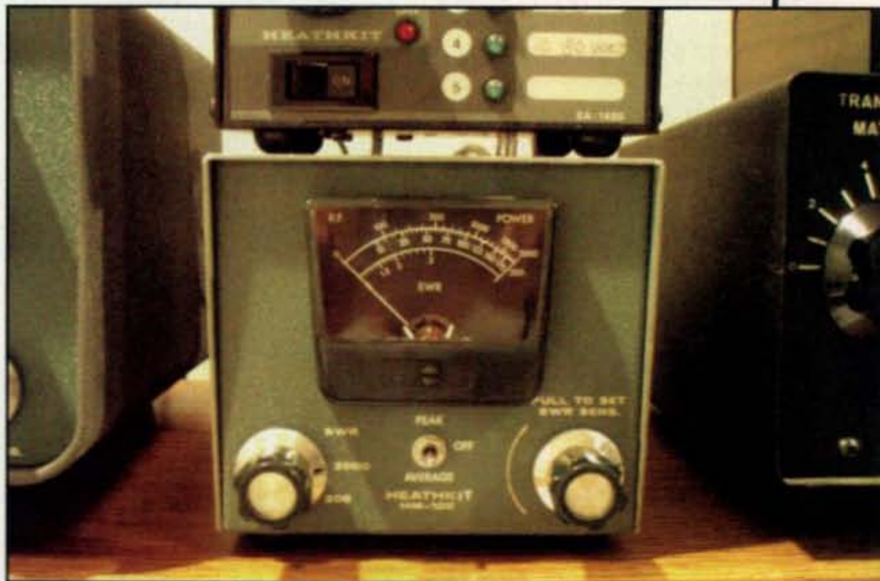
Photo A— The venerable Heathkit HM-102 SWR/Wattmeter modified for reading peak as well as average power. The only evidence on the outside is a new toggle switch and dry transfer lettering added to front of the meter base assembly, directly underneath the meter. (Photos courtesy of the author)
