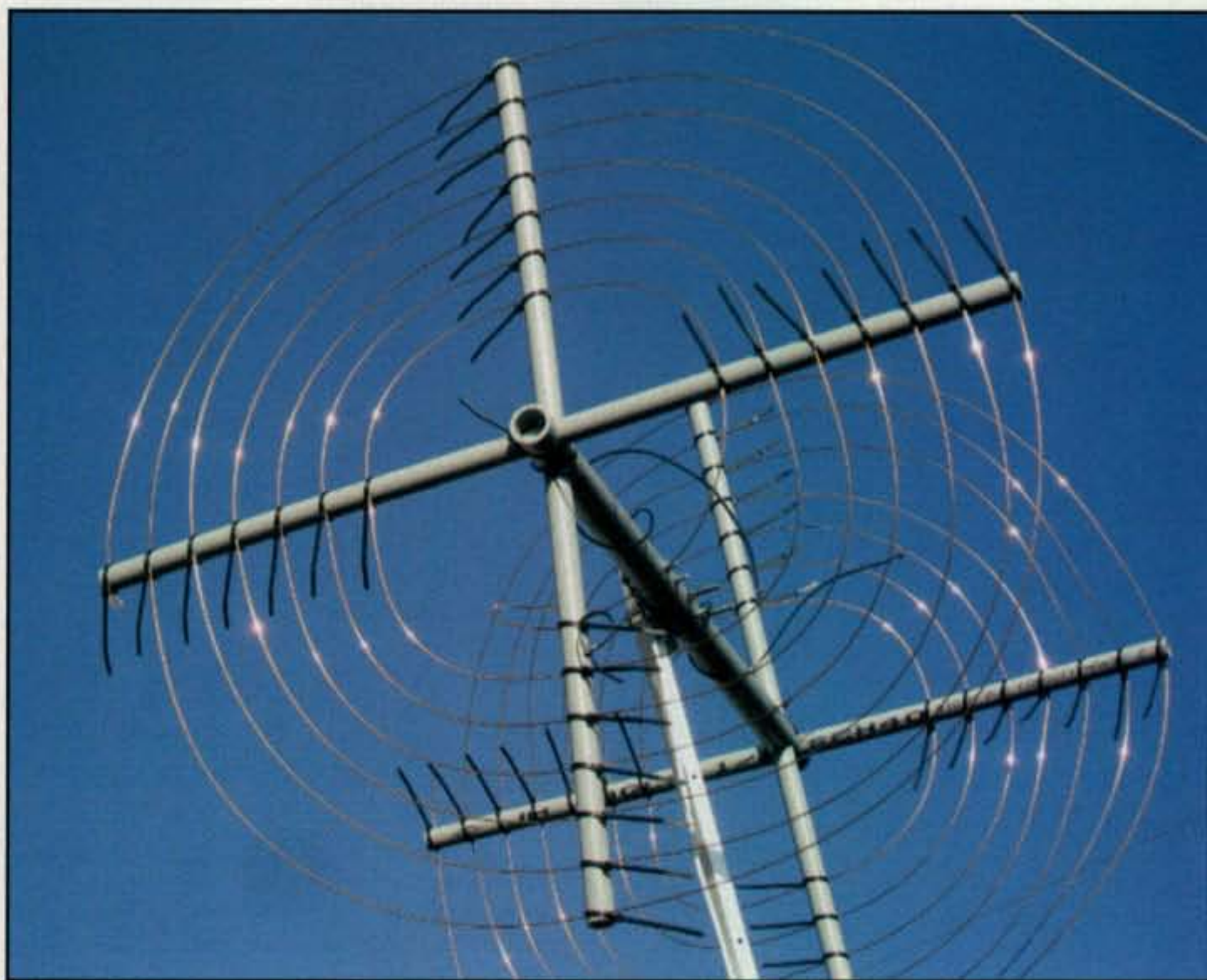
Photo A— The TAK-tenna can get you on the air from some very tight places, such as apartment balconies or campsites. This 40-meter antenna is only 26 inches from end to end, and the spiral elements are just 32 inches in diameter. (Photos by the author)
