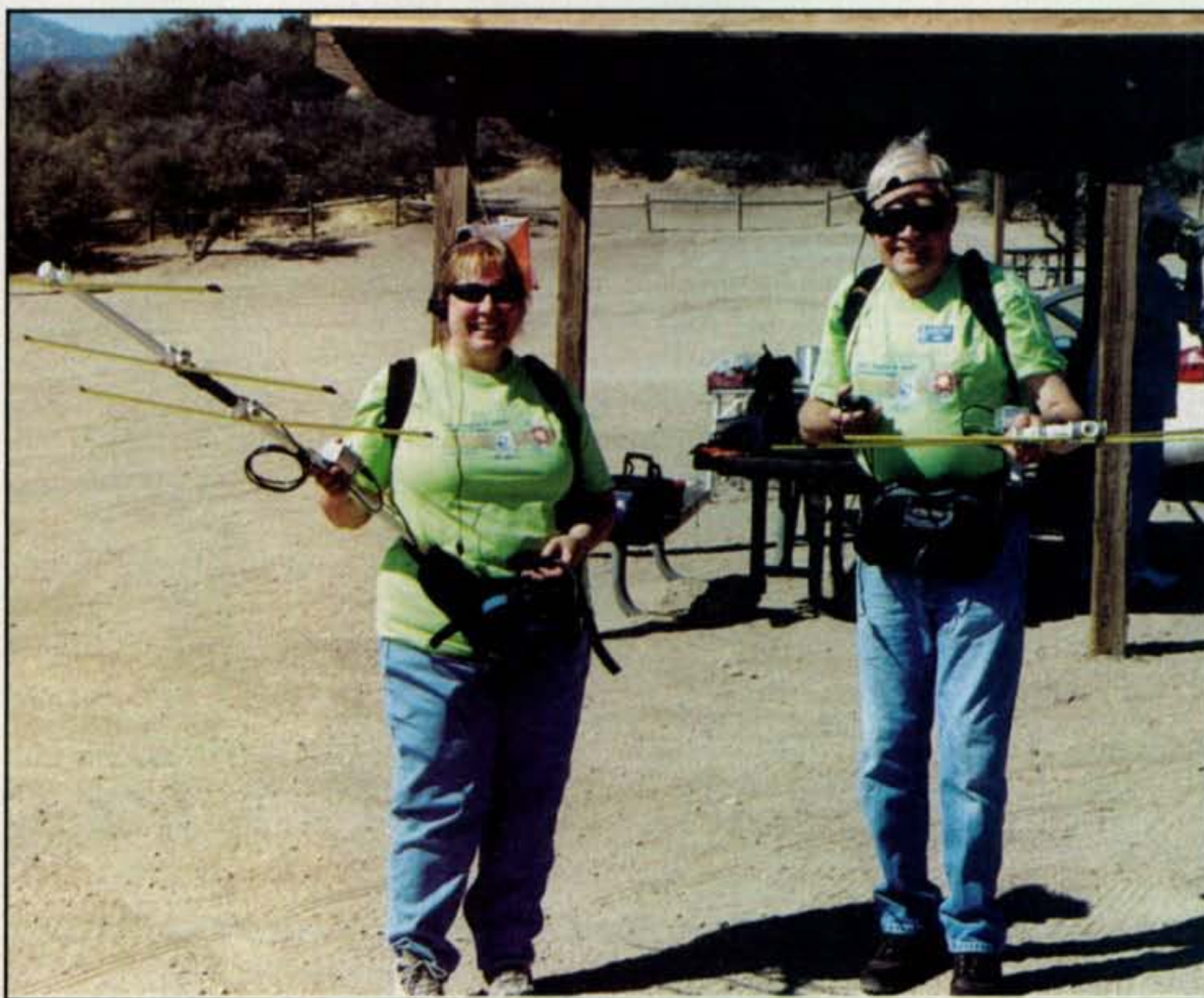
Measuring-tape Yagis and active attenuators are easy to build and are all that is needed for on-foot foxhunting with a 2-meter hand-held. Mary and Mike Cegelski, KC8YLC and K8EHP, are practicing for an ARDF championship event in the California desert.
