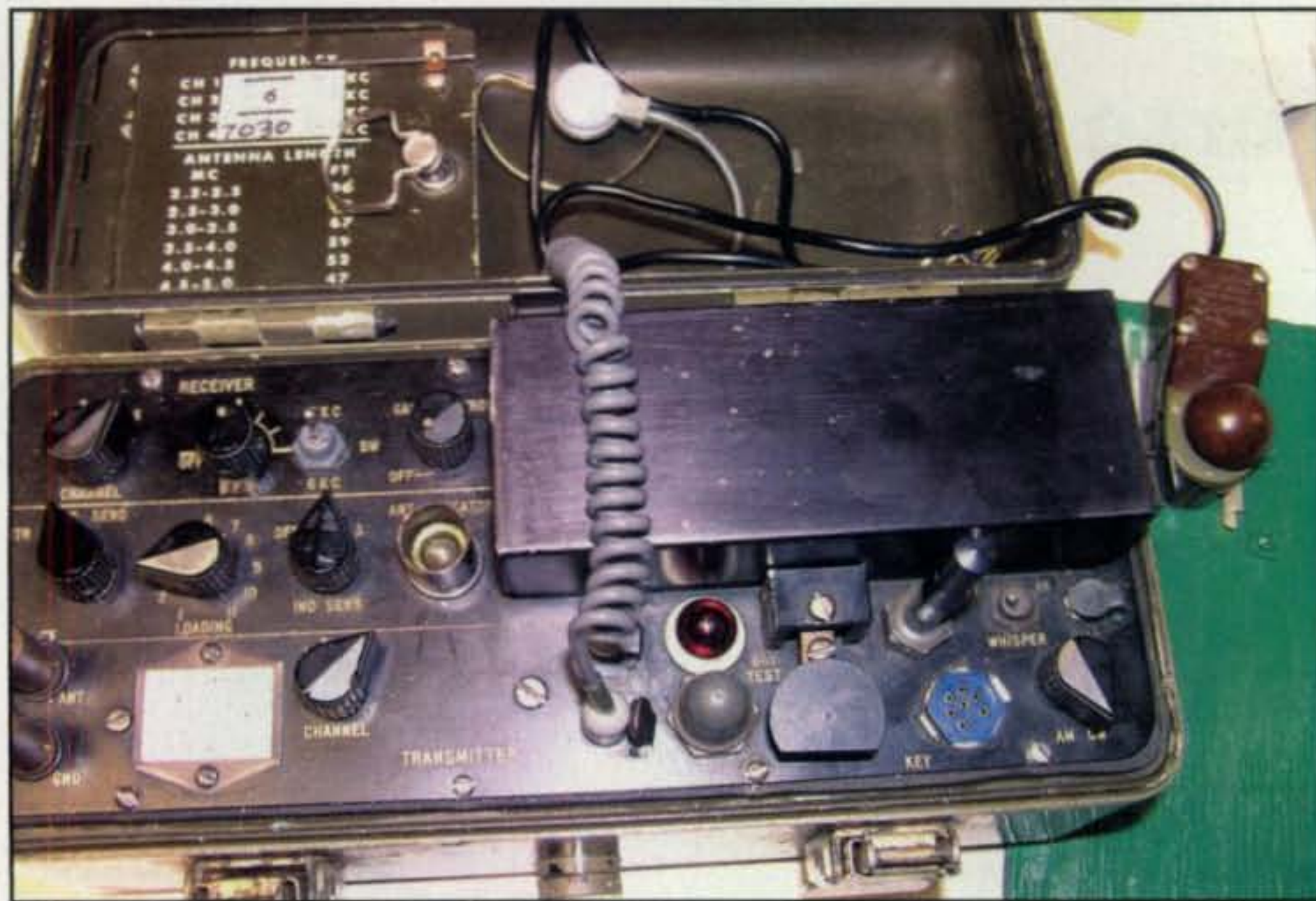
Photo 10— Close-up view of the classic PRC-64 CW transceiver. Batteries install in the bottom, the roll-up antenna plus key stores in the lid, and the little rig is easily tweaked for operation on 40 meters. It is a nice gem, if you can find one. They are scarce.
