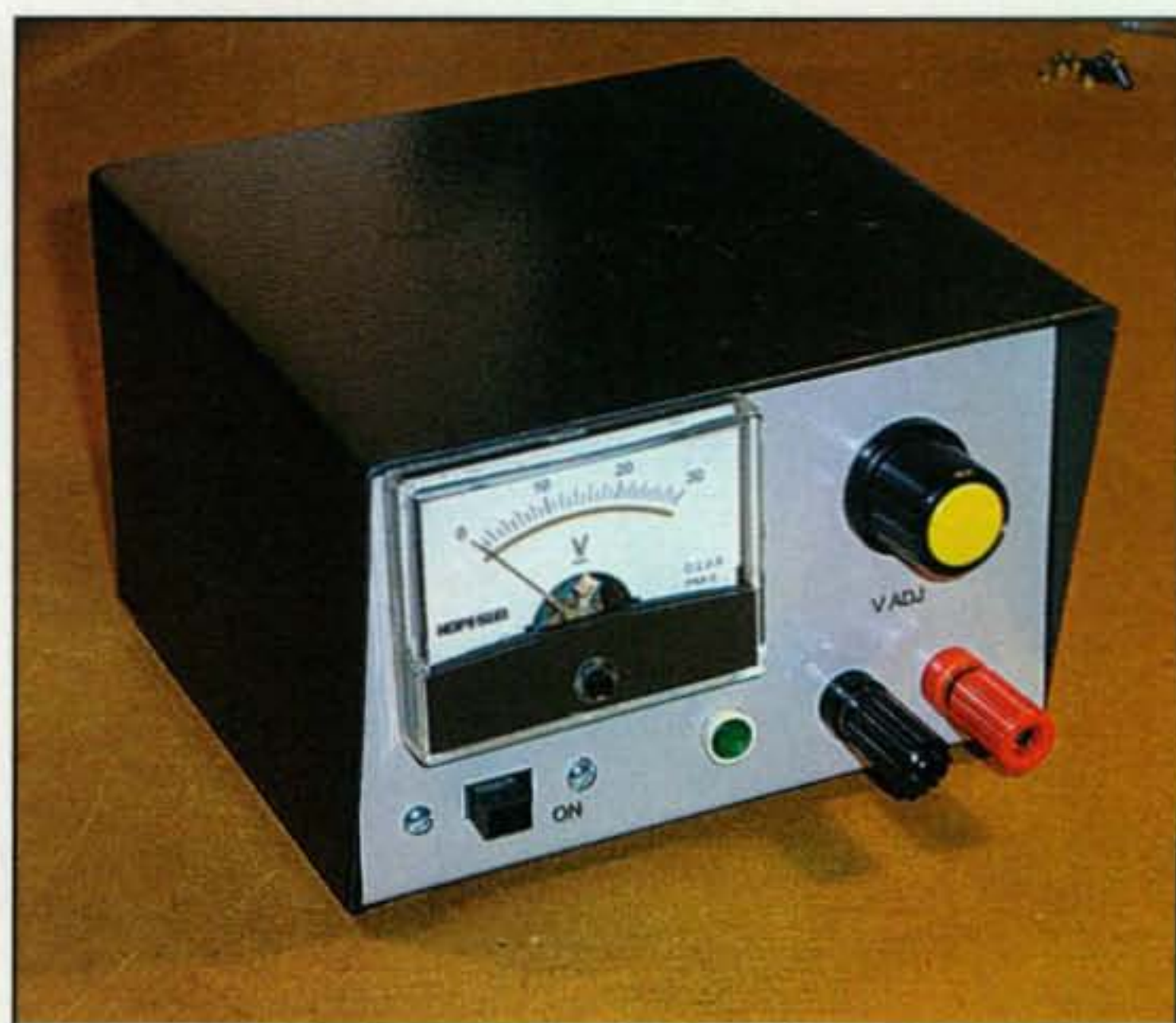
Photo E—The finished silk-purse supply looked like it was always meant to be this way. It provides up to about 0.9A of current at any voltage between about 2V and 26V.
