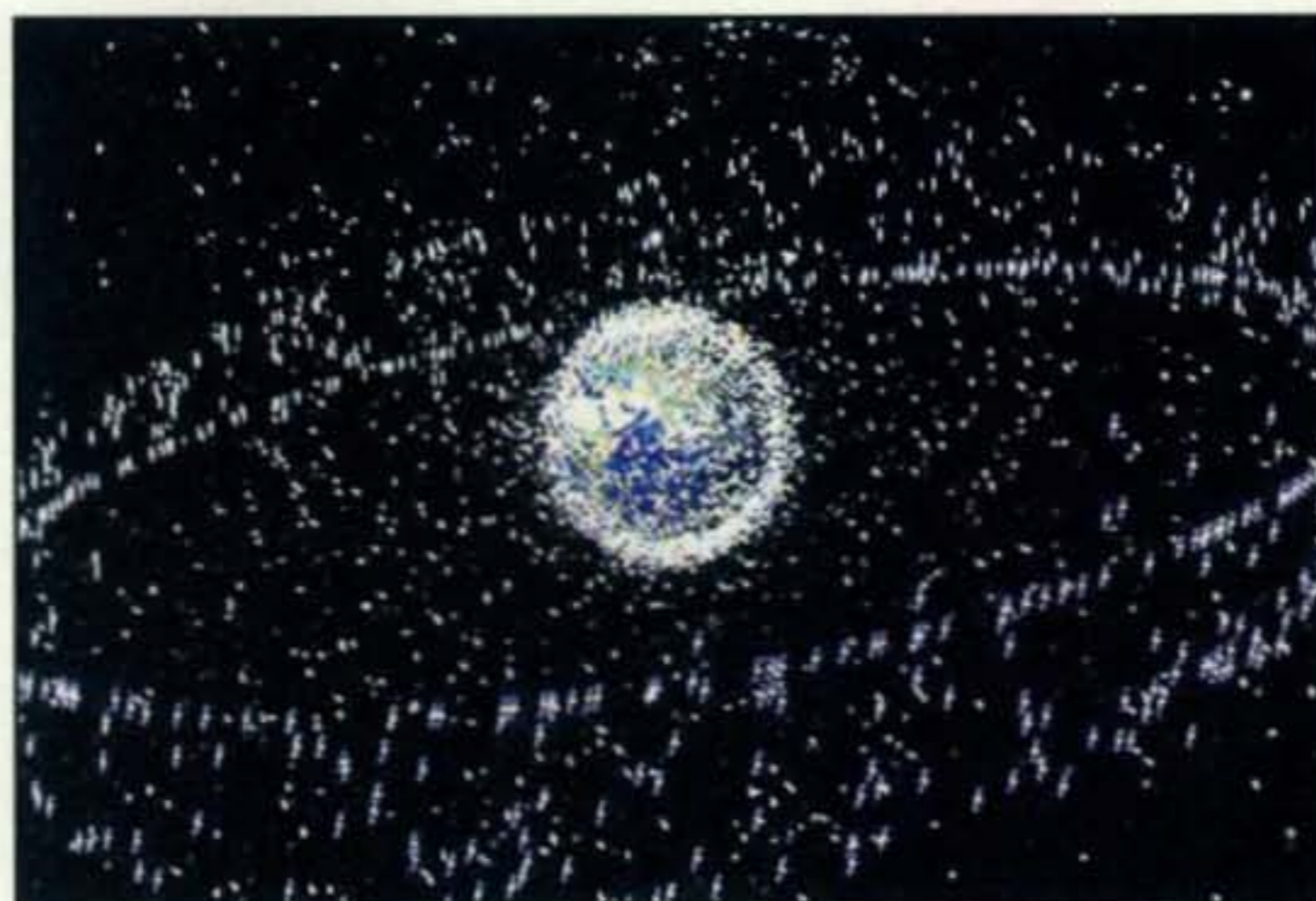
A NASA diagram of the thousands of manmade objects, 95 percent of which are junk, orbiting the Earth in both low and geosynchronous orbits. (Courtesy NASA)
