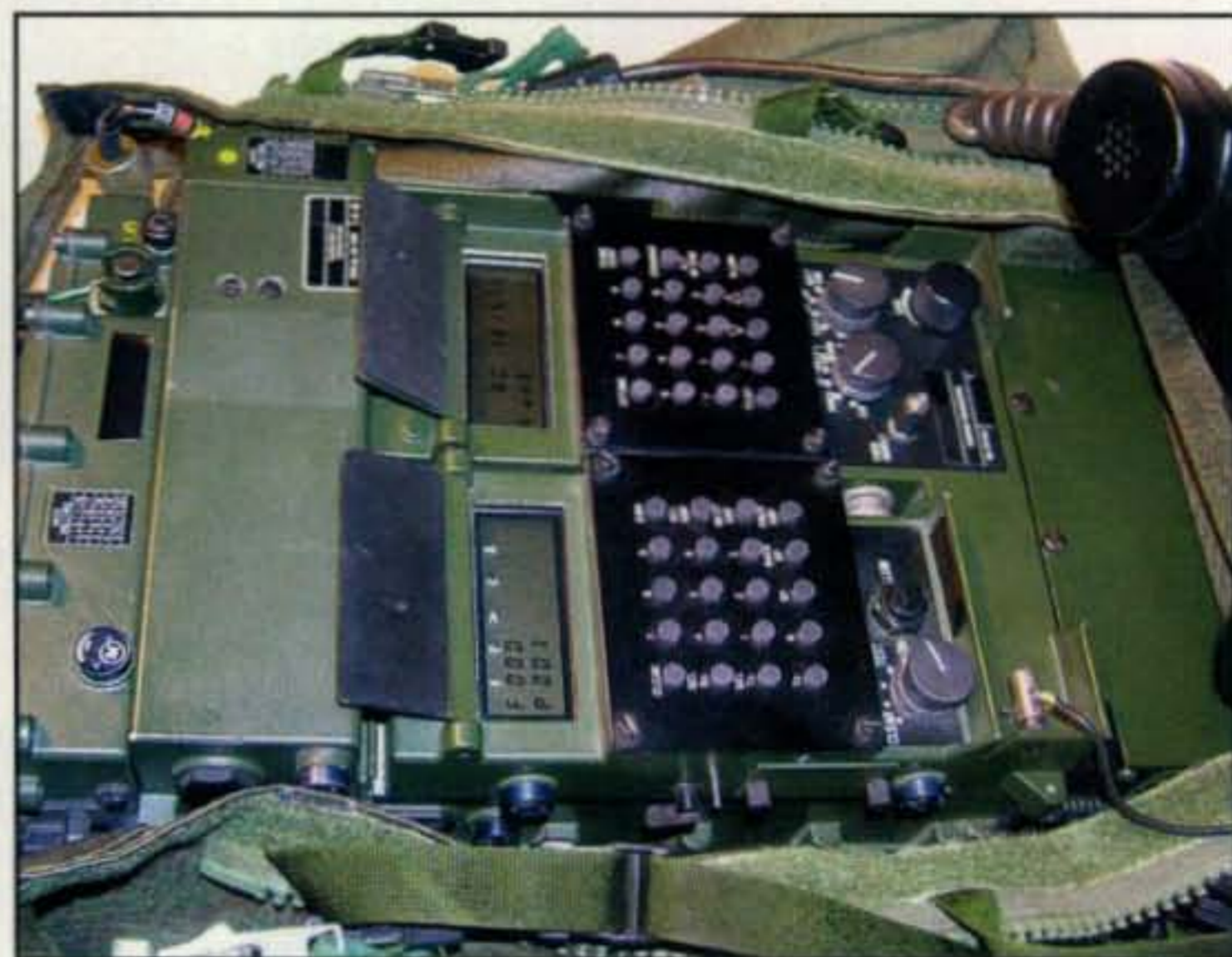
Photo 8— Close-up view of Paul's PRC-319 British military backpack transceiver. This is big-time portable, running 50 watts, covering 1.5 to 40 MHz, and weighing 23 pounds.
