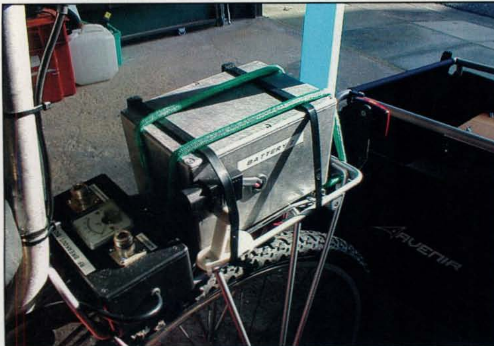
Photo 3— G4AKC shows us the protective case used for holding four gel-cell batteries on the back of the bike. It is flanked by an antenna mount (left side of photo) and removable bike trailer (right side of photo).
