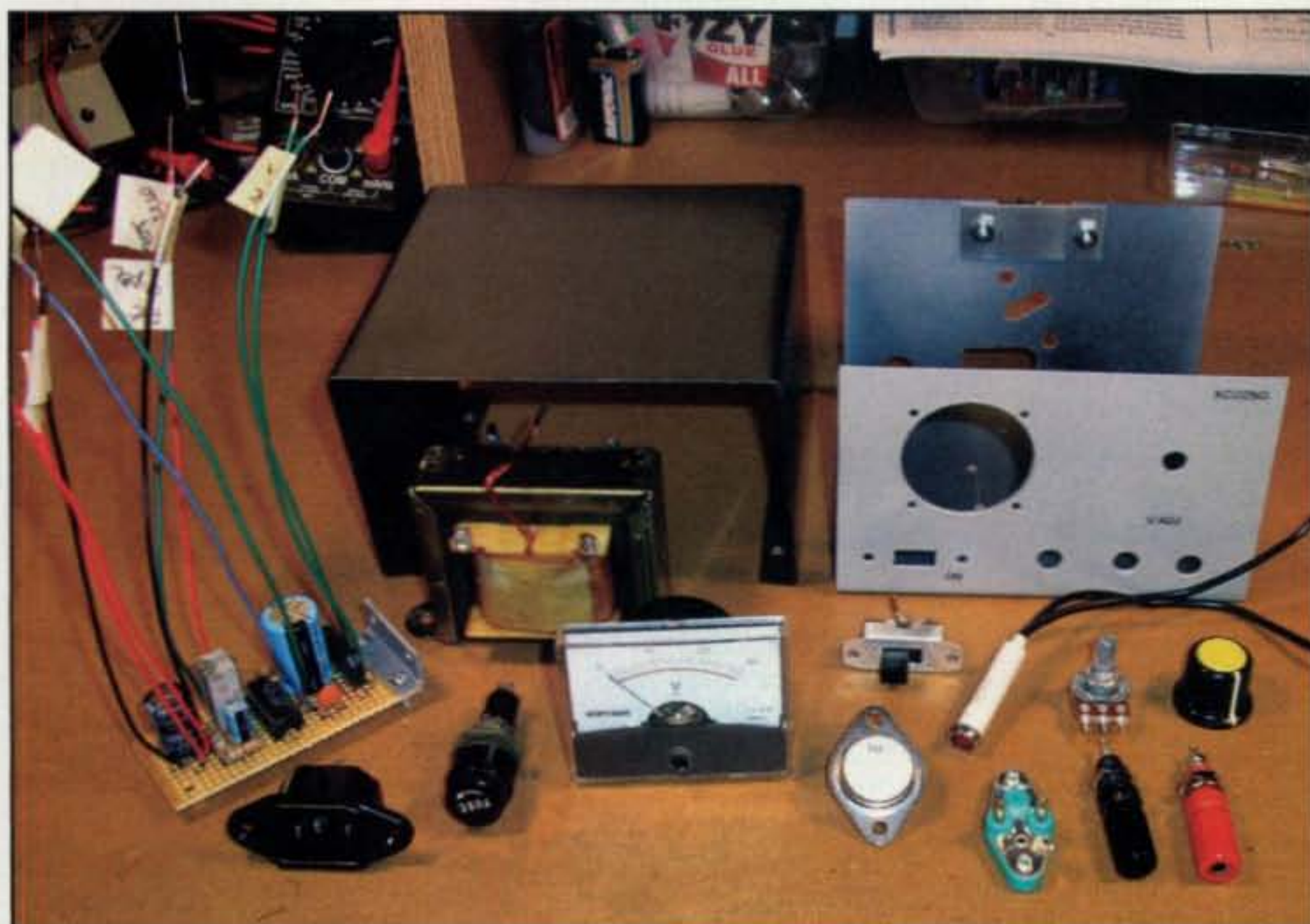
Photo C—The parts of the supply were laid out in preparation for final assembly. Note the parts salvaged from the original supply and the board on the left that holds the rectifier, filter capacitor, and regulator.
