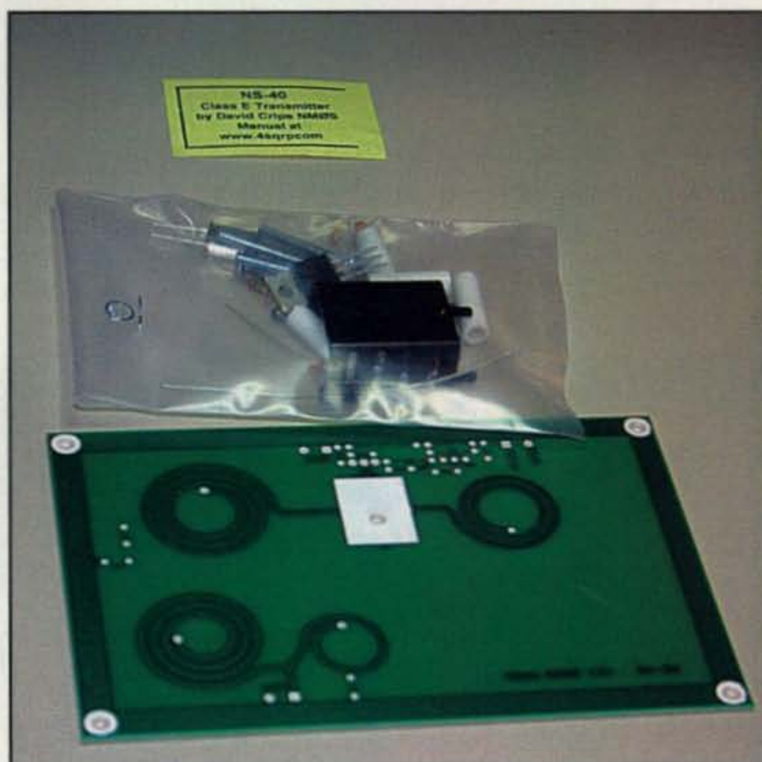
Photo 4— The NS-40 QRP transmitter kit as received and ready for assembly. Kit consists of only 14 components, but do not be distracted by its simplicity. A large amount of high-tech engineering and complex mathematical calculations in its design result in an overall input-versus-output efficiency of nearly 90 percent. (NS-40 photos and fig. 1 courtesy of Jay Bromley, W5JAY, and XYL Kathy, WQ5T)
