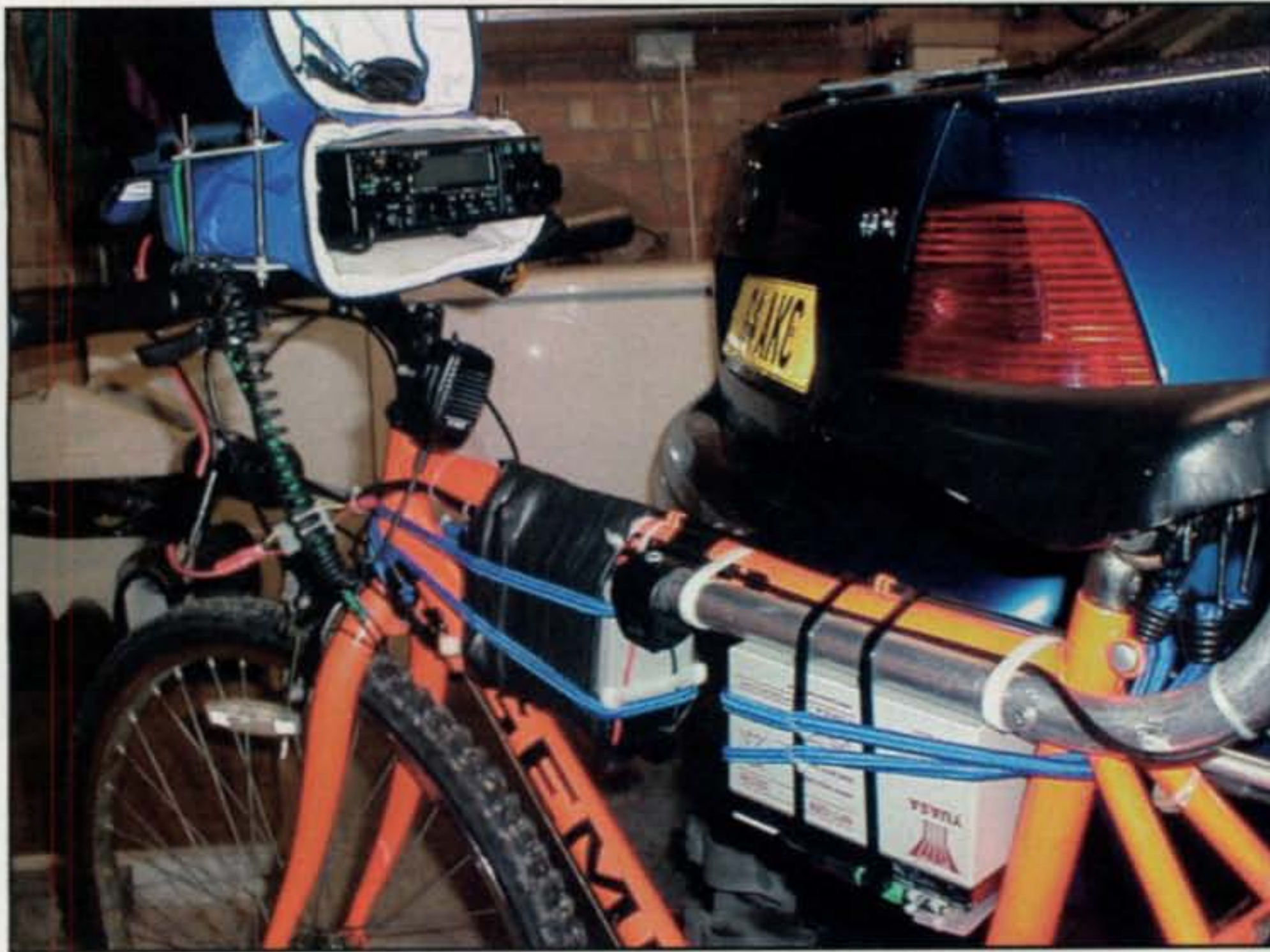
Photo 2— Garage-shot photo of G4AKC's Alinco DX-70 nestled in a handlebar bag with zip cover for protection from harsh weather and bumpy roads. Air circulation in the bag is limited, so David holds RF output to 50 watts maximum—which helps with heat, RF exposure safety, and long battery life.
