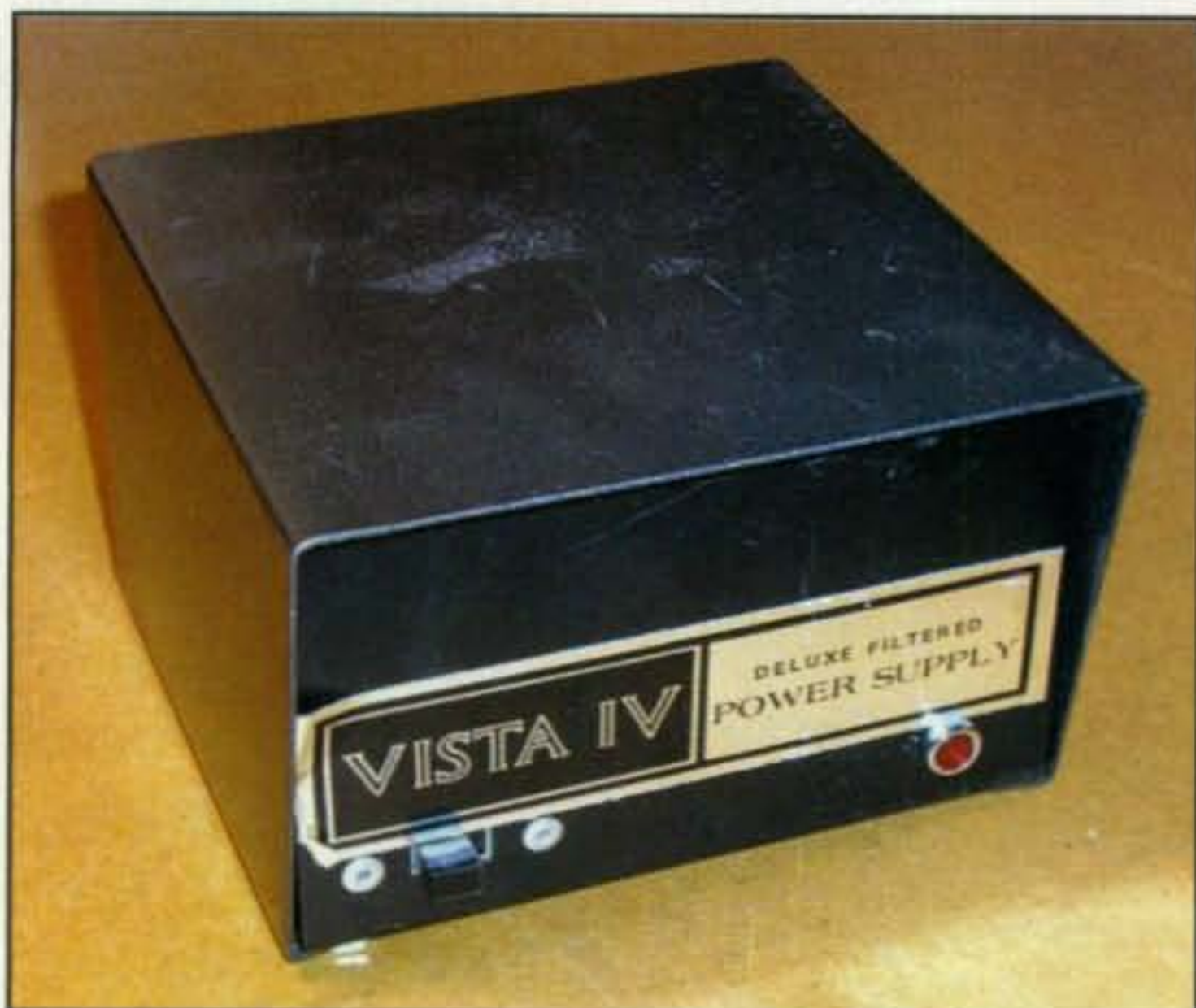
Photo A— The original power supply provided 12V at up to 1.5A but was a little the worse for wear.
