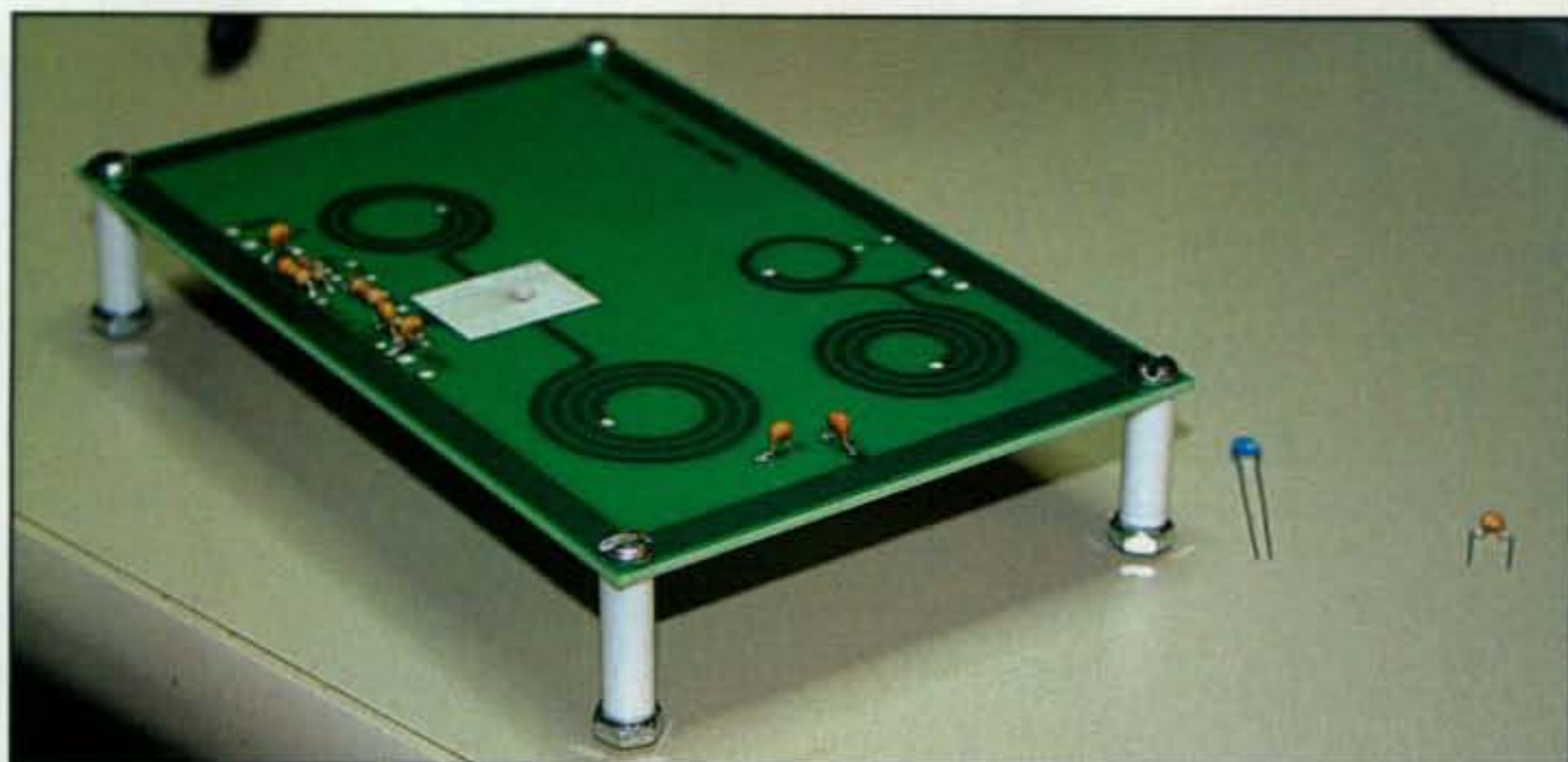
Photo 5— This midway of assembly, 10 or 15 minutes later photo of the NS-40 shows all seven capacitors and three resistors mounted with only transistors, crystal, and wires for external connections still to be installed. Notice there are no coils to wind. They are etched directly into the PC board and quite precise in inductance—an innovative and clever idea.
