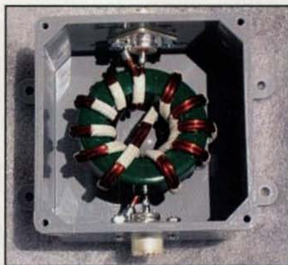
Photo C— Inside view of Balun Designs LLC Model #1113u 1:1 ratio current balun.
