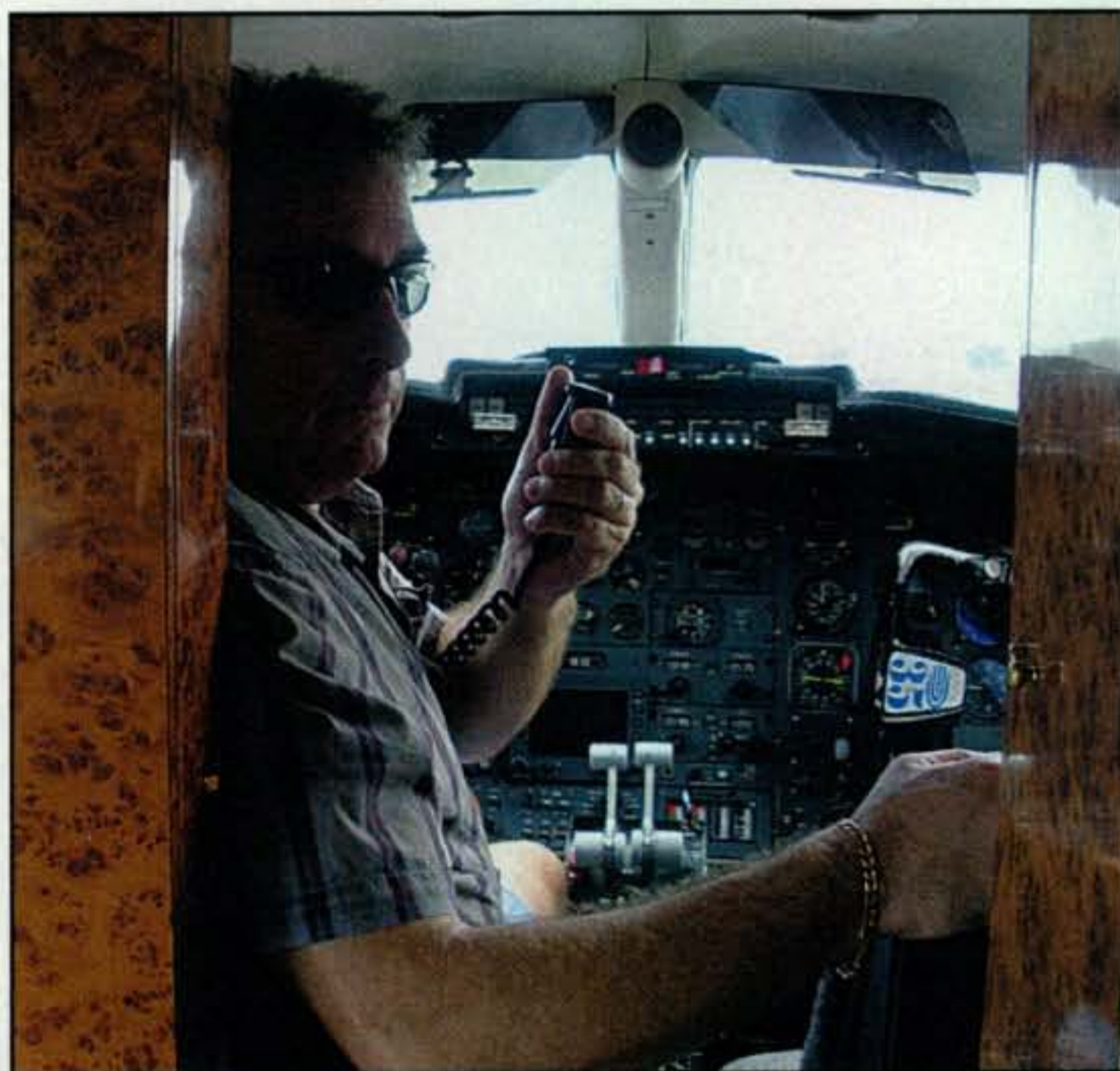
Photo 3—Joey in the cockpit and operating as N4ZUW/aeronautical mobile. The rig is commercial 100-watt transceiver with automatic antenna tuner, included in the airplane's gear. The antenna is random wire located between a wing and the tail. The high-in-the-sky location helps to radiate an outstanding signal heard near and far.
