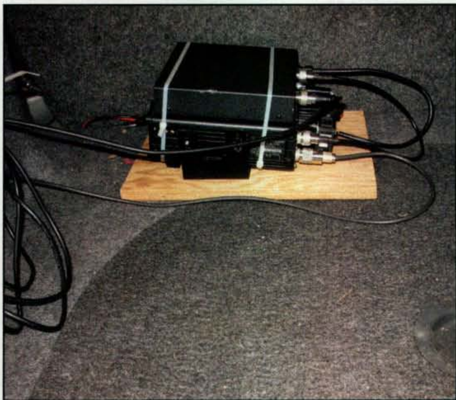
Photo 11— In-trunk view of W5APS's setup shows the main body of the IC-706 and LDG-7000 tuner strapped together. The wood base raises the gear off the carpet and helps air circulation so the rig hopefully does not overheat.
