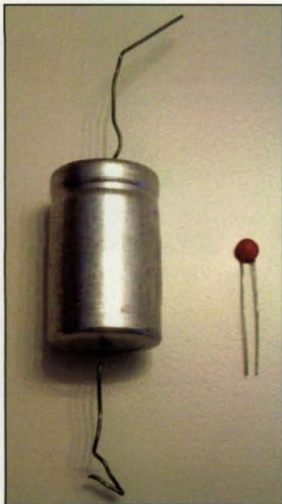
Photo A— Size comparison of a 10- \mu F capacitor (left) and .01- \mu F/10-nF capacitor (right). Think low frequencies (50 Hz to 50 kHz, typical) for large capacitors and high frequencies (500 kHz to 500 MHz) for small capacitors as a keep-it-simple guideline and you are right on track.
