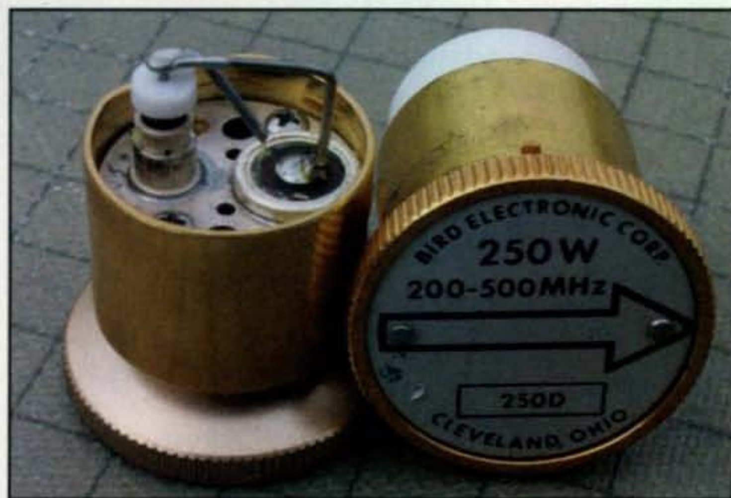
Photo E— A Bird® slug uses the same detector diode for both forward and reverse readings.
