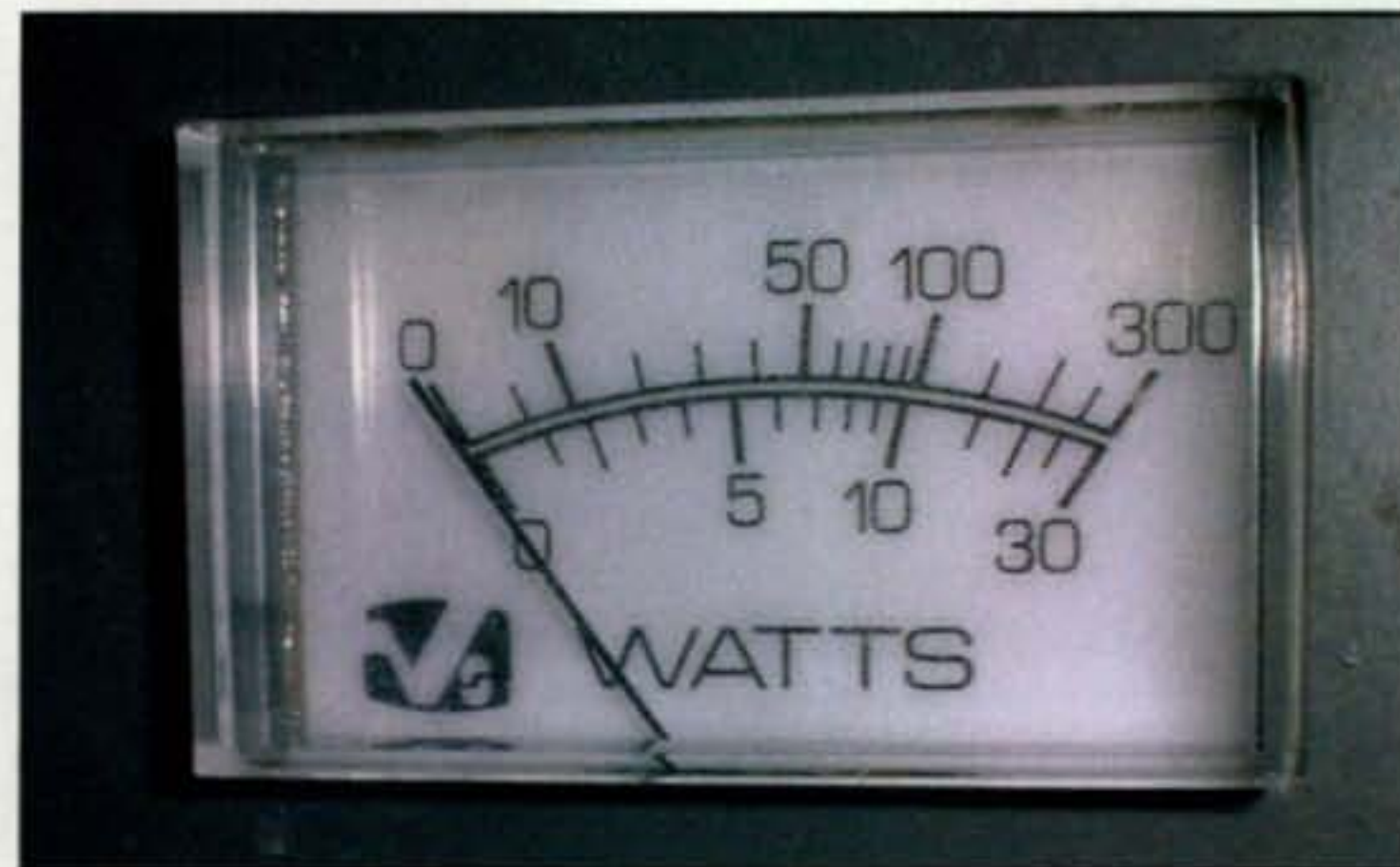
Photo D— Typical SWR-meter scale. Note that it is not linear.
