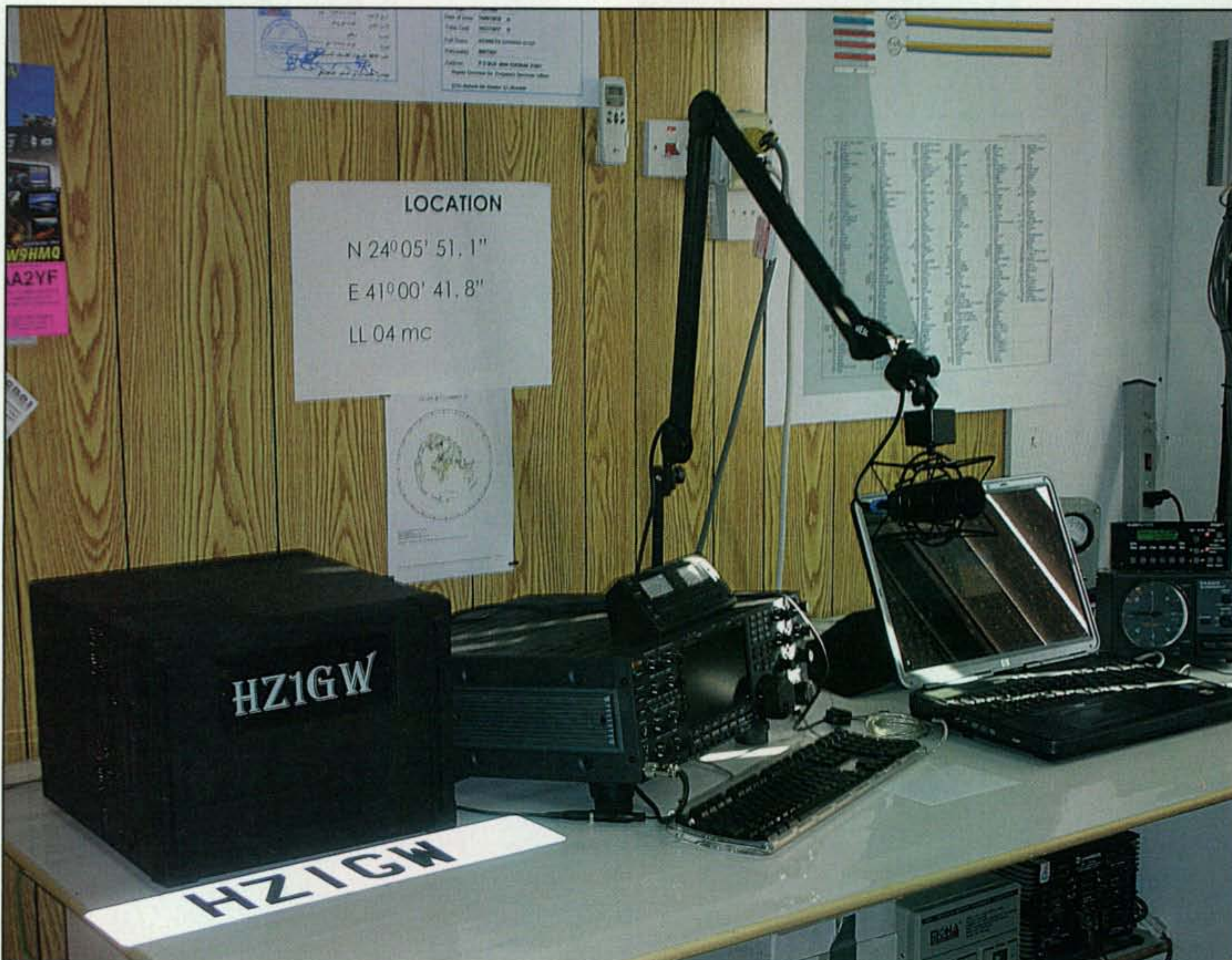
The HZ1GW shack near Medina, Saudi Arabia, consists of an ICOM 7800 transceiver, ICOM PW1 amplifier, and Heil PR-781 microphone.
