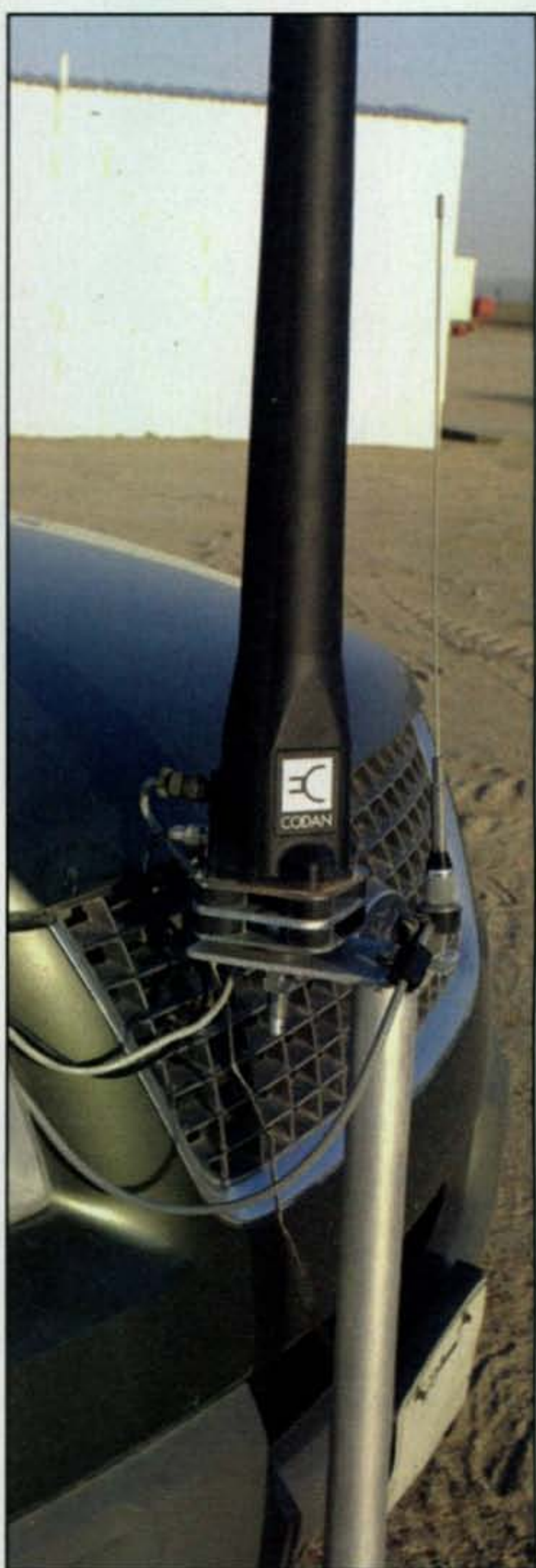
A close-up view of Ken's front-mounted mobile antennas. The multiband HF antenna is a Codan 9350.
