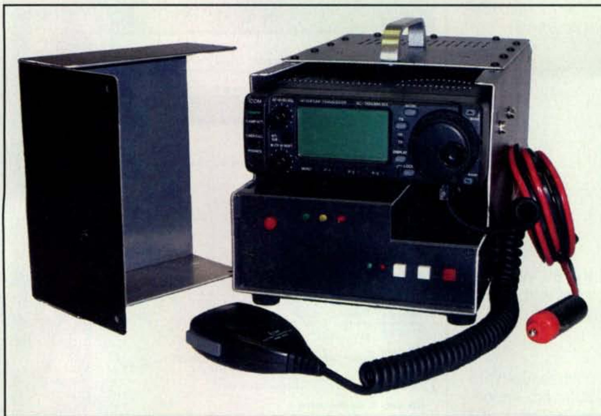
Photo B— The MFJ-706 is a Grab-and-Go Emergency Communications Center that requires you only provide an ICOM 706 and antenna. (Photo courtesy MFJ Enterprises)
