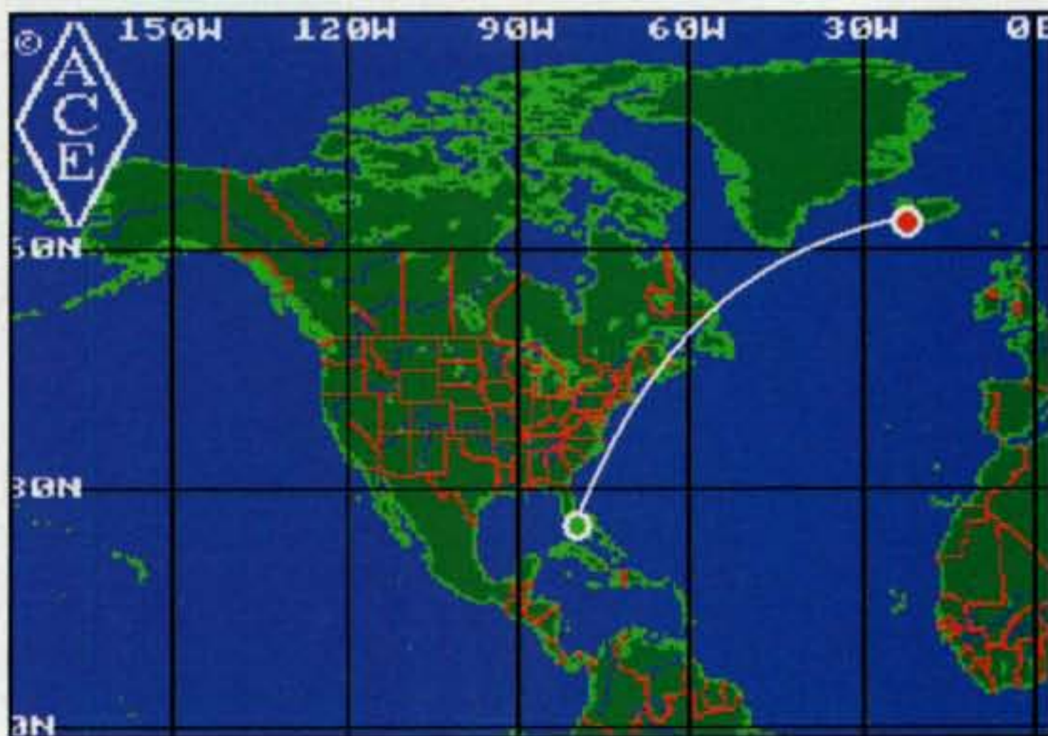
Fig. 1—The selected radio circuit between Iceland and Florida. (For figs. 1–7, source: NW7US using ACE-HF Pro, v2.05)
