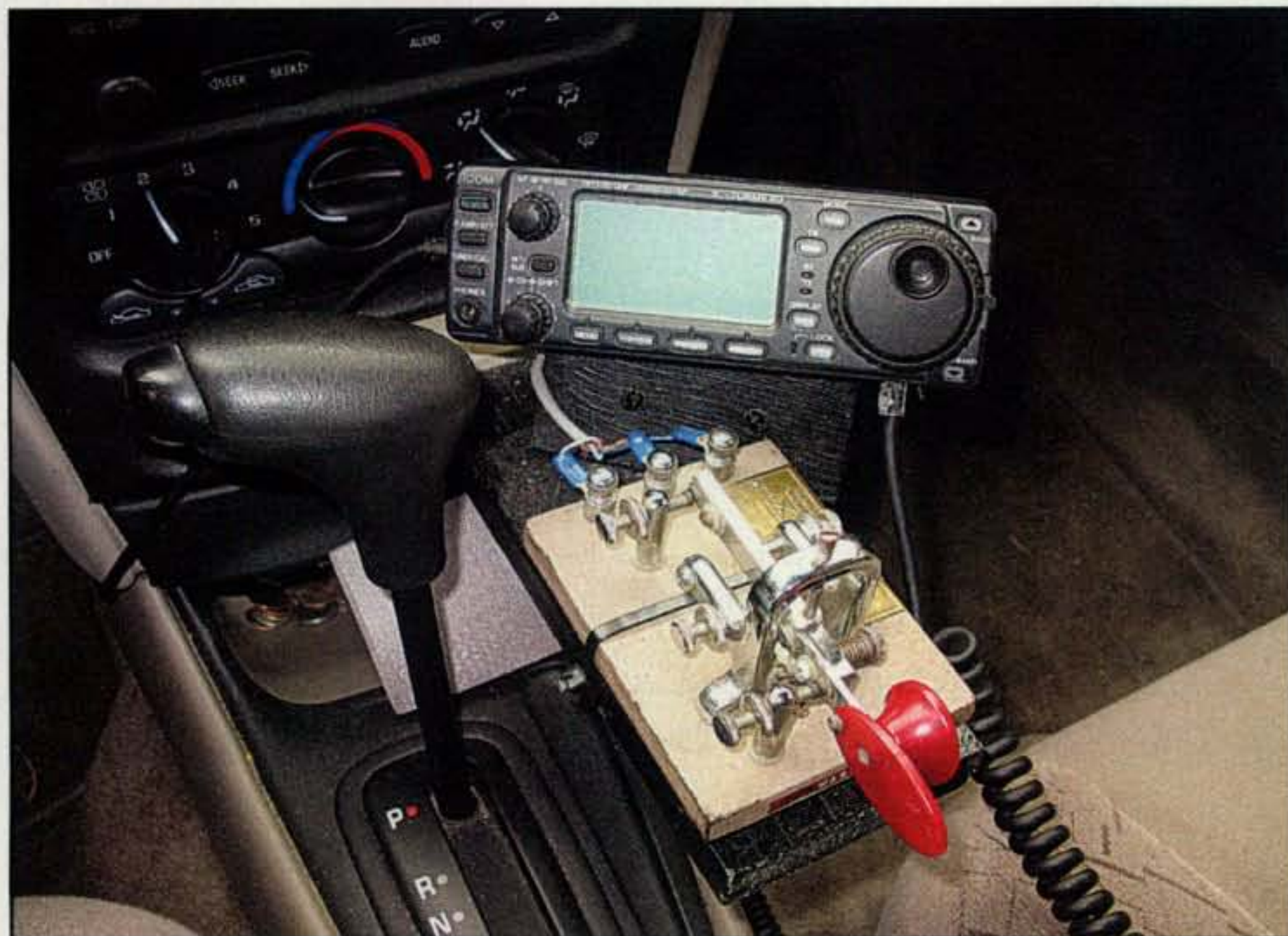
Photo 9— Installing mobile gear in modern automobiles with crowded interiors can prove quite challenging. Jim Hurley, W5APS, sidestepped the dilemma by first visualizing the best spot for his ICOM IC-706's control head and Vibroplex paddle and then making a "push-in" wood mount to hold them in that place. (Photos 9, 10, & 11 courtesy of W5APS)
