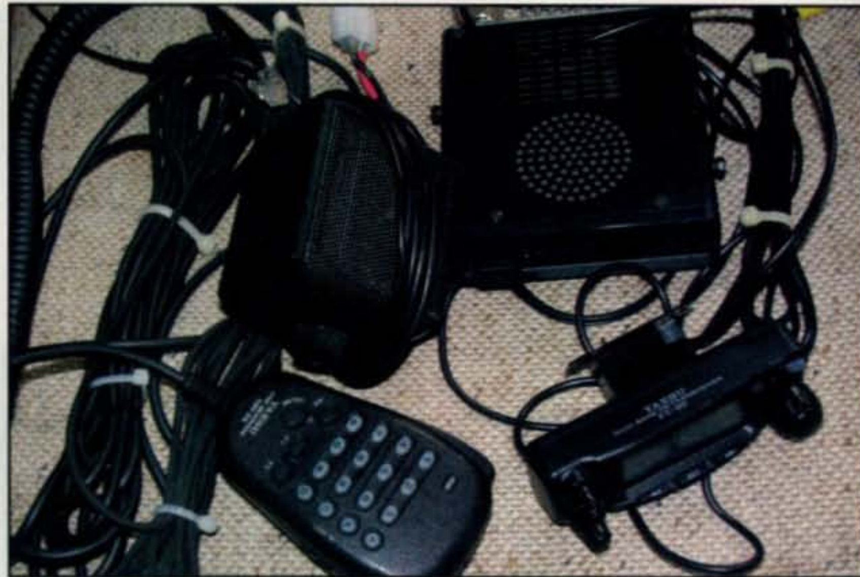
Photo 3— Here is an example of a good, used FM rig. This is a compact 2M/70cm radio in working condition. The original power cord and mounting bracket are missing but can easily be replaced. This rig has all the features of anything brand new, but it comes at a bargain price and it works.
