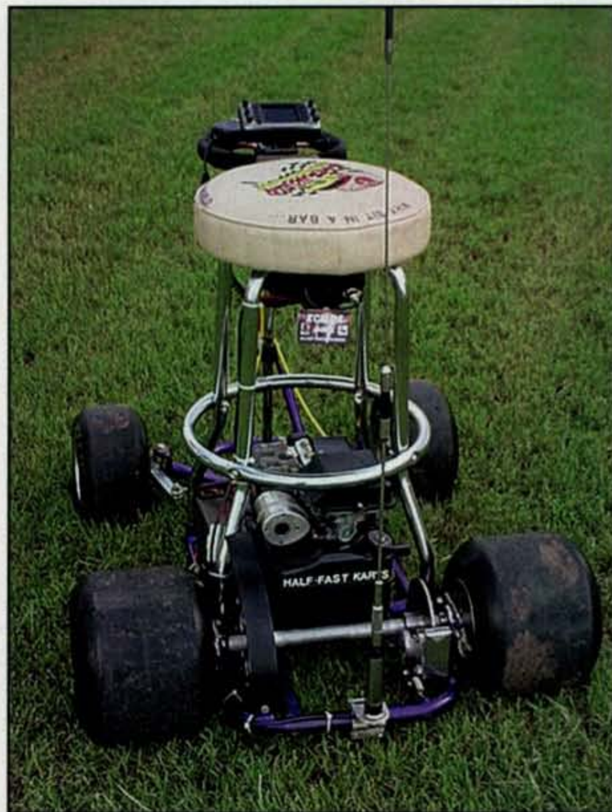
Photo 1—Look . . . in the parking lot . . . out in the grass. It's a . . . yes, friends, it's a motorized barstool mobile and proud owner Jim Smith, KC5LQA, has won several awards riding it in parades. Specifically, it is a 2003 model Barfly with 3.5-HP engine, padded steering wheel, ICOM 2800 transceiver, Comet dual-band antenna, and gel-cell battery. Ride on, Jim! Ride on! (Photo courtesy of KC5LQA)
