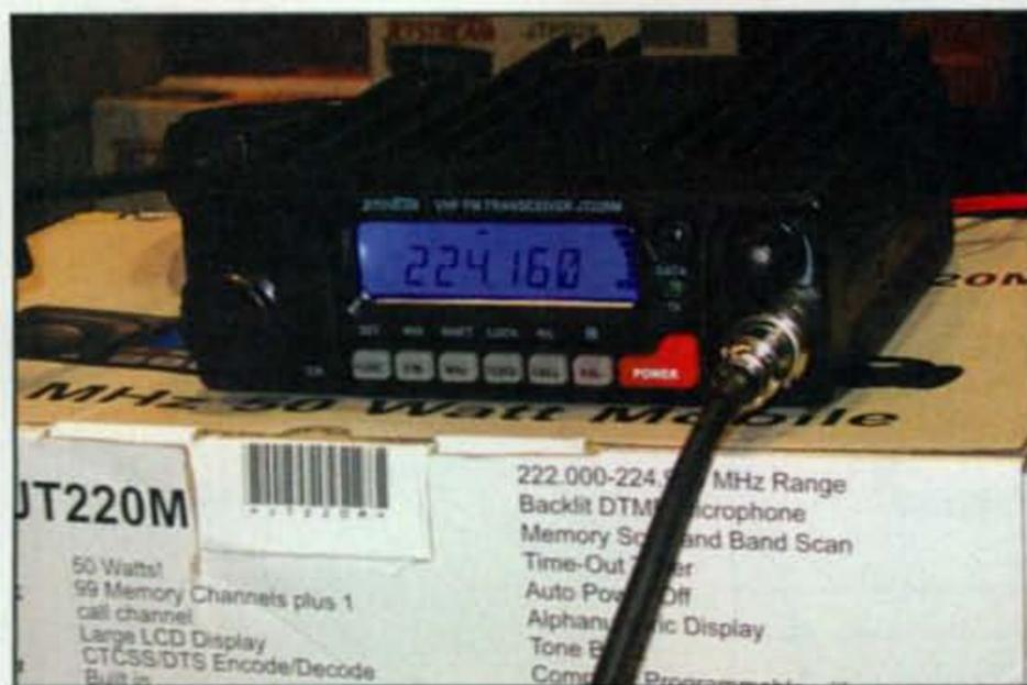
Photo G— JetStream's JT220M 50-watt 222-MHz mobile.
