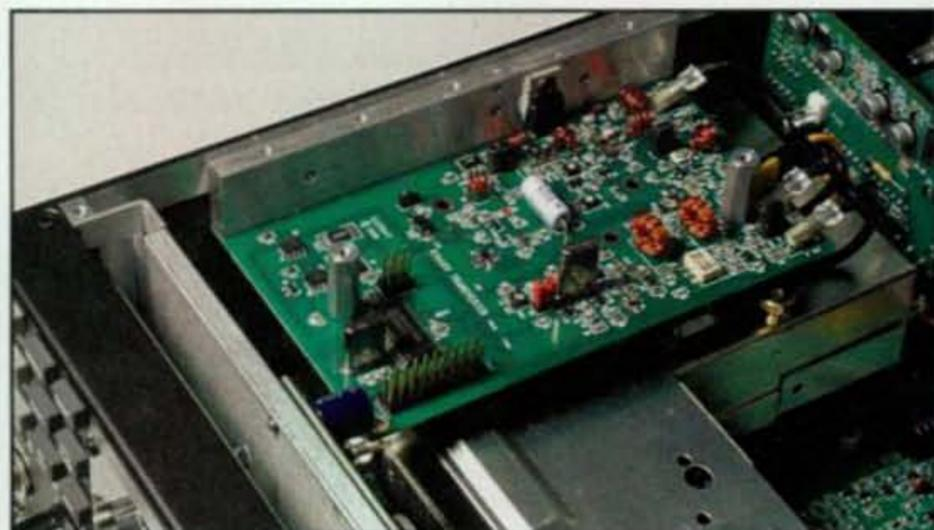
Photo H— Elecraft's K144XV internal 2-meter module mounted inside the K3 transceiver.
