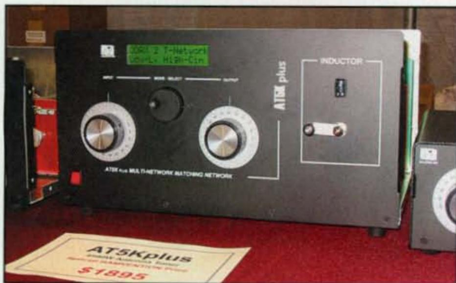
Photo M—The Palstar AT5Kplus is a 4500-watt antenna tuner.
