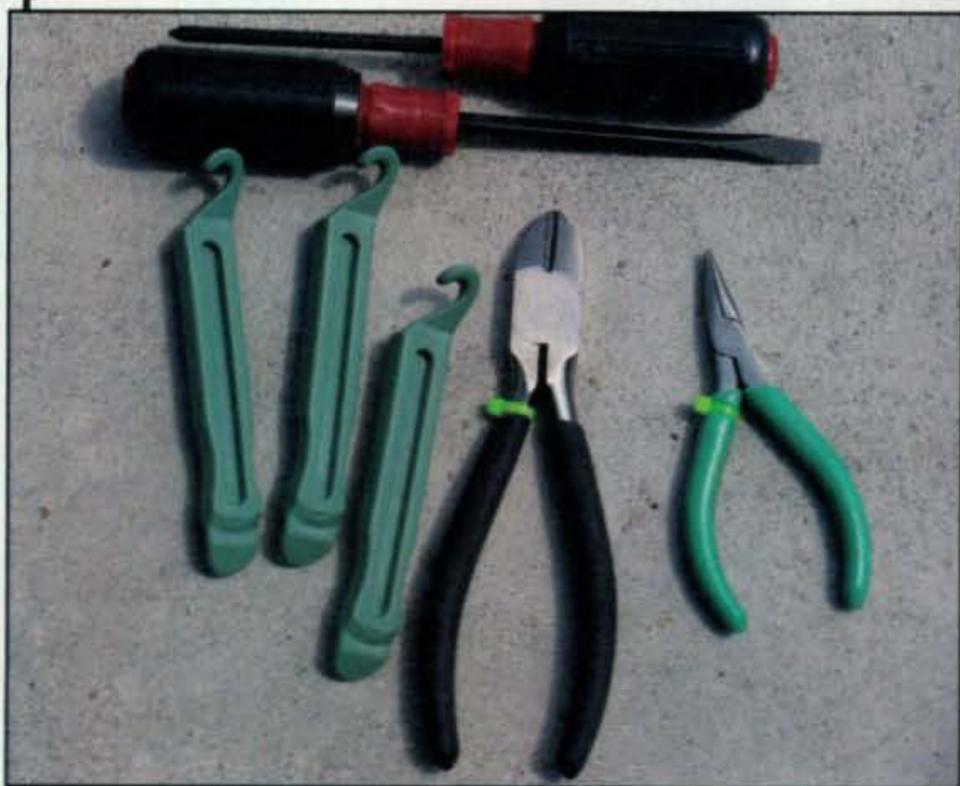
Photo 1— Tools for uninstalling a radio system are the same as those for installing a radio system. The strange-looking green objects on the left side of this photo are plastic bicycle-tire levers. Read the text to learn how to use them on your car or truck. (Photos by the author)
