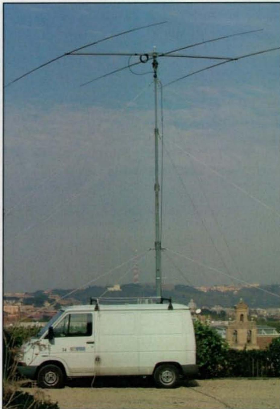
The 20-meter Yagi (shown here) and the 15-meter beam both had good views from the top of Aventino Hill for working long path to Japan.
