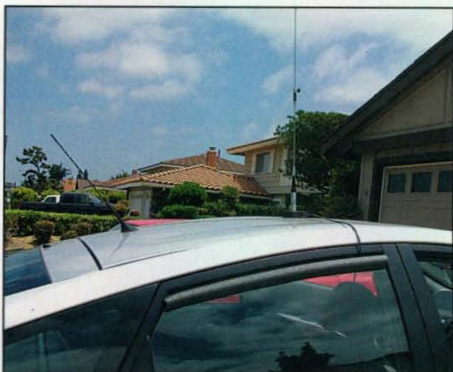
Photo 8— It might be a good idea to have a magnet-mount antenna on hand so you can get back on the air quickly.
