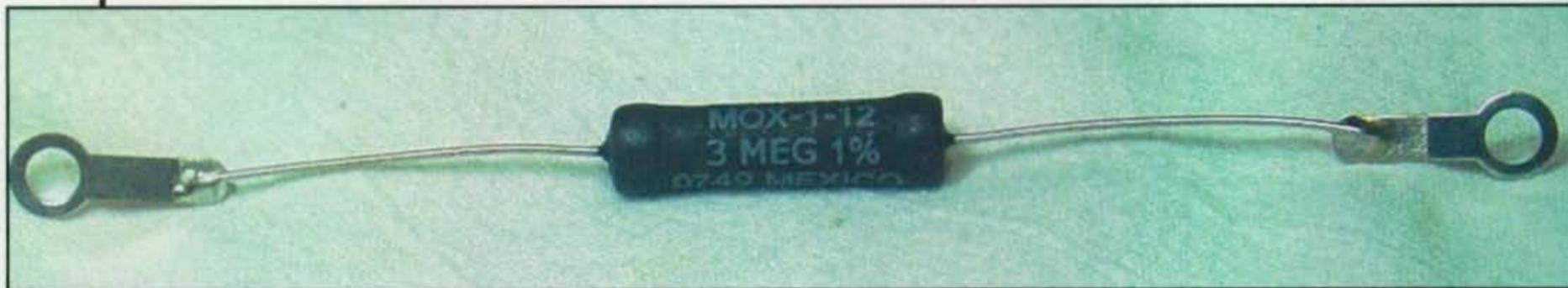
Photo A— The 3-megohm resistor ready for mounting on the triband dipole.
