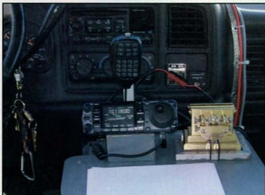
*Photo E— Phone or CW, KØHL can work the world. Note the well-constructed arm rest, and even with a lot of gear aboard, all the equipment is clear of the airbag deployment zones.*
