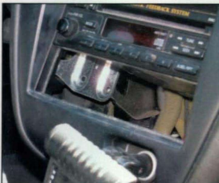
Photo 2— The mobile radio was un-installed from the dashboard where a plastic pocket used to be. The radio came out easily because it was held in place with black paper mache and radio-control modeler's servo tape.
