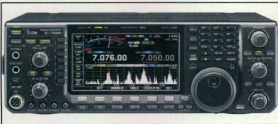
Photo J—ICOM's new IC-7600 high-performance HF/50-MHz all-mode transceiver.
