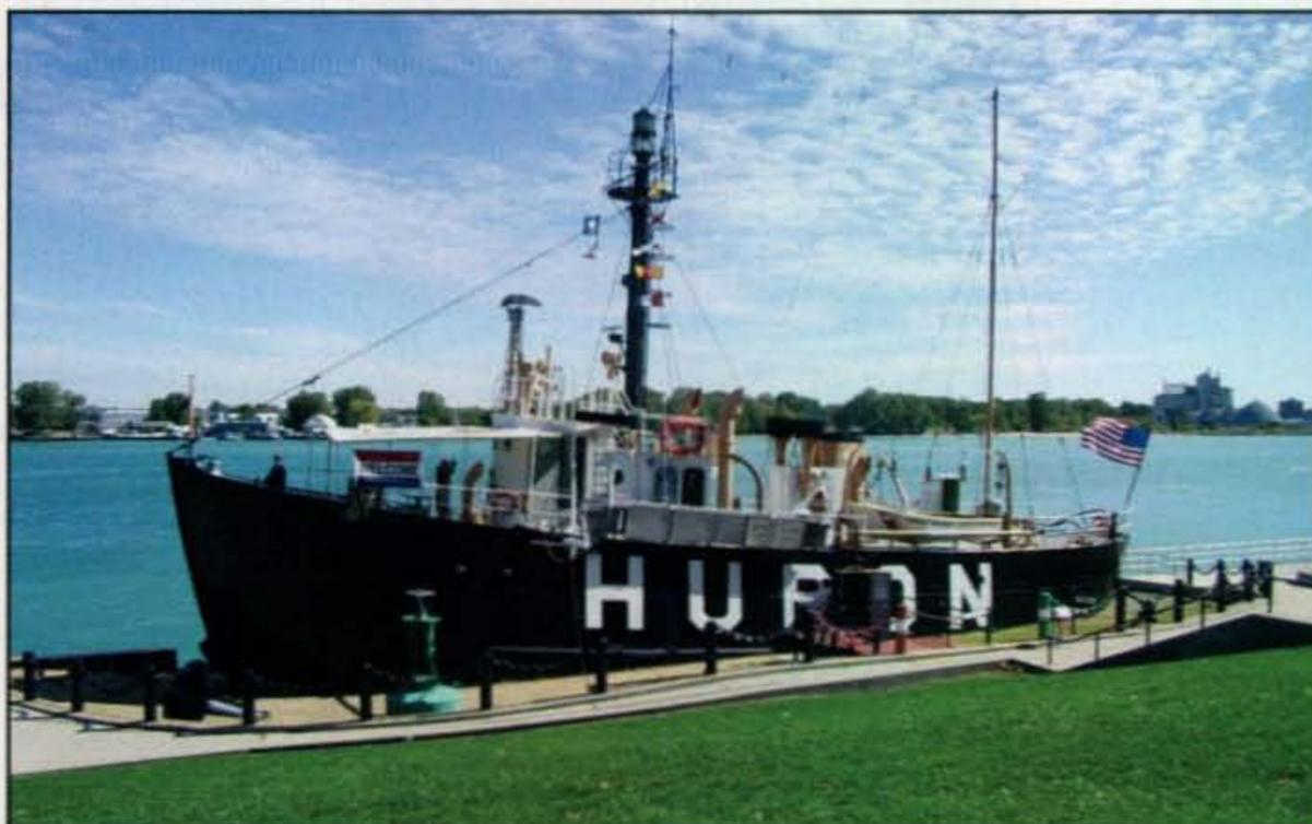
Photo 4— Lightships are akin to floating lighthouses, and prior to the evolution of GPS for navigation, they marked dangerous waters, entrances to harbors, and more. Shown here is the retired-from-service Lightship Huron which now resides at Port Huron, Michigan.
