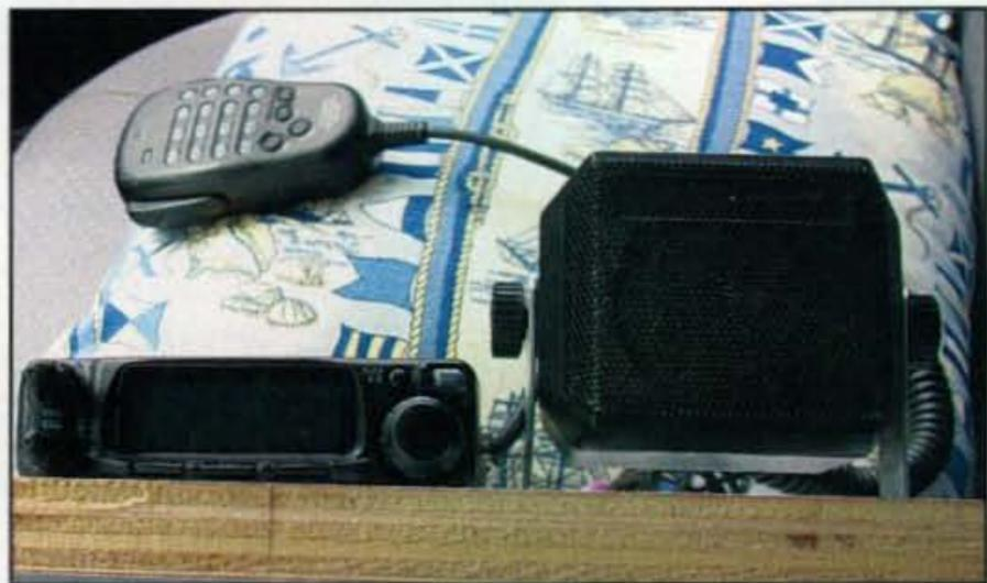
Photo 9— The old radio can be mounted on some sort of carrying platform for temporary use in the new vehicle. This “system” can also be used as a back-up station in any vehicle during an emergency.
