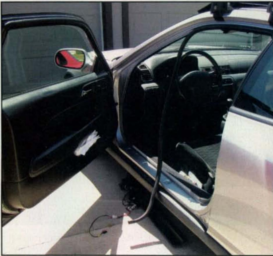
Photo 4— Plastic trim pieces were pried away from their fasteners using the tire levers and the wires were pulled out.
