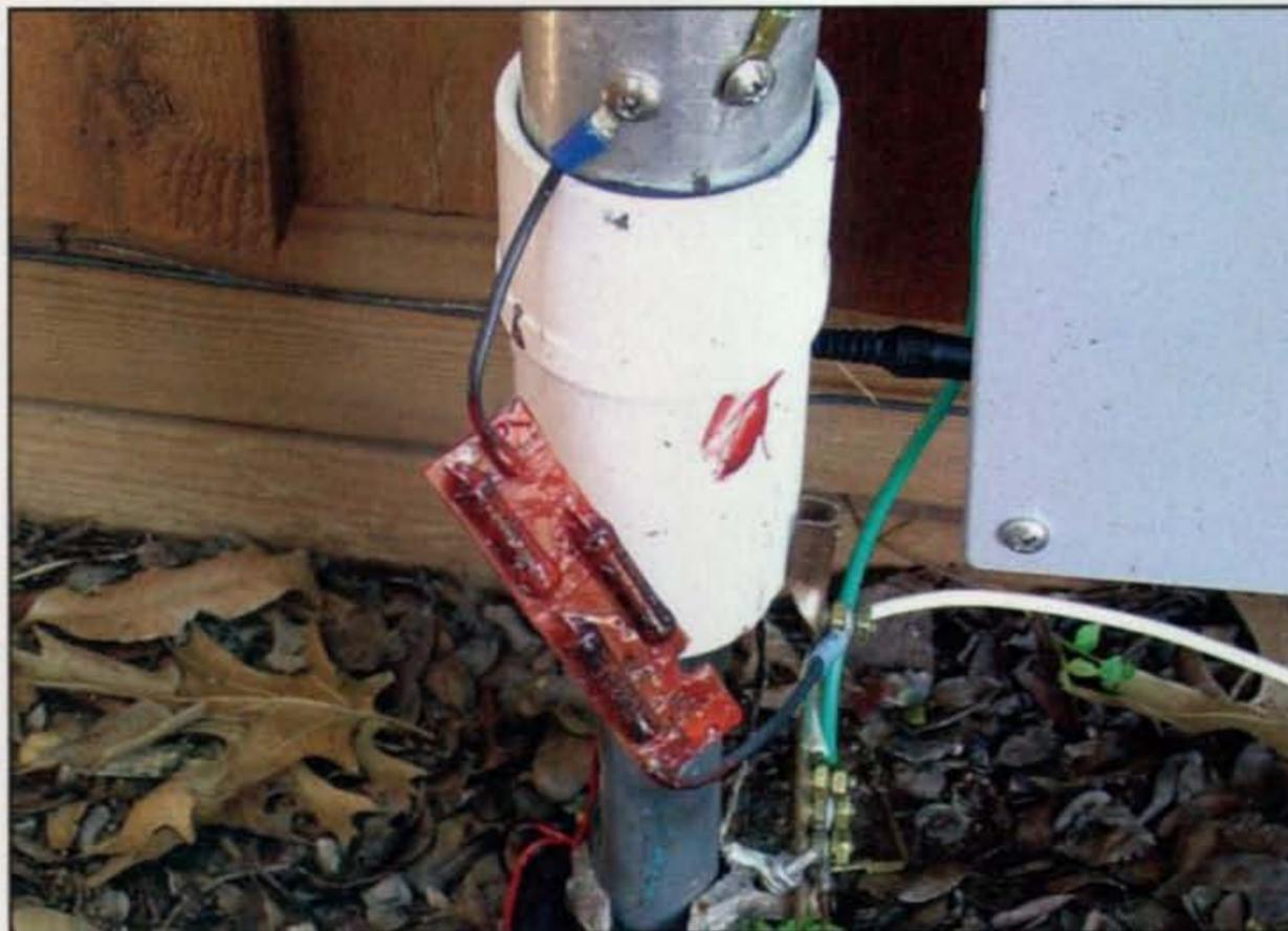
Photo B— Three 3-megohm resistors in series on per-board at the base of author's 43-foot vertical.
