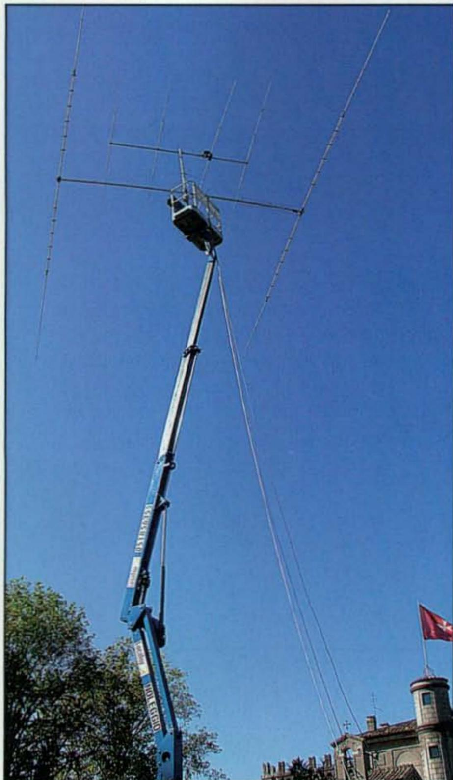
The 10- and 40-meter beams were installed on the platform of a rented cherry-picker and faced in opposite directions. See text for explanation.
