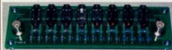
Kit includes PCB, assembly manual, 8 switches for the following PADS: 20, 20, 20, 10, 5, 3, 2, and 1 dB; 1% resistors, and BNC in & out connectors, all for \$49.95 per kit. Check details at [www.midnightscience.com](http://www.midnightscience.com) 405-517-7347
