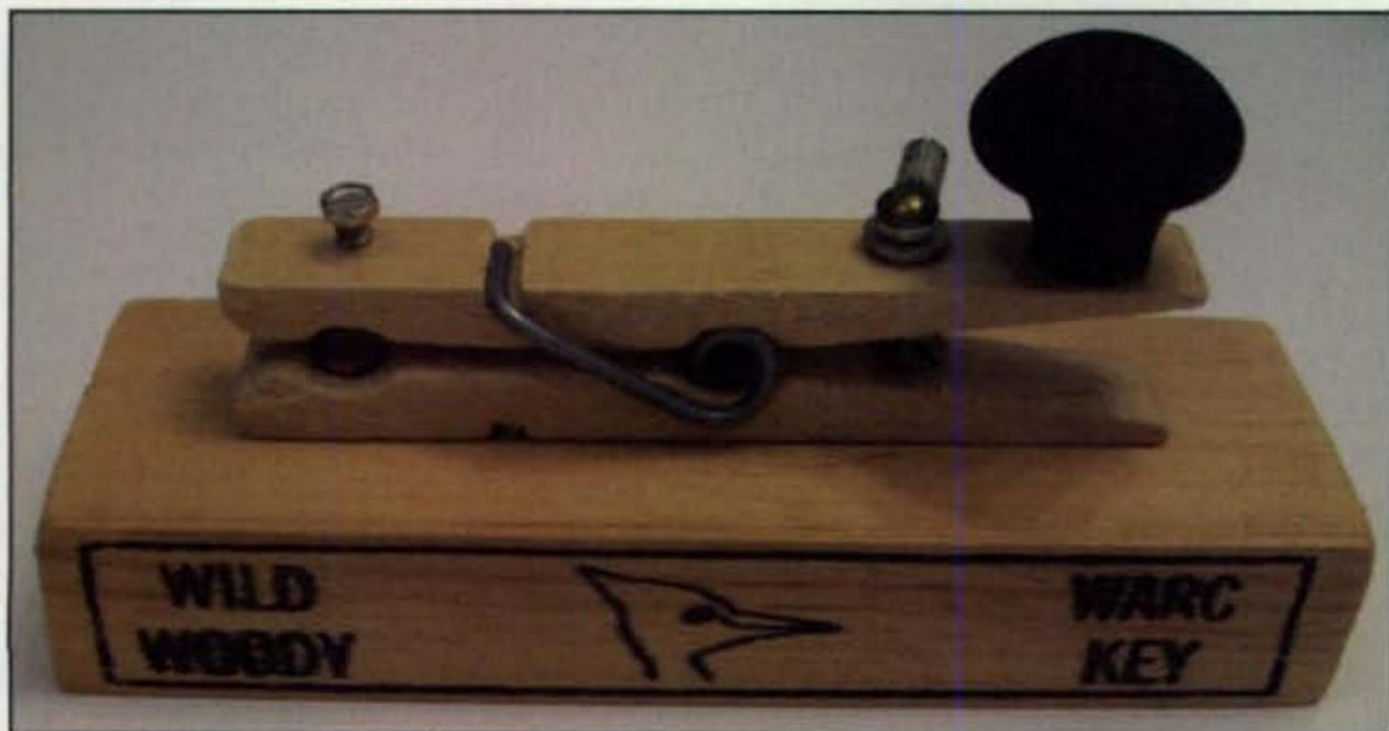
Photo C— This little looney is one of my own K4TWJ Wild Woody WARC Keys. It is made from a clothespin and works well for hanging poor CW operators out to dry. The key's spring is bent and stretched to reduce tension, and screw tips serve as contacts. It is the perfect pumper for heavy-fisted ops.
