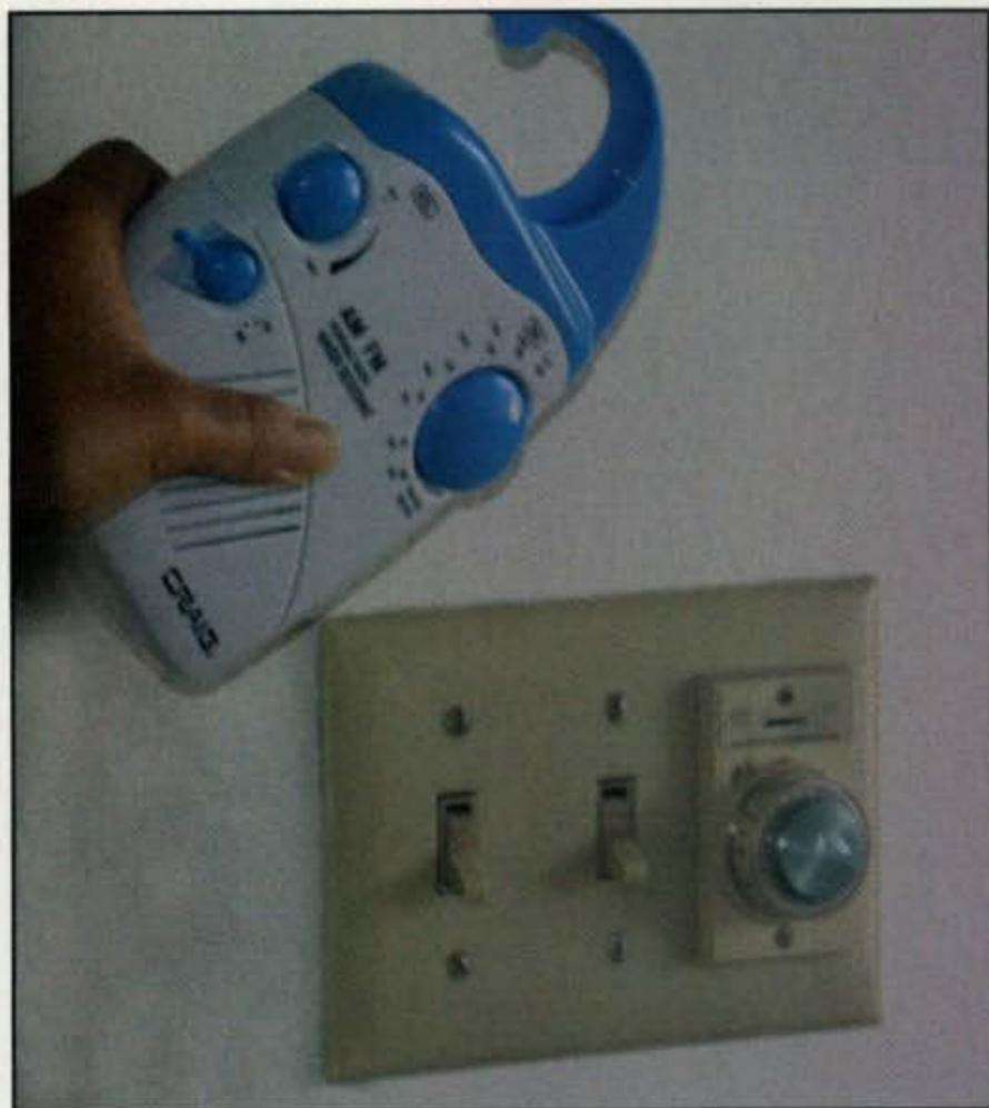
*Photo C— An ordinary AM receiver can be used to find EMI. Tune the radio to a blank spot on the dial and listen for the buzzing interference. Move the unit from left to right and go forward in the direction of the loudest noise.*
