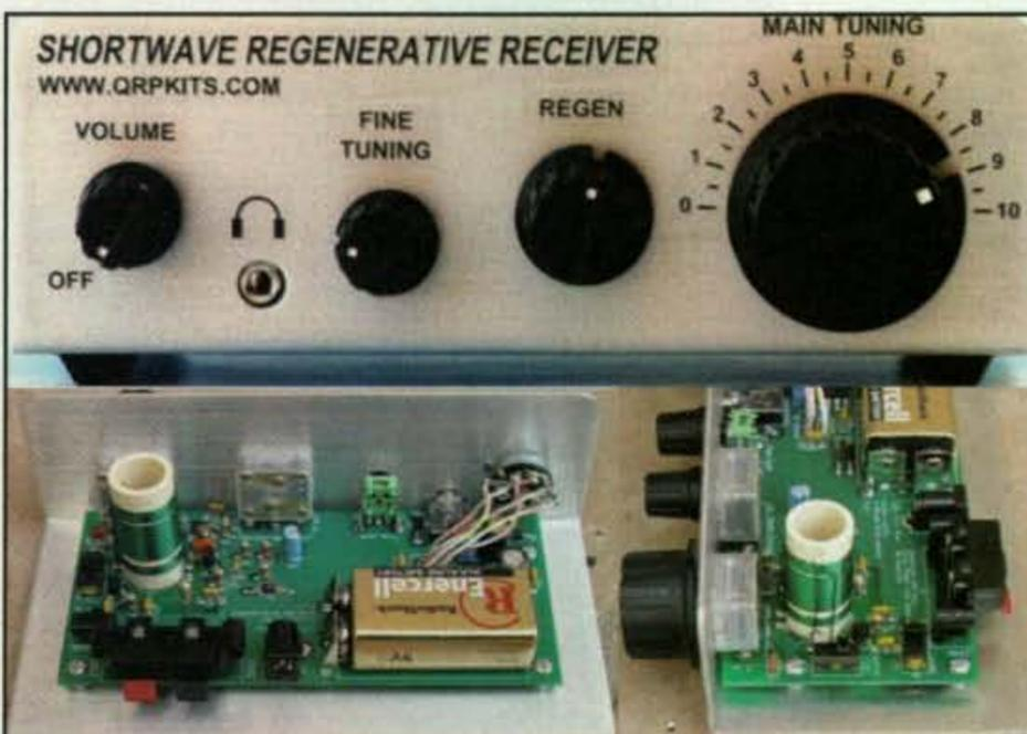
Photo Q— Hendricks QRP Kits' Scout Regen Receiver is a new, simple two-band regenerative-receiver kit.
