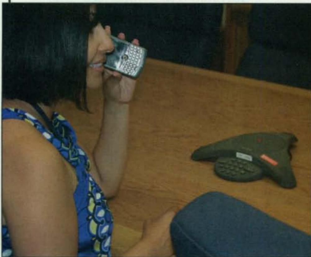
Photo A—A cell phone interfering with a conference-room speaker-telephone is an example of radiated interference.
