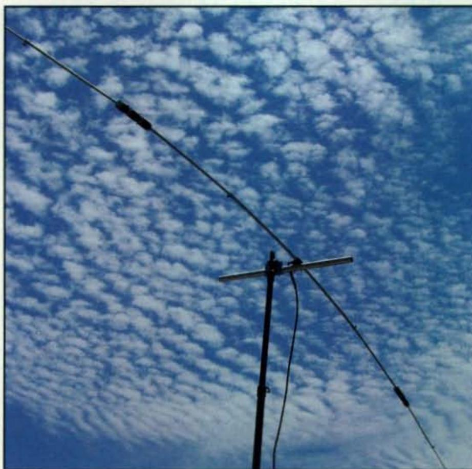
Photo D— The Super Antenna assembled as a 30-meter rotatable dipole.
