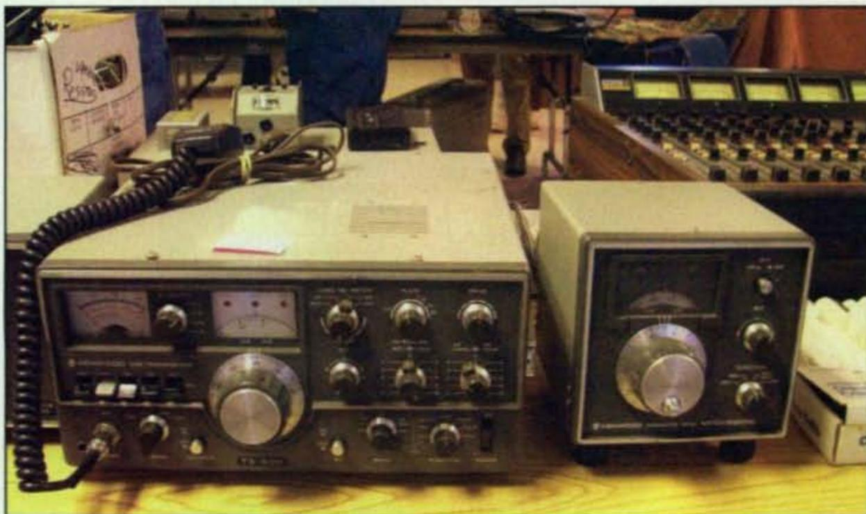
*Photo D— Another time-proven HF transceiver favored by many amateurs is Kenwood's TS-520. Add new driver and power amplifier tubes, maybe new filter capacitors, a tweak or two, some cabinet cleaning, and you have a romping good transceiver at a fair-and-square price.*
