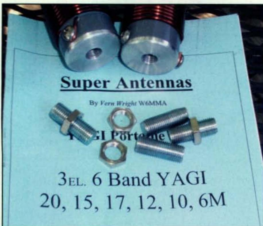
Photo C— All-Thread and nuts from old toggle switches are used to add 30 meters to the antenna's capabilities.
