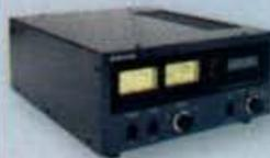
The HL-2.5KFX is the lightest and most compact self-contained 1.5kW output HF LINEAR amplifier in its class. The amplifier's decoder changes bands automatically with most modern HF transceivers.
