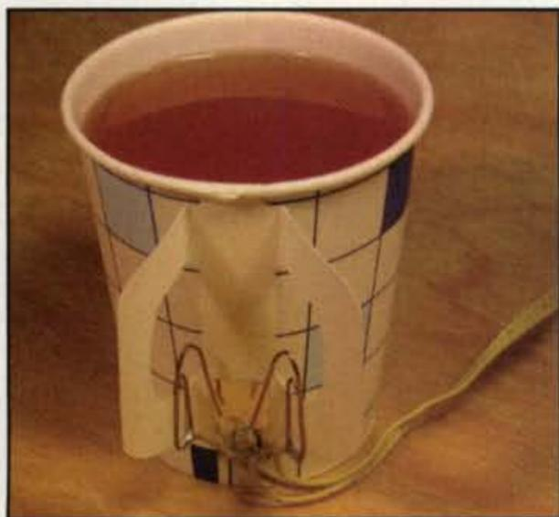
Photo J— OH6DC presents the every CW devotee's dream—a dual-lever paddle disguised as a paper coffee cup. Each handle is fitted with a precision-bent gem clip that, with handle moves, contacts a big blob of solder between the handles. We know you can't wait to make your very own copy of this treat, so details are in the text.
