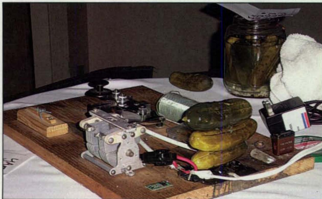
Photo D— Here you see the hot Pickle Keyer of Gordon West, WB6NOA, as photographed by Editor Rich Moseson, W2VU, at the 2005 Dayton Hamvention®. Big juicy pickles are placed between stainless-steel skewers and 120 volts AC is applied to the pickles through the key. What happens next? Well, one of my Wild Woody Keys with its arm blown off on the left side (obviously from a past demo) is a good clue.
