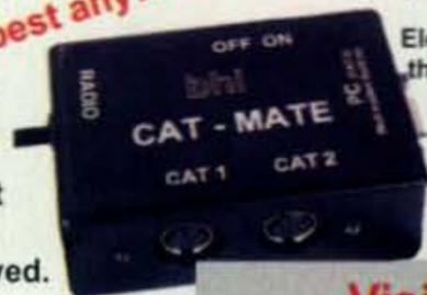
Electronic "Y" splitter that enables more than one accessory to be used via the CAT port on the Yaesu radio.
