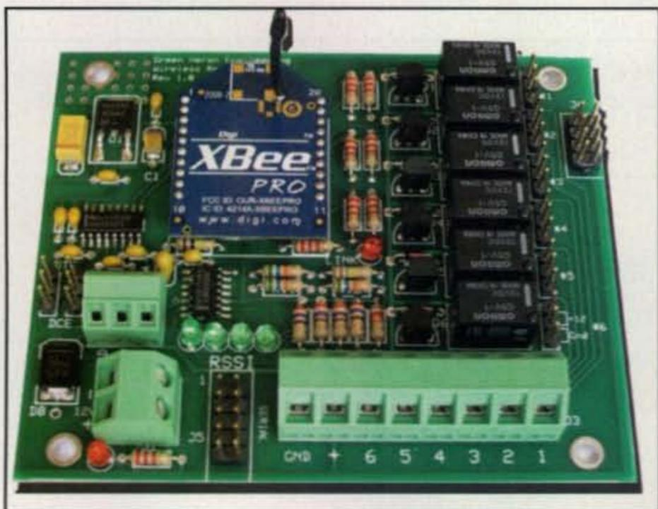
Photo G— Green Heron Engineering is introducing a wireless station switch controller to let you operate tower-mounted switches and relays without running an extra cable. This board is the heart of the system. It's mounted in a weatherproof enclosure.
