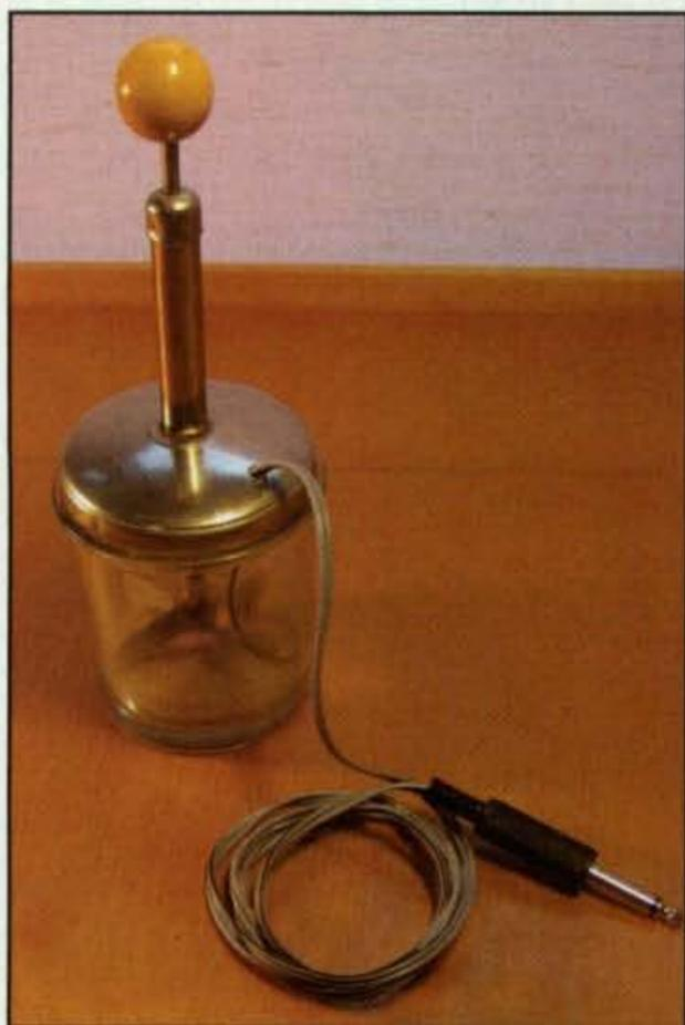
Photo H— The Onion Chopper Key was devised by Jari Vainio, OH6DC, and it is equally at home in the shack or in the kitchen. Key wires connect to the plunger rod and a piece of copper-clad PC board inside the chopping bowl. Note the colorful keying knob atop the chopper. Every ham needs a key like this! (photos H, I, and J courtesy of OH6DC)
