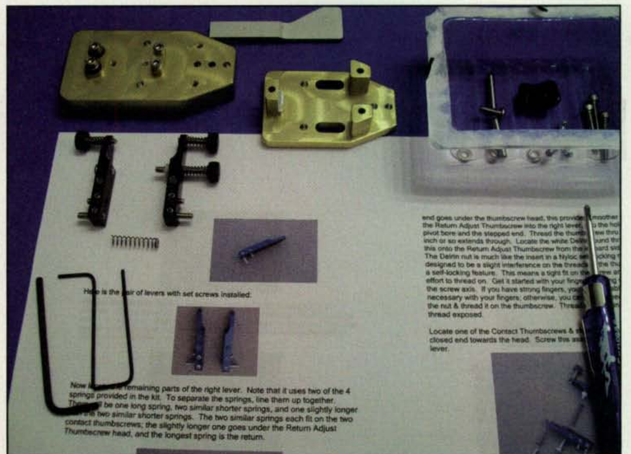
Photo D— Twenty or thirty minutes later the Bushwhacker is slightly over half assembled. The mechanism (all those loose parts you see) will be protected by the gold anodized aluminum frame. The fingerpiece is approximately .75 inch by .75 inch, with center area 1.5 inch above the desk when mounted on the optional .5-inch thick base.
