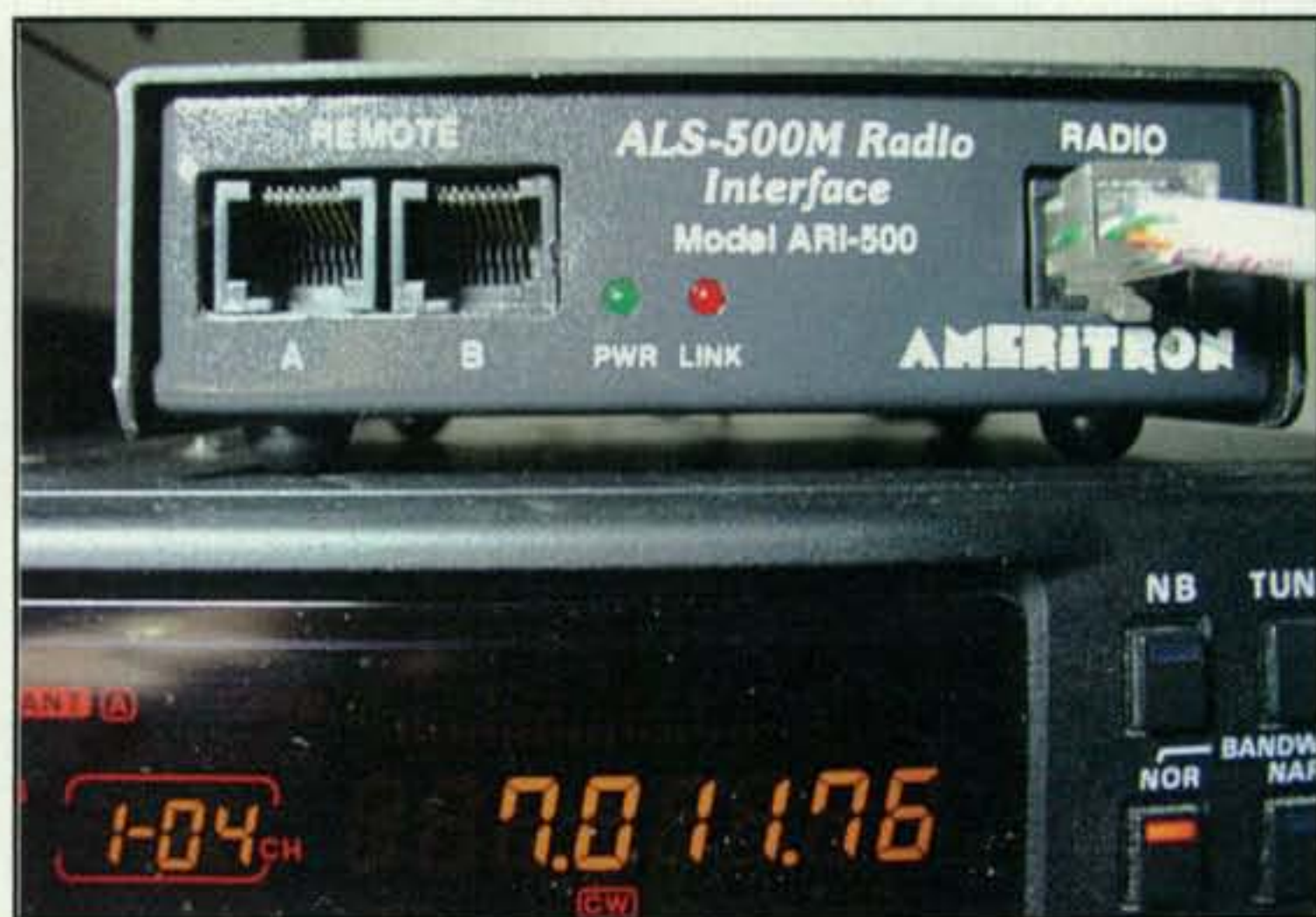
Photo E—ARI-500 on the author's transceiver. If used, the ALS-500RC plugs into REMOTE A.
