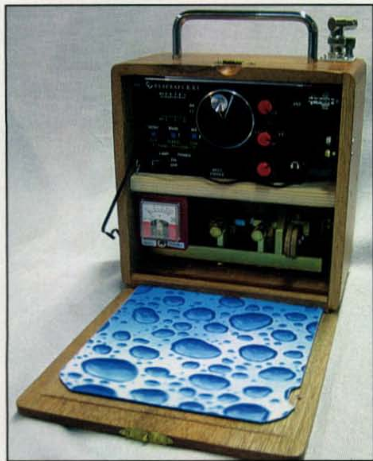
Photo A— This all-in-one-box QRP station assembled by Bob Zimmer, NV1X, truly deserves a second look. It consists of an Elecraft KX-1 transceiver fitted with custom knobs, a 12-volt/1.2-amp/hour battery, K4VIZ right-angle bug and battery monitor meter in a fancy wood cigar box. Nice! (Photos A & B courtesy of NV1X)
