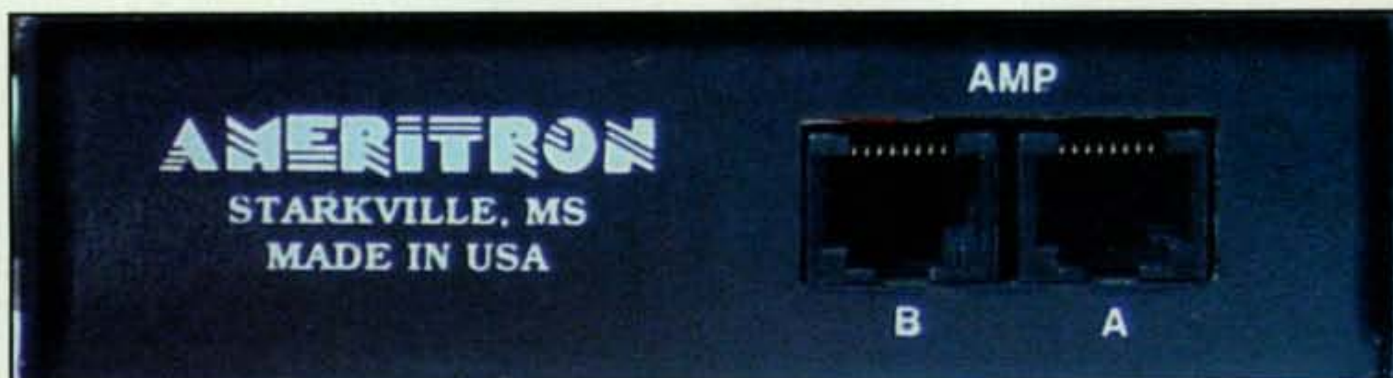
Photo F—Amplifier interface cables connect to these ports on the rear of the ARI-500.
