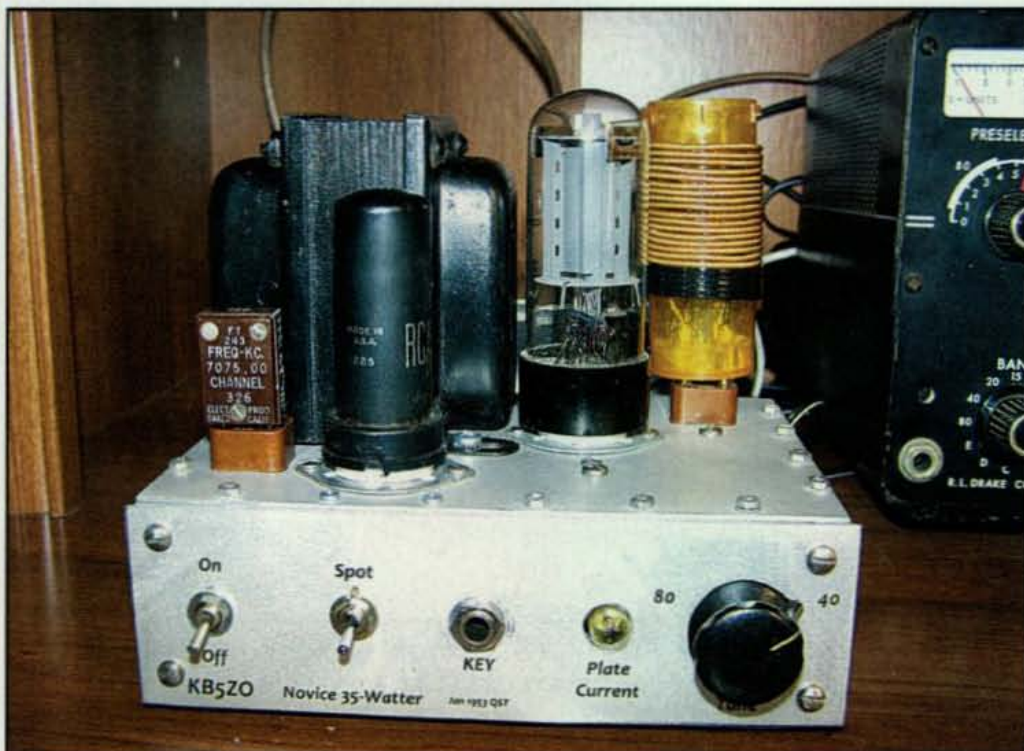
Photo C— Reuben (Ben) Staff, KB5ZO, went all out, homebuilding his two-tube transmitter (6AG7 driving a big 6L6) on a metal chassis. The little gem has plug-in coils that mate with dual crystal sockets, and it pumps out 14 watts on 40 meters or 22 watts on 80 meters. Note the use of a pilot lamp in lieu of a plate current meter. Here you tune for minimum lamp brightness. Total class! (Photos C, D, E, and F courtesy of KB5ZO)
