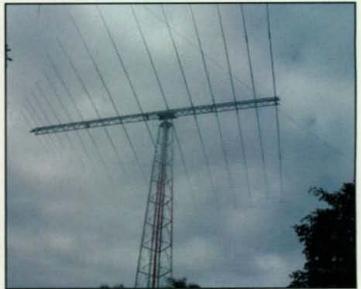
The big 16 element Log Periodic atop the 48 foot tower. (Photo courtesy of Doug, ZP6CW)
