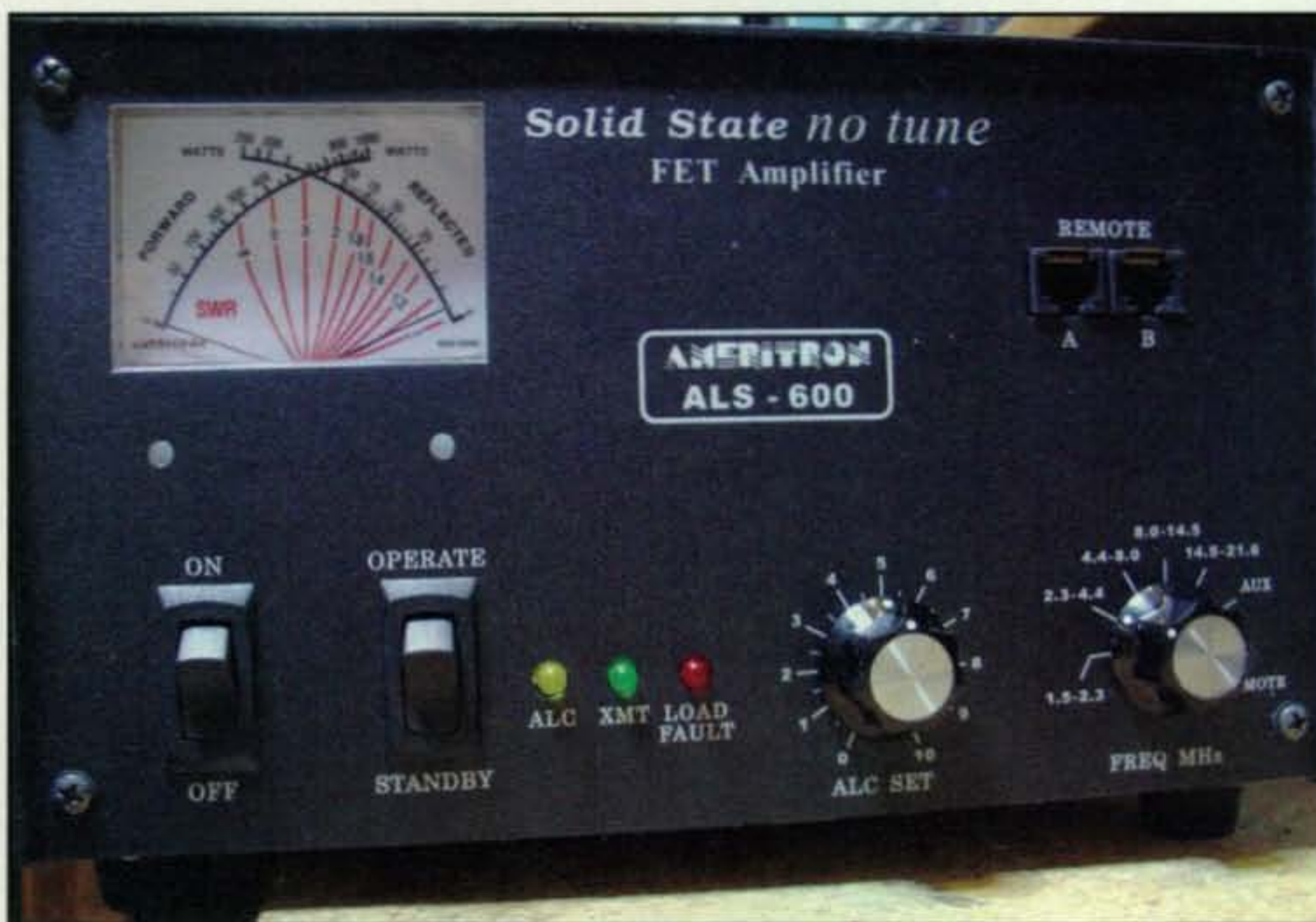
Photo A— The ALS-600 provides 600 watts PEP on SSB from 1.8–30 MHz. RJ45 jacks (upper right) provide optional remote-control capability.
