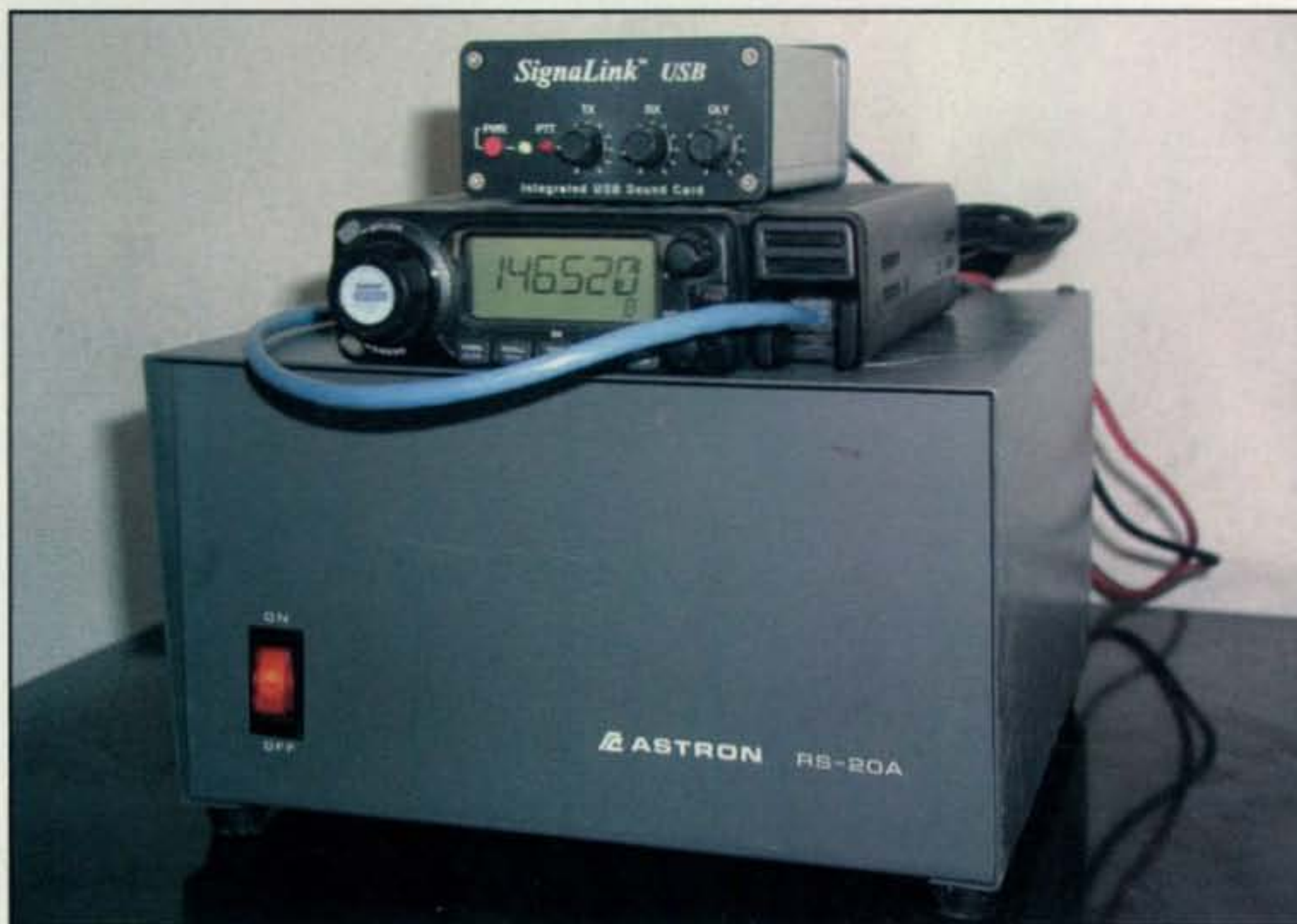
Photo B— WB6JAR's VHF station set up for remote operation via cell phone using a Signalink sound card adapter and Skype software.
