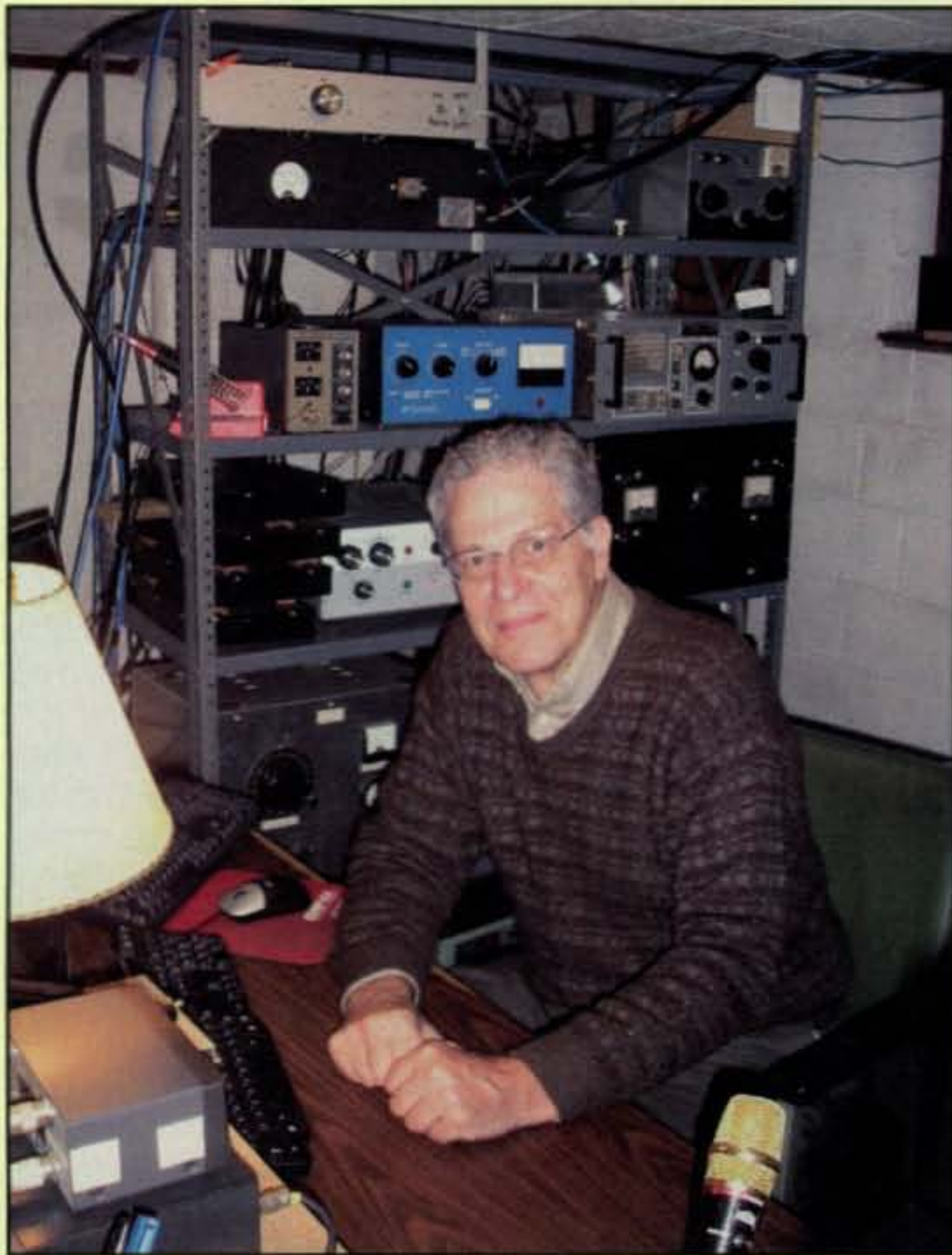
The metal shelf unit behind Joe contains the "guts" of his VHF/UHF station, filled with transverters, amplifiers, and other assorted goodies (except for his 2300-MHz station, which is barely visible on the window sill at the right).
