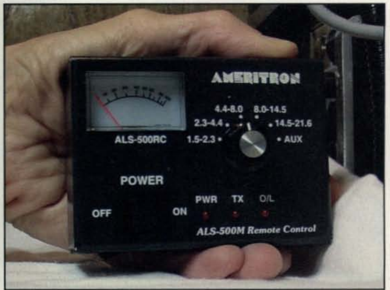
Photo C— The compact ALS-500RC provides all the control and monitoring needed.
