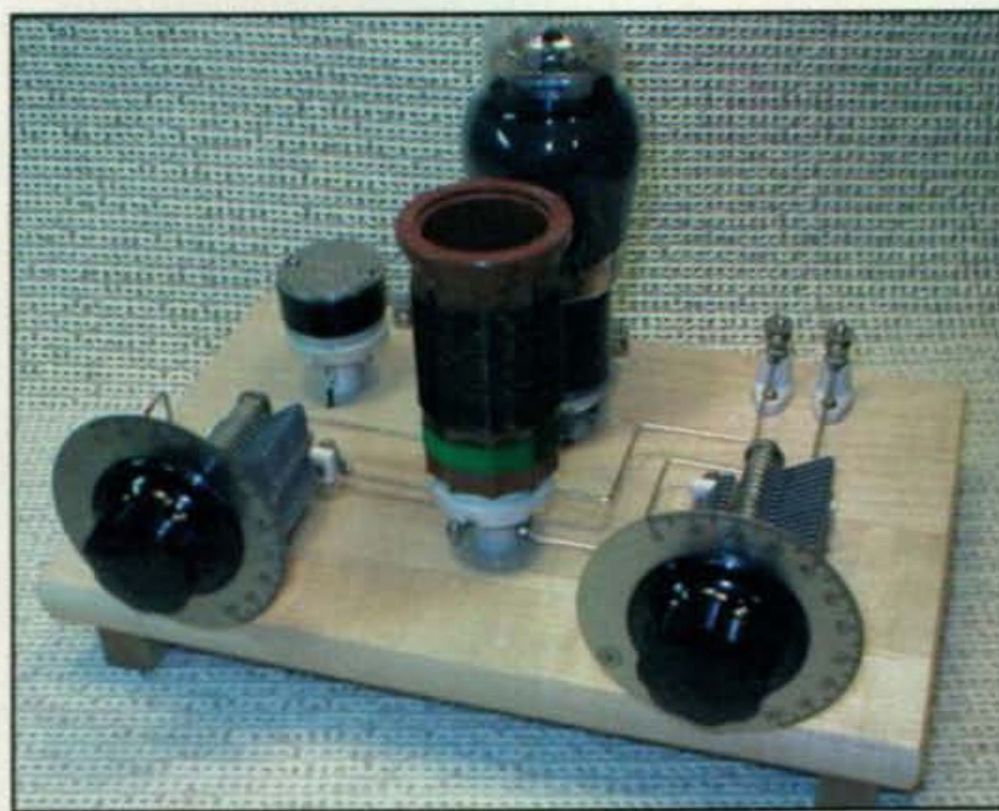
Photo A— A late 1930s-style transmitter like this heartthrob built by Louis Vermond, VE3AWA, truly brings tears of joy to an old-pro amateur's eyes. The ST-100 tuning condensers, CIR tube sockets, and R-100 RFCs are from National. The round LD2-type crystal is a Bliley. The output standoffs are of E. F. Johnson manufacture. The coil form is an SWF-4 Hammarlund, and the dials are Millen-10009's. The rig pumps out 10 watts on 80 meters. Wow! (Photos A and B courtesy of VE3AWA)
