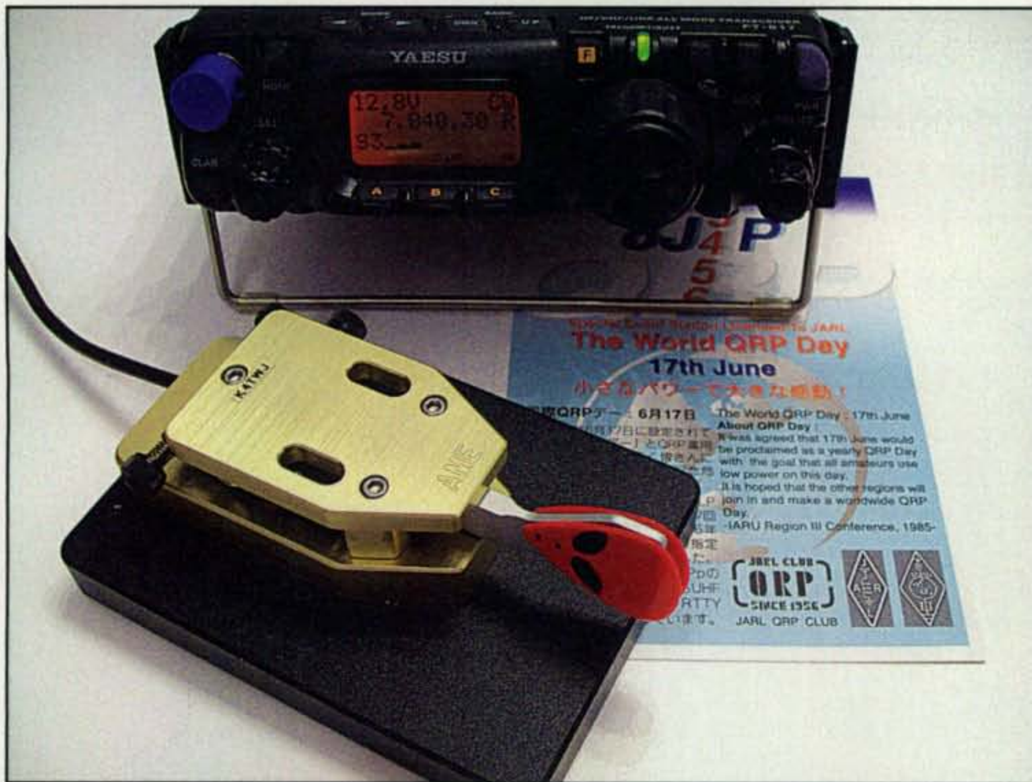
Photo E— Here is the fully assembled and fine-adjusted Bushwhacker paddle (with a couple of guitar-pick fingerpieces I added for flash and class) in operation with my Yaesu FT-817 during World QRP Day. The little Bushwhacker looks and handles quite well. It is not in the Begali or N3ZN class, but neither is its price. More details in the text.
