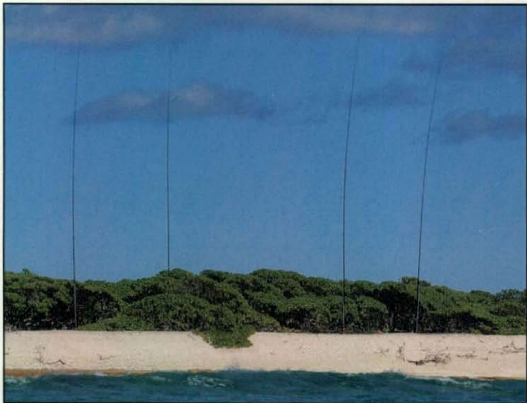
Photo C— Here's how VP6DX uses his Spiderbeam poles—to build a 4-square vertical antenna using four 18-meter Spiderbeam poles to support four vertical radiators.
