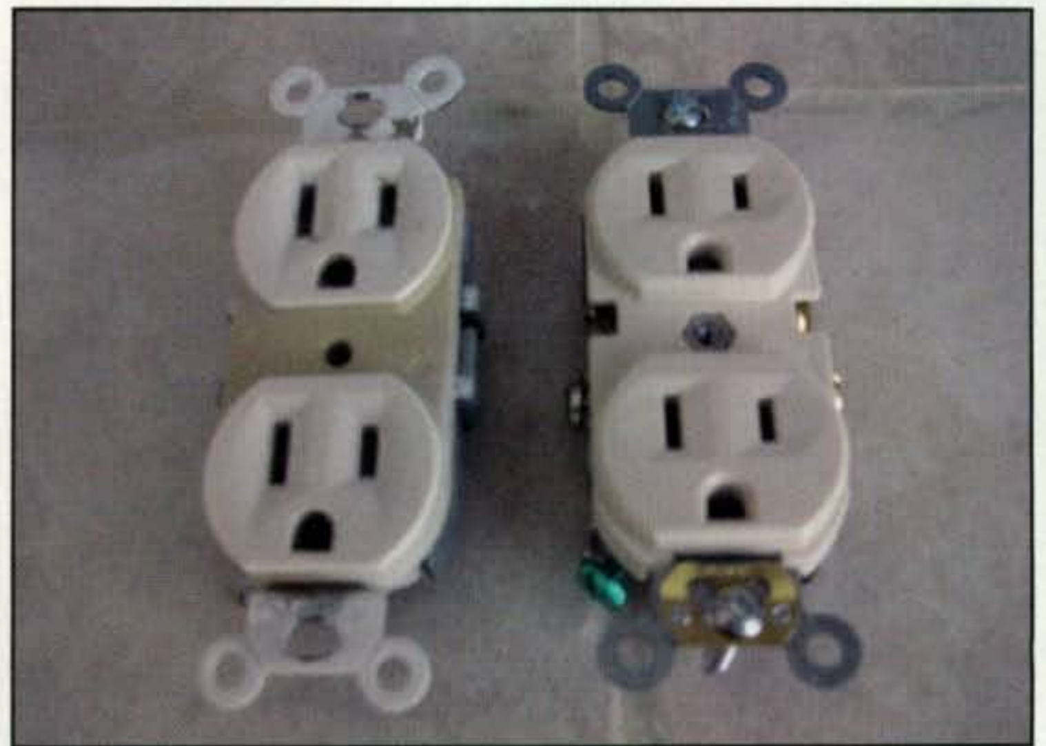
Photo 6— Inexpensive AC outlets should be replaced with better-quality units. Many of these in my new house were either very loose or too tight.
