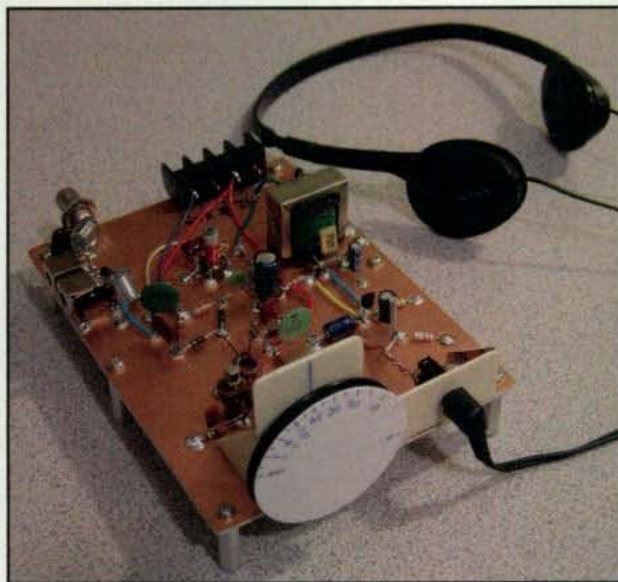
Photo B— Close-up view of Mike's prototype Reggie transceiver built Manhattan style on a large piece of unetched copper-clad board. This version has tiny IF cans, which were changed to regular toroids for production as a kit by QRPme.com. (Photo courtesy of AA1TJ)
