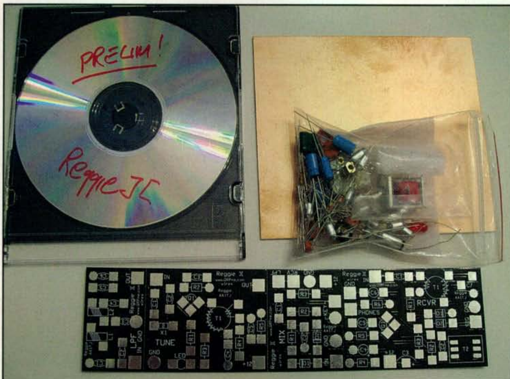
Photo E- The new Reggie II mini transceiver kit as received from W1REX of www.QRPme.com . You start by snapping the four boards apart and placing components in bags or boxes with their respective boards. Full instructions are on the QRPme website or on the CD that comes with the kit.
