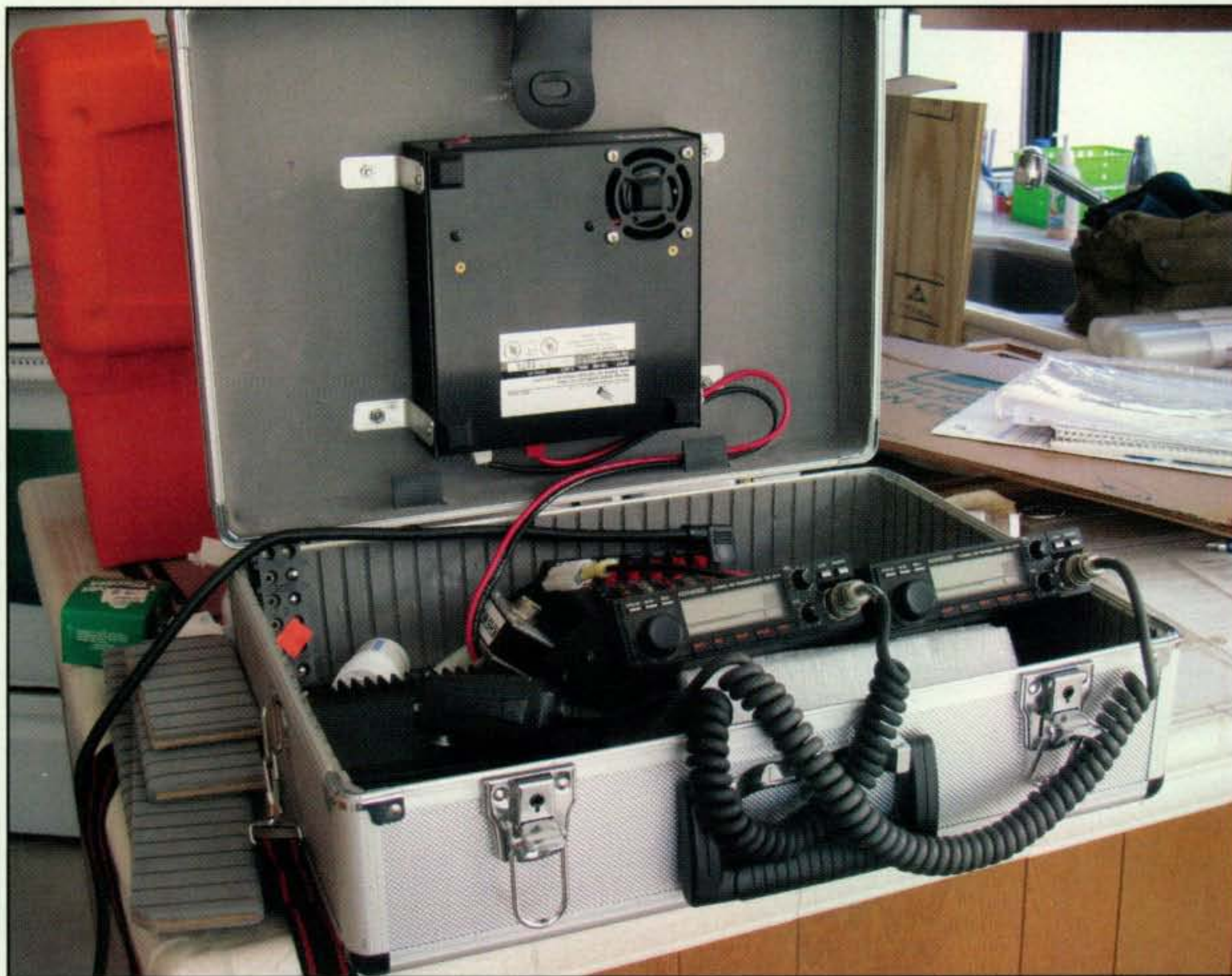
Photo 1— A three-band VHF/UHF radio station can be made with mobile radios mounted in a briefcase-style toolbox available from a local hardware store for about $20. A compact 23-amp switching power supply powers the rigs if AC is available. The portable station can also be powered using a large 12-volt battery box. (Photos by the author)
