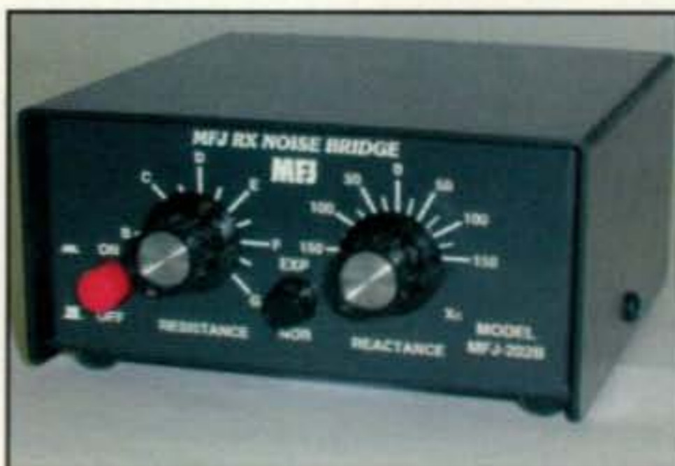
Photo G— Meet the poor-man's antenna analyzer—the noise bridge. When used in conjunction with your HF receiver or transceiver, it measures an antenna's resonant frequency and feedpoint impedance. The item shown is the MFJ model 202B, available from amateur radio dealers nationwide.
