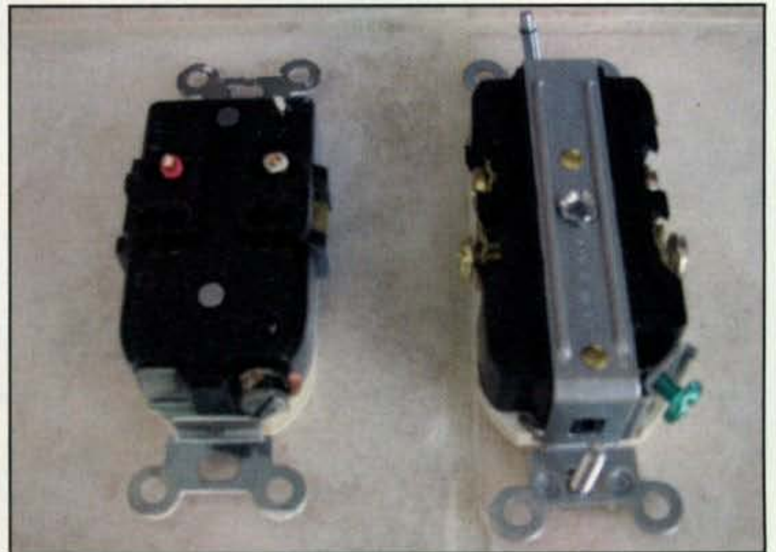
Photo 7— The outlet on the left has push-in connectors and is imported. How secure can a push-on connector be after 20 or 30 years? The unit on the right is an upgrade, with screw-down terminals, more robust contacts, and made in the USA. Both are from the same manufacturer.
