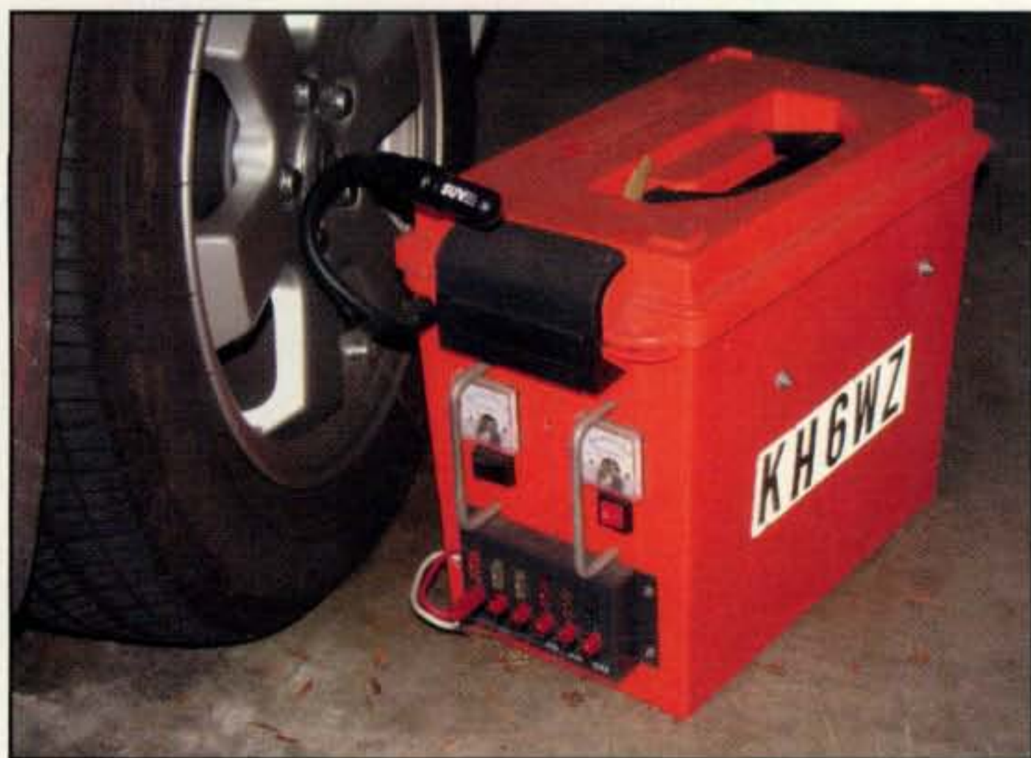
Photo 2— The portable station can be powered with a large gel-cell. I housed my battery box in a sportsman's "dry box" available from a local camping equipment store. I added a small Rig-Runner unit and voltage and current meters to the box.
