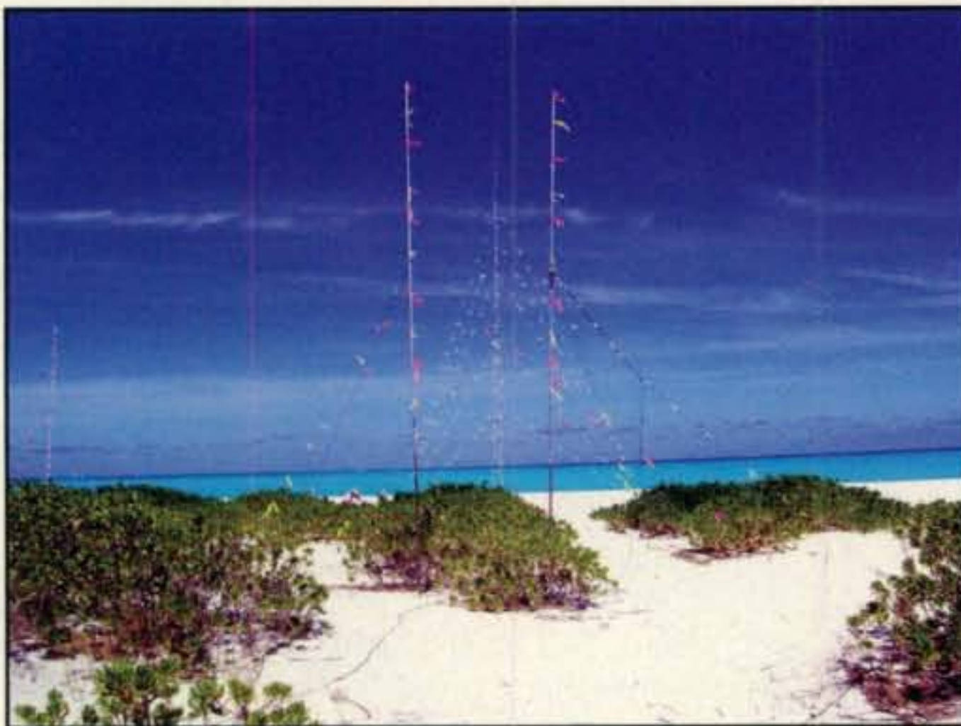
The antennas on Midway (K4M) had to be "flagged" for the protection of the birds who could have been hurt flying into all that aluminum. (Photo courtesy of Tom, N4XP)
