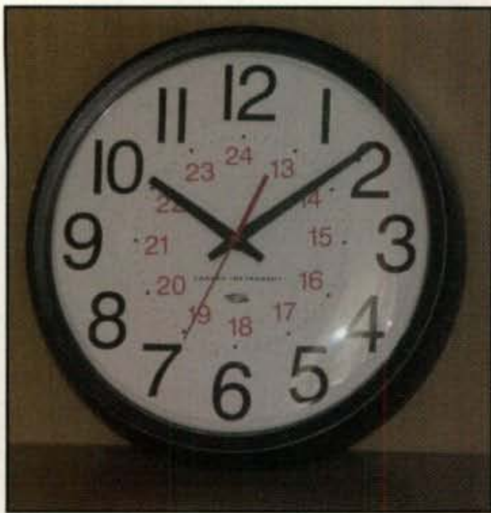
Photo 6—A station clock is a great decorative yet functional accessory for any ham station. This analog clock was on sale at a local office -supply store. It has an "atomic time" function that automatically re-sets for Daylight Savings Time. A by-pass switch enables one to set the clock to a different time zone, such as Universal Time.
