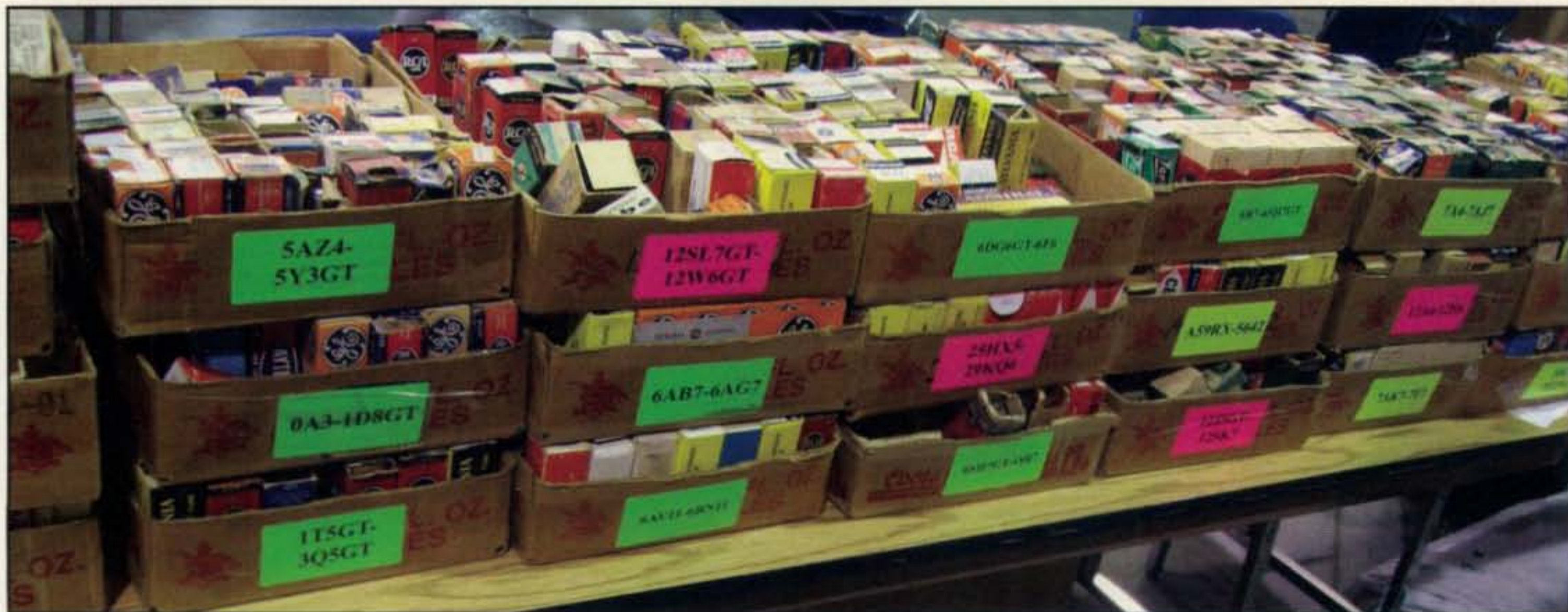
Photo D— A couple of hamfest flea-market acquired RF and IF amplifier tubes can breathe new life into a vintage receiver and they are usually available at reasonable cost. Check your receiver's or transmitter's manual or look at its existing tubes for proper numbers before asking for help locating the tubes.
