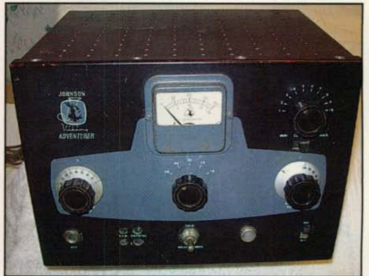
Photo B— This well-kept Johnson Adventurer transmitter purchased at an unbelievably low price at a hamfest produces a beautiful vacuum-tube-quality 25-watt signal on the 80 through 10 meter bands. Plug in a crystal, add a VXO circuit in series with the crystal, and it can easily cover 10 to 20 kHz of a favored band segment.
