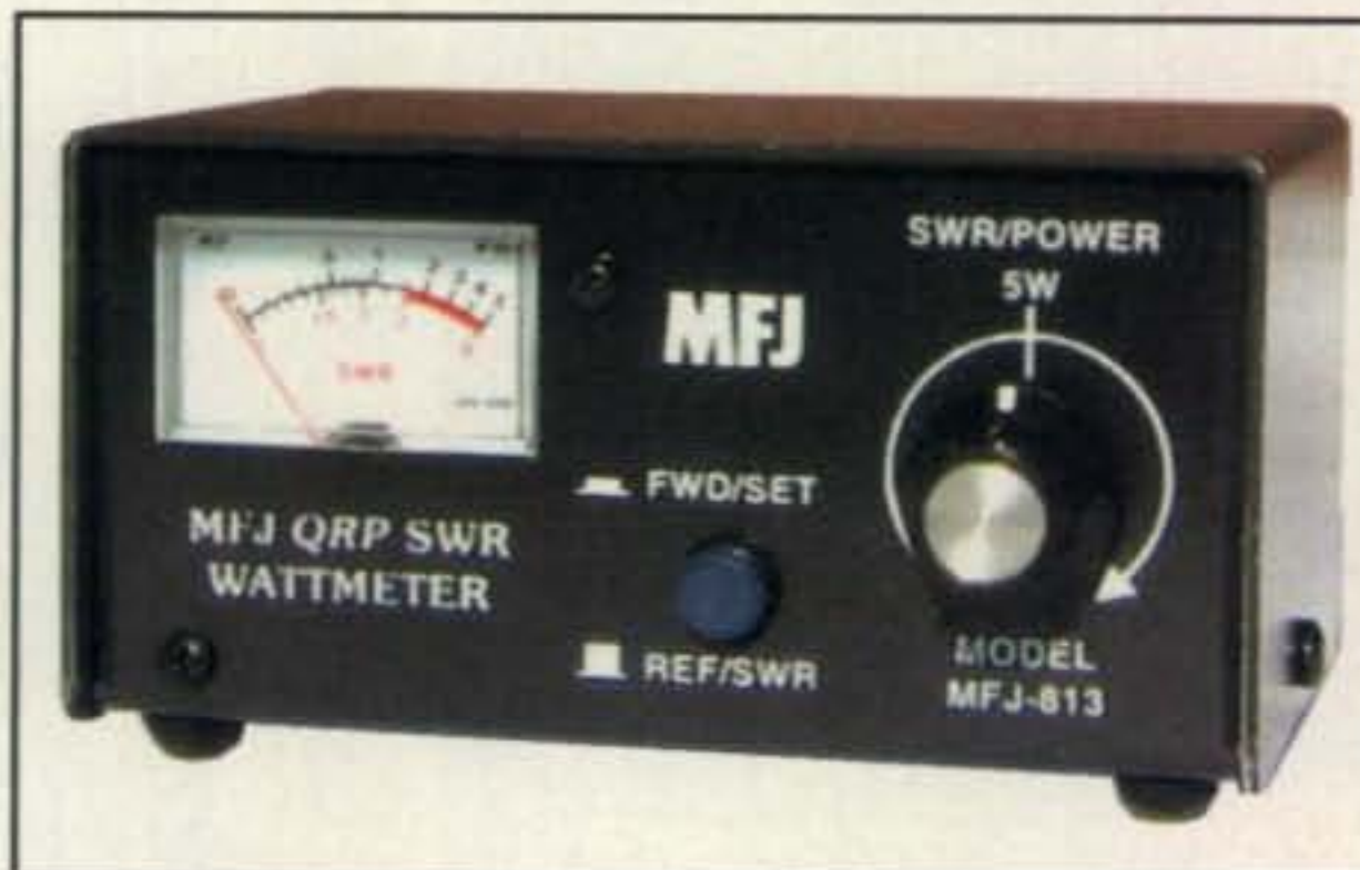
Photo 3— Working on QRP radios, running on-the-air QRP signal trials, or setting up antennas can all be made a little easier through the use of the compact MFJ-813 QRP Wattmeter and SWR Bridge which reads forwarded and reflected power from zero to 5 watts and covers 1.8 to 50 MHz. (Photo courtesy of MFJ)
