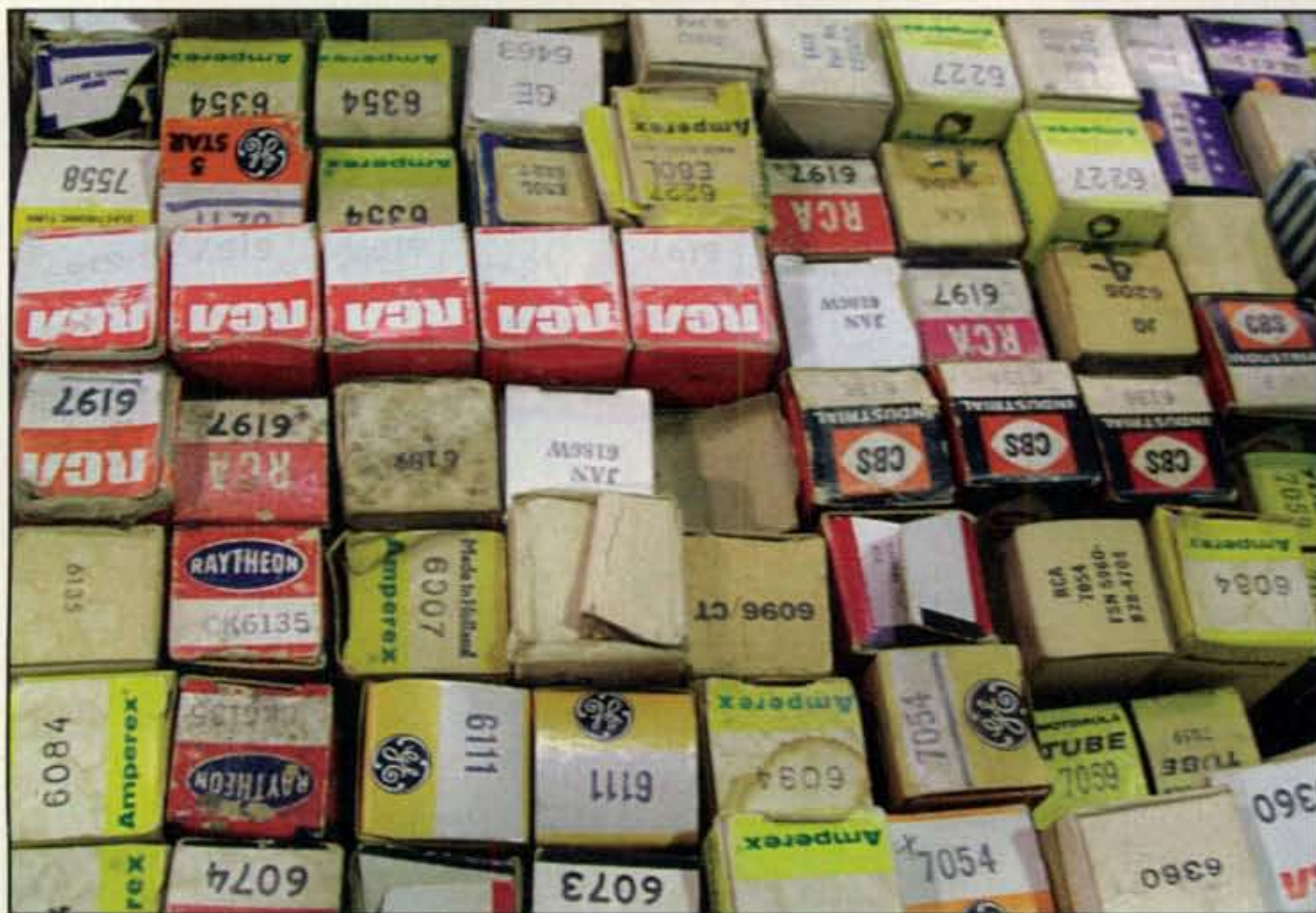
Photo E— Many times conventional tubes can be replaced with four-digit industrial equivalents and the resulting performance plus extended tube life make them "good buys." Tube dealers usually have a cross-reference or replacement guide on tube types.
