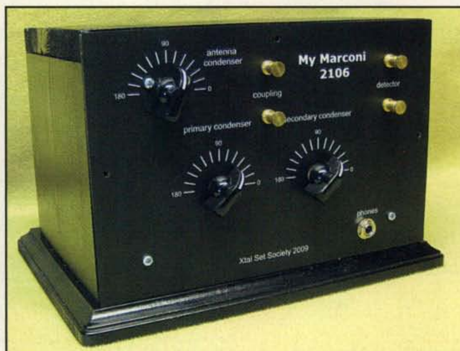
Photo D— This spiffy little 2106 crystal set, also available as a kit from the Crystal Set Society, is fashioned after Marconi’s original type 106 receiving tuner. Its 10-inch by 6.6-inch front panel includes a 10-mil thick lexan plastic sheet with black-and-white graphics on the back, and the optional cabinet adds to the set’s historical glamour!
