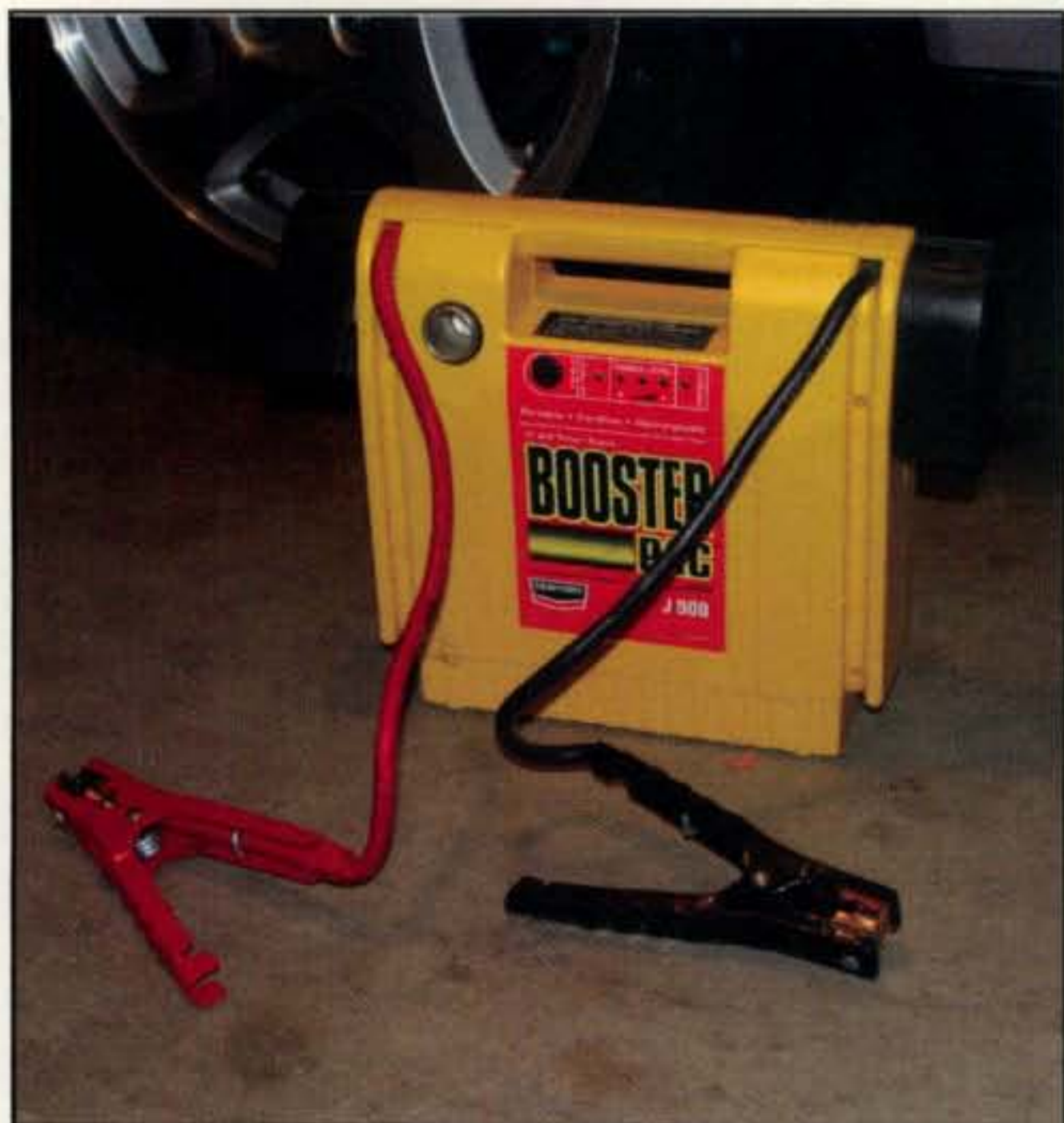
Photo 4— A booster battery can be used to jump-start a vehicle. It is also a very handy source of 12-VDC power for ham radio sets.
