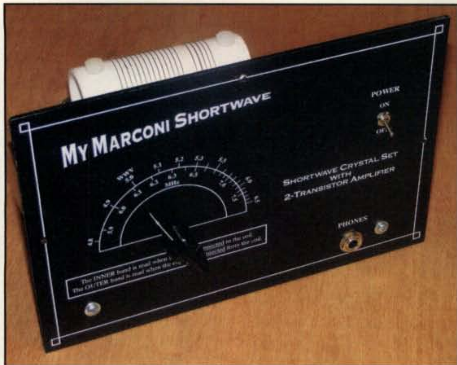
Photo E—A shortwave crystal set? Yes, indeed, and it works reasonably well to boot. This new kit from The Crystal Set Society covers the always active range of 5 to 7.5 MHz and includes a two-transistor audio amplifier to give it “big radio” signal levels. An optional wraparound cabinet (8" x 7" x 6") adds a finishing touch of class.
