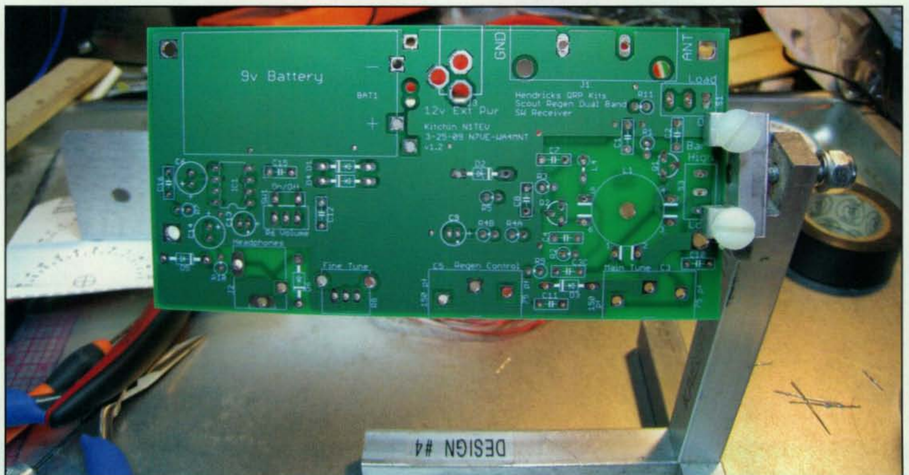
Photo C— The PC board for the Hendricks Scout Regen kit is a double-sided board with plated-through holes for easy soldering.
