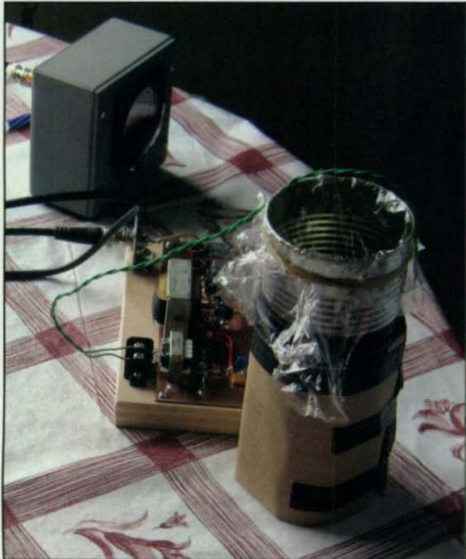
Photo D— Can and cardboard speaker baffle portion of the AA1TJ Code Talker transmitter designed by Michael Rainey, AA1TJ. Look carefully and you can see the circuit assembled "Manhattan Style" in the background. (Photo courtesy of W1REX)
