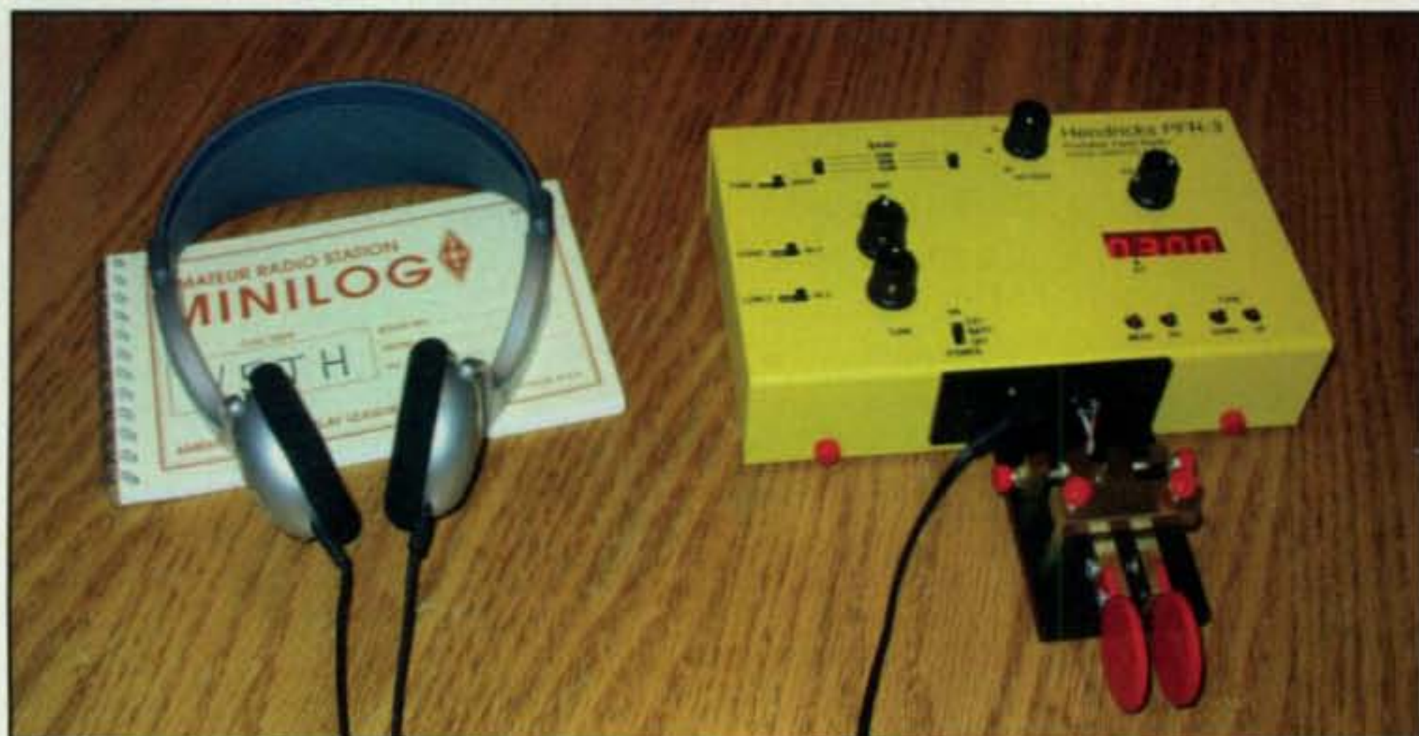
Photo H— Here is the new Baby Black Widow CW paddle kit from W5JH attached to the front of a popular PFR-3 QRP transceiver for stand-alone field use. The paddle can also be removed and used stand-alone style with any other transceiver. (Details in text.)
