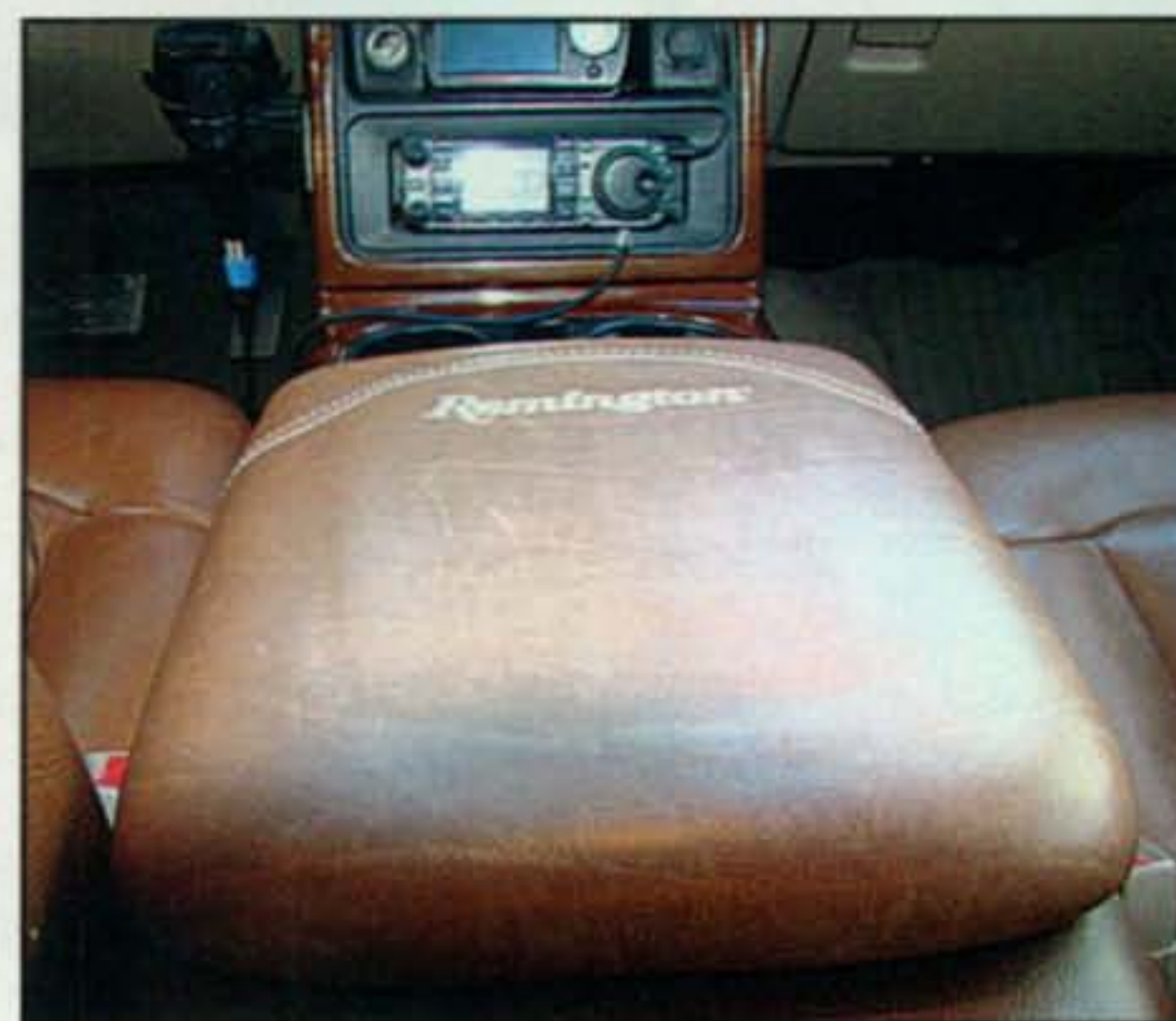
Note the "hidden" armrest installation that places controls at the operator's fingertips.
