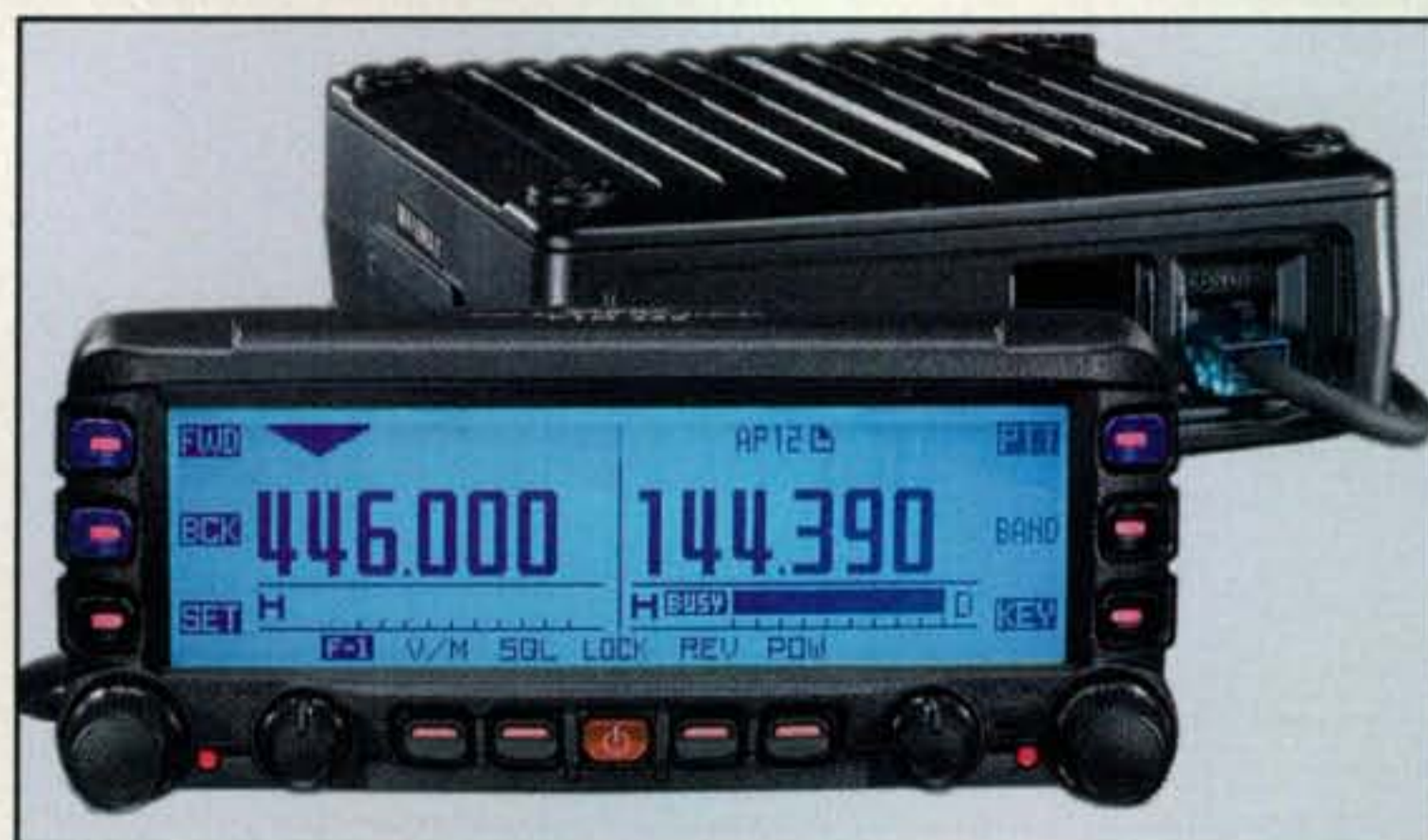
The brand-new FTM-350R from Yaesu is a tri-bander, operating on 2 meters, 222 MHz, and 70 centimeters (only two frequencies at a time on the display). Plus, it's APRS-ready and compatible with an outboard GPS receiver.
