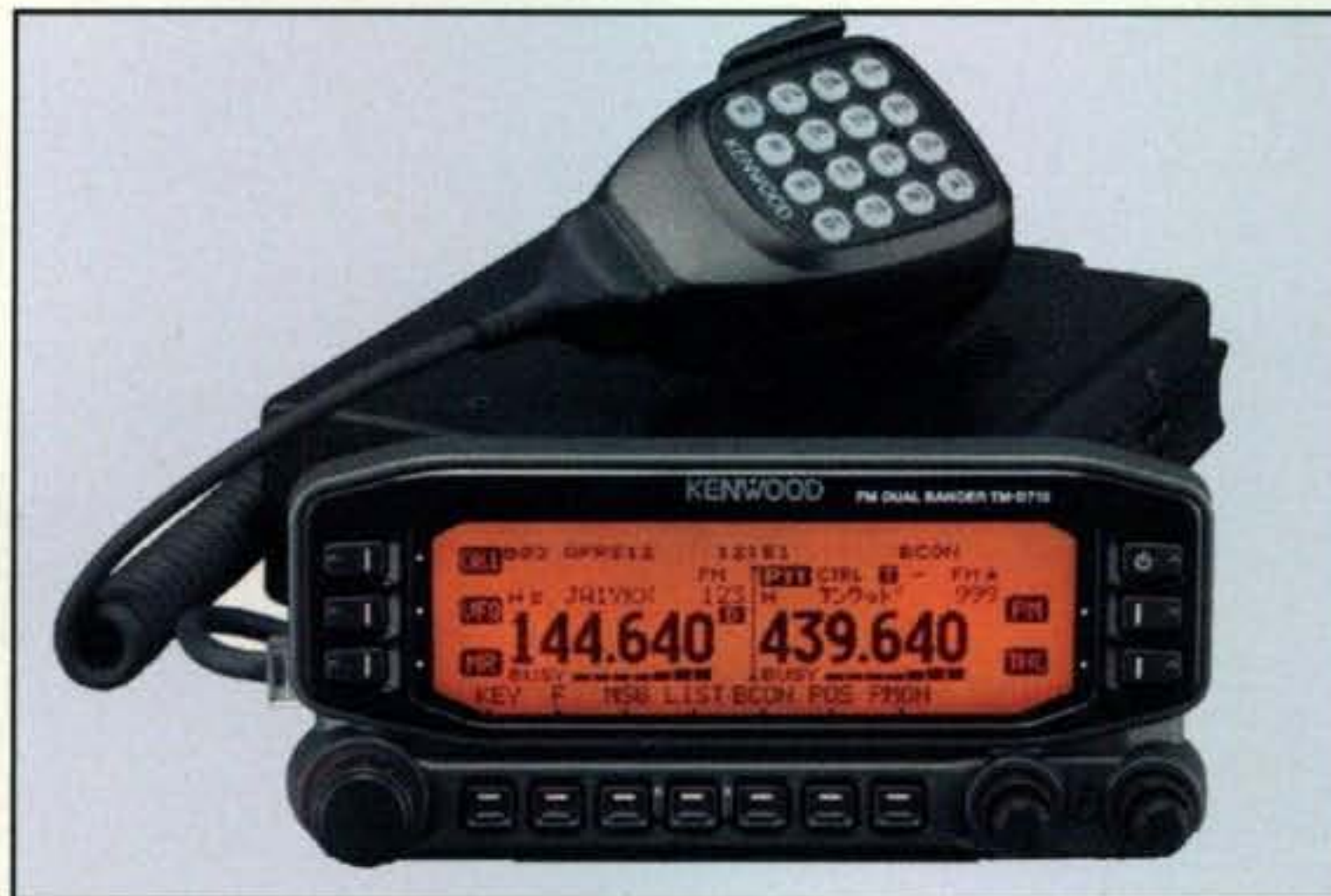
Kenwood's new TM-D710A is not only a true dual-bander (two simultaneous frequency displays) for 2 meters and 70 centimeters, but comes APRS-ready and can team with the AvMap G5 receiver to give you full mapping on the big display screen. Plus, it can be used to remotely operate a Kenwood TS-2000 HF rig via the company's Sky Command system.
