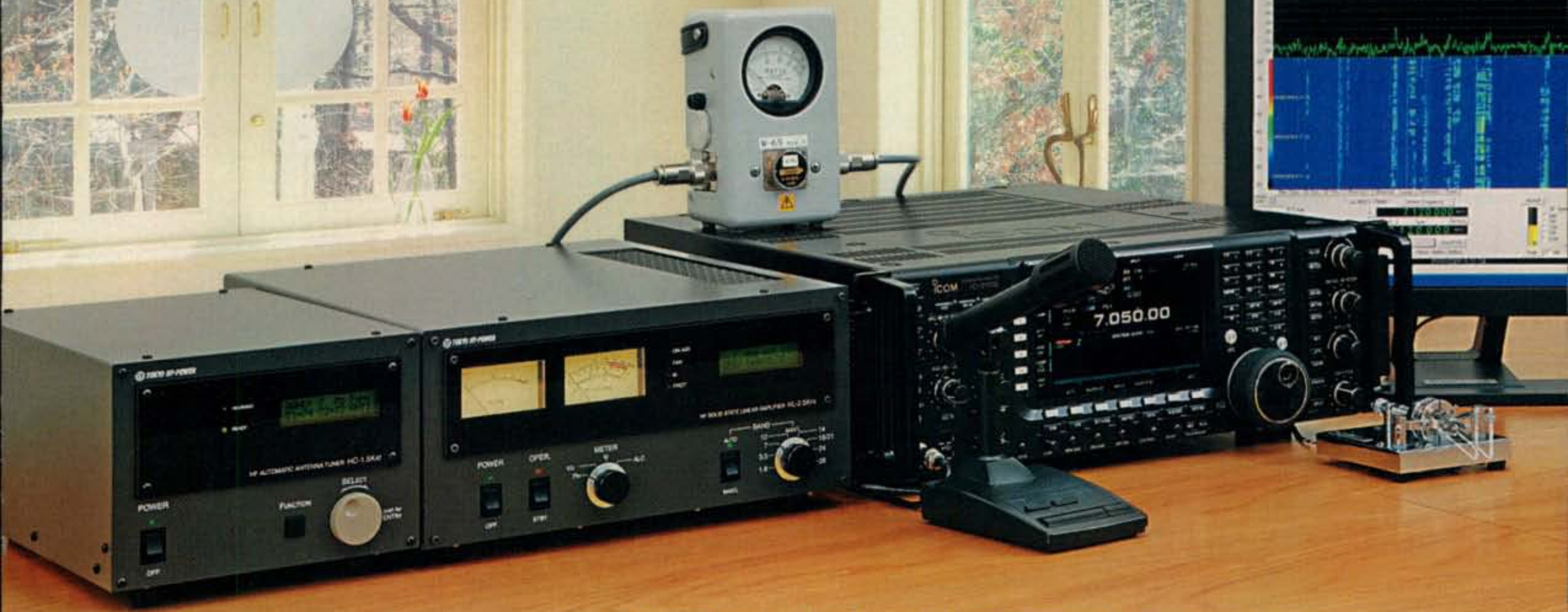
Photo : From left HC-1.5KAT (HF 1.5kW Tuner with Auto Band Set Feature), HL-2.5KFX (HF 1.5kW MOSFET Linear) and IC-7700 Transceiver
