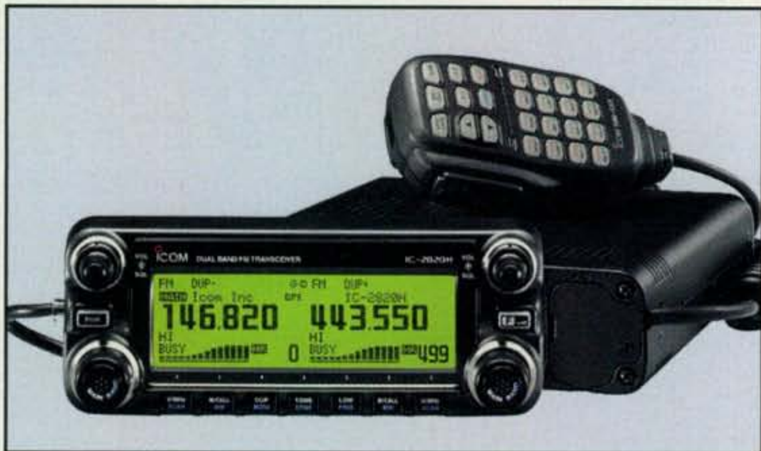
ICOM's top-of-the-line dual-bander is the IC-2820H, which not only offers a huge frequency display and built-in D-STAR capability, but built-in diversity receive if you have two antennas and set both VFOs to the same frequency!
