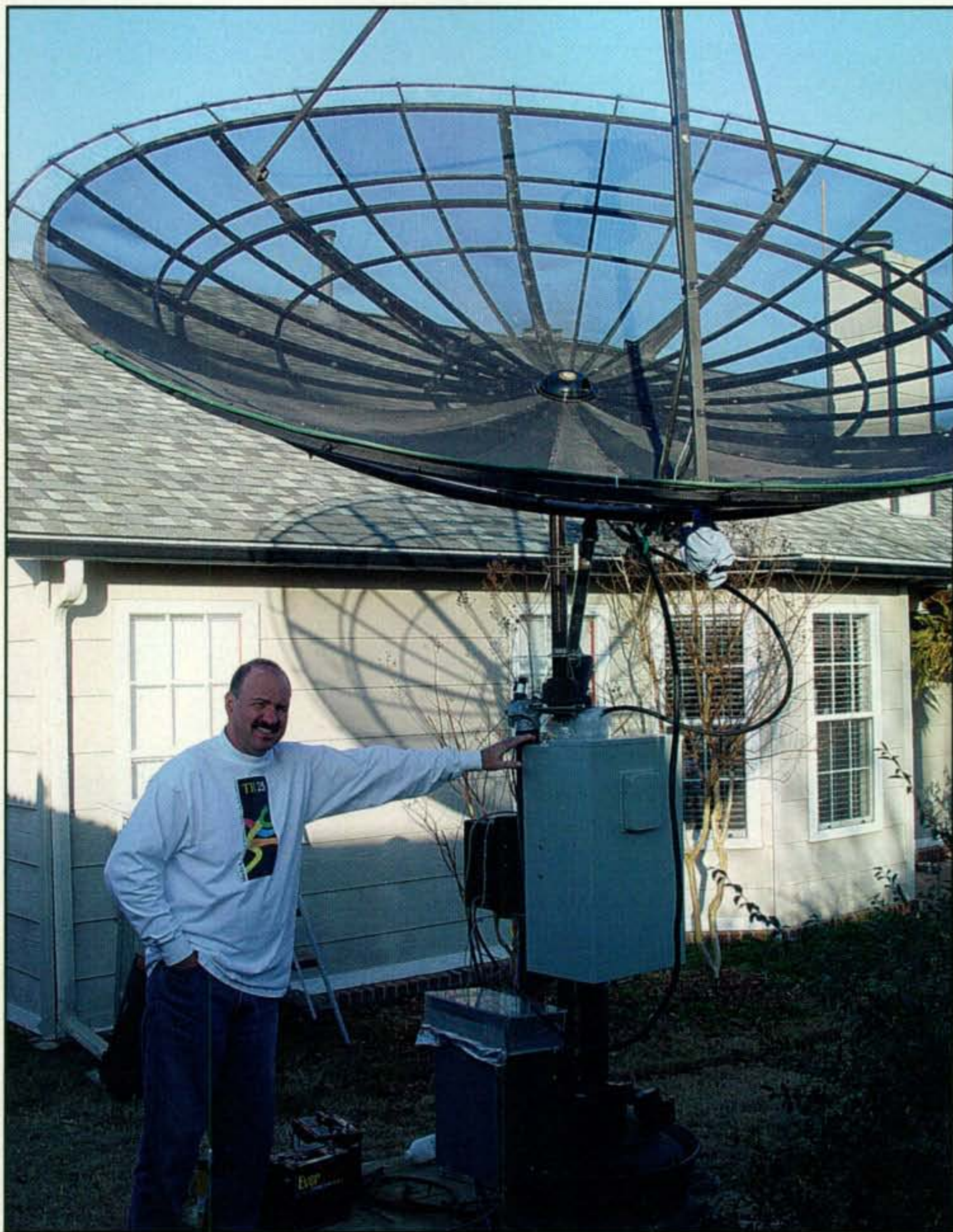
Photo 4— WD5AGO points to the watertight cabinet that houses his 200-watt solid-state amplifier for 13 cm, which is mounted just below his 3.1-meter dish.
