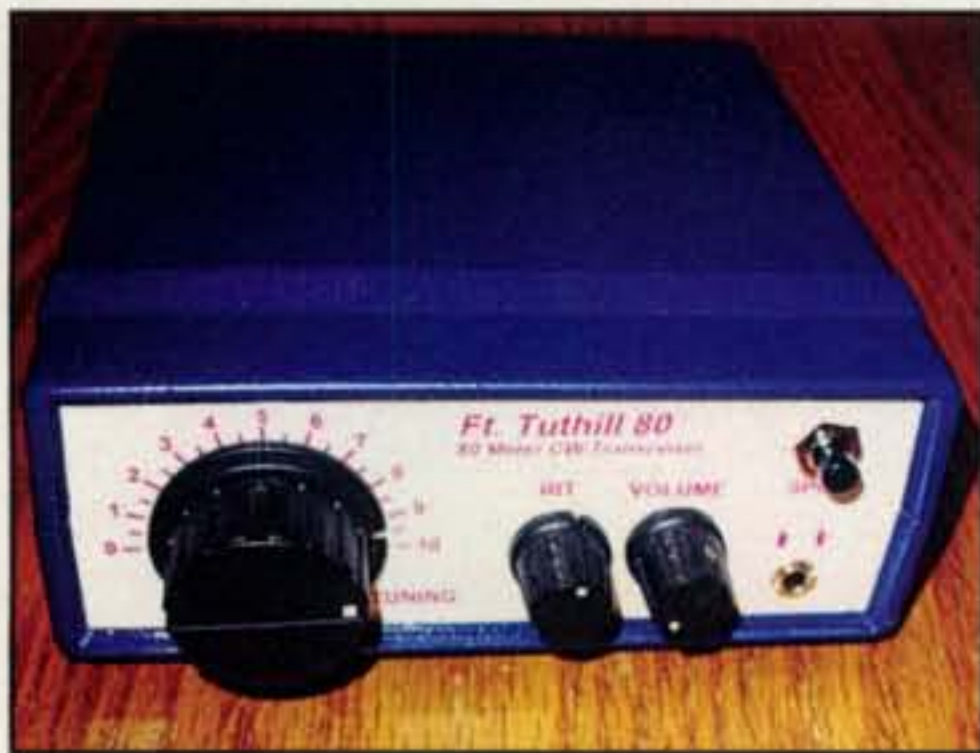
Photo F— One of the new Tuthill 80 mini transceiver kits available from < www.azscqrpions.org >. This beauty was built and mounted in a neat blue enclosure by W5JH.
