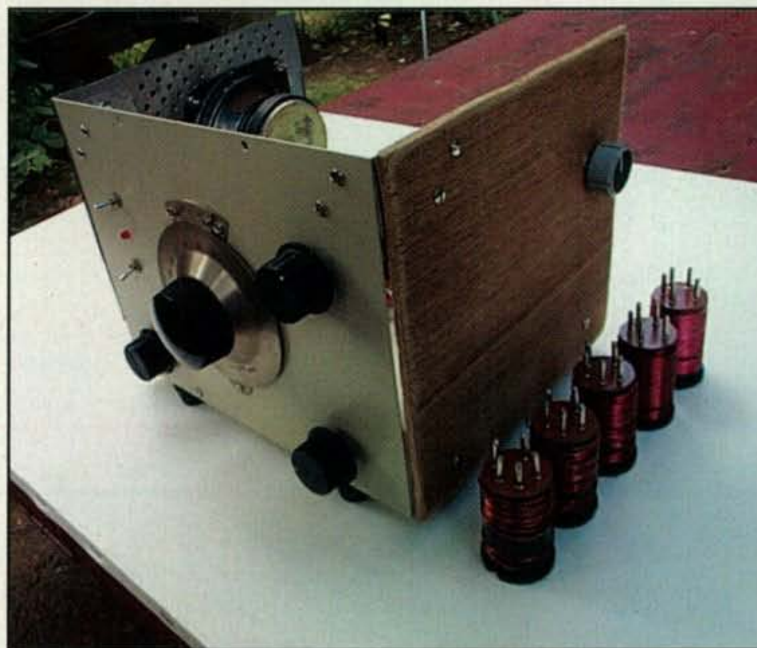
N1TEV's high-performance regenerative receiver will cover 480 kHz to 18.5 MHz, depending on which coils you plug in.
