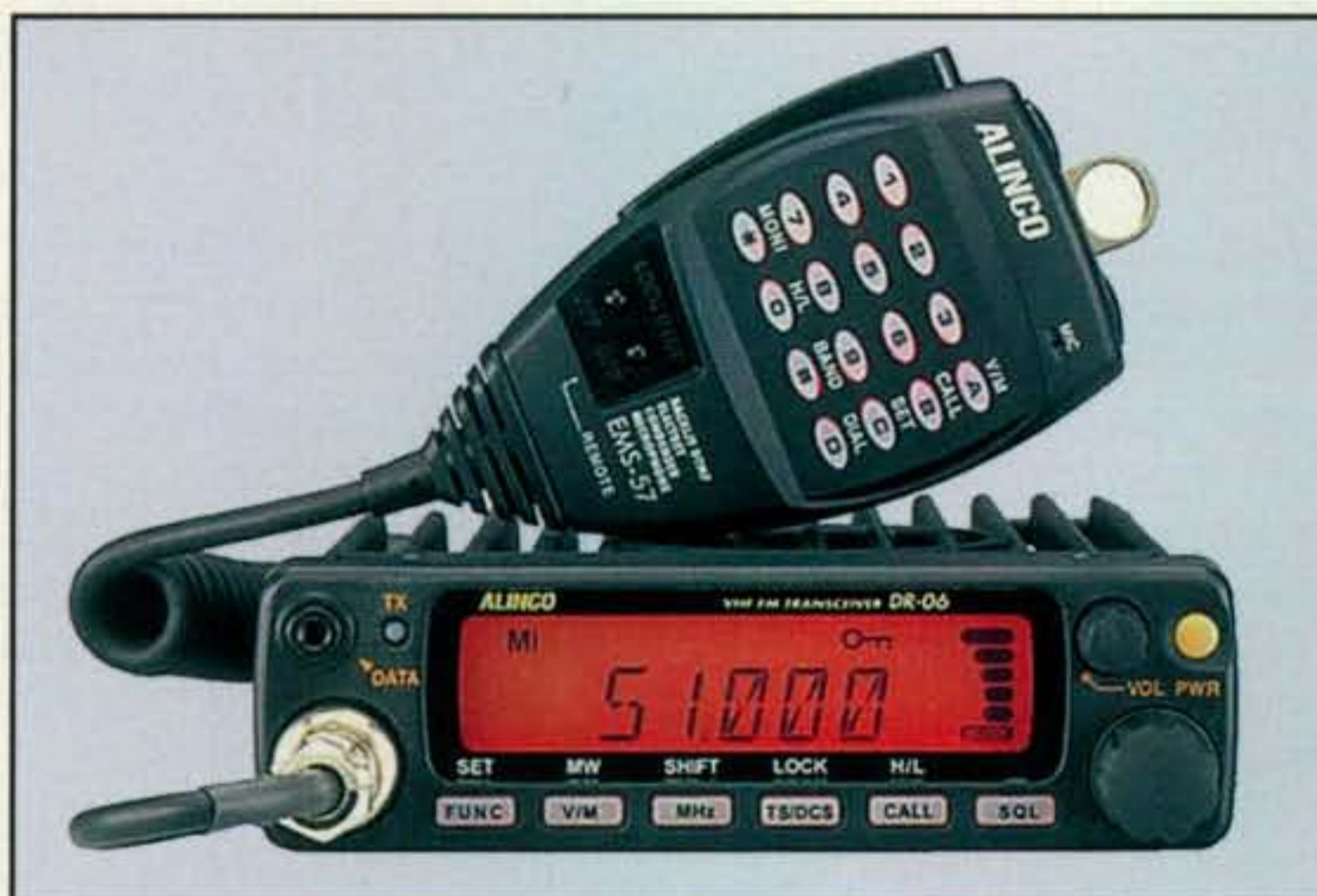
The Alinco DR-06 is one of the few 6-meter FM rigs on the market today. Alinco also has single-banders for 2 meters, 222 MHz, and 70 centimeters.
