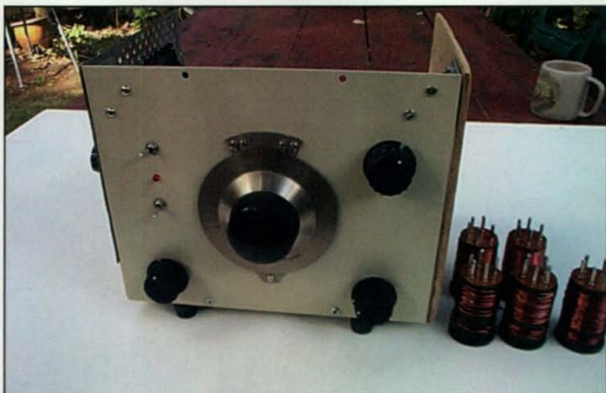
Operating this radio is a two-handed job. One hand spins the tuning dial while the other controls the regeneration level, as the two controls work in tandem.
