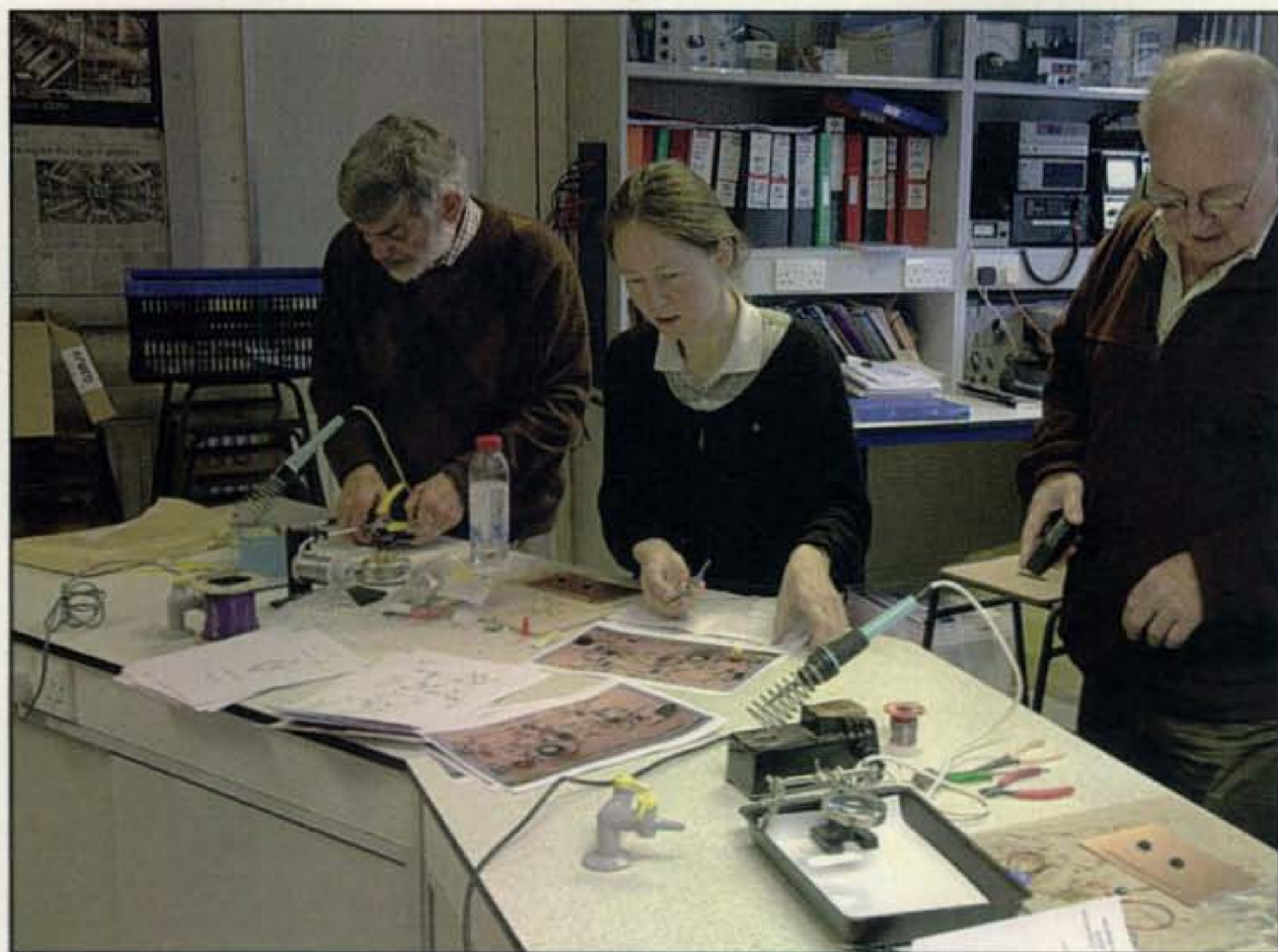
Photo C— Rev. George Dobbs, G3RJV, looks on as Agnes, M3XYF, and Clive, M5CHH, work as a team begin assembling a Sudden receiver during the buildathon at the Rishworth Convention in England. Note the two IC sockets pre-installed on the board and easy-to-duplicate layout guide, both included in convention kits supplied by W1REX of <www.qrpme.com>.
