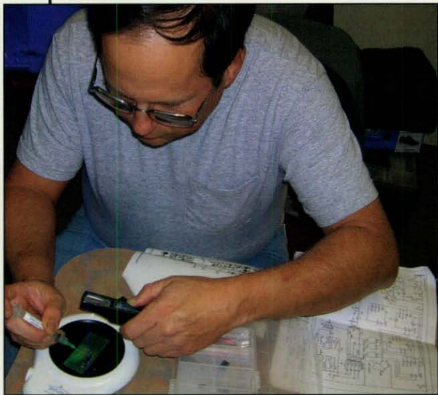
Arnie Grubbs, KA0NCR, using a solder-paste syringe on a PC board. Solder paste and a low-airflow heating tool from a craft store can make mounting surface-mount parts easier.
