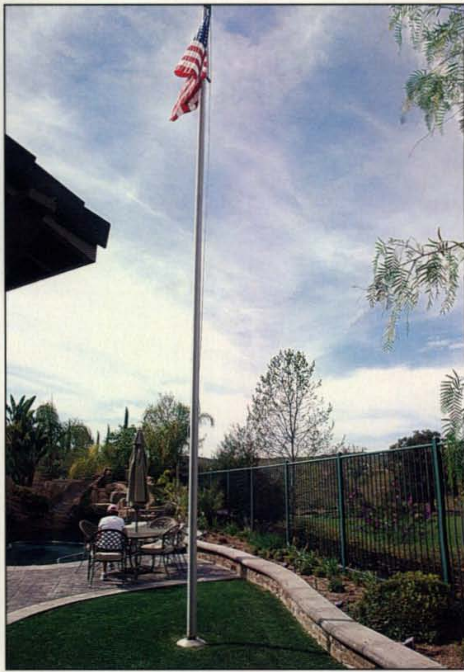
Photo F— Proceeding through a second gate and around a corner, we find Howard's main antenna, a 28-foot tall flagpole vertical with 80 radials ready for action.
