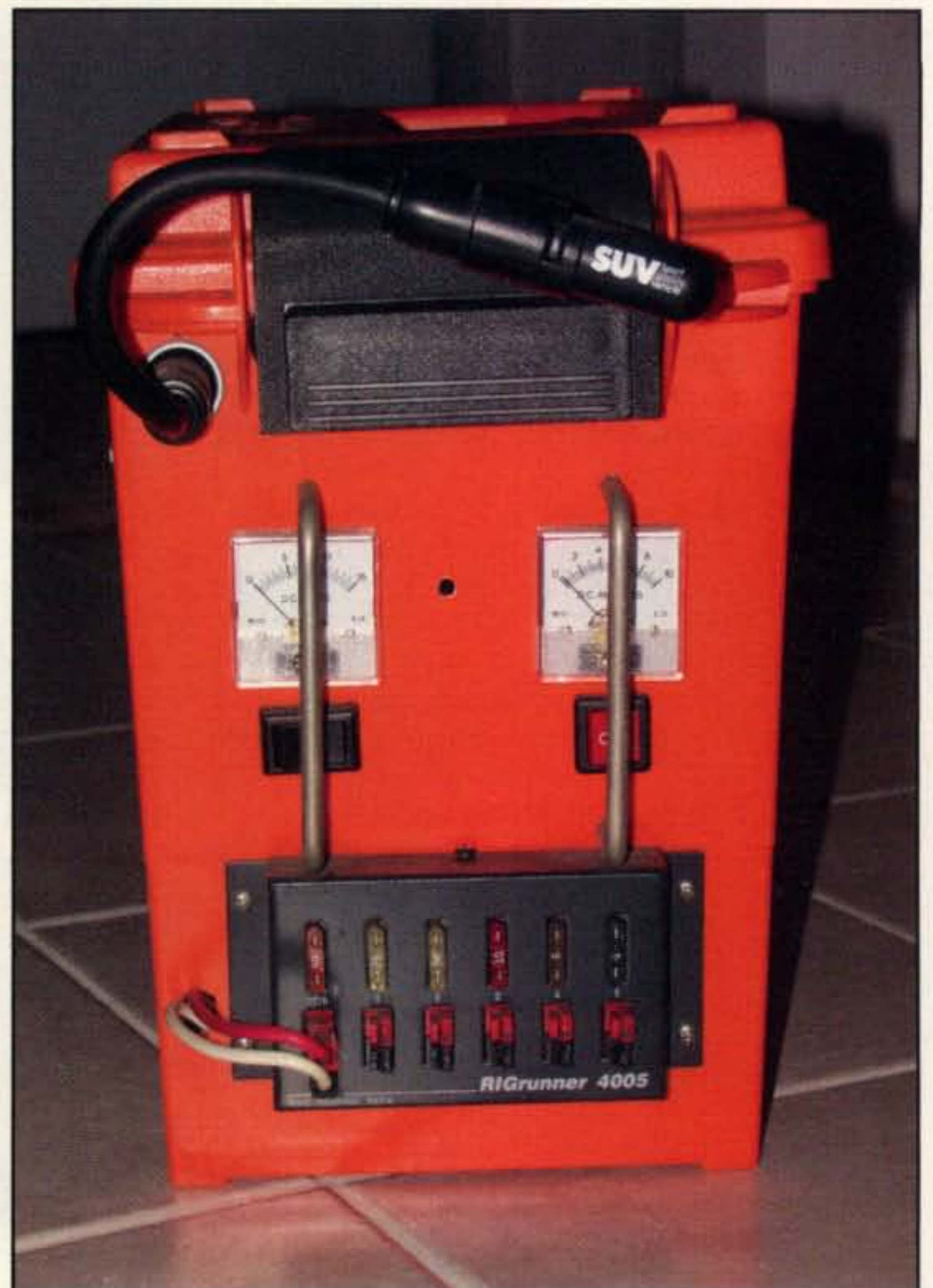
Photo E— The homemade power box includes enhancements such as meters to monitor battery condition and multiple DC outlets. The wire handles help protect the meters from damage.
