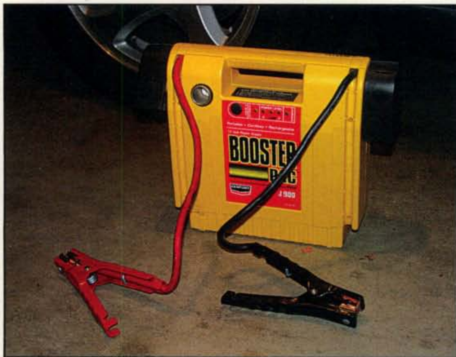
Photo B— An automotive emergency starter battery can be used as a portable power source, but some minor modifications will increase safety and convenience.
