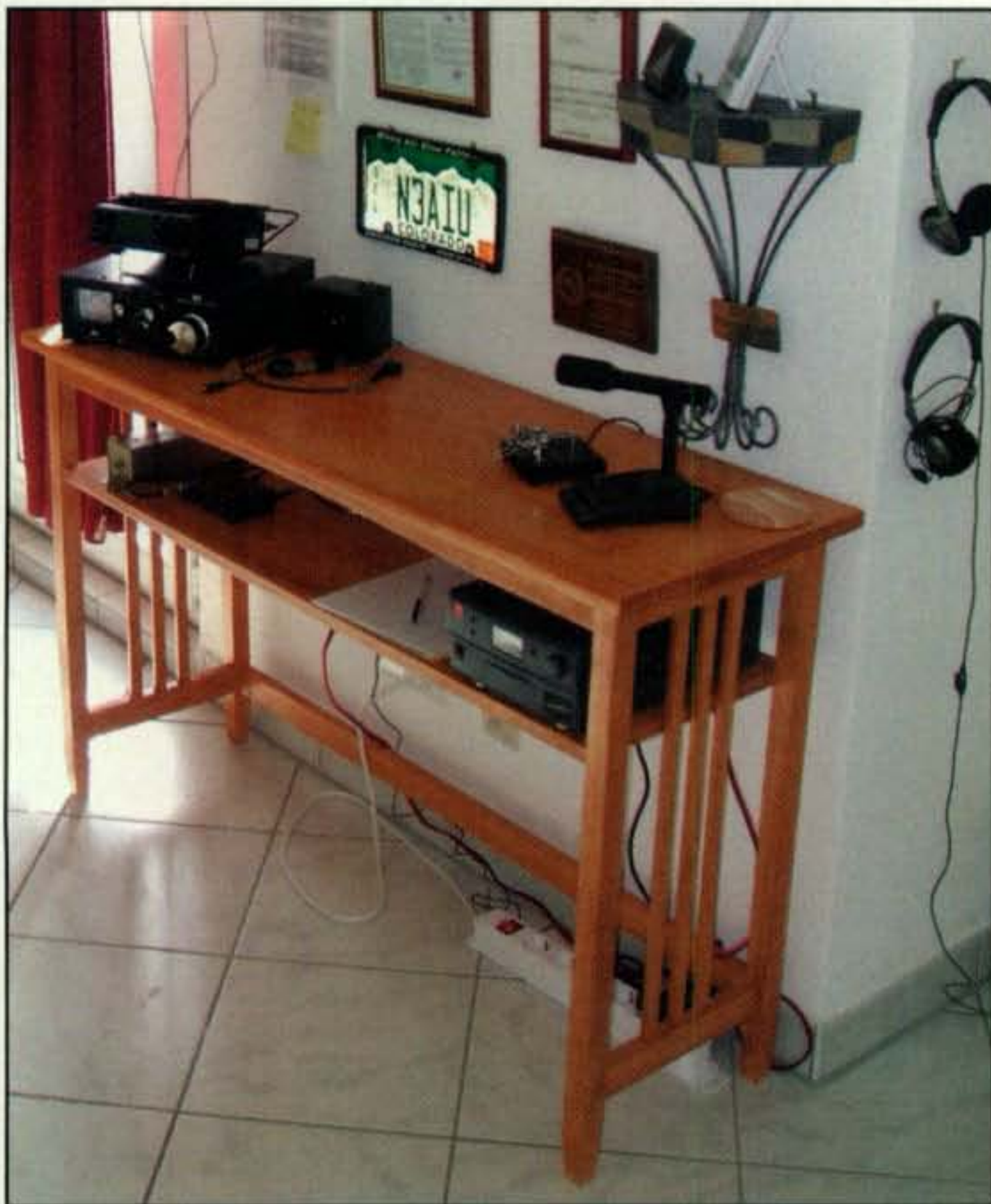
Photo B— My Amateurfunkstelle, or “amateur radio station,” in Gauangelloch. The transceiver and impedance matcher are on the left, station accessories are on the right, and the power supply is on the lower shelf.
