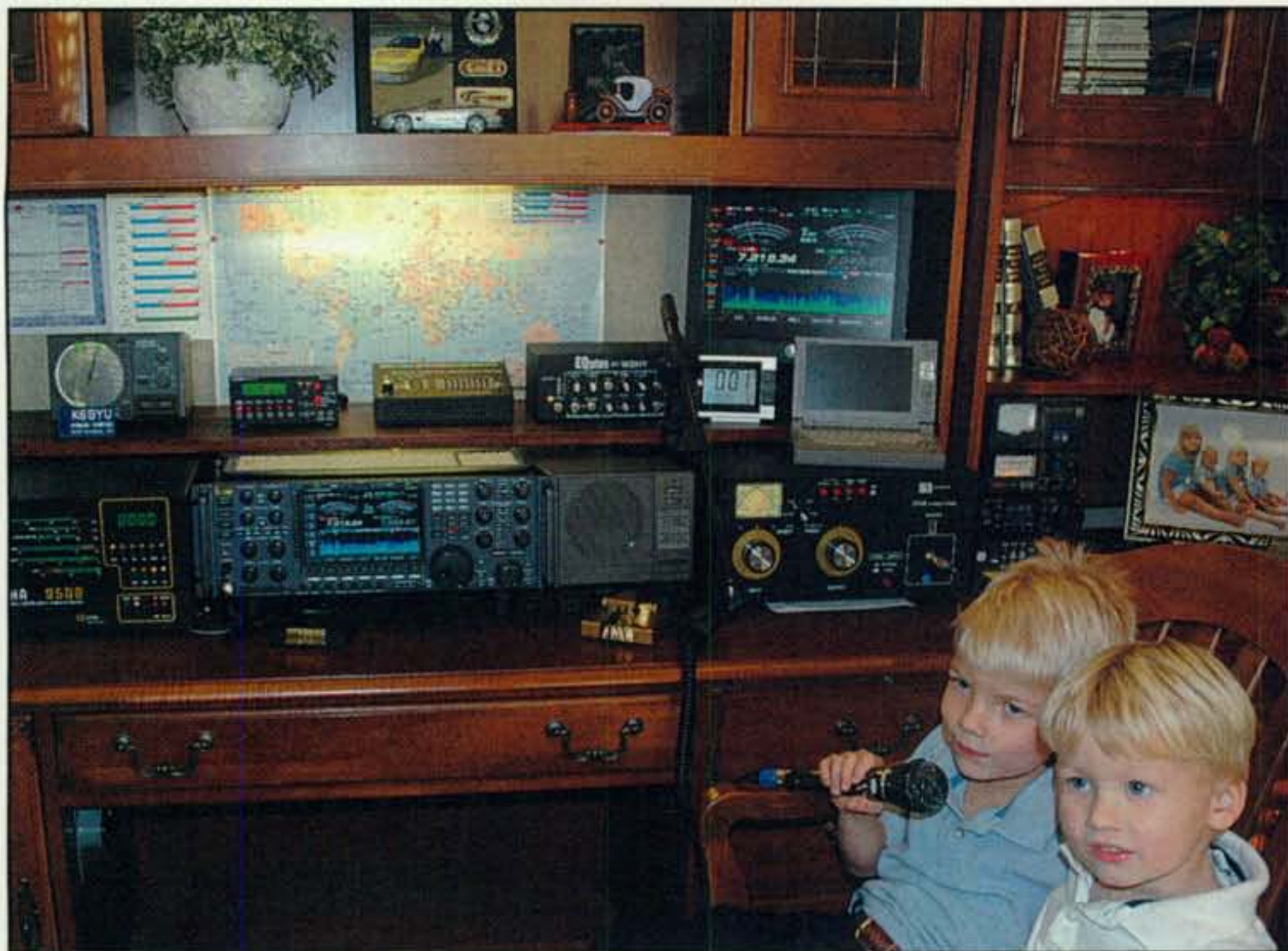
Photo G— Indoor station at K6BYU has it all: deluxe transceiver, high-power amplifier, tuner, remote controls, and junior ops.
