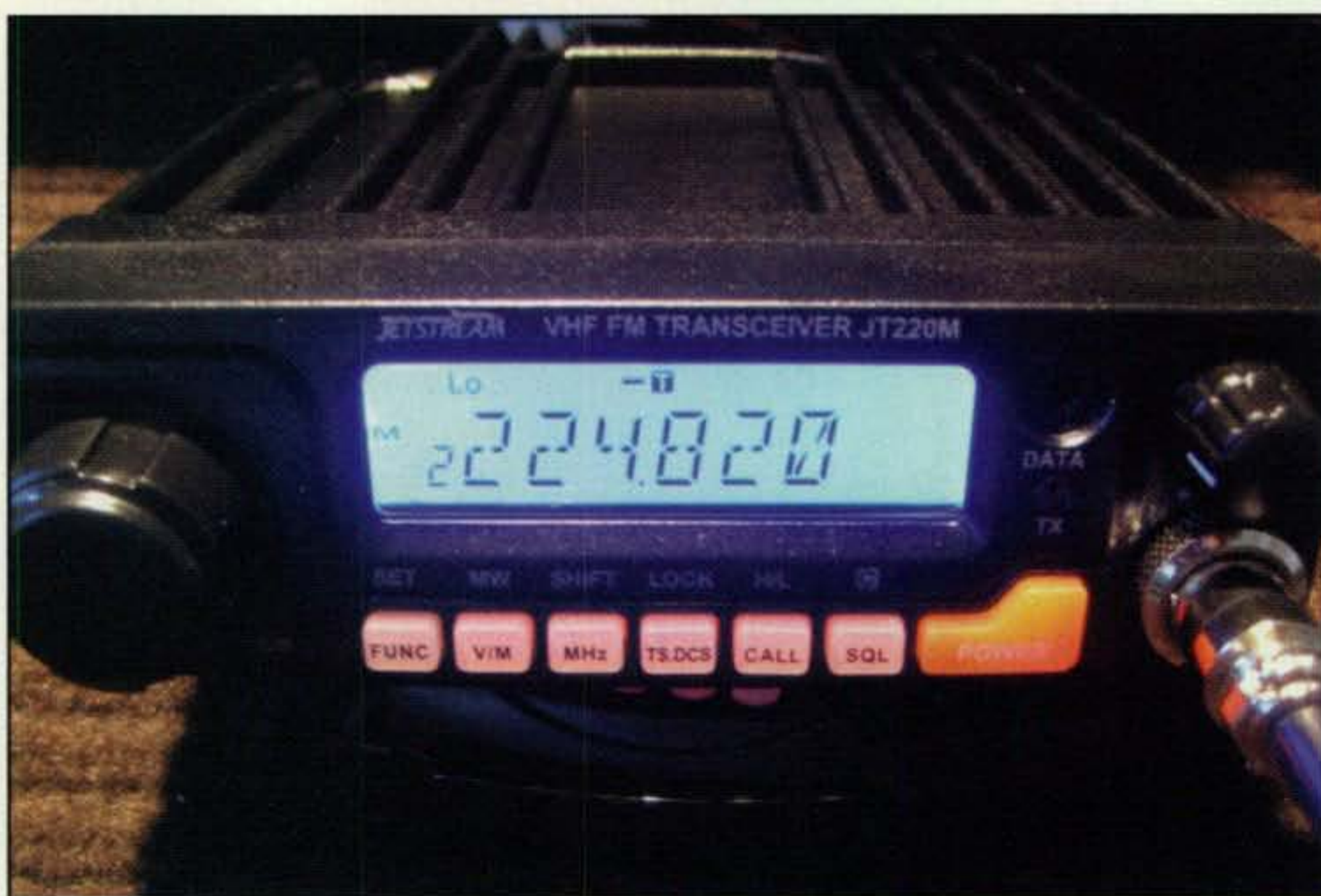
Jetstream's JT-220M 50-watt mobile rig for 222 MHz. The display is very bright, and this is at the low brilliance level!
