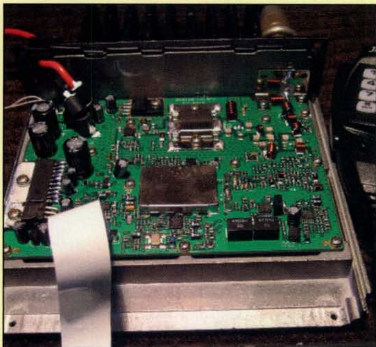
The front panel is connected to the rest of the radio by just one ribbon cable, suggesting possible remote applications in the future.
