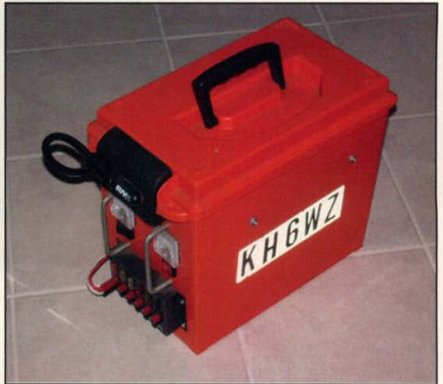
Photo D— My dedicated portable power box is a sportsman's dry box that I have modified for ham use, including a light for nighttime operating.
