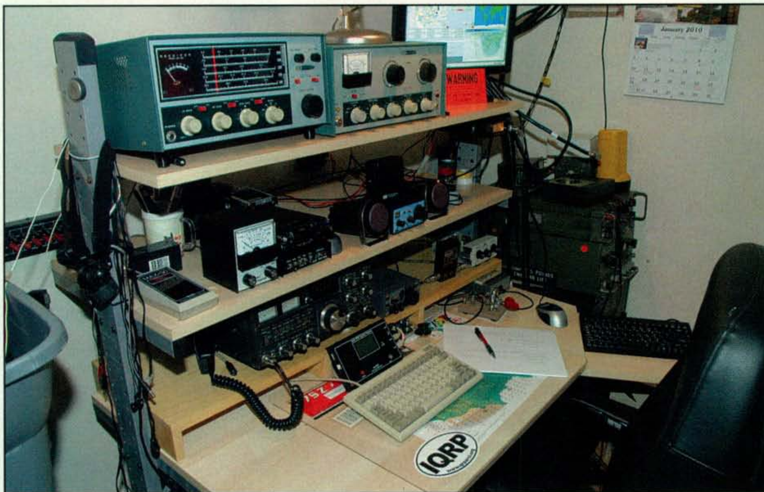
Photo A— Here is where it all happens at K7SZ. This is the IKEA desk that has served me well for over eight years. The "big stuff"—i.e., the boatanchors (Heathkit HR-10 RX/DX-60 TX)—is on the top shelf along with computer monitor. (A flat-screen monitor takes up much less room than the older CRT monitors, it runs cooler, and it does not put out tons of RFI!) The next two shelves hold QRP radios and the Yaesu FT-726 VHF/UHF multimode rig.
