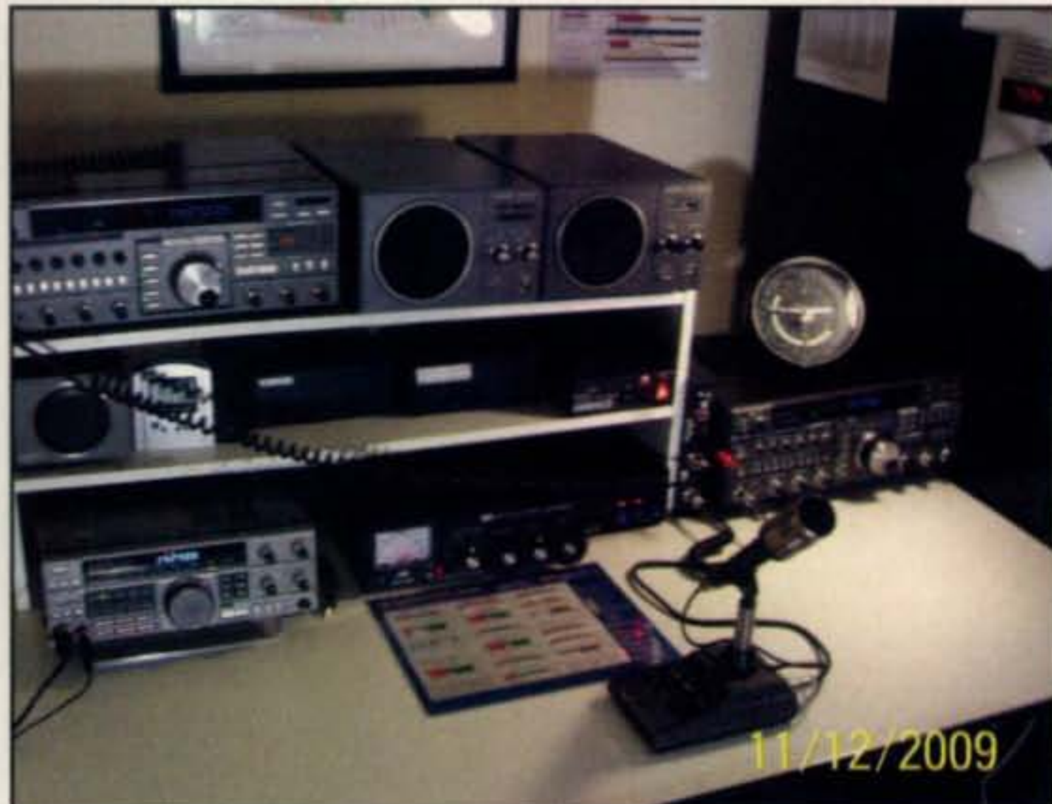
Photo D— Indoor station of KC0VFO includes Yaesu FT-736, TS-440, tuners, amps, speakers and more. Home is where the ham gear stays for sure! (Photo courtesy of KC0VFO)
