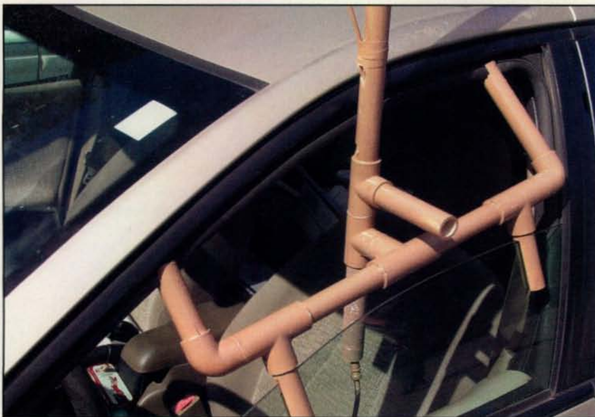
Bob Thornburg, WB6JPI, invented this simple removable window mount for rotating VHF RDF beams and produced some kits for it. That resulted in new T-hunters in the Los Angeles area. Contact him by e-mail (wolfbob@csnsys.com) to see if he has any kits left. (Photo by KØOV)
