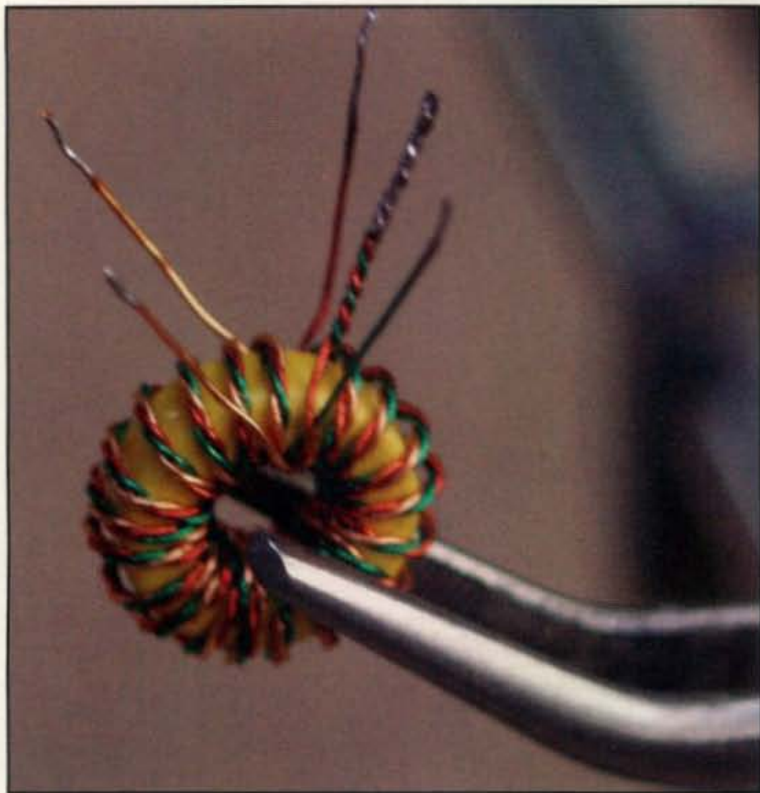
Photo D— Here is how T1 for the Gnat looks after being tri-filar wound with 20 turns for 80 meters. The secondary winding ends are to the left and the center-tapped primary windings are to the right.
