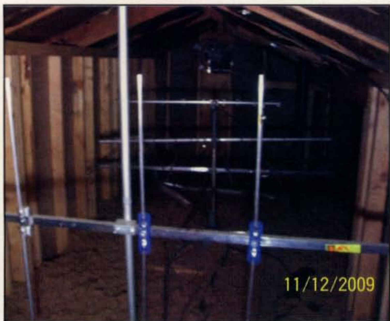
Photo C— A vertically polarized 2-meter beam as seen from another point in the attic. Terry definitely puts attic space to good use! (Photo courtesy of KC0VFO)
