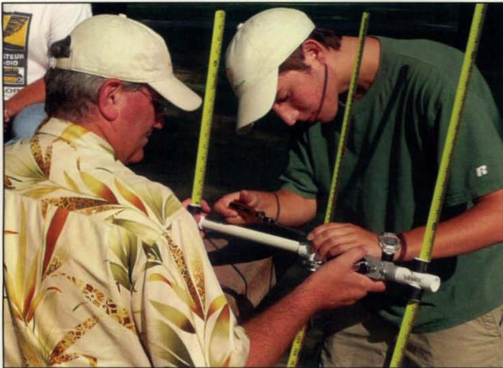
At a recent radio-orienting session in a southern California park, Max Praglin, KI6SYD (at right), built his own 3-element tape-measure Yagi for 2 meters, then went in the wilderness and found all five hidden transmitters. (Photo by April Moell, WA6OPS)
