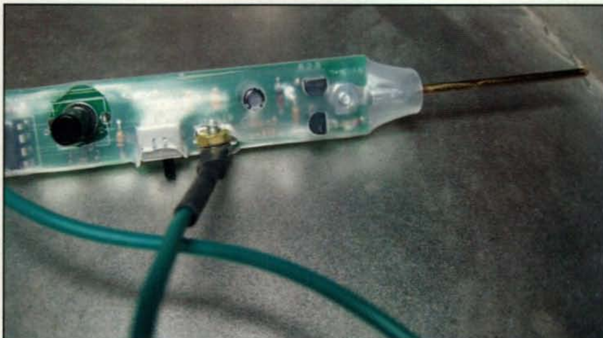
Photo C— Signal tracer/injector probe end showing volume control and inject/trace switch (next to wire).
