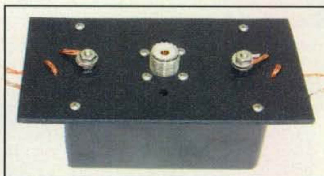
Photo C—MFJ has brought out some new match-making products which include the boom-mounted, 1:1 current, choke-style balun designed to match unbalanced feed lines (coax) to the balanced driven element. The balun is mounted in a molded case that uses an SO-239 for input and tinned copper wire leads for output.
