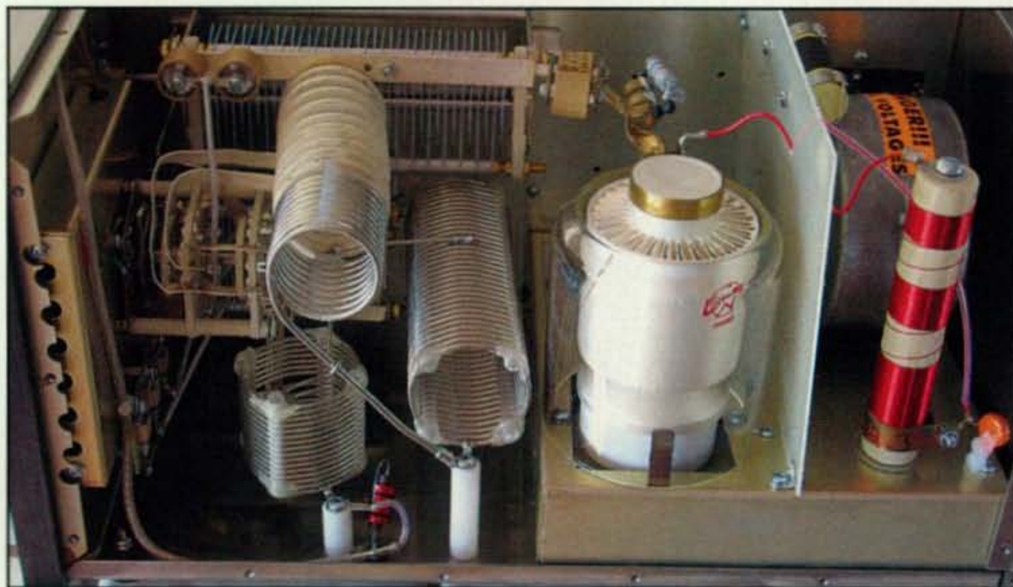
The AL-1200 tank compartment with the Eimac 3CX1200A7 tube and chimney installed. (Interior photos by the author)
