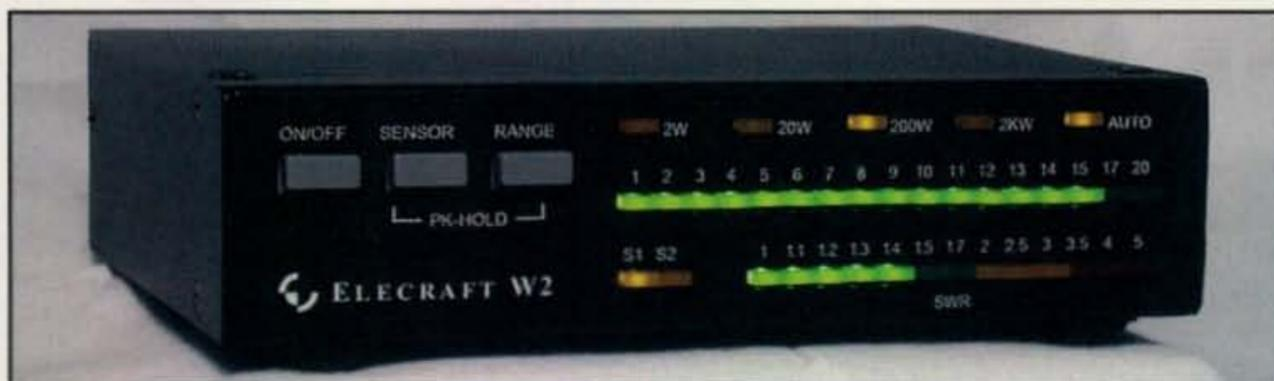
The Elecraft W2 wattmeter covers power up to 2000 watts and the HF-6 meter bands as well as 144–450 MHz. (Photo courtesy of Elecraft, Inc.)
