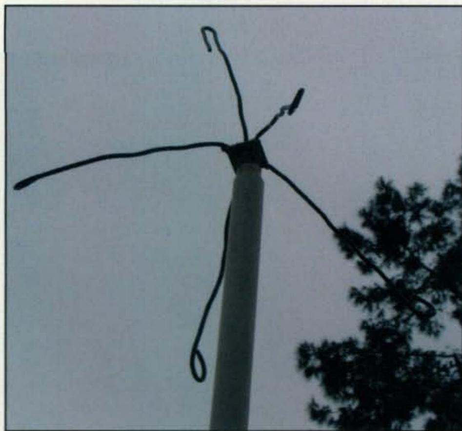
*Photo E— A squishy ground plane can be a very useful item in your emergency comms kit. Make one for each band on which you operate.*
