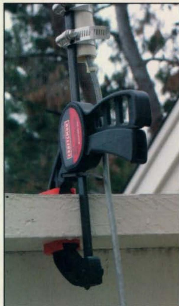
Photo F— The PVC-pipe mast is equipped with a woodworker's quick clamp for fast and easy mounting on just about any horizontal surface or edge.
