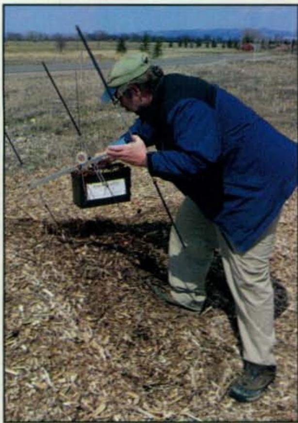
*It was yet another well-concealed transmitter for the Gallatin Ham Radio Club foxhunt in Bozeman, Montana in April 2009. Cyrus Smith, NU7Q, has just pulled the foxbox out of a pile of wood chips. The beautiful aluminum Yagi with flexible element tips was designed by Harley Leach, KI7XF. (Photo by AB5CK)*
