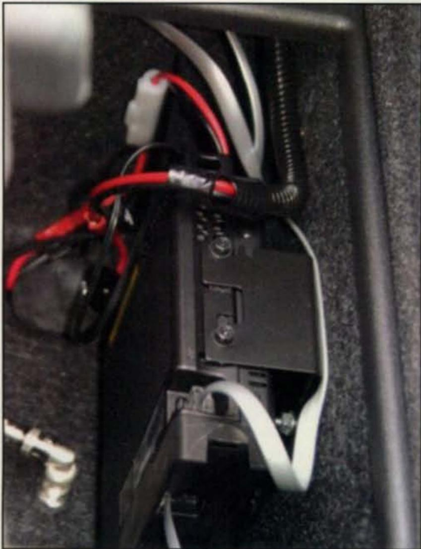
The Kenwood transceiver fits neatly into a rear hatch storage compartment. Note the antenna connection through the floor.
