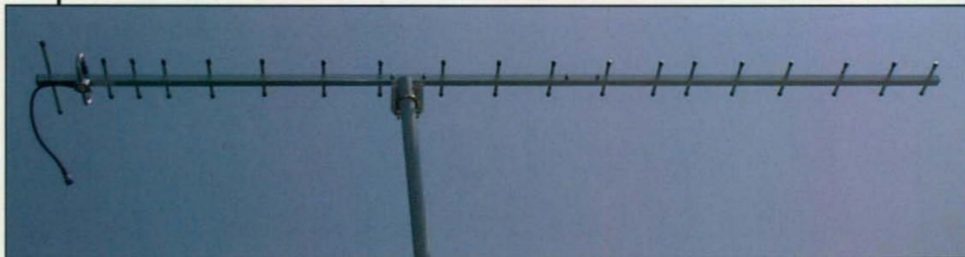
Photo C—A long Yagi with tightly tuned elements results in a narrow bandwidth. Bandwidth may be broadened, but at the cost of losing gain.
