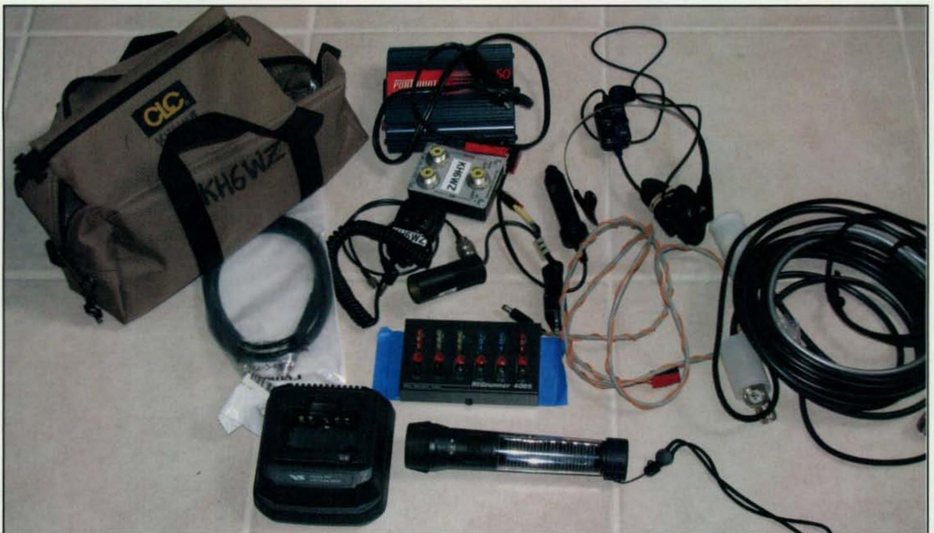
Photo C— An HT with some accessories can be turned into an effective emergency station for local contacts. The base stand charger at the lower left uses 12 VDC, a very useful feature.
