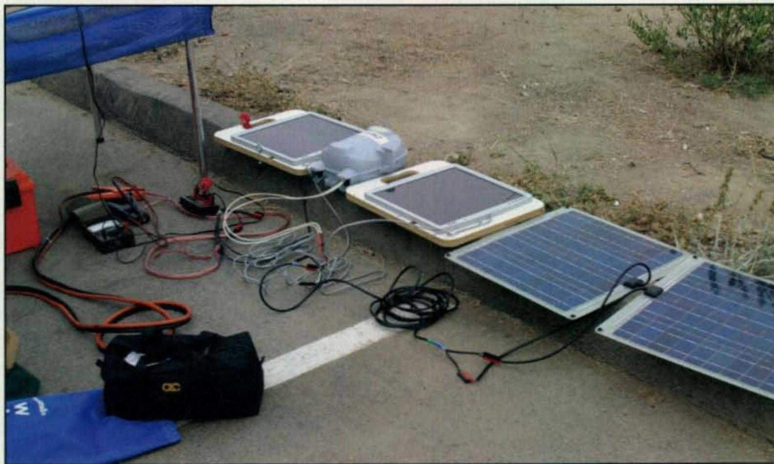
Photo A— Gel-cell batteries and solar chargers are among the most practical alternative power sources for your ham gear. Many have built-in charge controllers and nice housings for easy installation.
