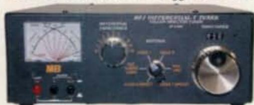
Two knob tuning (differential capacitor and AirCore™ roller inductor) makes tuning foolproof and easier than ever. Gives minimum SWR at only one setting. Handles 3 KW PEP SSB amplifier input power (1.5 KW output). Gear-driven turns counter, lighted peak/average Cross-Needle SWR/Wattmeter, antenna switch, balun. 1.8 to 30 MHz. 10 1/4"Wx4 1/2"Hx15 in.
