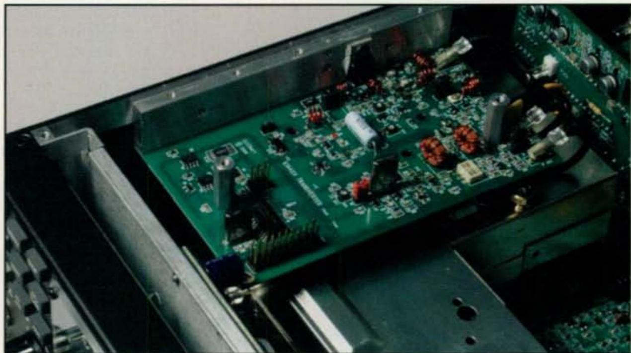
*Elecraft's new K144XV internal 2-meter module installed in the K3. The module cover is removed for illustration purposes. (Photo courtesy of Elecraft, Inc.)*
