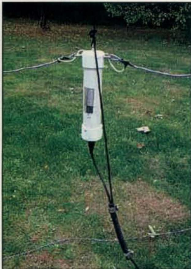
This picture shows a 1:1 balun attached at the feedpoint of a dipole antenna. These baluns can be purchased or made at reasonable cost.
