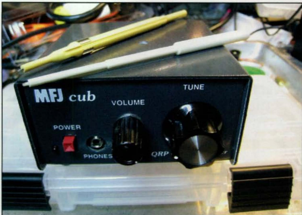
Photo D— Completed kit in case with the required tuning tools on the top.
