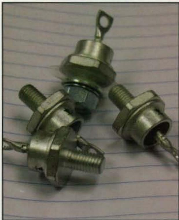
Photo C— Stud-mount rectifiers work great for these protector circuits and have hefty ratings.
