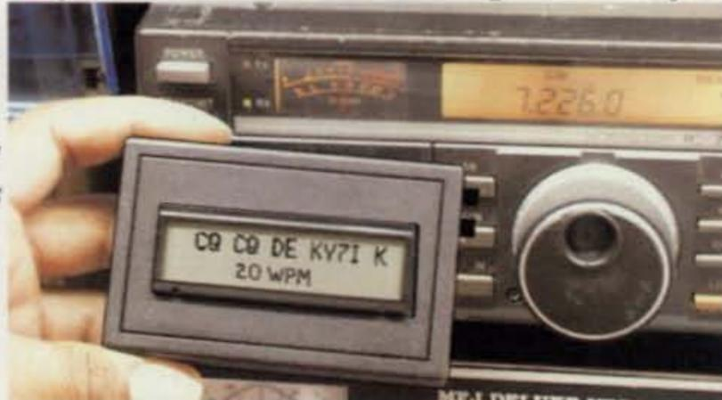
your receiver speaker until the lock LED flashes in time with the CW. Digs out weak signals. Phase-Lock-Loop even tracks slightly drifting signals.
