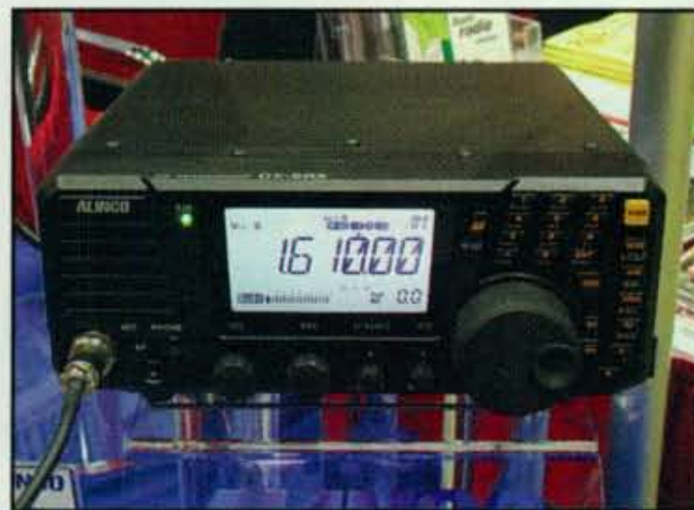
Alinco's first new HF entry in several years is the 160- to 10-meter DX-SR8. It includes a general-coverage receiver that tunes down to 135 kHz.
