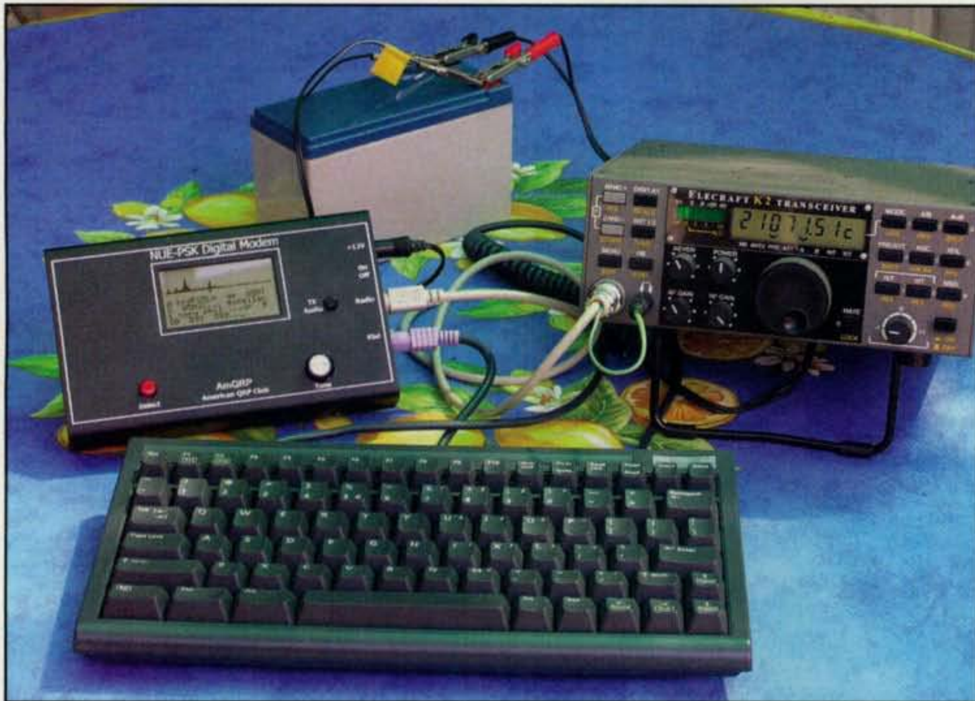
Photo F— The PSK-NUE digital modem set up with keyboard, K2, and battery makes a compact, portable digital station.
