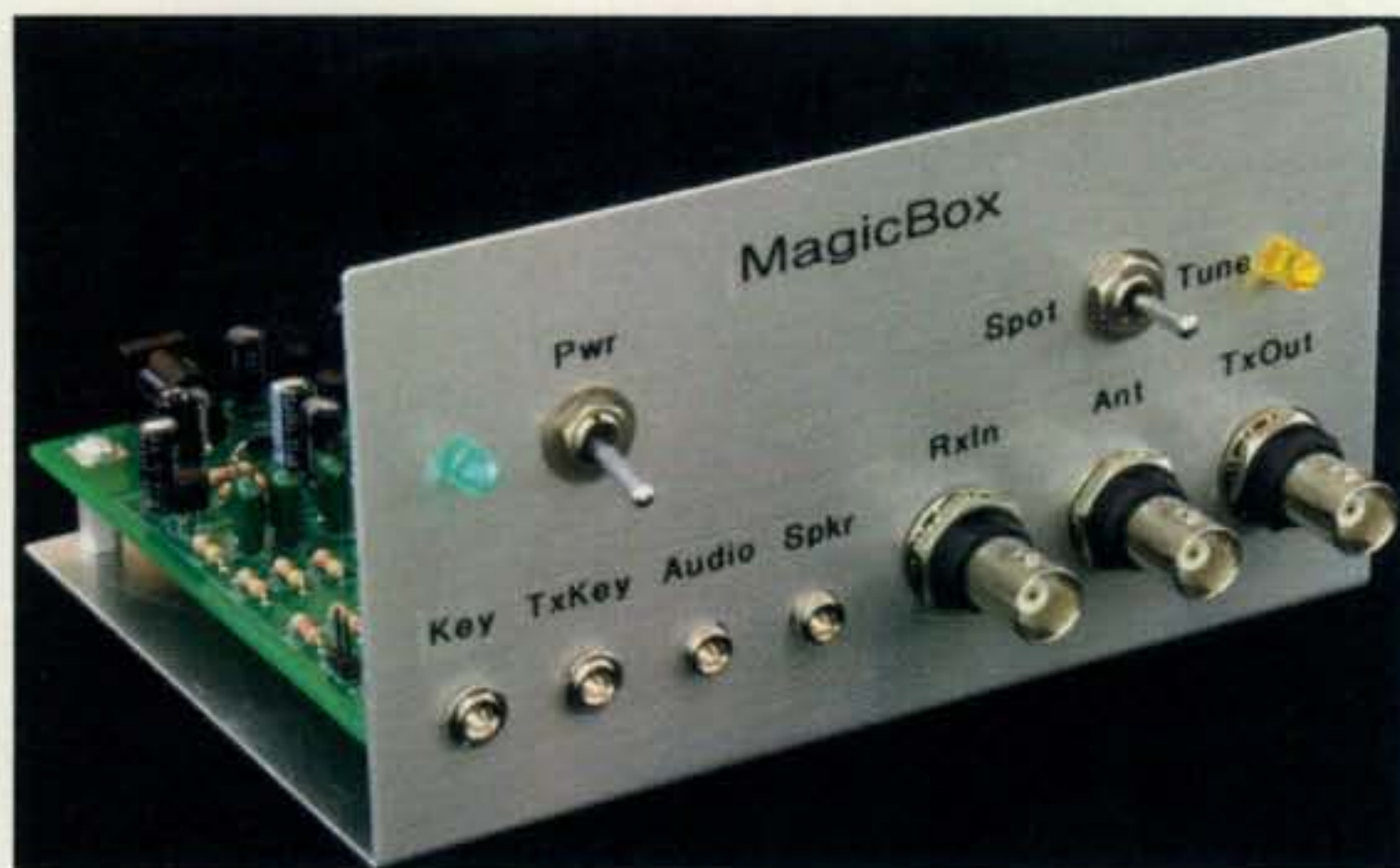
Photo D— Jim Kortge, K8IQY's Magic Box will do the heavy lifting when you need to interface a separate transmitter and receiver.
