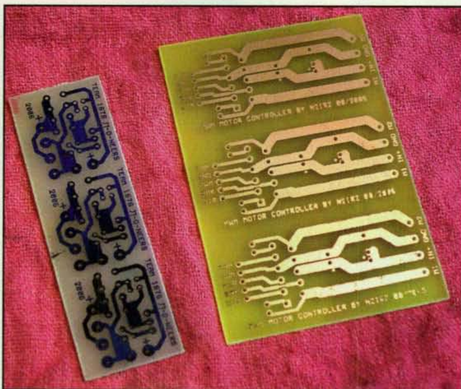
Photo E— Some printed circuit boards that I drilled with my CNC machine. Despite having only a few dozen holes, it's still faster and more precise to let the machine do it.
