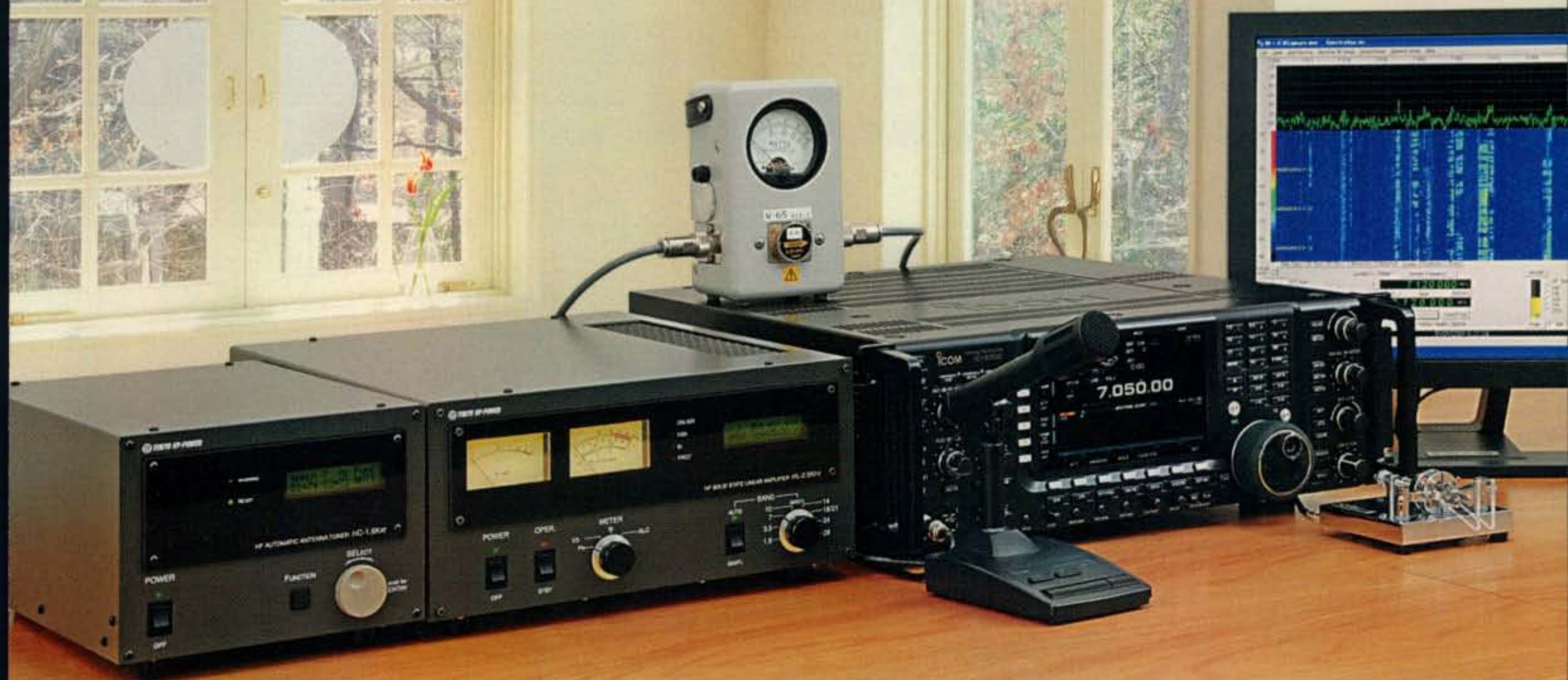
Photo : From left HC-1.5KAT (HF 1.5kW Tuner with Auto Band Set Feature), HL-2.5KFX (HF 1.5kW MOSFET Linear) and IC-7700 Transceiver
