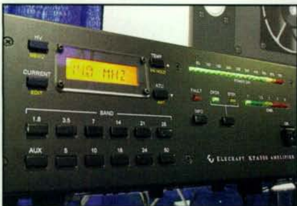
Elecraft has entered the standalone amplifier market with its 1.8–54 MHz solid-state KPA-500 that, logically, puts out 500 watts.
