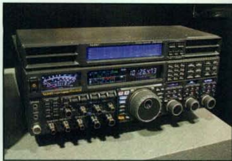
The Yaesu FT DX 5000 comes in three different models and is built for the serious ham. It covers HF plus 6 meters.
