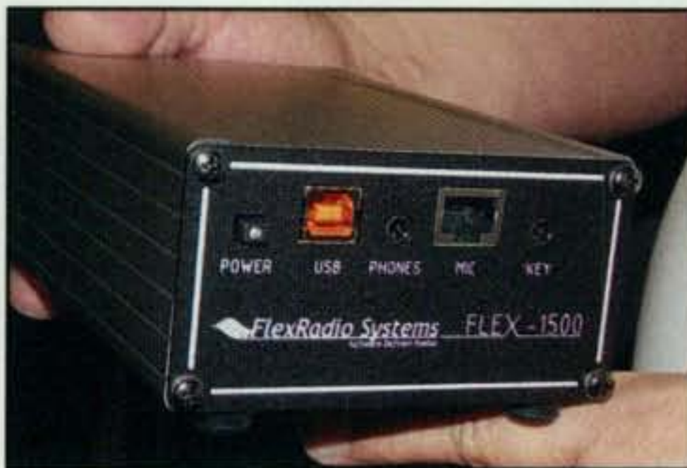
The new Flex-1500 from FlexRadio is a QRP SDR, or low-power software-defined radio. It puts out 5 watts on the HF ham bands plus 6 meters.
