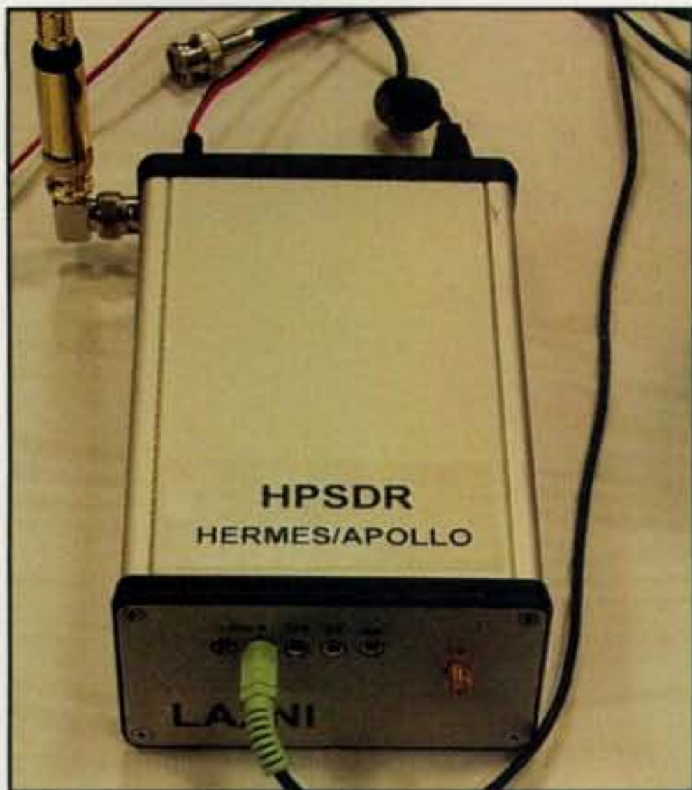
TAPR's Hermes transceiver is a 'high-performance software-defined radio' (HPSDR) putting out 15 watts on 160–20 meters.
