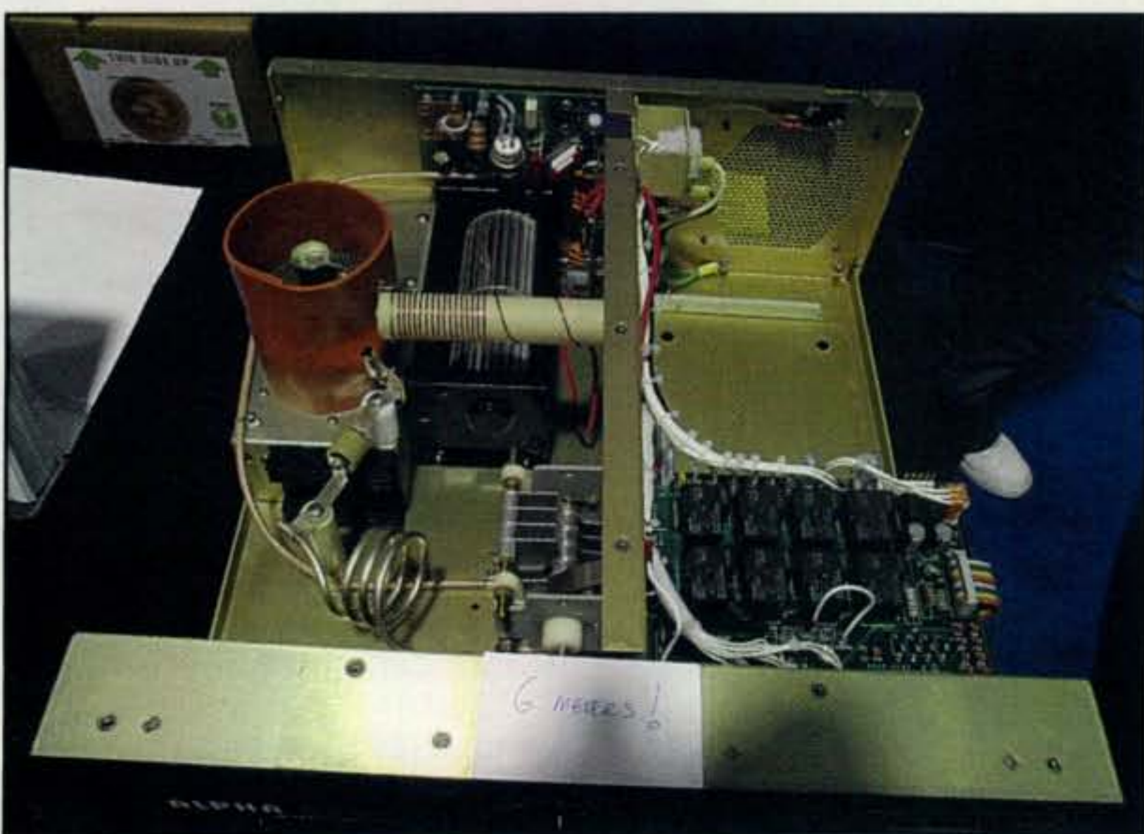
The Alpha 8406 is a 6-meter-only amplifier, generating up to 1500 watts of output.
