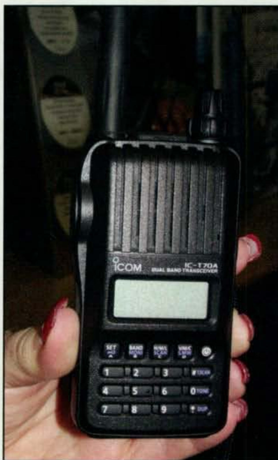
The IC-T70A is one of two new HTs introduced by ICOM. It covers 144 and 440 MHz, while the IC-V80A is a single-band rig for 2 meters.
