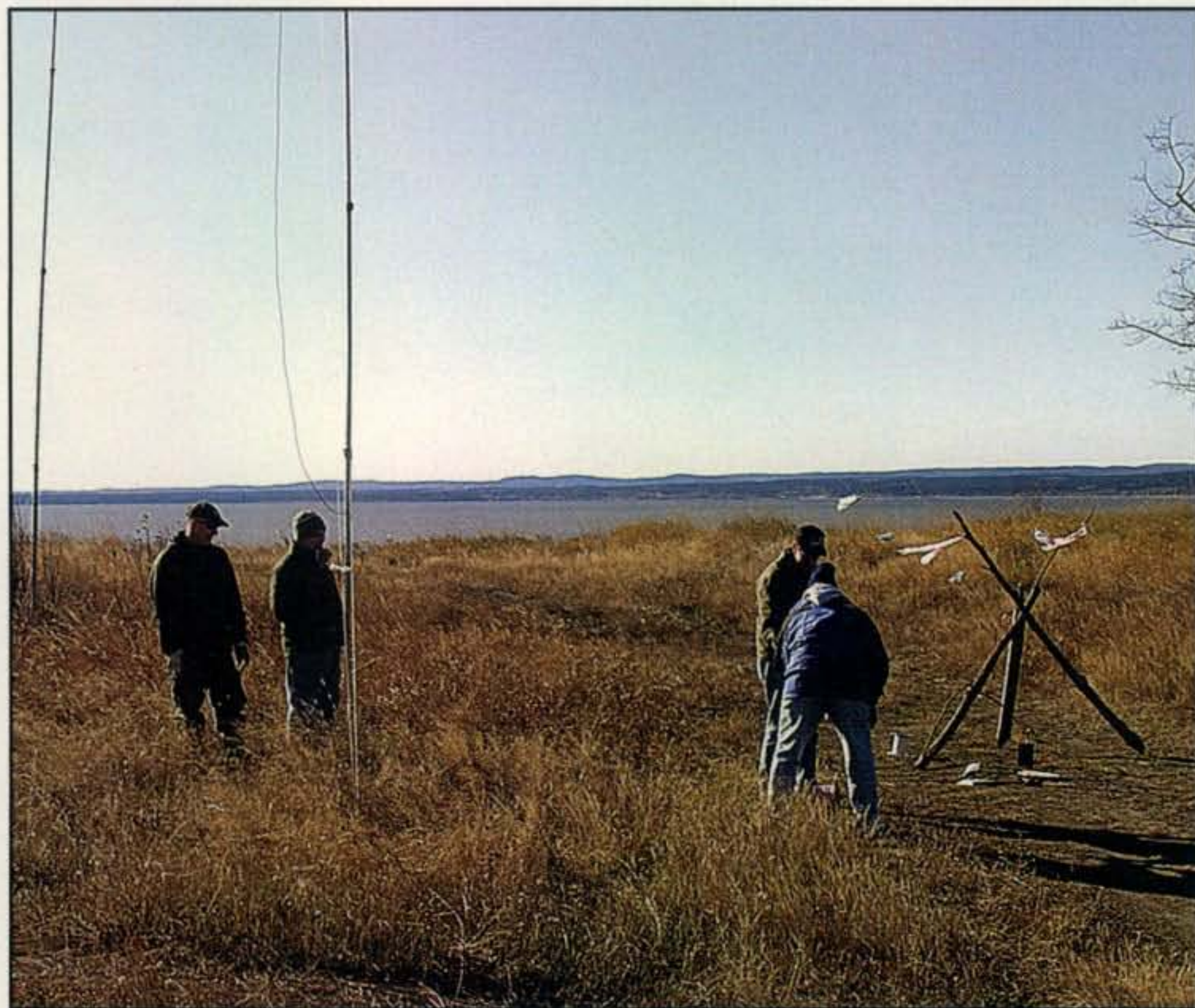
The VE2DXY antenna farm overlooking the north shore of the St. Lawrence River. The river, which is tidal at this point, contains enough salt water as a ground plane to provide an excellent path over water to the US and the Caribbean.
