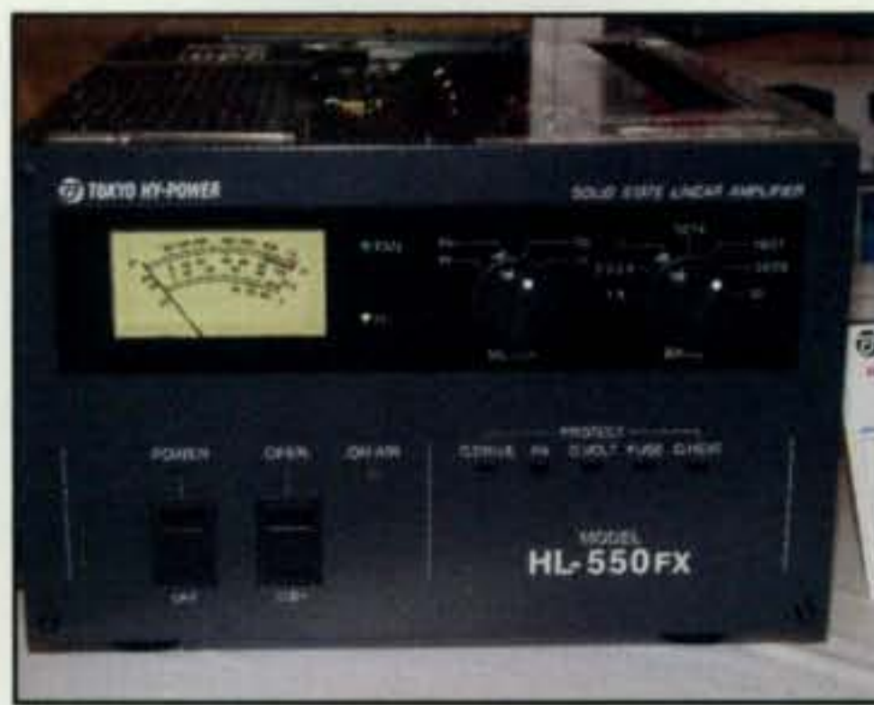
Tokyo Hy-Power's HL-550FX puts out 600 watts on 160–6 meters and weighs only about 20 pounds.
