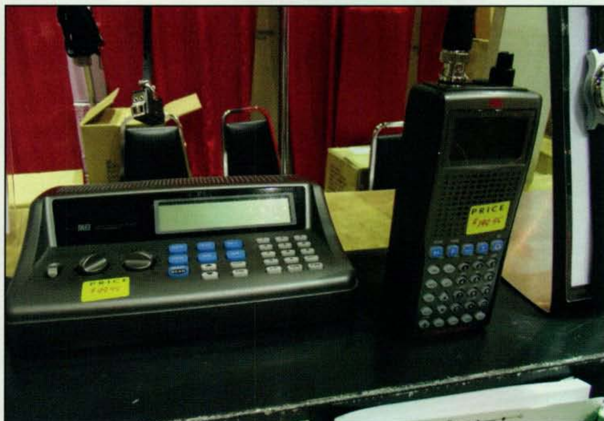
MFJ has entered the scanner market with two models, the MFJ-8310 desk scanner and the MFJ-8322 handheld analog trunking scanner.
