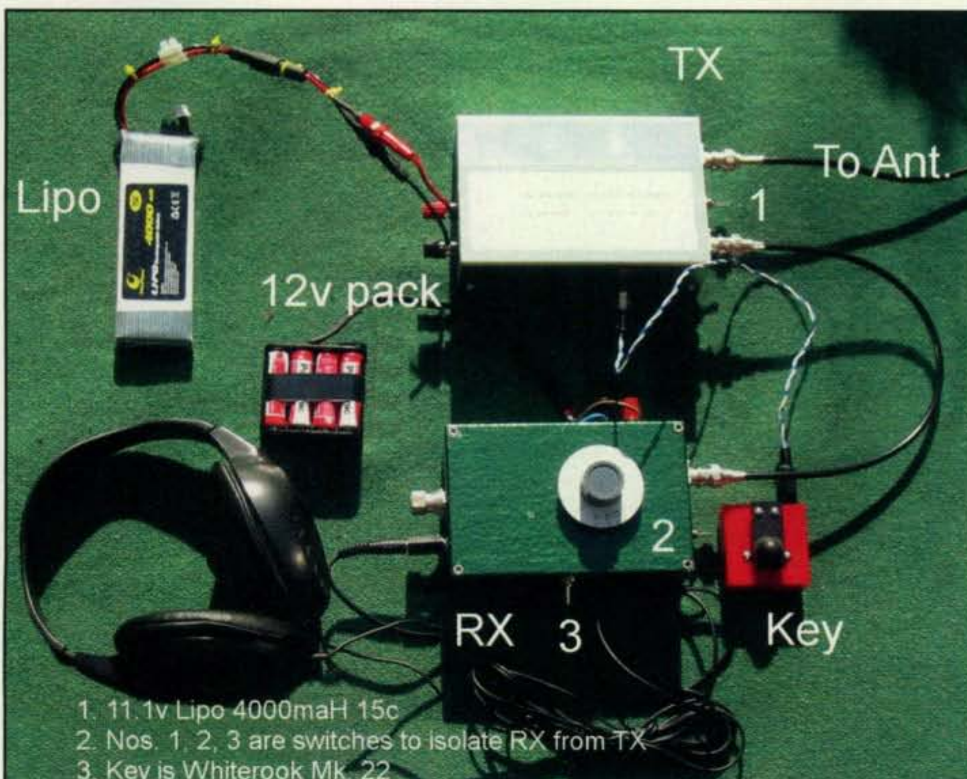
Photo B— Ian Maxwell, MMØMXW's portable setup, which he uses for hilltopping. See the text for a description of all the parts.
