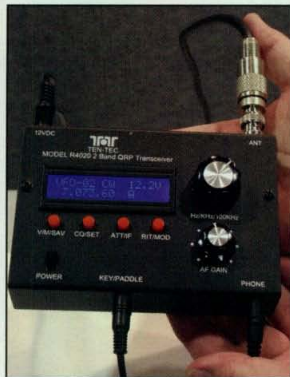
Also in the QRP category is a pair of new dual-band transceivers from Ten-Tec. The 4020 (pictured) covers 40 and 20 meters; the 4030 covers 40 and 30!
