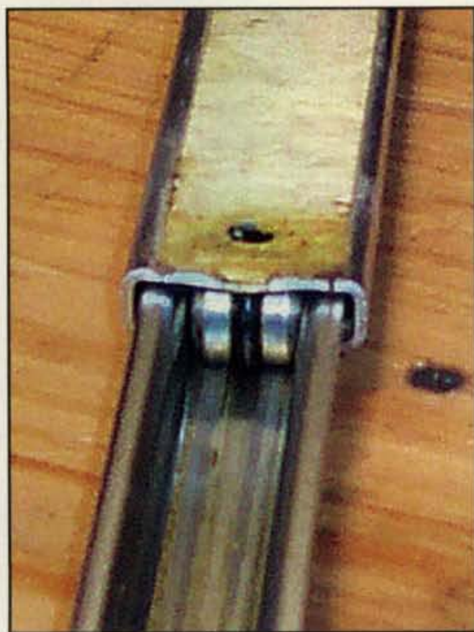
Photo C— A special drawer slide which uses a roller with a rubber O-ring to eliminate any play or wiggle in the system. This type is used for relatively light loads. Even the slightest amount of play in the rail will harm the machine's accuracy.
