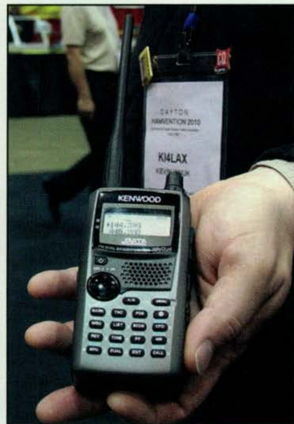
Kenwood's newest handheld for 2 meters and 70 centimeters includes a built-in TNC and APRS software as well as an integrated GPS receiver for sending out your exact location on APRS.
