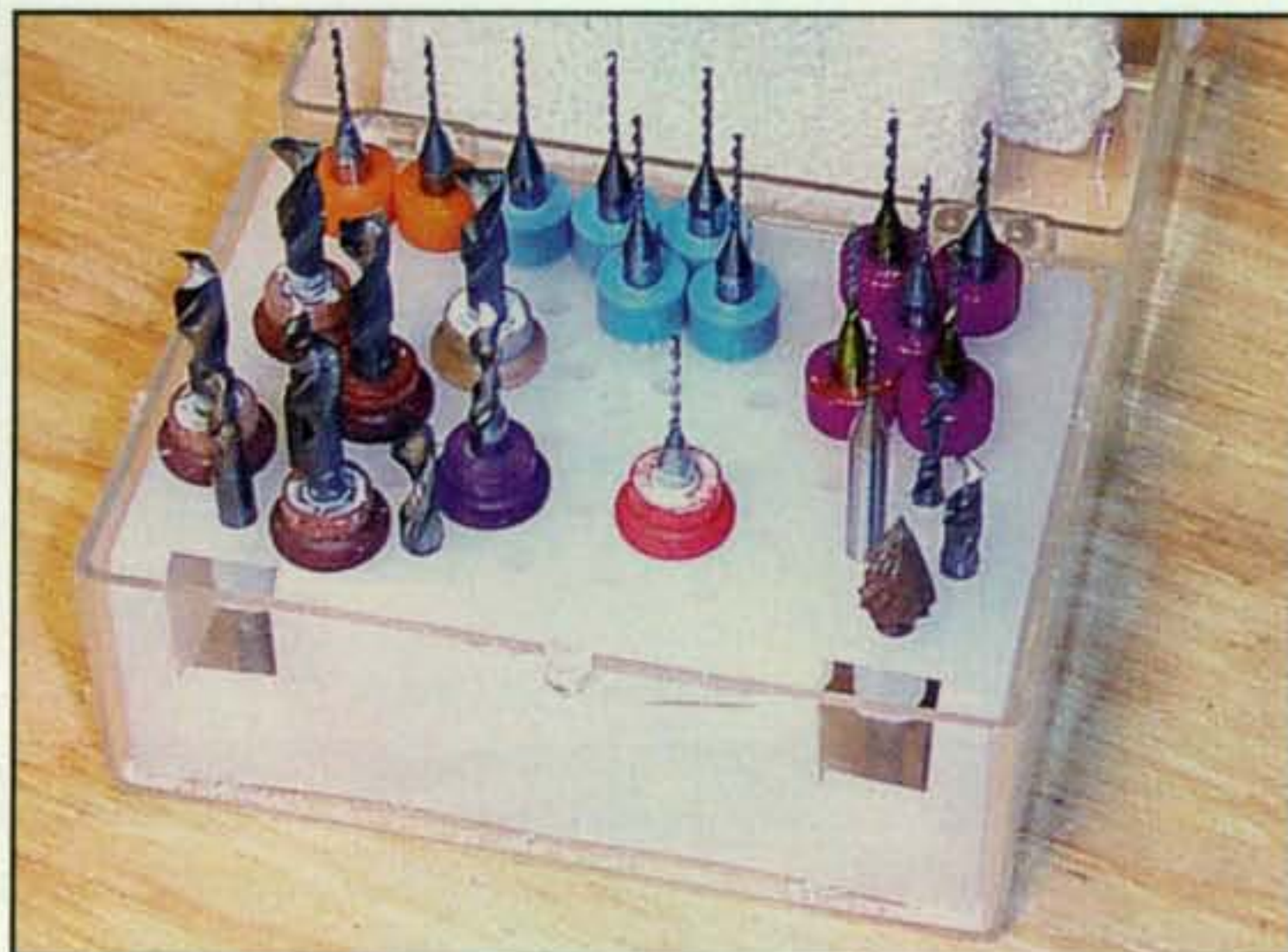
Photo D— An assortment of carbide PC-board drills. Carbide is very hard, allowing thousands of holes to be drilled in highly-abrasive glass-epoxy PC boards, but it is also very brittle, breaking easily if used in a manual drill press
