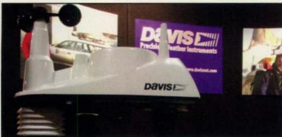
The Vantage Vue weather station from Davis Instruments is wireless and solar-powered.
