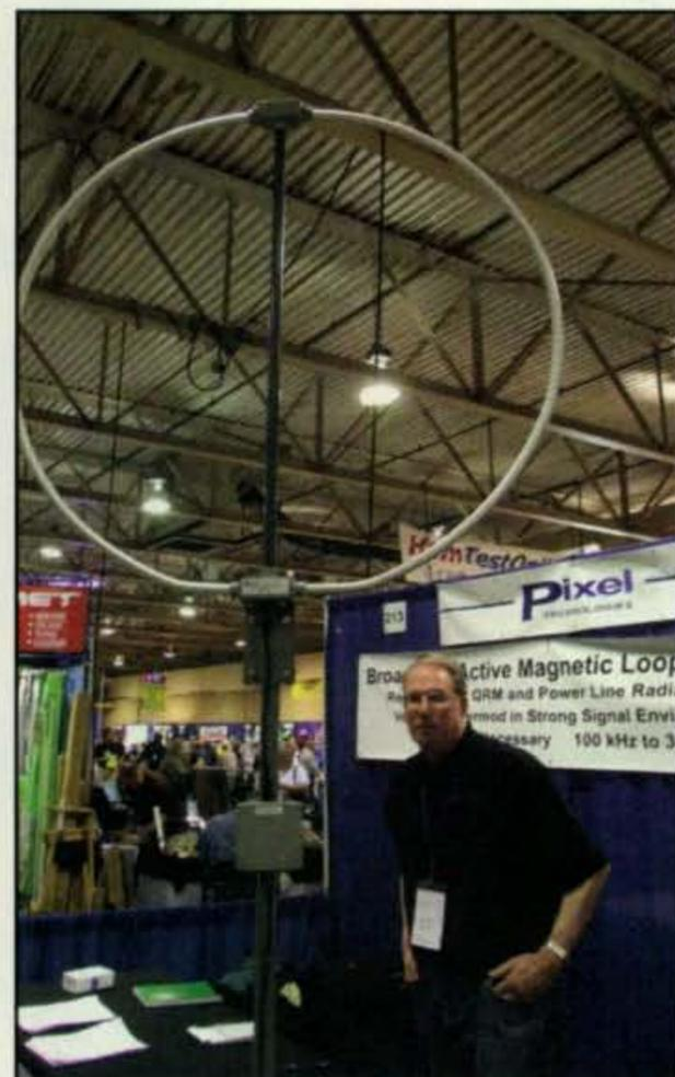
The RF-Pro 1 loop antenna from Pixel Technologies reportedly covers 100 Hz to 30 MHz.
