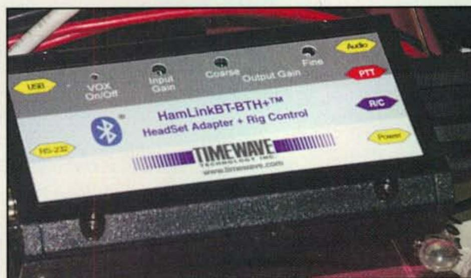
TimeWave Technology's Ham Link BT-BTH interfaces a laptop computer with a USB port to a ham transceiver through the MIC jack, allowing control of many radios via Bluetooth.
