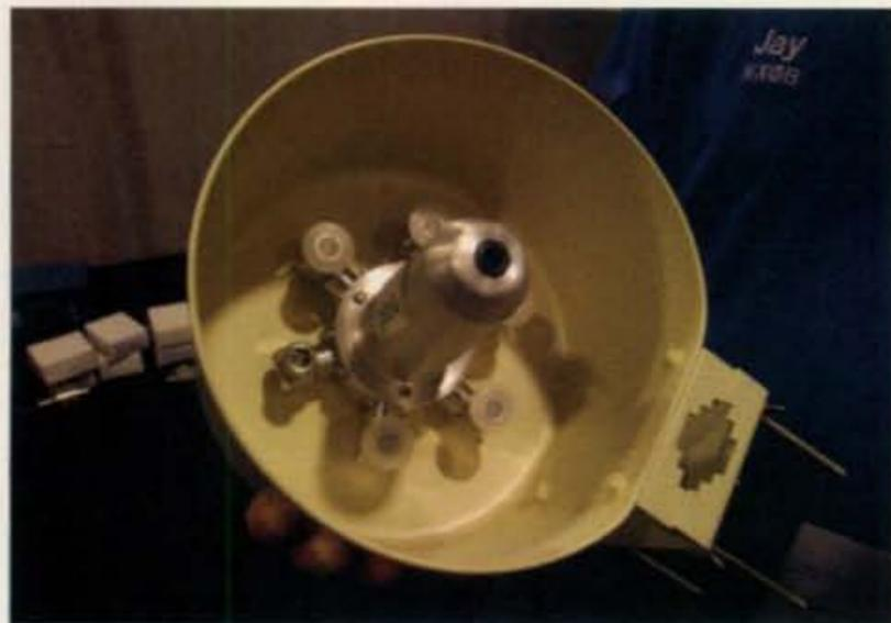
Array Solutions also represented Germany's Hofi-Technik company at the show, bringing several products, including the motorized antenna switch seen here.
