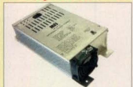
75 Amps continuous. Adjustable 13.8-14.2 VDC output. Reverse polarity, over-current/temperature, brown-out input protection, 7.8 lbs. 6 1/2"Wx3 1/2"Hx10D in. 108-132 VAC. Great for Ameritron's ALS-500M mobile amplifier!
