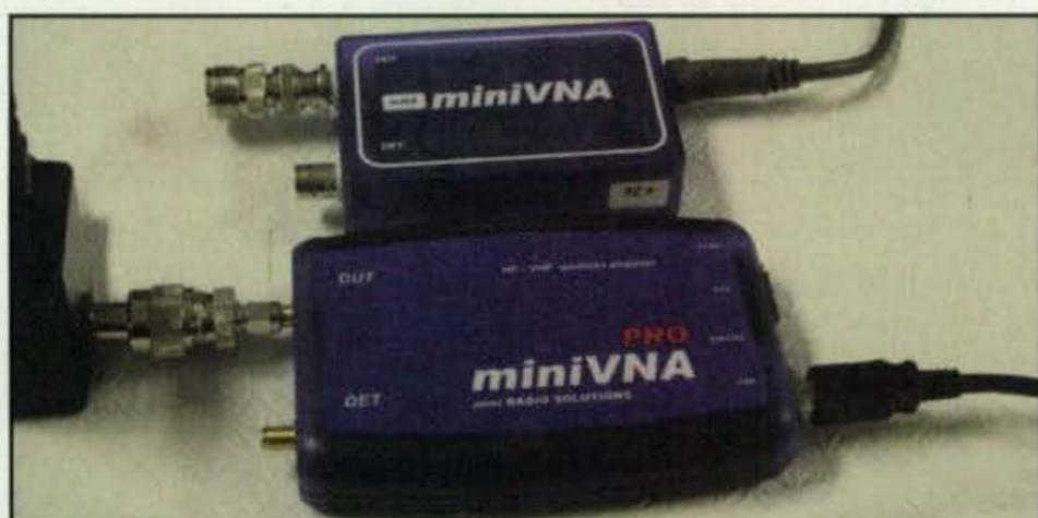
The MiniVNA and MiniVNA Pro antenna analyzers from W4RT Electronics.
