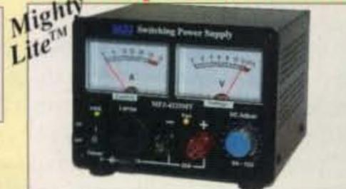
22 Amps continuous, 25 Amps maximum. Like MFJ-4125 but adds Volt/Amp meters, cigarette lighter plug. Adjustable 9-15 VDC Output. 5 1/4"Wx 4 1/2"Hx6D in. Weighs 3.7 lbs. Use 85-135 VAC or 170-260 VAC input. Replaceable fuse.
