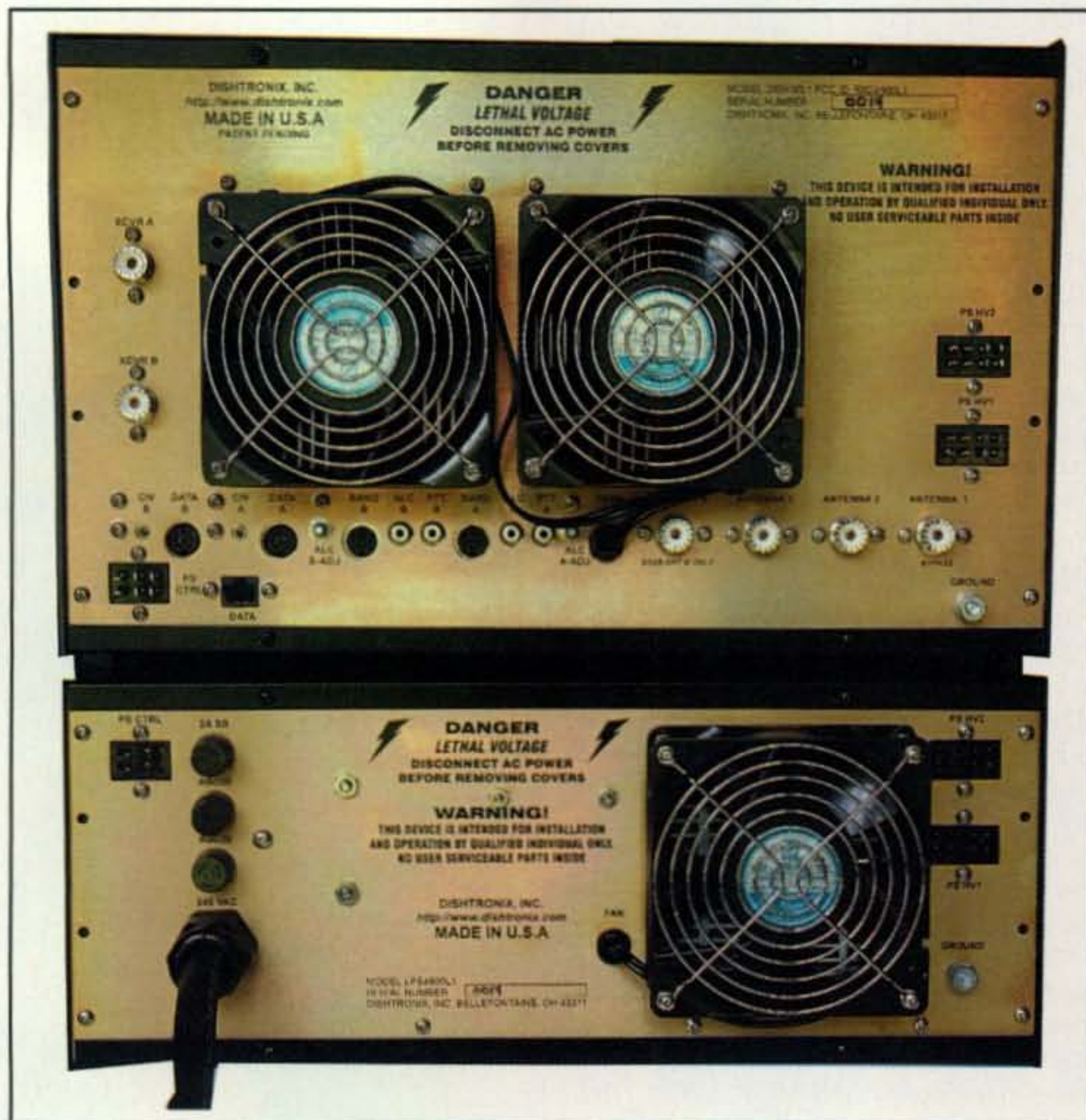
Rear view of the DX-2400. Note the inputs and RF and computer control from two transceivers, and outputs for four antennas. A four-position antenna switch is built in.
