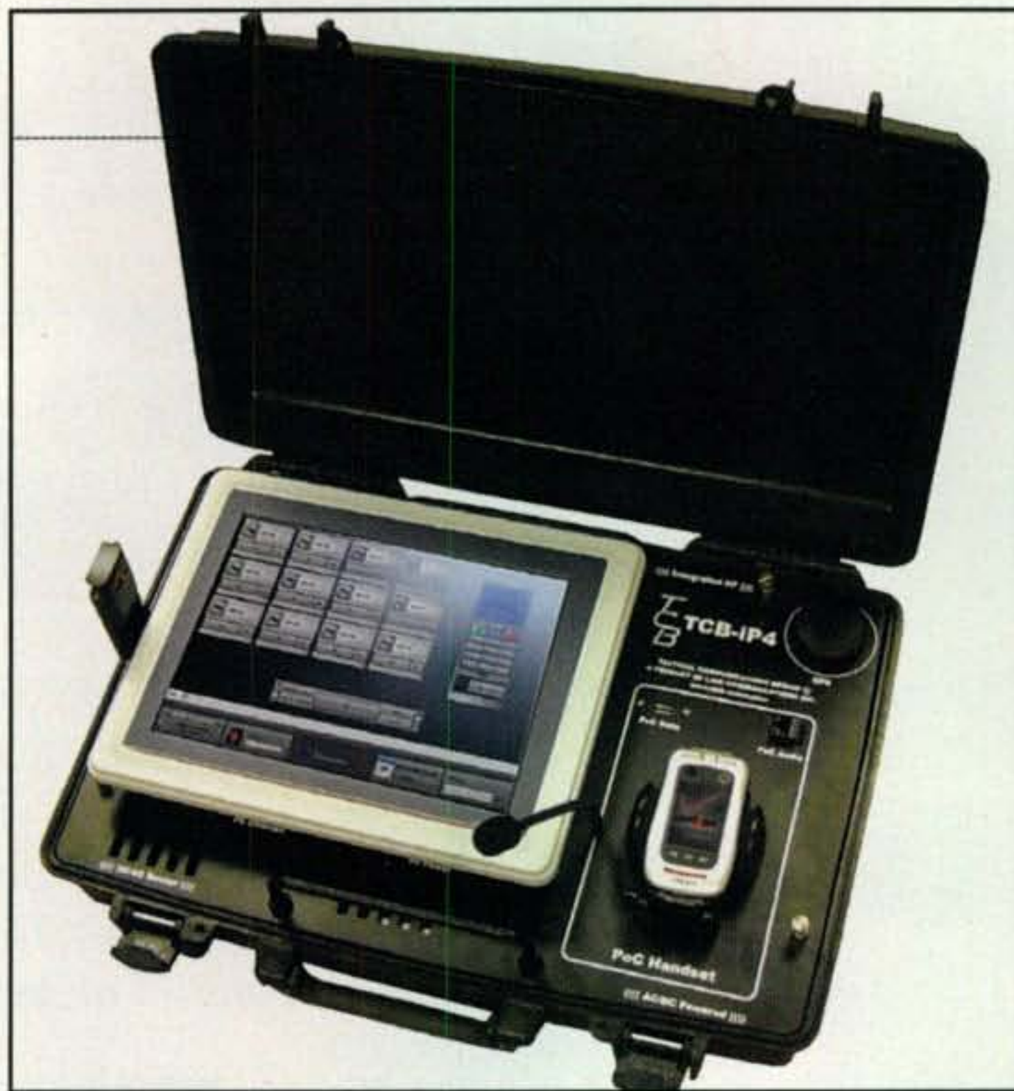
Photo D— Expected to be seen soon at your next disaster drill or actual community emergency is the TCB-iP4 computer controllable, four-port, radio interoperability system which has built-in 5-watt VHF, UHF, and 800-MHz secure APCO P-25 radios.
