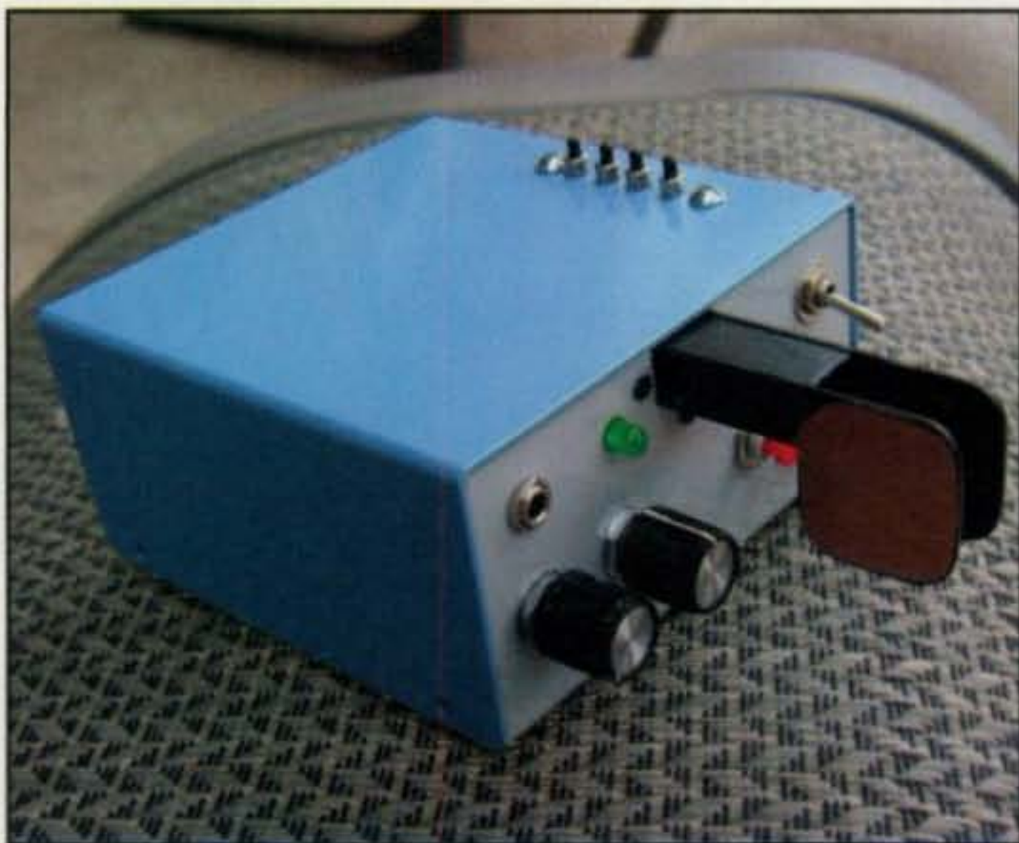
Photo A— Bill Prats, K6ACJ, sent along this photo of a nifty little accessory box he made as a companion to his older 706 and some simple QRP rigs. It contains a set of touch paddles, a NESCAF filter, and a K1EL K10 keyer, as well as all the batteries.
