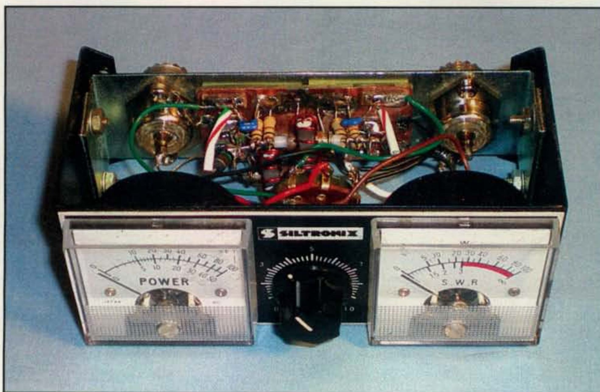
Photo D— This is Charlie Lofgren, W6JJZ's SWR meter after transplantation of his homebrew Manhattan-style Stockton Bridge.
