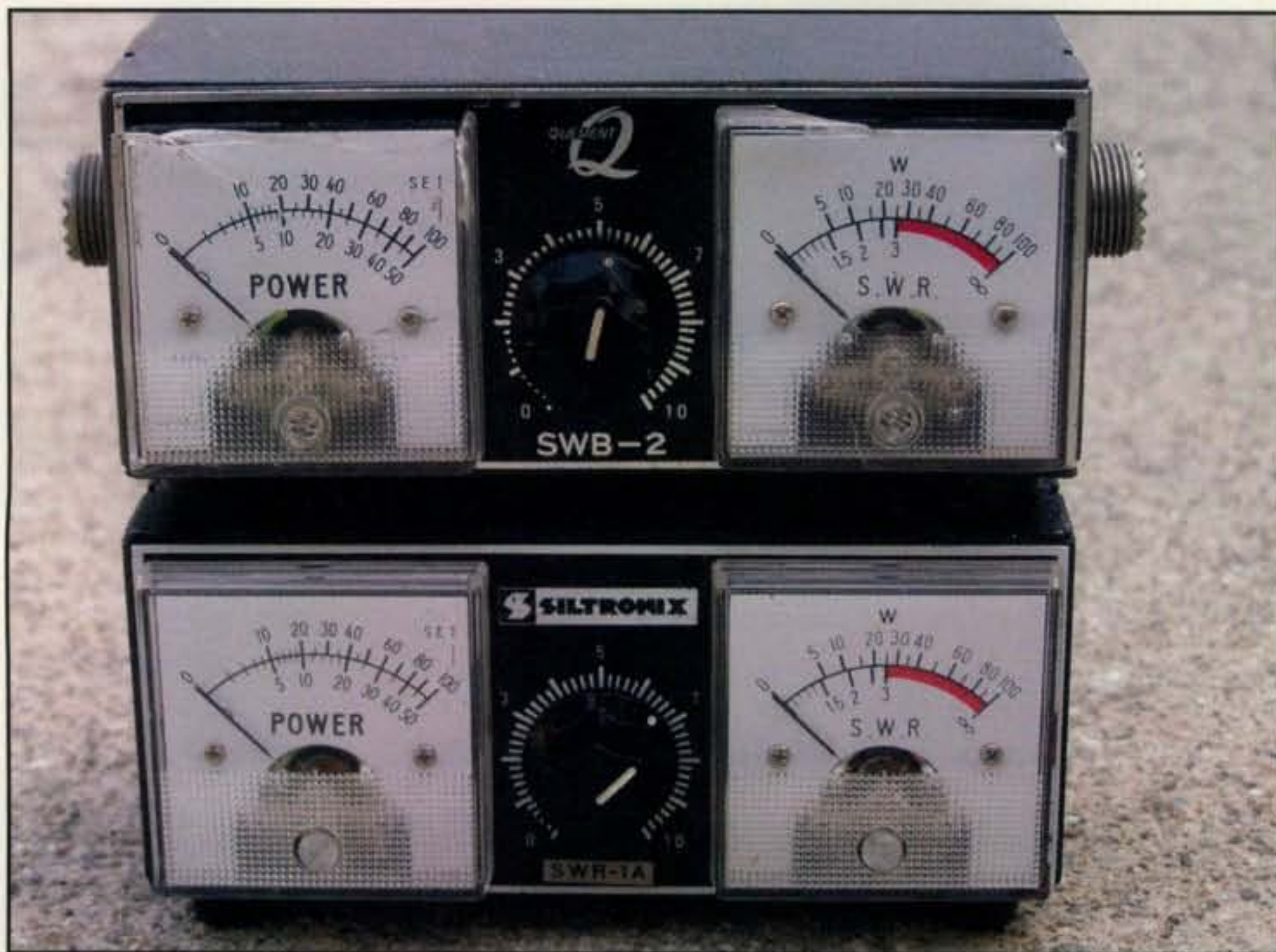
Photo C— Two versions of the same SWR bridge. The top one appears to have had a harder life than the bottom one, but it cleaned up nicely and works well after a little surgery.
