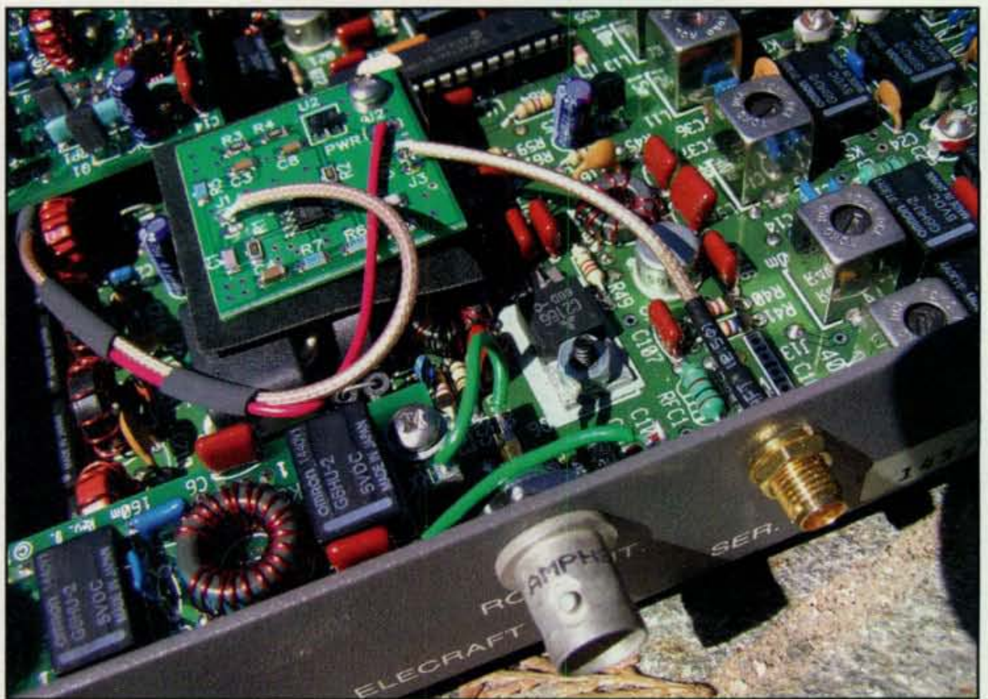
Photo F— The author's K2 with Clifton Laboratory's buffer amp installed. The board is mounted on a threaded standoff which replaced a very conveniently located screw on the main circuit board.
