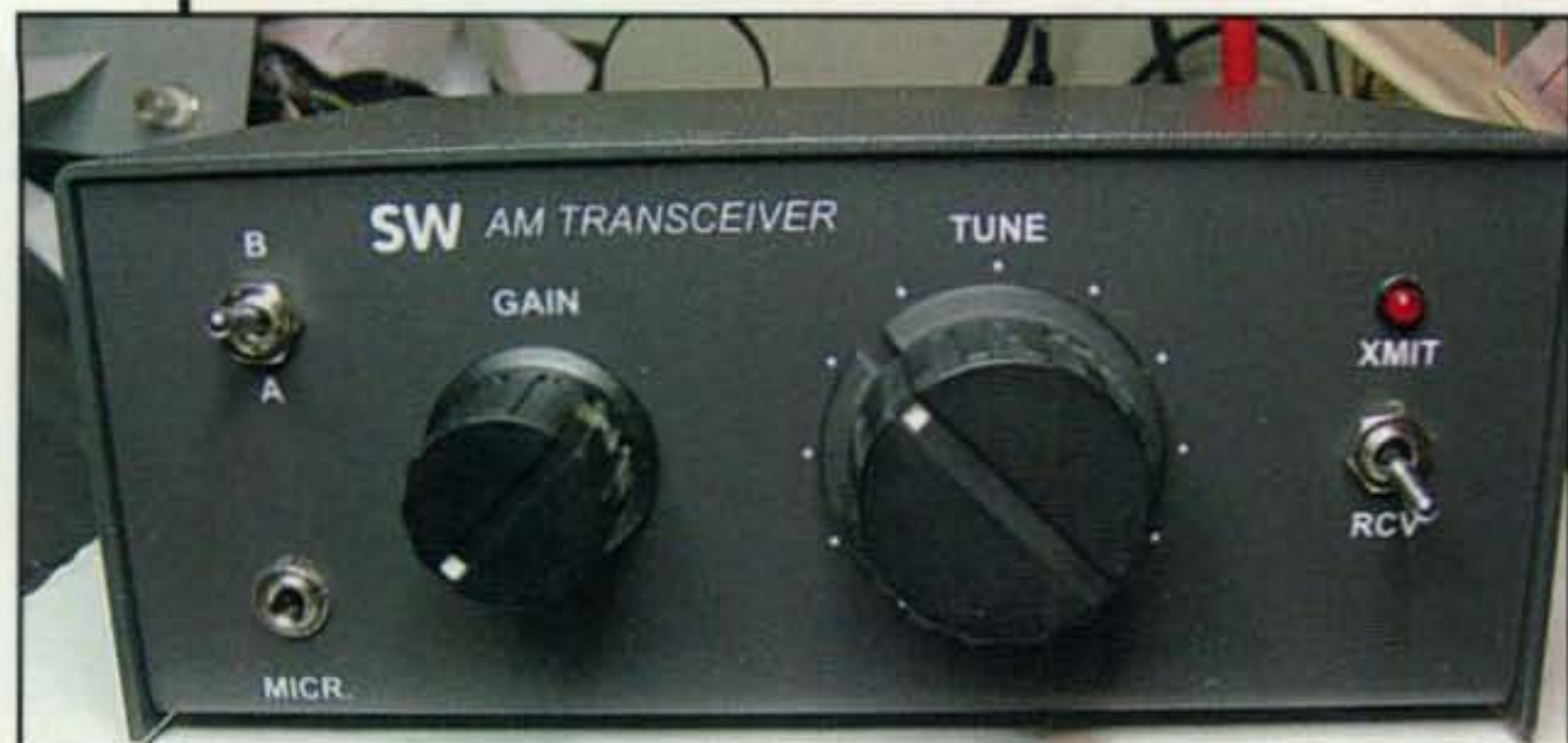
The finished Retro-75 75-meter AM transceiver from Small Wonder Labs.
