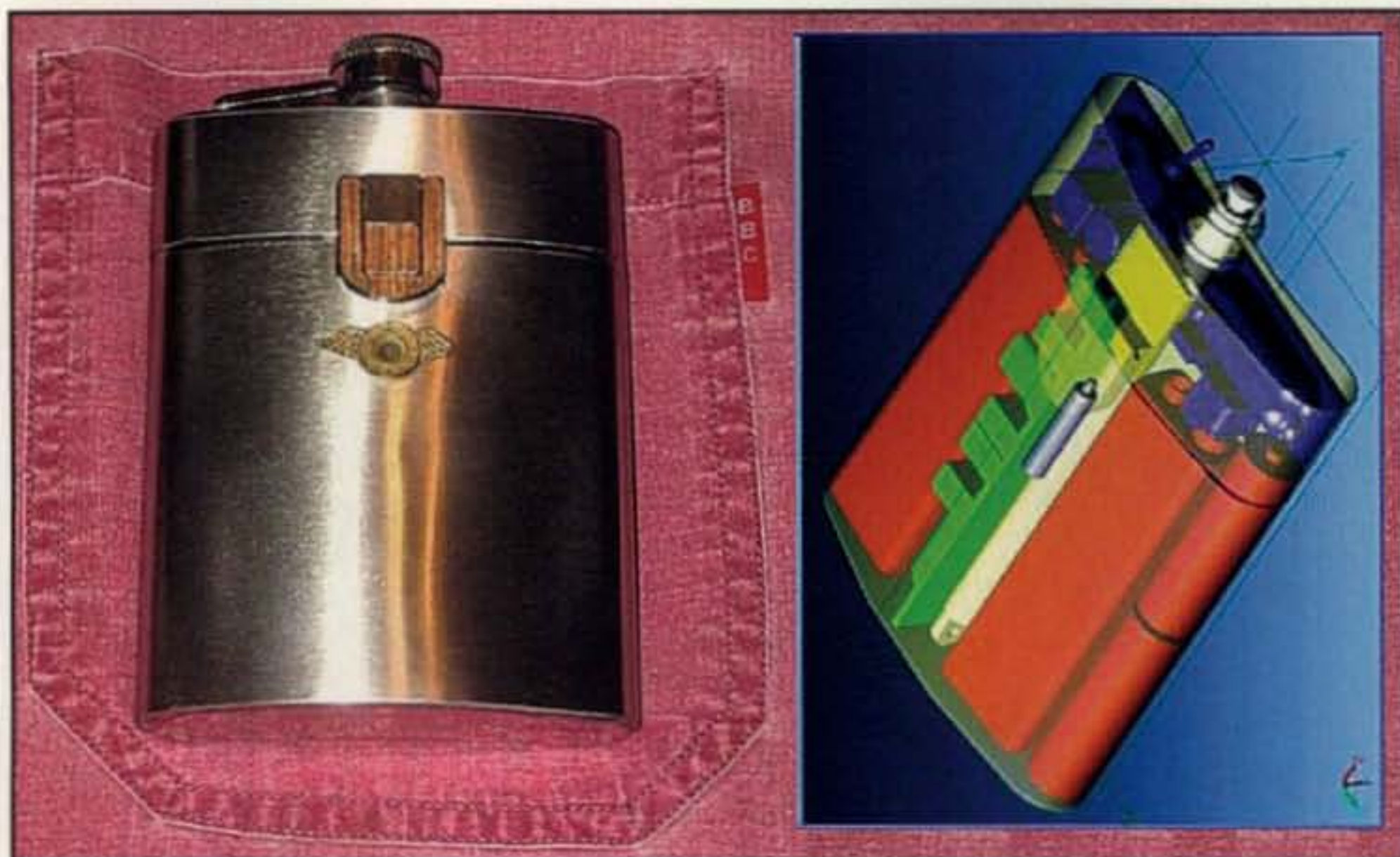
Fig. 3- 1942 Pocket Locator showing external view (left) and interior layout (right).
