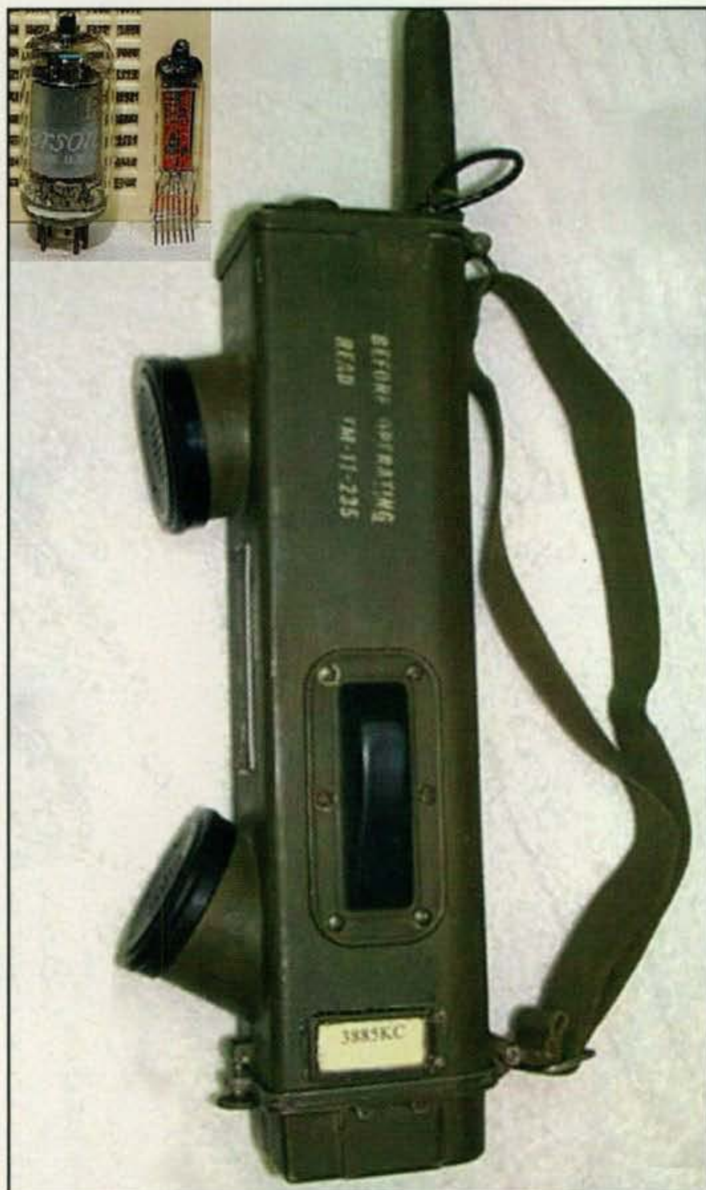
Fig. 1.— BC-611F handie-talkie, and miniature and subminiature tube-size comparison (upper left). →
