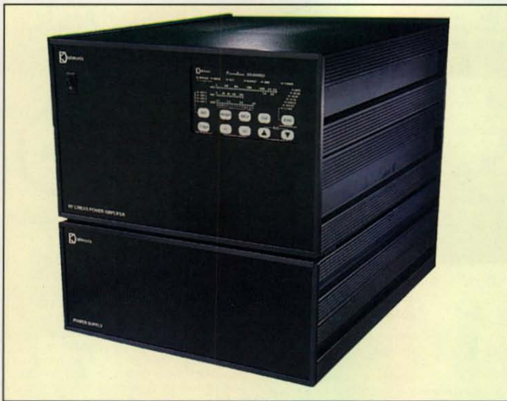
Front view of the Dishtronix DX-2400L1 “Prometheus” amplifier. Power supply is at the bottom.
