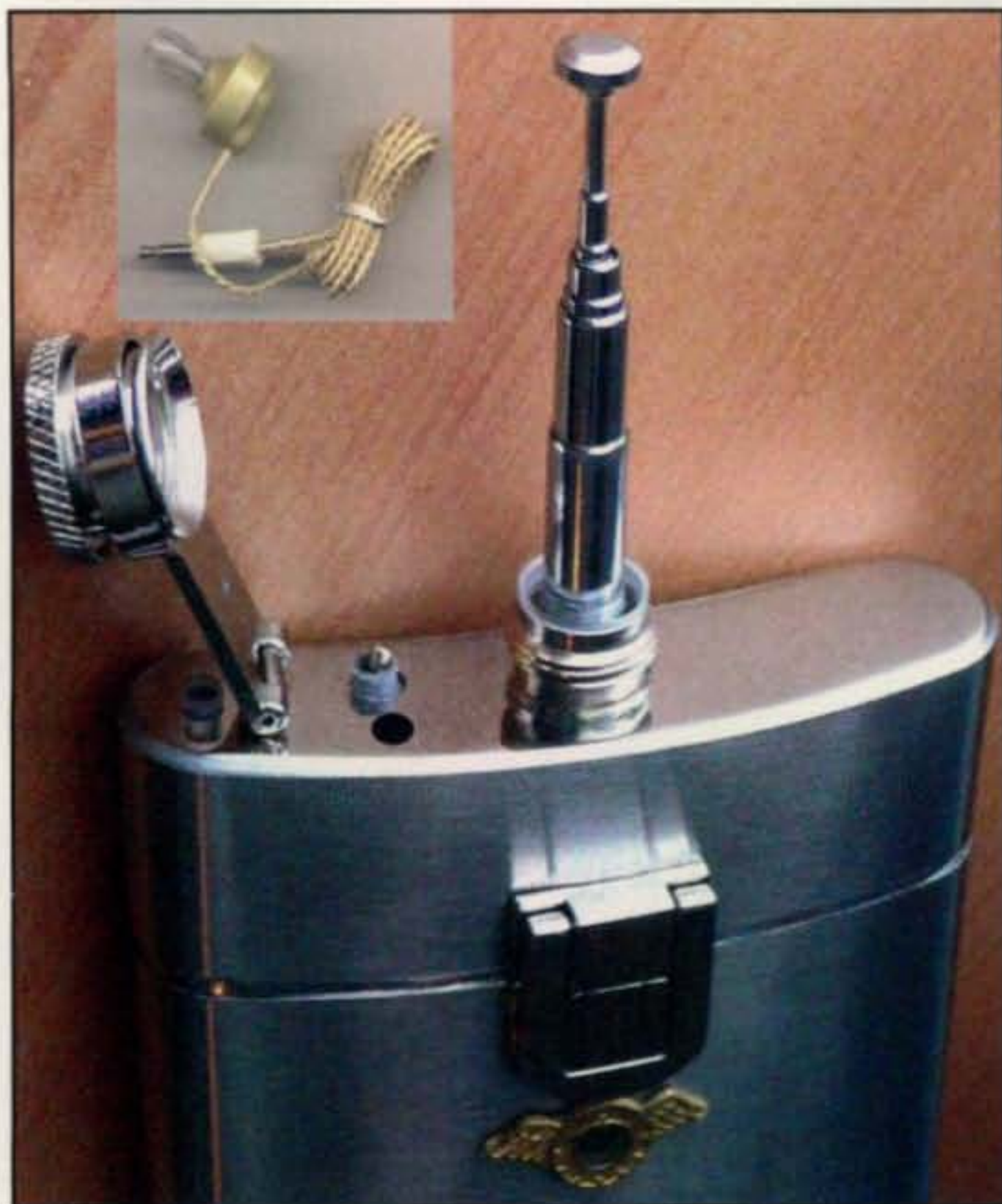
Fig. 7— Cap-strap key, transmitter button, transfer switch, and 30-inch telescoping antenna. The cap with hinged strap is the transmitting key, with cap extending left and down. The strap is pushed gently against the transmitting button for keying messages; a toggle lever (inside a sealing collar) operates the send/receive transfer switch. The audio output jack is optional, with inside plastic casing to provide a shield against outside contaminants.
