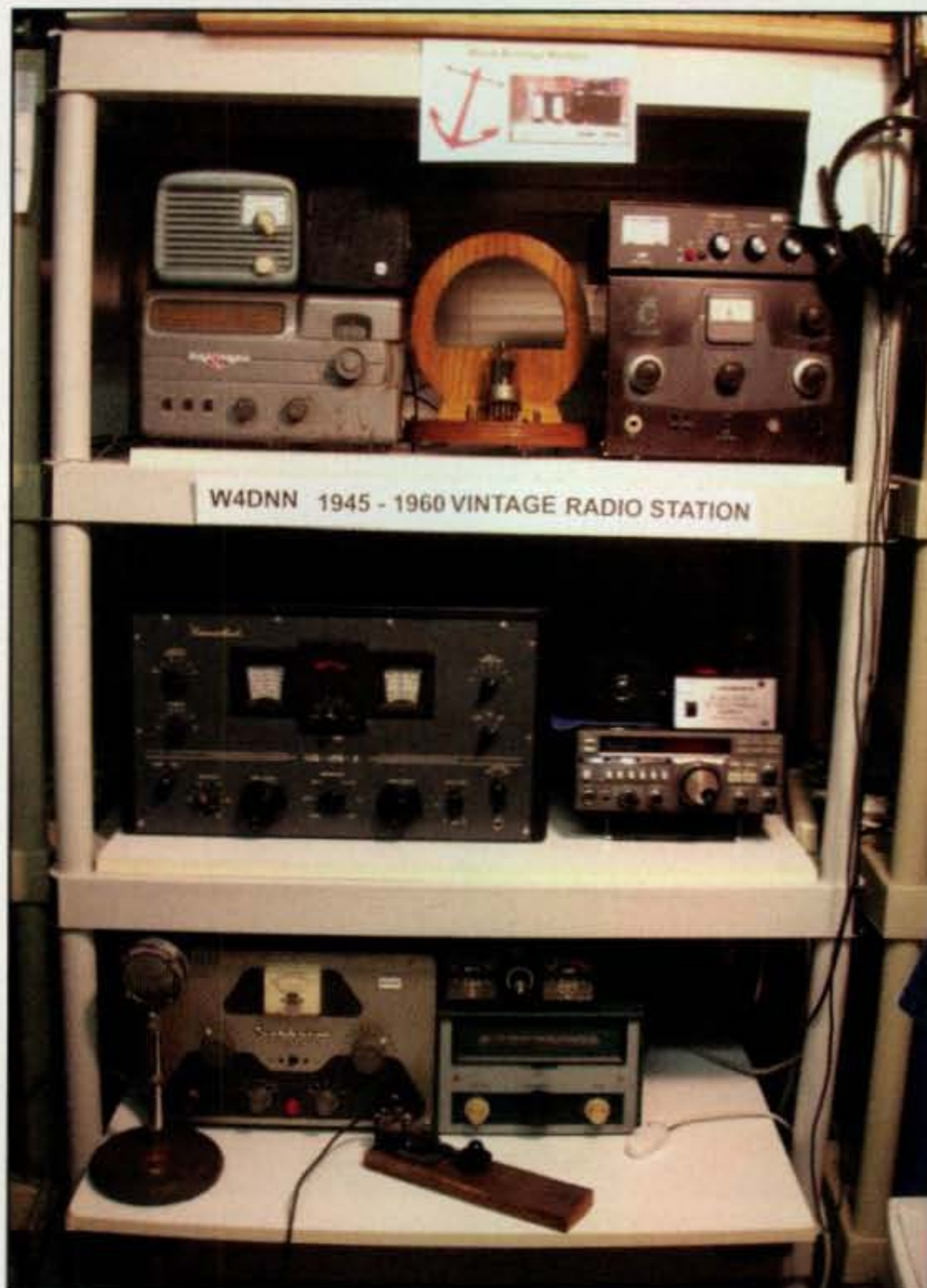
Photo D— Today's vintage station at W4DNN includes a 1960 DX-40 transmitter, a 1945 Hammarlund HQ125X receiver, and a vintage 1941 operator. On the shelf is Dennis's original Novice station—a Johnson Viking Adventurer transmitter and National SW-24 receiver.
