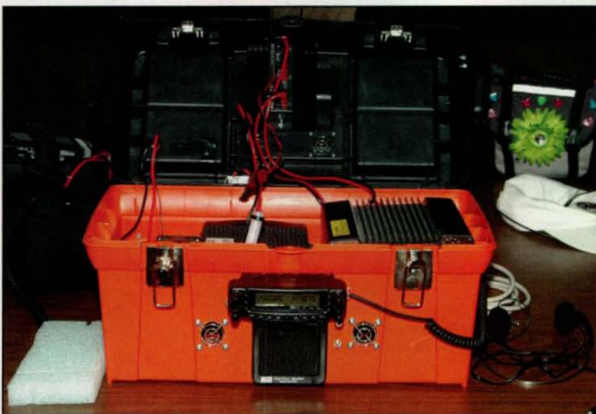
Using a plastic tool box from one of the "big-box stores," David, KA4KKF, made prudent use of the space to include his radio gear, gel-cell battery, dual cooling fans, switch-mode power supply, and packet equipment.
