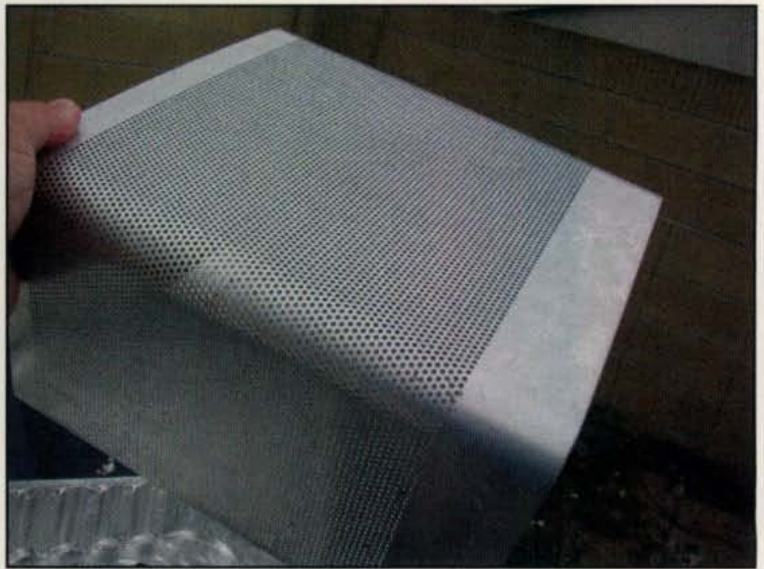
Photo 17 — I used Jasco Speed-O-Matic finish stripper to remove all paint down to the bare metal. I used a cheap aluminum-foil lasagna pan to soak the cabinet one surface at a time. The perforated cabinet made it difficult to completely remove the old paint in one pass. A second application was needed, and an old brush was used to “push” the old finish out of the holes. After chemical stripping, I used a random-orbit sander with 150-grit paper to roughen the surface to ensure good paint adhesion and to add a slight texture to the finish.
