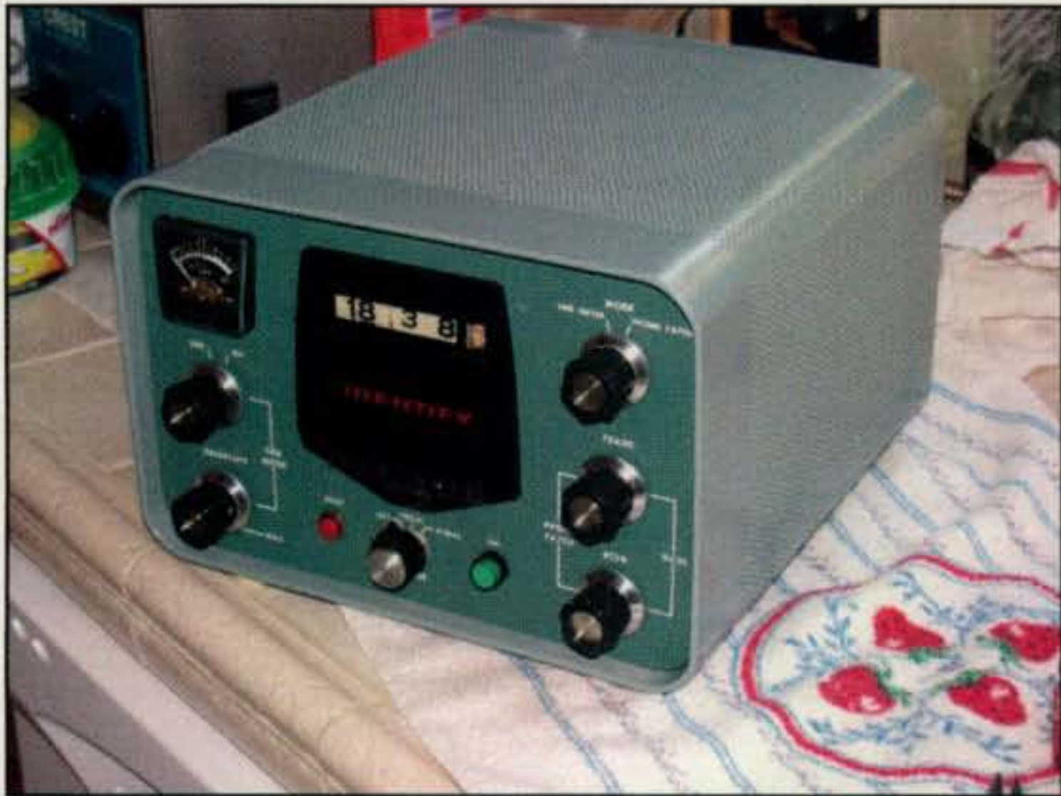
← Photo 18 — New “Heathkit Gray-Green” spray paint is available from an eBay seller for about $15 a can. One can is enough to refinish several cabinets with multiple coats. I spray paint using very fine “fog coats” by holding the can an arm’s length or more away from the surface. This prevents running, dries quickly for the next coat, and helps to add some texture to the surface. I applied five fog coats to the cabinet and let it dry in my garage for a full week. As a final step, I applied a coat of automotive paste wax to the surface. Once again, the holes caused some problems. I used an old toothbrush to scrub and push the wet wax out of the holes.
