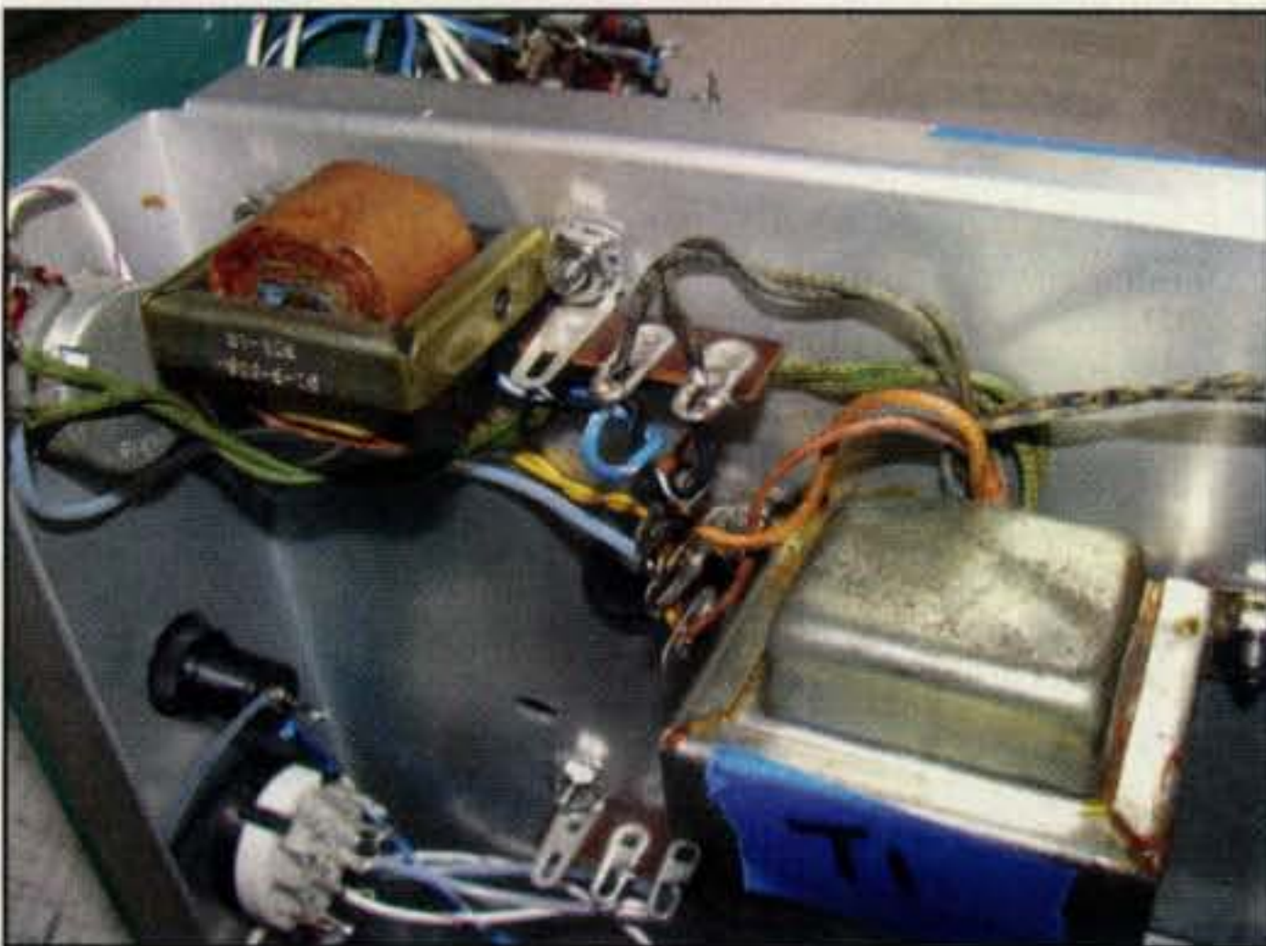
Photo 11 — When wires are short, a terminal strip can be used to make things look neater, rather than splicing the wires and using tape or heat-shrink tubing. In this same photo you can see some masking tape being used to identify components.
