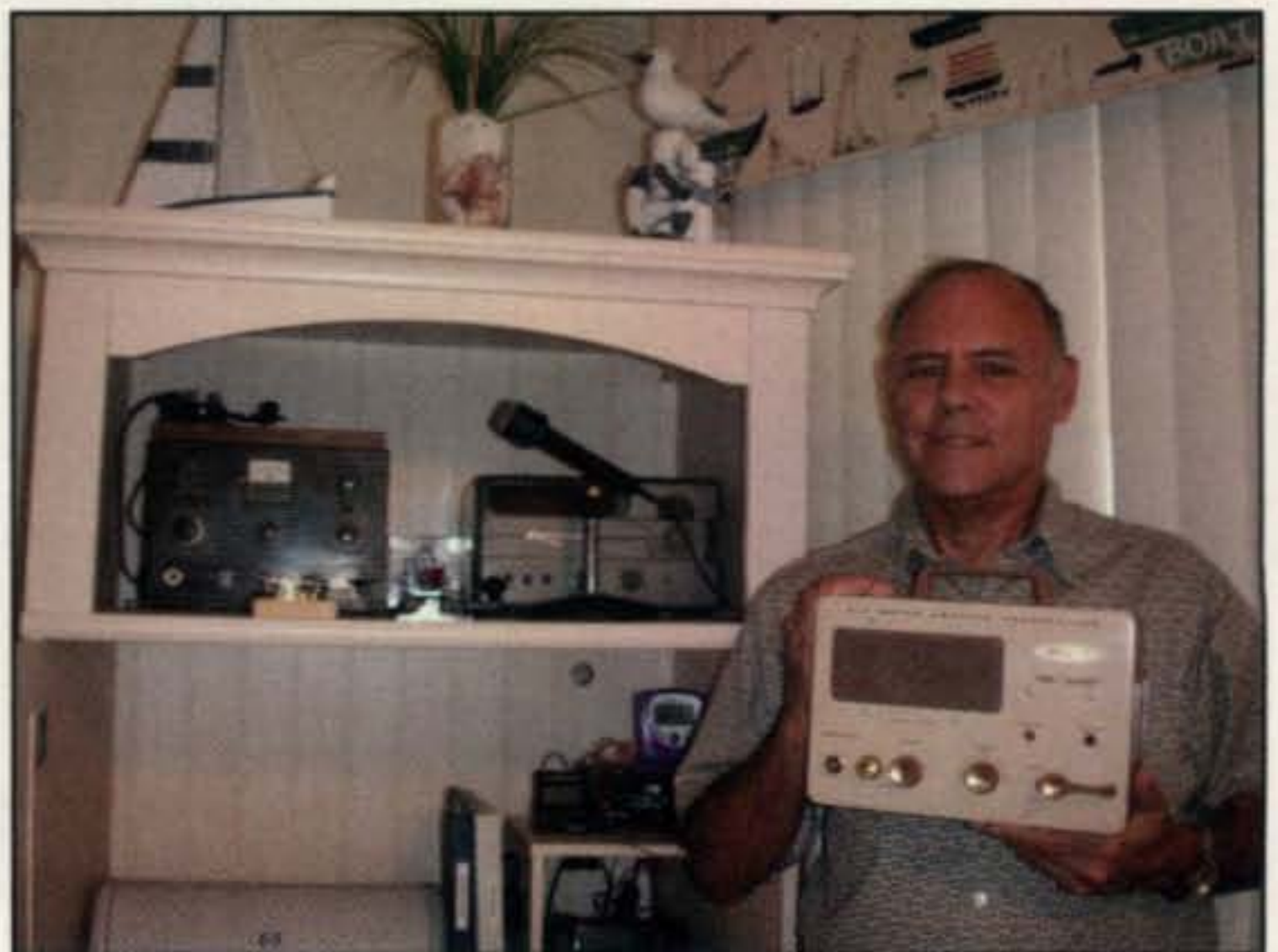
Photo C— The 1960 version of QRP: The Heathkit HW-29 “Sixer” or “Benton Harbor Lunchbox.” Heath made matching versions for 10 and 2 meters, the “Tener” and “Twoer,” respectively.
