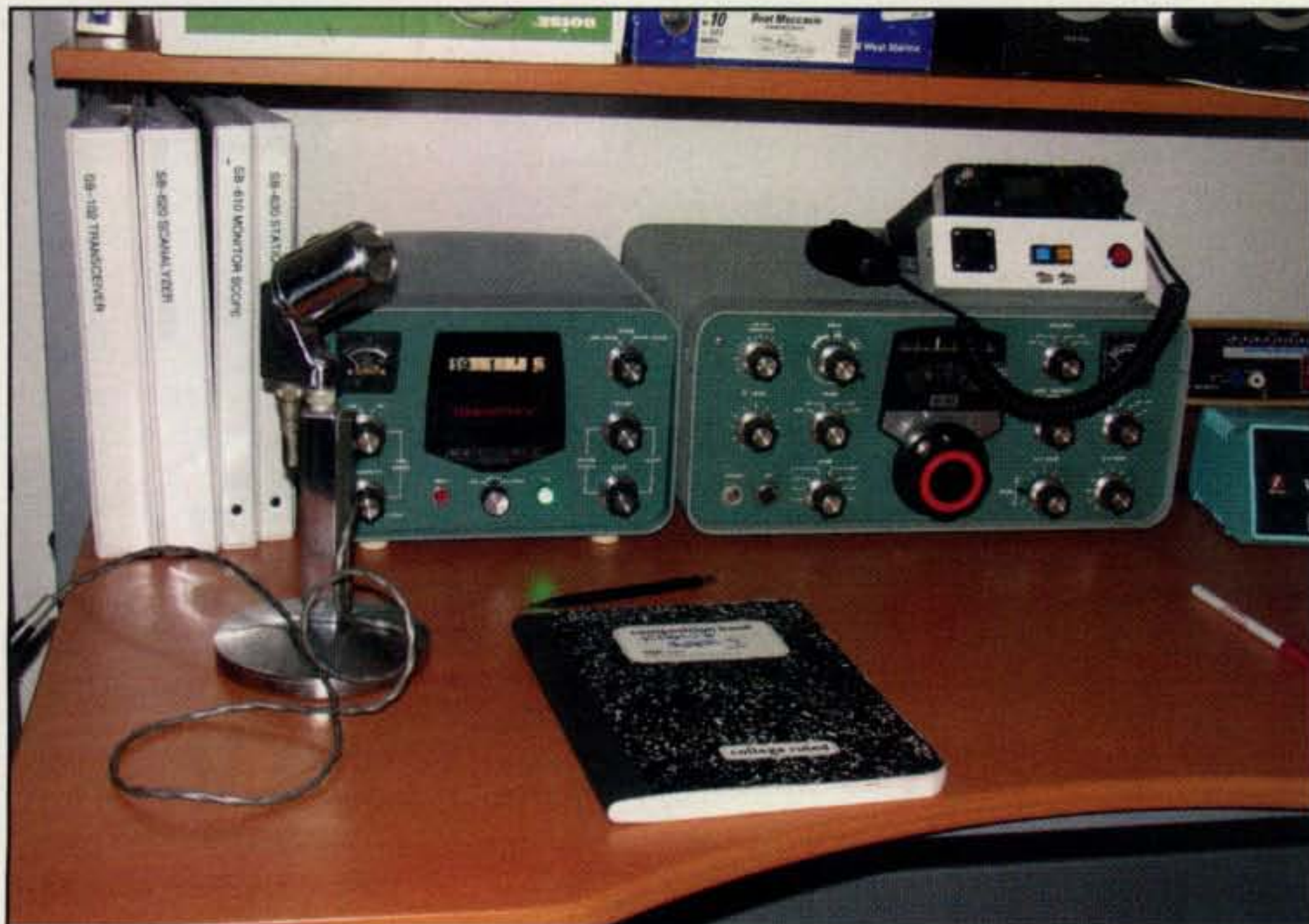
← Photo 19 — The SB-630 station console looks pretty good next to the SB-102 transceiver. I used white rubber feet (96 cents for a set of four, instead of black “riser feet,” around $12 to $15 for a set of two on eBay). The transceiver does not have the correct main tuning knob, and is next on the list for refurbishment. And no, this is not the SB-101 I mentioned earlier; this is another unit waiting in line for refurbishing.
