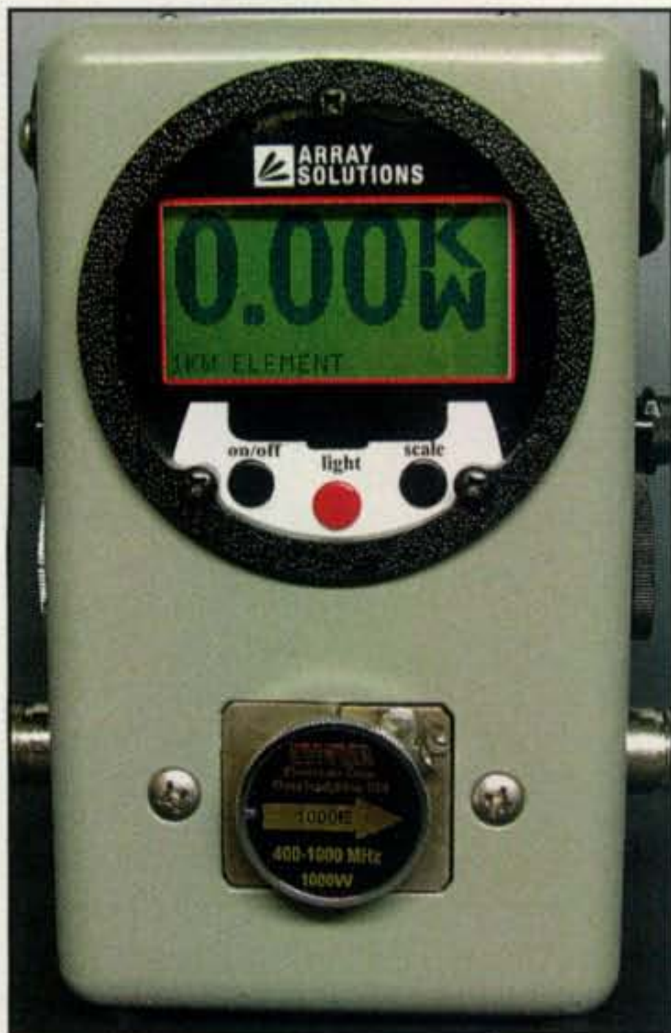
Photo E— If you would like to update your Bird 43 wattmeter and give it a modern digital readout, now you can with the AS43A, thanks to our friends at Array Solutions.
