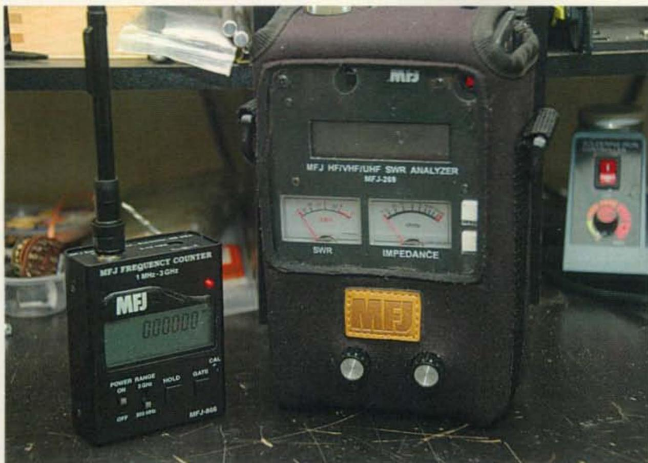
Photo E— I am at a total loss without these two pieces of test gear: the MFJ model 886 frequency counter and the Model 269B antenna analyzer/counter. These two devices, a quality digital multimeter, and some hand tools are a great start on work/test-bench equipment.
