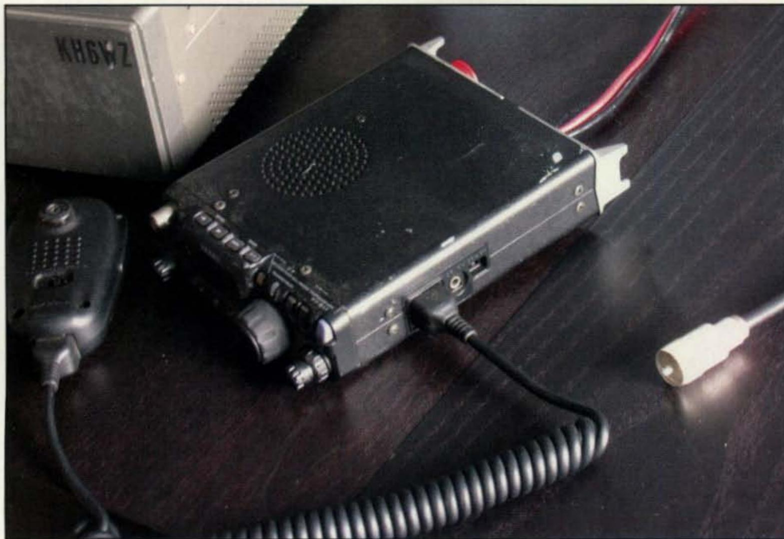
*If you have trouble operating a mobile rig, remove it from the vehicle and run it on a bench power supply in the house. In this case, the outside temperature was 80-plus degrees, with the full noon sun beating down on the car. Operating the rig in an air-conditioned house with refreshments made learning much more fun. The coax runs outside to the mobile antenna on the vehicle.*
