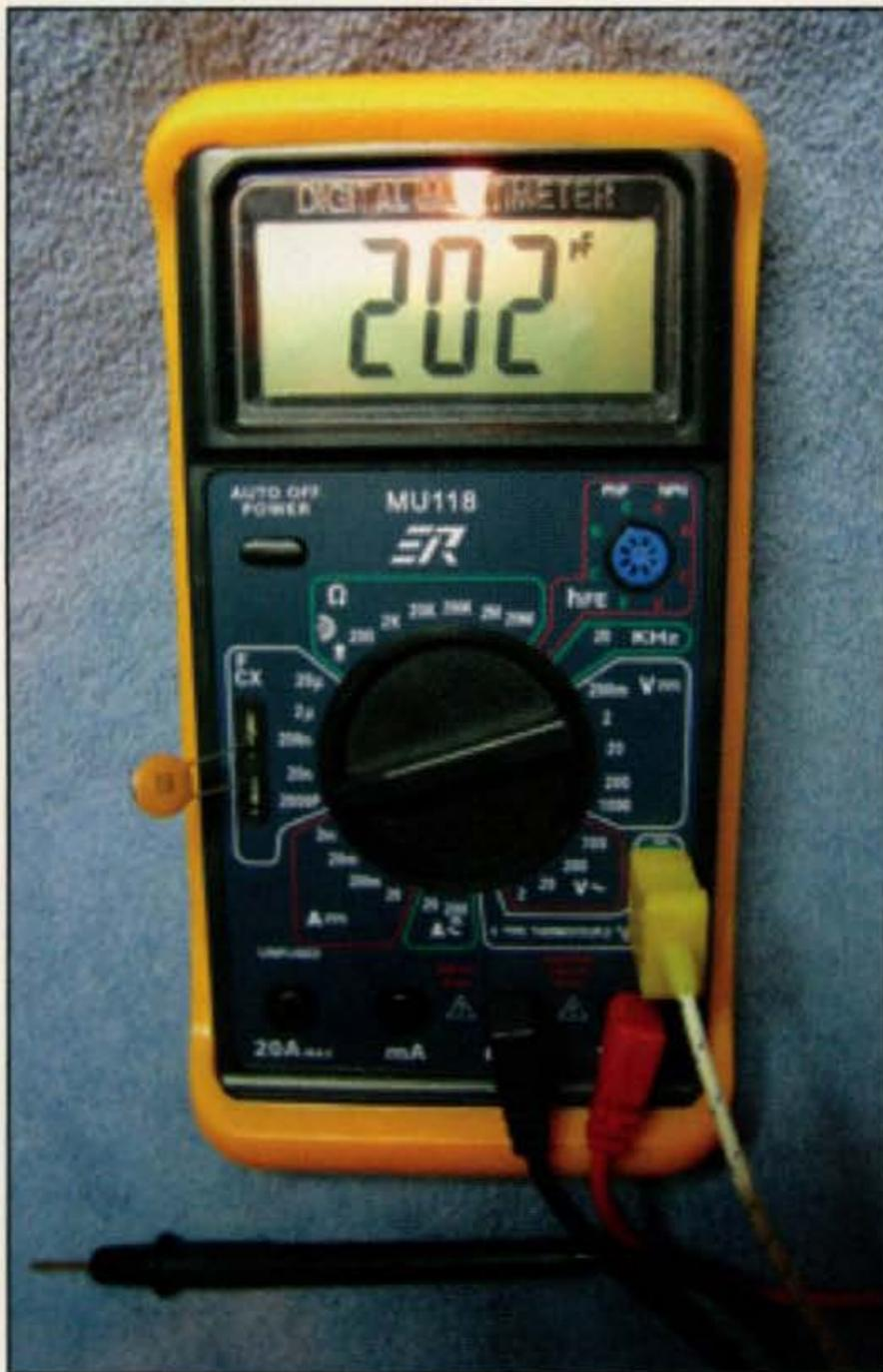
*Photo A— This inexpensive multimeter has a transistor tester as well as a thermal probe and capacitance meter. It is sold by Tower Electronics at <<http://www.pl-259.com>>.*
