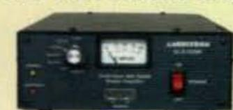
ALS-500M, \$849. 500 Watts PEP/400W CW output, 1.5-22 MHz, instant bandswitching, no tuning, no warm-up. SWR, load fault, thermal overload protected. Remote on/off control. DC amp meter. Extremely quiet fan. 13.8 VDC. 9W x3 1/2 Hx15D in., 7 lbs. ALS-500RC, \$49, Remote Head.
