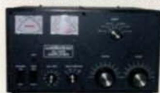
AL-80B, \$1495. Gives you full kilowatt SSB PEP output (85 Watts in) from a whisper quiet compact desk-top linear. 14Wx8 1/2 Hx 15 1/2 D inches. Plugs into 120 VAC outlet. Graphite plate genuine 3-500G tube. Nearly 70% efficiency. Weighs 48 lbs.
