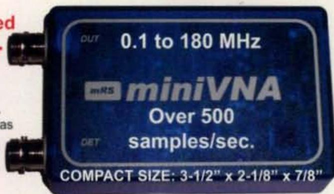
The miniVNA allows you to quickly analyze any antenna over a user defined frequency range between 0.1 and 180 MHz. In real-time, you can see at a glance where the antenna is resonant, and the SWR, return loss, impedance, phase, etc. as a function of frequency. The best (minimal) SWR frequency is automatically found and displayed.
