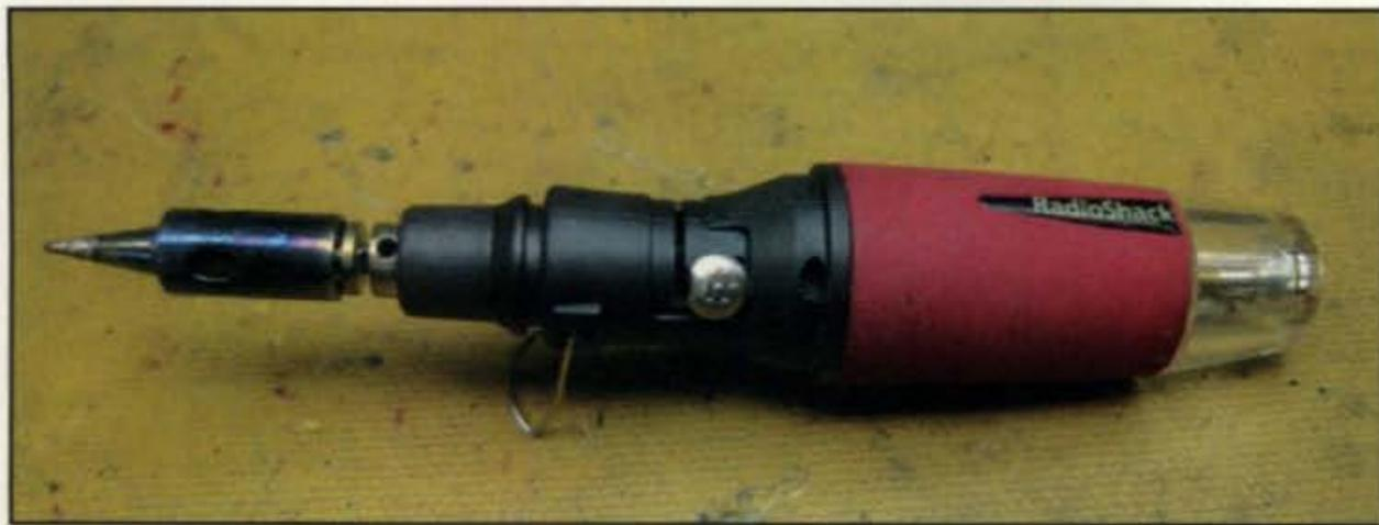
Photo B— RadioShack 64-2188 butane-powered soldering iron.
