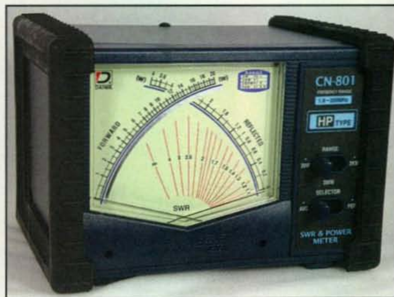
Photo B— Front view of the new Daiwa CN-801 HP3, a 1.8- to 200-MHz cross-needle SWP/power meter.
