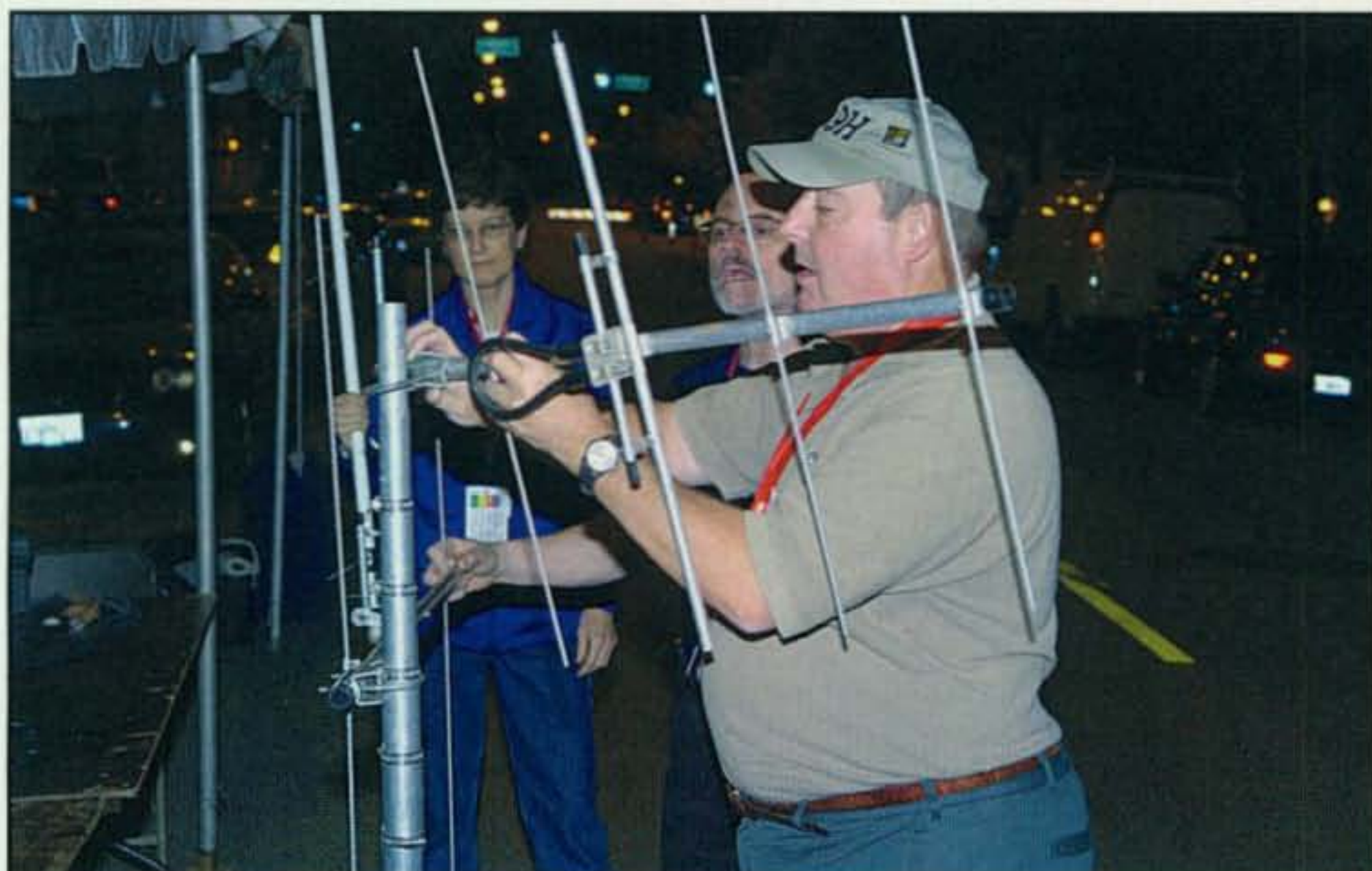
Don Whiteman, KK9H, sets up the 220 MHz link to net control for the Bank of America Chicago Marathon. (Photos courtesy of K9RST)
