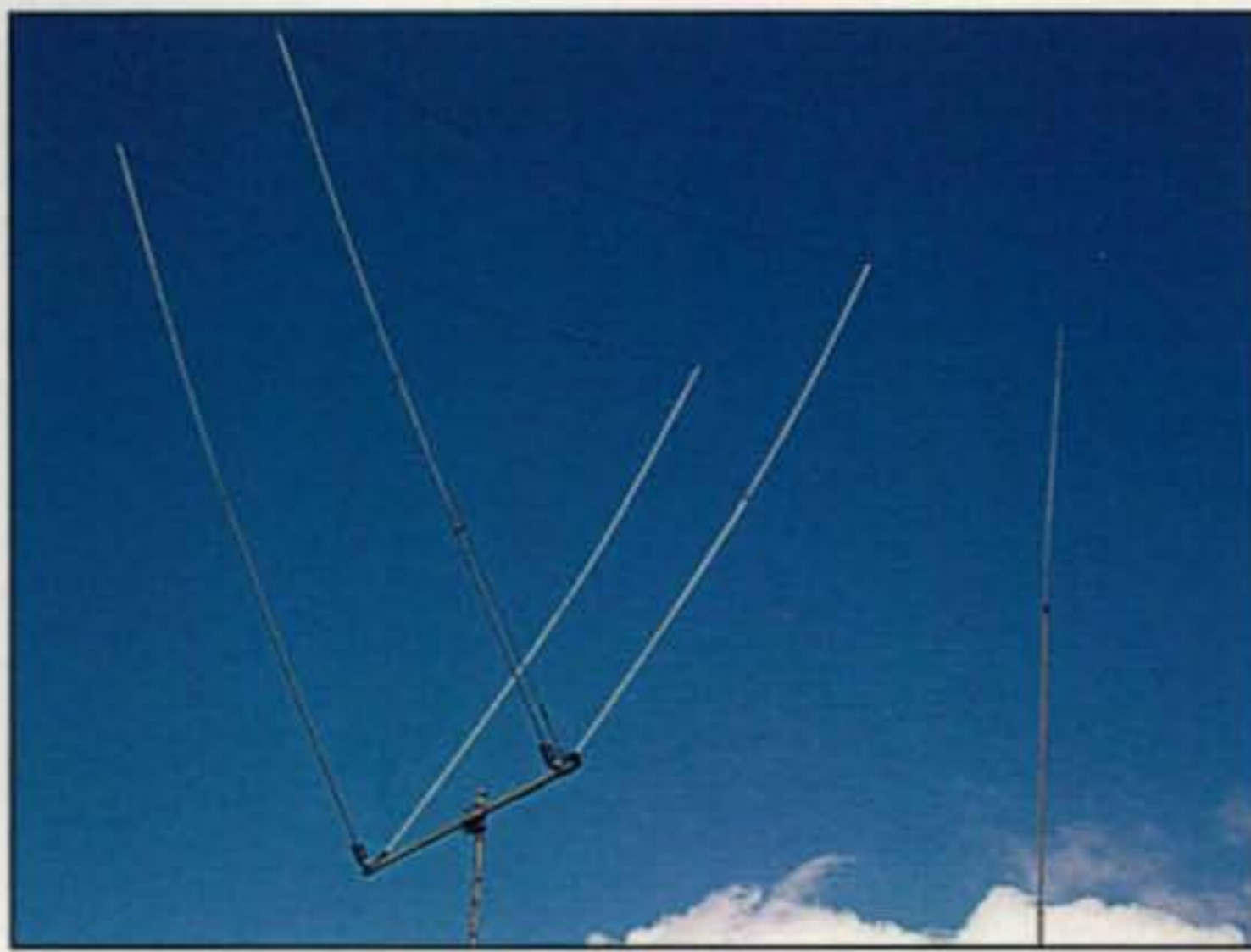
Photo C— Here are a couple of photos of Vortex Antennas Whirlwind series—a two-element delta loop for 10 meters, and a wide spaced, three-element delta loop for 6 meters.
