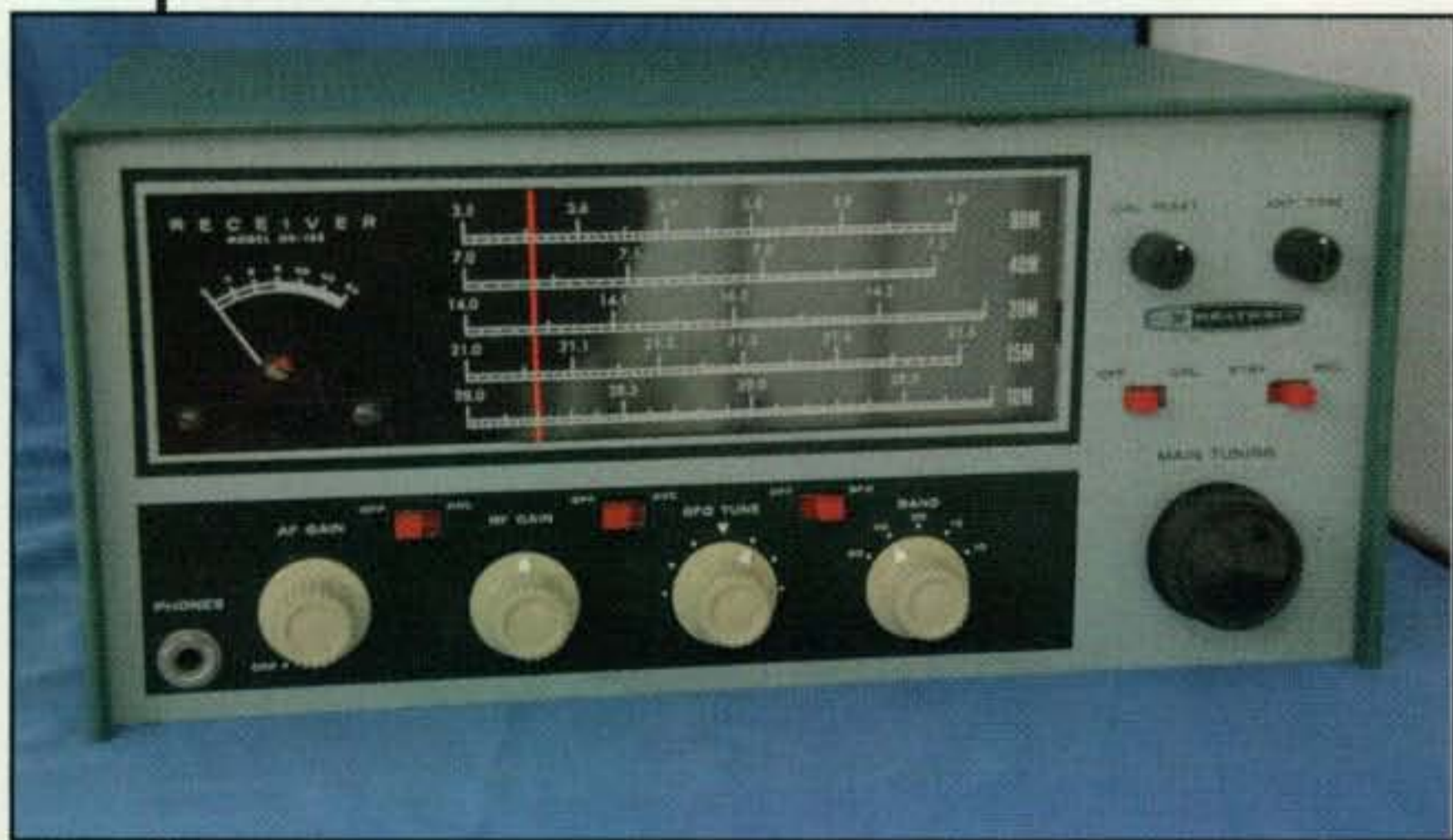
The Heathkit HR-10 is a nice-looking receiver and, for the time, a good value for the money. This single-conversion superhet was a mainstay for Novice class operators in the mid 1960s.
