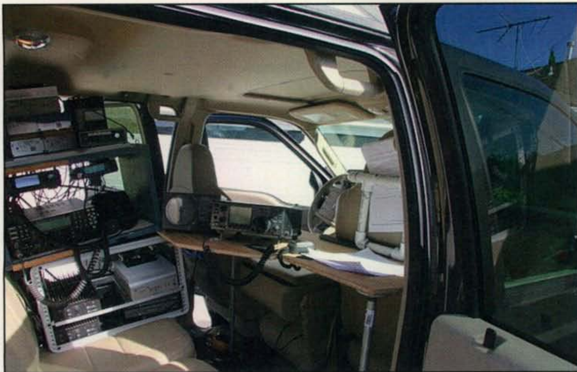
Photo 2— Cramped but efficient, here is the operating position at N6TEB/R. This console is located in the mid-section of the SUV and is usually operated while safely parked on a hilltop. A platform is made from plywood, and is supported by plumbing hardware.
