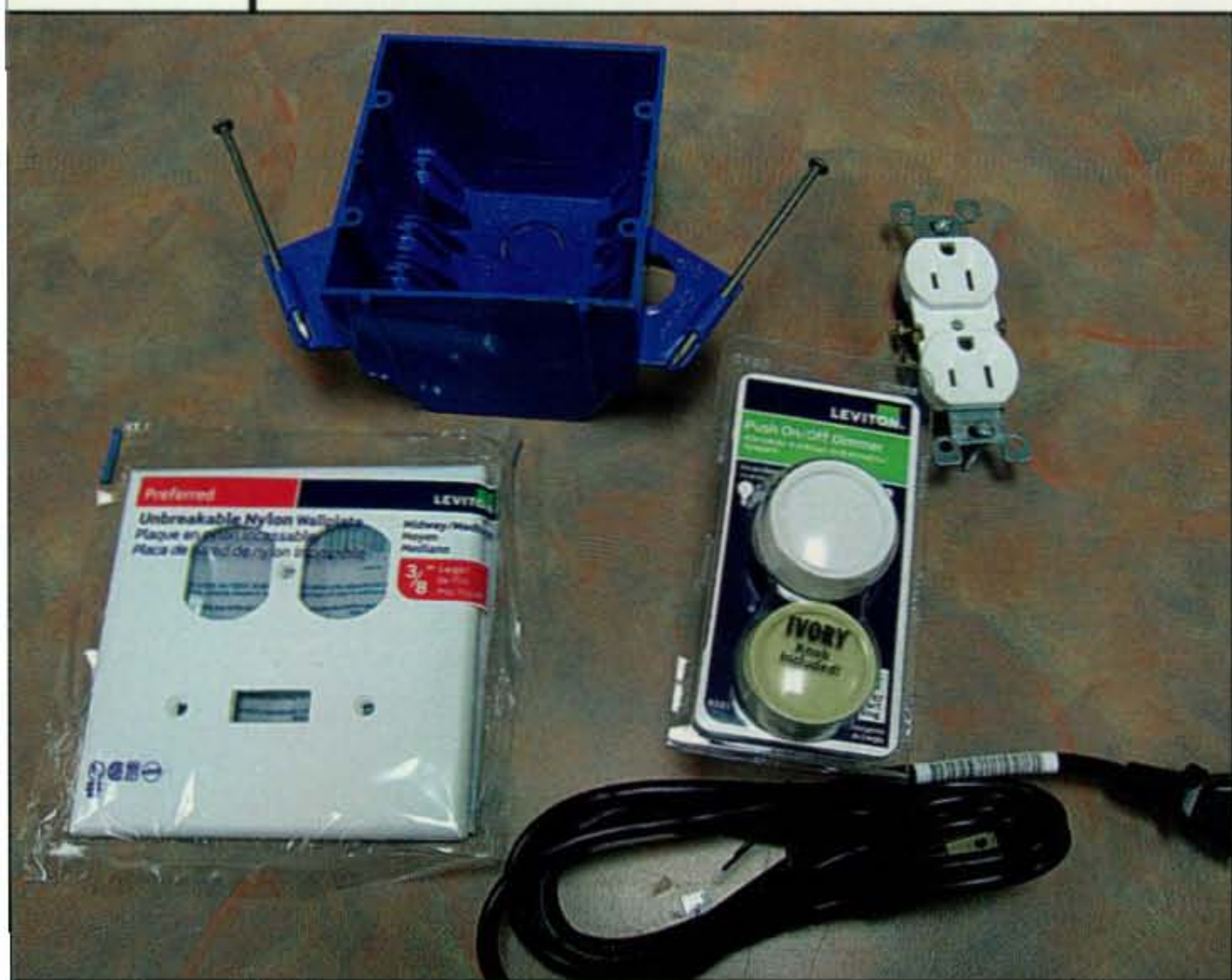
Here are the parts needed to build the soldering iron controller.
