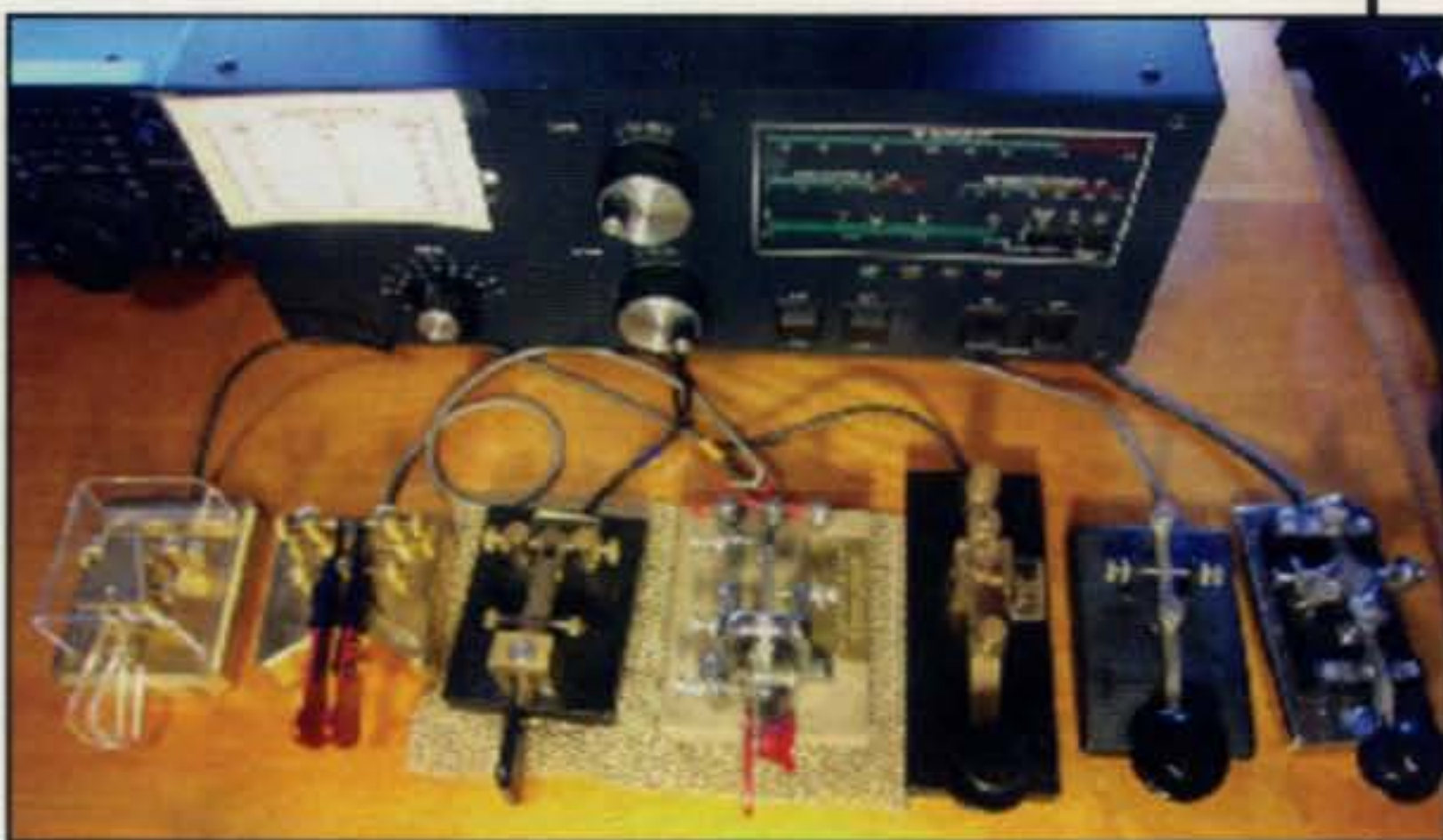
These keys are on the desk at W6SL. John identifies them as follows (left to right): Scheunemann Dirigent Morsetasten Iambic; Begali Iambic; Kent Single Paddle; Vibroplex 1963 Single Paddle; Kent KT1 Straight Key; Wm. Nye straight key (discontinued); Chinese Army Key D-117. The straight keys are hooked in parallel. All of the paddles go to a Daiwa D-210 keyer. (Photo courtesy of John, W6SL)
