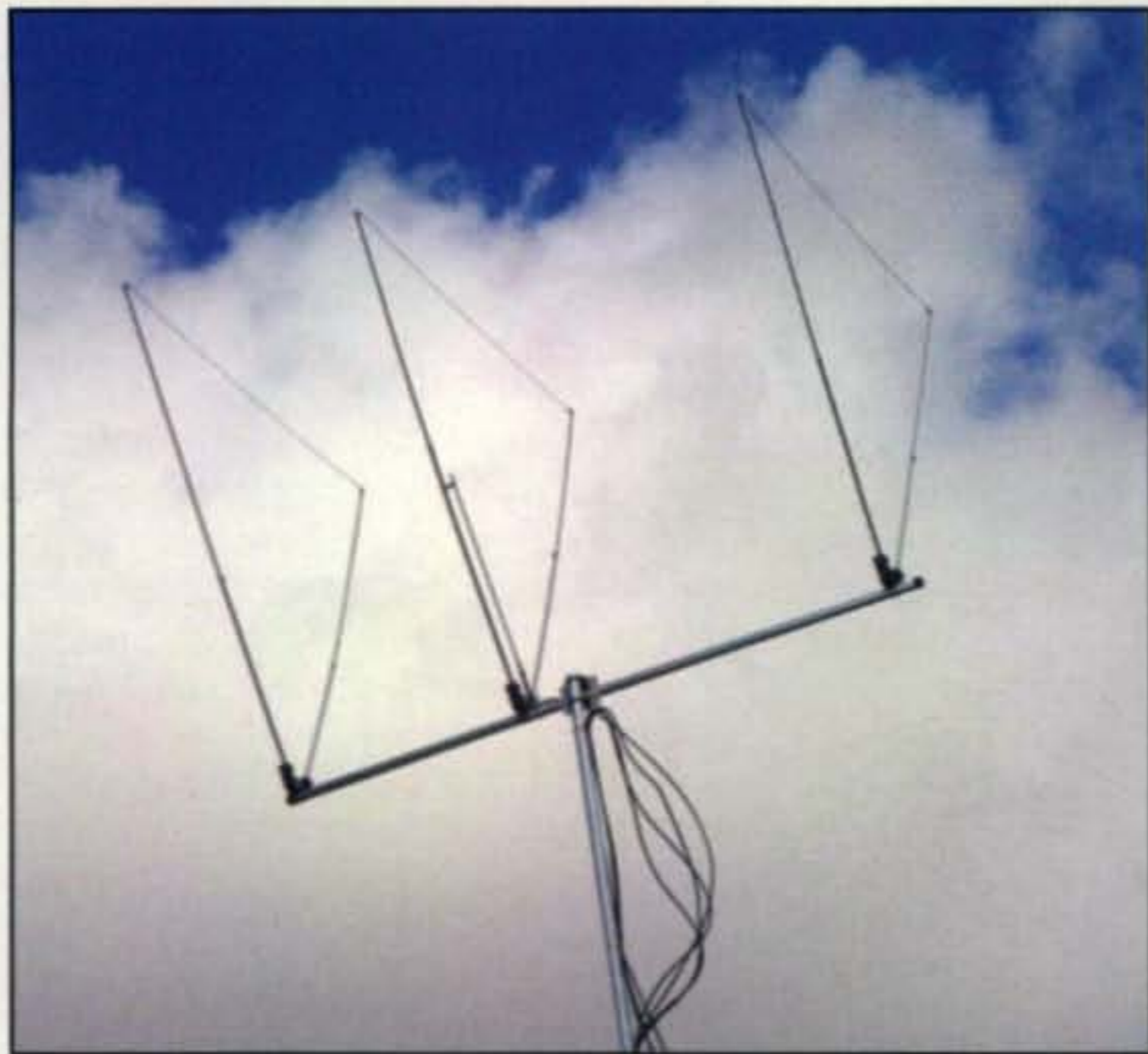
Photo C— Here are a couple of photos of Vortex Antennas Whirlwind series—a two-element delta loop for 10 meters, and a wide spaced, three-element delta loop for 6 meters.
