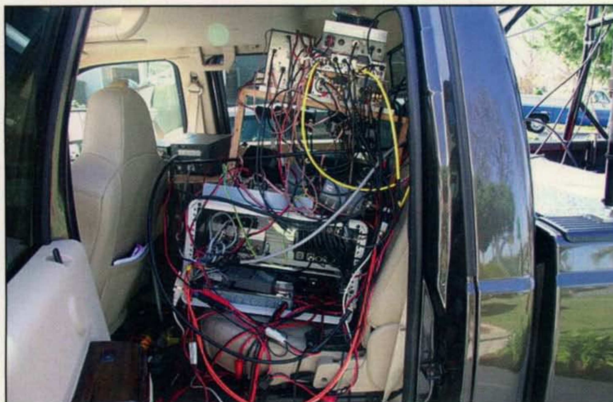
Photo 3— This is a rear view of the operating console. Wires and radios, radios and wires, oh my. The units are securely strapped down to each other and to the seat.
