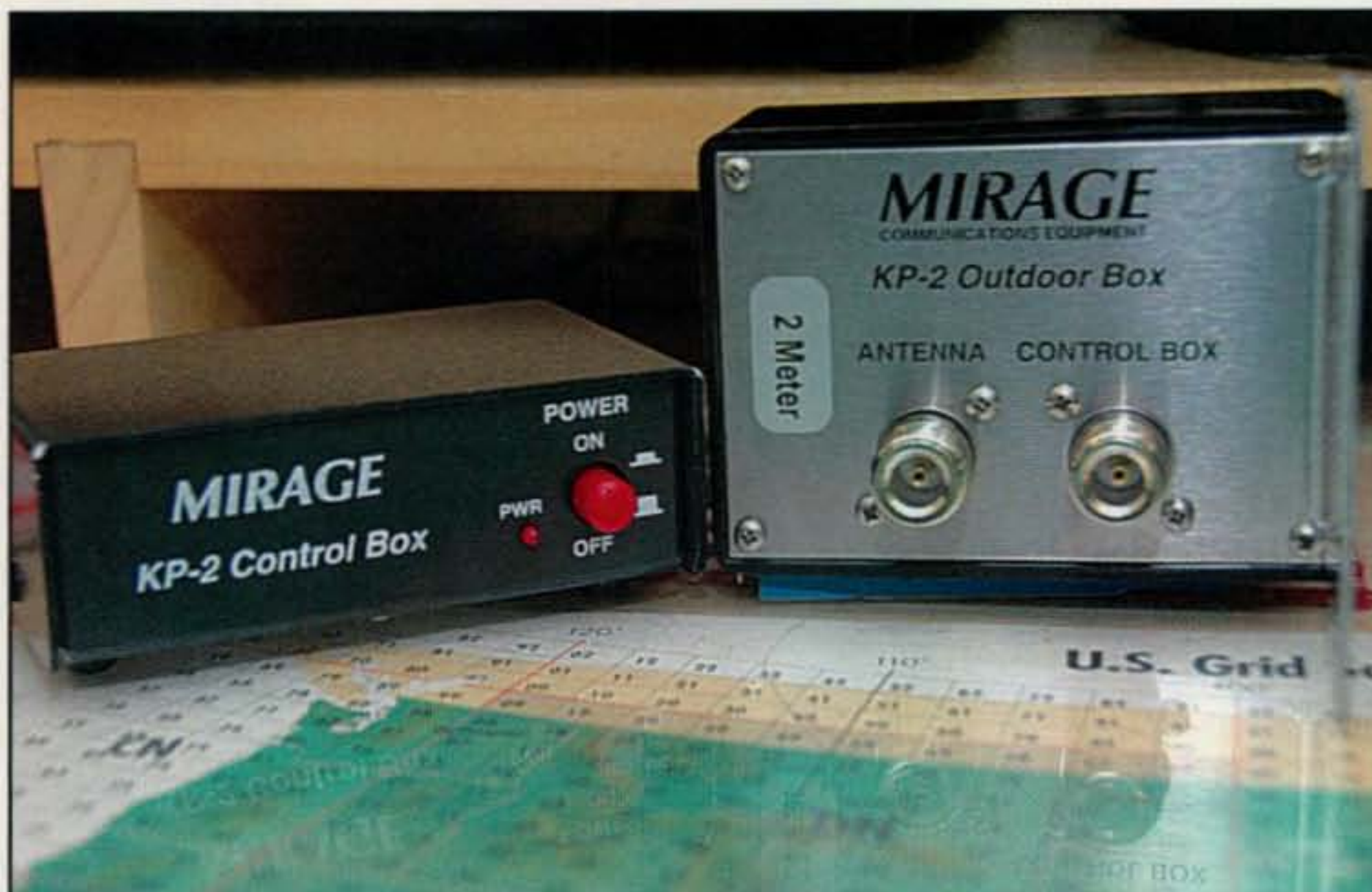
This Mirage 2-meter mast-head preamp is one very nice piece of VHF+ gear at a reasonable list price of $199.95. Sure it sounds like a lot of money, but it really improves your 2-meter reception while keeping the overall noise to a bare minimum.
