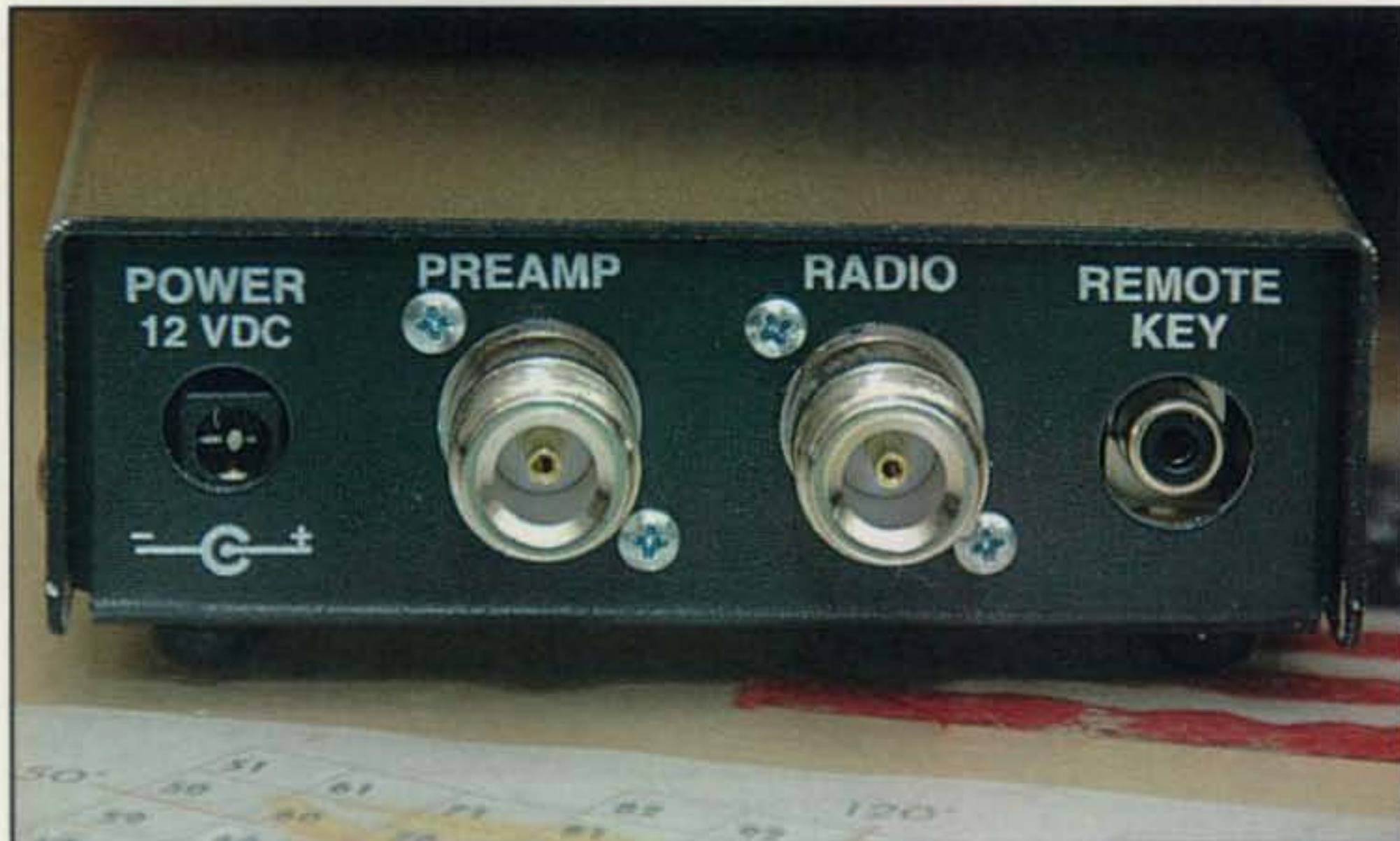
This is the back end of the Mirage control box. Notice that it takes 12 VDC and this is applied to the coaxial cable going to the mast-head preamp to provide working voltages for the preamp circuitry. Nice, neat and clean.
