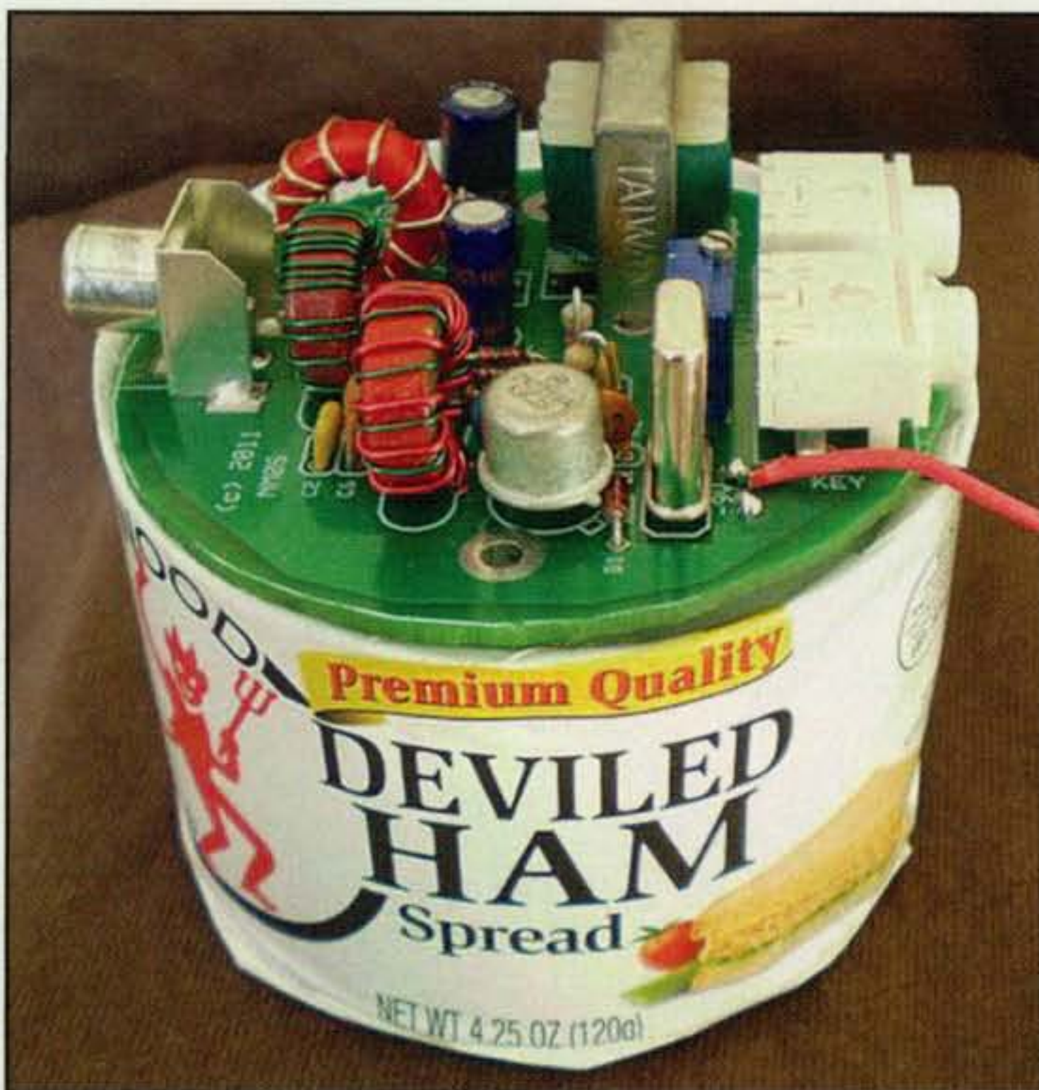
The 4SQR Hamcan transceiver from the Four States QRP Group has only 26 parts.
