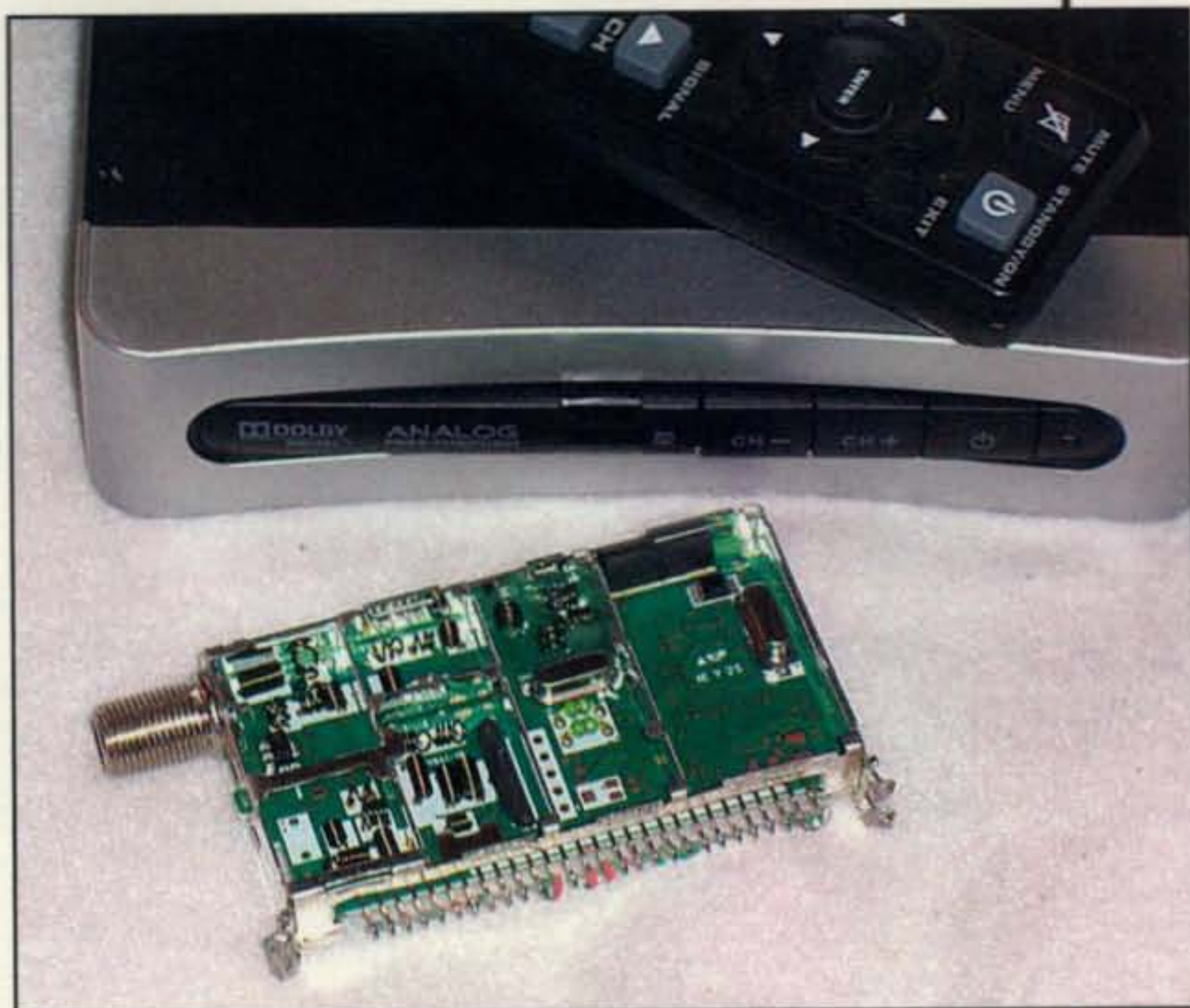
Photo A—A $40 HDTV converter and its simple tuner.
