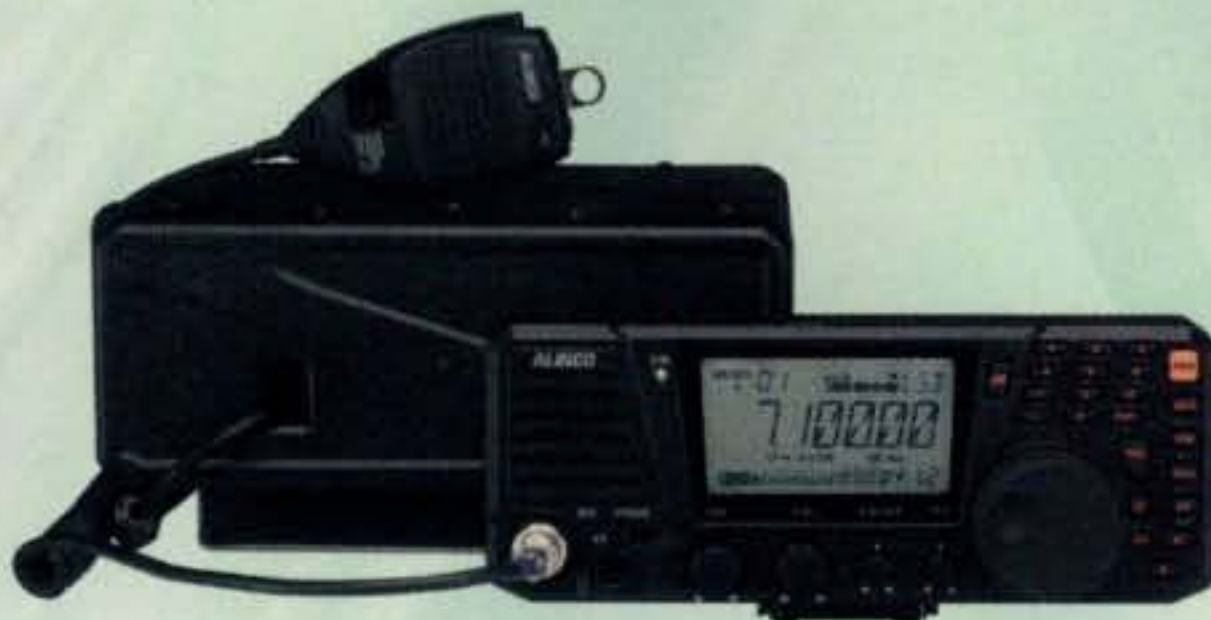
HF 100W SSB/CW/FM/AM DESK-TOP TRANSCEIVER DX-SR8T
