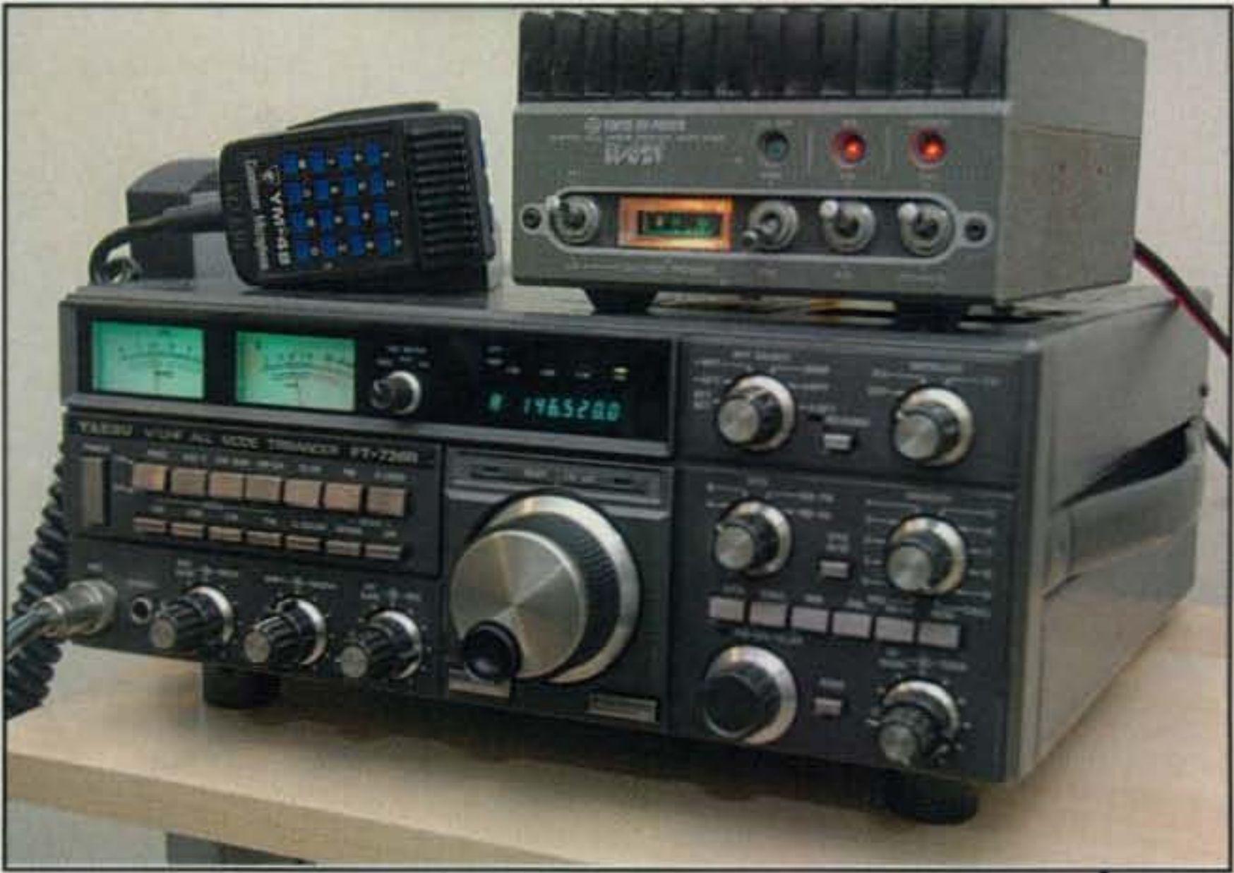
My VHF+ workhorse, the Yaesu FT-726R. This is an "oldie-but-goodie" that has three bands in one box. Currently I have 144-MHz and 432-MHz modules installed (one of these days I'll find a 6-meter module!). I bought this rig about three years ago for $400 including shipping thanks to an internet auction site. Not a bad deal! It has the satellite board installed that gives me full duplex on both bands so I can hear my downlink signal while transmitting on the satellite uplink.
