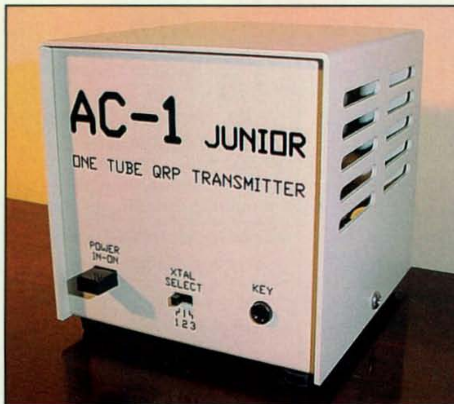
Photo D— Front view of Glowbug 40-meter CW transmitter. (Glowbug photos courtesy of Dwight Morrison, KG4HSY)
