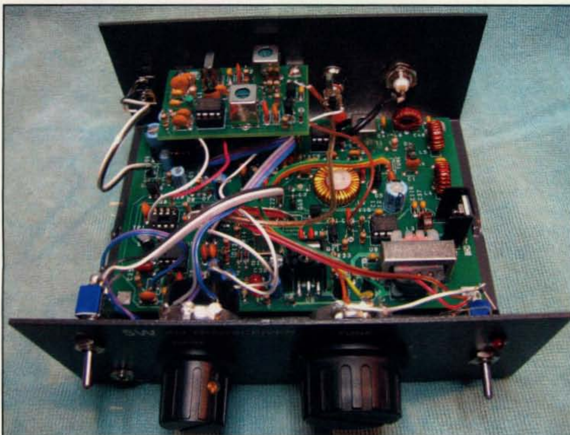
Photo C. Retro-75 with finished Retro-Helper installed and ready to go!
