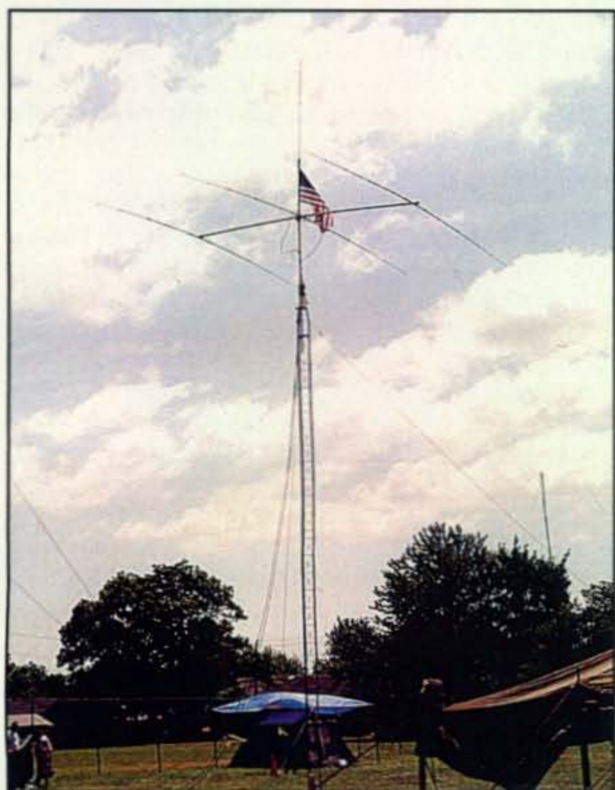
This tower and antenna at the Long Island Mobile Amateur Radio Club (LIMARC) Field Day operation is typical of temporary stations clubs may set up and use not only for Field Day, but for emergency field operations as well. (N2GA photo)
