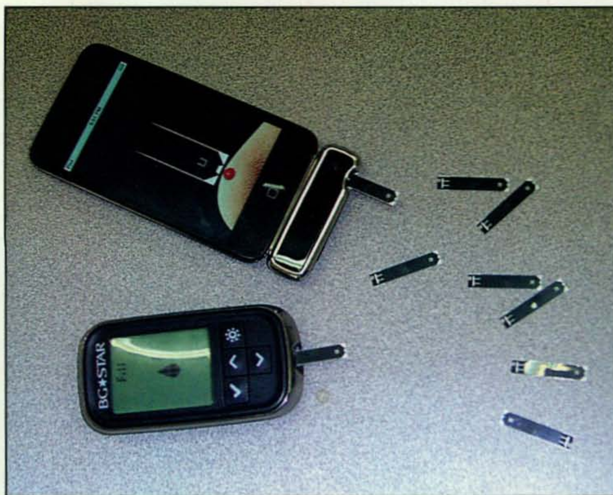
A glucose testing meter, test strips and an iPhone set up with a special module to let it serve as a test meter!
