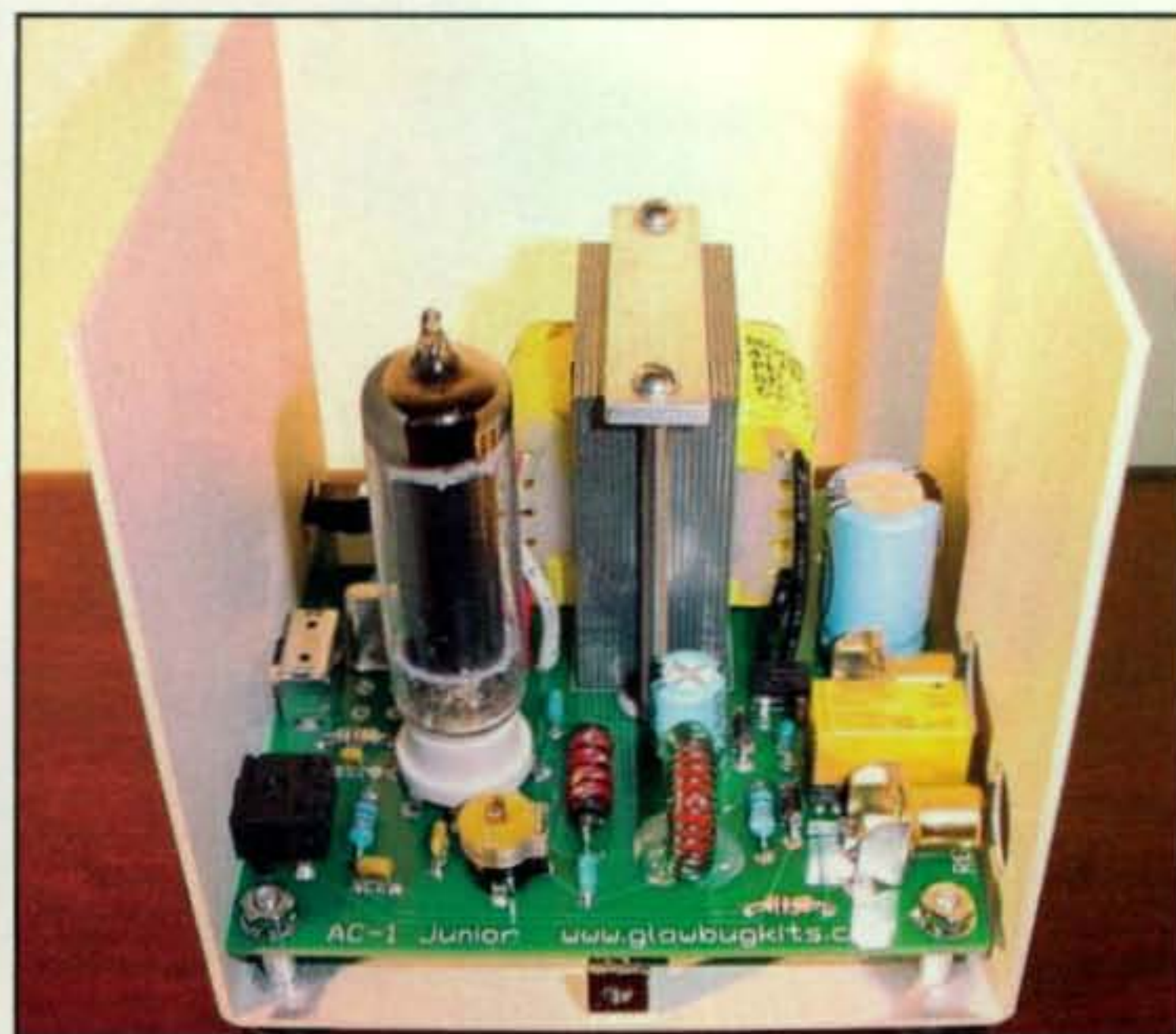
Photo E— Inside view of the Glowbug. Notice the single toroid near the front and the power transformer mounted sideways to fit on the board.
