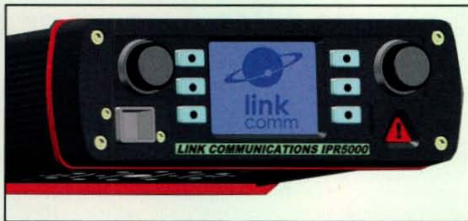
Photo C— Link Communications has revealed its IPR5000 radio, which it calls a revolutionary new radio system that is able to provide PTT communications over an IP network along with GPS-based Automatic Vehicle Location (AVL).
