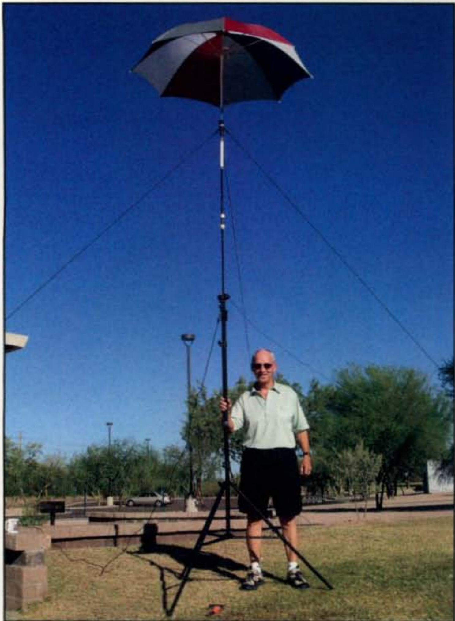
Now that's what we call a top-hat! Bill Maynard, W7ZT, with his umbrella antenna.
