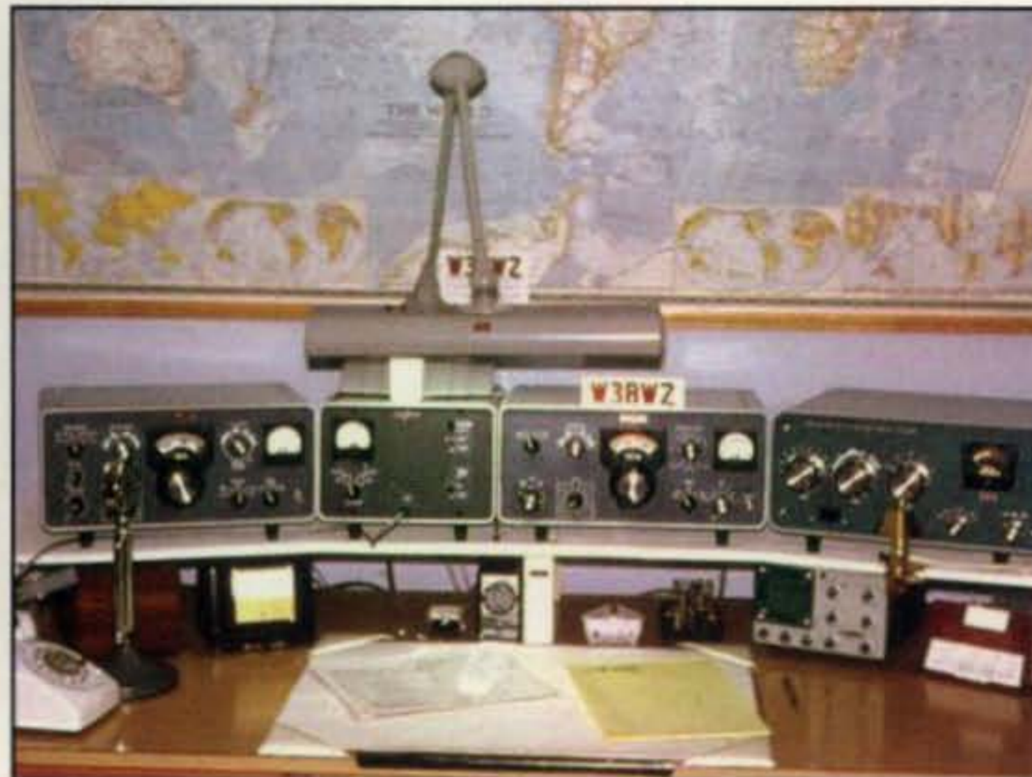
For those who don't recognize this gear, it's a Collins S-Line circa 1966. That's a Heath SB-200 amplifier on the right with a Heath Monitor Scope under the shelf. (Photo courtesy of Lynn, W4NL [ex-W3BWZ])
