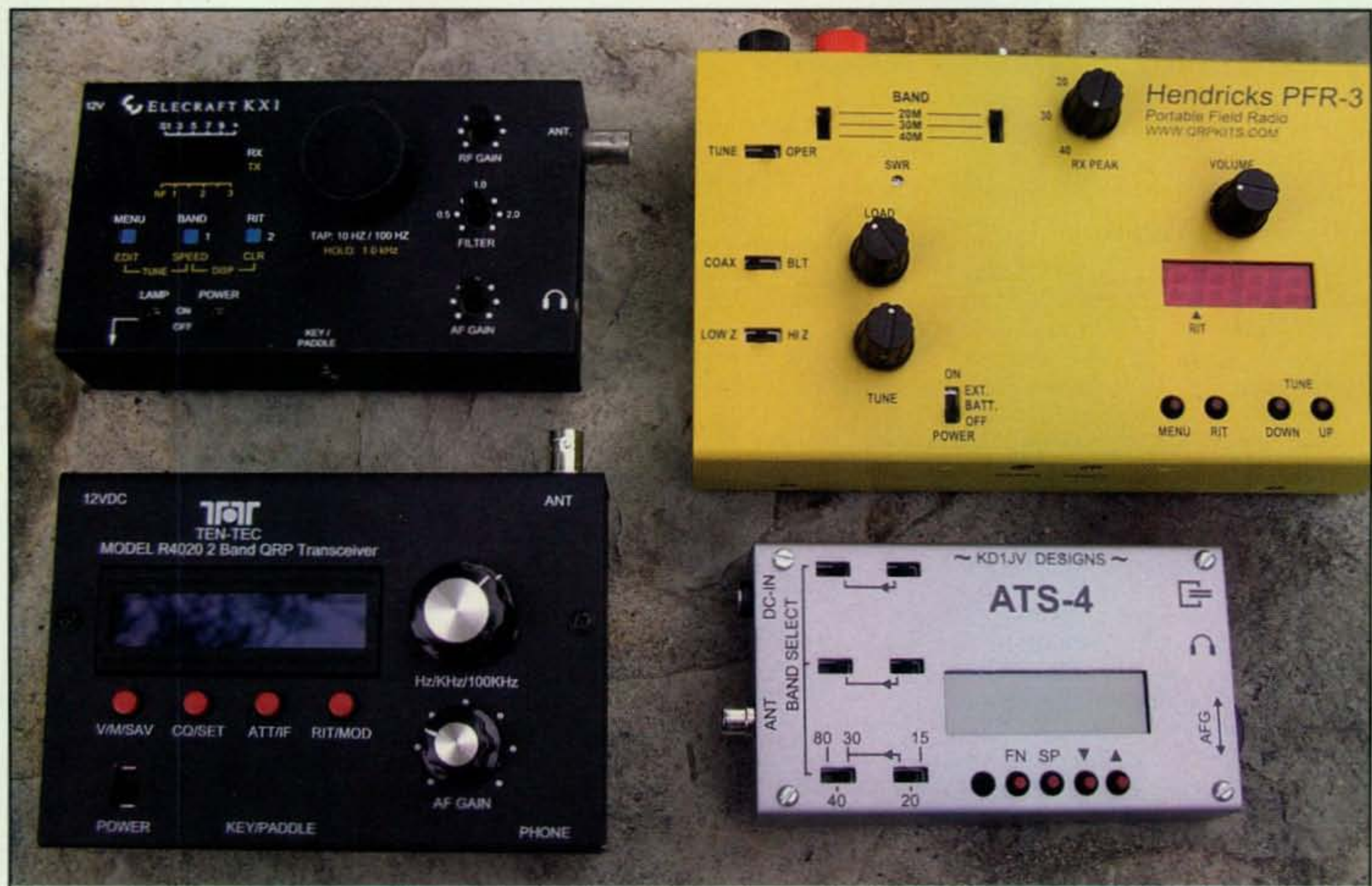
Photo E— Clockwise from the upper left corner: the Elecraft KX-1; Hendricks QRPKits PFR-1; the ATS-4 by Steve Weber, KD1JV; and the Ten-Tec R 2040.
