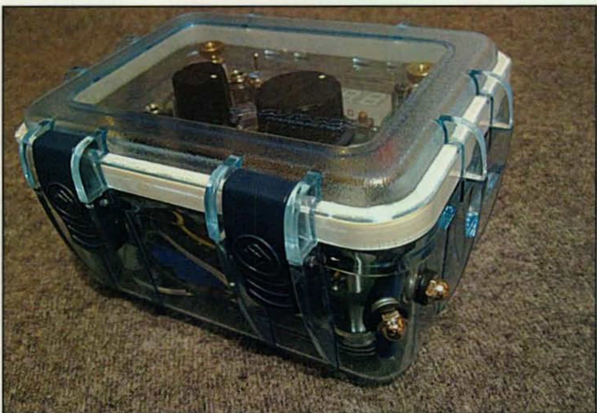
Photo C— The two cap nuts on the SW-20 are the contacts for the keyer-touch paddle.
