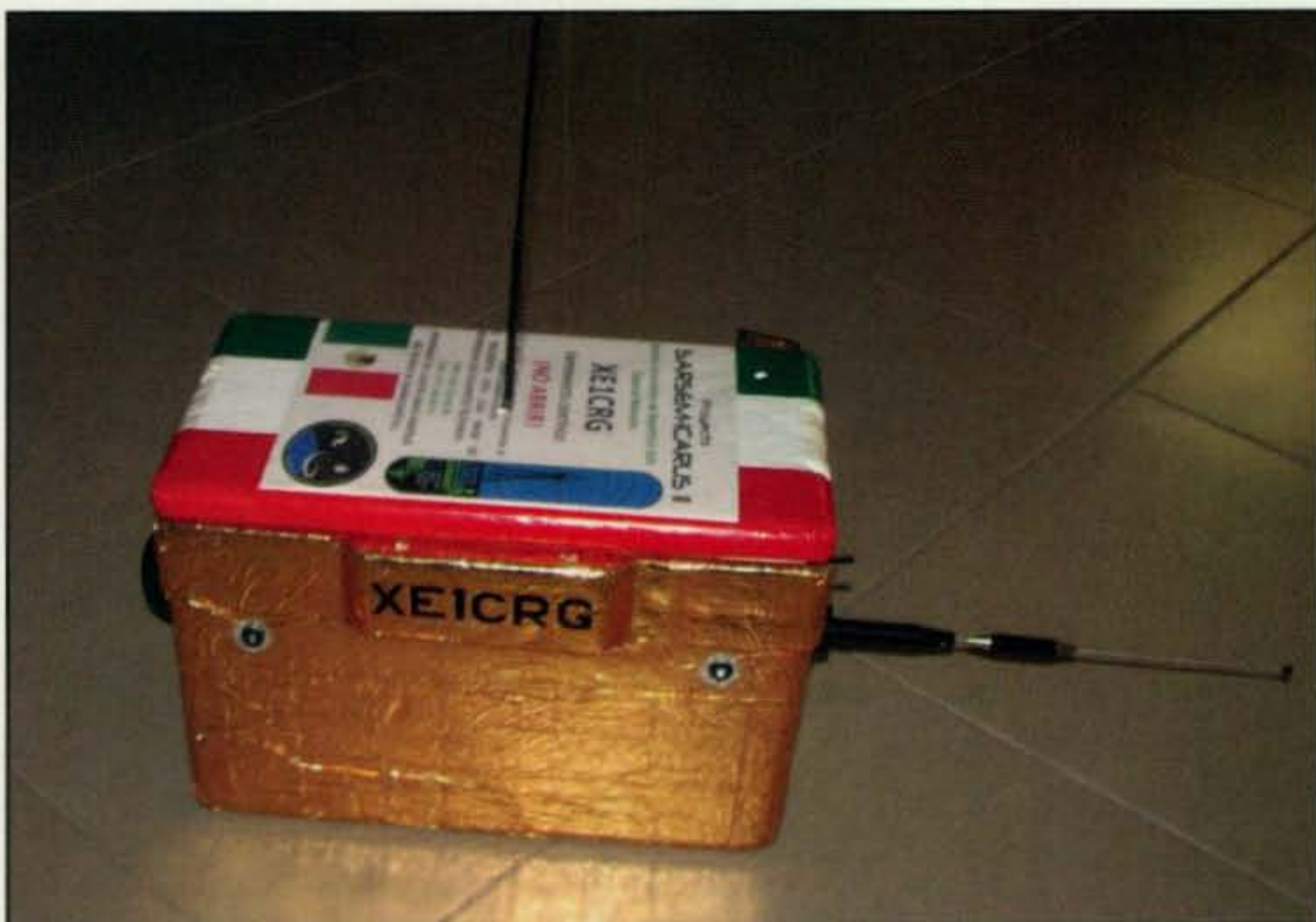
Photo F.—The SARSEM-ICARUS II capsule (Aerostatic Sub-Space Repeater) as successfully flown in November 2010.
