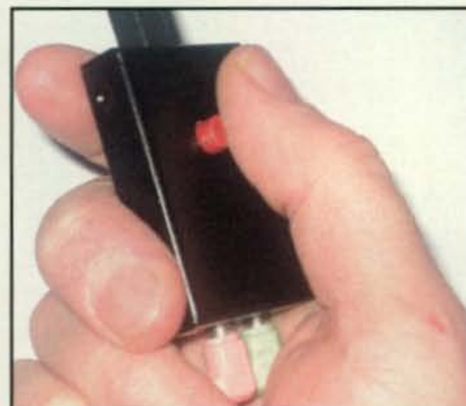
The latest version of laptop-based Remote employs an RRC PC Client which packages the needed software, audio codec, and PTT function into one slick unit the size of a USB memory stick. You just have to download the radio software from the web and you will be in control of your radio wherever you are.
