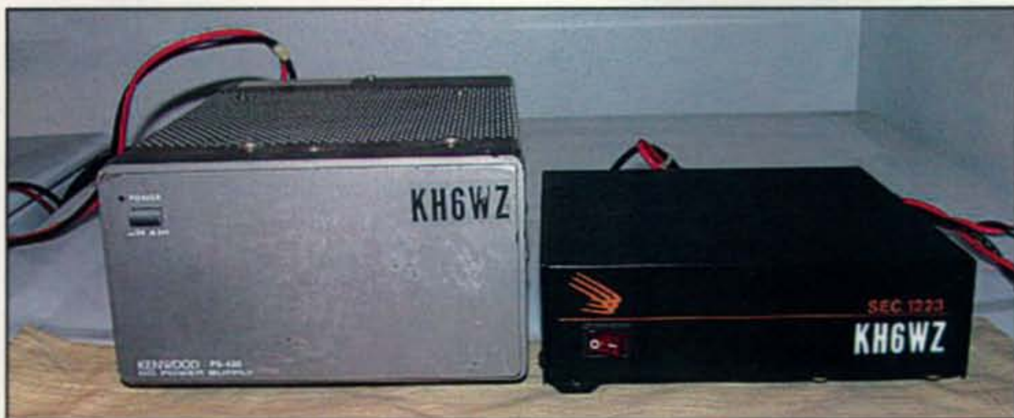
Photo G— Guess which power supply is the SMPS (switching mode power supply). Switchers are smaller, lighter, and run cooler than linear regulated power supplies. They can save energy, too.
