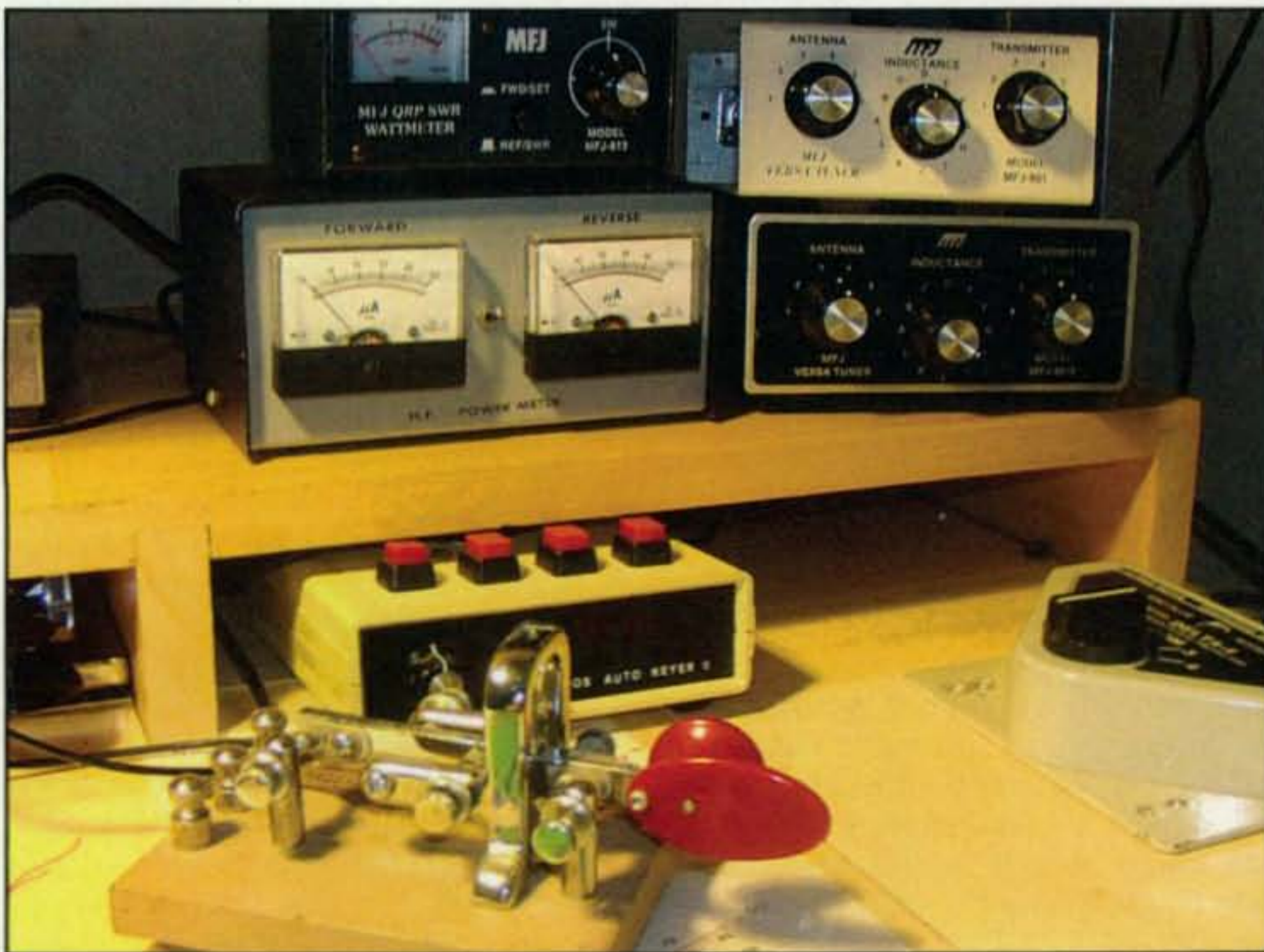
Photo D— This is the ATU/switching system at K7SZ. The top MFJ model 901 tuner controls the Mega-Loop, while the bottom MFJ Model 901B tuner controls the 40-meter EDZ. The antenna switch to the right lets me choose between the Mega-Loop, EDZ, and the MFJ 40/80M vertical.
