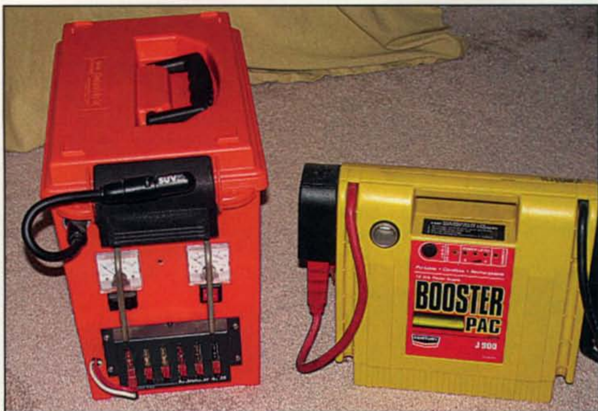
Photo H— This portable power supply (the Orange Box) has appeared in various forms over the years. It is basically a big gel-cell in a handy box with a power supply and battery charger. It is useful for portable operations, and when unplugged from the AC outlet it does not consume any power. The yellow unit next to the Orange Box is a commercially-available unit sold as an emergency automobile jump-start power source. (See sidebar for more on the Orange Box.)
