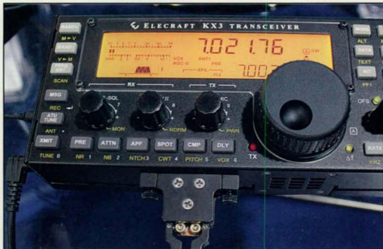
*Prototype of the new Elecraft KX-3 portable all-mode transceiver kit.*
