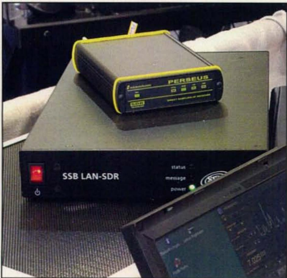
Photo E—SSB Electronic from Germany introduced the new SSB-LAN SDR (software defined radio) receiver this year, which you can operate through your computer anywhere on your home WiFi network, as well as a software upgrade to the Perseus receiver, also seen here.
