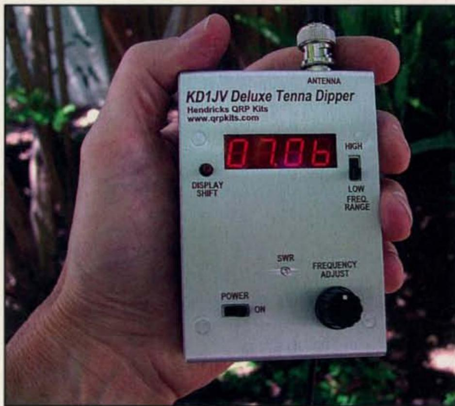
Photo B— The Deluxe Tenna Dipper from Hendricks QRP Kits, showing that the attached antenna is resonant at 7.060 MHz.
