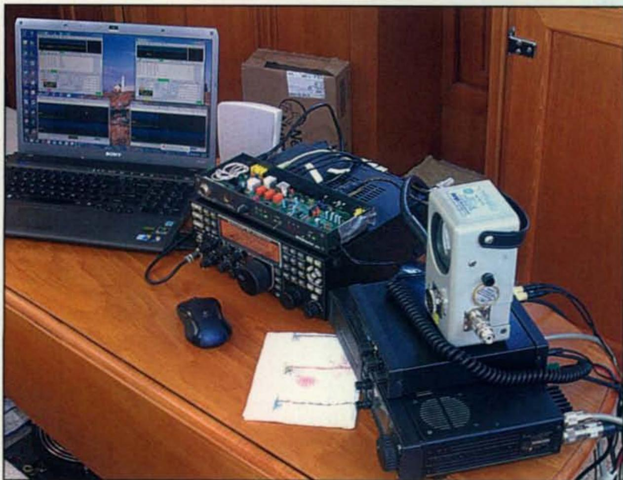
KS7DX—two versions of WSJT running, V7 on the left and V9 on the right. The ICOM 706MKII G is running HF and 2 meters. The 6-meter antenna is in use on the upper deck, which is why there is an open port on the Bird wattmeter. The duct tape on the side of the RigBlaster is for an emergency repair for the power supply.
