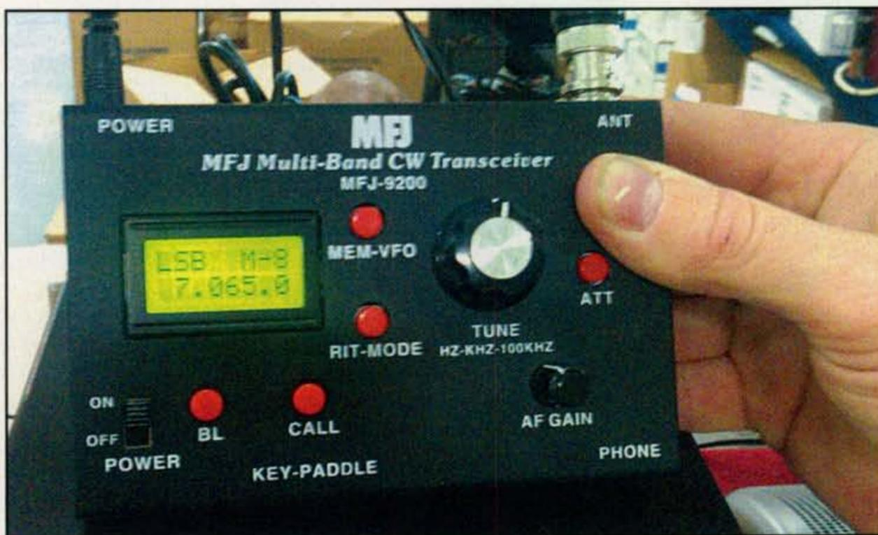
Photo D— MFJ is moving from its single-band QRP (low-power) rigs to the MFJ-9200 "QR-Pocket" transceiver. It operates one band at a time, but you can change bands by swapping out band modules.
