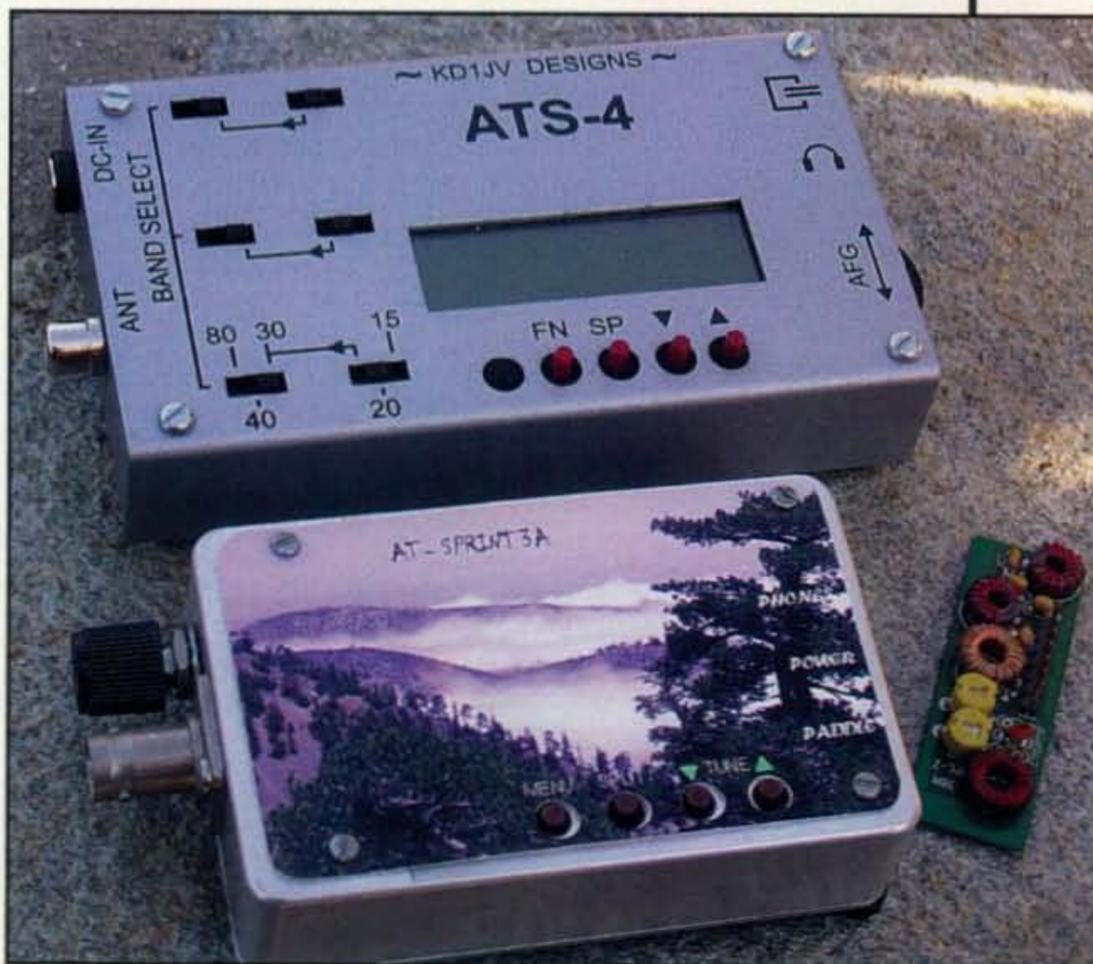
Photo A— The Altoids®-size ATS-3A with one of its band modules shown beside the newer ATS-4, which trades the modules for internal switching.
