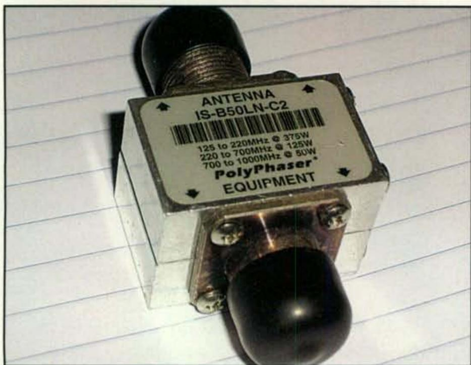
This is a PolyPhaser VHF/UHF surge protector for your antenna feedline. It will protect your gear from induced currents from static discharge and nearby lightning, but not from a direct strike.
