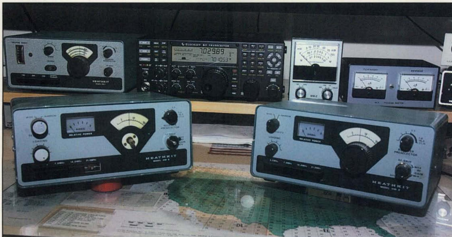
Photo D— Two Heathkit HW-8s on the author's bench. The grungy-looking one is being restored, using parts from the nicer-looking (but not repairable) "parts rig."
