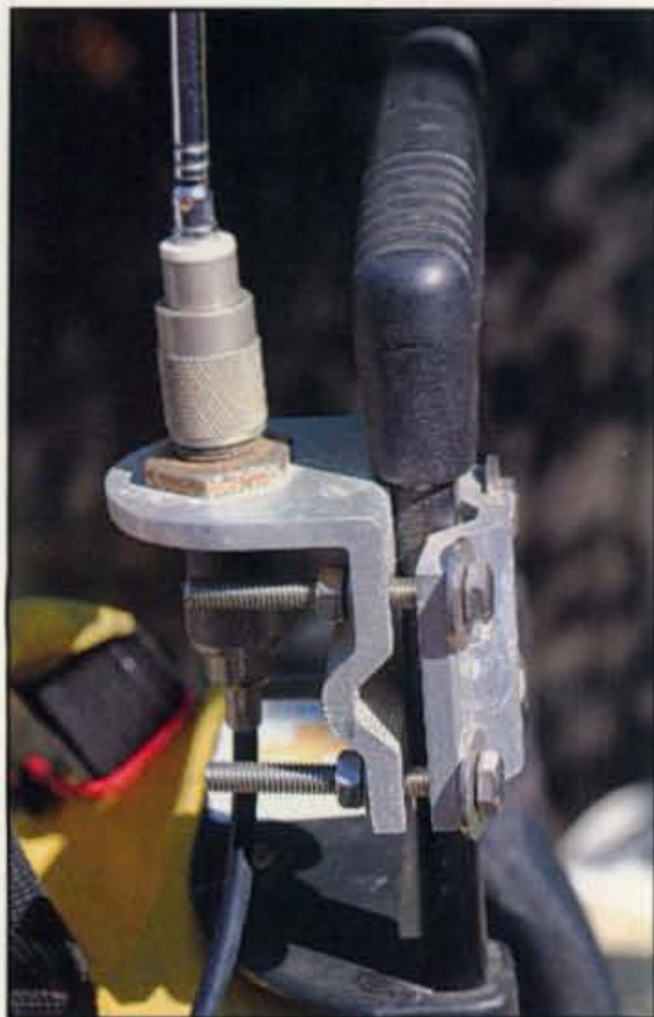
Photo D— An L-bracket designed for a mirror-mount antenna on a truck can attach to the pull-up handle on the roller bag and either support a small antenna or provide a connection point for coax leading to an externally mounted antenna.
