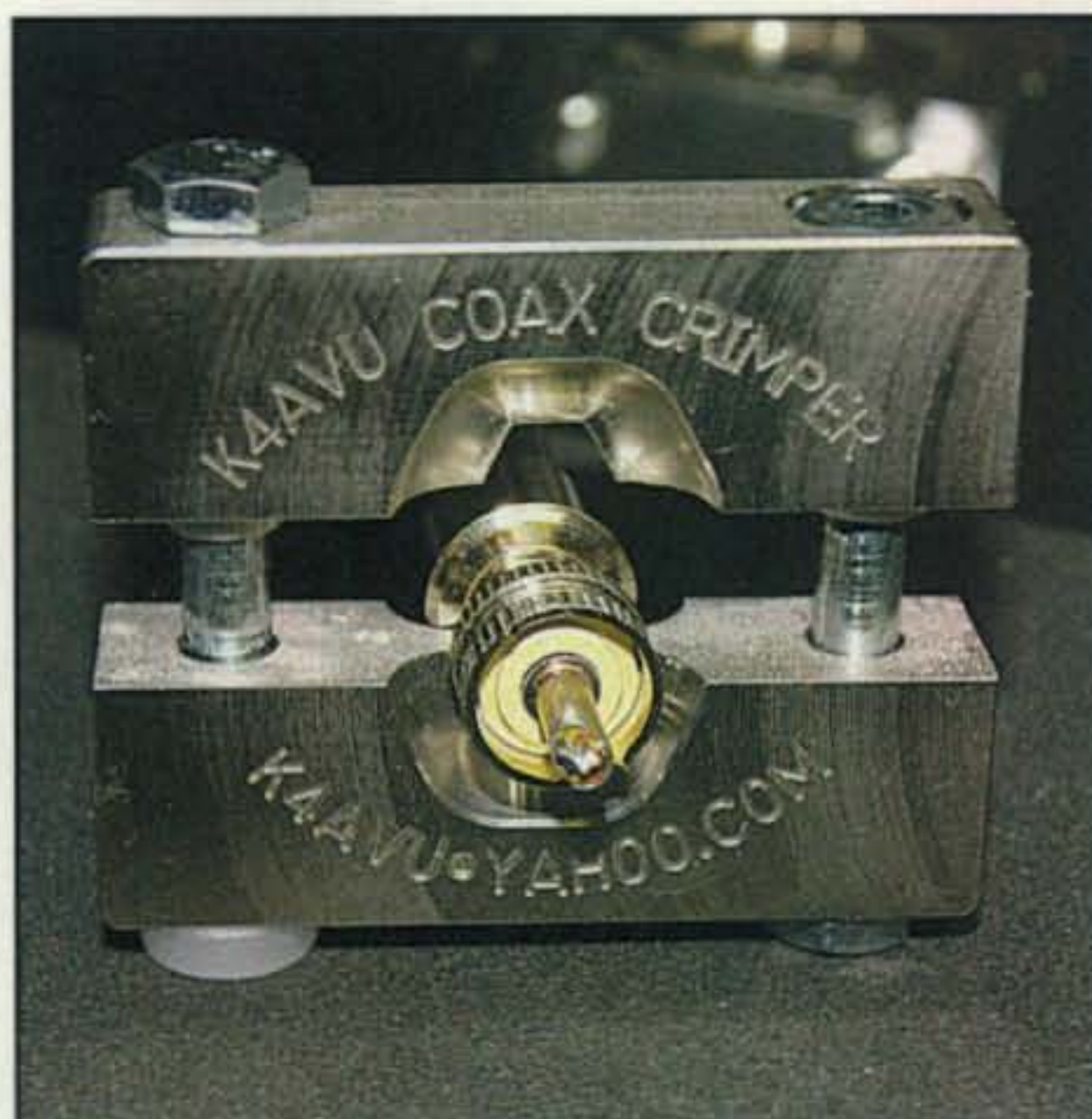
Photo A— K4AVU has brightened your world and his with an improved 303 stainless steel version of the Coax Crimper.
