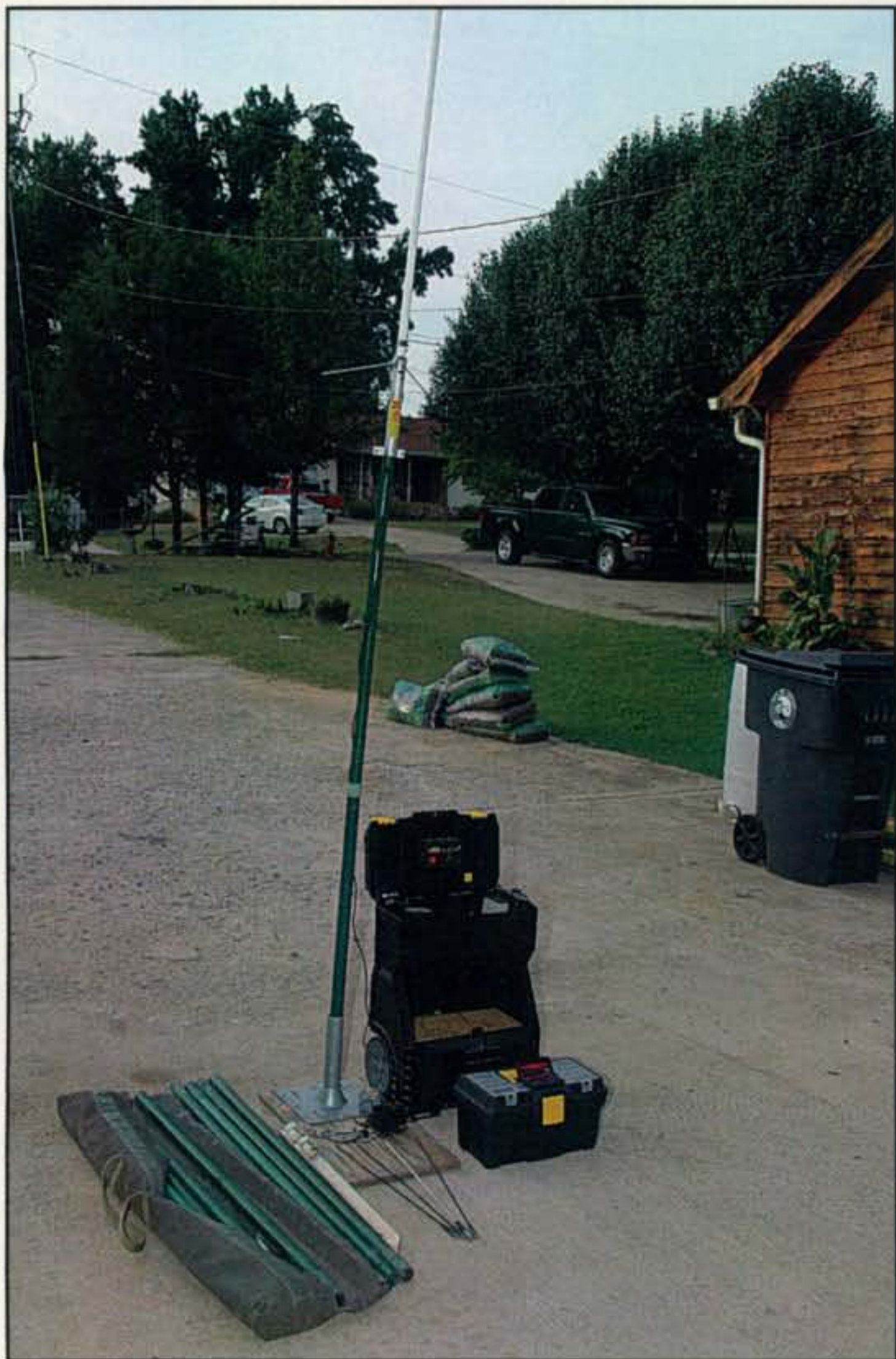
The Go-Radios are housed in a Stanley™ mobile work center; batteries are in the lower compartment. Additional batteries (four 7-amp/hr gell-cells) are housed in a Stanley™ toolbox. Also included is a small digital volt/ohm/milliammeter. The homebrew antenna mount is to the immediate left of the radio container. The green fiberglass mast set is shown along with the primary VHF/UHF antenna, a Diamond X-50A (on the short green mast).
