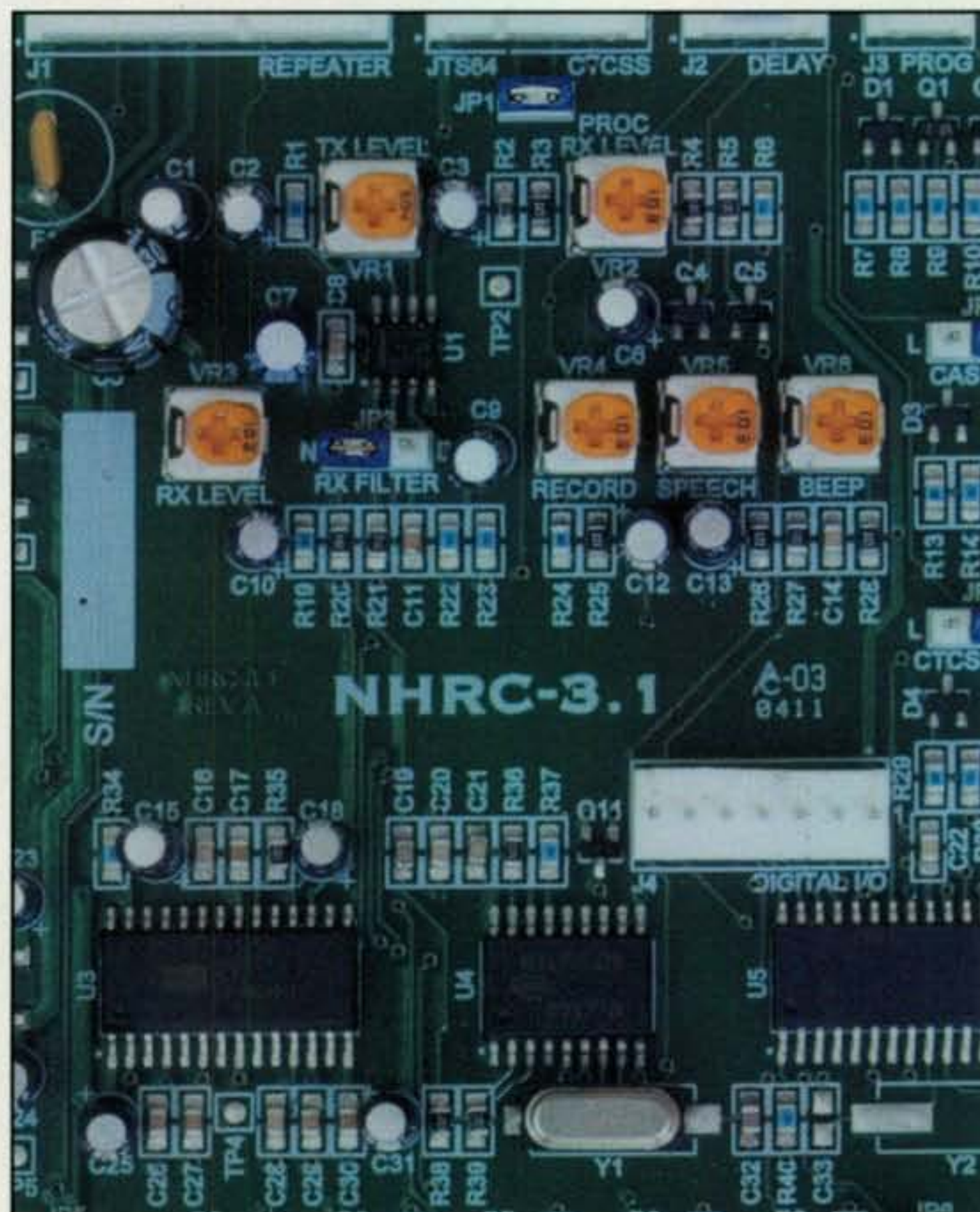
Photo C—NHRC has come out with version 3.1 of its repeater controller which comes with stored speech.
