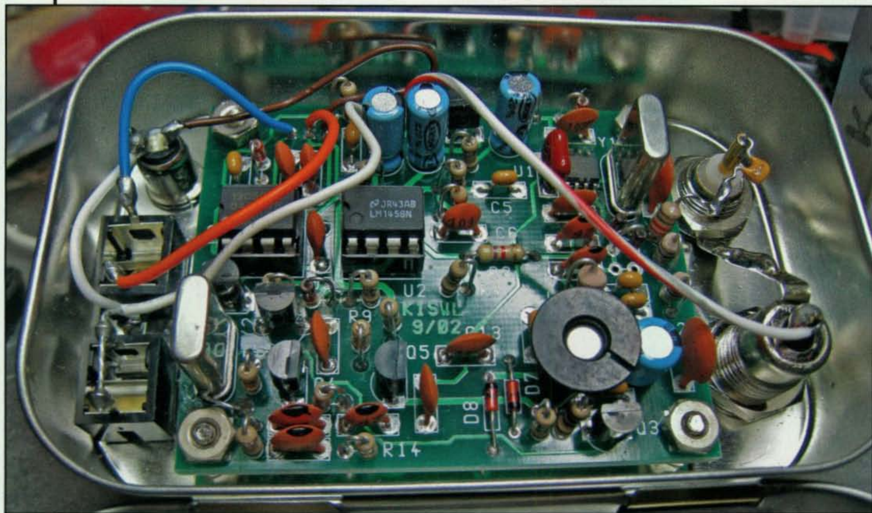
Small Wonder Labs RockMite in mint tin. Notice most of the resistors are mounted upright.
