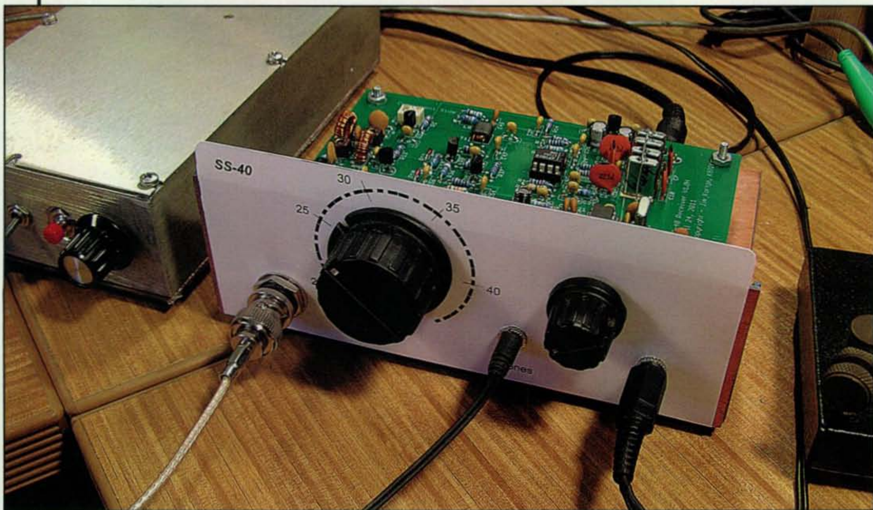
The Four State QRP Group's SS-40 receiver, mounted in an N6GA Quickie-Almost-Box.
