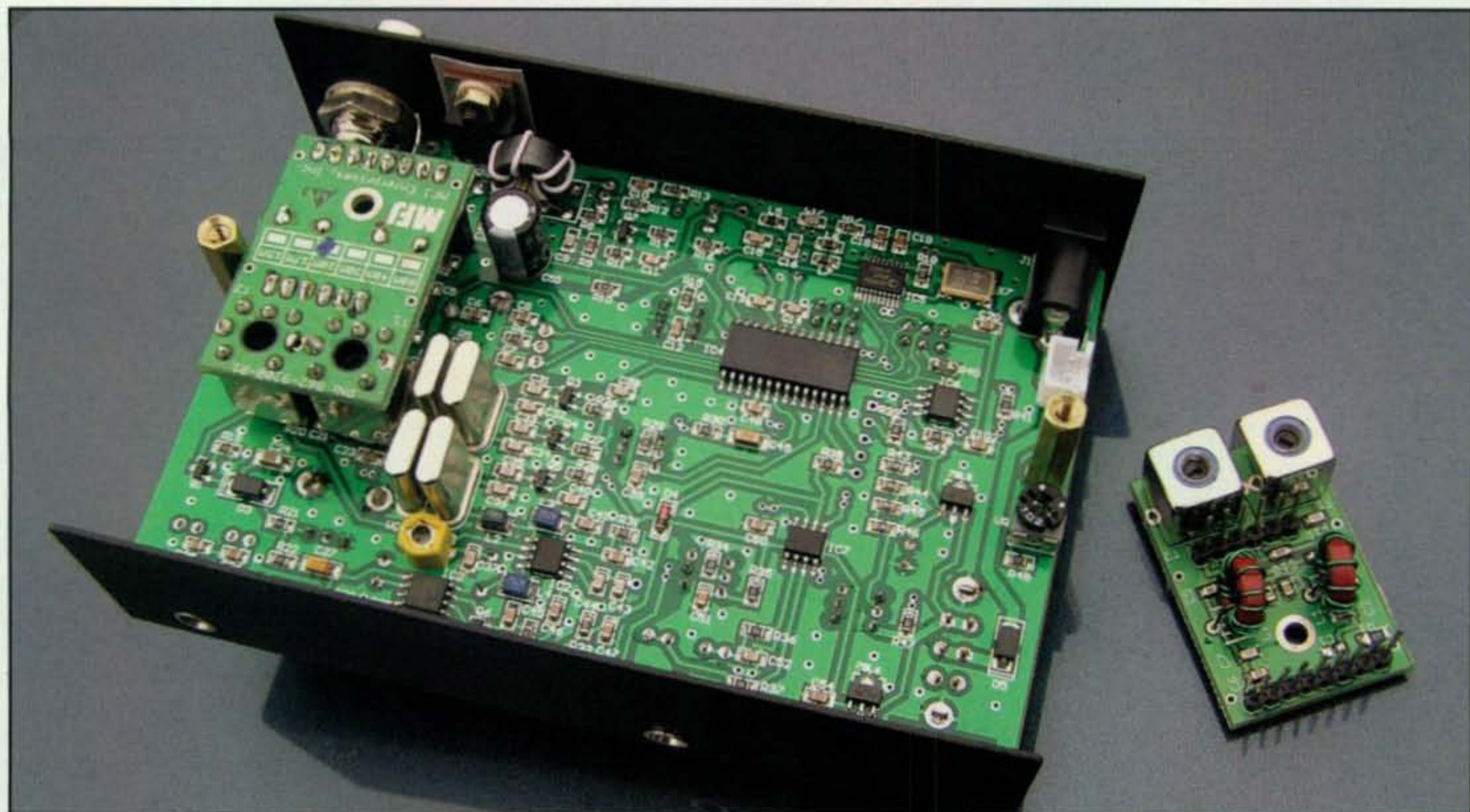
MFJ-9200 with its back off, ready for a band change. The board to the right is one of the band modules.
