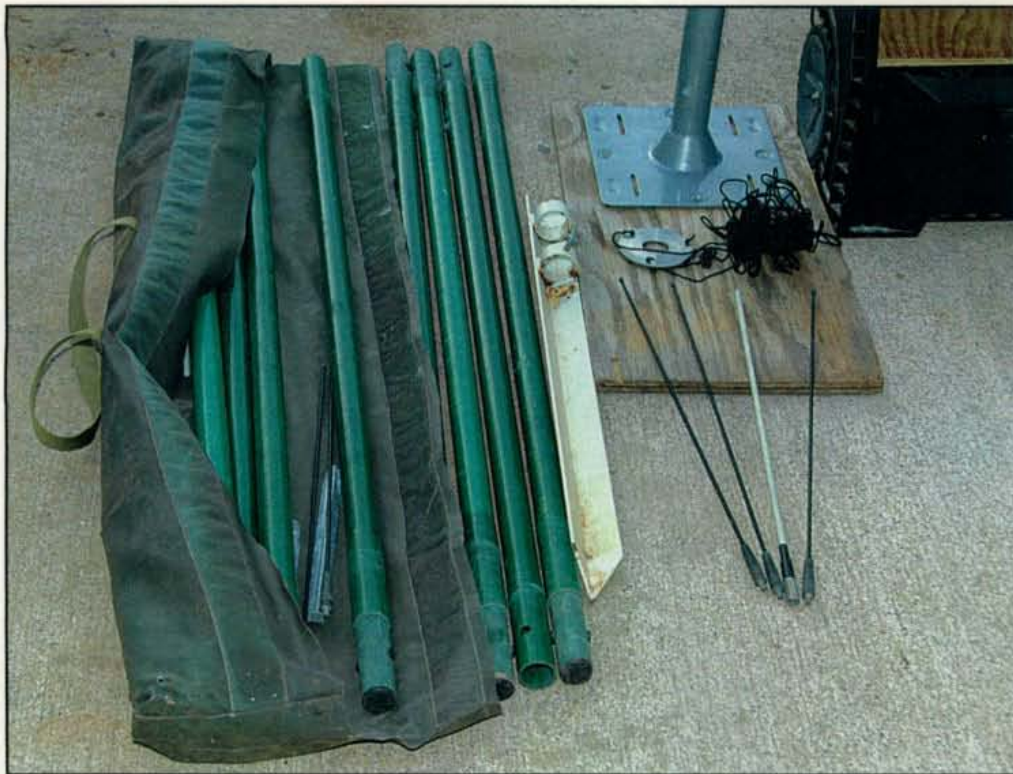
This illustration shows a close-up of the fiberglass mast and antenna system that I procured from Fair Radio Sales about four years ago. The poles snap together, and I have enough 4-foot poles to erect a 32-foot mast! The original antenna that came with the mast system has been cut down to resonate on 2 meters. The main radiating element (white) and the three radials (black) screw into an insulator complete with a 20-ft. length of RG-58 terminated in a BNC connector to fit the radio. Shown also is a ground stake (white angle iron) that can be driven into the dirt if you lack any other form of antenna mount.
