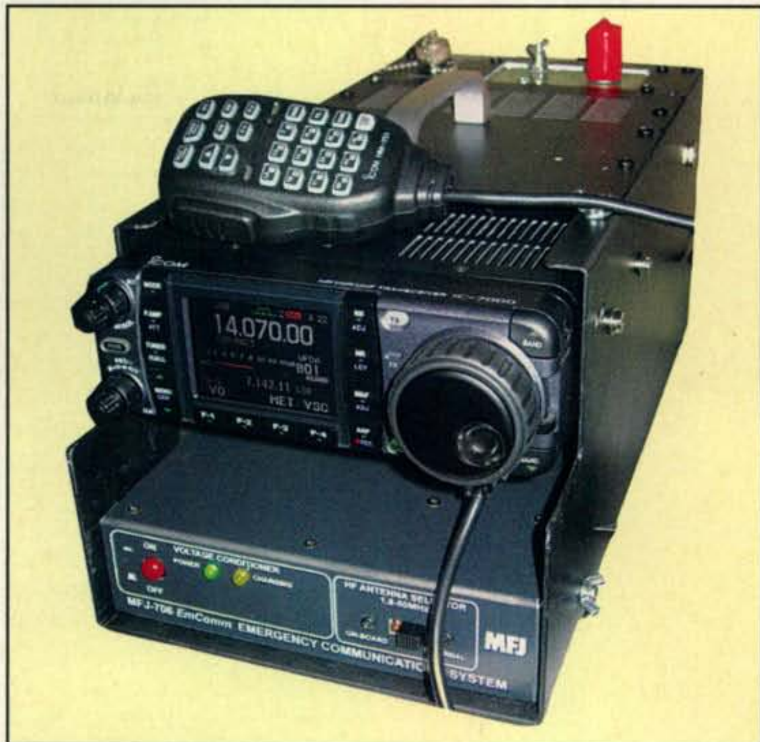
Photo C— The MFJ-7000 is an EmComm box that turns the ICOM IC-7000 into an instant and foolproof portable/mobile emergency communications center. It covers all HF, VHF, and UHF amateur radio frequencies available on the IC-7000.
