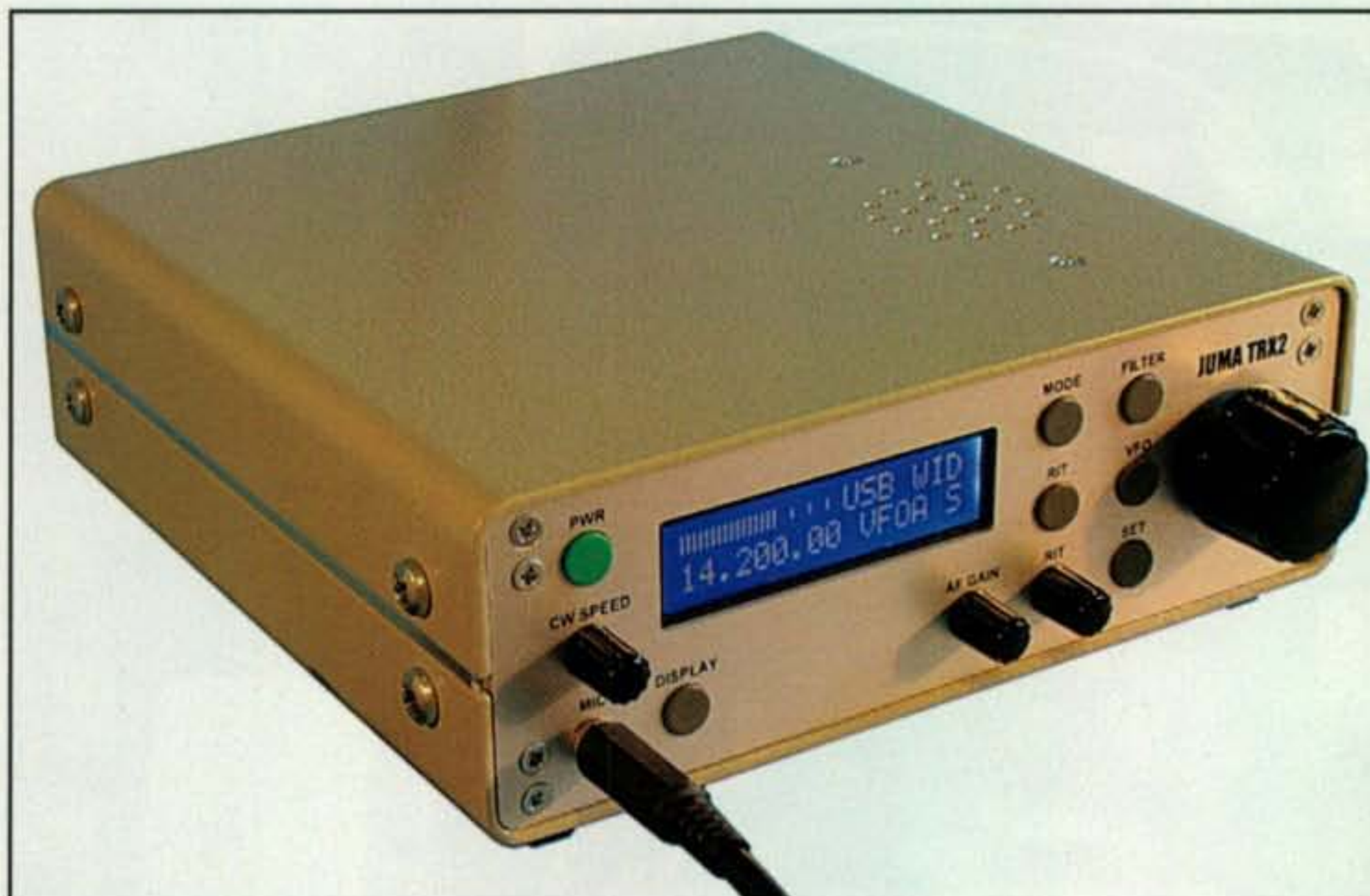
Photo B— The JUMA TRX-2A, a compact 160- through 10-meter, 10-watt, CW and SSB transceiver.
