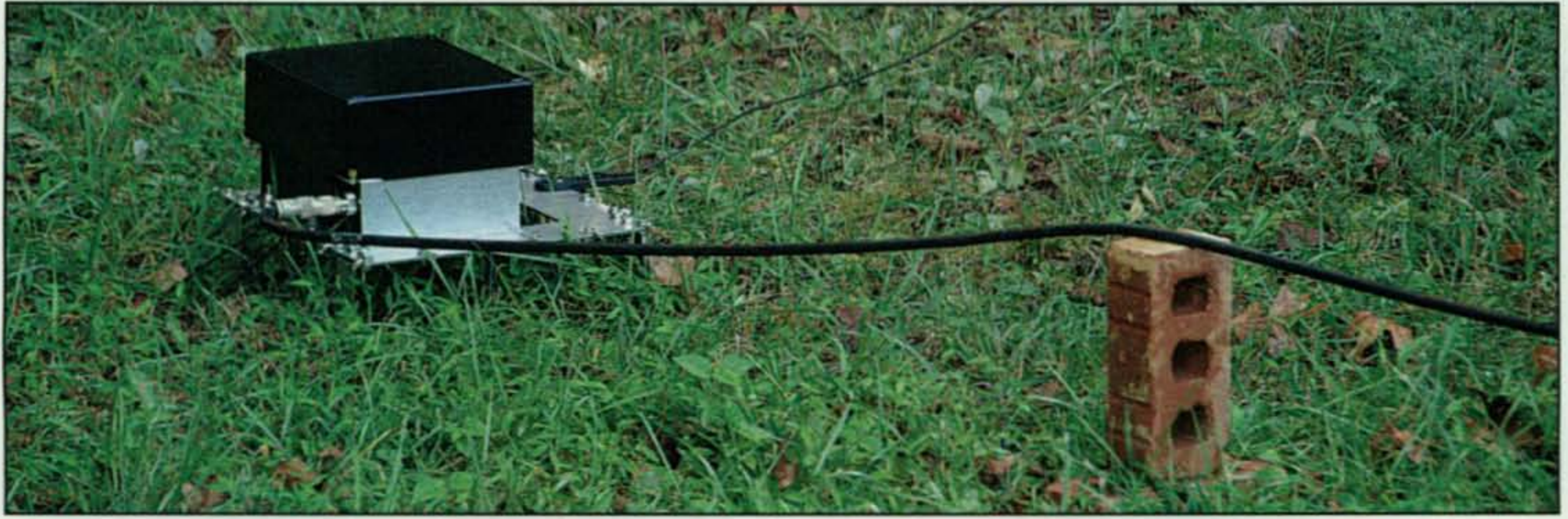
This is a closer shot of the ATSA-1 tuning unit taken from only 10 feet away. Notice that you can barely see the vertical wire extending upward from the left of the unit just above the coaxial cable. From a few feet farther away the vertical radiating element is totally invisible. Talk about "stealth"!
