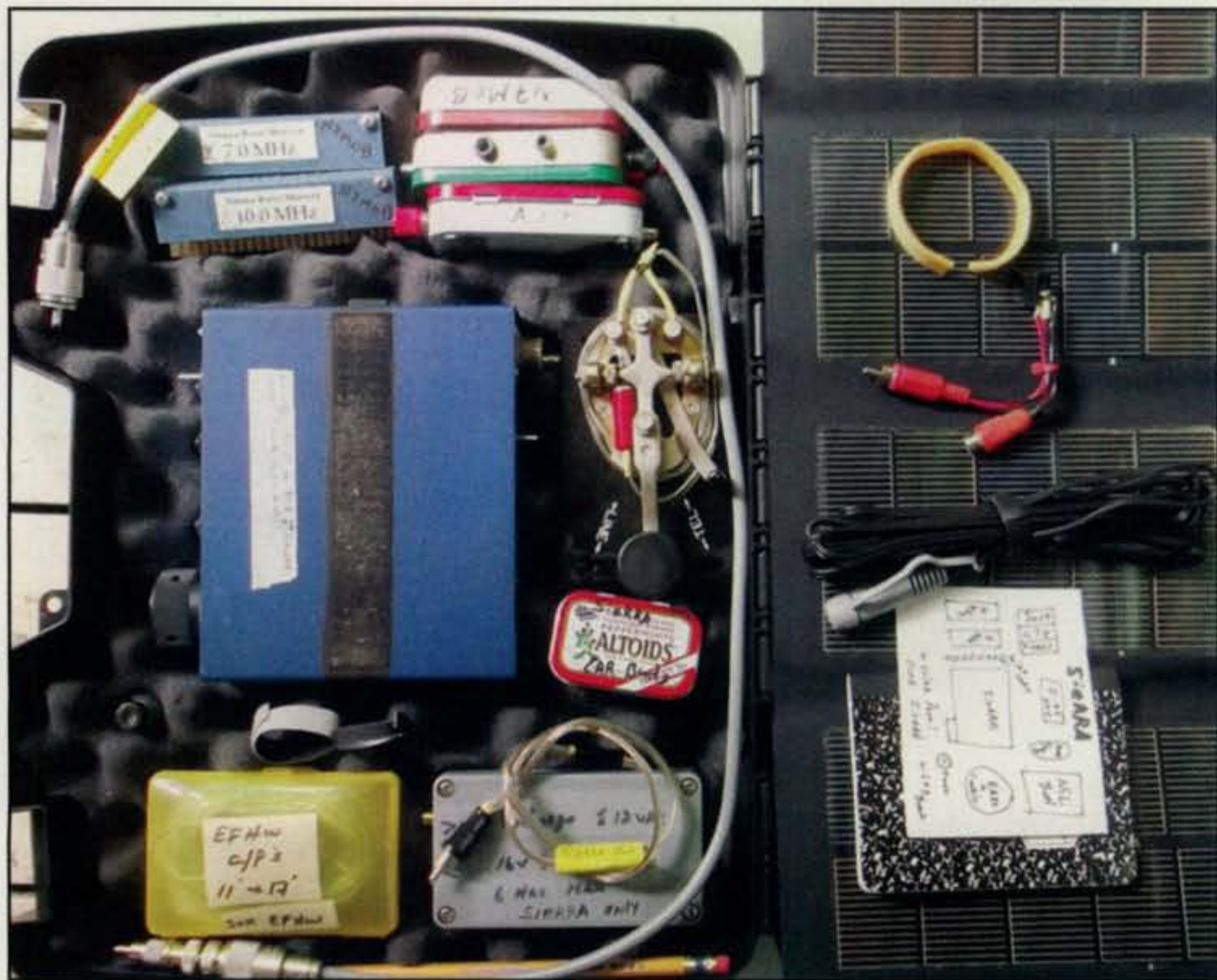
Photo A—N7MOB's QRP station in a padded case. Besides the Sierra he includes batteries, two antennas, two tuners, a key, earbuds, and a folding solar panel.
