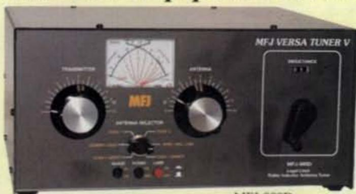
New, improved MFJ-989D legal limit antenna tuner gives you better efficiency, lower losses and a new true peak reading meter with no price increase. Easily handles full 1500 Watts SSB/CW over 1.8-30 MHz. New dual 500 pF air variable capacitors give you twice the capaci-
