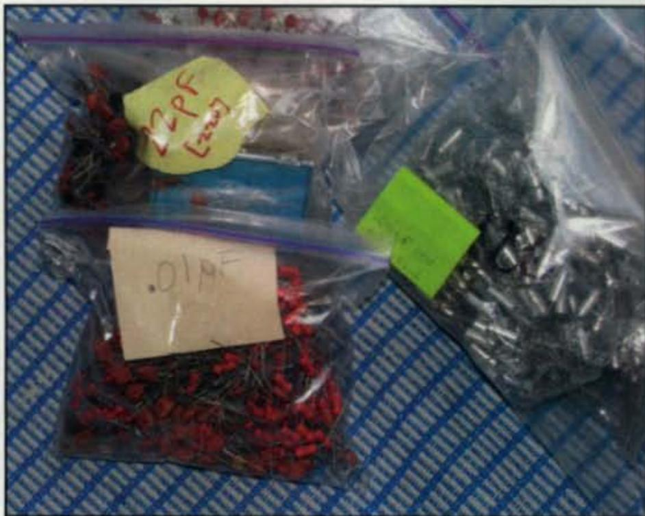
Photo 8— Plastic zipper-top bags can be used to store lots of different small parts, such as transistors and capacitors.
