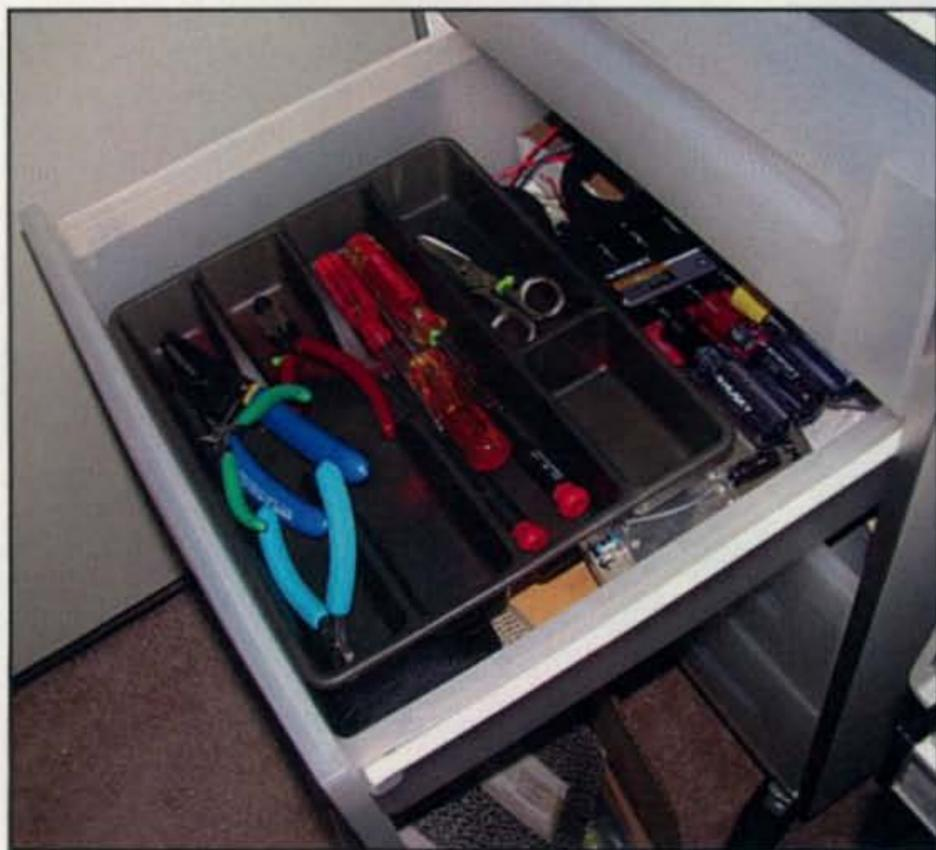
Photo 3— These plastic silverware trays are an example of "set in order." Small hand tools are placed in compartments, rather than jumbled into a single tray. An even better solution would be to have each tool fit into its own cut-out within the tray.
