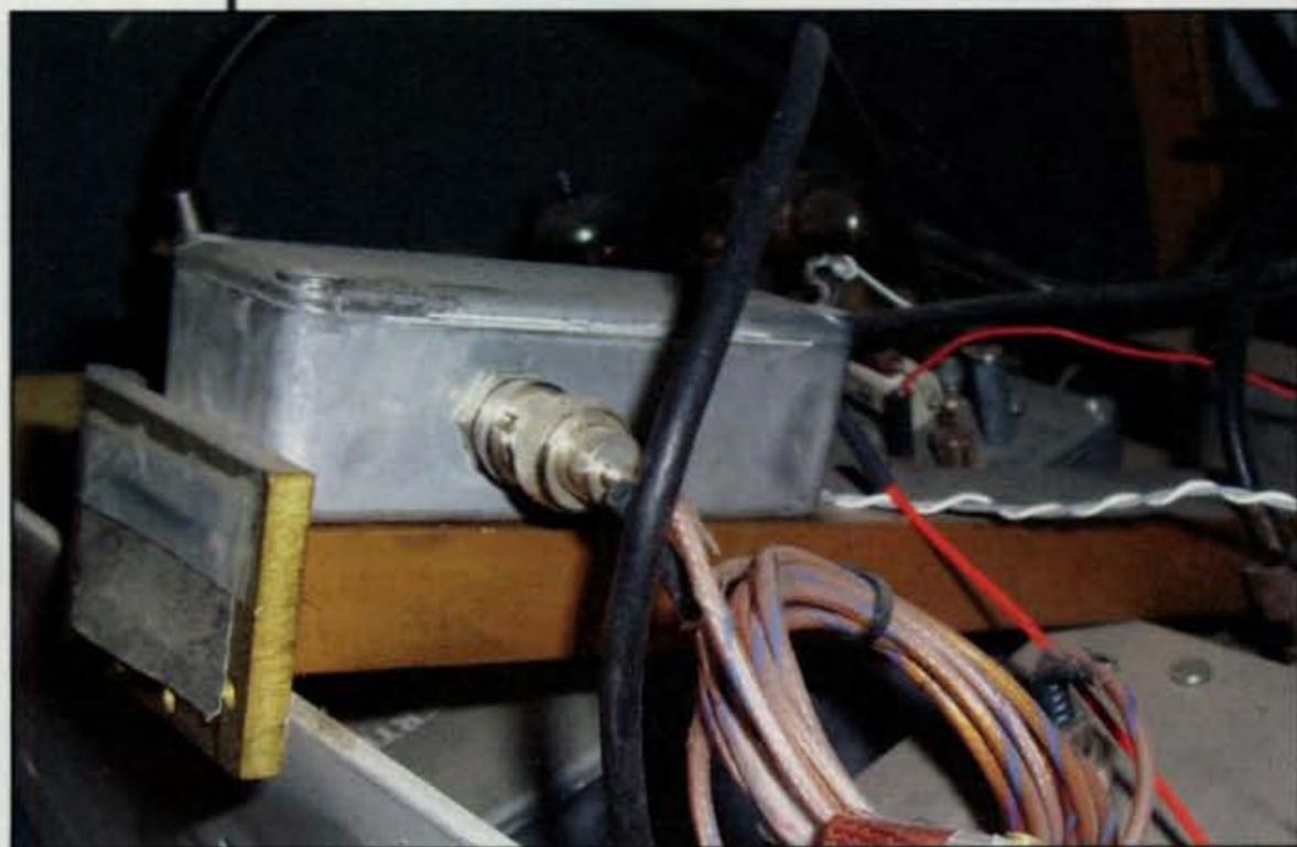
Photo A— Preamp with an input SWR > infinity!
