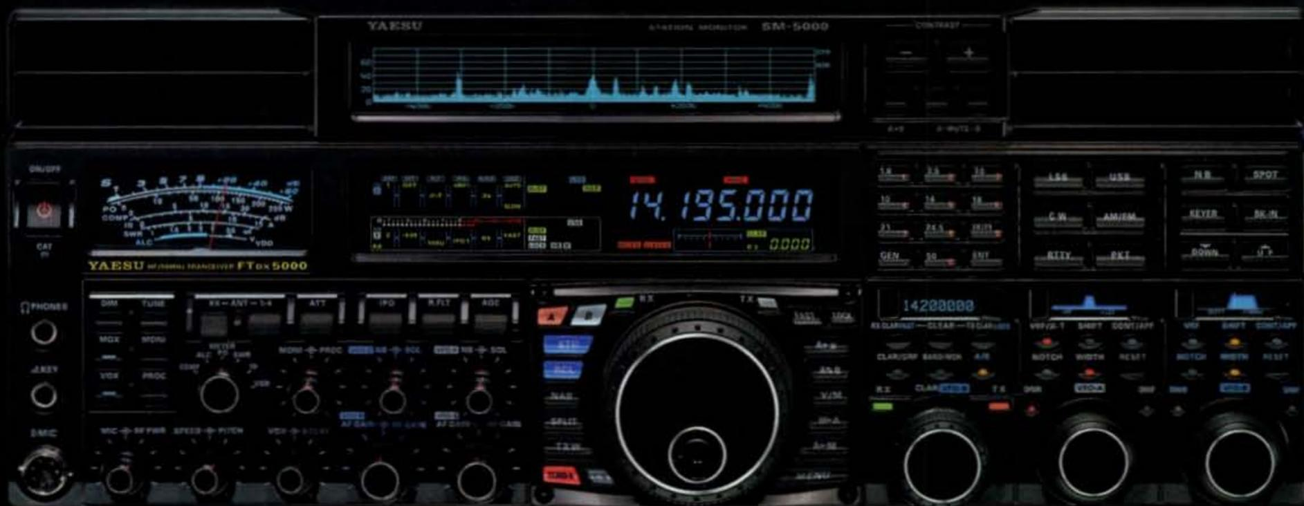
**Two Totally Independent Receivers - The VFO-A/Main Receiver utilizes Super Sharp Roofing filters to give you the highest performance and best flexibility**
