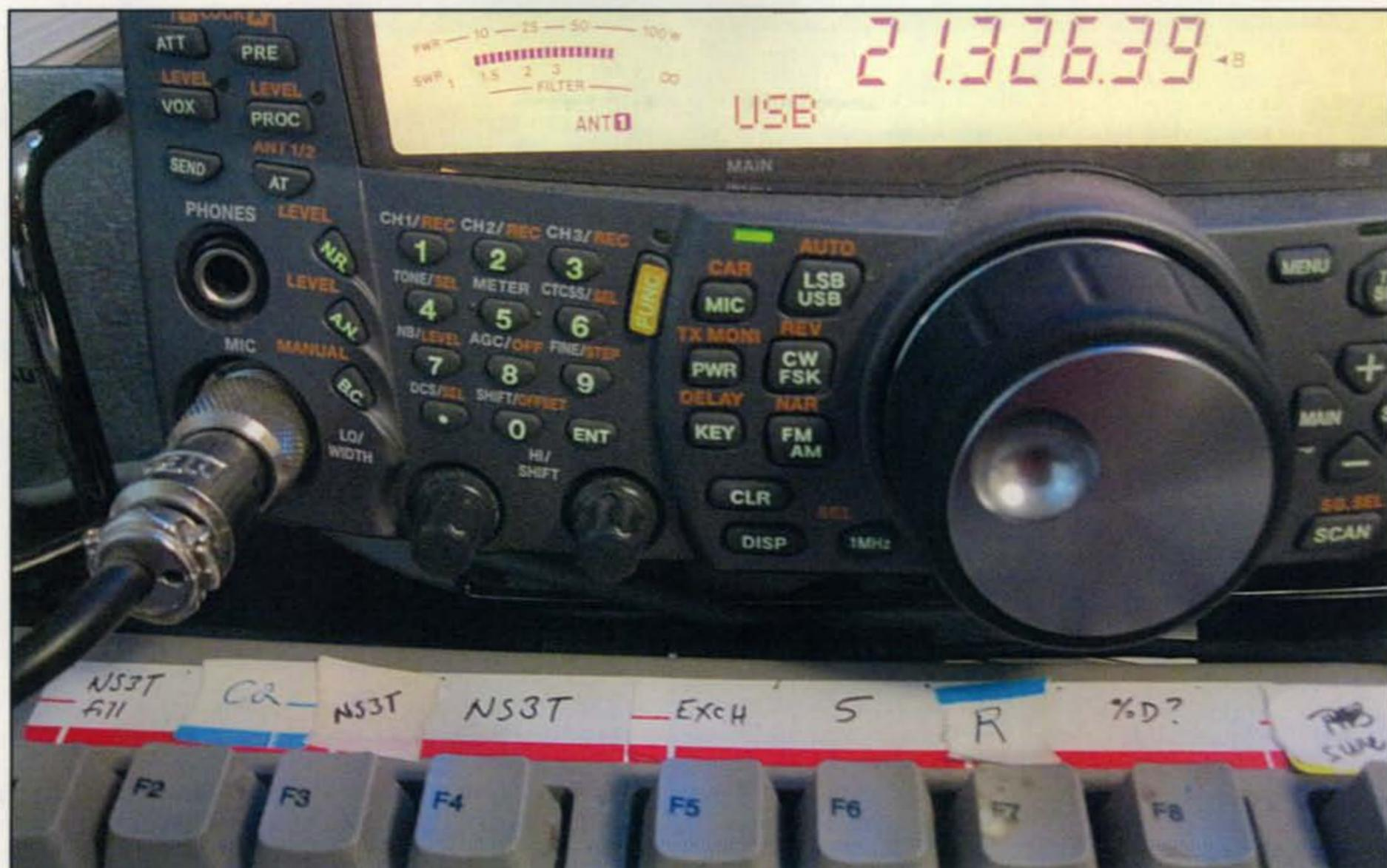
Closeup of Jamie's number-one radio and computer keyboard. The audio from his computer is fed into the rig's mic jack. Note that the function keys each are labeled for a different segment of contest exchange.
