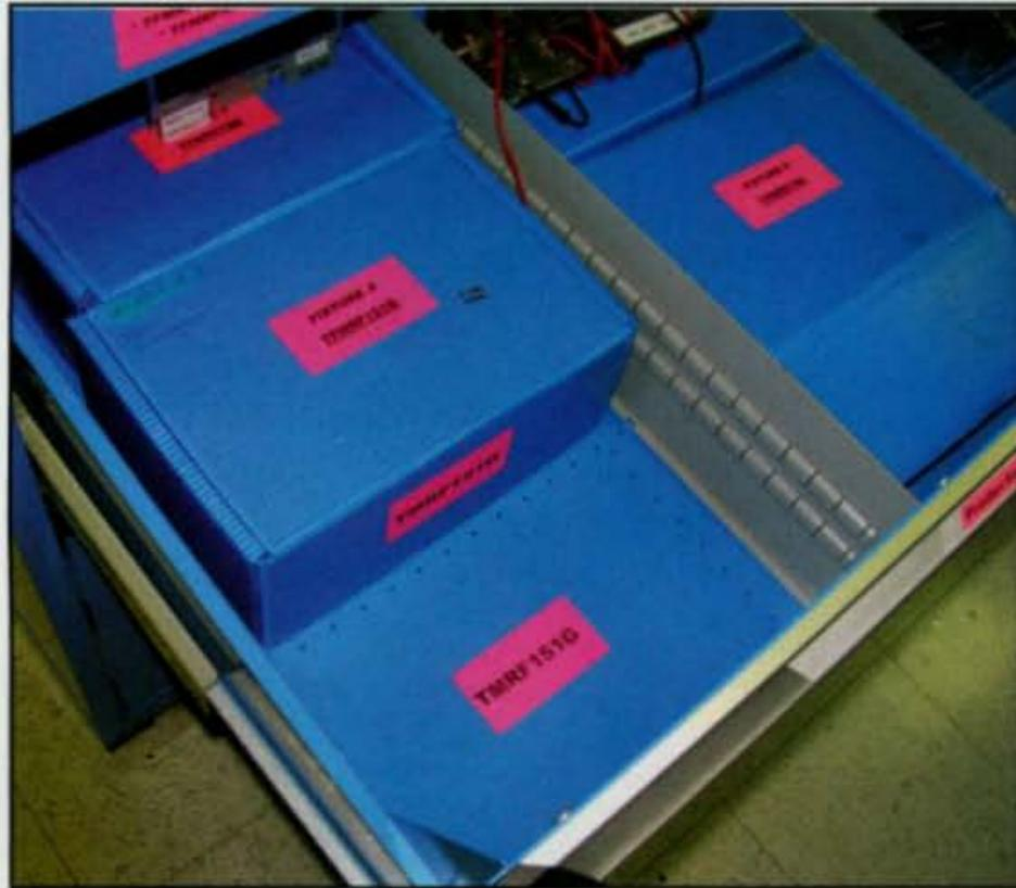
Photo 5— Each test fixture is further organized into an individual storage box within the drawer. Can you see the open space on the bottom left? Each space is marked, so everyone knows “TMRF151G” is in use on the factory floor.
