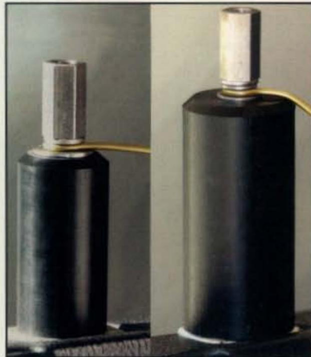
Photo E— GeoTool is also bringing to market two new Delrin insulators which provide a wide gap to reduce the resonant-frequency-raising capacitance between the bottom of the antenna and the mount.
