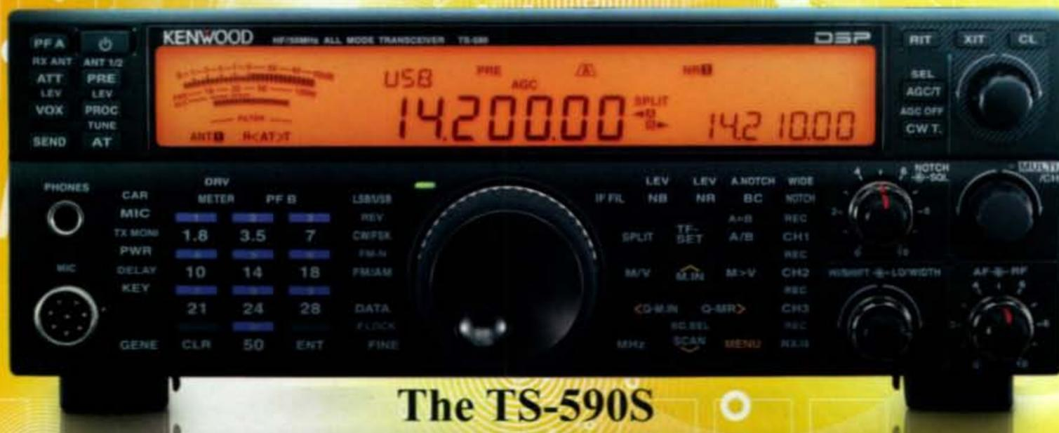
Kenwood has essentially redefined HF performance with the TS-590S compact HF transceiver. The TS-590S RX section sports IMD (intermodulation distortion) characteristics that are on par with those "top of the line" transceivers, not to mention having the best dynamic range in its class when handling unwanted, adjacent off-frequency signals.\*
