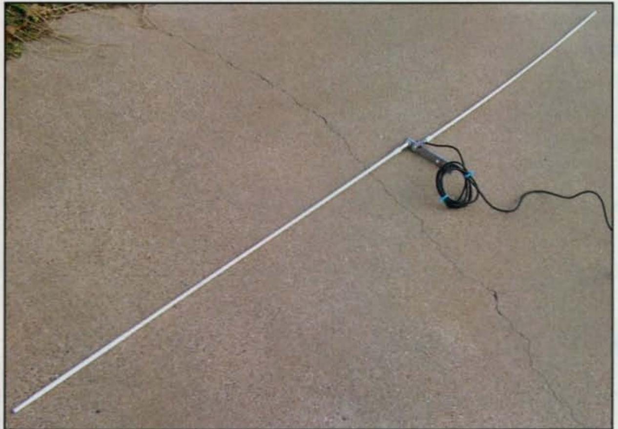
Photo C— Ten-meter portable dipole made from CB whips.
