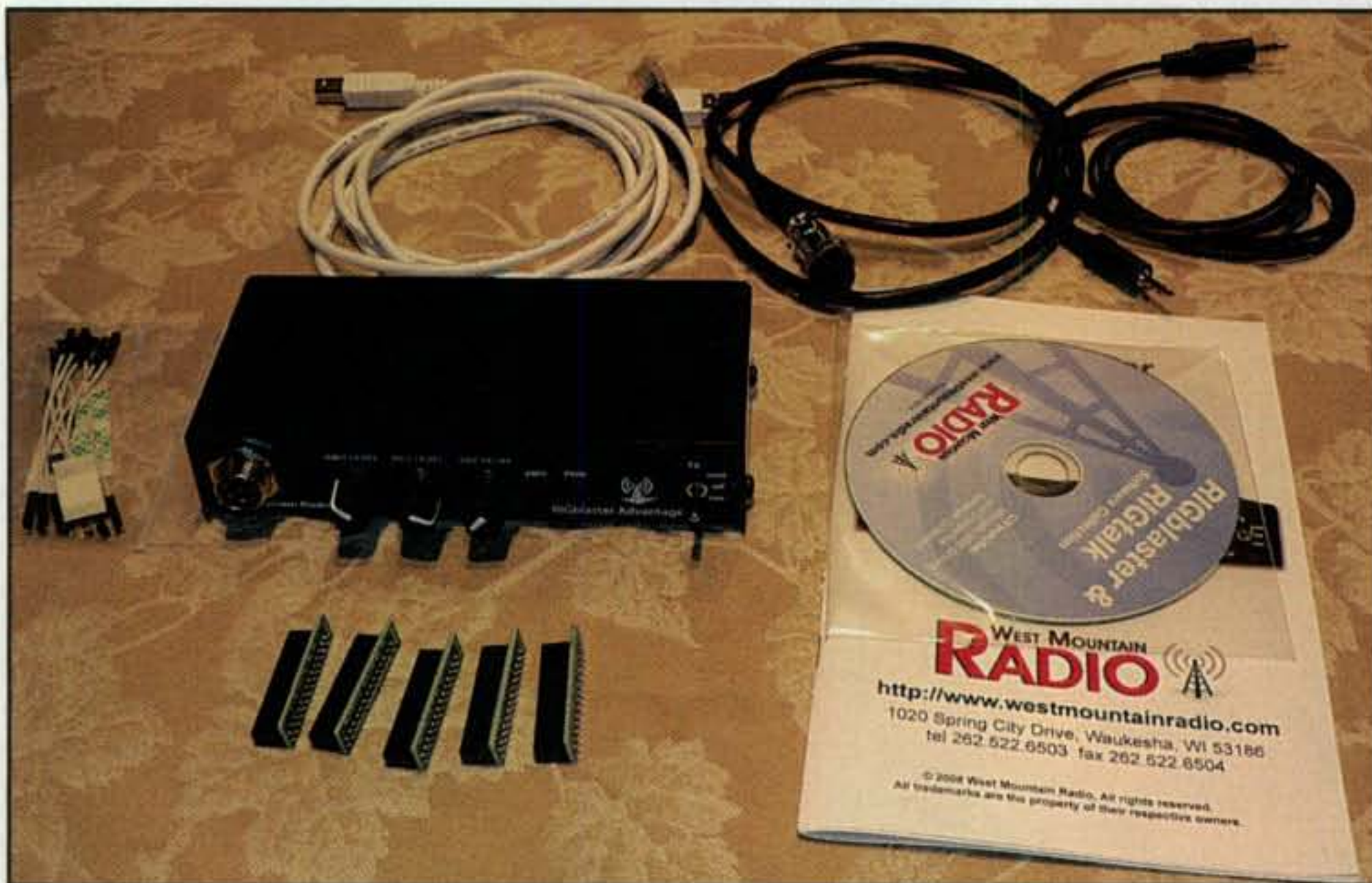
Photo D— The West Mountain Radio RIGblaster Advantage as it first comes out of the box.
