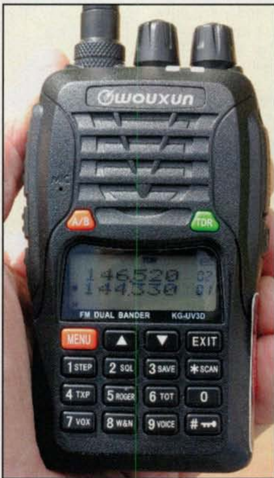
Also joining the U.S. ham market from China is Wouxun KG-UV3D, one of several two-band models from this manufacturer. The KG-UV3D has FCC Part 90 certification.
