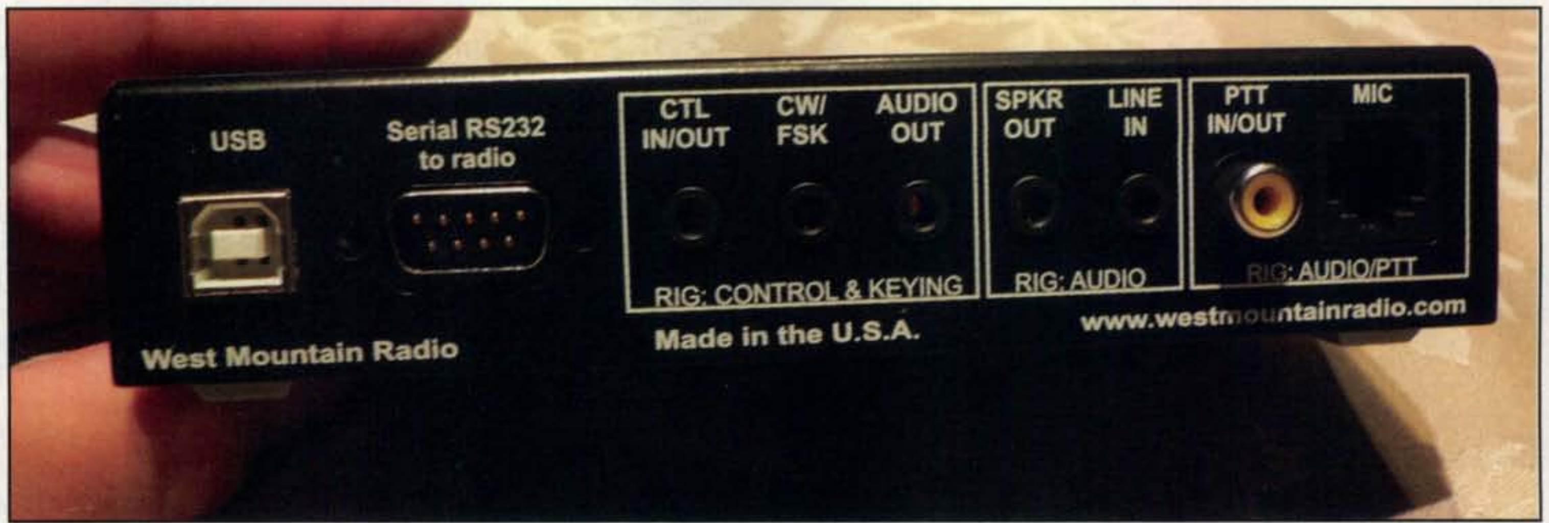
Photo B—Rear panel of the RIGblaster Advantage. Note both USB and serial ports.
