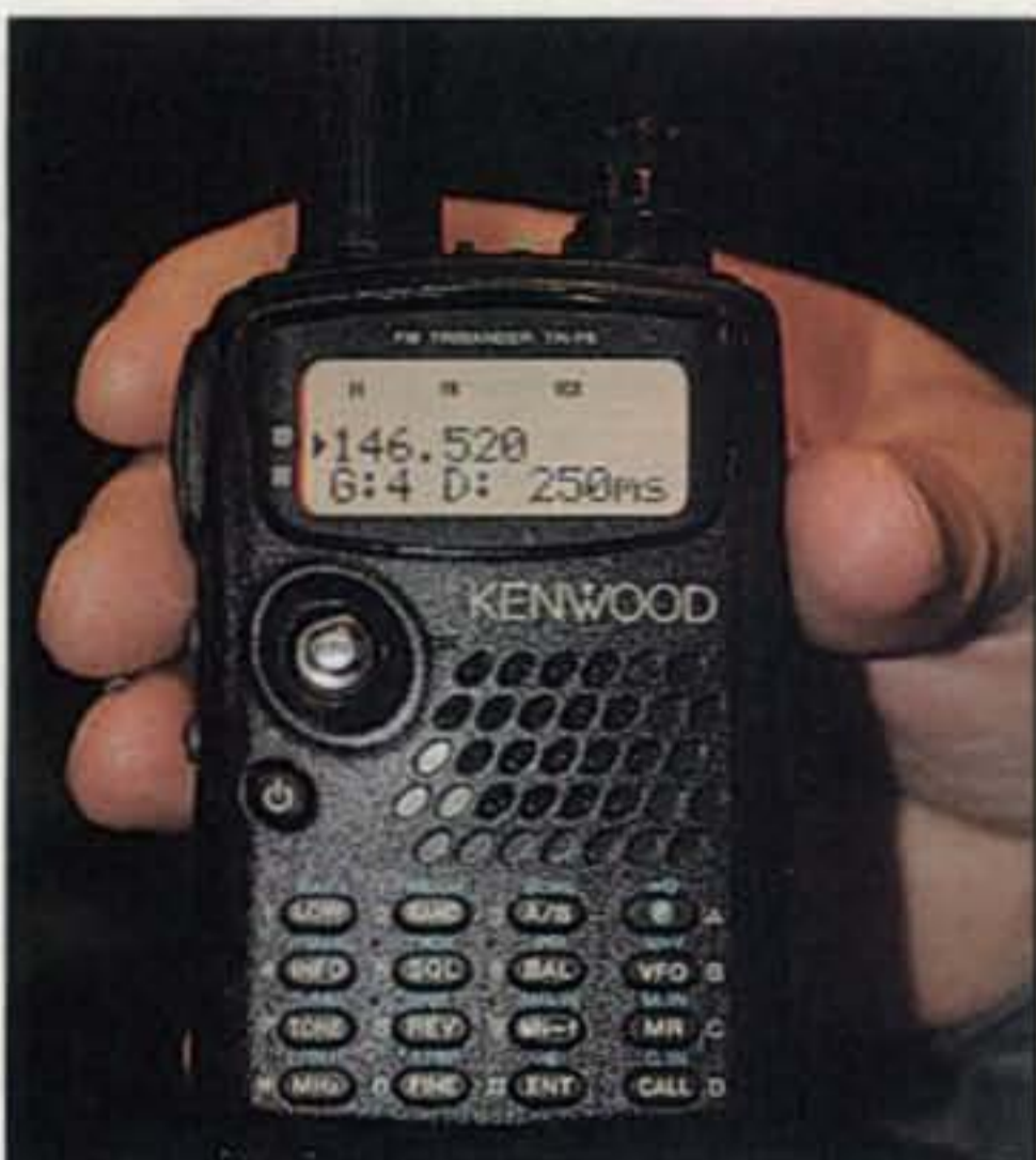
The popular Kenwood TH-F6A covers the 222-MHz band as well as 2 meters and 70 centimeters, with broadband receive (including CW/SSB) from 100 kHz to 1300 MHz.
