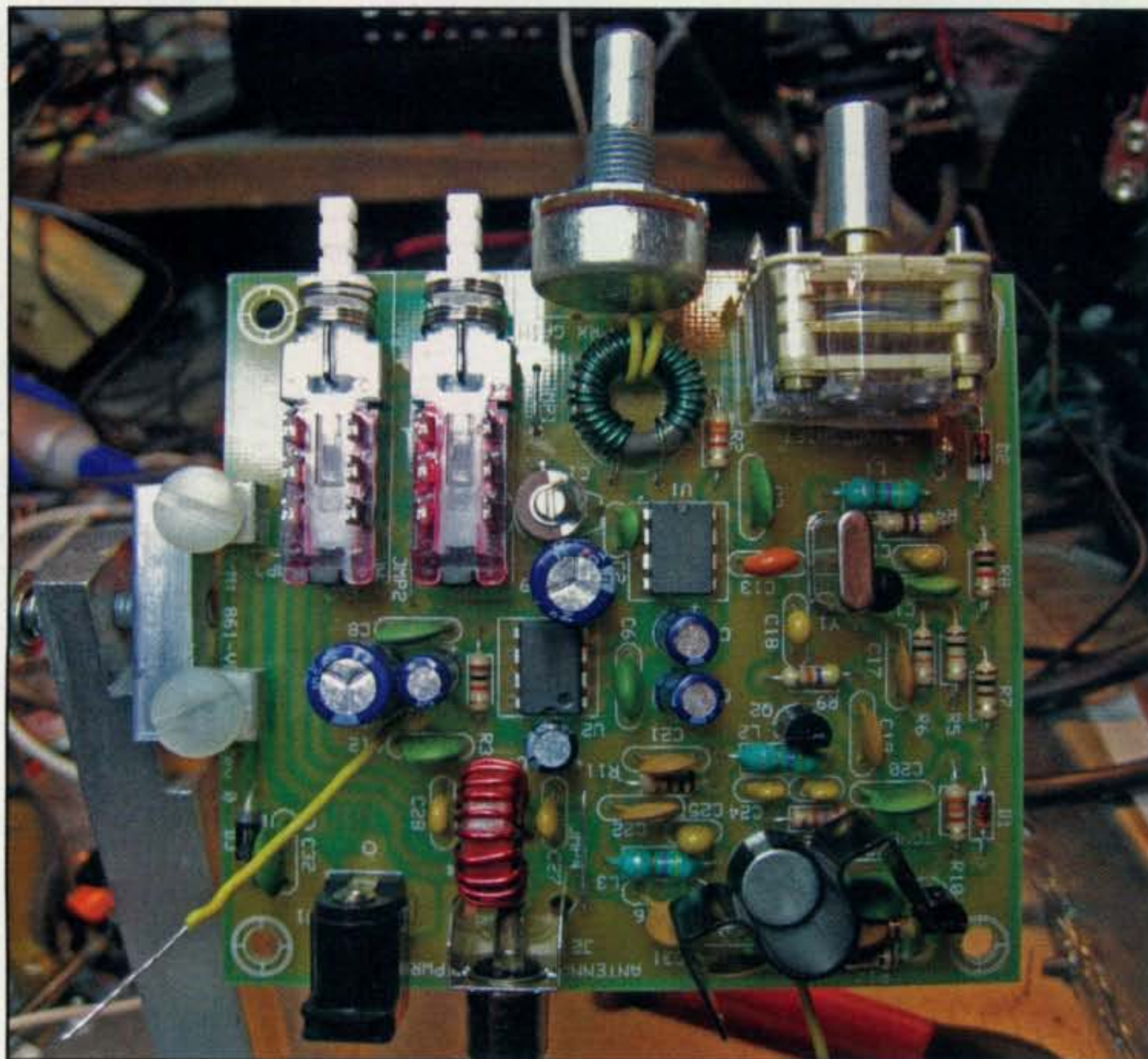
Photo B— Board with all parts mounted and ready for mounting in the case.
