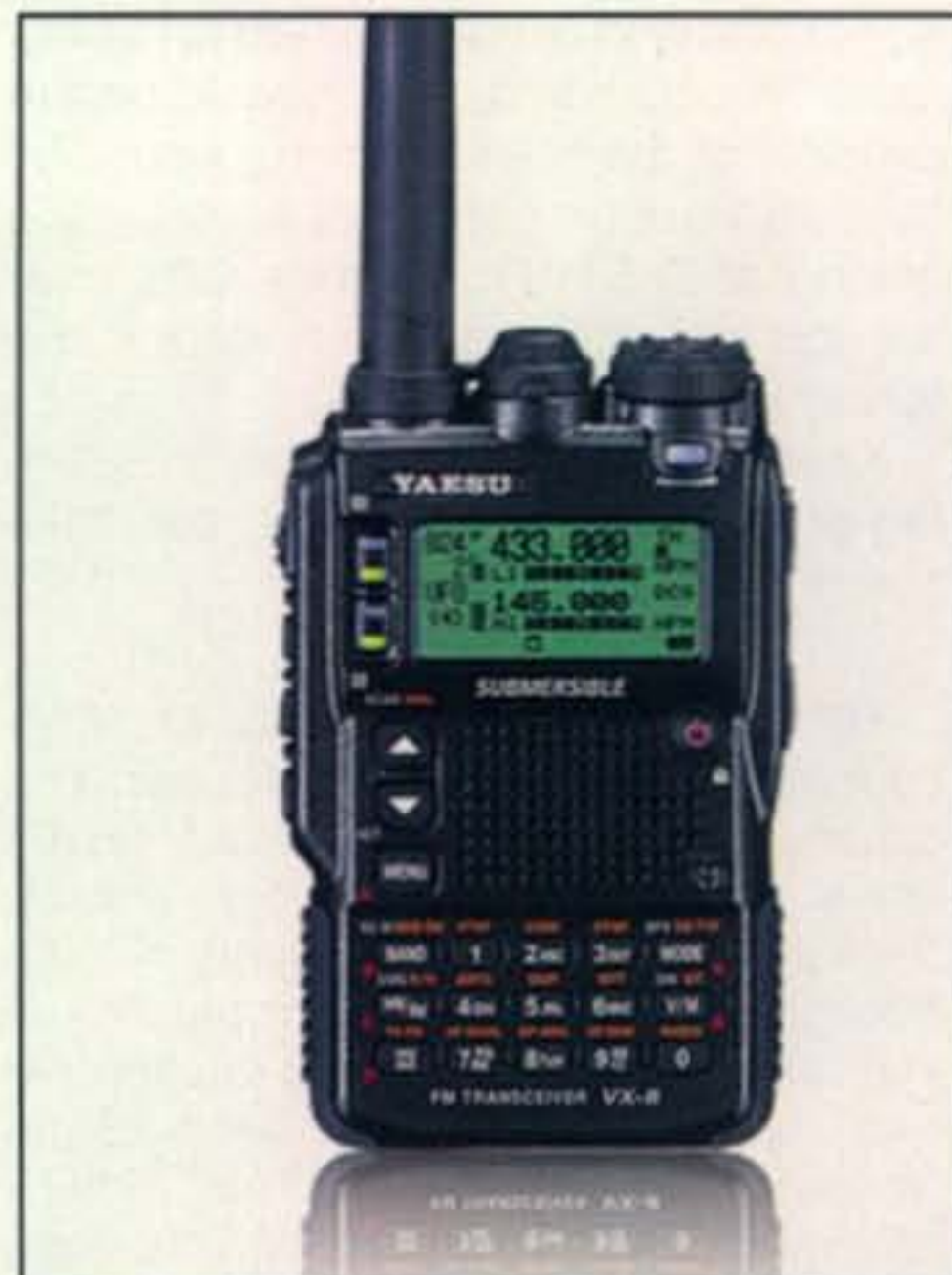
Yaesu has the only quad-band HTs on the market today, the VX-7R and the VX-8DR (pictured). Both cover 6 and 2 meters, plus 222 and 440 MHz. The VX-8DR has a built-in TNC for APRS, and an optional GPS receiver is available.
