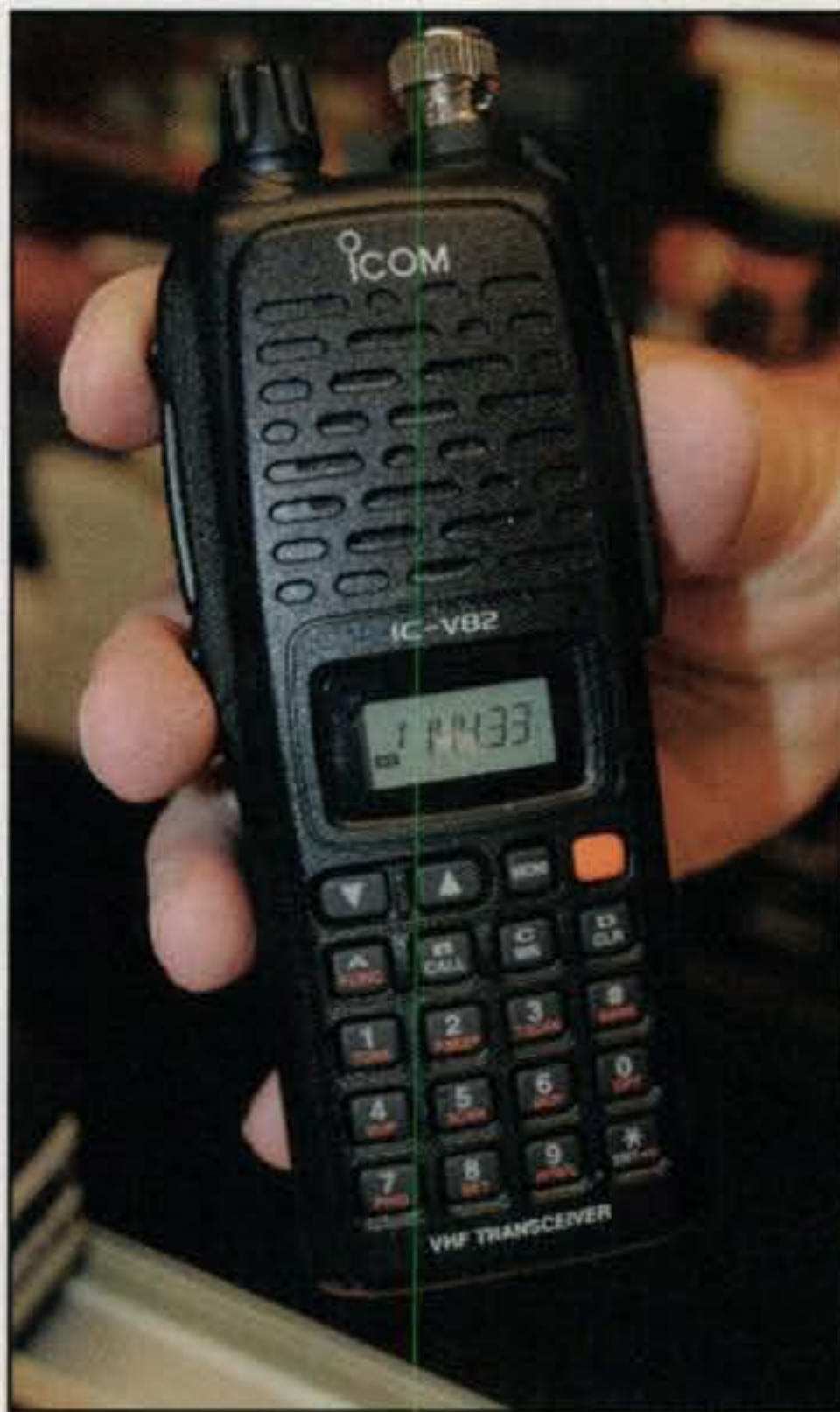
The ICOM IC-V82 continues to be a very popular 2-meter-only handheld with its 7-watt high-power output.
