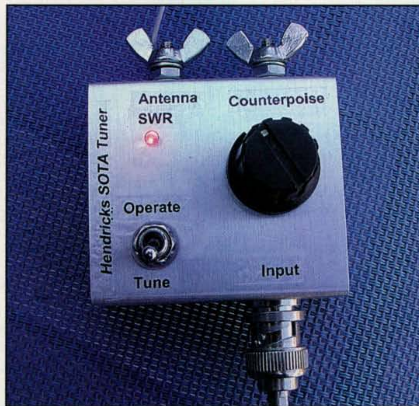
Photo B— Hendricks QRP Kits SOTA tuner, small in size and just over 2.5 ounces.
