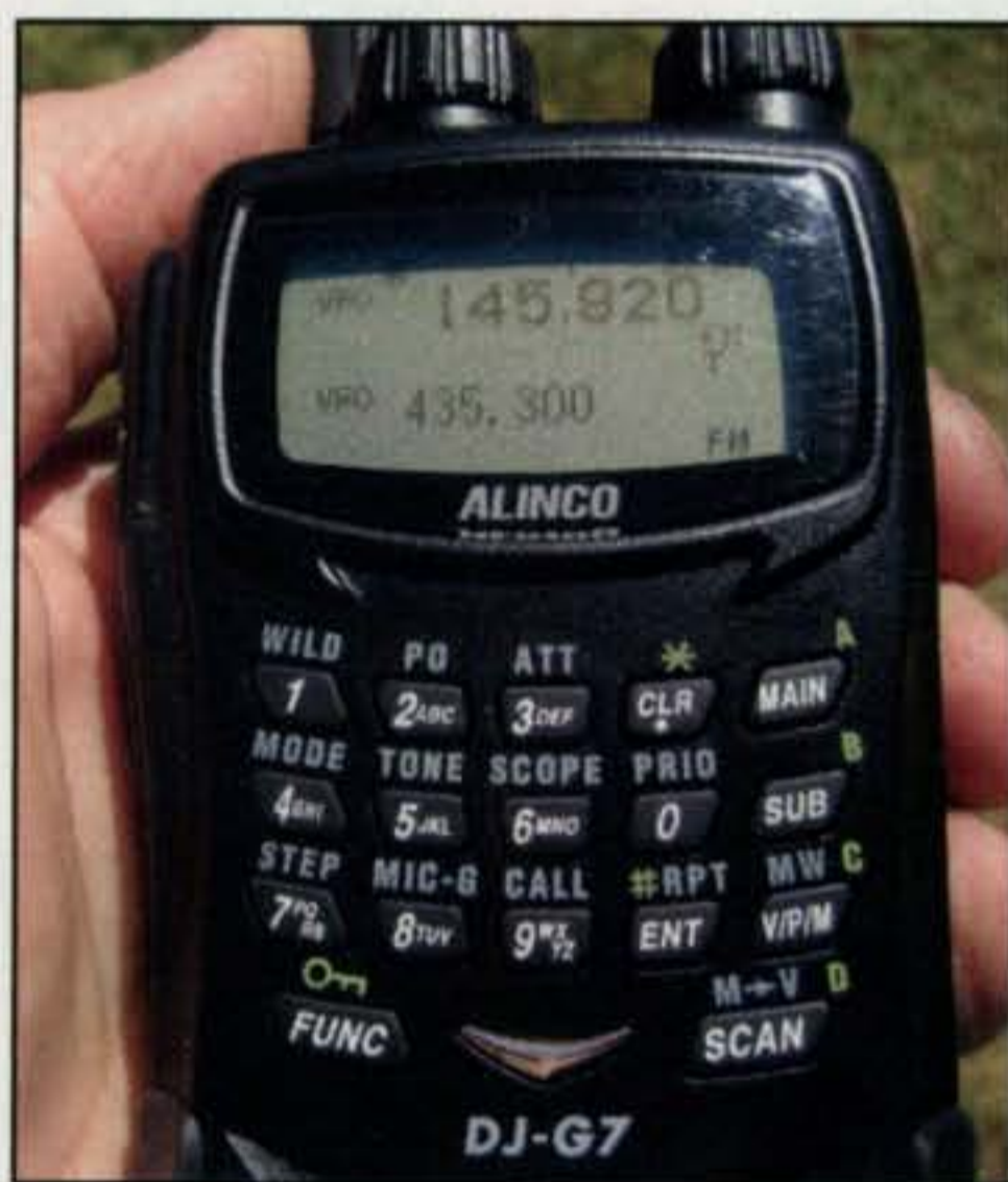
Alinco's DJ-G7T covers 2 meters, 70 centimeters and 23 centimeters (1.2 GHz), plus a wide-band receiver ranging from the AM broadcast band through 1300 MHz (AM/FM only).
