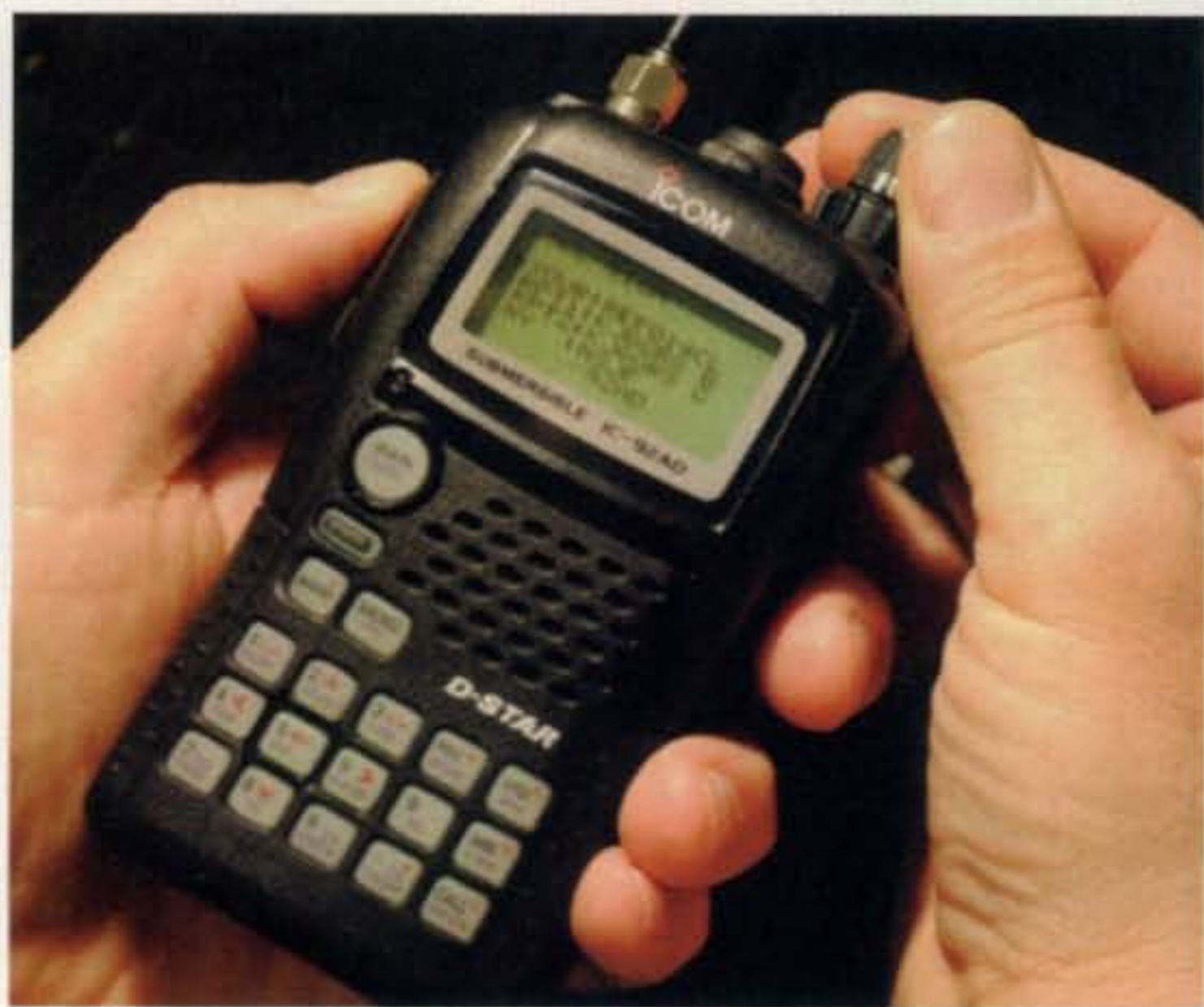
The IC-92AD is ICOM's top-of-the-line dual-band HT, with full-duplex capability for operating FM satellites, and D-STAR capability built in. You can also get an optional GPS microphone.
