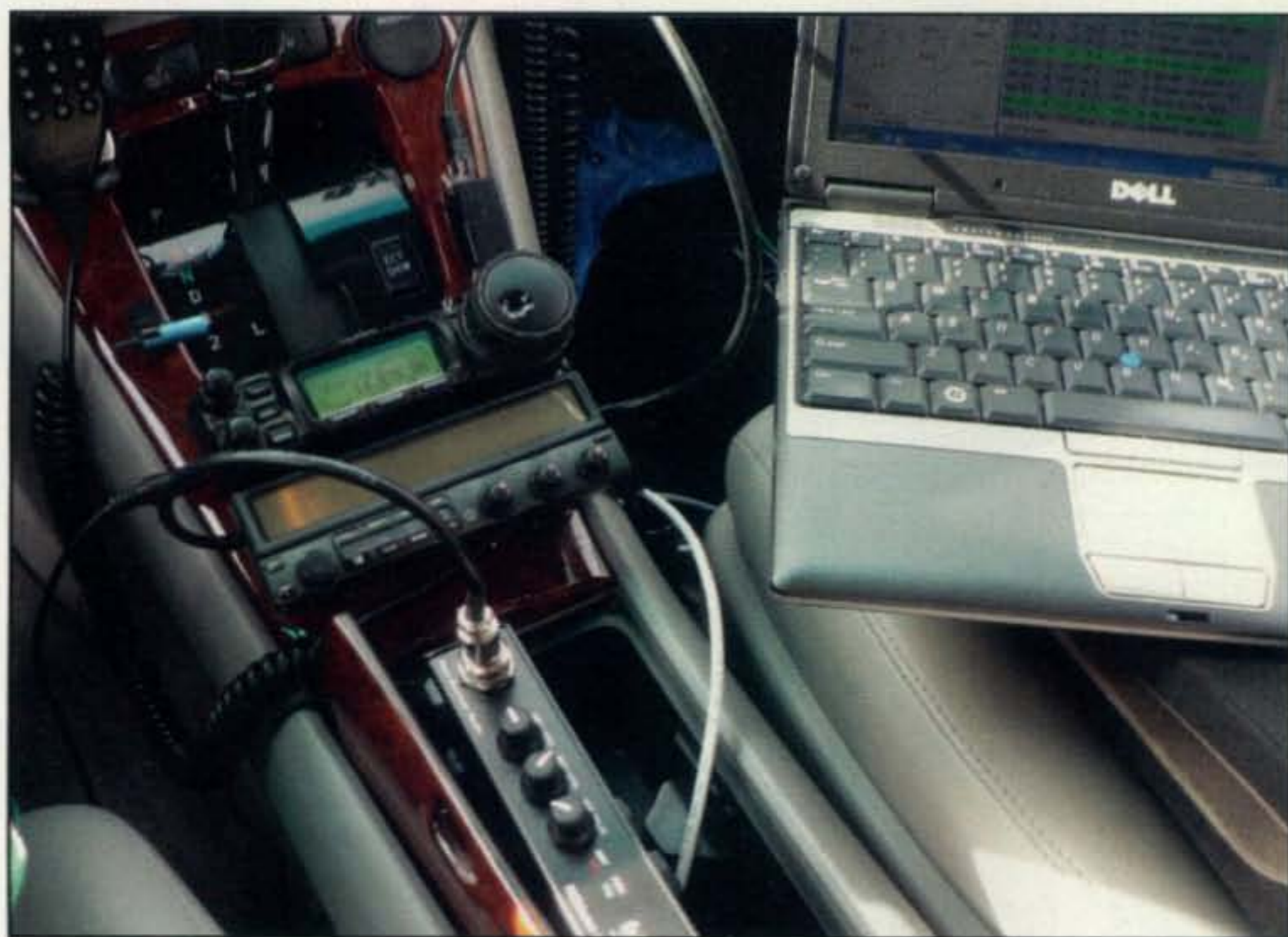
Photo G— The Mobile/Rover station setup used the RIGblaster Advantage and a Yaesu FT-857D for operating PSK-31 from the author's car, overlooking Stanford University.
