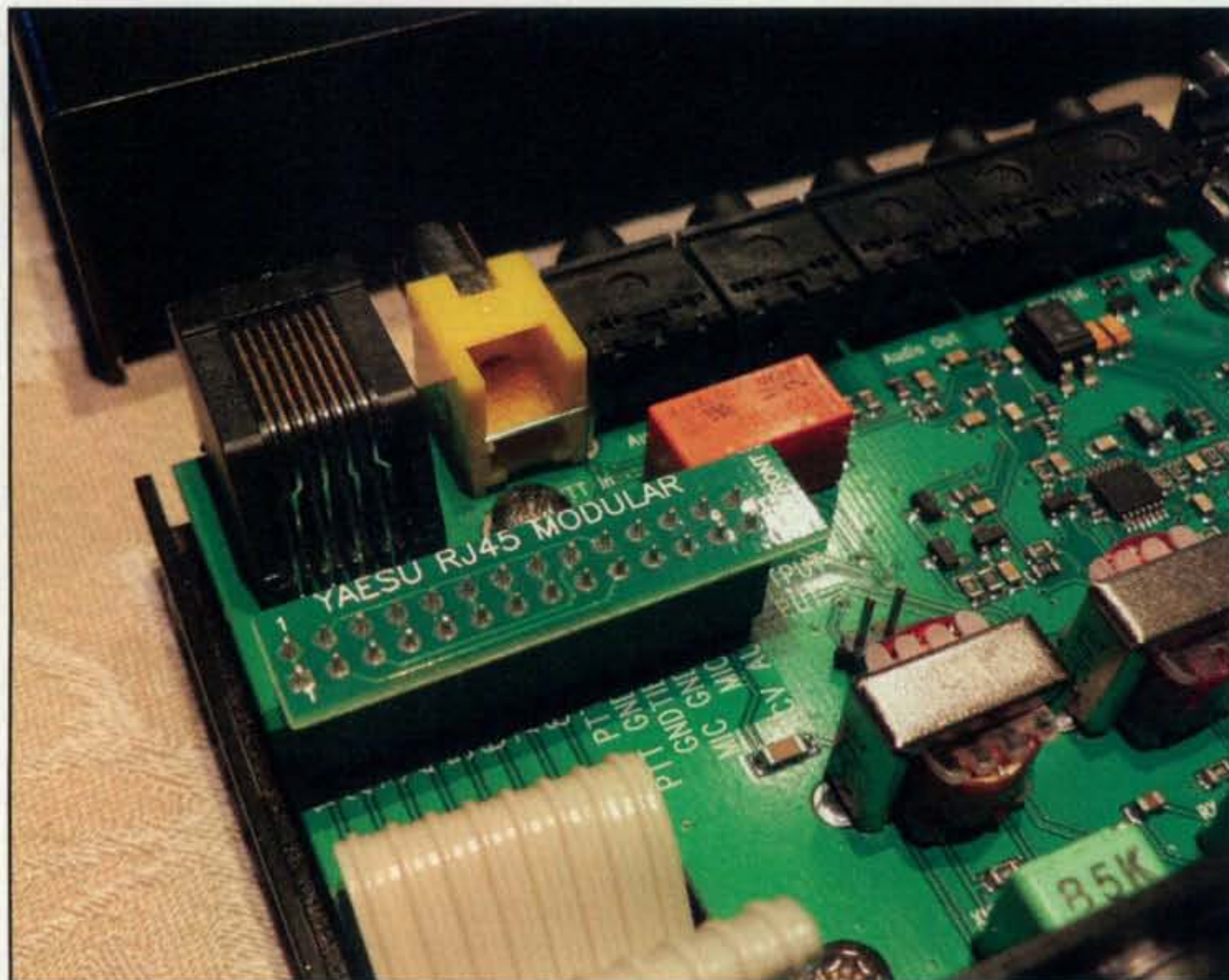
Photo C—Closeup of Instant Setup Connectors, or ISCs, with one installed on the RIGblaster Advantage.
