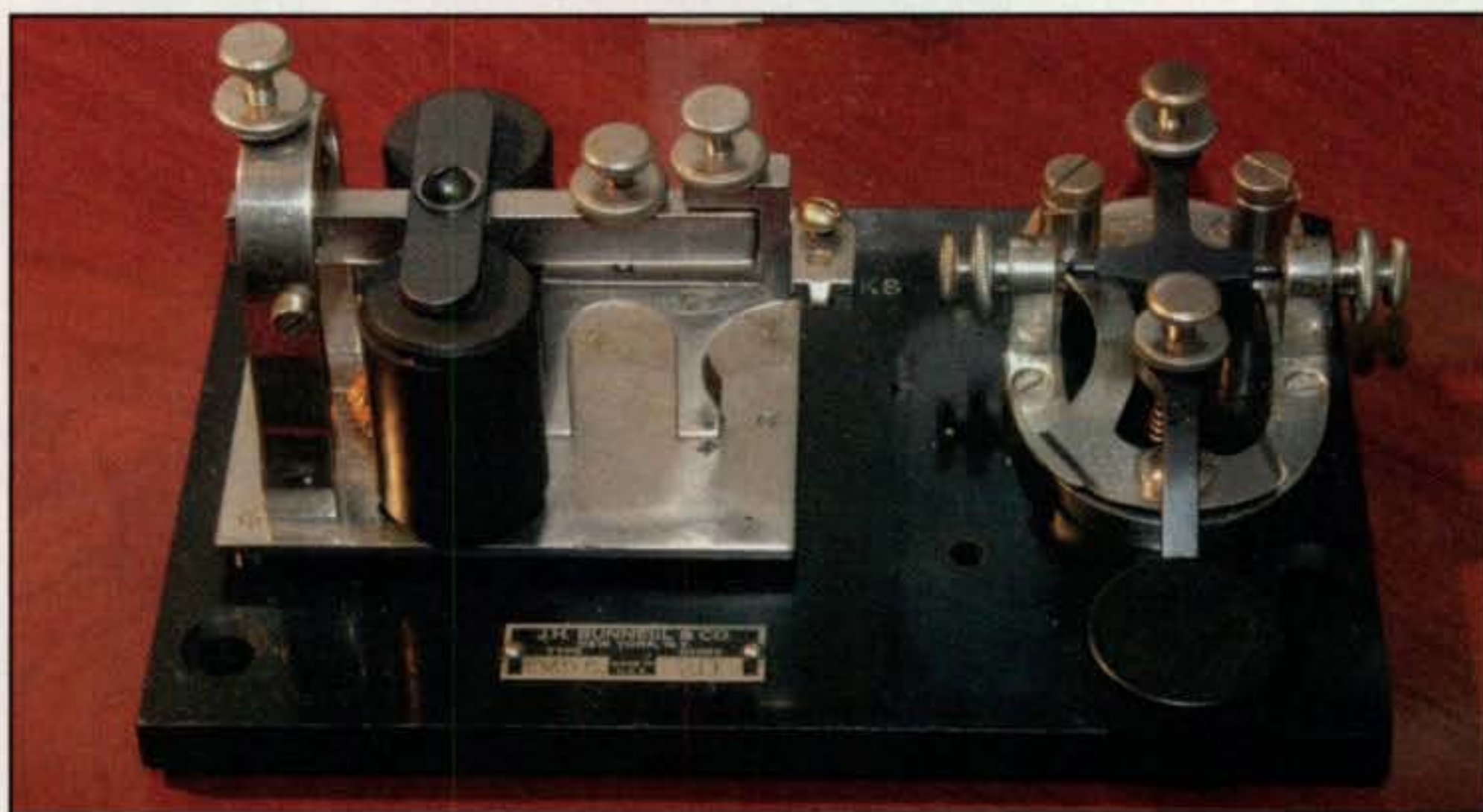
Photo D— Recently I decided I needed a bit of turn-of-the-century nostalgia for the front room (my wife Pat says I can!), so I purchased an antique J.H. Bunnell telegraph sounder with straight key. This device was used in the days of land-line telegraph to transmit Continental Morse code (different from the International Morse we use in ham radio). In place of a tone in a receiver the operator copied “clicks” produced by the sounder. This one works; a 9V transistor radio battery is all that is needed to sample what it must have been like in the “old days.”
