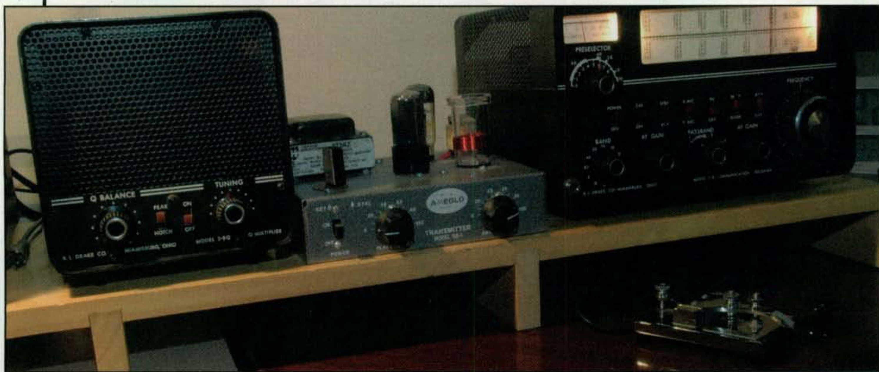
Photo A—The Drake 2B receiver (circa 1960) on the far right hooked to my clone of the Ameco AC-1 two-tube crystal-controlled transmitter (middle) was my first choice to operate on SKN 2012. The Drake 2B-Q-speaker/Q-multiplier is the black box on the extreme left of the picture. However, plans changed and I ended up using the gear seen in photo B.
