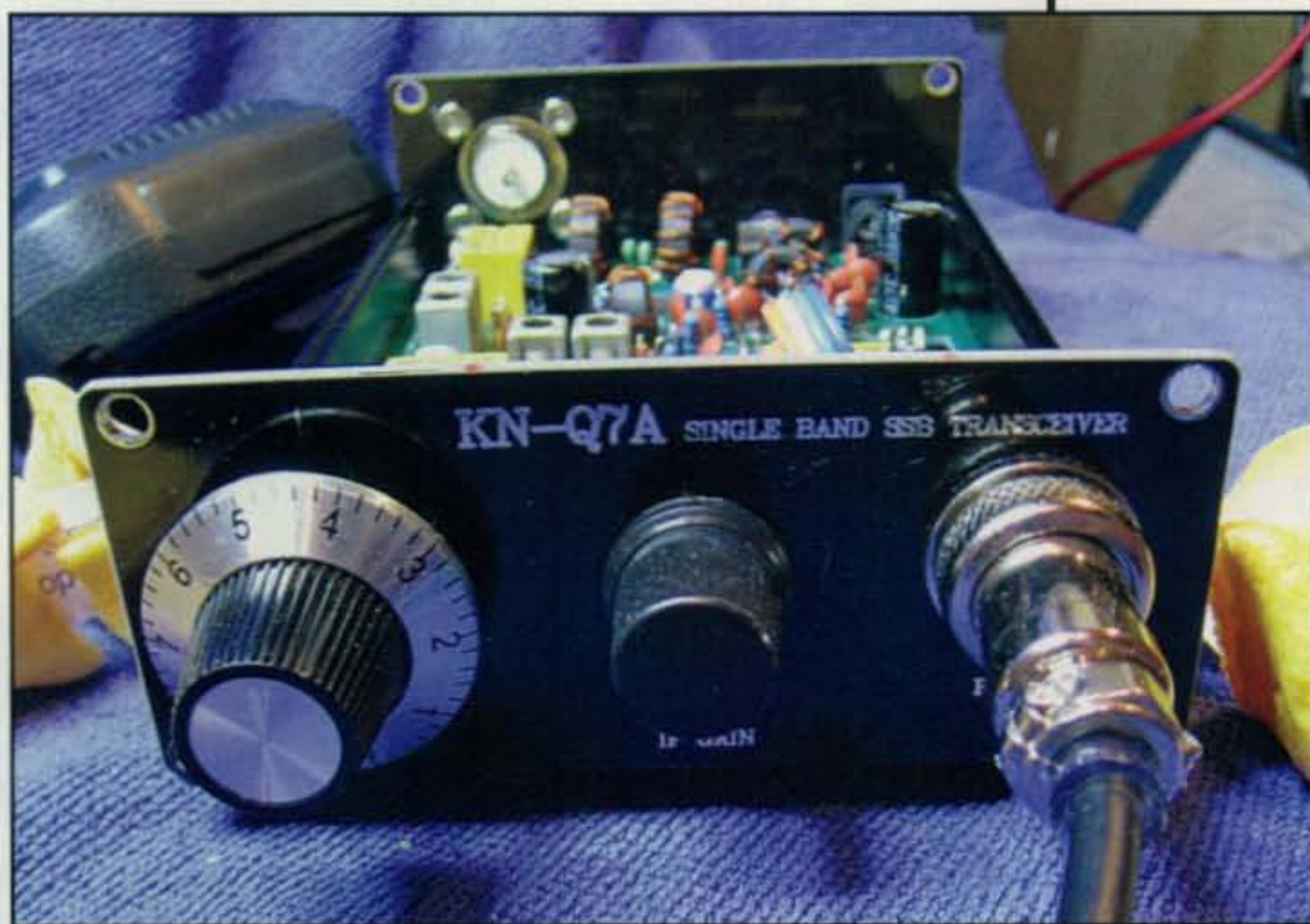
Photo A— The KN-Q7A 40-meter transceiver kit from CRKits.com in China may be ordered directly or from a U.S. distributor.
