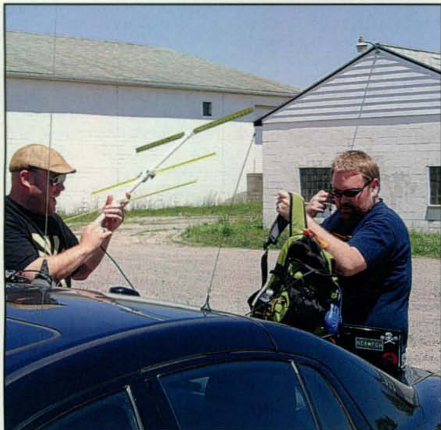
Photo D— Tracking the A1 balloon launch with our homebrew 2-meter tape-measure antenna.
