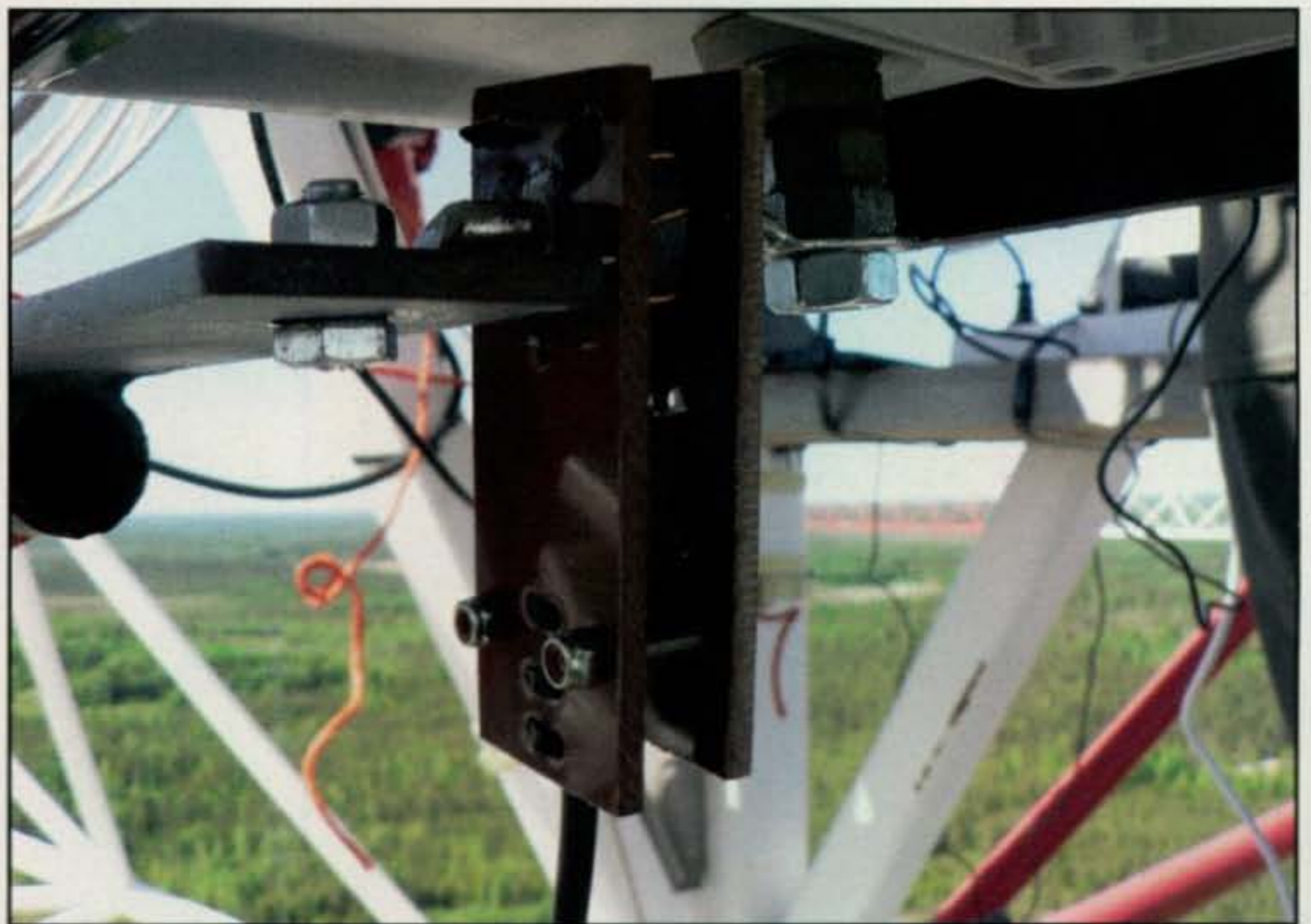
Photo F— For actual measurements we needed a two-port VNA. One port was feeding the antenna just like a transmitter would normally do. To the other port we'd connect a current transformer (shown in photo) and that transformer would be connected to the element we were measuring. The first measurement would be for feed element in order to get reference of phase and current. After this we'd measure all the other elements, normalize those values to driven element values, and compare normalized results with simulated ones. Measuring the antennas this way seems to be quite novel.
