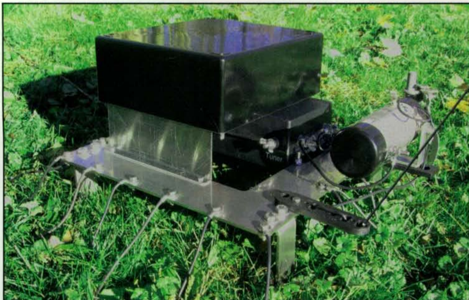
Photo B— The key to the effectiveness of DX Engineering's low-profile remote tuning unit is that it can easily be hidden in bushes with only a 26-foot piece of wire that extends vertically and is practically invisible but allows you to operate on the 40-meter band and up.
