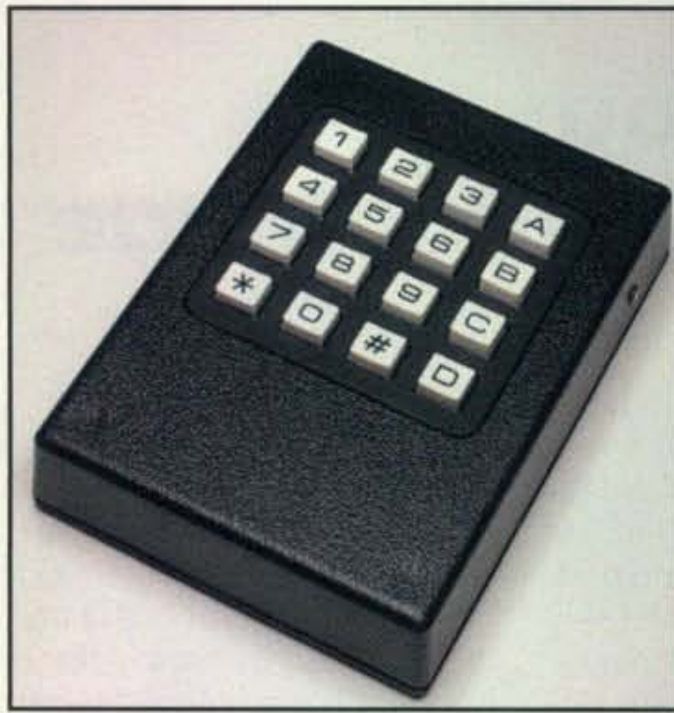
Photo D – The QSYer by W2FS allows direct frequency entry on many rigs that do not offer this as a standard feature.
