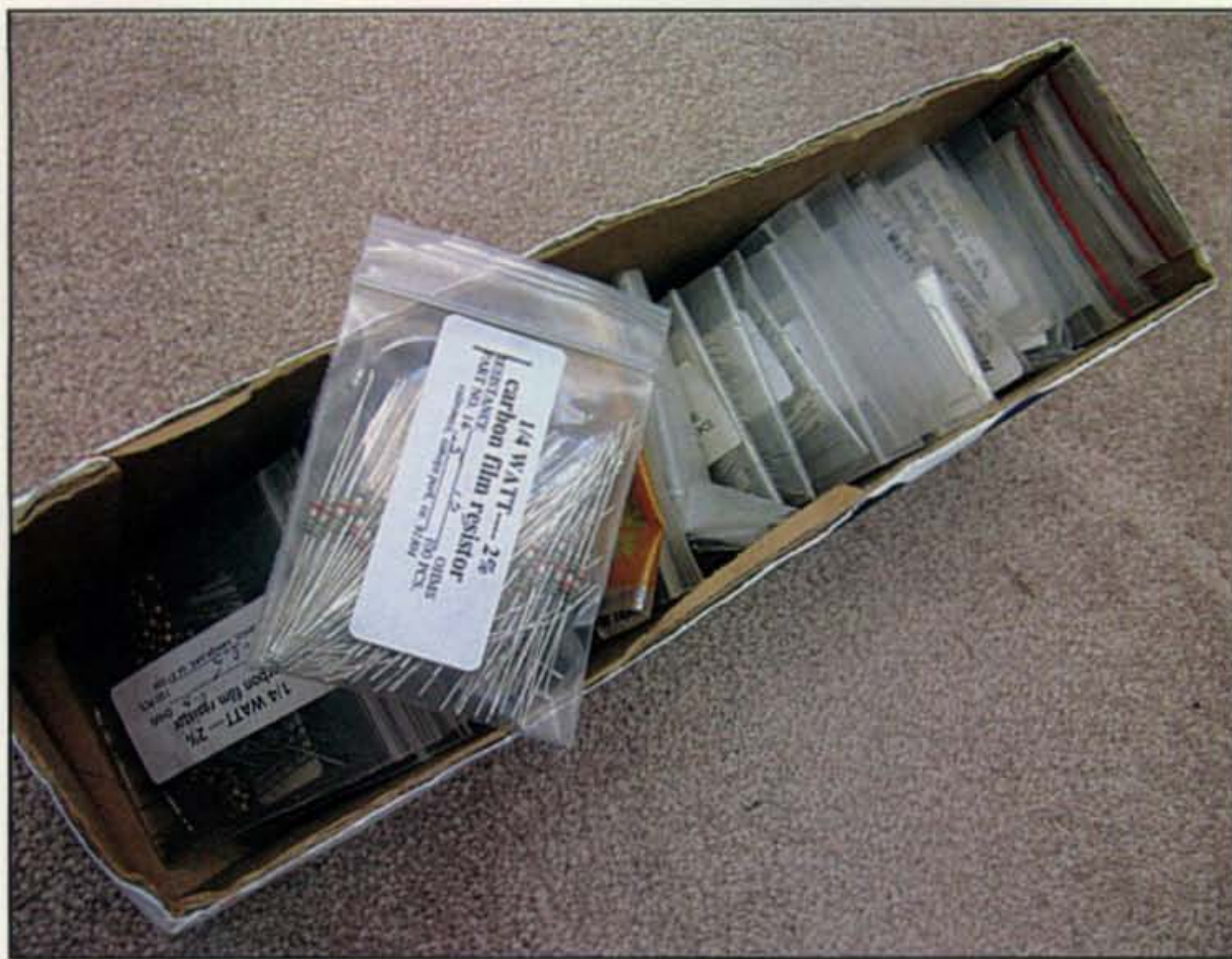
Photo 2— Sorting by a component's first significant digit is a good way of storing, sorting, and selling multiple values of similar items. Here is box "5" of one-quarter-watt resistors. Values go from one-half ohm to 5.6 megohms.
