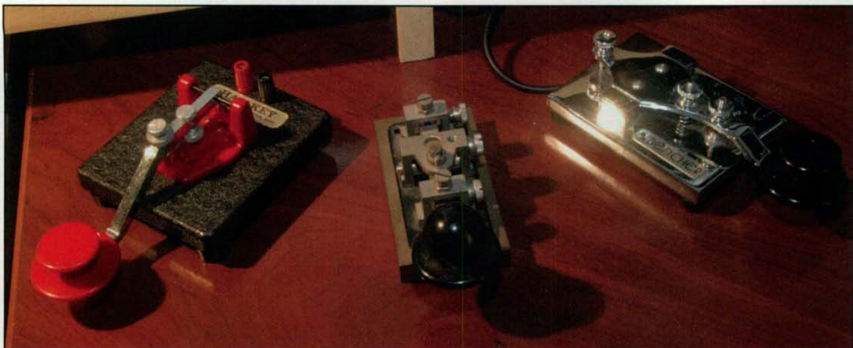
Photo C— I don't collect keys or paddle sets. . . . Well, OK, maybe I have a small collection! Shown here are my three straight keys left to right: HamKey HK-3, WW II British key, and the Bencher RJ-2. All perform well and are a blast to use.
