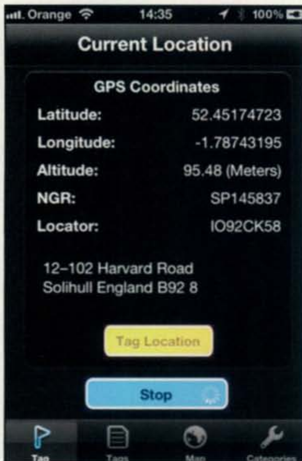
Photo E— MtagIt is the name of a new ham app for your iPhone. It calculates your grid square and enables you to tag the location with your own definable category.
