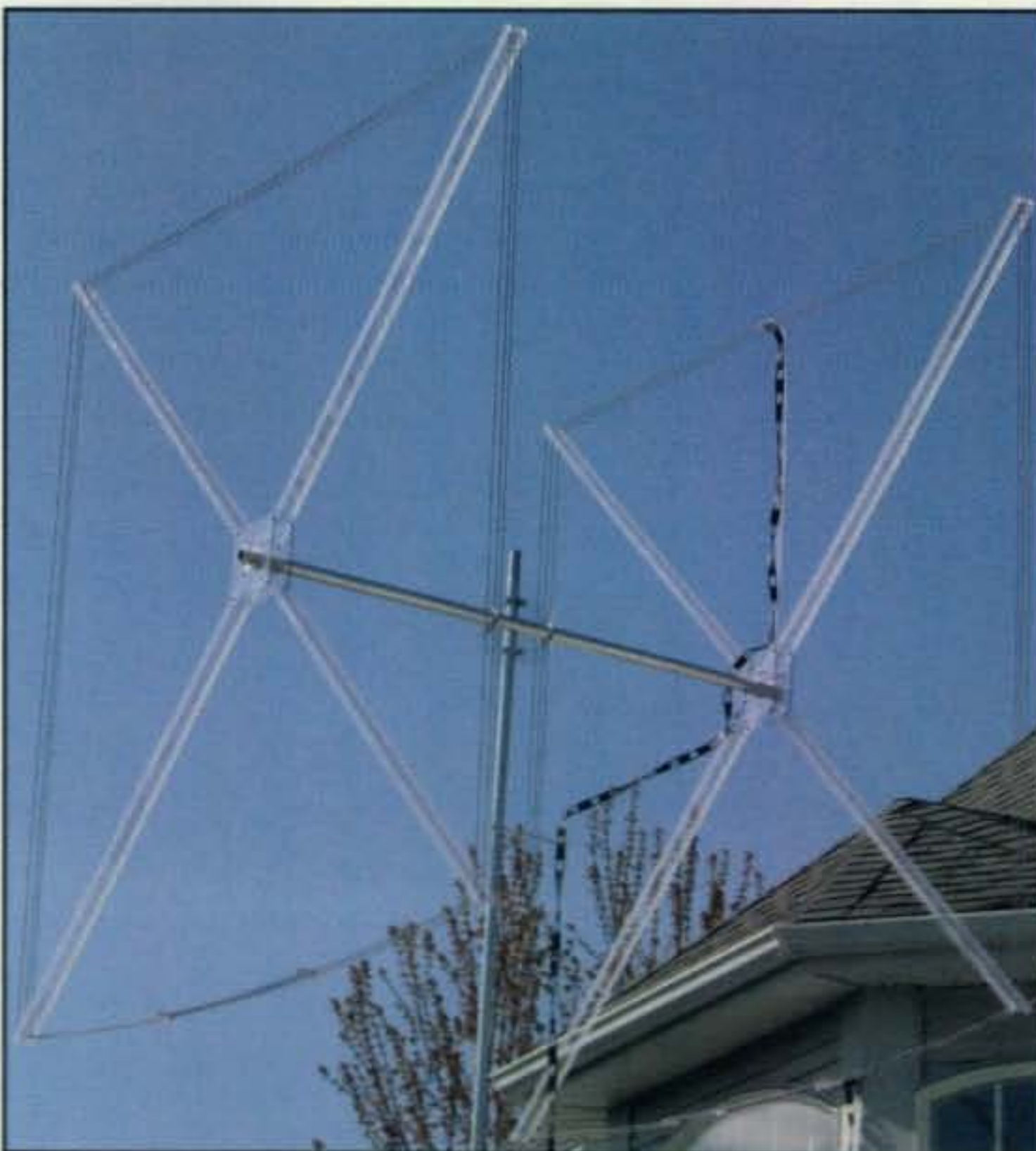
Photo A – Light Beam Antenna is particularly proud of its Light Beam and Light Beam Plus designs which can operate on 20, 17, 15, 12, and 10 meters at a height of 30 feet while still providing a low surface area.
