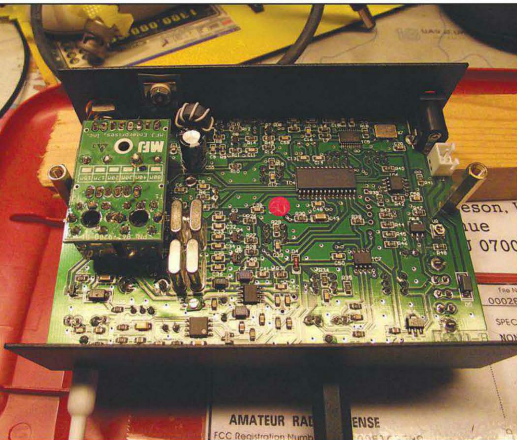
Photo D— Interior of the 9200. The removable band module is on the left.
