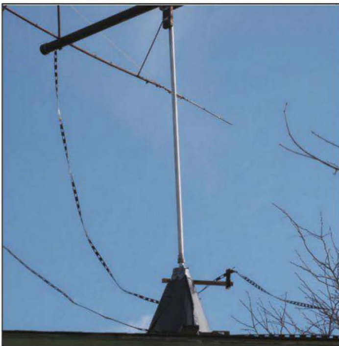
Photo C— Ladder line and mast configuration.
