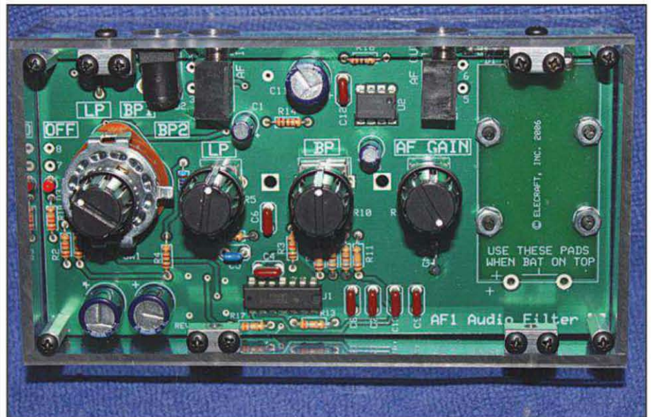
Finished Elecraft AF-1 audio filter kit enclosed in the W8FGU clear Lexan case. See text for details.
