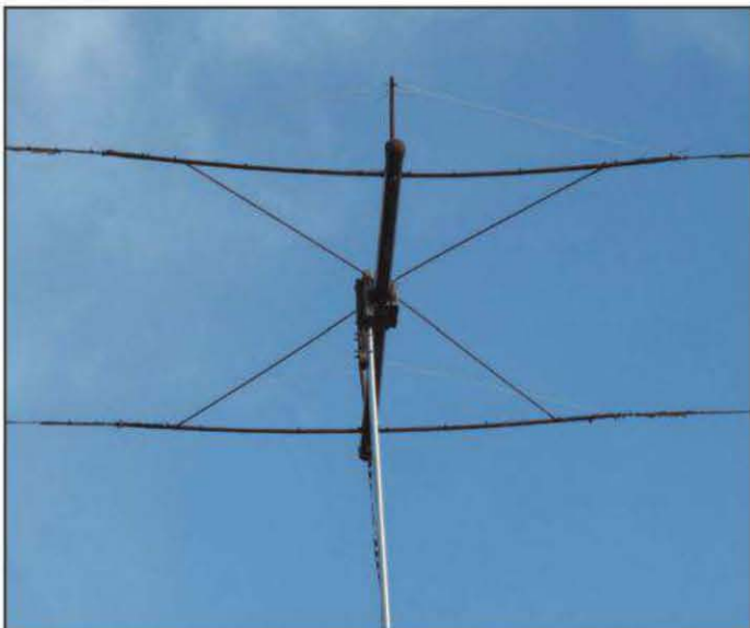
Photo B— PVC beam at 34 feet.
