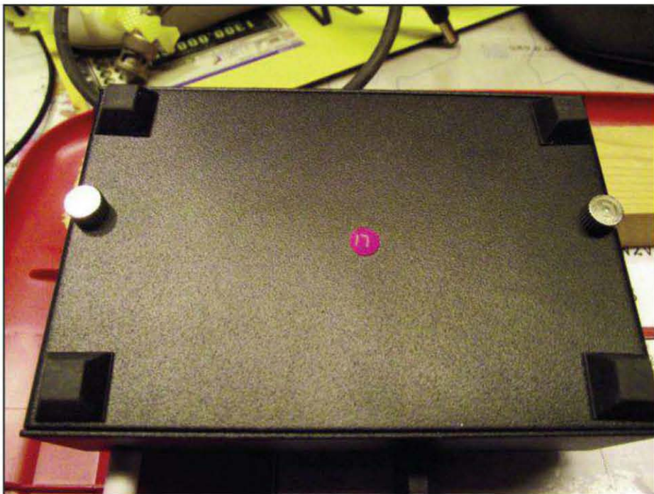
Photo C. The thumb-screws on the bottom of the rig need to be removed in order to change band modules. Don't lose 'em!
