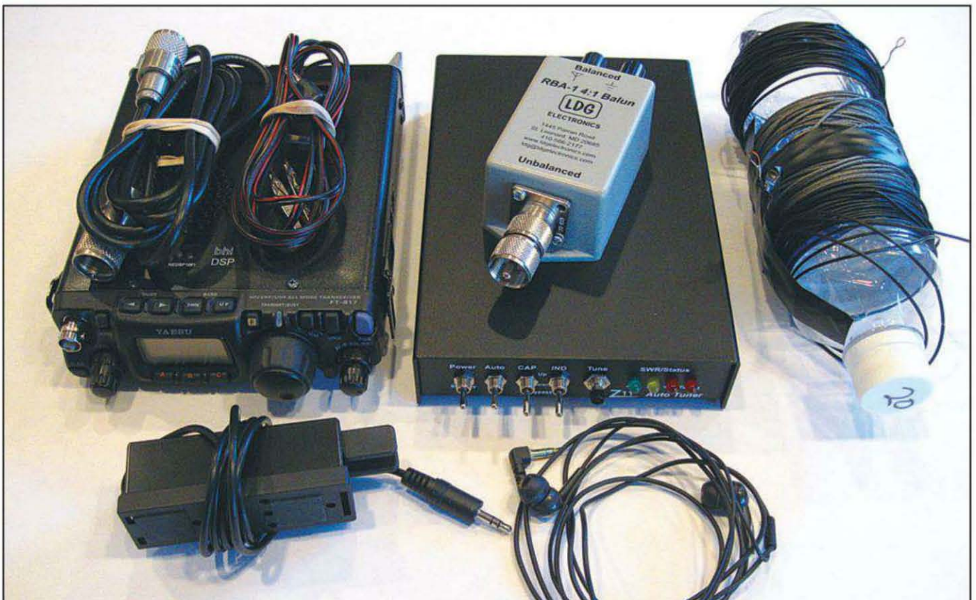
Photo B— Equipment on our first trip included my FT-817 and LDG autotuner, but they turned out to need a lot of power from my gel-cell battery. I made no contacts on this trip.
