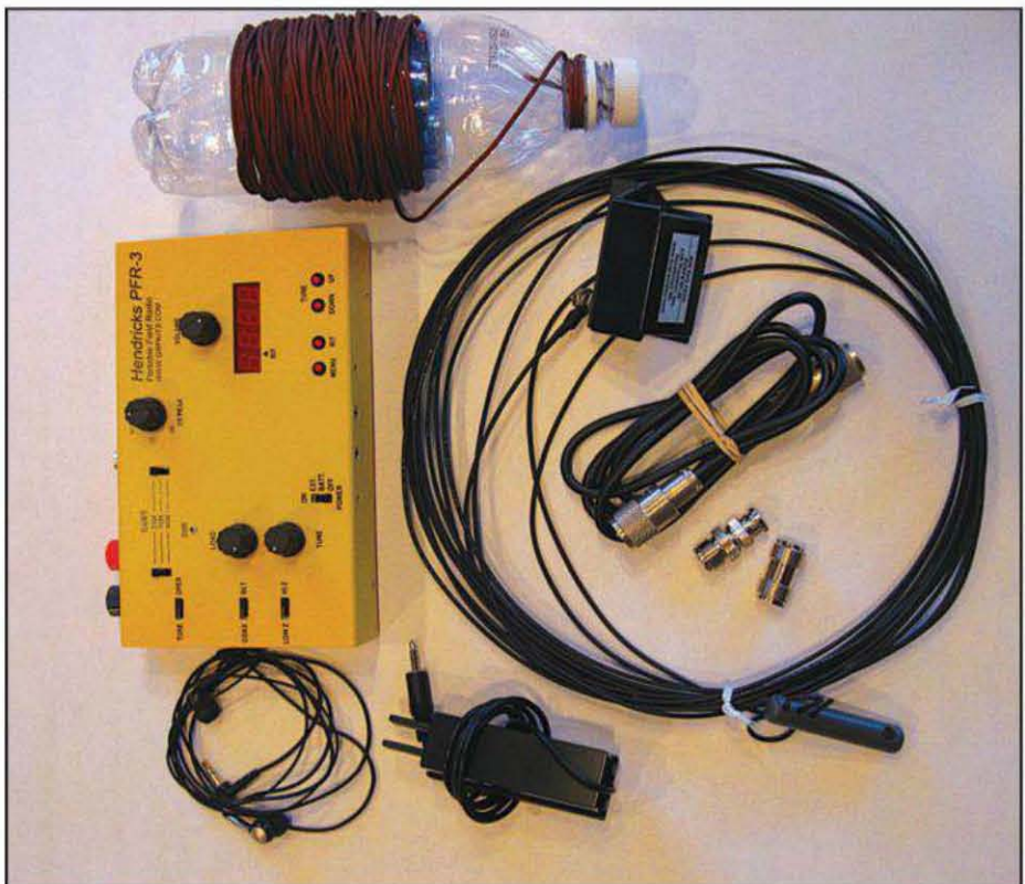
Photo D— On the second trip, my station was built around my Hendricks PFR-3 transceiver with built-in manual tuner. It used much less power and got me two QSOs.
