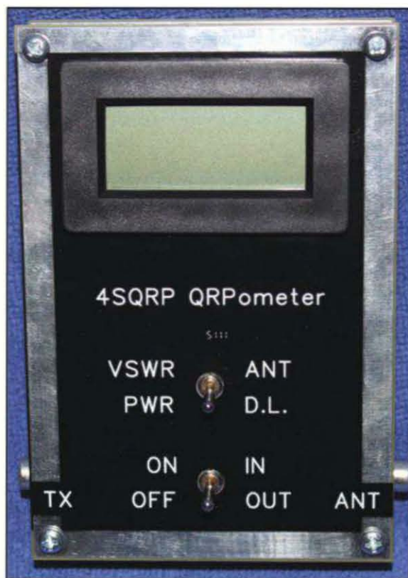
Four States QRP Group (4SQR) QRPometer assembled and ready to go. (All photos by KØNEB)
