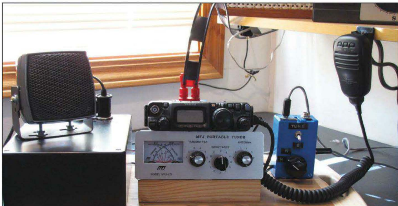
Photo A— QRP station mounted on a wooden cutting board. This arrangement makes it easy to operate it from home or just pick it up and take it to a remote location.
