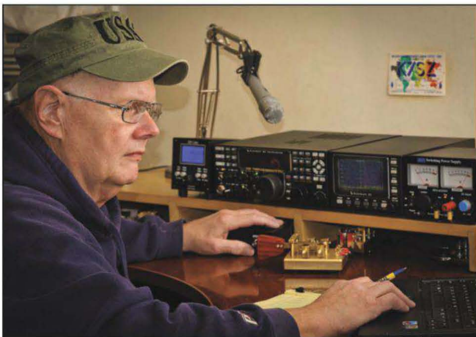
Here I am at the controls of K7SZ at the Bent Dipole Ranch in beautiful downtown Dacula, Georgia. In the background, left to right: SDR Cube transceiver kit, Elecraft K3 transceiver kit, Elecraft P3 panoramic adapter kit, and a finally a MFJ switching power supply. (Photo by Mike Boatright, KO4WX)
