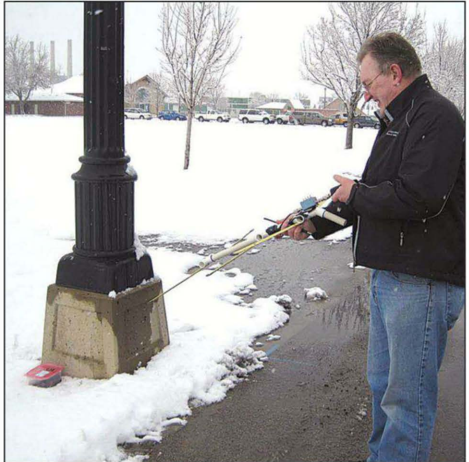
If you're going to put on a foxhunt in Salt Lake City during February, you may encounter some fresh snow. Hider Larry Jacobs, WA7ZBO, put his five little transmitters in plastic tubs to keep them dry. John Hardy, K7ALA, is hunting with a measuring-tape Yagi, resistive attenuator, and handheld. This hunt was part of the 2011 annual Utah VHF Society Meeting. (Photo by Larry Jacobs, WA7ZBO)
