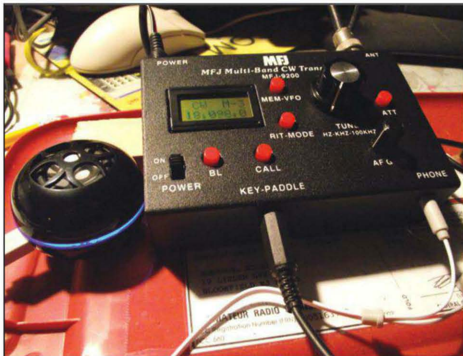
Photo H— The "Tiny Tweakers" amplified speaker that I picked up at a local office supply store (left) provides enough volume to let me operate without using headphones.
