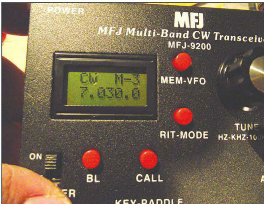
Photo G— The LCD display provides you with a wide array of information. In this photo, it tells you that you're in CW receive mode, on memory channel 3, which is 7030.0 kHz.
