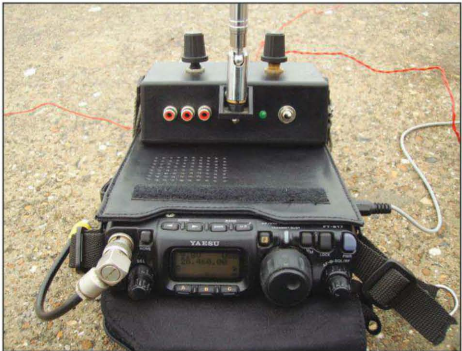
Photo B— Andy, GØFTD's, FT-817 with tuner/pre amp/dummy load/antenna mount attached.
