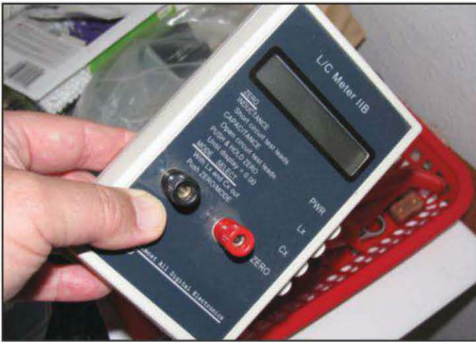
Photo 4— A capacitor and inductor tester, such as this item available in kit form, should be in your collection if you build and test your own gear.
