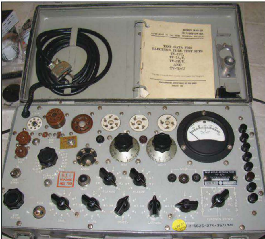
Photo 3— A US Army TV-7/U tube tester, purchased on eBay, is a great tool for testing old tubes.
