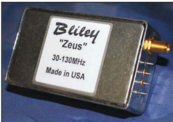
Photo A— Bliley has reason to be proud of its newest product, the Zeus Series OCVZXO oscillators which can perform as phase-locked microwave signal sources in applications such as DROs, low-noise test equipment, synthesizers, microwave communication systems, and radar applications.
