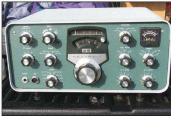
Photo 1— Classic tube gear from the 1970s and earlier is still alive and well in many ham shacks today. Here is a very clean Heathkit SB-100 transceiver recently seen at a local swap meet.
