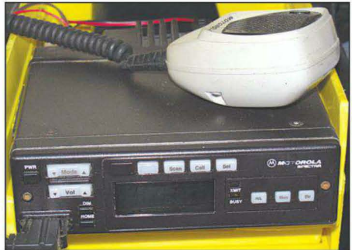
Photo 5— The Motorola Spectra is one example of a great commercial radio unit that can be easily reprogrammed for the 902–928 MHz ham band.
