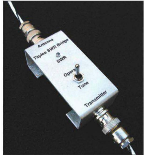
Photo A– Front view of Hendricks Kits QRP SWR kit (photo courtesy of KI6DS)
