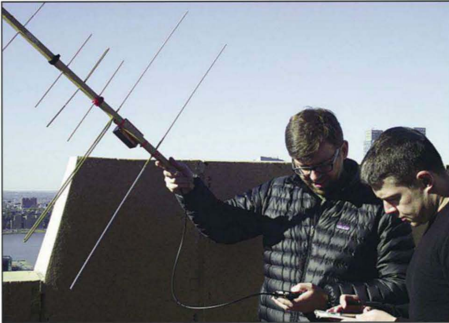
A handheld radio and a handheld beam antenna are all you need to work some FM satellites. This antenna is a homebrew "Cheap Yagi" designed by CQ Antennas Editor Kent Britain, WA5VJB. Here Dave Clausen, W2VV, and Bill Ward, KD4ISF, try to work SO-50 from a hotel balcony in New York City. Note the angle of the antenna, as described in the text. (W2VU photo)
