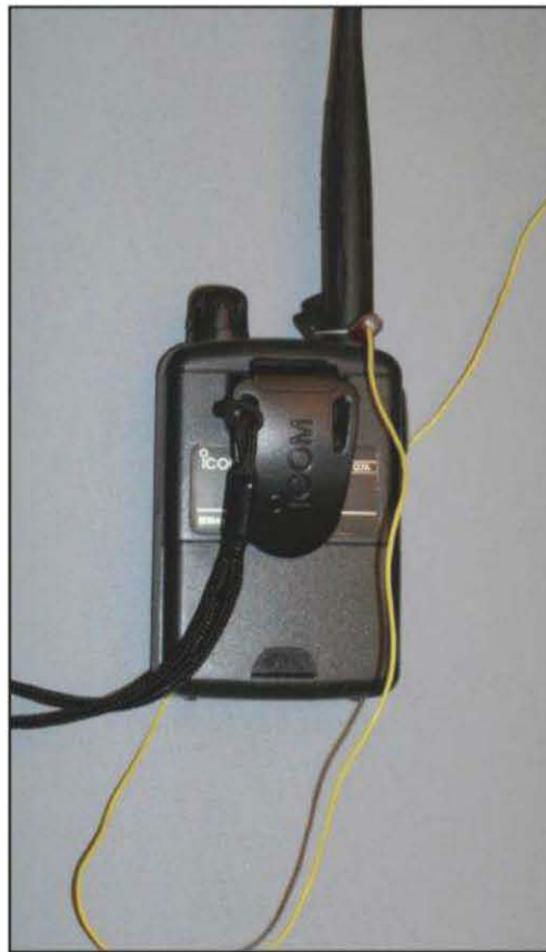
Photo D— Ground radial or counterpoise for small transmitters.
