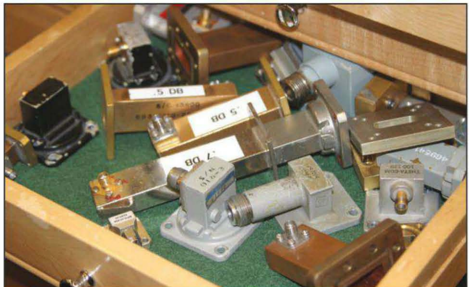
Photo 6— One of the best places to find various microwave cables, connectors, and waveguides is the surplus market. These very-low-loss components are must-have pieces to complete a high-performance microwave system.
