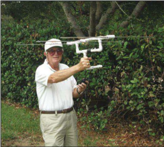
Ted Luebbers, K1AYZ, added some PVC pipe to his 2-meter measuring-tape Yagi to give it a nice handle that balances the antenna and keeps his hand from affecting the directional pattern. He used it on the first Foxhunting Weekend event of the Royal Harbor Amateur Radio Club in Tavares, Florida. (Photo courtesy K1AYZ)
