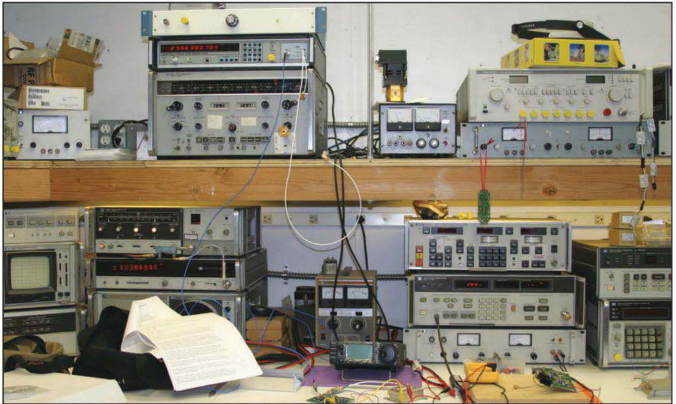
Photo 9— Specialized RF test instruments are a great value and can be found as surplus in many cities, as well as on eBay. Most of the test gear shown here is rated for the UHF and into the microwave frequency region.
