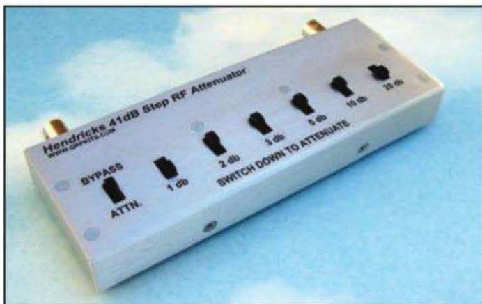
Photo C—Hendricks 41dB attenuator kit. The kit comes with case and BNC connectors. (Photo courtesy of KI6DS)
